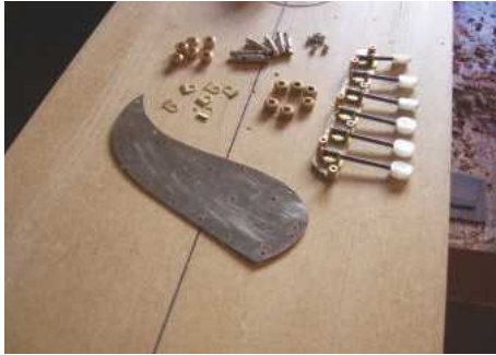
23 The disassembled Staufe-Mechanik
