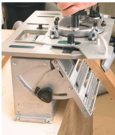
16 The mortise & tenon jig is designed for a variable clamping angle when cutting the tenon
