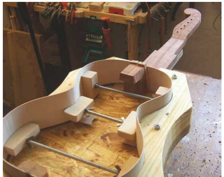
32 A dry fit of the heel-to-rib wedges
