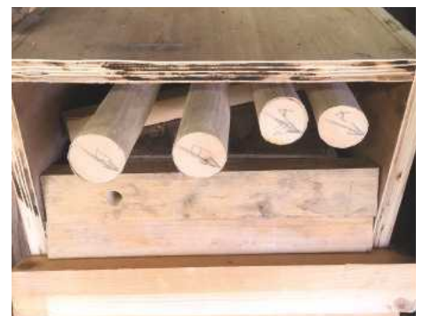
Two pairs of chair legs in the steam box, ready for steam-bending
