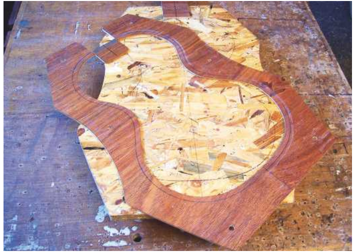
12 The mould 'well' prevents damage to the soundboard
