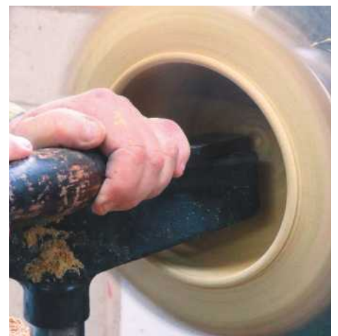
21 Light cuts using a round-nosed scraper will clean up the inside of the bowl
