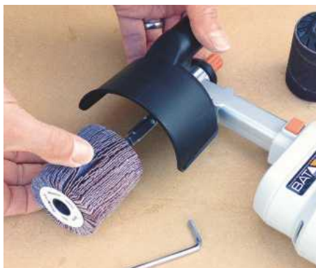
A cast alloy arm protruding from the front end of the body houses the drive for the steel shaft, over which the wheel is fitted
