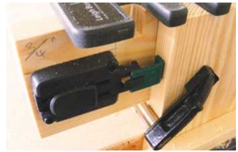
The stop is moved to the pin position in order to cut the matching joint
