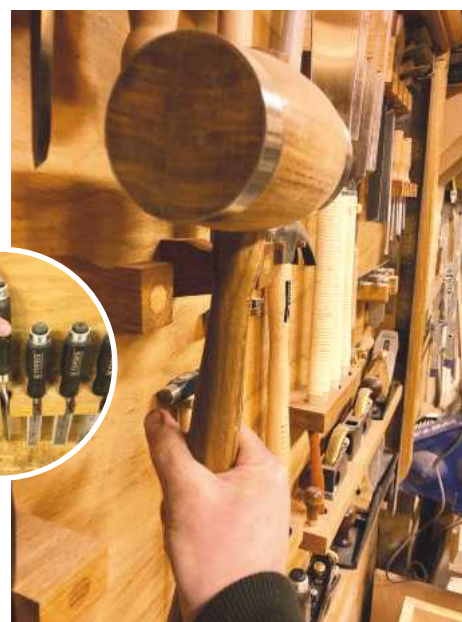
3 A handmade oak dead blow mallet being placed on its custom holder
