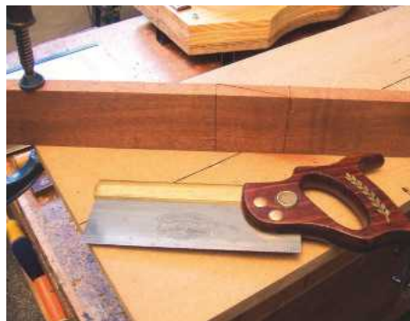
14 A scarf joint is cut into the sipo mahogany to form the headstock joint
