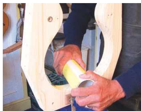
9 The inside edge of the mould should be flat and smooth
