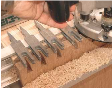
5 Copying a traditional furniture making technique, variable position jigs allow the spacing of sockets to be made closer towards the edges of a wide joint
