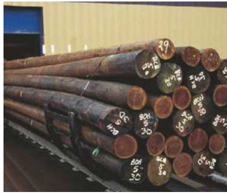
Telegraph poles after treatment in a pressure vessel
