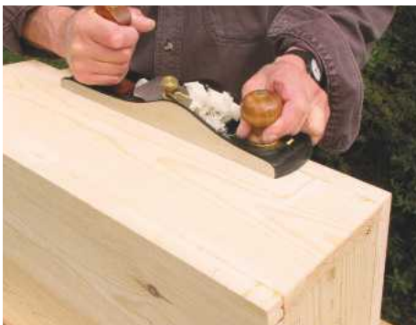
11 When the glue has dried, plane the edges flush on the sides and around the base
