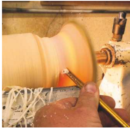
20 The colours showing through the walls of the bowl let me know how thin I'm getting. I will keep stopping to check with my fingers, being careful not to touch the hot bulb with my hand
