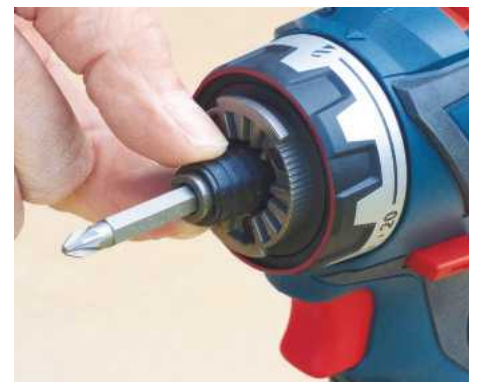
At the end of the motor shaft is a spring-loaded, 1/4in hex socket, enabling bits to be directly inserted
