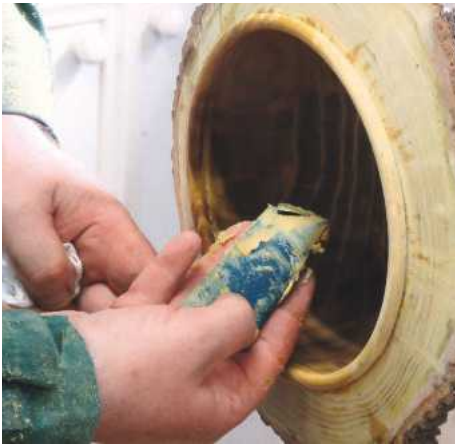
22 Wet sanding creates a slurry rather than dust
