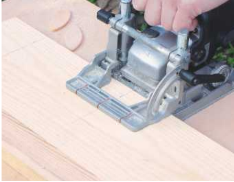
2 If using softwood, front and rear panels will need jointing. Reinforce edge joints with biscuits
