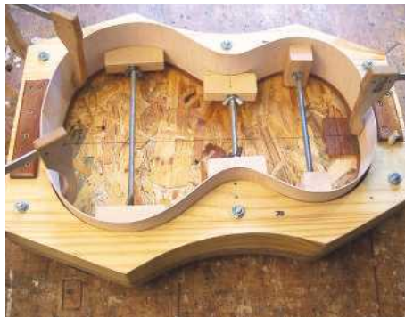
26 The ribs held inside the mould
