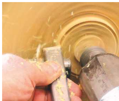
6 Tidy up the chucking spigot with a skew chisel
