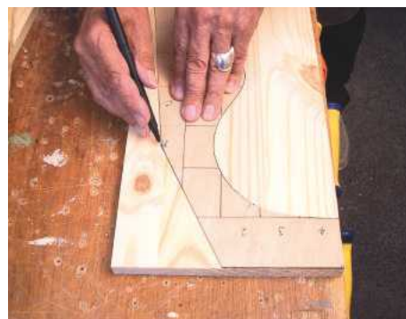
6 The body shape is transferred onto boards to make the mould
