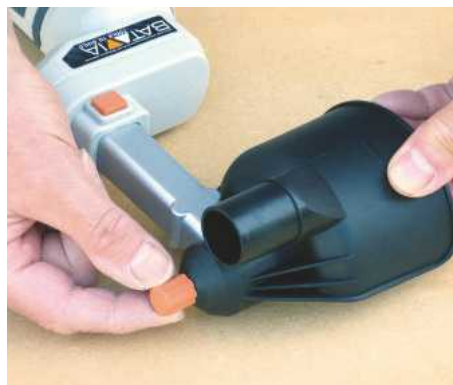
A semi-circular plastic guard gives some protection from the rotating abrasive and is secured at the rear of the arm with a screw
