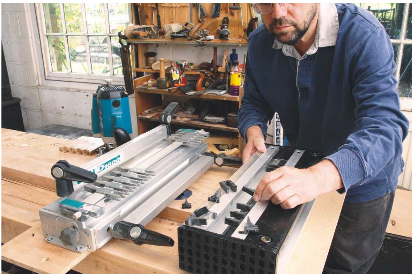
1 Setting up a couple of dovetailing jigs: one with infinitely adjustable spacing (left) and one with fixed spacing (right)
