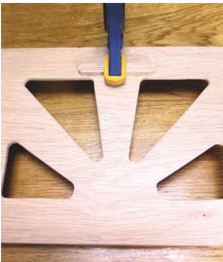
6 Small oak block glued to rear of front support
