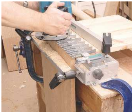
8 Cutting sockets requires the board to be clamped vertically in the jig so the length of board is limited by the bench height
