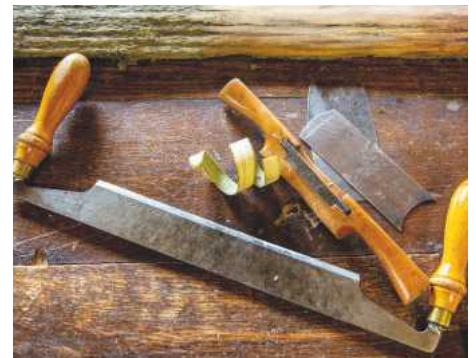
Old oak fence posts look as though they're rotten, but the drawblade reveals what Lynne calls 'brown marble'. Spokeshaves and scrapers are used to shape and finish
