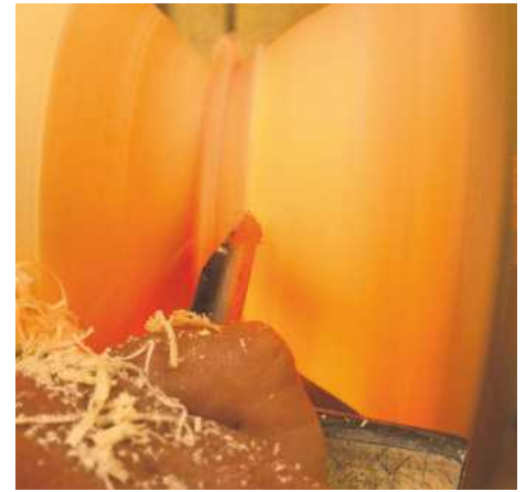
21 I am aiming for a nice consistent pale-yellow colour throughout the piece. You'll see I've now switched to using the signature gouge as I find it will fit into the detail better at the bottom of the bowl section
