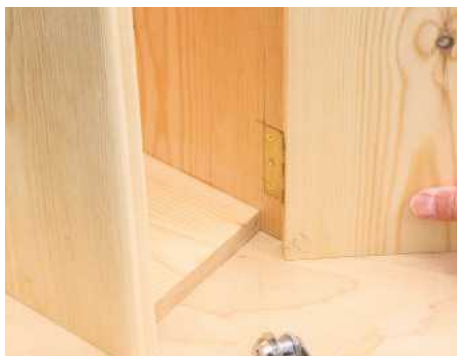
15 Cut the roof panel to size, bevelling the rear edge. Check for an even overhang all around
