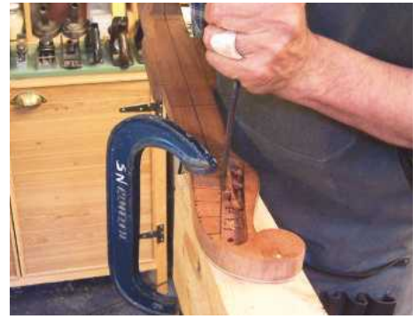
21 The Staufe-Mechanik housing under preparation
