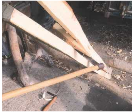
Tangential cleaving – guiding the split
