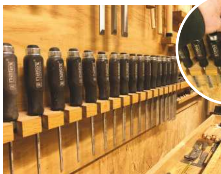
2 Bevel edge chisels from 3mm up to 50mm all have their own place
