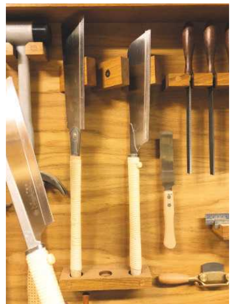
6 Pull saws sit in shallow holes, which lock the bottom in and the tops are held by magnets
