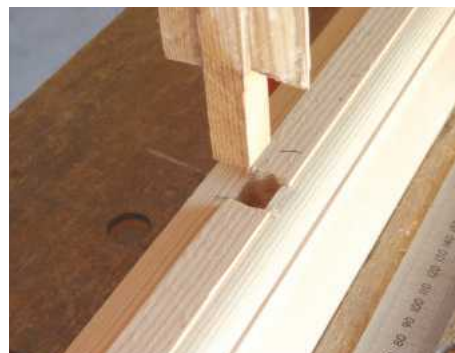
Mounted in a router table, the profile bit made life that much easier, ensuring consistent results
