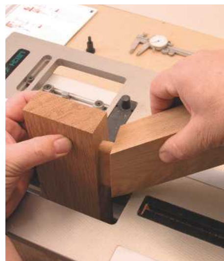
17 The angled tenon has matching angled shoulders while the mortise is a conventional straight one
