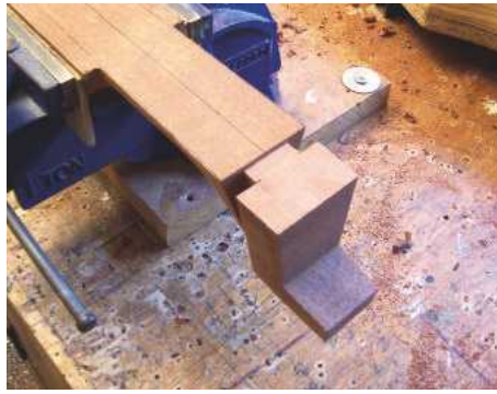
20 The ledge at the top of the heel to accept the soundboard
