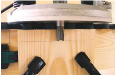
Setting the router cutter depth; the line is drawn by placing the timber that will form the second part of the joint under the template and then marking along the underside with a pencil
