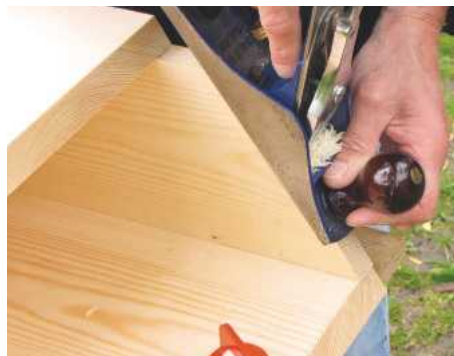
12 Carefully trim both sides flush, checking their angle with a sliding bevel
