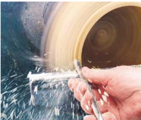
17 Cut a bead using a spindle gouge with the wings ground back...
