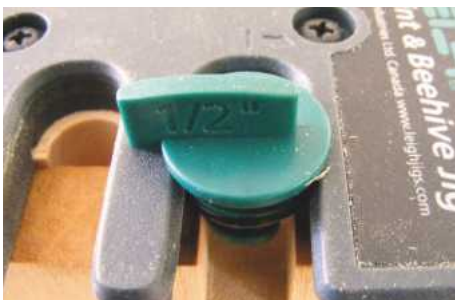
The step-over cam shown in alignment position; the socket to the left has yet to be cut
