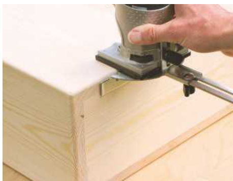
20 Using a bearing-guided router cutter, round over the edges of the box before sanding
