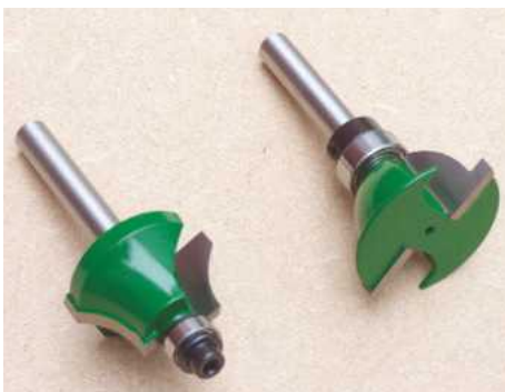
Consisting of a pair of 1/2in shank scribe and profile cutters, I only wish I'd found them sooner
