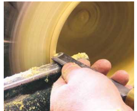
19 Alternatively, cut the bead using a skew chisel
