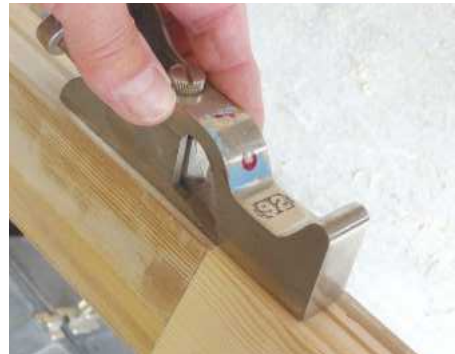
Using a moulding plane was hard going, and I had to do final shaping with a small shoulder plane and abrasive paper
