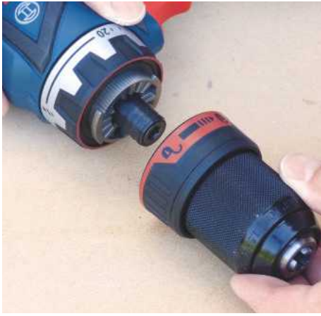
With the relevant unit aligned with the end of the drill, you twist the collar to click it into position
