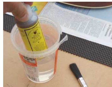
Place the bottle in a container of hot water (not boiling), so the glue becomes less viscous
