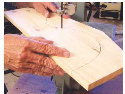
7 The mould boards are then roughly cut out on the bandsaw
