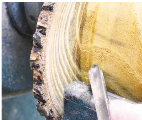
12 A smaller spindle gouge enables access to the underside of the rim...
