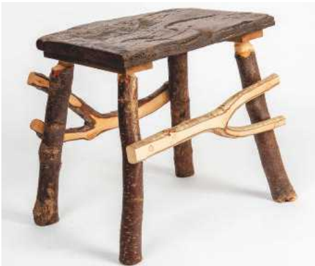
Stool; oak, blackthorn, cherry and hazel. The seat is made from a 430-year-old floorboard, the legs are blackthorn, and the cherry and hazel stretchers have been spokeshaved to reveal the pattern of bark, sap- and heartwood
