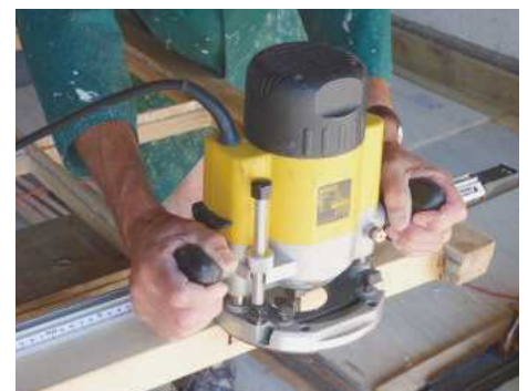
I glued and screwed new full-length pieces to the bottom rails, then cleaned them up
