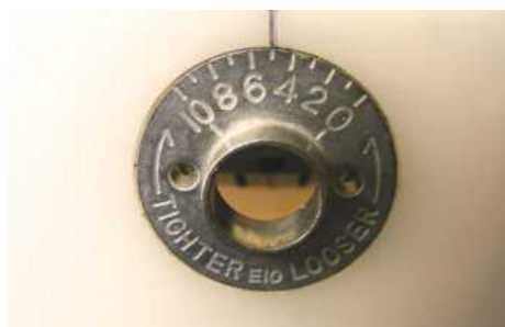
Guide bush set up at the mid-position '5'; the line needs to be marked centrally from front to back on the sub-base
