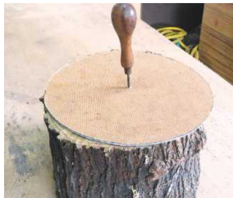
3 Locate the centre at both ends and mount between centres
