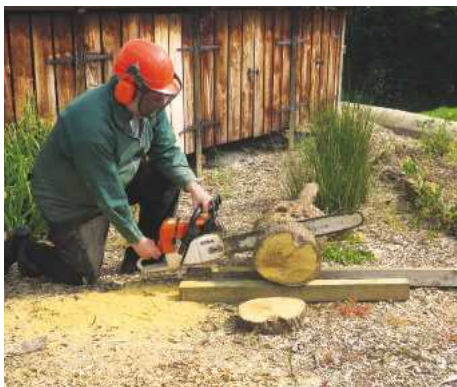
2 Remove at least 50mm before cutting your blank
