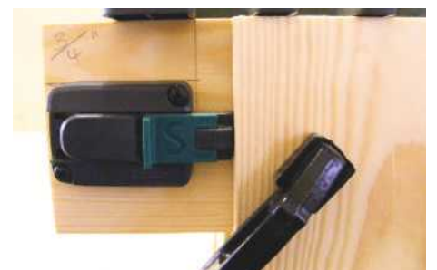
The adjustable side stop in socket position is slid up to the edge of the board and ensures repeated accuracy
