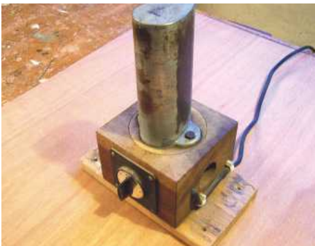
25 A commercially available heated bending iron
