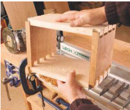
7 Through dovetails cut on the jig are being assembled on the frame of this box
