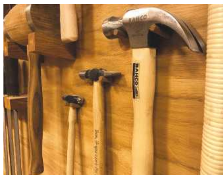
5 Hammers hang on oak dowels, which are drilled and glued in at a 10° angle
