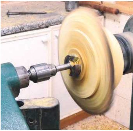
14 Drill a hole in the centre of the bowl...
