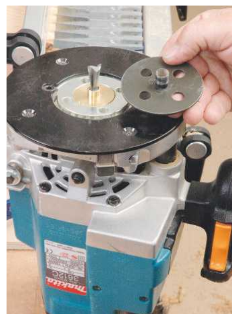
3 Routers are powerful cutting machines that must be tightly controlled. Guide collars locked in place around the cutter shaft enable the router to be accurately guided by the fingers of a jig
