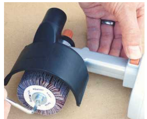
To change a sanding wheel or drum, you depress the spindle lock button and insert a hex key at the end of the shaft to release the wheel's retaining screw
