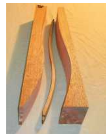
Two 'formers' in which a back slat is held once out of the steamer
