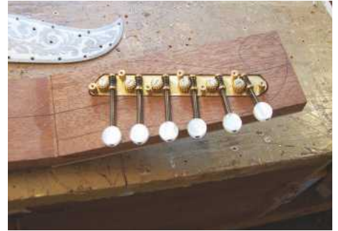
24 The headstock showing the Mechanik in place
