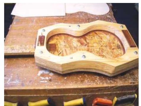
10 The completed mould – note the removable block to allow the neck through
