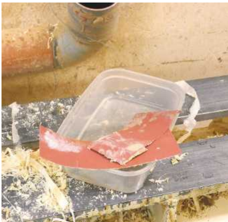
22 When I first made this type of work from wet wood, I would friction dry the bowl's surface with heat generated from the sanding process. Nowadays, however, I tend to wet sand the surface and I find this is more effective as well as enjoyable
