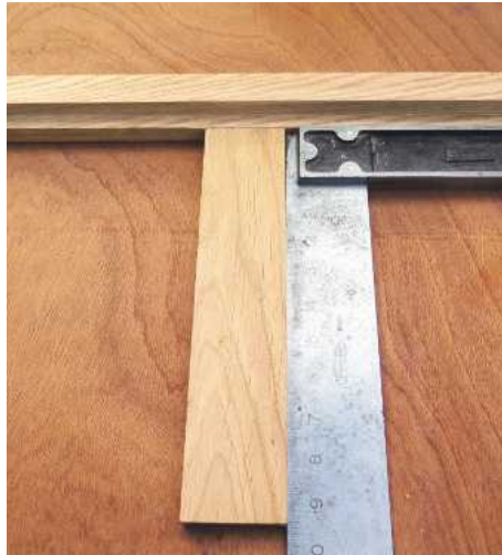
4 Rear section tenoned into front
