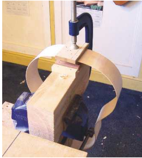
29 The inlay is cramped into place
