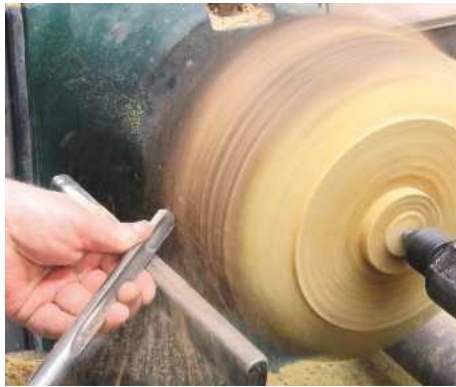
9 Chopping cuts quickly remove excess wood but...
