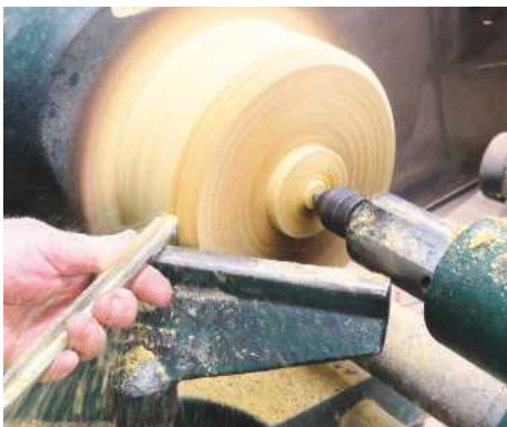
11 Now the bowl part is cylindrical, shaping will be much easier
