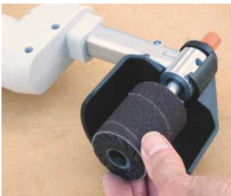
Sleeves are a pretty tight fit, so swapping one means using the spindle lock button while twisting the abrasive free
