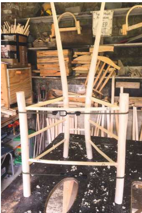
Chair temporarily assembled using bungees and dummy rails ready to check the back frame fitting
