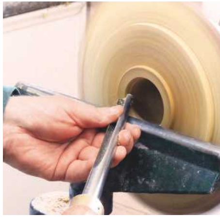
15 ... and hollow from the hole towards the rim
