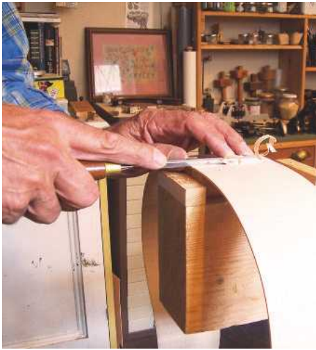
28 The tailblock inlay slot is cut out with a sharp chisel
