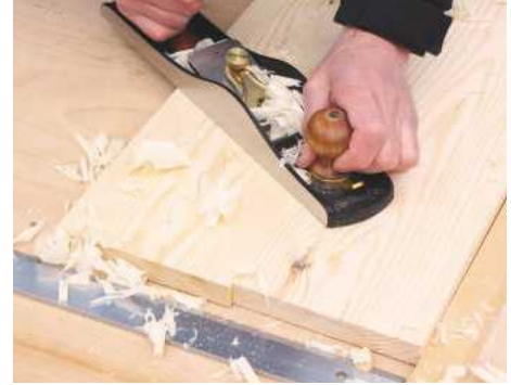
4 When the glue has dried, level the boards with a bench plane, checking them with a straightedge
