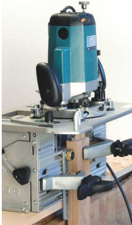
13 A dedicated mortise & tenon jig has the router attached to a guide plate, which is slid around the joint as it is cut
