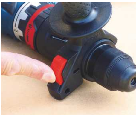
There's provision for a hexagonal depth rod, though oddly none is provided
