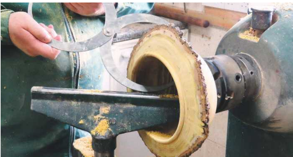
20 Check for an even wall thickness using double-ended callipers
