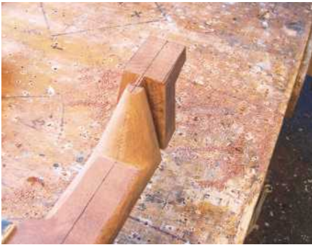
19 The cone-shaped heel nearing completion
