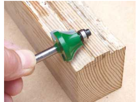
Trend came to the rescue with their Craft Pro range of cutters. In fact, their bearing-guided glazing bar set (CR/SSP2) was pretty close
