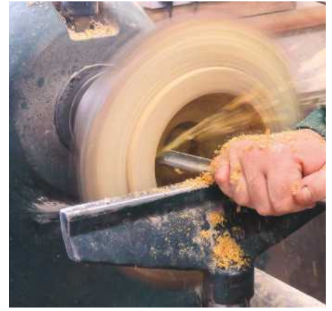
16 Keep the cut near the tip of the tool
