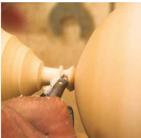
25 You don't want to make the stem too thin as the piece will not look balanced. The bevel of the spindle gouge must be in contact with the wood or the cutting edge will dig in and ruin all your hard work so far
