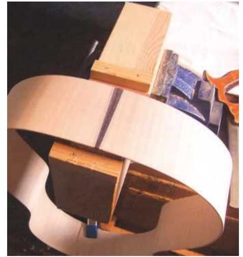
30 Once in place the tailblock inlay is looking good
