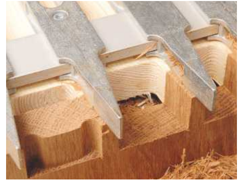
6 Using tapered fingers and a straight cutter enables the jig to produce a good set of through-dovetails
