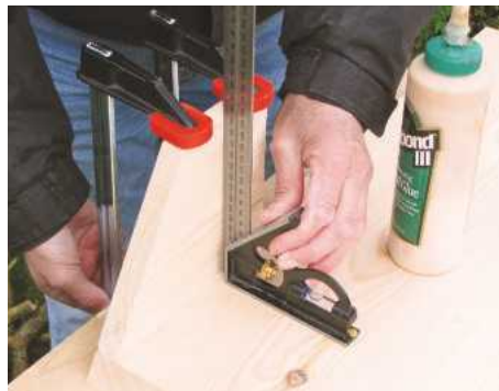
9 Glue the short end first with PVA, checking for square as you tighten the cramps. Allow this to dry
