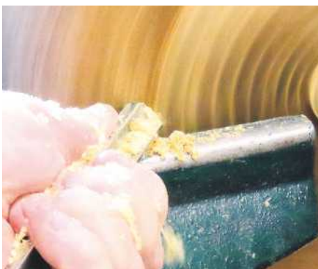
5 Use the tip of the tool, keeping the wings away from the wood
