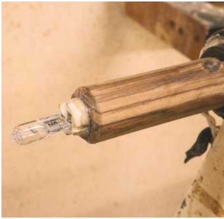
19 The best way to judge the wall thickness when you get thin is to use a light. This is a 12V shop-built lamp holder with a very sensitive circuit breaker, just in case
