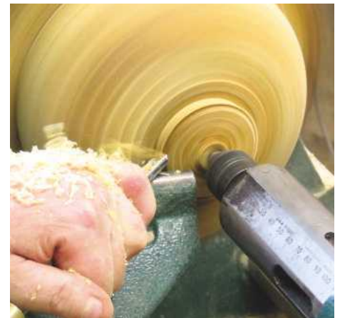
25 ... to turn away the chucking spigot
