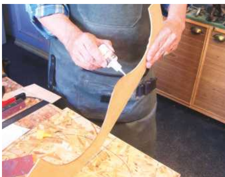
5 Hardening the template edges with CA adhesive
