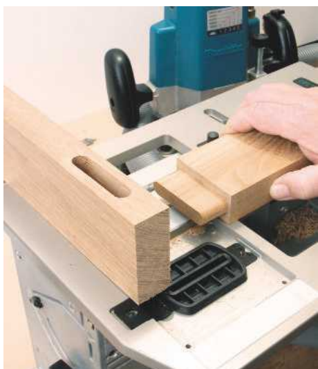
15 The finished mortise & tenons have matching rounded ends. The template for this joint can be seen clipped in place beneath the wood
