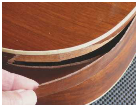
The guitar had either been knocked over or dropped, resulting in a couple of serious splits to the ribs
