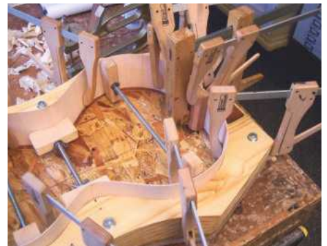
27 The tailblock in place
