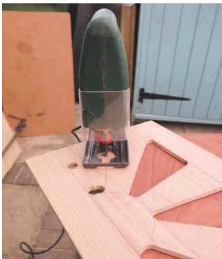
2 Carefully cutting the starburst pattern with a fine jigsaw blade
