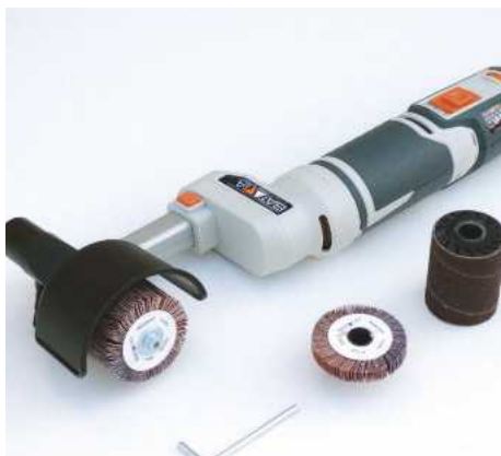
The two flap wheels and sanding drum included are fairly coarse at 80 grit
