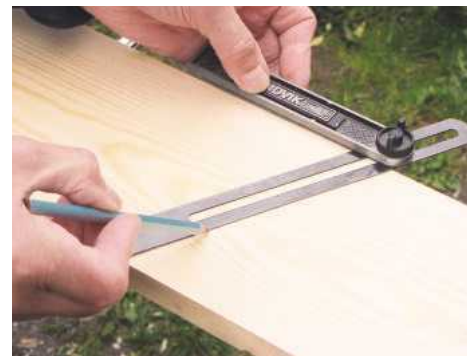
7 Set a sliding bevel to 60° and mark the top edge of the side panels. Saw and plane the ends
