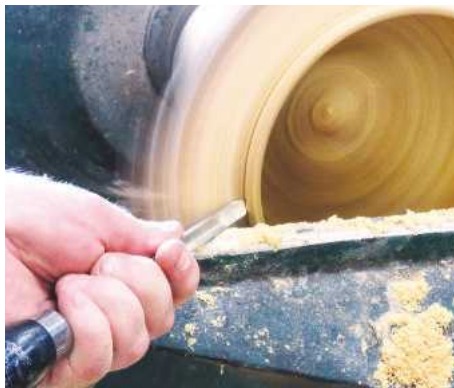
18 ... but keep the wings away from the wood
