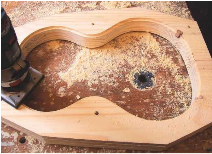
11 A rebate is cut on the underside of the mould body
