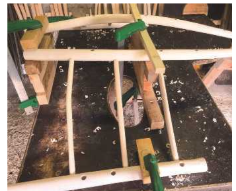
Chair sides in the jigs, ready for drilling
