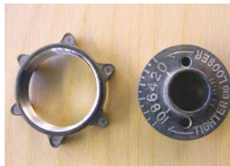
Guide bush and nut; the bush is elliptical, but this isn't clear in the photo!
