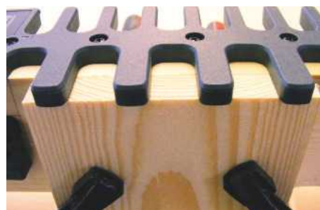
Timber aligned and clamped for the first joint; note the even overlap of wood in the recesses at each end, which ensures the joint is central
