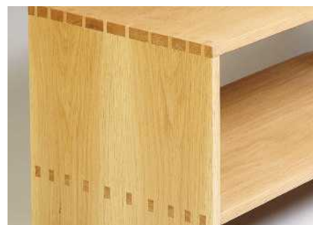
12 The assembled row of mortise & tenons completely match the row of dovetails above them, cut with the same jig settings
