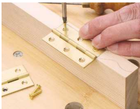
17 Mark out the positions of 65mm brass hinges and chisel recesses carefully. Drill and fit screws
