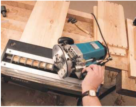
4 The simplest set up, but one used a lot in furniture making, is a fixed spacing jig for making a row of half-blind dovetails
