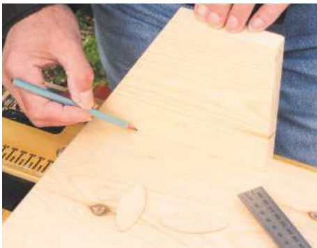
8 Cut biscuit slots on all four panels. This fixed short end is above the hinged door
