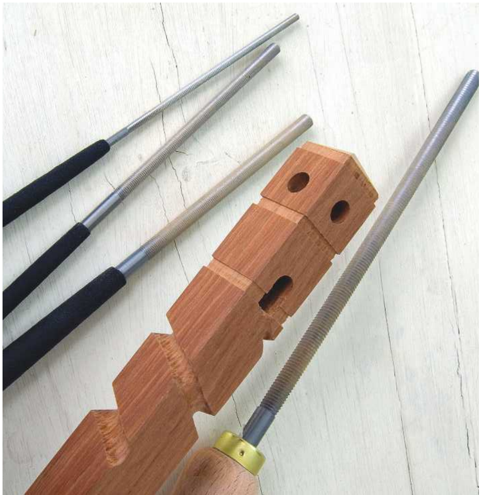
A test piece. (Windows drilled. Door drilled and chiselled. Roof and corbels mitre-sawn.) Pathway filed
