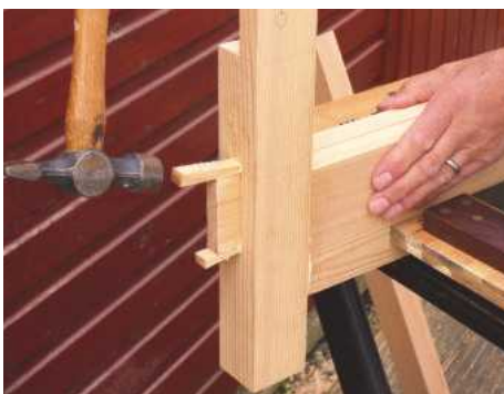
19 Apply exterior glue to the tenon surfaces and assemble the rail and stiles. Cramp across the width and tap wedges into the mortises
