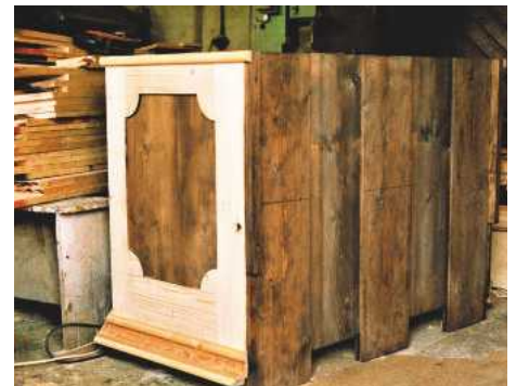
5 Base cupboard from rear – the infilled corners of the side frames can clearly be seen
