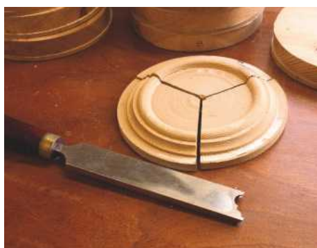
15 Turned bolection moulding on its MDF faceplate – with specially shaped scraper
