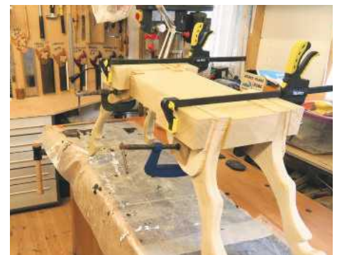
3 Legs glued and cramped to the lower body block
