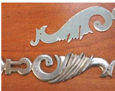
19 Steel escutcheon with its aluminium template
