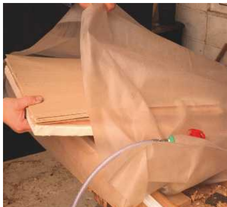
9 Using a single curved former (rather than a pair of cauls), the laminated sandwich is inserted into a vacuum bag to press tightly onto the former
