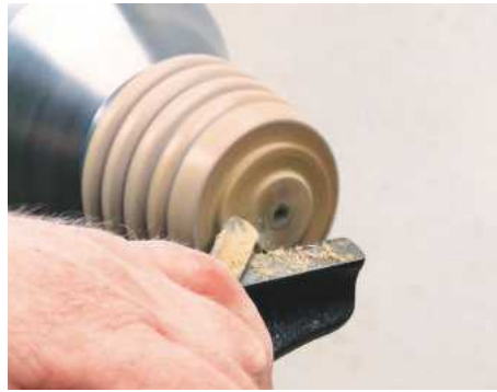
29 Reverse the lids onto the chuck and remove the chucking spigots
