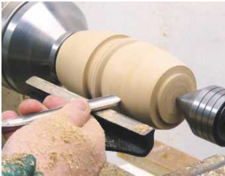
7 Use a spindle gouge to shape the box. I made mine a barrel shape
