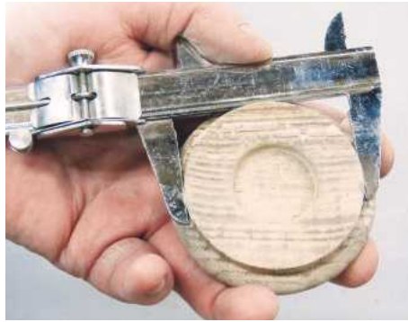
17 Measure the diameter of the tenon...
