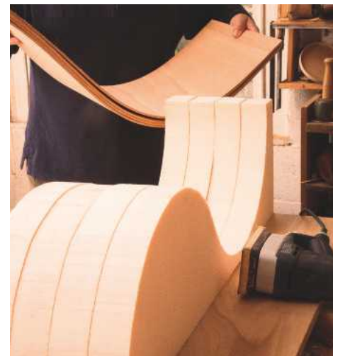
10 Large section formers are built up from rigid expanded polyurethane sheet
