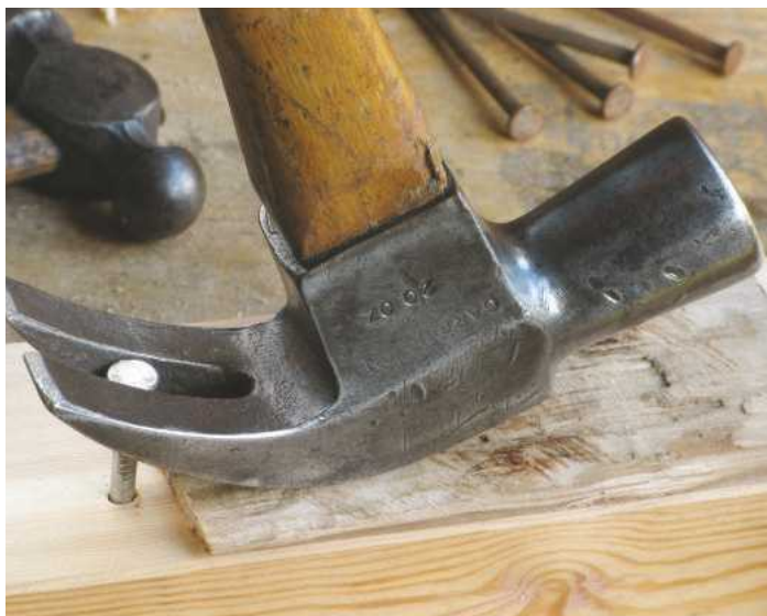
34 Pulling a nail with the adze-eye claw hammer
