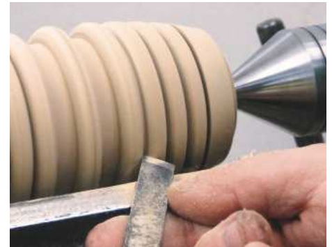
9 ... or a skew chisel on its side
