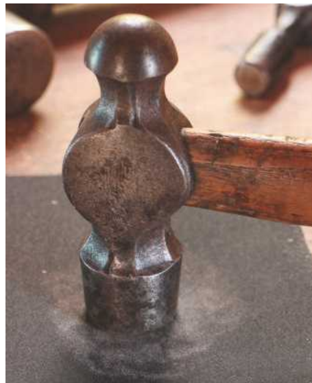
29 Abrade the hammer face to improve traction on the nail
