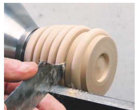
15 Use a narrow parting tool to part off the second lid
