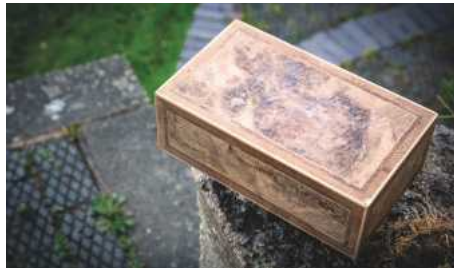
When it comes to clasps or inlay, box-making is an obvious example of combining the woodworker's skills with those of the jeweller or metalworker. To separate the lid, Richard's planning to use a Japanese saw: "The trick is to tape along the cut so that the kerf is held stable; cut down one side, then the next, retape, turn it over, and cut the other sides"
