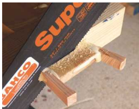
20 Once the glue has dried, saw off the excess tenons and wedges just proud of the stiles. Plane the surface flush on each stile
