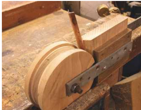
25 Fitted in jig prior to bending...
