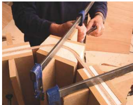
7 Large scale cauls built up in sections provide a versatile way of laminating wider boards
