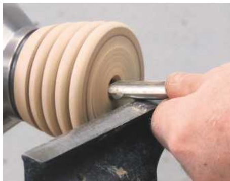
20 ... and start hollowing from just inside the hole, then swing the handle away from you
