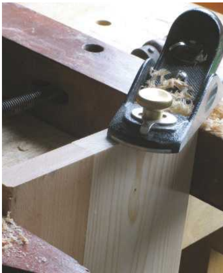
28 Alternatively, clamp the board edge-to-edge with a backing piece
