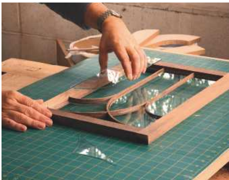
6 The laminated glazing bars and glass cut to match are fitted in the frame of a cabinet door
