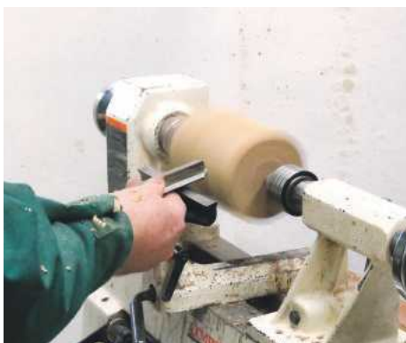
1 Rough the blank down to a cylinder
