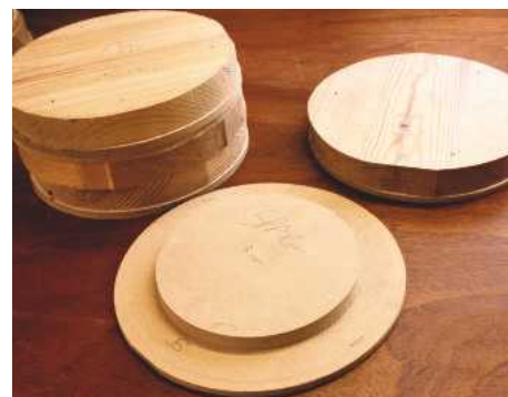
14 Rebated MDF faceplate used for circular moulding
