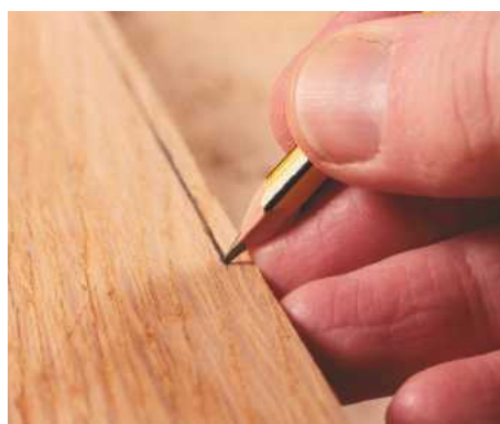
8 Run a pencil along the edge to be trimmed
