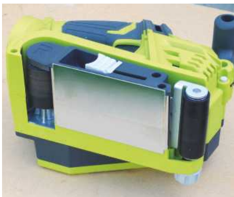
An 80mm wide steel platen provides a sufficiently flat area for the belt
