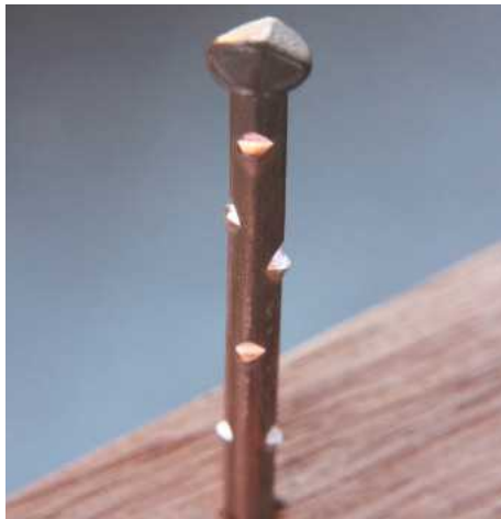
31 Ragging a copper boat nail with an old chisel
