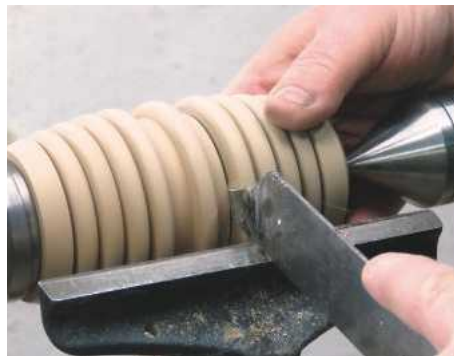
11 Use a narrow parting tool to part off the right-hand lid...
