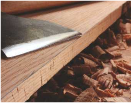
10 The hewn edge is ready for planing to the line
