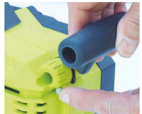
You can lock the front handle in any one of three different positions, by first depressing a button underneath the sander
