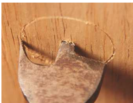
6 ... then centre the bit on the second side...
