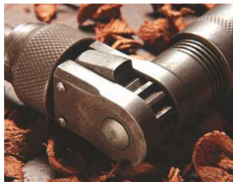
3 Ratchet wheel, pawl and selector ring
