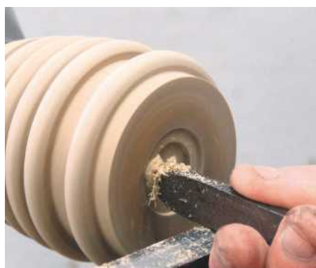
14 Use a parting tool to cut a recess to hold a coin
