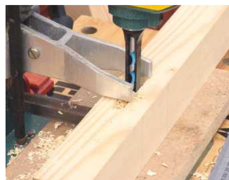
9 Mark each mortise with a gauge, plus matching tenons on the rail. Chop out from each side with a hollow chisel mortiser or by hand
