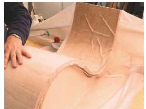
11 Large deep-section formers can be used for laminating in a vacuum bag provided the bag is carefully positioned to follow the curves before suction is applied
