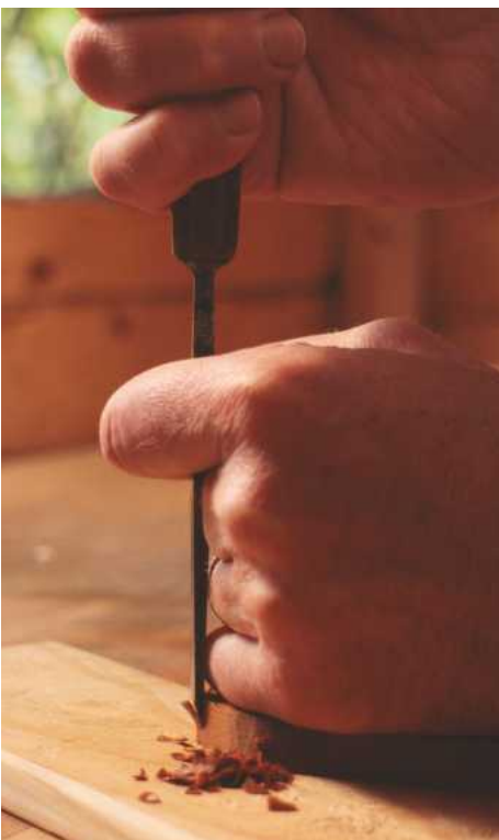
14 Thread the blade between forefinger and knuckles
