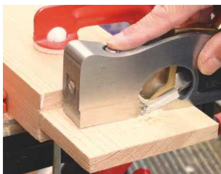
11 If necessary, trim the tenon cheeks with a shoulder plane, ensuring these are flat. Check tenon corners fit snugly into their mortise
