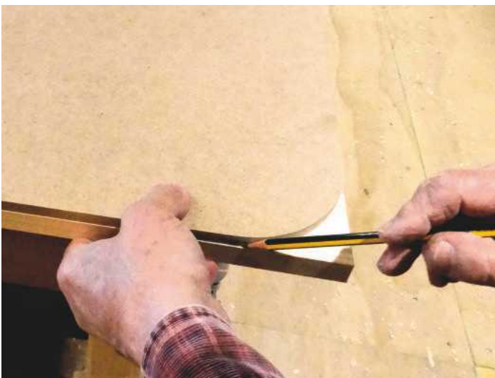
3 Cut the template accurately then draw round it to ascertain the waste
