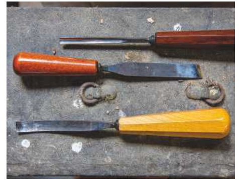
There was a time when you could buy chisel blades on Tottenham Court Road for £1.50, then add your own handles; round ones are attractive, but octagonal ones don't roll off the bench!
