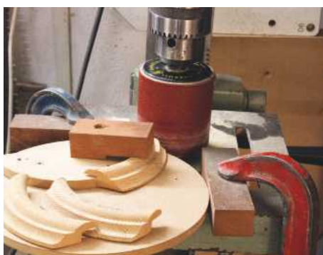
16 Jig used with pillar drill to impart curve to mitred corner of turned bolection moulding
