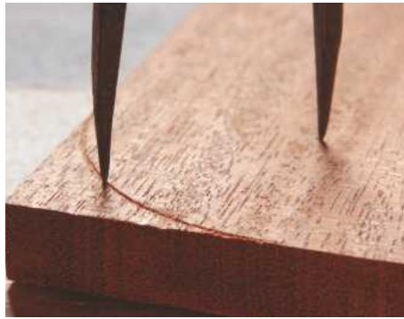
11 Scribe an arc around the corner with dividers
