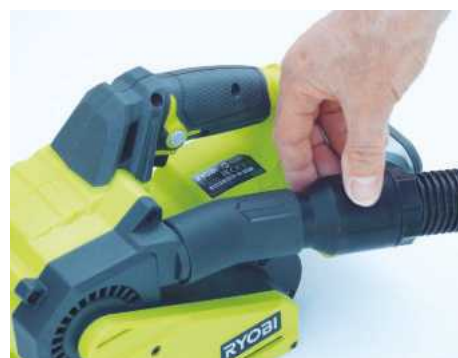
An angled plastic adaptor connects the hose
