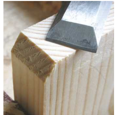
27 Cut a chamfer on the far end before planing
