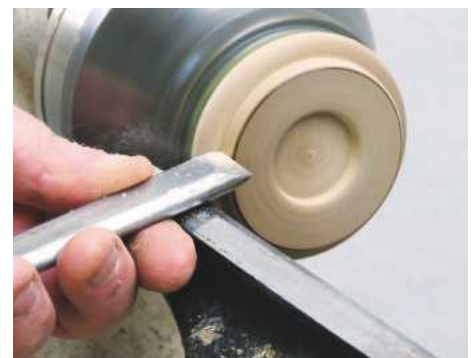
27 If you then cut the tenon to this mark, the lid will fit perfectly
