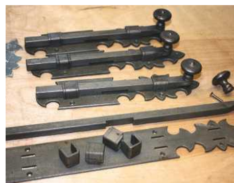
20 Almost completed bolts with their aluminium template
