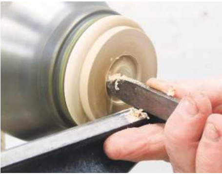
16 Cut a similar recess on the opposite side of the middle section
