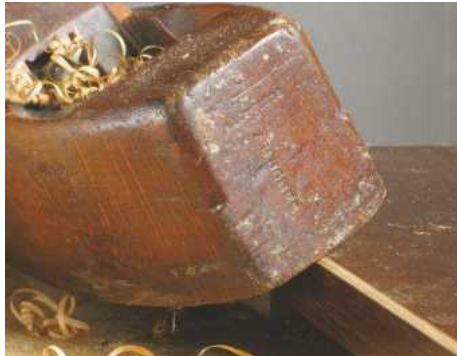
22 Chamfer the far edge before planing across the face
