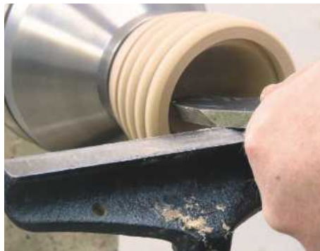
23 Take light cuts with a round-nosed scraper to smooth out the hollow
