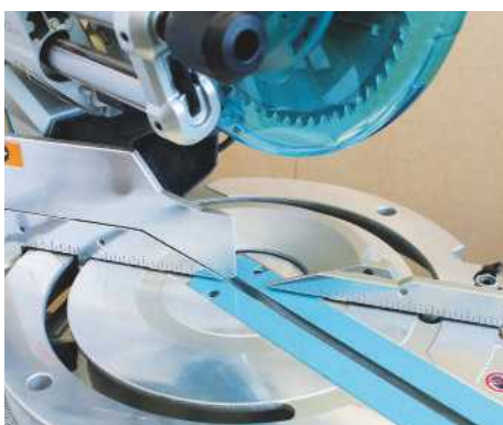
Mitres can go up to an impressive 60^\circ
