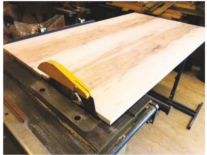
2 One over length end about to be trimmed, using the already trimmed half as a guide
