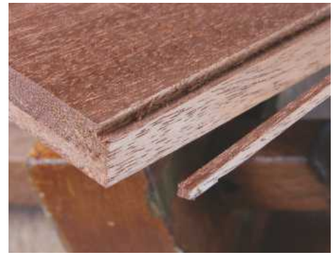
21 Waste is parted in a single usable strip
