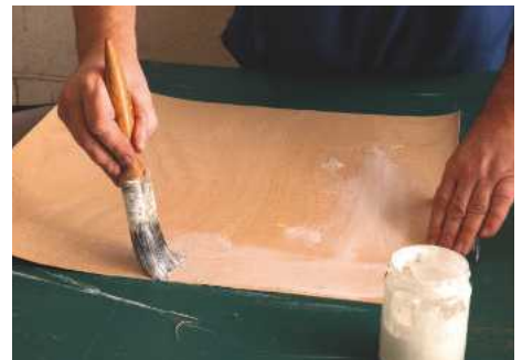
13 PVA glue is suitable for bendy veneers because it sets semi-flexible
