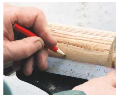
3 Mark the exact centre of the cylinder
