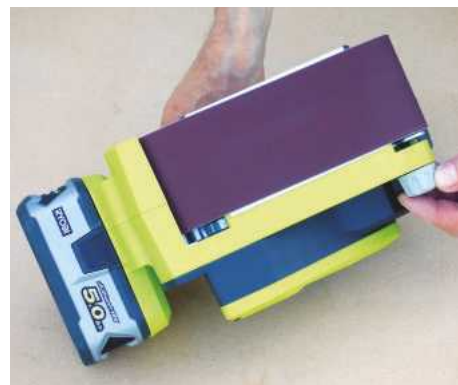
Tracking is adjusted in the normal way, rotating a knob at the side of the roller
