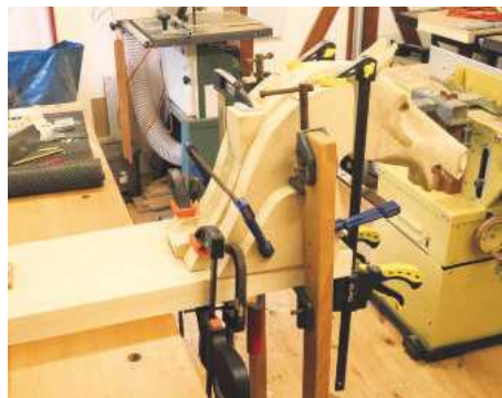
2 Head, neck and muscle blocks glued and cramped to the upper body block
