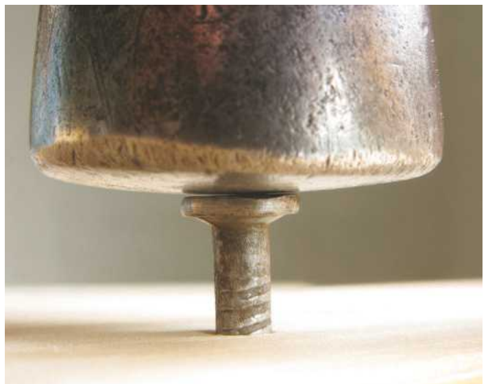
35 Domed striking face centred on the nail head
