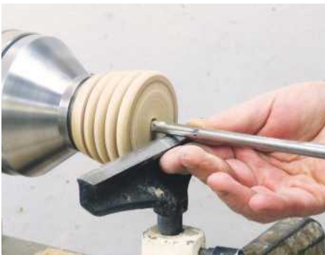
19 Use a spindle gouge to drill a hole down the centre...
