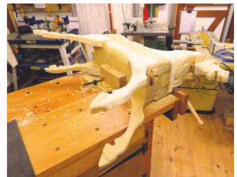
7 Bench dogs used to hold horse during carving
