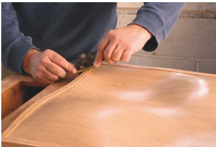
14 Three-dimensional curved shapes, formed by laminating onto a former in a vacuum bag, open up new possibilities in furniture making
