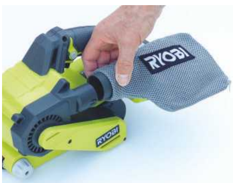
With dustbag fitted there can still be a small amount of dust discharged, so you need to make sure this is twisted firmly on to the port
