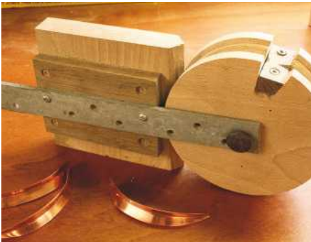
24 Jig for bending copper leaves – basic but effective
