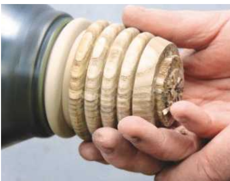
25 ... and offer up the lid. The lid should fit somewhere on the chamfer and if the lathe is running as you do this...
