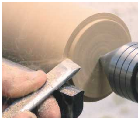
2 Cut a chucking spigot on both ends
