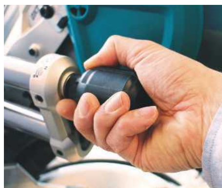
The locking knob for bevel-cutting is nicely positioned
