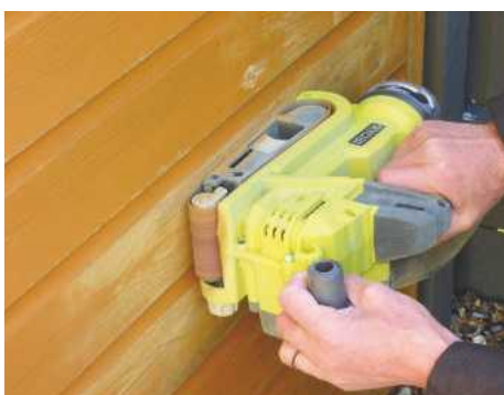
Applying too much downwards pressure when sanding caused the belt to veer to one side, though lifting off the tool meant the belt corrected itself
