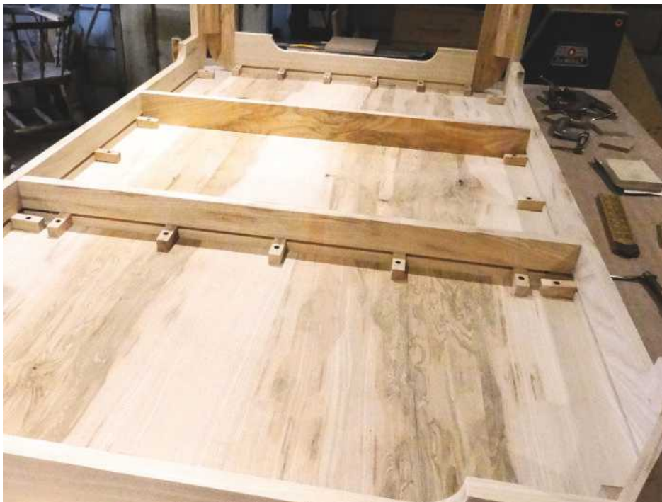
10 Buttons pinch the top, primarily across the grain where any warping should be dissuaded
