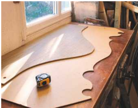
3 Router template for the profiled shelves – also one for the top of the cupboard
