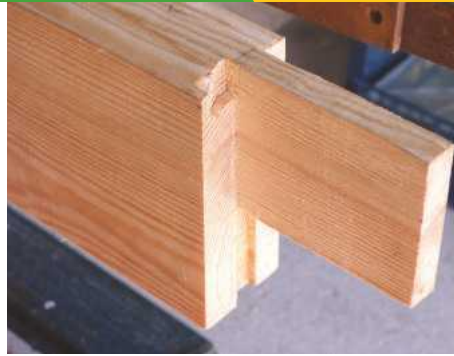
14 You'll need to scribe the tenon shoulders where they intersect with the stiles. Do this with an appropriate in-cannel gouge
