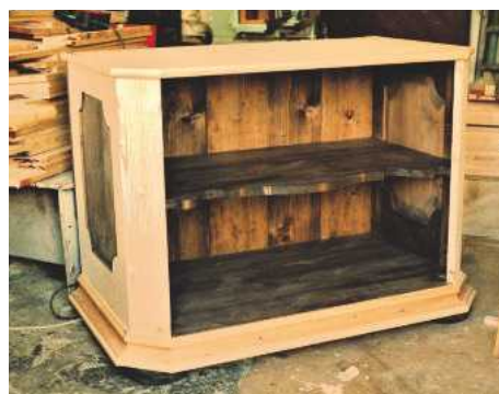
2 Base cupboard with ornately profiled shelf, amidst piles of maple for a kitchen job
