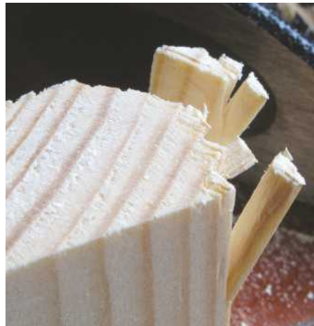
26 Planing end-grain splits unsupported fibres from the edge
