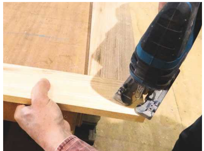
4 Jigsaw away the waste leaving a clear margin
