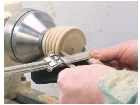
18 ... and transfer this to the underside of the lid
