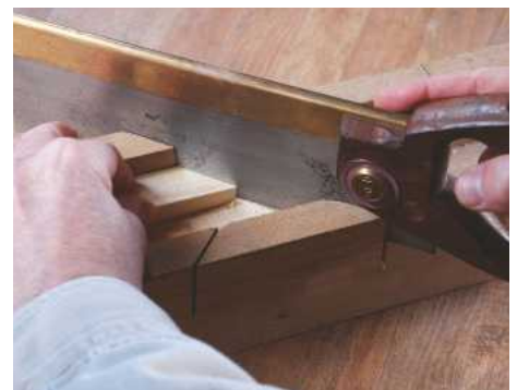
16 Using the 45° guides to cut a mitre
