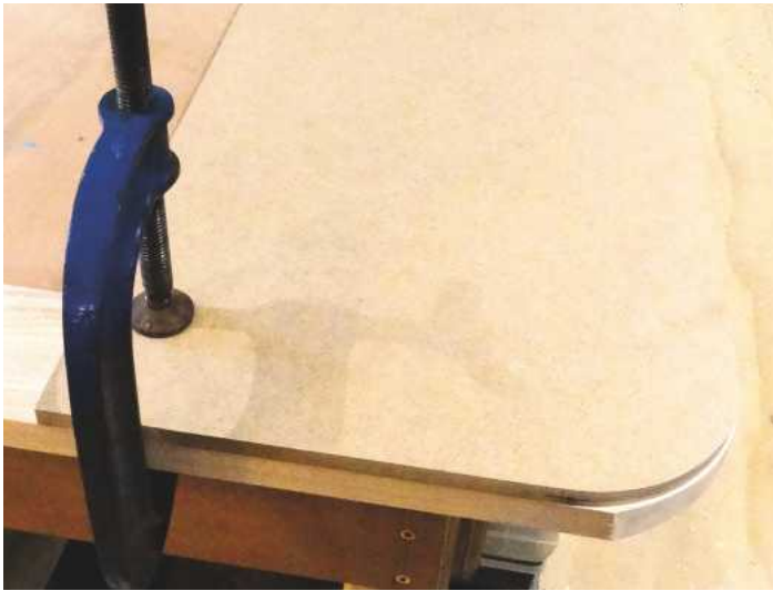
5 Cramp the template in place
