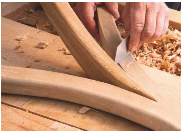
15 Glue lines being scraped from a component made of laminated maple and solid oak
