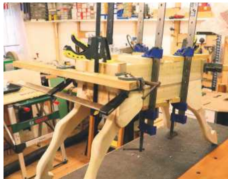
4 Side and end body blocks glued and cramped to the lower body block
