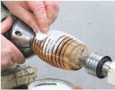
28 Fill the grain with liming wax
