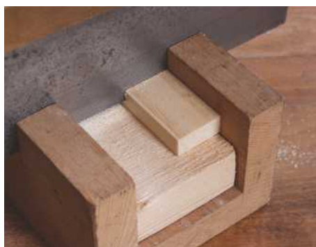
17 Sawing an end square using perpendicular guides
