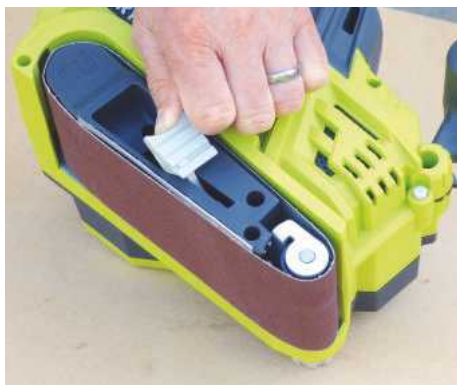
To change a belt you simply open out the spring-loaded side lever, which retracts the front roller
