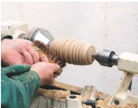
10 I used a bronze brush to pick out the timber's softer spring growth
