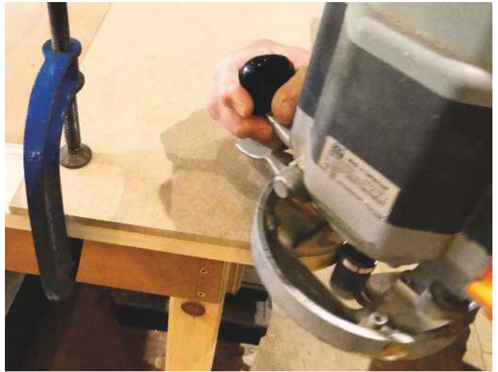
6 Run round it with the router
