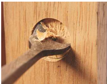
4 Bore with the centre bit from one side...
