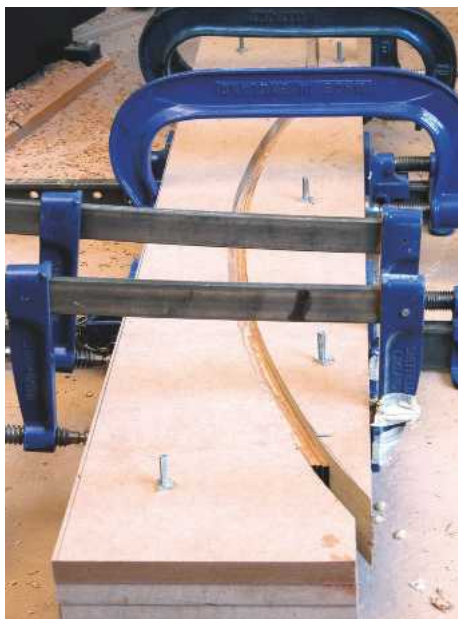
2 The strips of oak, glued together in layers with synthetic resin, are pressed between two formers, or 'cauls', made from MDF boards
