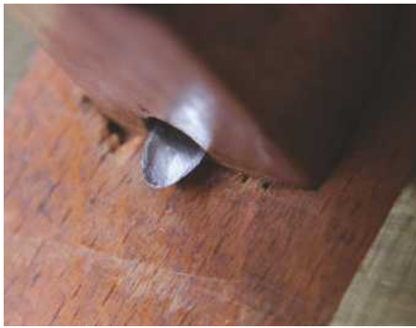
19 The cutting gauge has a knife-edged blade
