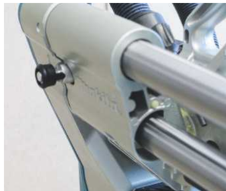
Bevel cuts go up to 48^\circ on the left...
