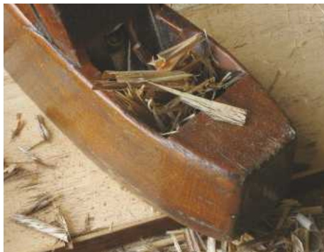
23 Cross-grain shavings are typically short and brittle
