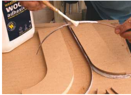
4 Miniature scale laminating with walnut strips to form cabinet glazing bars. Note how the bar branches in two directions
