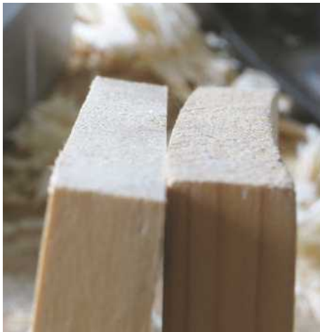
25 A cupped board is flattened for a small loss in thickness
