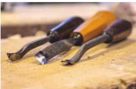
To keep his carving chisels bright, Richard favours the felt mop of a stone-polishing wheel, and a smear of jeweller's rouge
