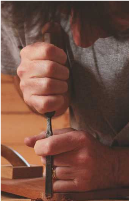
13 Apply upper body weight to drive the chisel downwards
