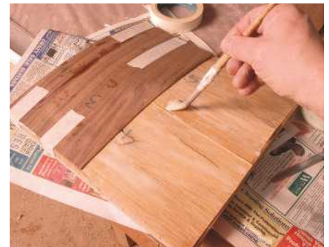
8 To form the curved lid of a box, inner layers of oak and outer layers of walnut are laminated in alternate directions, producing custom-made curved plywood
