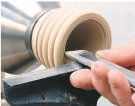
22 Use a skew chisel on its side to cut a straight-sided recess just inside the marked line. This should be about 6mm deep
