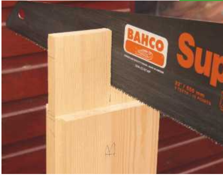
13 The tenons on the bottom rail are franked for strength, rather than haunched. Mark the joints and saw away the waste
