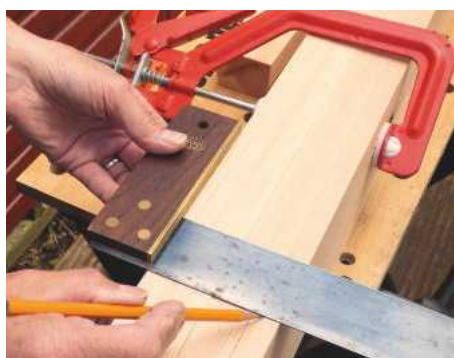
8 Cramp both stiles together and mark out the mortise positions. Each stile is then cut to a length of 350mm, including horns
