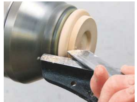
24 Use a skew chisel to cut a small chamfer on the tenon...
