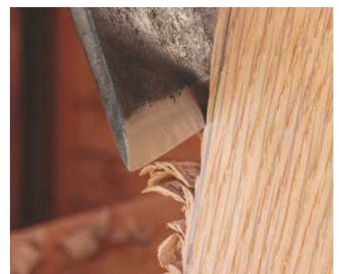
9 Hew with the grain, using stop cuts to prevent splits
