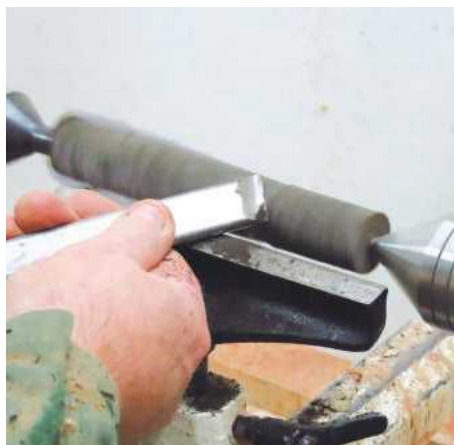
7 Plane the feet to a cylinder with a skew...
