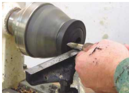
17 Turn the lid round and shape the front with a spindle gouge
