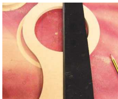
4 Draw a vertical line through the centre of the clock
