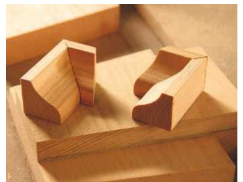
12 Mitred corners of architrave
