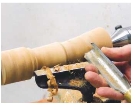
10 Rough the vase to a cylinder and start the taper
