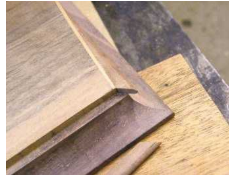
18 The moulding is made in two parts
