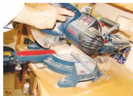
3 The tenons were dealt with on the sliding mitre saw, using a depth stop
