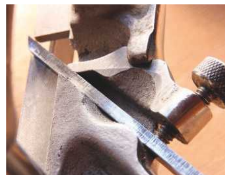
7 The Record 043's lever cap has a recess for the thumb...
