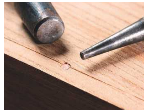
19 A nail head sunk using a tapered set
