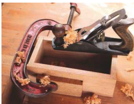
5 Sides, ends and base clamped for planing top edges
