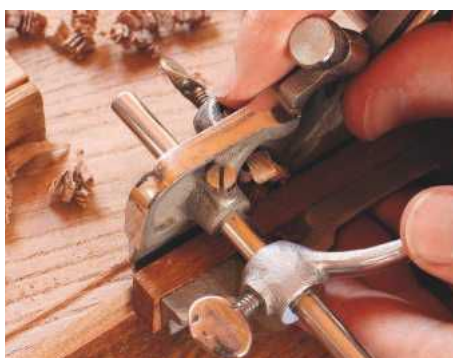
12 Planing a \frac{1}{8} in rebate in the lid to fit its groove
