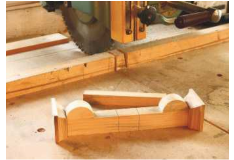
9 Brackets, made as one and ready to be parted, with packer behind for safety
