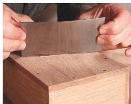
25 Finishing the base with a card scraper
