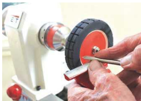
8 To give a crisp line between colours and to remove any overspill of paint, I put the work back on the lathe and make a 'V' cut
