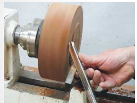
1 Use a pull cut to flatten the bottom...
