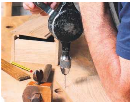
14 Boring clearance holes for nails in the base
