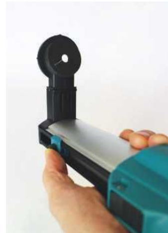
The telescopic extraction take-off is easily adjusted
