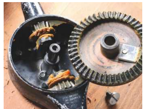
16 The alloy body encloses a double pinion mechanism
