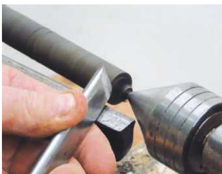
9 ... and use the skew to clean up the ends of the feet
