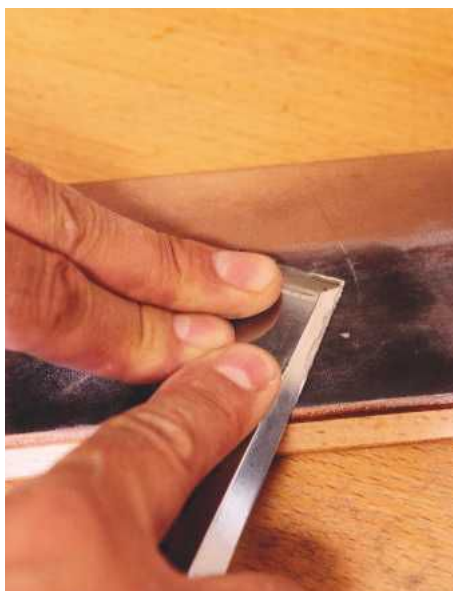
The blackening of strop charged with a honing paste shows that it is removing steel
