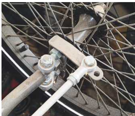
9 Steering arms fabricated from mild steel
