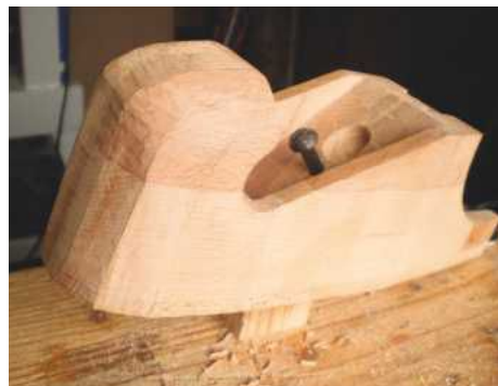
11 More shaping, screw recess and locking screw
