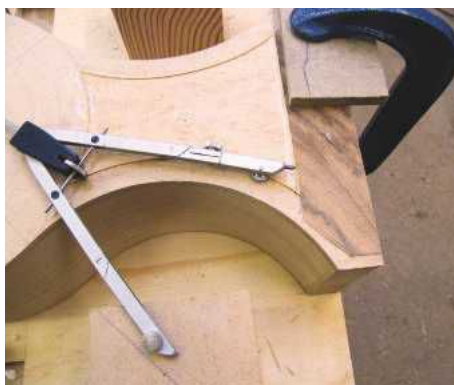
11 Note the stringing that is applied before the veneer
