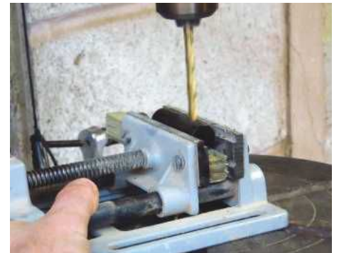
24 Drill two 5mm holes in each foot
