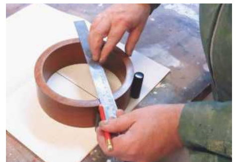
18 Mark the positions for the feet..
