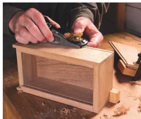
23 Planing the base flush with the sides...
