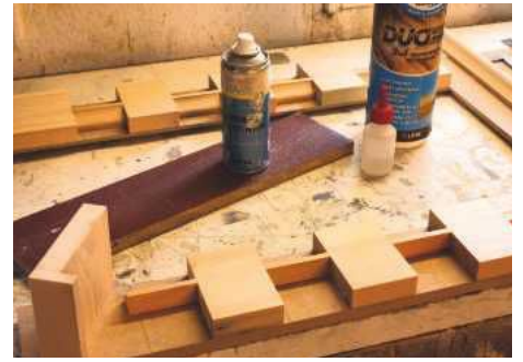
6 Base block about to be glued in position
