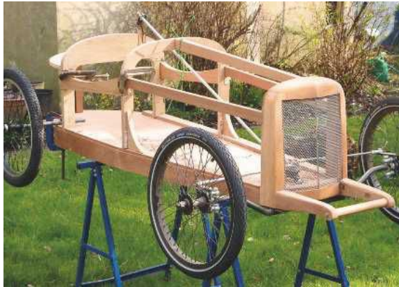
3 Finished frame prior to panelling
