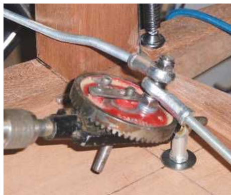
8 Modified hand drill and rod-end bearings
