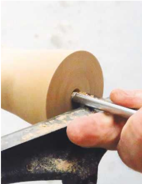
11 Drill a hole down the centre...
