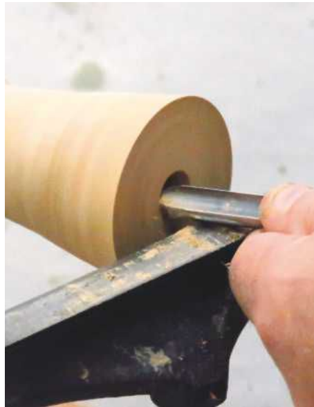
12 ... and hollow with a spindle gouge
