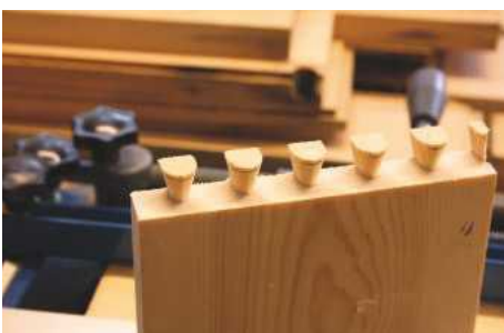
18 Pins reduced in width – with slight vertical ridge showing to front
