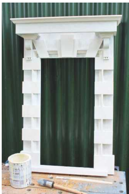
21 Surround primed outside the workshop
