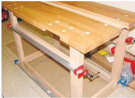
8 The bench top in a dry assembly with the bench framework
