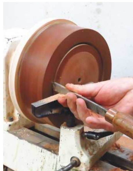
5 Use a parting tool to cut the ring...
