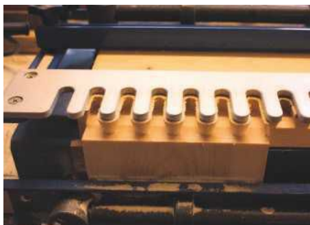
16 Set of dovetail pins routed in jig – to be used for the guttae
