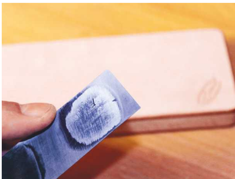
This chisel has been honed on a diamond stone and leaves a dull finish
