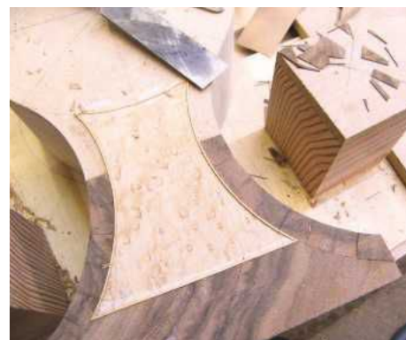
12 Keep the wedges a uniform size, radiating inwards towards the centre of the curve
