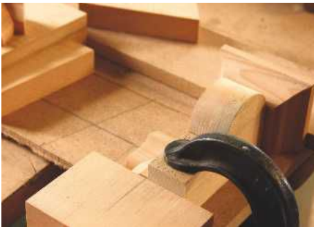
13 Bracket temporarily clamped – while architrave corner is glued in place
