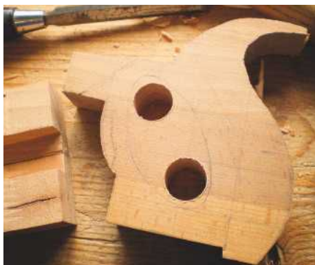
7 Ready for sawing out with the coping saw
