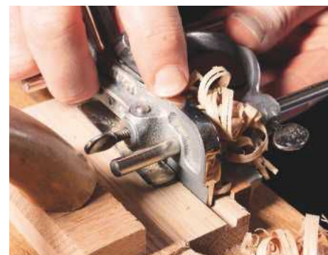
10 Ploughing the groove for the sliding lid
