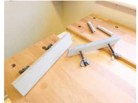
12 ... including 19mm dog holes for clamping work
