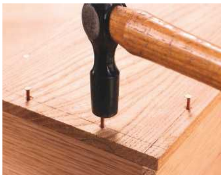
18 Hammer head centred and in line with the nail
