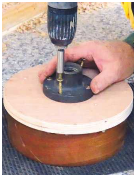
4 You then need to replace the screws in the faceplate with longer ones
