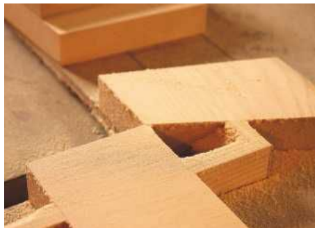
14 Architrave corner and voussoir sanded flush after gluing
