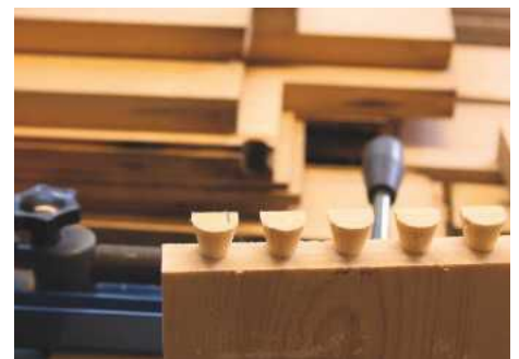
17 Pins fresh from jig before modification with offset marked
