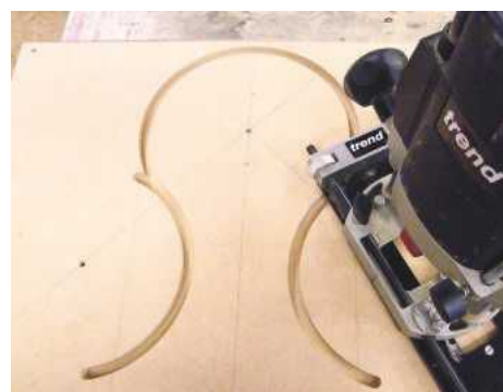
2 Stop cutting when the cutter reaches the radiating lines
