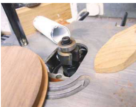
23 Note the use of the lead on timber to prevent the cutter kicking back
