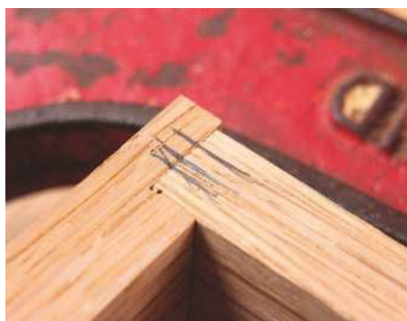
6 Marks used to identify corners
