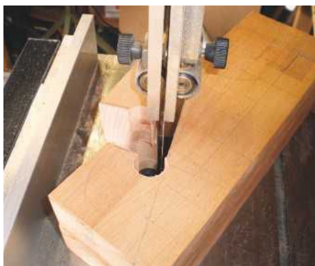
3 Cutting out the waste on the bandsaw
