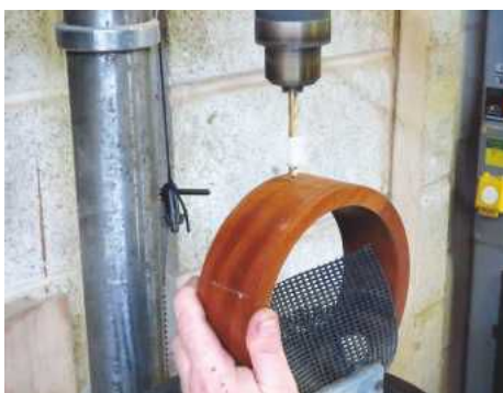
26 Drill the mating holes in the ring
