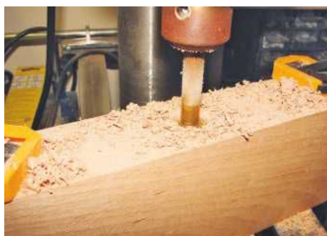
1 The mortises for the leg joints were cut using a Forstner bit...
