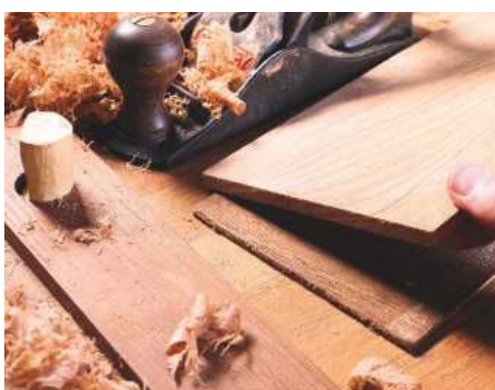
2 A plywood spacer enables the plane to clear the stop
