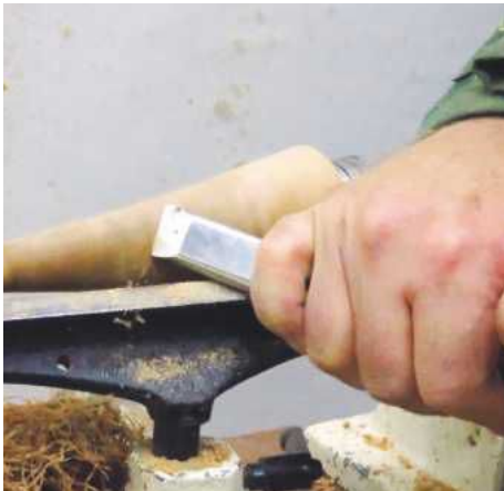
14 ... then complete the outside taper with the skew
