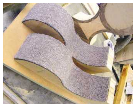
15 The carpet tiles glued to the moulds
