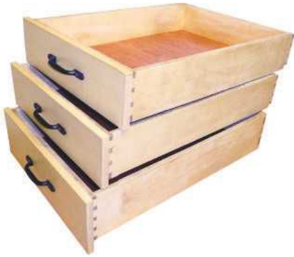
7 The drawer components were dovetailed together
