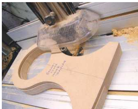
7 If care is taken, two or more pieces can be trimmed at once
