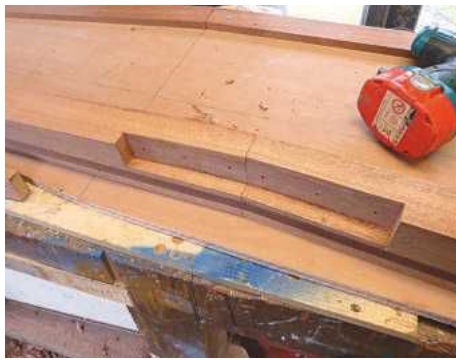
1 Forming the chassis rails
