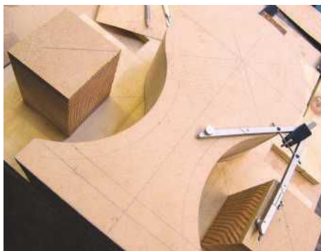
9 A simple jig ensures accurate marking out
