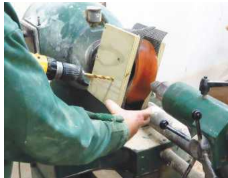
21 Drill holes for two bolts right through the cradle, insert bolts, then tighten
