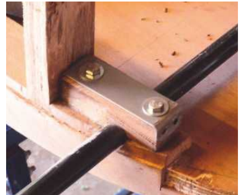
6 Wood and metal axle 'sandwich'
