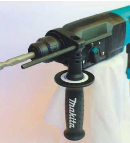
The SDS, with side handle and depth rod fitted
