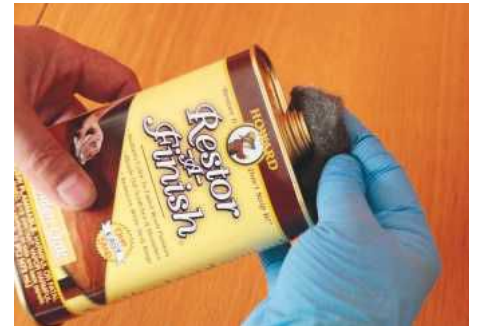
Apply a small amount of the finish onto a pad of steel wool...
