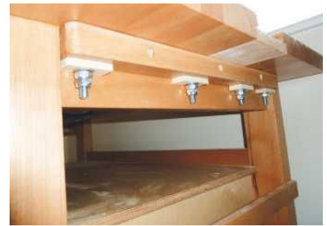
9 M10 bolts are the linch pins of the top-to-rails construction
