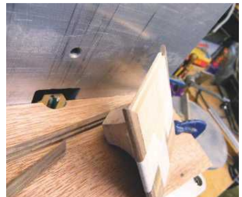
22 Note the false floor on the router table, which gives maximum support to the workpiece
