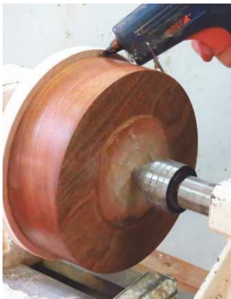
3 Centre the blank on the ply and hot-melt glue in place
