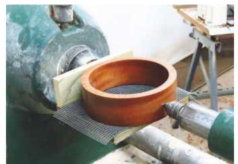
20 Mount the part-built cradle on the lathe and put the ring in place
