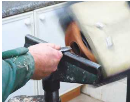
23 ... and widen it to a taper using a skew
