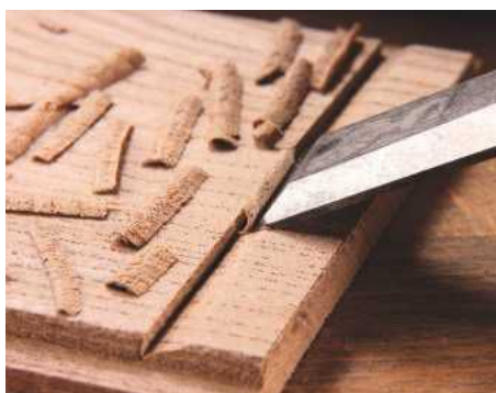
21 Cutting a shoulder for the rebate plane
