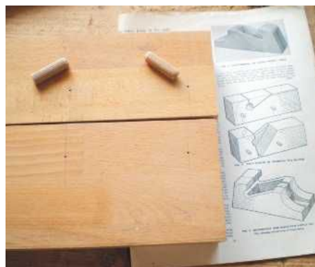
2 Setting the two body halves for dowelling
