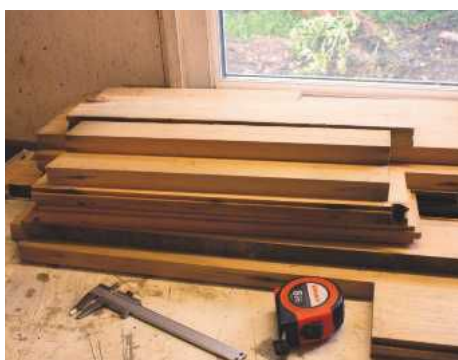
1 A generous amount of prepared stock reclaimed from a pair of Victorian doors
