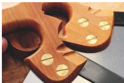
Attention to detail includes soldiered saw nuts for the handles
