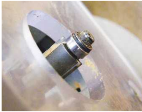
17 Note the smaller bearing, which provides the 1mm rebate
