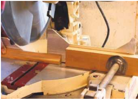
4 Accurately cutting short lengths of architrave on the chop saw
