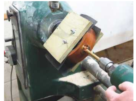
22 Drill a small hole through the ring...
