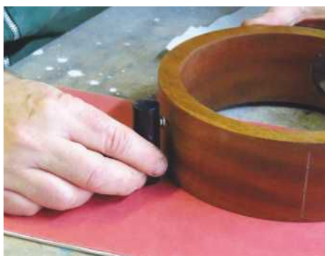
25 Insert dowel centres and locate on the ring
