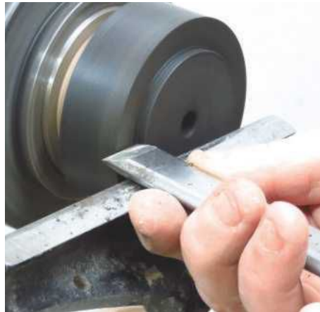
15 Cut a spigot on the lid to fit the step in the vase
