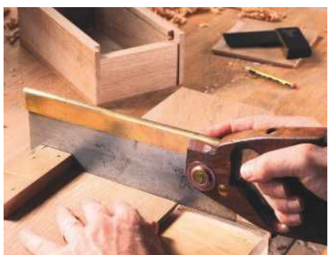
11 Sawing elm for the lid using the bench hook
