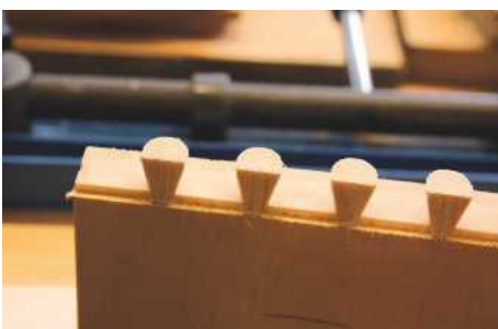
19 Finished pins now reduced in height and cut to their final depth on saw bench
