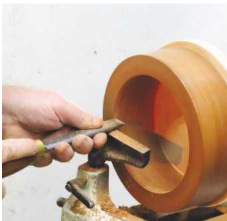
6 ... then clean up the inside surface of the vase with a skew chisel
