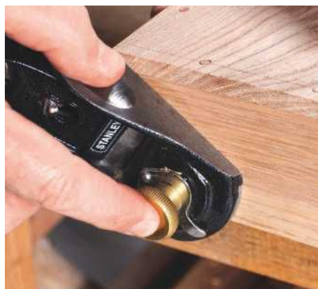
24 ... and the sides and base flush with the ends
