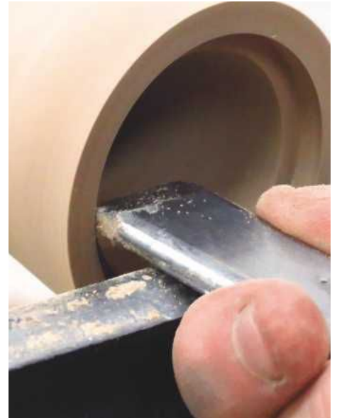
13 Cut a step at the entrance of the hole...
