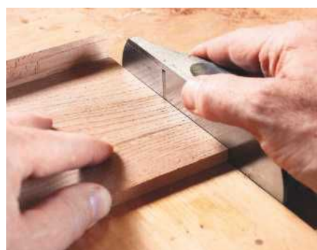
3 Using side two of the bench hook as a shooting board
