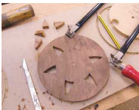
24 Cut the openings with a fret saw
