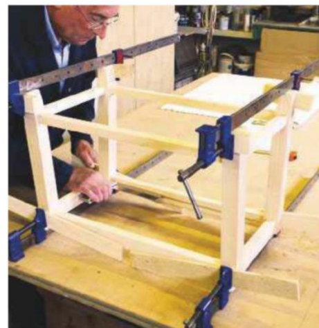
18 The frame in final assembly mode
