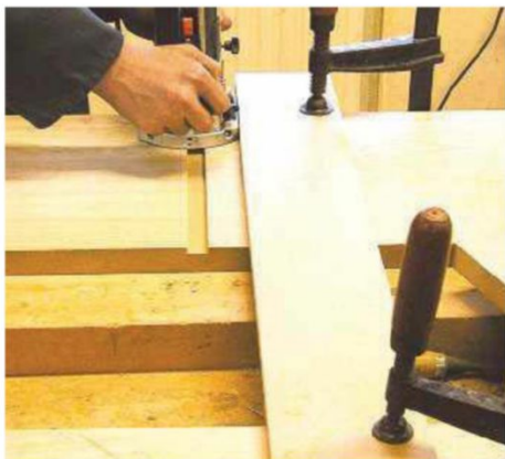
1 With the upright panels cut to size, rout the 7mm-deep shelf housings...
