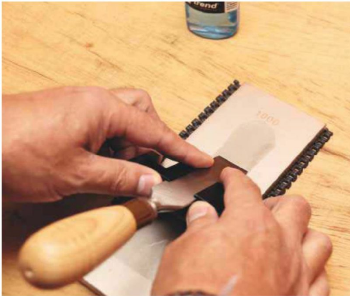
The wide roller on the guide keeps things very stable as you work on the stone
