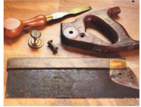
13 Disassembled for restoration
