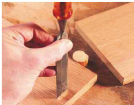
6 Deepening the line across the face of the board...
