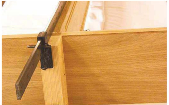
13 Assemble the carcass in stages, starting with the mid sections...
