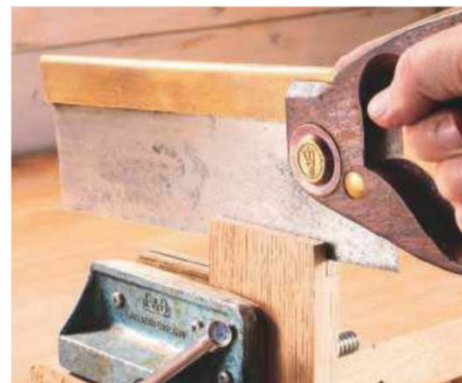
21 Sawing the floor of the rebate...
