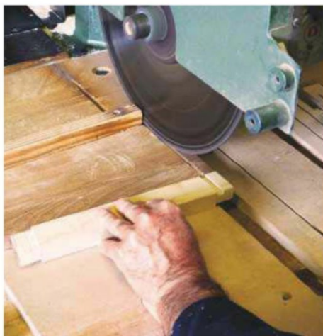
17 A jig is made to cut the angled shoulders
