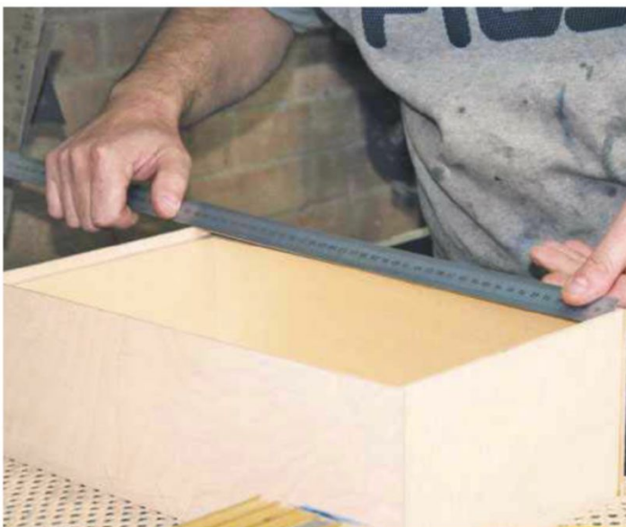
8 Measure from the box rim to make sure that the lid top will be a good fit
