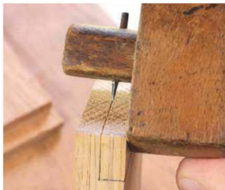
20 Continuing the line across the end-grain
