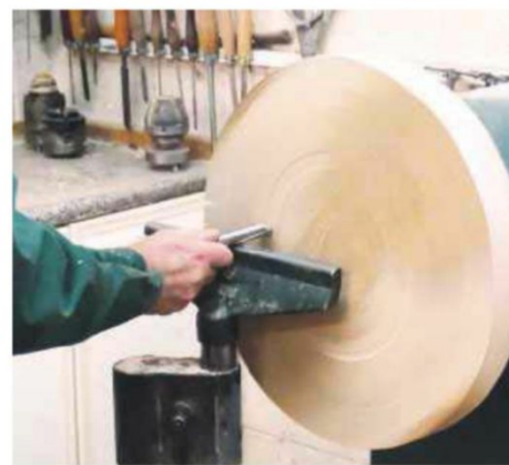
13 Mount your platter blank on the lathe and turn the back...
