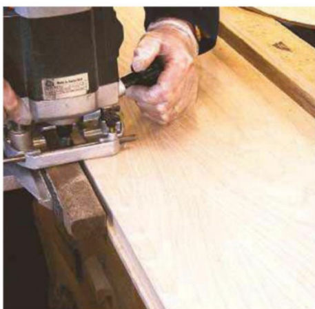
4 The back edge of the sides and top is rebated for the back panel
