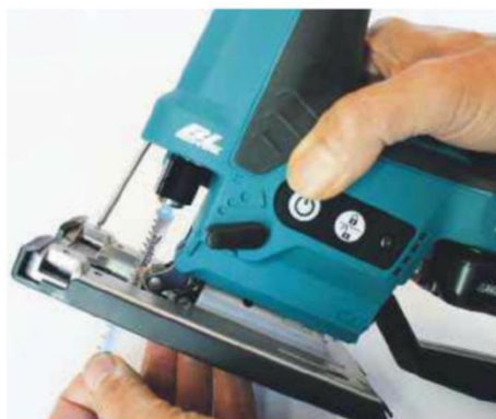
New blades are simply pushed into place with a click...
