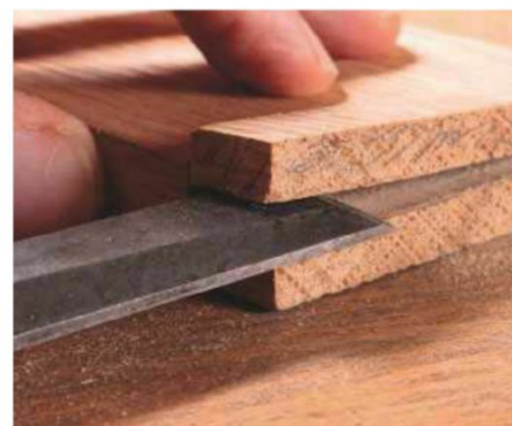
23 Breaking out the waste with a chisel
