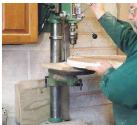
9 Drill holes through both discs around the circumference of the drawn circle
