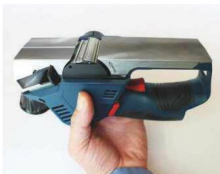
Accurate milling on the aluminium base ensures consistent accuracy
