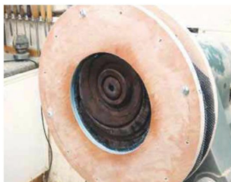
2 Wall plaques can be moved around between the two ply discs to any centre you want
