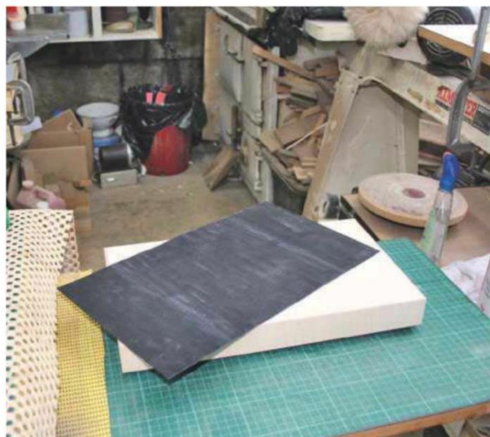
13 Double veneering the lid using a piece of black veneer with the grain running vertically prevents telegraphing
