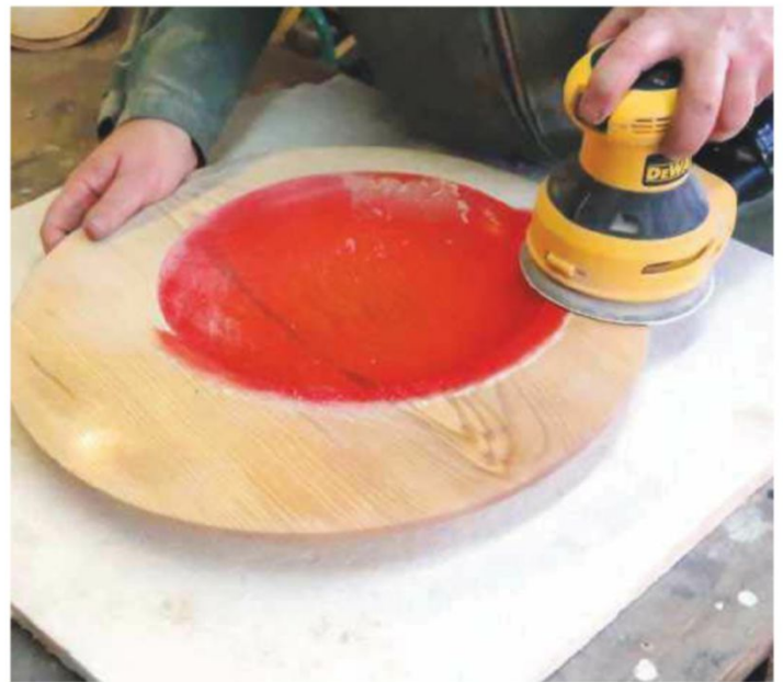
21 I used a random orbital sander to remove the paint overspray...
