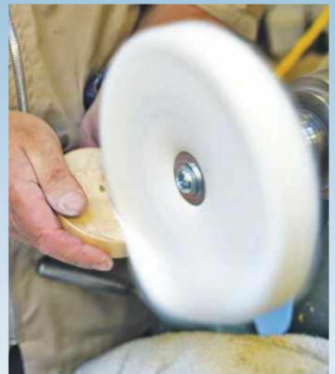
30 Sand through to 400 grit and buff to a shiny finish using the Beall or Chestnut three-stage buffing system, using tripoli and white diamond followed by carnauba wax
