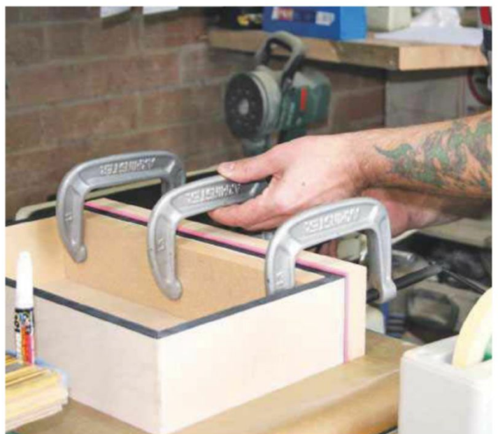
17 Attach four clamps to the positioned marquetry
