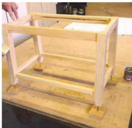
19 First sealing coat on the frame
