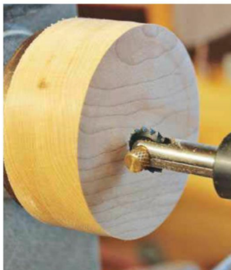
A flat on the sleeve sits on the toolrest, which delivers support and retains the correct angle
