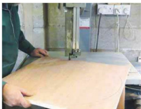
3 Cut two discs from 18mm ply on the bandsaw
