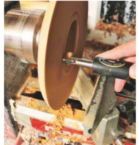
Working the face on this softer sapele gives fast results
