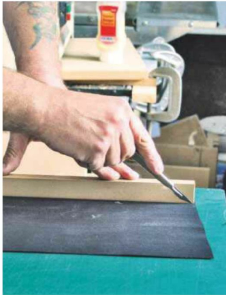
15 Cut the box inner lips with black veneer to about 0.5mm wider than the box thickness and 20mm longer than the length
