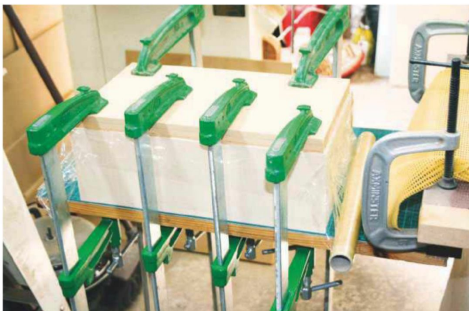
10 With glue on the inside corner of the lid, groove the lid and place under a pressure block held with clamps
