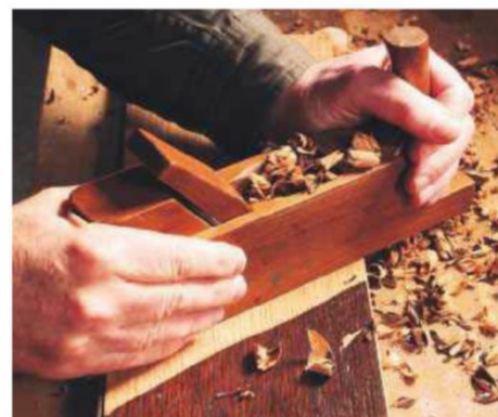
1 Stripping stained oak back to plain timber with the scrub plane
