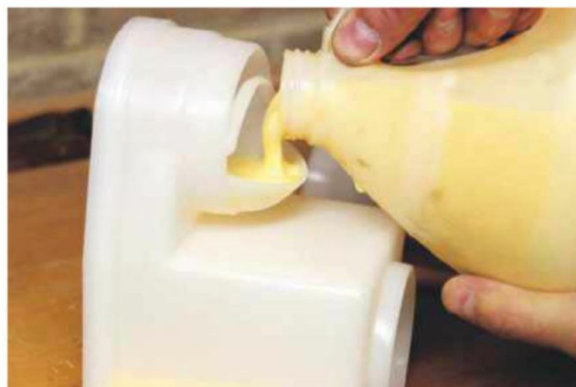
The glue container is tipped on its end to allow the glue to be poured in
