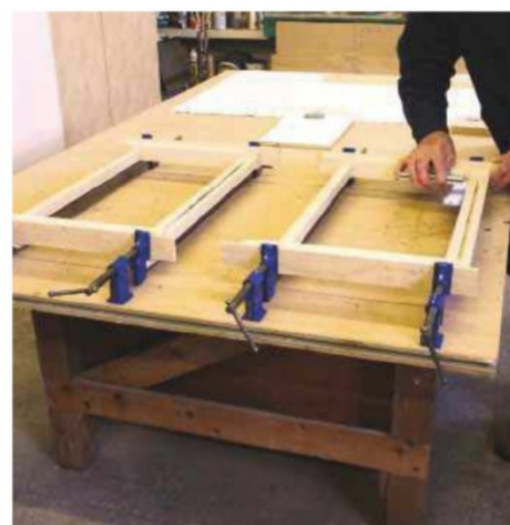
15 The first stage of the base frame construction
