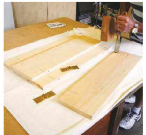
6 Cutting the edges of the hinge recesses
