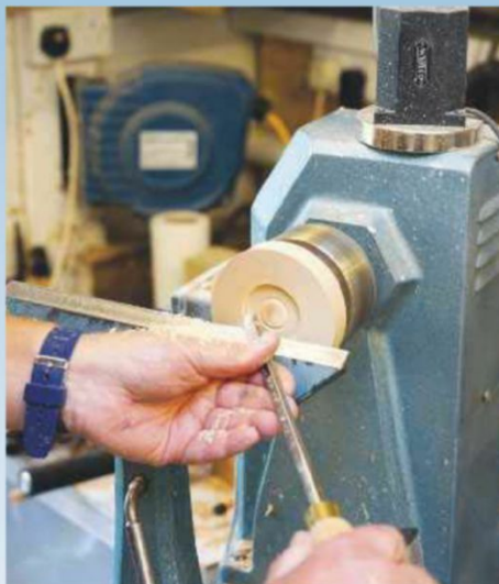
29 True up the base and cut a recess to chuck the piece, then true up the face and sides
