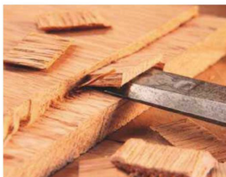
9 Removing wood in smaller bites near the depth line
