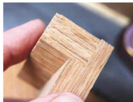
25 The sawn rebate is on a par with the chiselled one
