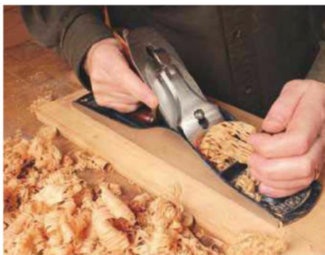
2 Smoothing away the scrub plane's furrows with the jack plane
