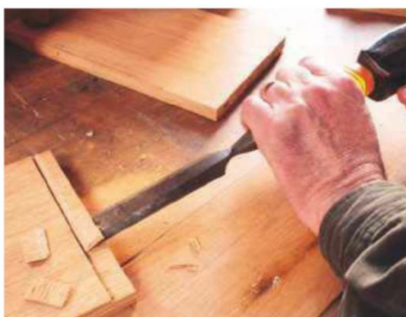
8 ... then splitting out the waste from the end of the board
