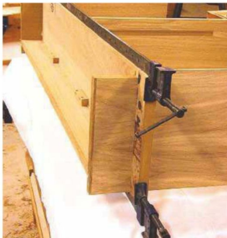
15 The bottom plinth is added before gluing up the sides; note the screw blocks reinforcing the plinth face
