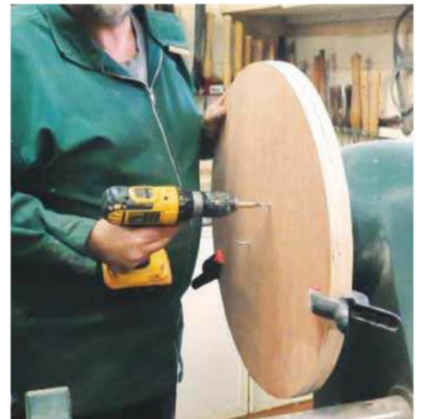
7 Mount on the lathe and temporarily screw the two discs together
