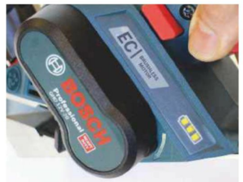
The battery indicator enables the user to know at a glance just how much working power remains
