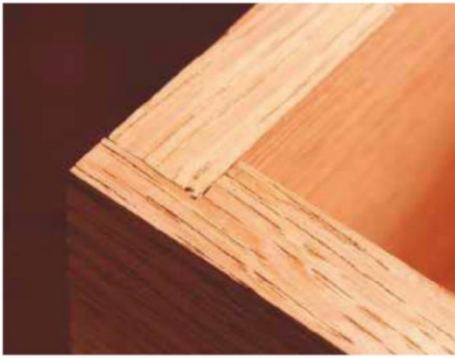
11 A fair fit for the chiselled rebate joint
