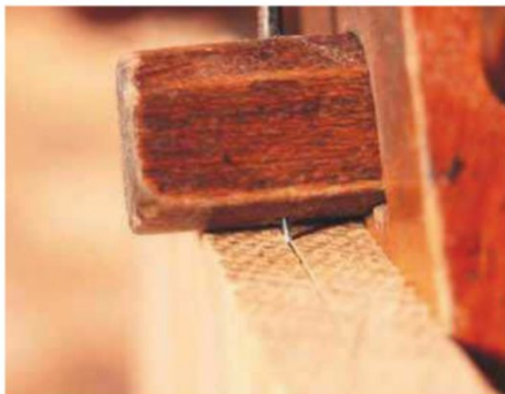
5 Using a marking gauge on the end of the board
