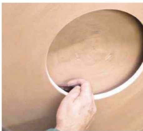
11 Soften the inside corner of the hole with abrasive
