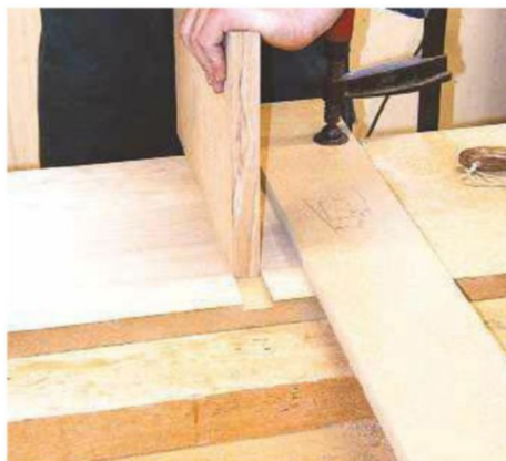
2 ... which should be a snug fit; note that the vertical divider housings are only 3mm deep
