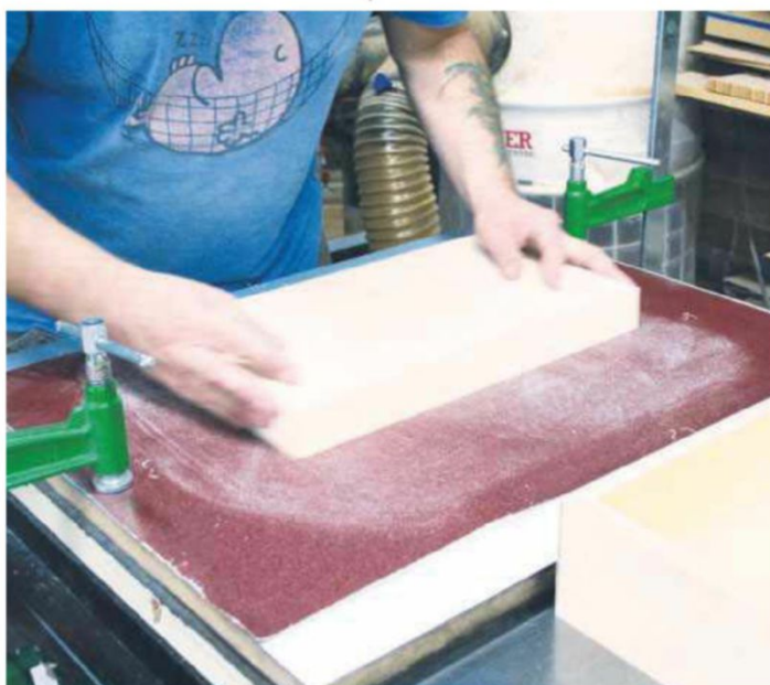
12 Remove the bandsaw marks using a sanding board. The lid should sit on the base with a nice join
