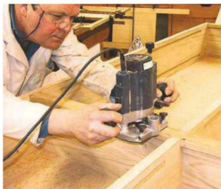
16 Run a router and chamfer bit carefully over all arrises to soften them a little
