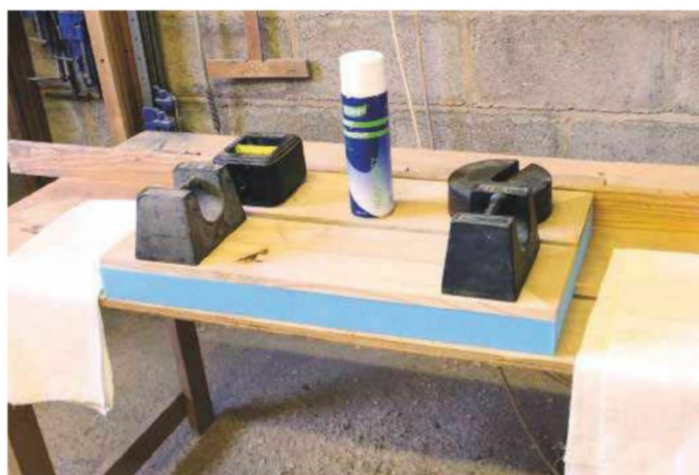
23 The foam is glued to the pad frames
