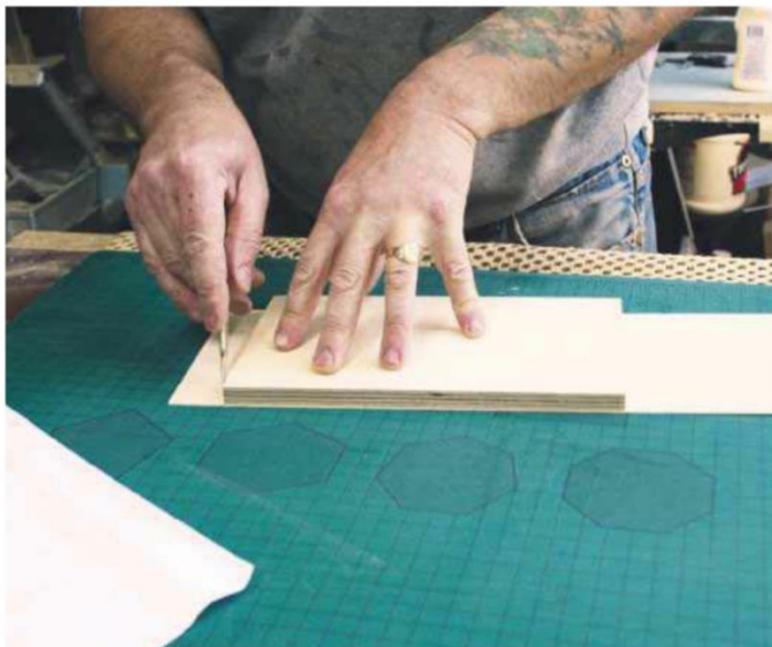
3 Arrange the box parts on top of the sycamore veneer and cut round with a scalpel
