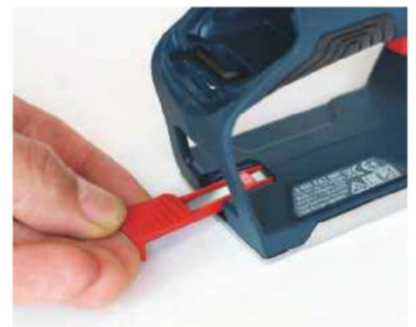
A spare blade can always be available – note hex key above in battery compartment
