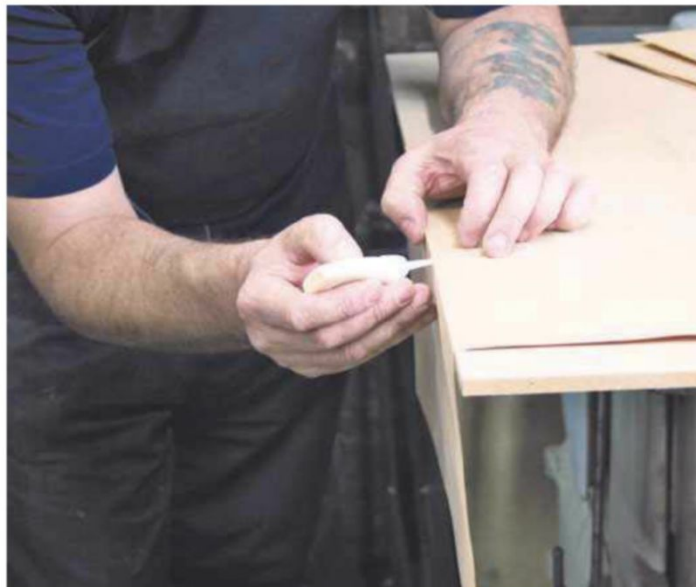
4 Tape up one side of the veneers, turn them over and open up the seam to add glue
