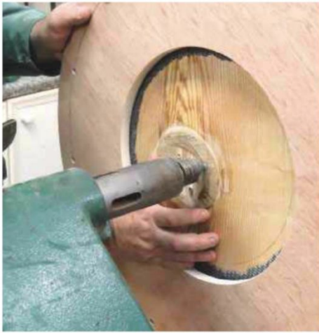
17 Sandwich the platter in the doughnut chuck and bring the tailstock up to the centre of the scribed circle. Tighten the four coach bolts
