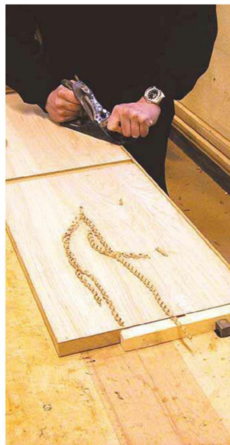
8 Clean up all lipped edges with a plane, scraper or sander, but take care not to cut through the veneer
