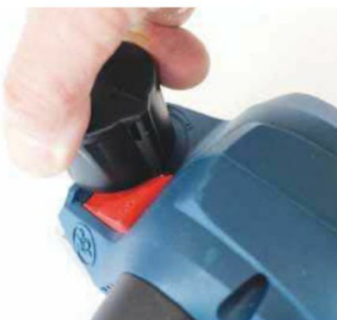
1st stop; depressing the 'Maximum' button will gain you an additional millimetre of cut
