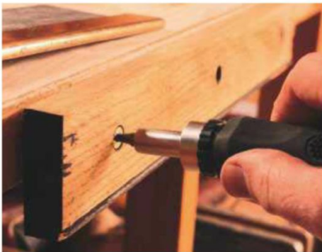
17 Adding an oak jaw to the bench to improvise a saw clamp
