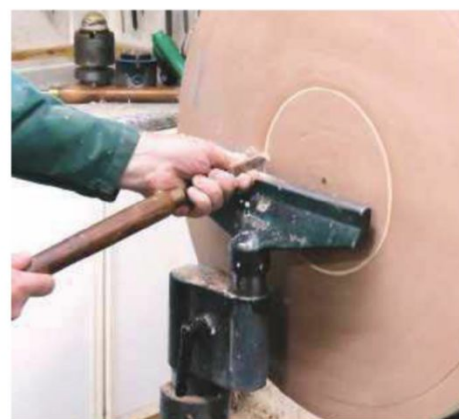
10 Remount on the lathe, sandwich spacers between the two discs and cut a circle out of one disc
