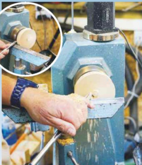
28 The last process is to take the 25mm piece parted off at the beginning and turn it into a base
