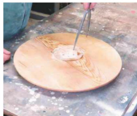
16 Scribe a circle for the bowl part, and clearly mark the centre of this circle
