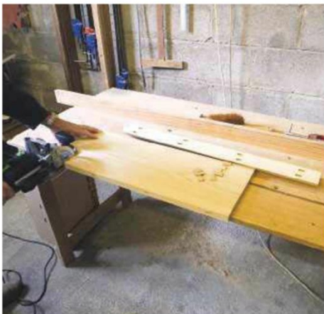
4 Domino jointing the top
