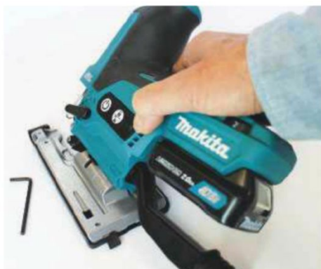
The base pivots for bevels – note on-board hex key
