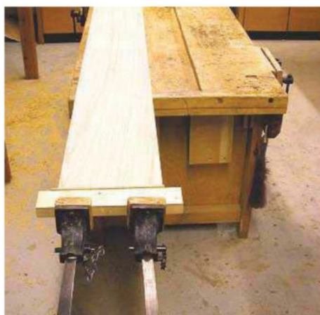
5 The top and bottom edges should be lipped first...
