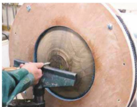
1 The setup for removing the chucking point
