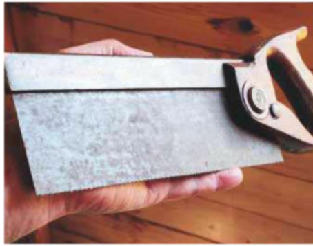
12 The S & J tenon saw as found, with blunt and rusty blade
