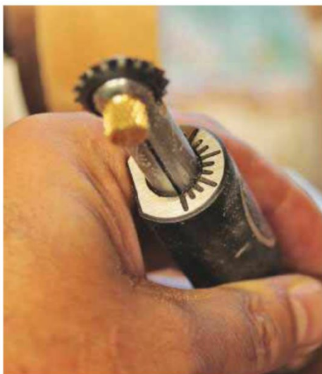
The sleeve rotates to register against the cursor mark on the tool shaft
