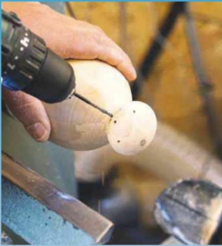
19 Use a bradawl to mark holes and drill for the eyes and mouth using a 3mm drill bit...
