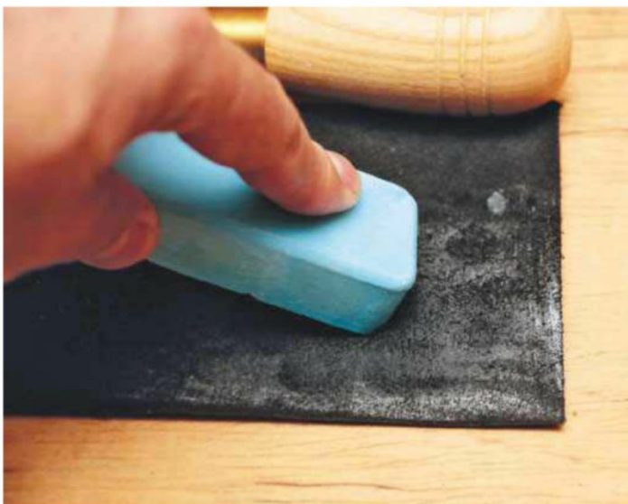
The honing compound is quite hard and chalky when applied to the leather
