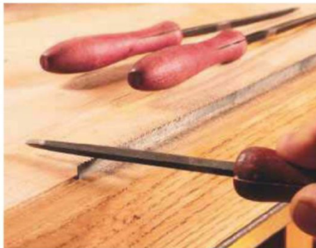
18 Sharpening the rip teeth with a triangular saw file
