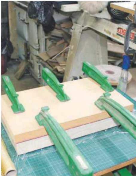
14 Roll some glue onto the lid and press the veneer firmly before adding the foam, 18mm MDF and clamping up
