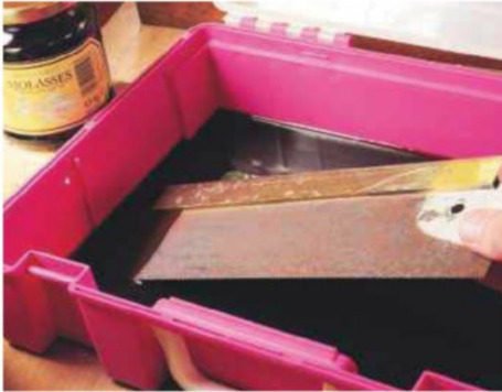
14 Bath time for the blade, with Sellotape protecting the brass
