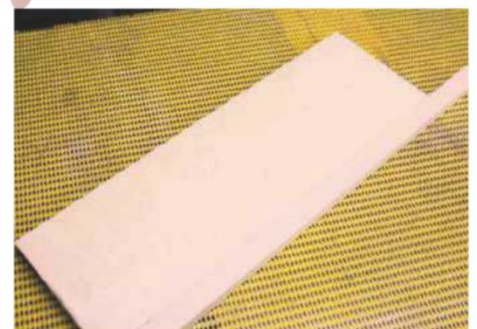
1 Substrate sandwich: sycamore was added to birch plywood to create the base edge
