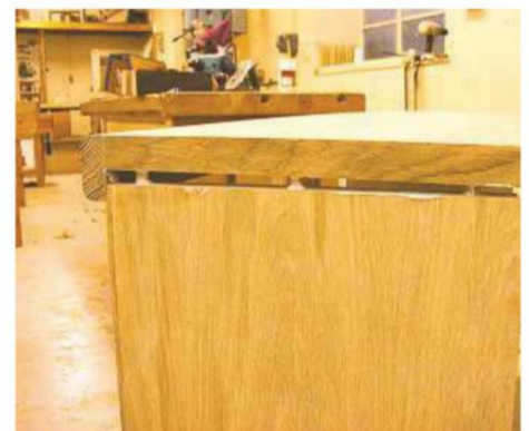
17 The lower units should be sized to allow the top to sit on the uprights rather than between them
