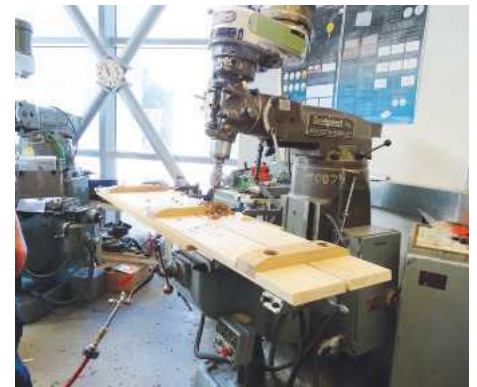
16 Drilling the circular mortises for the legs on the long bench
