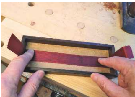
16 The ribbon was glued to the bottom before the lining. To guard against fraying, seal the cut ends by looping them back
