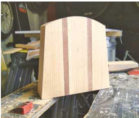
5 The top's corners were sawn off, and the curve perfected with a rasp, spokeshave and file
