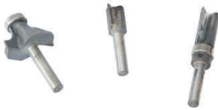
5 I used a template-following straight 1/2in cutter with a top bearing to reproduce the template's outline
