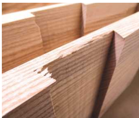
9 Breakout from the CNC router...
