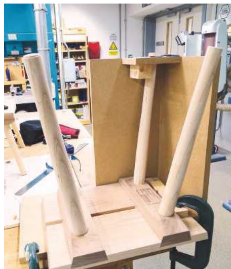
20 The leg-levelling jig; just add flush saw
