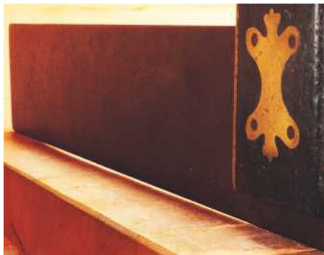
2 The try square exposes severe cupping in the block-built surface
