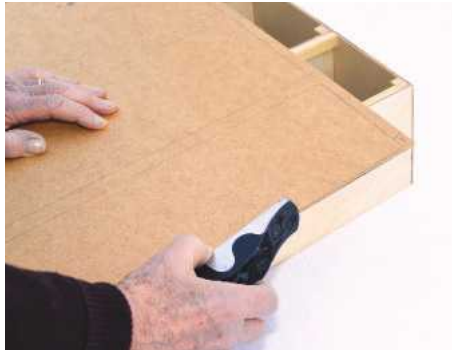
11 Measure the back panel accurately, cut slightly oversize and plane or sand to fit into the rebates. I used 3mm MDF here – the plan was to cover one side with card and to paint the other side
