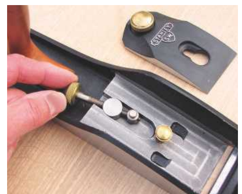
The traditional Norris-pattern lateral blade adjuster
