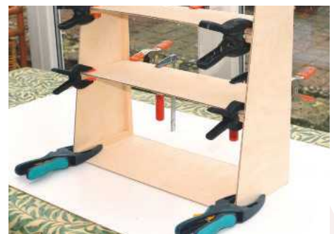
9 Glue the shelves to the shelf supports at the back and sides and insert the top panel into the rebate. Plenty of cramps are useful as always! Cut stripwood to fit the front of each shelf and glue to the top surface to form a ledge
