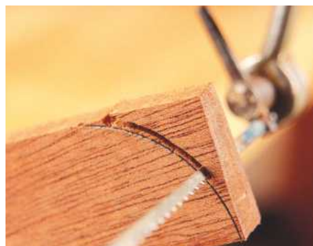
21 Cutting away waste with the coping saw
