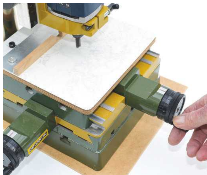
2 I made a false table from an offcut of Formica laminate with an adjustable fence
