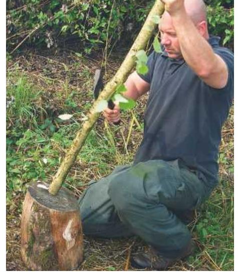
3 Roughing out a stave
