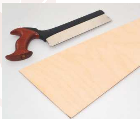
2 Use Fig.1 and mark out the sides, top and bottom, shelves and back on the plywood sheets. Cut out the pieces with a fine-tooth saw but leave the back panel at this stage so that it can be cut exactly to fit at the final stage where slight adjustments may need to be made
