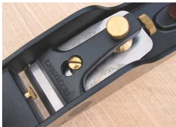
The aluminium lever cap is a snug fit and fast to tighten
