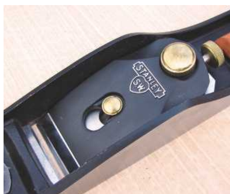
Made from aluminium, the lever cap is incredibly light
