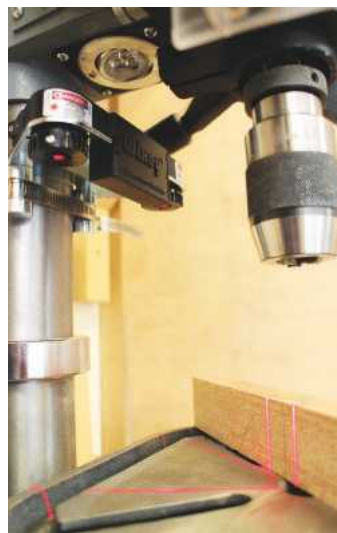
Calibrating the laser lines to plumb. Note proximity of drill press worklight
