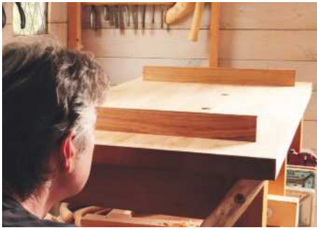
12 Sighting between winding sticks to check for twist
