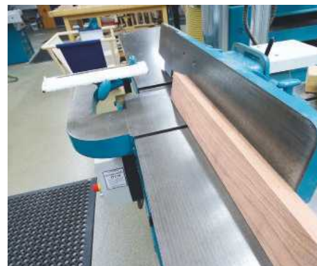
8 Tidying the sawn bevels on the overhand planer (Wadkin refurb)
