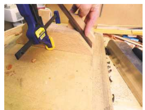
14 The timber is held at precisely 45° to the plane and 90° against the fence
