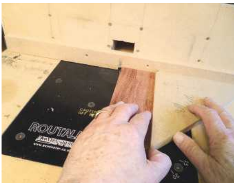
1 Bare-faced tenons were cut at the router table using a simple 90° guide
