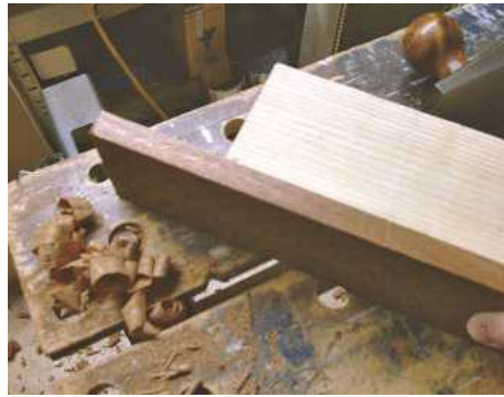
3 The laminae of ash and sapele were fixed together with Gorilla glue, which I find reliable and easy to use
