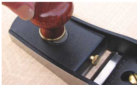
You slacken off the knob to slide the throat plate back
