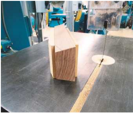
11 Jig to hold the dovetail profile rails...
