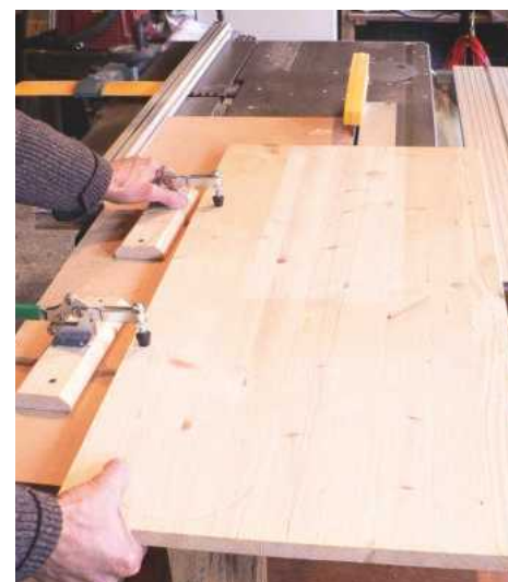
3 A taper jig was used on a table saw to cut the end plates' shape
