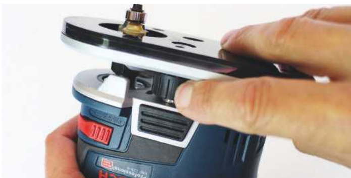
Adjusting the fine tuner, the lock is on the other side
