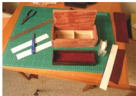
19 With the ash linings in place, the leather trim was folded over card and added
