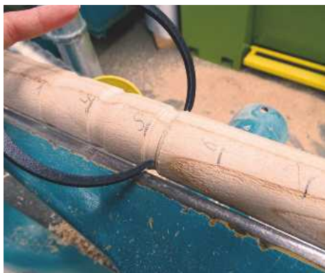
6 Developing the tapered legs with the aid of jig-marks and turning callipers
