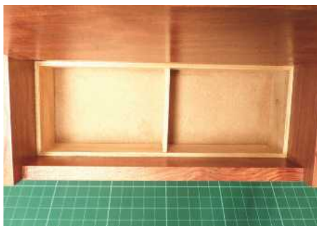
18 The 3mm ash linings were shot to a push-fit, mitred at the corners and half-lapped in the middle
