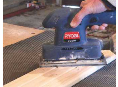
11 Three rails were sanded together with 120, 180, and 240 grit abrasive pads
