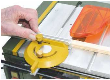
4 Cut the stripwood into 12 x 15mm sections and then into the lengths as shown in Fig.2
