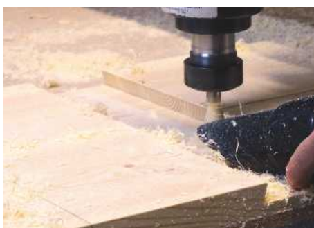
4 The CNC router at work on the dovetail grooves
