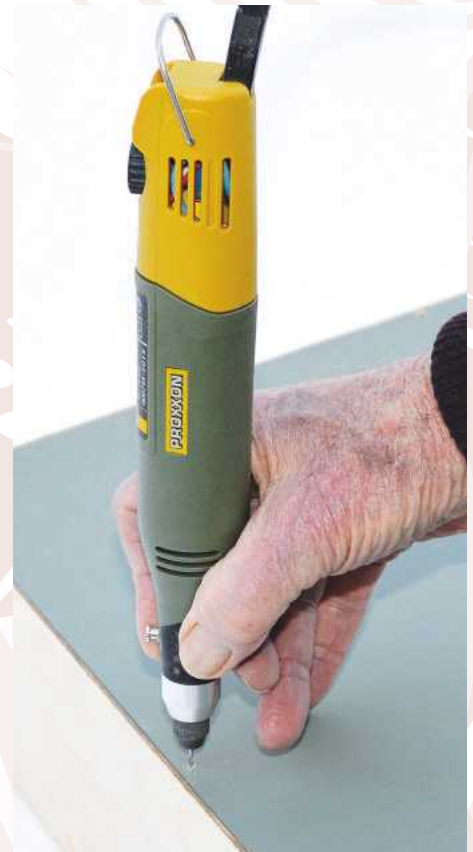
13 The back panel is finally screwed into position with six small short screws. Make sure the screw tips do not protrude
