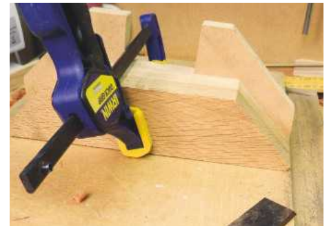
13 Made from scraps, the bird-house jig looks rough and ready but is actually a precision tool for jobs like trimming the mitres on the lift-out tray
