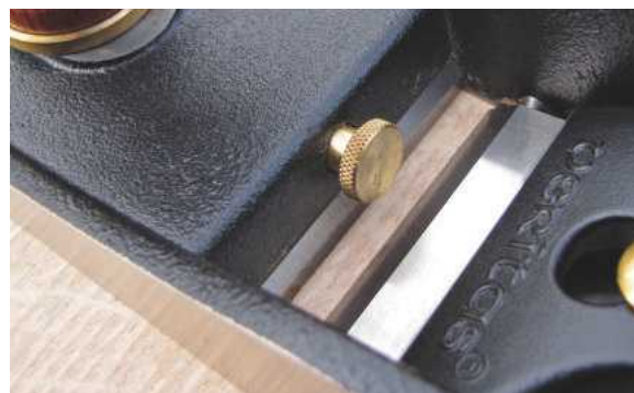
Rotating this screw prevents the plate from hitting the blade
