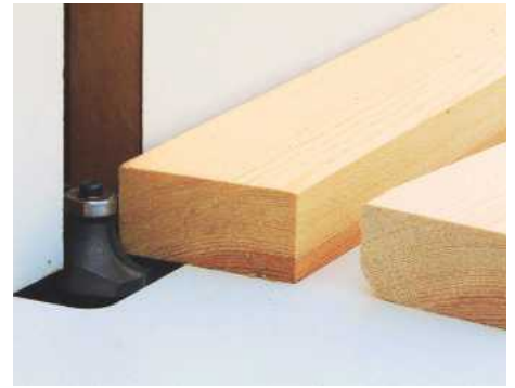
6 The outer edges were rounded with a 3in round-over cutter with top bearing in the router table
