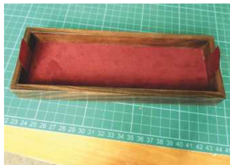
17 The finished tray with its card-backed leather trim, which matches the bottom of the box
