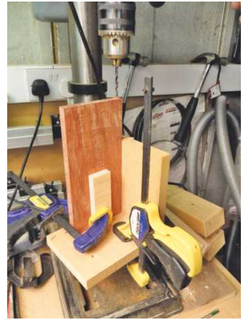
9 Everything was clamped in position and then double-checked before drilling commenced
