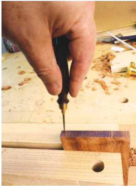
8 After plotting with the gauge a deeper mark was made with an awl to locate the brad-point bit
