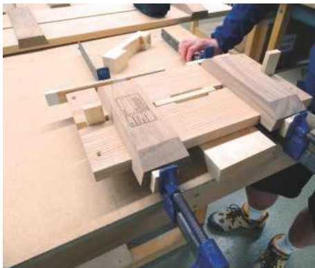
14 Cramping the job together, note various blocks and spacers
