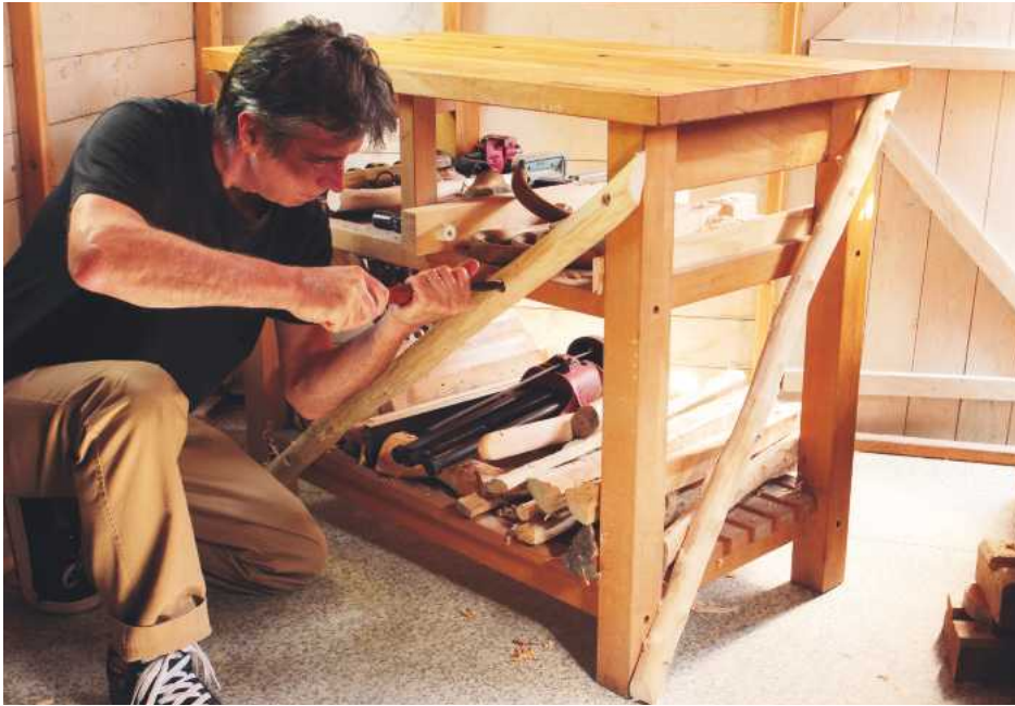
15 Fitting rustic ash and maple diagonals to cure racking
