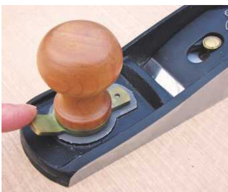
The substantial brass lever for closing the mouth
