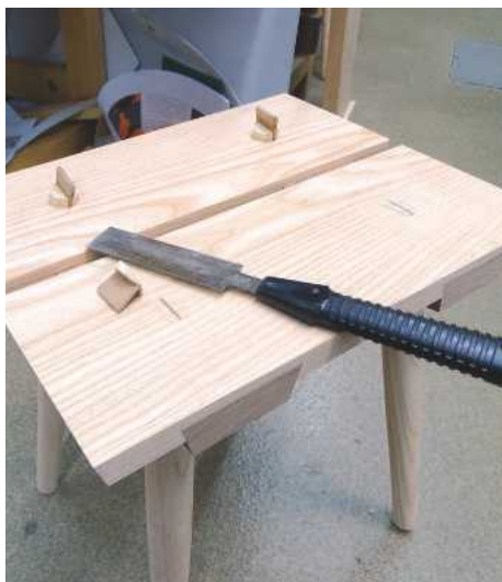
19 Trimming the tenon ends
