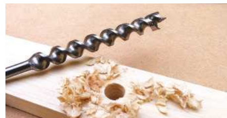
Hole drilled using a Jennings bit
