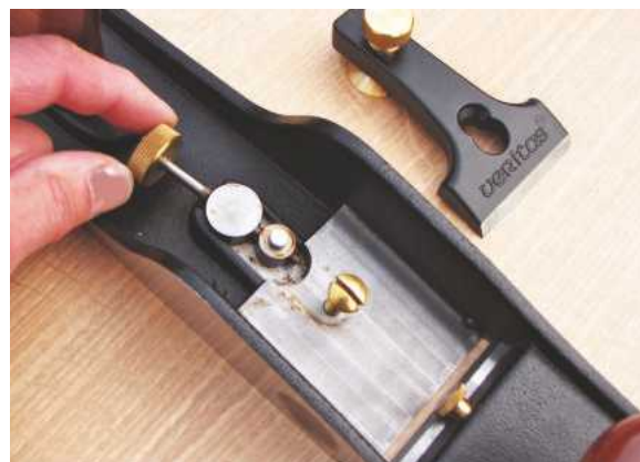
This is the best lateral adjuster mechanism of the lot
