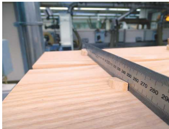
18 Aligning the wedges with a steel straightedge
