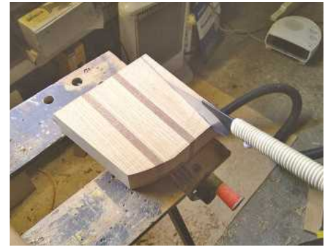
4 To remove the waste from the bevelled front and back, I used a saw followed by a plane to refine the shape of the block
