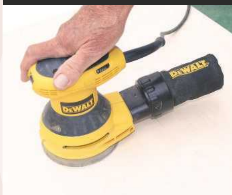
1 It is worth taking the trouble to orbitally sand both sides of the plywood sheet first, so that you have a very smooth surface to start with
