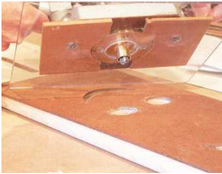
4 The finished curve was created using a template with the router
