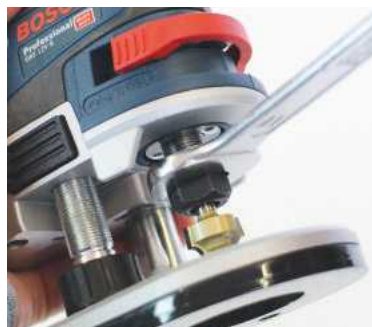
Tightening a bit in the collet
