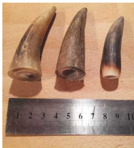
8 The stages of horn nock production (from left to right) – the cut off tip drilled with a cone, worked down, and awaiting polishing and grooves
