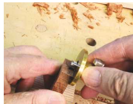
6 Using an offcut, a gauge was precisely centred for positioning the pin holes in the lid
