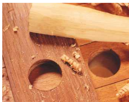
23 The planing stop is anchored by an ash peg
