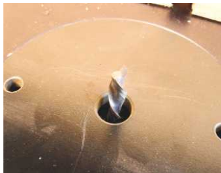
2 Use of a down-cut spiral bit in the router table produced a nice clean shoulder
