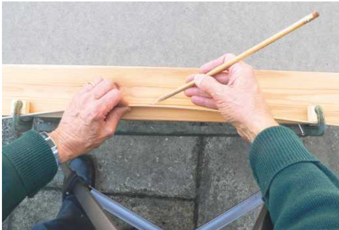
7 The bottom curve was drawn out with a slat and clamp...
