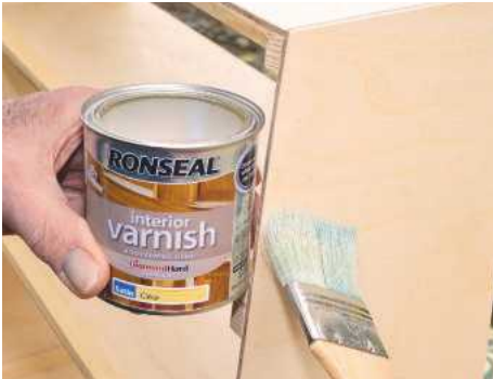
10 Apply at least two coats of clear satin varnish, rubbing down between coats
