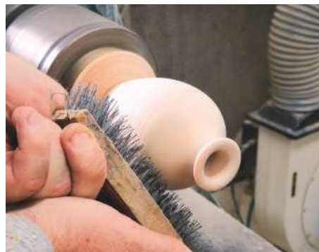
14 Use a stiff wire brush to scratch the wood and remove the softer growth
