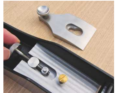
A Norris-style adjuster provides lateral movement
