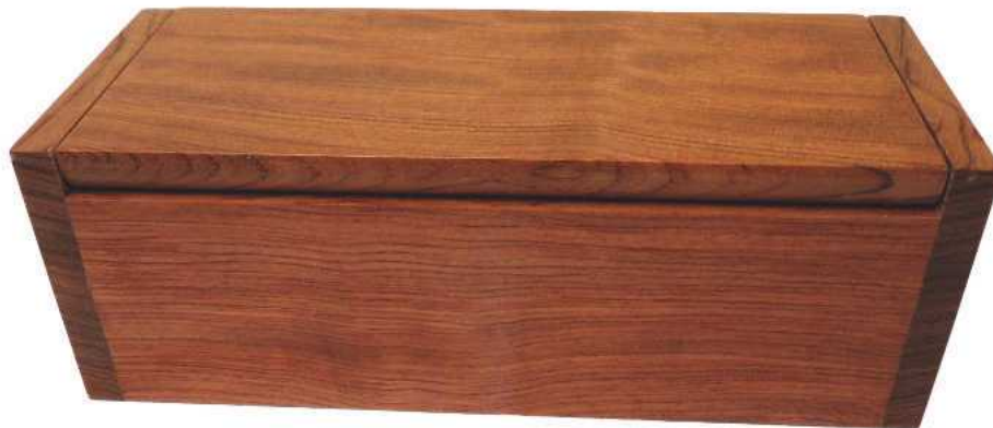
12 Rear view showing relieved rear edge to the lid, which allows easy movement
