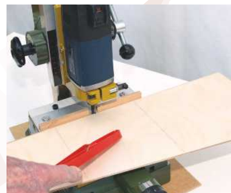
3 Rout 3 x 1.5mm deep rebates along the top, bottom and back edges of the two sides and along the back and sides of the top and bottom pieces. Using a router to form a rebate produces a neat, accurate joint but it is not essential and if you don't have a router, then you can use stripwood to form the rebates
