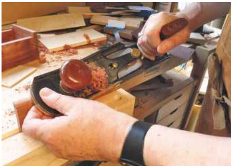
10 To allow the lid to open, the underside of the rear edge must be rounded so that the lid will lean backwards and stay open
