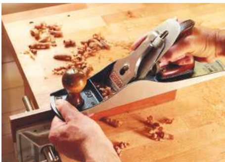
16 Set fine, the Record 5 1/2 straightens an edge for the planing stop
