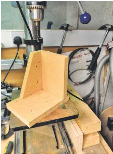
7 This simple jig held the lid at precisely 90° in both planes for a perfectly aligned hole
