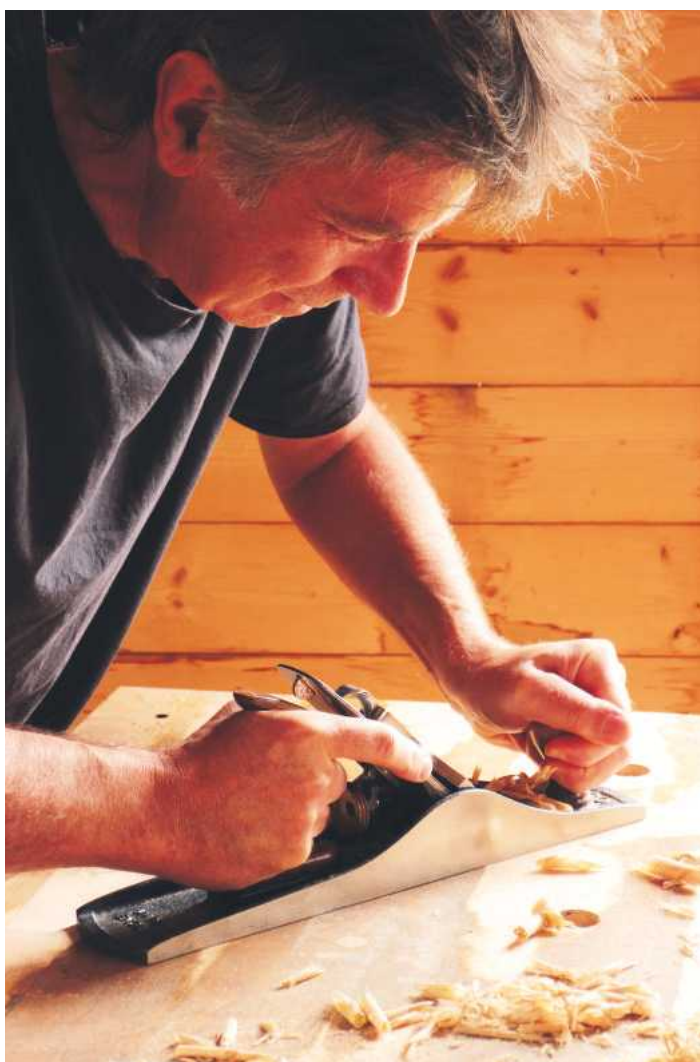
7 Working across the surface at 45° with the Record 5½...
