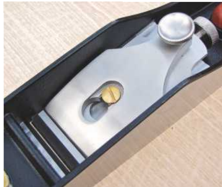
Unlike the other planes, this lever cap is stainless steel
