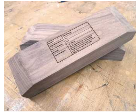
13 Information block lasered onto the underside of a seat component
