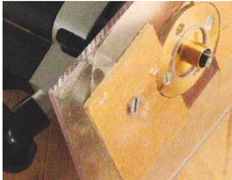
10 A 1/2in straight cutter in a bushing was used against the running board of the jig
