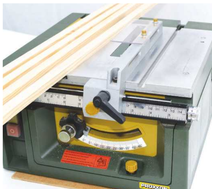
3 The Proxxon FET table saw is extremely useful for cutting small pieces of wood accurately
