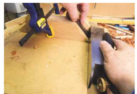
15 The Macassar ebony was mitred for the lift-out tray using a No.9 plane. If using an ordinary jack, ensure that the cutter sits square to the sides
