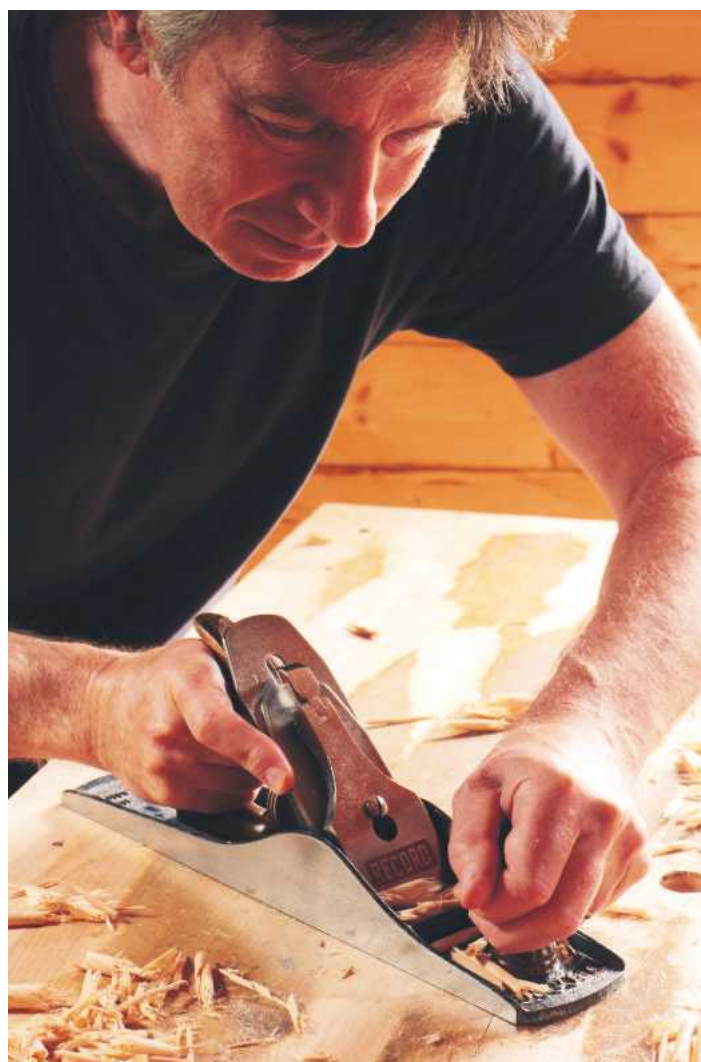
8 ... and again at 90° to the first pass
