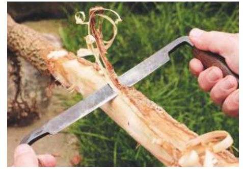
14 Barking a maple pole with the drawknife to brace the bench
