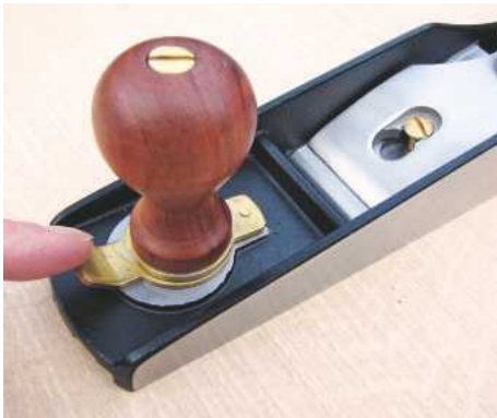
The Quangsheng's mouth is set with this brass lever
