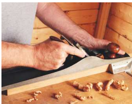
5 Straightening the edge of an oak straightedge with the jointer
