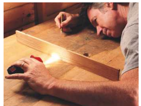
6 Shining a torch behind the straightedge to expose the ups and downs
