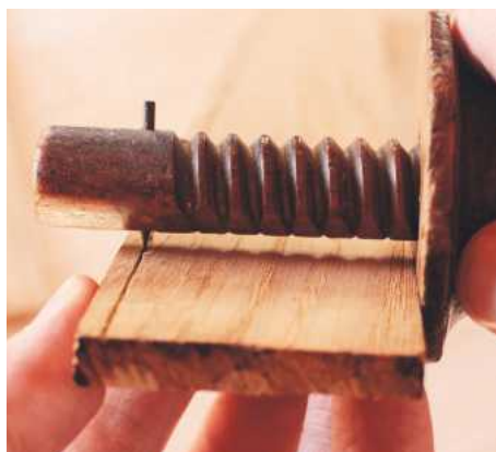
11 Scribing a sight line to make a winding stick
