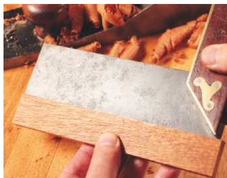
19 Checking the edge of the fence is square
