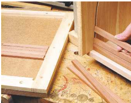
10 Try the slats in the carcass to ensure they run smoothly; chamfer the tongue edges if necessary
