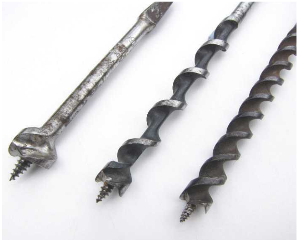
6 From left to right: centre bit, auger bit, Jennings pattern bit
