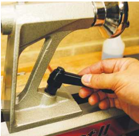
A well-positioned lock makes tailstock adjustments very easy
