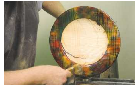
4 Don't overwork the sanding sealer as it will lift the colour off
