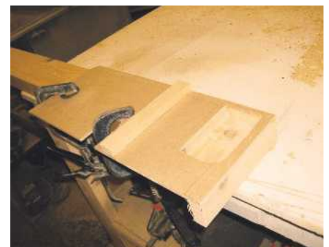
3 Because the rails were so long I made a jig to assist in cutting the tenons
