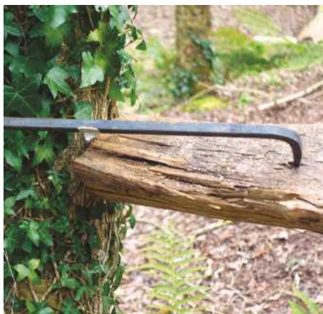
A steel dog stapling the baulk to a tree
