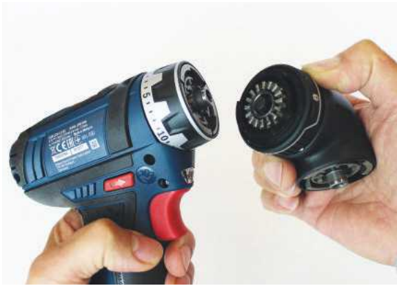
The two parts simply push together and twist to lock with a satisfying 'click'
