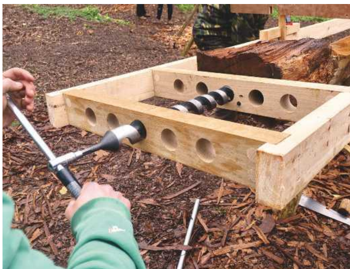
Jig with auger at work
