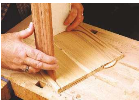
16 Try the completed tambour assembly in its grooves to ensure they all run smoothly
