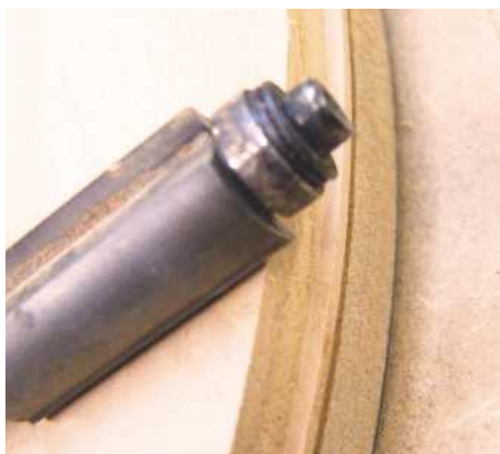
9 The smaller bearing makes a neat rebate
