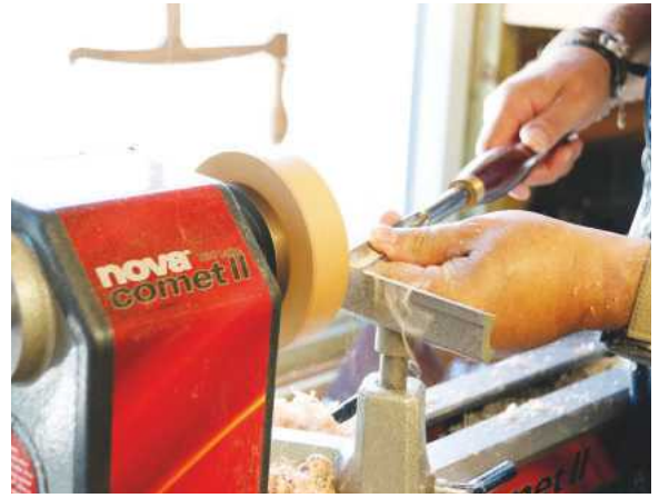
Working the interiors of bowls is easier with the tailstock removed
