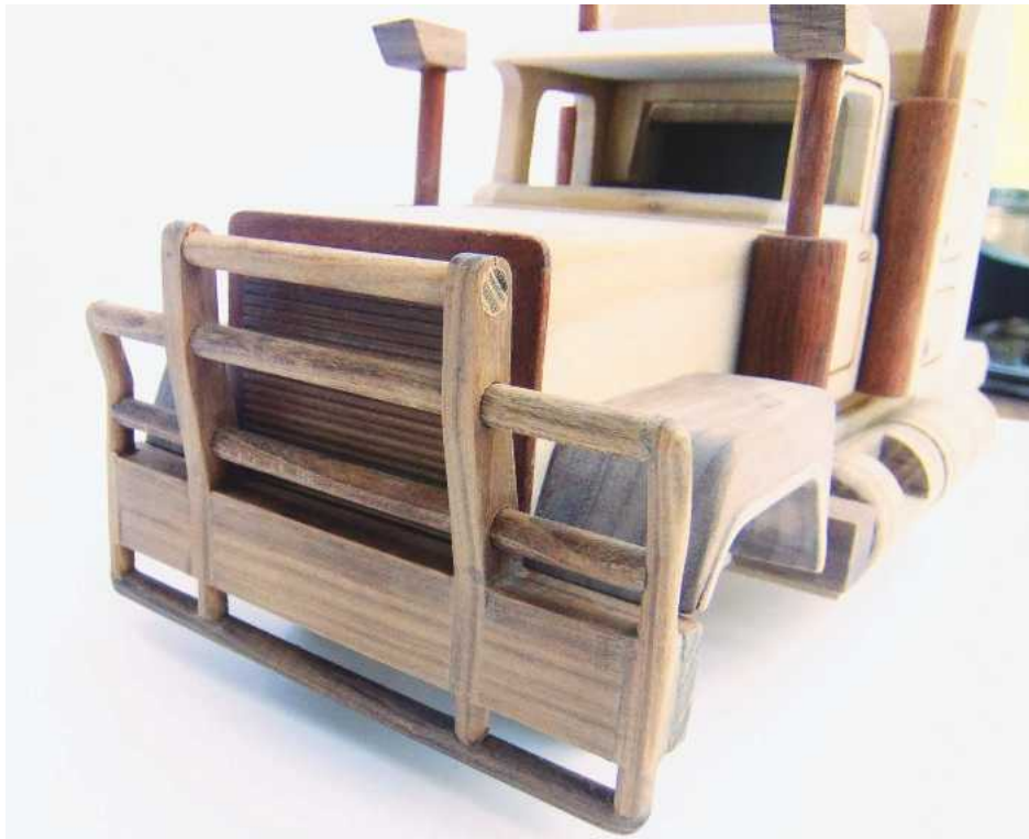
30 The front bumper is held in place with double-sided tape, so it can be easily removed for finishing later on
