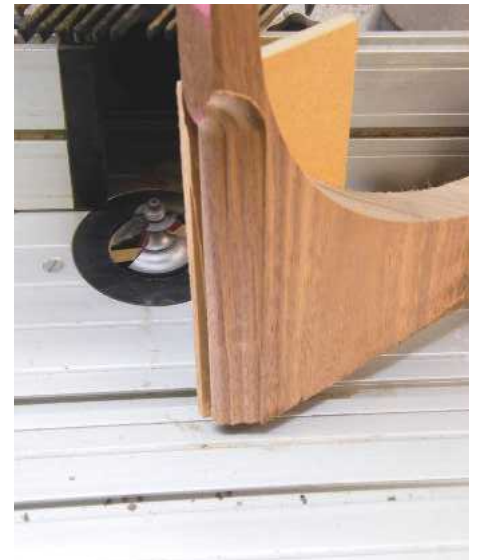
16 Check the depth of cut on some scrap of the same thickness
