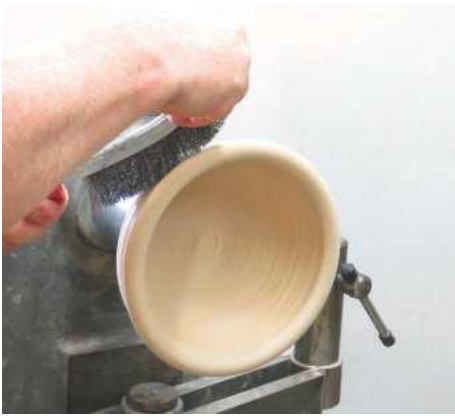
12 Use a stiff wire brush to texture the surface...
