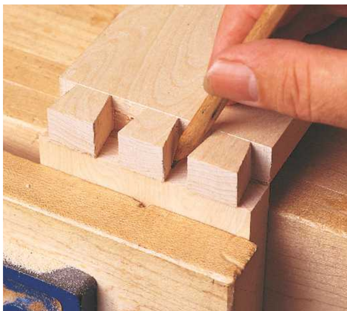
10 The pins are traced directly from the tails with a fine pencil. Hold the pieces firmly together, with the shoulder line for the tails accurately aligned with the rear edge of the lower timber, and the sides flush and square with each other. Be sure to cut to the correct side of the lines or the joint will be slack
