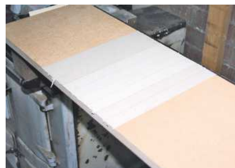
1 The surface of your sanding board needs to be absolutely flat; I shimmed this MDF board for the job
