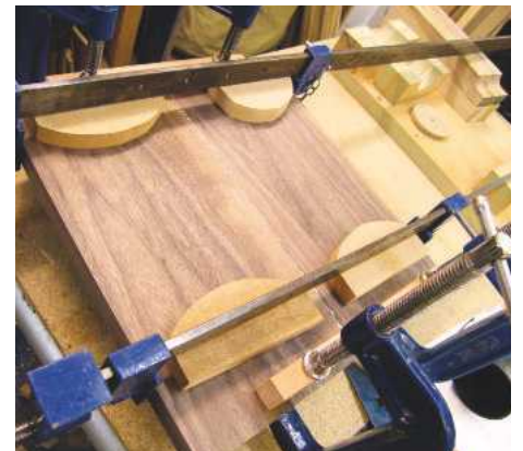
2 Note the scrap to keep the sash cramps level with the timber
