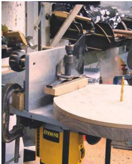
15 Note the use of the hold down clamp on the small table top
