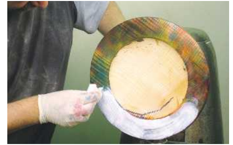
7 Rub liming wax into the opened up grain...
