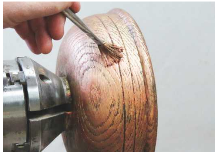
16 I use a glue brush to paint on the different metal acrylic paints...
