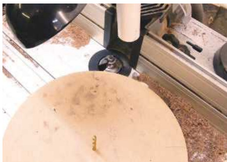
17 Note the lead on pin for added support (the safety guard has been raised for photographic clarity)
