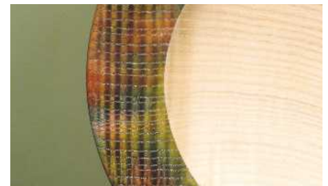
10 If it was sealed properly then the overspill will not have penetrated the wood
