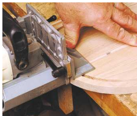
5 I used biscuits to joint the carcass of my bread bin
