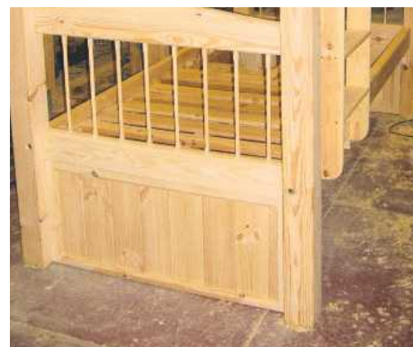
21 End panels were fitted to the bottom bunk to enclose the bottom
