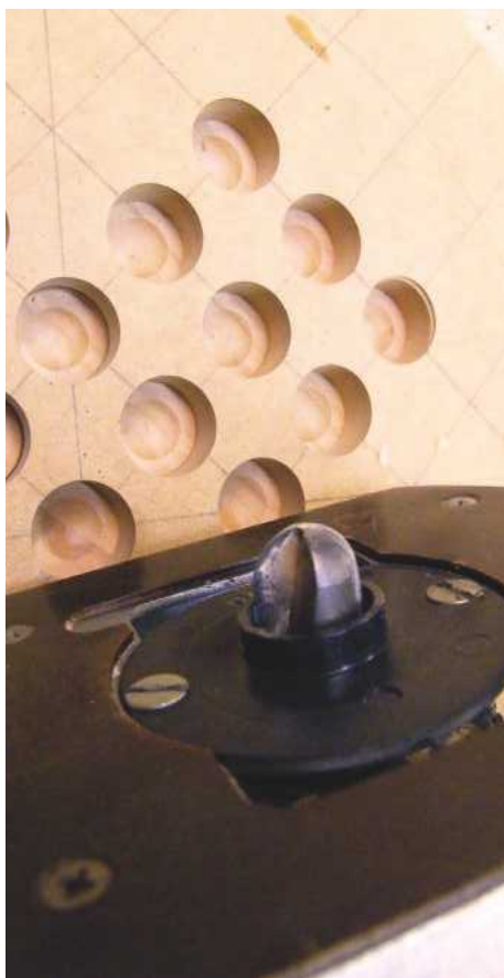
10 Use a 20mm guide bush to match the hole in the template
