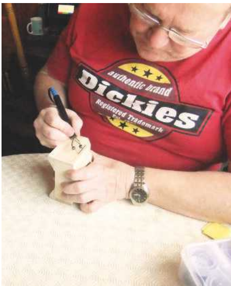
17 Using a pyrography machine to add door detail to the cab and sleeper cab
