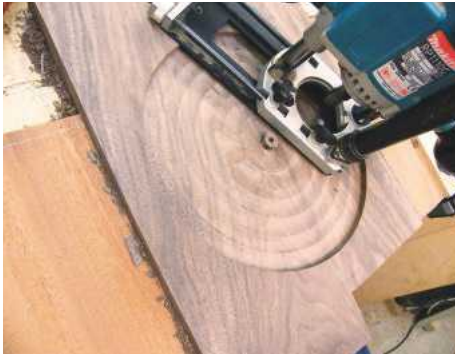
12 Gradually reduce the radius of the jig
