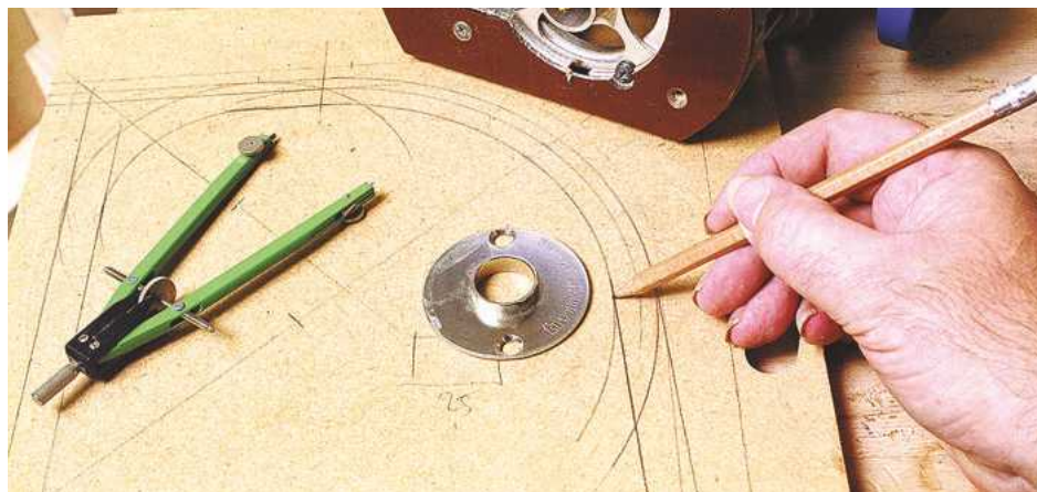
1 Determine the sizes and draw up a full-sized MDF template, taking into account your guide bush/cutter ratio
