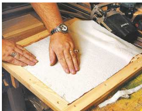
14 Cut the calico backing to size and smooth into place over the slats; a veneer roller will help when doing this
