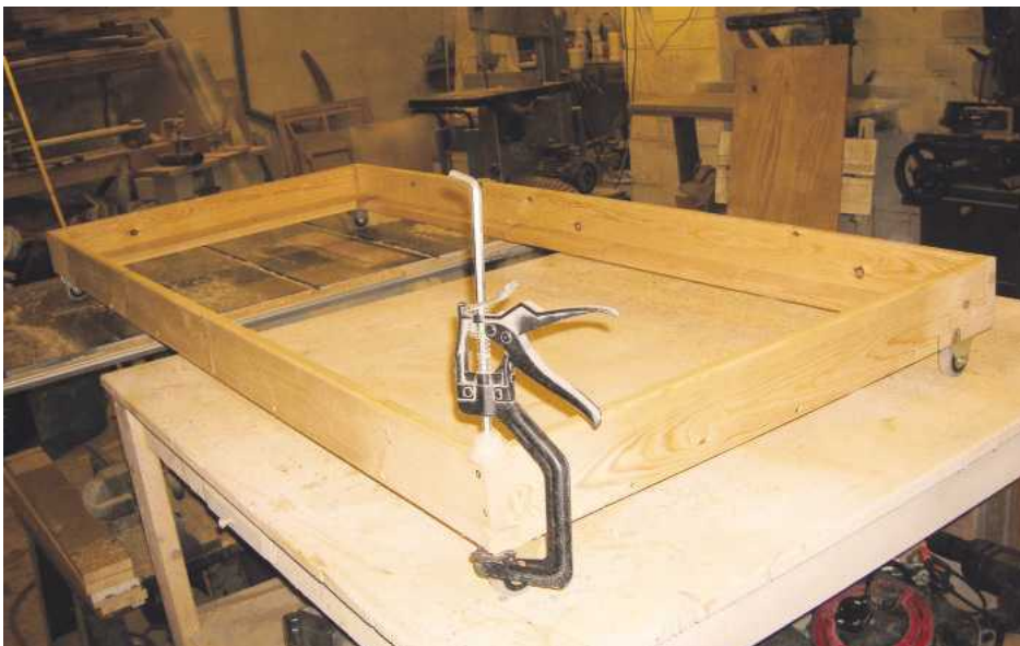
24 The pull-out out frame was built from four pieces of timber and fitted with wheels...
