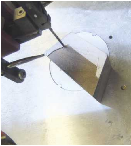
15 Cutting out one of the mud guards with a template in place
