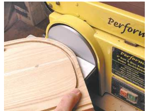
12 ... then cut and sand to shape on a disc sander, taking care not to scorch the edges
