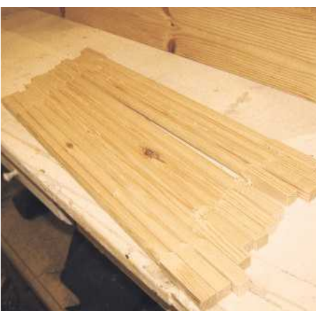
7 The centre sections of the spindles were shaped with a router
