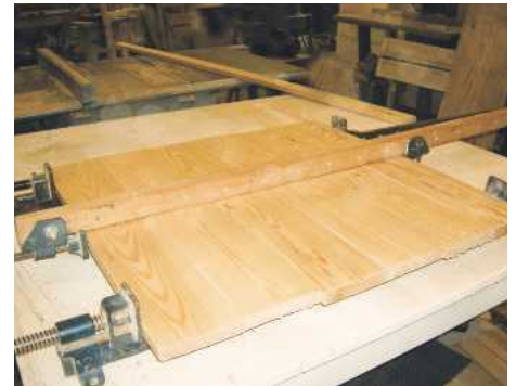
29 Laminated timber for the drawer fronts was left in clamps
