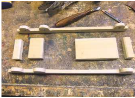
1 The two chassis members, the spacers marked out and cut to size, and the axle holes marked and drilled
