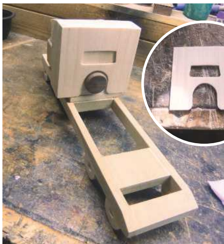
8 The back plate and tank are both turned from pieces of walnut
