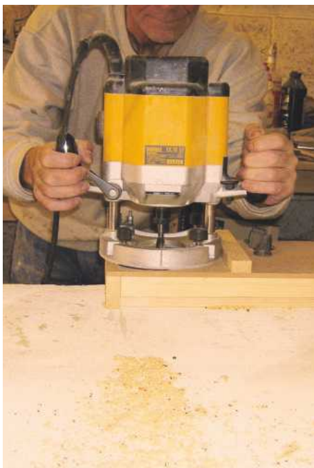
4 This jig provided a firm base for use of the hand-held router
