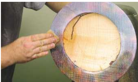
8 ... then remove the excess using Danish oil on a paper towel
