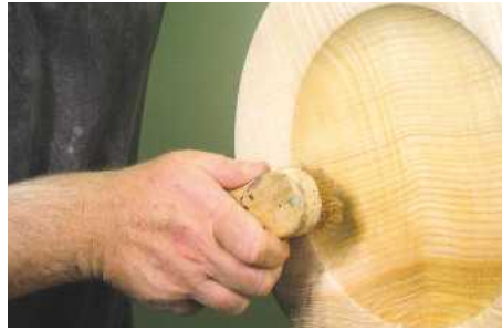
6 Use a small bronze brush to pick out the softer areas of grain
