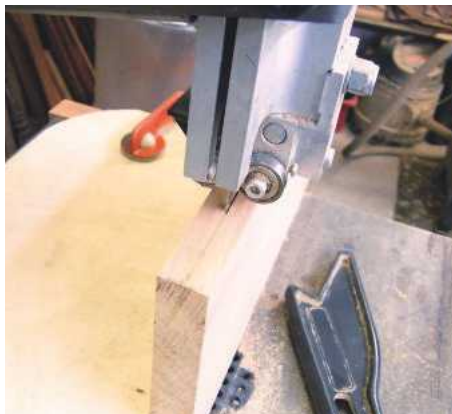
1 Cutting the 25mm board to make two 10mm boards
