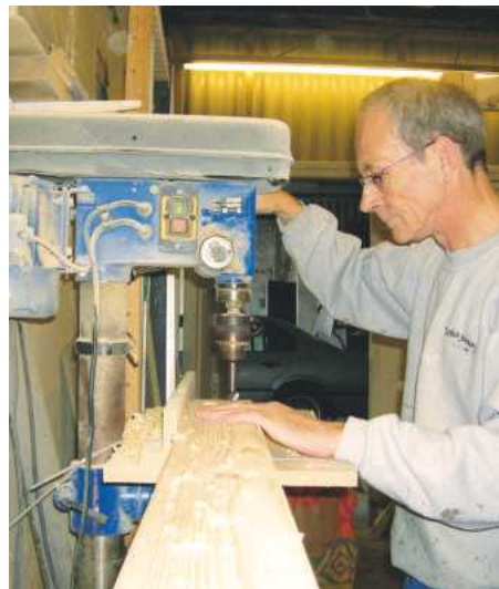
14 Pockets were cut into each of the side rails with a Forstner bit in the pillar drill...
