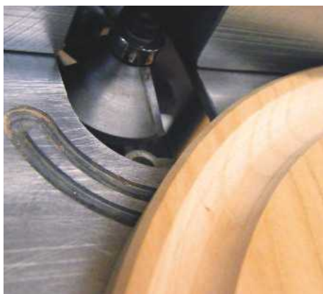
8 Cut the 2mm bevel around the perimeter of the circle
