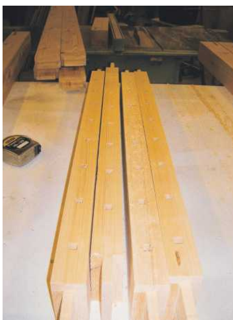
8 Spindle holes were cut with a mortiser in the head and footboard rails
