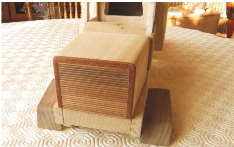
14 The small dowels glued in place to form the grill
