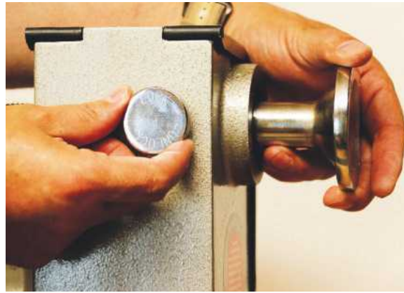
You lock the pulley wheel by pulling out and rotating this disc
