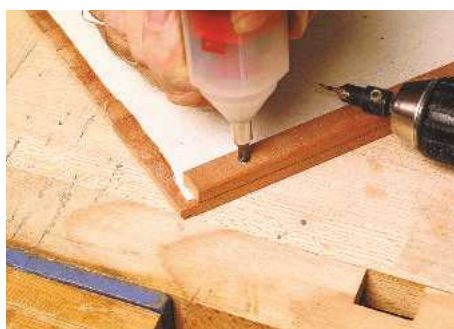
17 Screw a backing plate to the bottom slat to sandwich the backing fabric and prevent it coming unstuck in use
