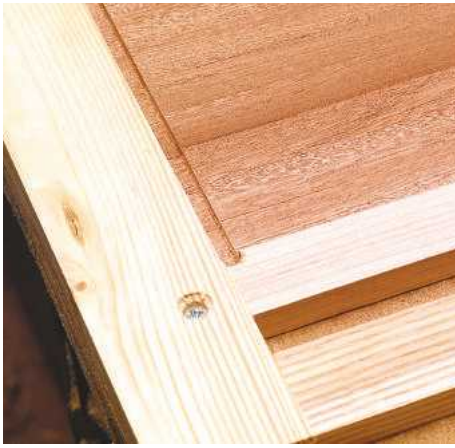
7 The routing jig must be perfectly square; use folding wedges or similar to cramp the slats together
