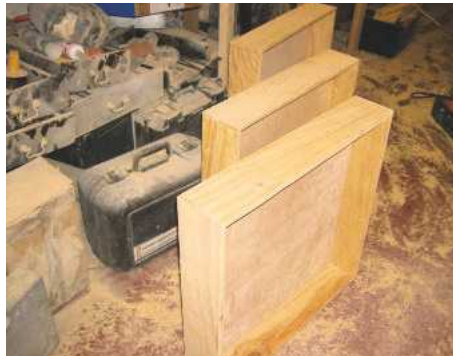
28 The drawer boxes assembled and ready for fitting
