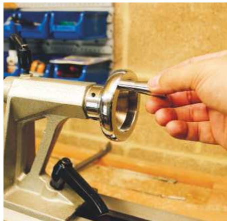
Top quality fittings, such as the quill advance, are a theme throughout the lathe
