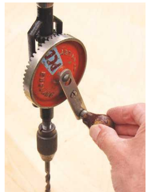
9 A hand drill offers you complete control...
