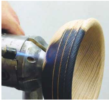
13 ... then heavily scorch the wood using a blowtorch
