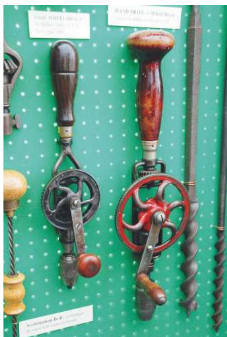
3 An unusual two-speed Millers Falls wheel brace
