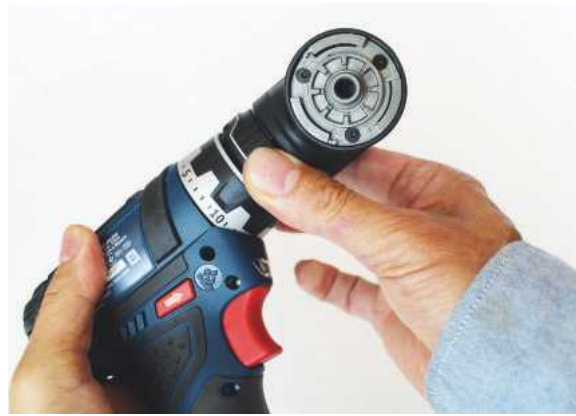
Grip the collar, twist and the chuck can be changed
