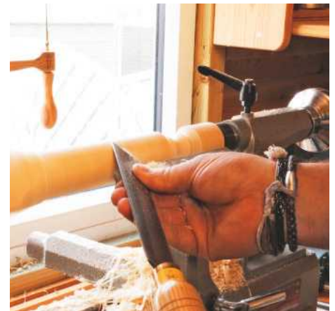
Between centres work is a very smooth, quiet and vibration-free ride
