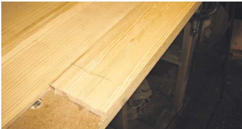
6 Pieces lined up and marked ready for routing the spindles
