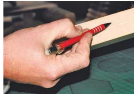
6 ... then clamp together, and mark a wavy pencil line along the underside's length
