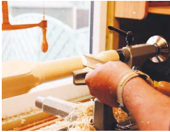
The toolrest is a tad short for longer spindle-type work
