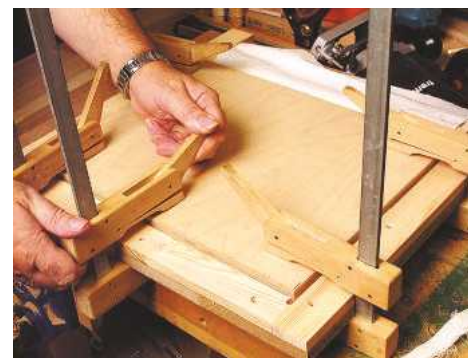
15 Apply cramping pressure with a caul; wax the face to prevent it sticking to the backing fabric
