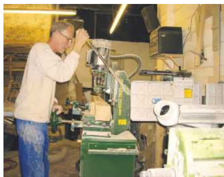
2 Cutting the mortises was a simple process thanks to the machine
