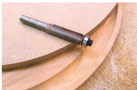
7 Use a bearing-guided trimmer to shape the circle
