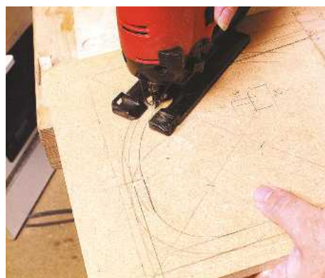
2 Jigsaw the curved leading edge of the template to just short of the line and carefully finish with a disc sander to remove...
