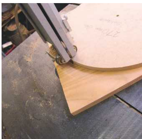
6 Trim close to the template without damaging it
