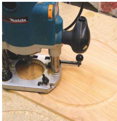
5 Press down on the compass point as the router is moved
