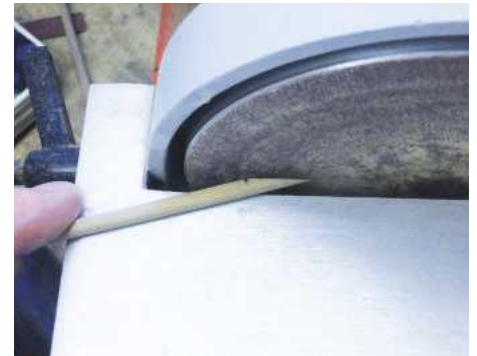
31 Using a disc sander to create the angled flat on the dowel
