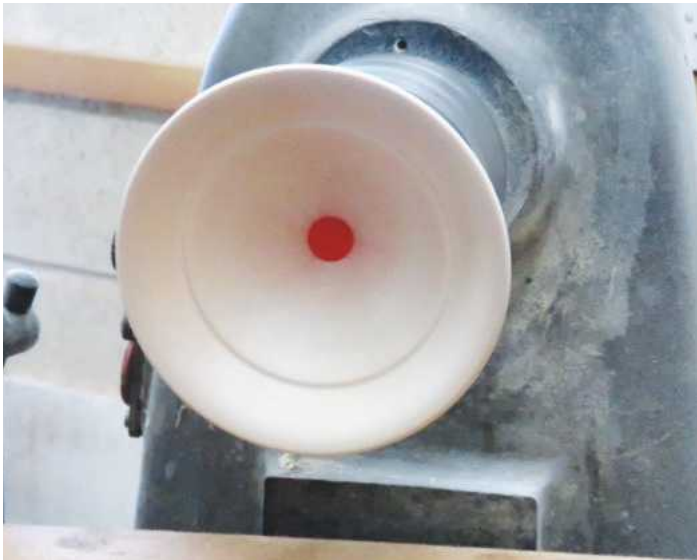
19 Put a small amount of thinned paint in the centre of the revolving workpiece...
