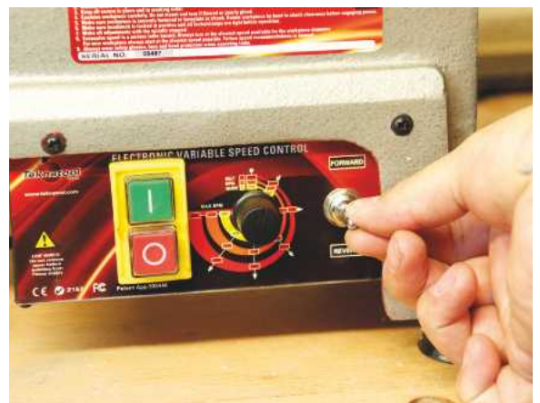
The lathe is put into reverse with the simple flick of a switch
