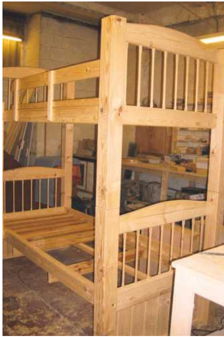
23 The guard rail screwed in place and slats fitted
