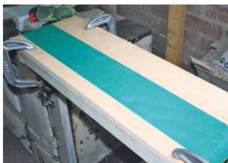
2 Apply double-sided tape to the top of the board and stick down 100mm of 100 grit abrasive paper
