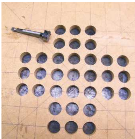
4 Use a Forstner bit to cut 20mm diameter holes
