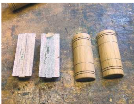
22 The fuel tanks, which were split in order to cut out the step after they were turned
