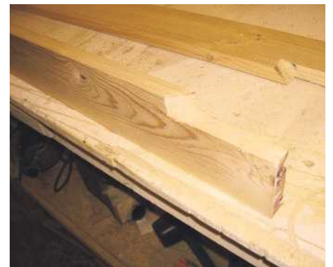
25 ... and the cut-outs were to take reinforcing triangular blocks on which to attach the wheels
