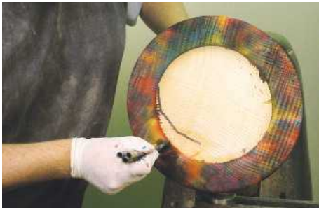
2 Use three glue brushes to stipple the stains onto the wood...
