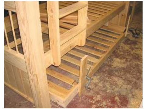
27 Scraps were clamped to the frame to check pull-out front depth
