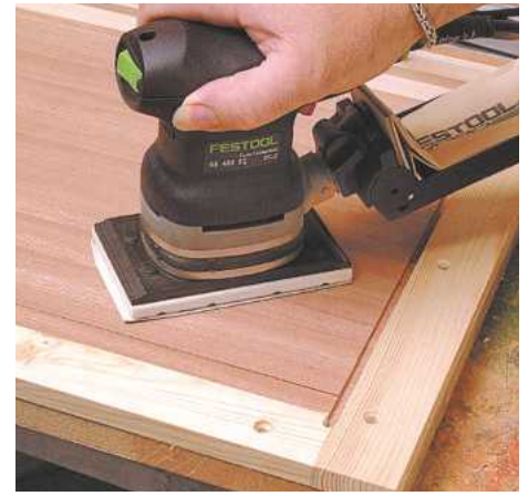
9 Sand the slats smooth then chamfer the front arrises with a plane or on a router table
