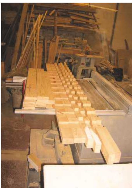
5 Notches were cut in the rail bearers to take the bunk bed slats
