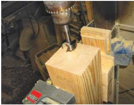
10 ... worked a treat, drilling the post holes with a Forstner bit
