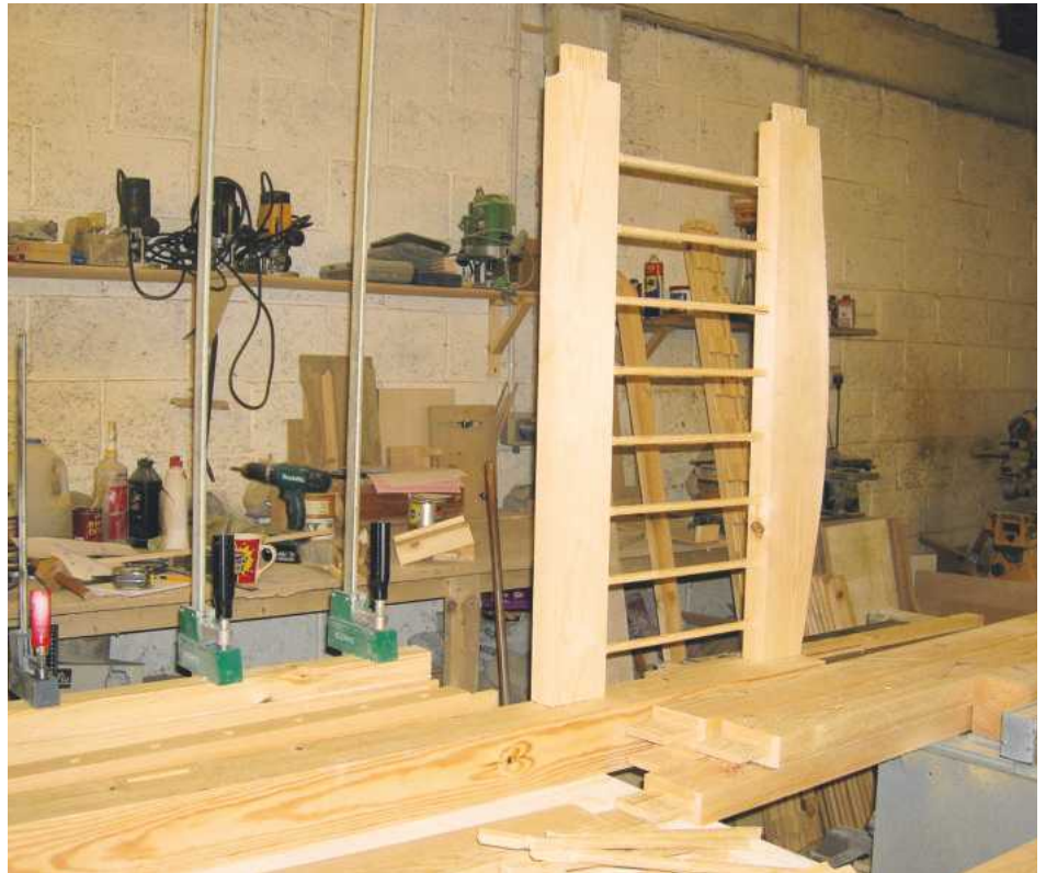
12 The first headboard passed its dry-fit examination...
