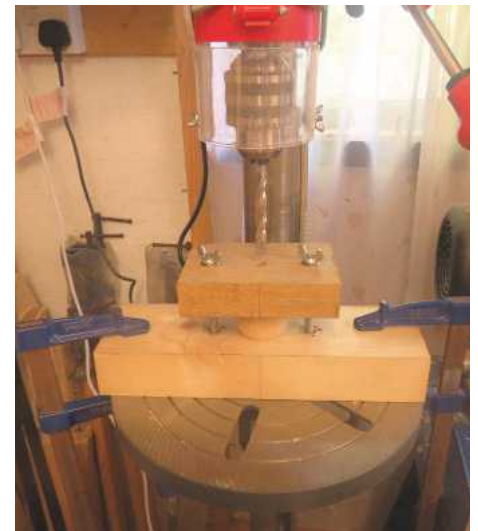
Chris' ball-drilling rig for drilling 50mm birch balls
