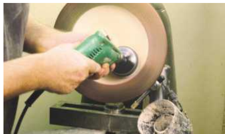
9 Power sand the inside to remove any stain overspill
