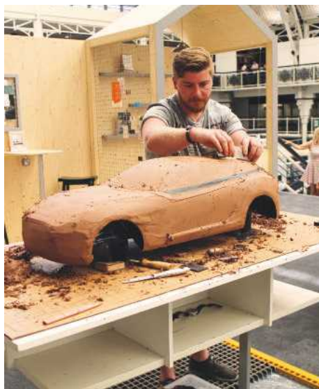
A clay model prototype takes shape under skilled (and sadly anonymous) hands
