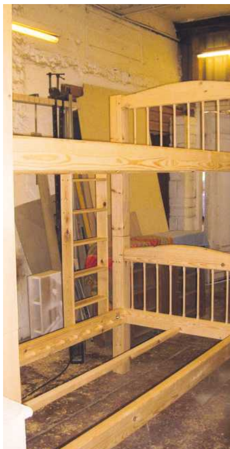
20 A robust ladder was screwed into place on the bed side
