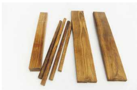
26 All of the round bars turned to 6mm on the lathe
