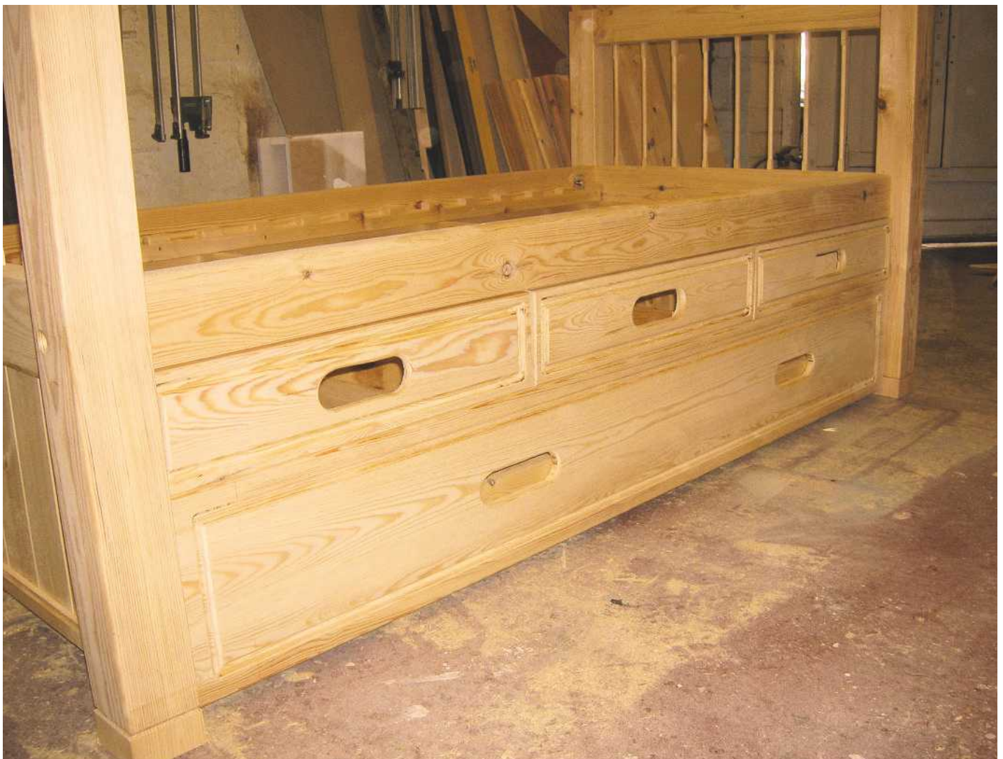
30 All drawer fronts and pull-out in place, ready for the finish
