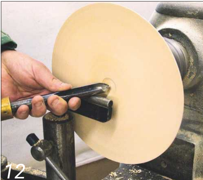
... and swing the handle, moving the cutting edge towards the centre
