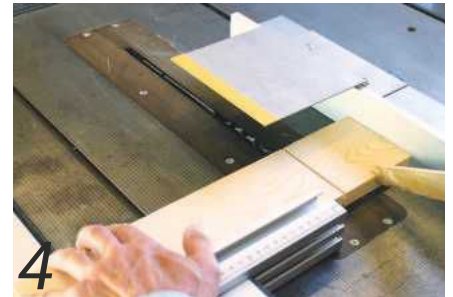
4 With a custom steel Suva guard fitted, this table saw procedure is as safe as I can make it; note push-stick
