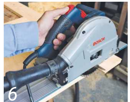
6 A rail saw makes cutting off the stile horns a tidy business
