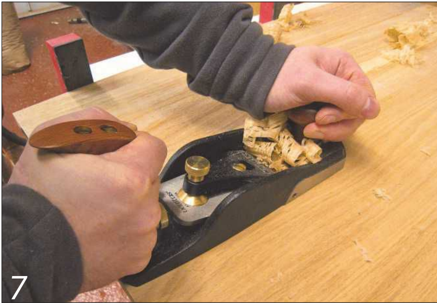
7 With most of the dried glue removed, clean up the joints with a bench plane. Check for flatness with a straightedge
