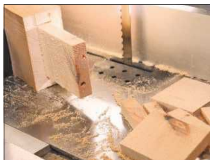
Using the basic mitre fence, it's very easy to cut a tenon in a minute or so
