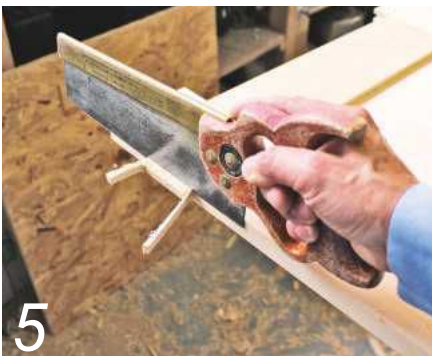
5 Trimming off the tenons and wedges the day after the glue up
