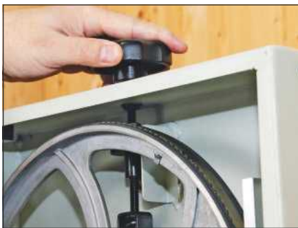
Initial tensioning is achieved with the top adjuster
