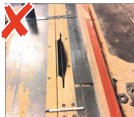
A dangerously modified machine: no guard and the riving knife has also been removed
