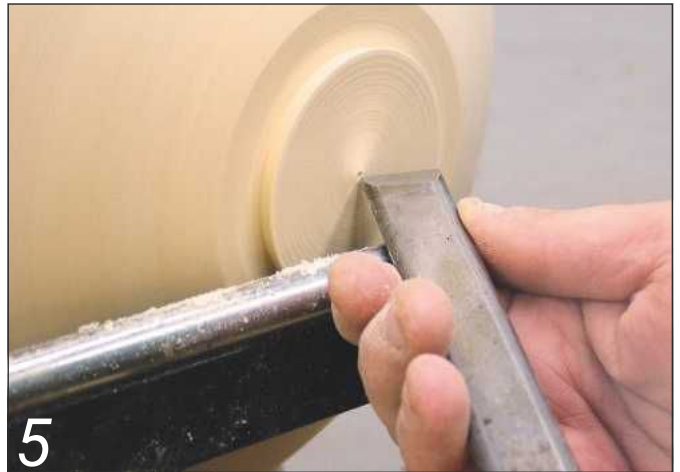
5 Dovetail the spigot and cut a pop mark in the very centre
