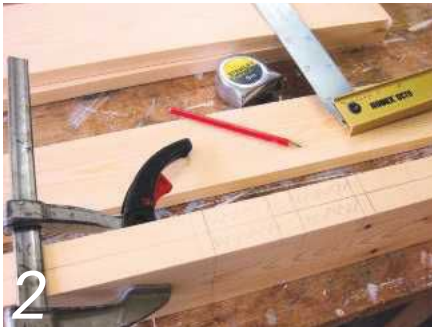
2 Careful marking out is essential; note clamp to enhance accuracy
