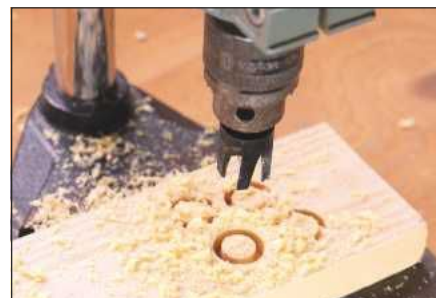
A drill stand makes cutting the plugs an easy job
