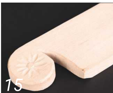
15 I formed the daisy simply by chopping vertically around the centre of the flower using a 10mm, No.7 gouge
