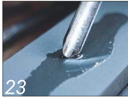
Sharpening a shell bit is rather like sharpening a gouge
