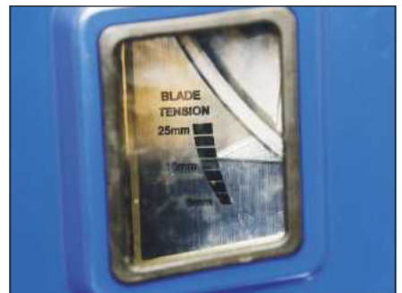
You can check the setting through the viewing window in the top door
