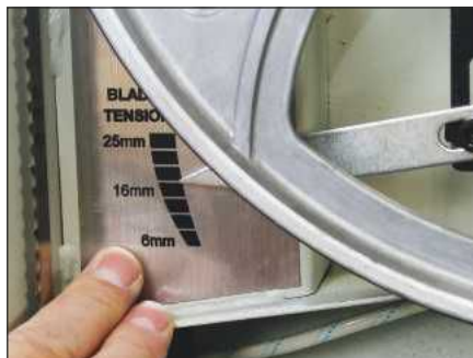
Tensioning can be assessed with the indicator
