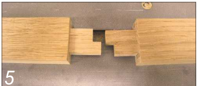
5 As rails meet in the centre of the legs, ends of tenons are stepped to enable them to fit over each other
