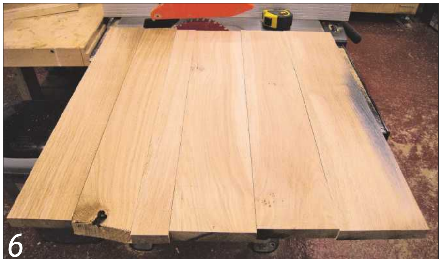
6 Arrange boards for each top so that grain pattern is pleasing and growth rings alternate. Glue and cramp together
