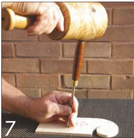
7 Whether to hold the tool at a low or high angle depends on the cut being made
