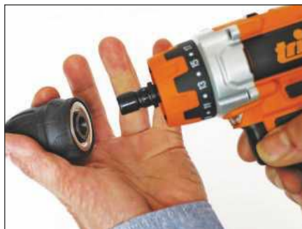
Removing the chuck from the drill exposes a 6mm hex bit holder beneath
