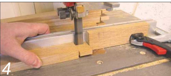
4 Tenons are safer to cut on the bandsaw. A stop cramped to the table restricts the length of cut
