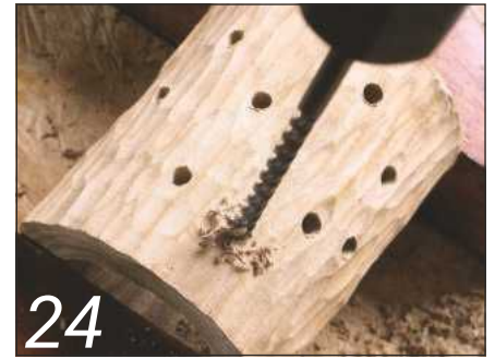
Jennings auger bit boring woodworm-inspired holes in a lamp shade
