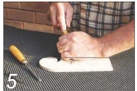
5 Wrap your fist around the blade with the side of the thumb rubbing the work and the other hand holding the handle
