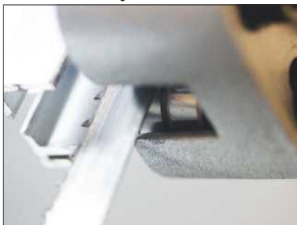
A neat feature is the use of double bearings for blade support
