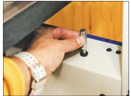
This post allows the table to be set perfectly square to the blade
