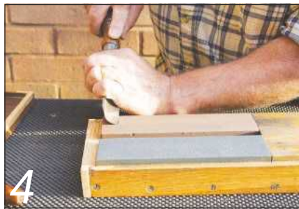
4 ... but rock the blade about its long axis to hone the entire edge. Sharpening gouges can be a little tricky, but it's important that your tools are razor-sharp
