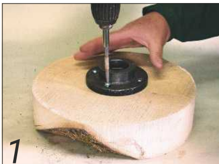
Find the centre of the blank and screw a faceplate to it
