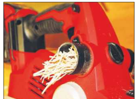
The dust outlet is easily overwhelmed when making wider cuts with the bag fitted
