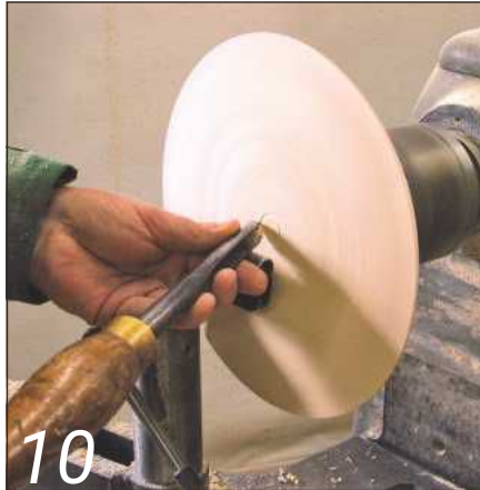
Start the hollowing with the tool handle well over the bed bars
