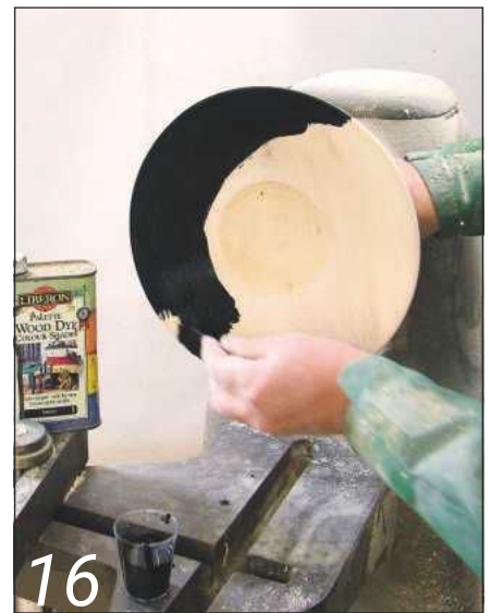
16 Ebonise the rim using Liberon ebony wood dye
