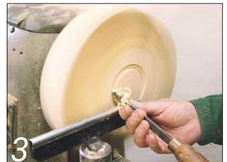
Use a parting tool to cut the chucking spigot
