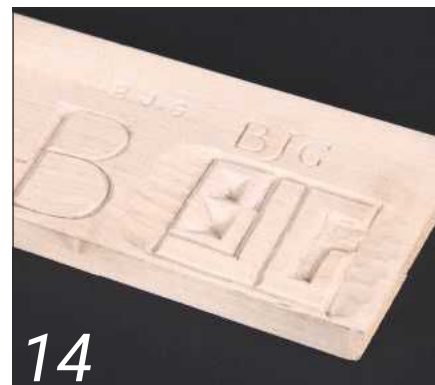
14 Letter carving can be done either freehand using gouges or using a set of alphabet punches
