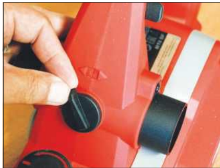
The side from which the shavings eject is controlled via this small dial
