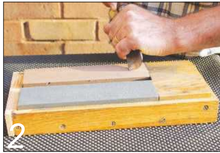
2 Move the blade longitudinally up and down an oil stone...
