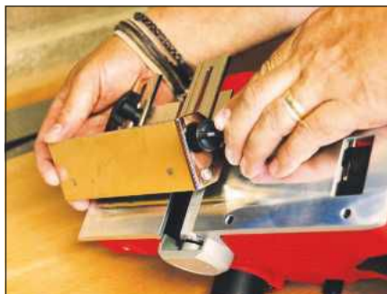
The fence is a great addition and can tilt for angled work
