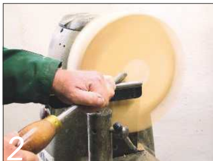
Flatten the face of the blank with a pull cut
