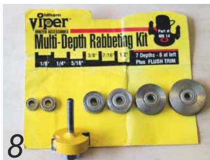
8 Detail of my very useful adjustable rebate cutter from American company Viper
