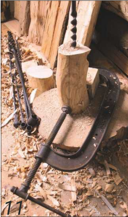
11 G-cramp set-up for getting a boot-hold on the work
