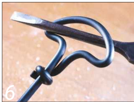
6 A screwdriver through the handle boosts leverage
