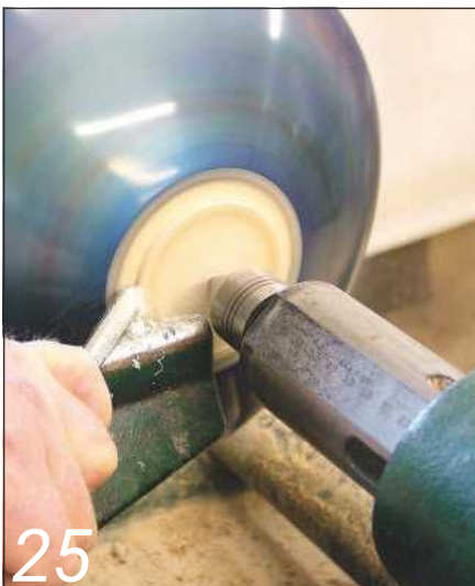
Reverse the bowl onto a mushroom-shaped dolly and remove the chucking spigot
