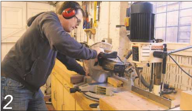
2 After planing timber to width and thickness, saw components to length, allowing extra for waste
