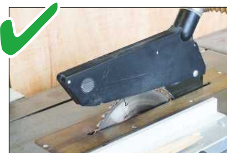
My standard setup, with guard and riving knife in place; note pushstick nearby
