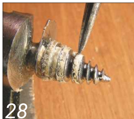
Cleaning the lead screw to maintain progress
