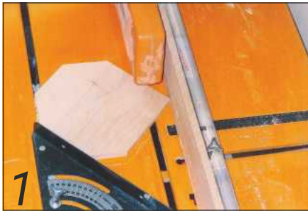
1 Making the octagons is easy if you start with a square piece and remove the corners
