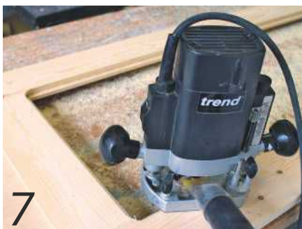
7 The rebate for the mirror is formed using a router fitted with a rebate cutter
