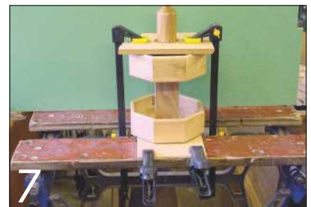
7 As well as checking for square, make sure the balconies line up at this point
