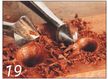
19 Snail countersink bits give a crisp result
