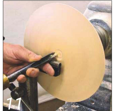
Once the cut is started, roll the tool anti-clockwise...
