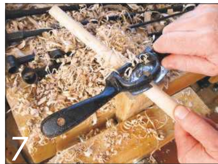
7 Shaping a handle for the Scotch augers with the spokeshave
