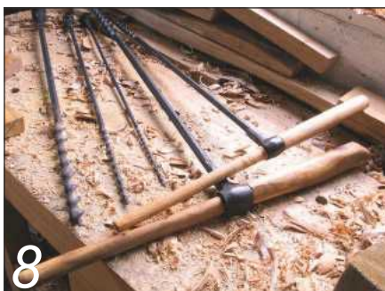
8 Scotch screw augers re-handled and ready for work
