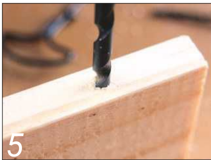
5 An auger gimlet guards against splitting near ends and edges
