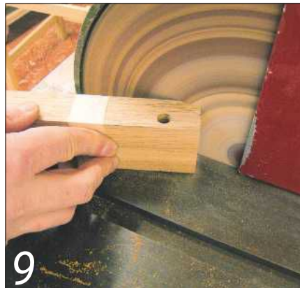
9 Front edges of support runners are tapered, so that each table slides into place easily. Shape on a disc sander
