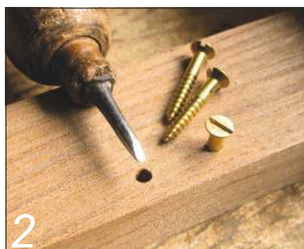
A bradawl makes pilot holes for small screws
