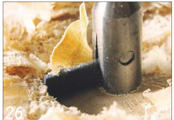
A Clark's bit hoists a sail of sycamore
