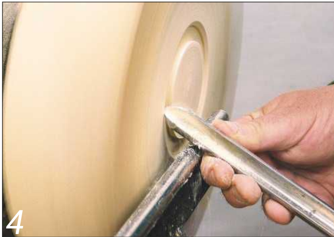
4 Shape the outside of the bowl with the bowl gouge
