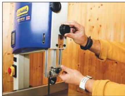
The height post is set with the double-function knob
