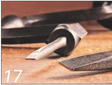
17 A Scotch iron brace with screwdriver bit gives good leverage
