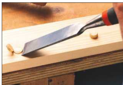
When removing waste, take care to ensure that the grain doesn't break off below the surface
