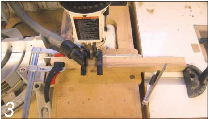
3 Cramping stops to each end of the mortiser fence restricts leg travel, ensuring mortise lengths are consistent
