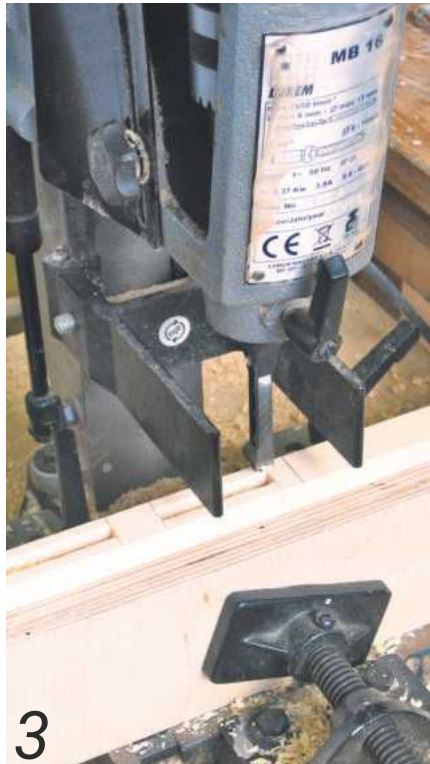
3 Even a basic bench mortiser will make a huge difference to making any kind of mortise & tenon frame
