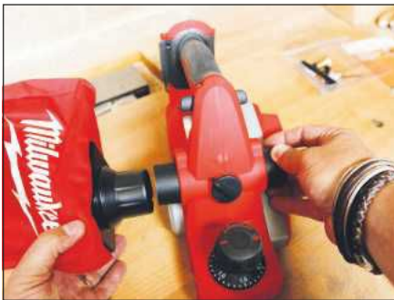
The supplied dust bag can fit to either side of the planer
