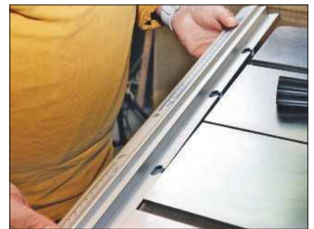
The fence rail on the BS350 removes easily for blade swapping
