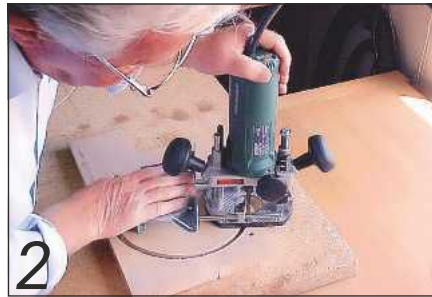
2 Cutting out the circular base with a trammel attachment for the router
