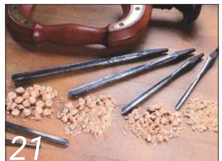
21 A set of shell bits and their characteristic shavings
