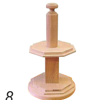
8 The first dry assembly, to check it goes together before cutting the rails
