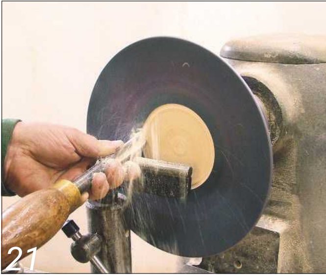
Complete the hollowing of the bowl part of the piece...
