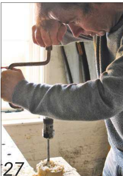
Boring into sycamore with a Clark's expansive bit
