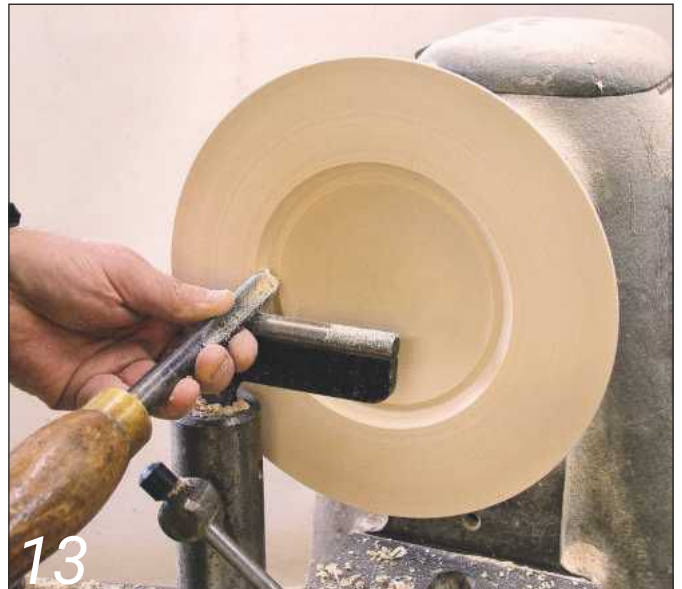
Repeat this cut going a little wider and deeper each time
