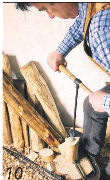
10 Boring the cable hole for a table lamp by half turns
