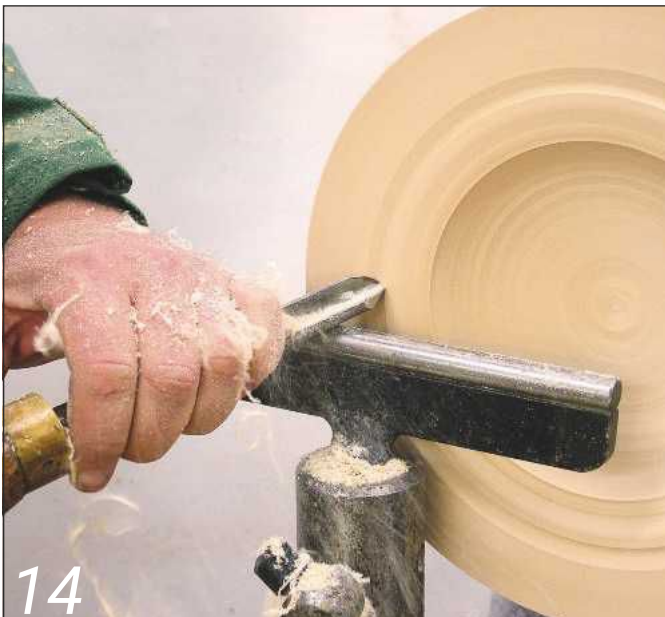
Use the same cut to shape the rim
