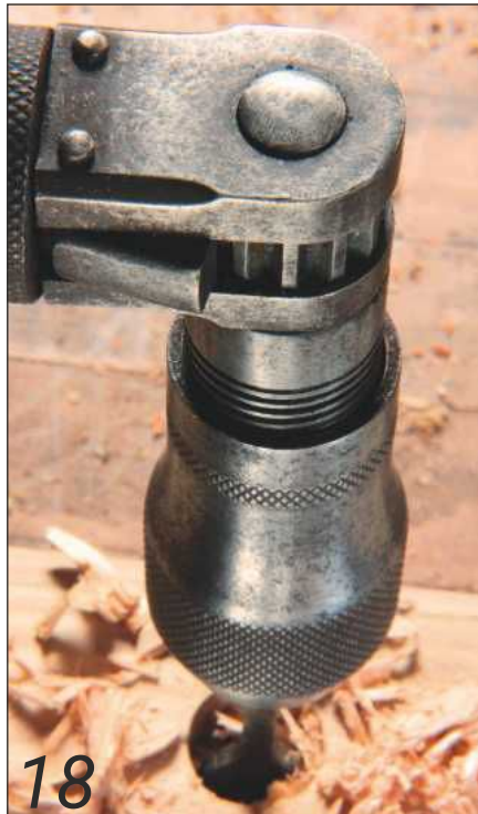
18 Gear wheel and pawl of the Millers Falls No.422 ratchet
