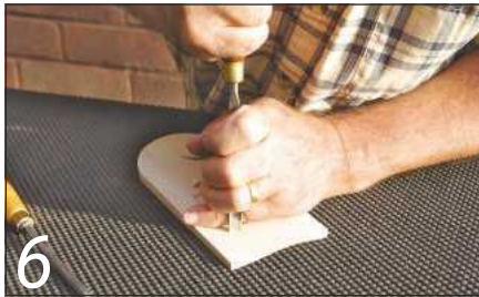
6 Hold a carving knife in a fist with your index finger providing the push
