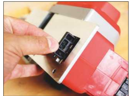
The parking shoe on the planer can be locked in flush if not required
