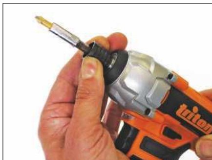
The impact driver has a sprung collar to assist in bit changes
