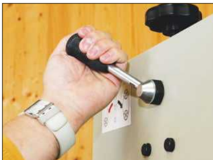
A tensioning lever allows fast blade swaps
