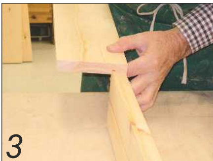
3 The inner faces need to be grooved and moulded to fit
