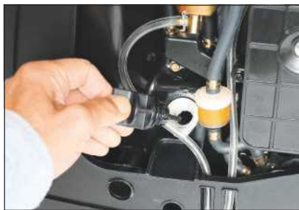
The filling port and tiny dipstick
