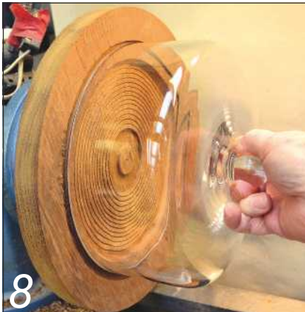
Cut a groove in which the dome is a loose fit
