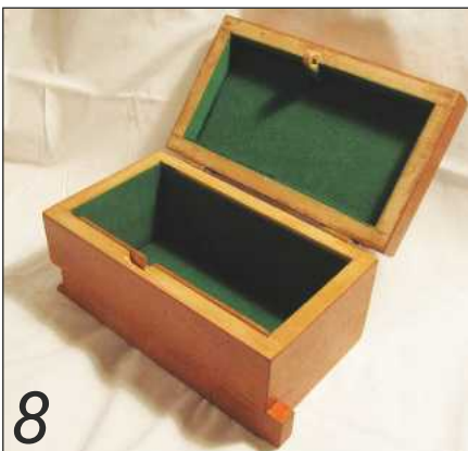
8 Here's one I made earlier. A completed box for an artist's paints and brushes, with veneer and baize lining – open... and shut
