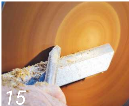
Clean up the surface with a gouge, leaving it slightly concave
