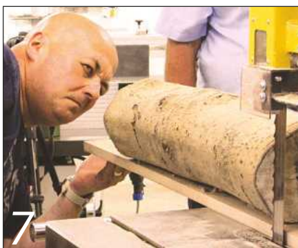
For smaller sections, an MDF board screwed to the log will provide a flat, stable face
