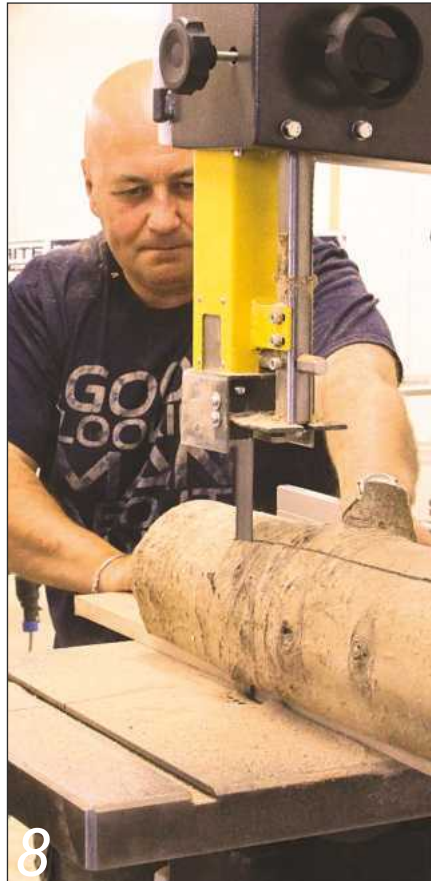
Screwing a board to the cut face increases its footprint on the table for extra stability
