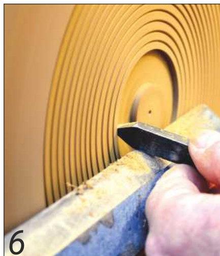
6 Cut a dovetailed recess to hold the board when it is reversed
