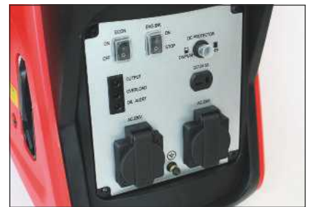
The control panel and outlet ports
