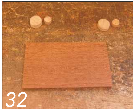
32 I cut the 3mm-thick piece into strips and then cut again to form the rear light and the backing for the front lights. The four small pieces shown here are the lights and these can be cut from dowel, or as I did, using a plug cutter and bandsaw, which means you can cut them from any wood you wish
