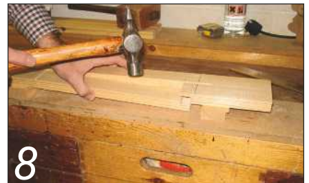
8 After cutting with the gents saw, turn the work over and give it a sharp tap to free the pocket
