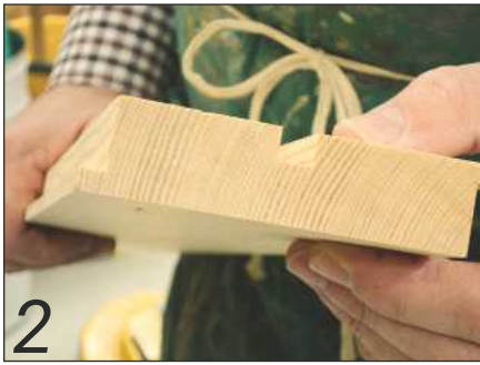
2 The cross-sections of the pulley stiles and head of the frame are identical
