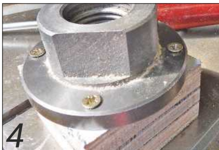
4 Screw a faceplate to the base of one of the blocks and make sure it's securely attached
