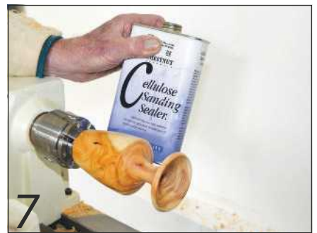
7 Apply at least two coats of sanding sealer. Work in a well-ventilated workshop as the fumes are strong
