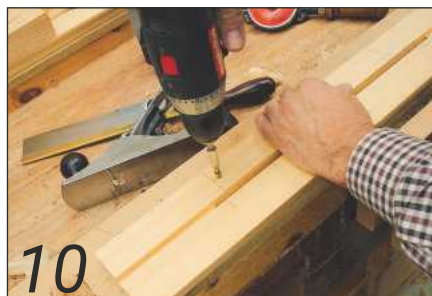
10 ... then fasten the pocket piece back into its stile with a countersunk screw
