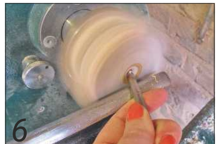
6 Turn the inside of the bowl to your desired depth using the small bowl gouge or fingernail gouge
