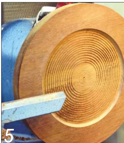
5 ... and a few grooves ensure good adhesion
