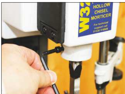
You need a hex wrench to secure the chisel
