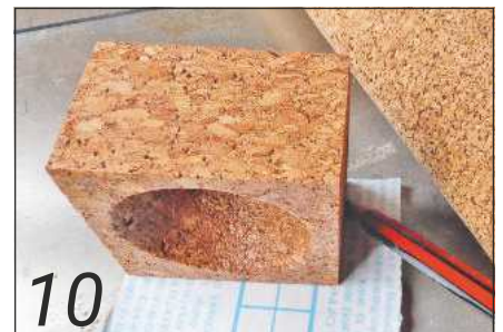
10 Leather or sticky-backed cork can act as a hinge. Mark the material to be the same width as the blocks (60mm)
