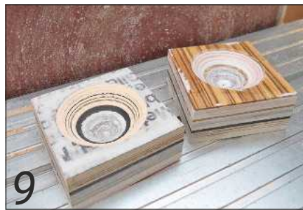
9 ... then you'll need to refine the finish using a disc sander or belt sander
