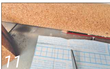
11 The height of the material should be cut to 30mm so that it will fit into the slits cut in the blocks. Use PVA to stick in place
