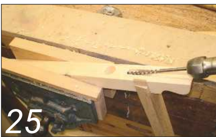
Two holes need to be drilled: one 8mm hole for the cord and one 32mm hole for the knot
