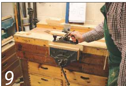
9 Remove the tongue from the back edge and plane the last of the tongue off...
