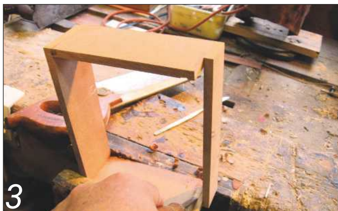
3 Chisel shallow housings into each end of the box for a thin wall, far enough back to make a snug slot for the thin plank that will become the secret catch
