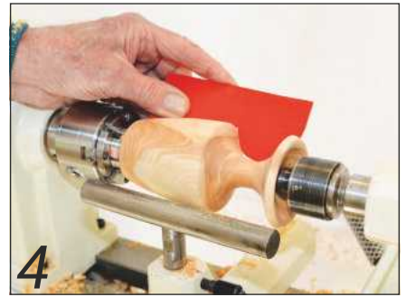
4 Replace the drill chuck with a revolving centre to support the work. Turn the body to shape using the half template as a guide
