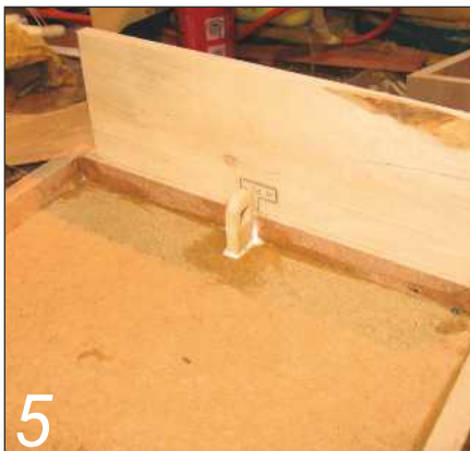
5 Having fitted an eye to the lid of the box, use the eye as a template to mark out an L-shaped slot on the sliding catch
