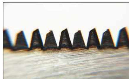
Close-up of triple-ground teeth
