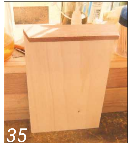
35 I cut a head board from 6mm timber and tapered the two outer edges. This was then stuck into place
