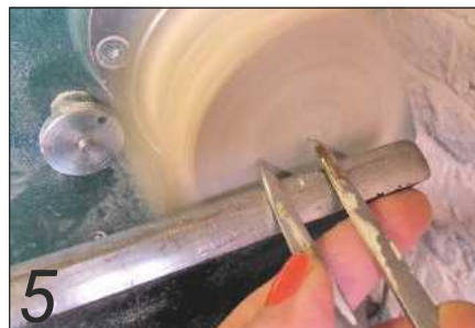
5 Mount the laminated block on the lathe and proceed to mark the size of your recess using the callipers
