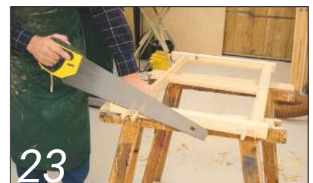
23 The sashes are sanded, horns and wedges cleaned off level, and the rebate formed
