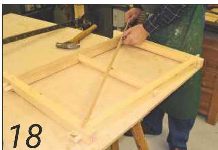
18 Check the glass panes are the same size; measure the distance between top and bottom rail
