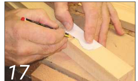
17 Not just decorative, joggles strengthen the joint between the stile and meeting rail
