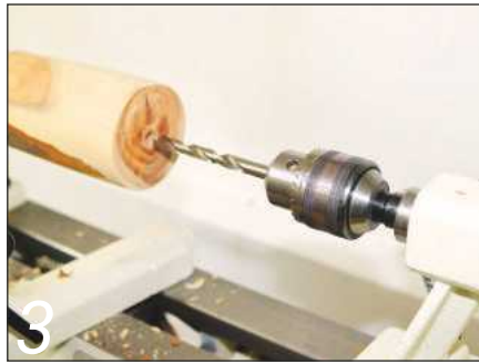
3 Fit a drill chuck in the tailstock with a 10mm twist drill. Drill a hole \frac{3}{4} of the distance into the blank, stopping frequently to withdraw the bit to allow the shavings to clear
