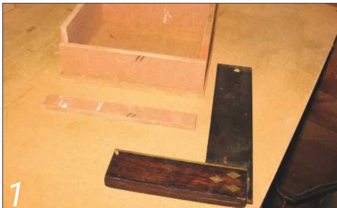
1 Cut off the bottom third or so of the front side, then assemble the four sides and a top upside down. Mark the cut edge so that you can be sure of an exact fit later
