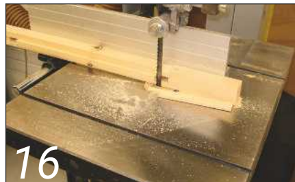
16 The bottom of the top stiles and the top of the bottom are left over length to allow 'joggles'
