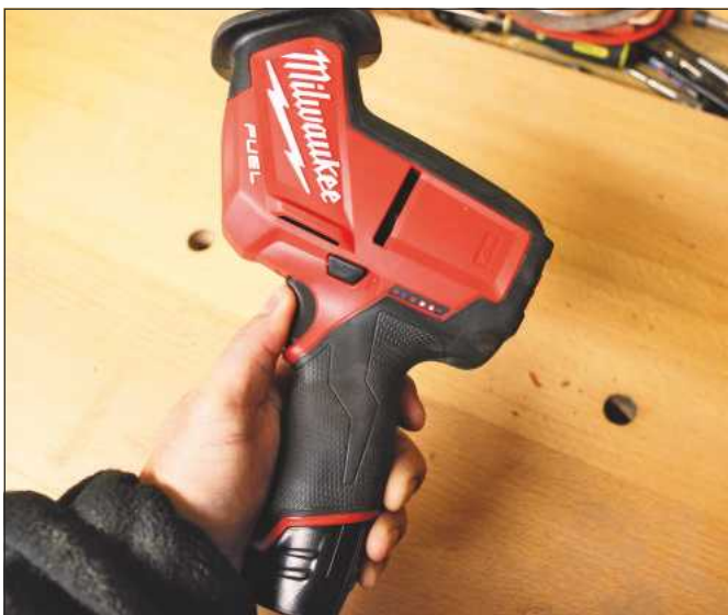
A touch on the variable-speed trigger illuminates lights on the tool to show the battery status
