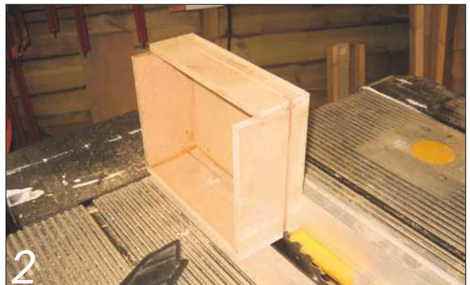
2 Saw through the assembled – and bottomless – box to form the lid (fence and guard removed for clarity). the safest way is by hand.
