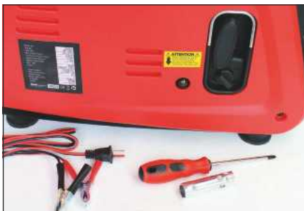
The starting handle plus supplied tools; note priming valve below 'Attention' sticker
