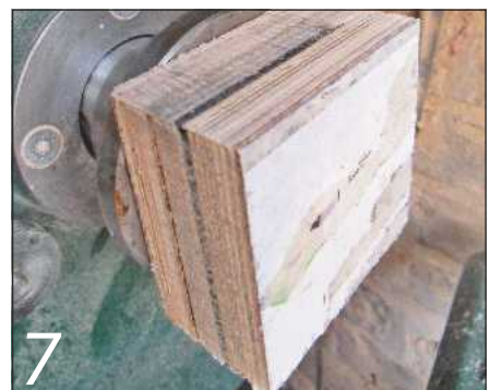
7 Mount a second block for the lid and repeat the process with the same-sized recess
