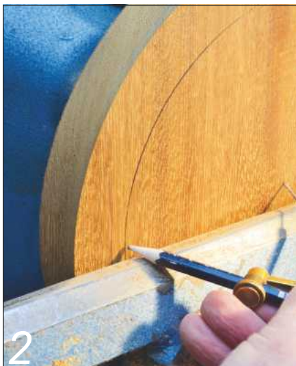
2 Mark the approximate diameter of the tile
