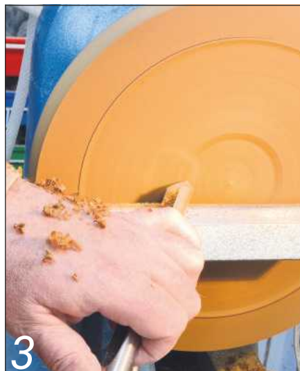
3 Clean up the surface and begin the recess for the tile
