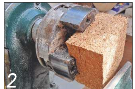
2 Mount one of the blocks onto the lathe using a four-jaw chuck
