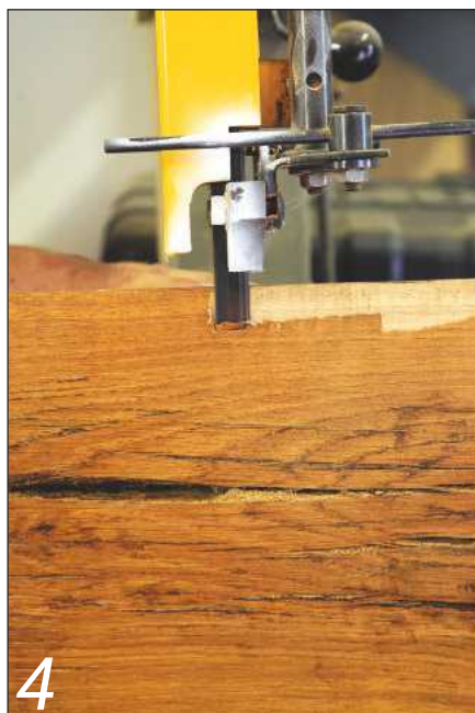
A conventional blade will struggle to clear the waste from a deep-ripping cut like this, and accumulated dust slows the cut and heats the blade
