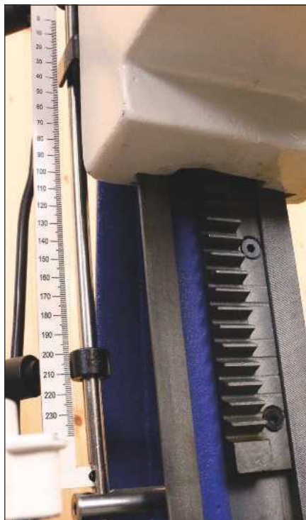
The rack and pinion slide on the plunge head keeps things running smoothly
