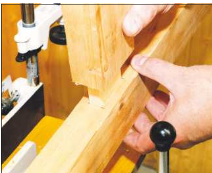
The resulting mortises are clean and square
