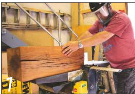
Planing one side of the oak gave a flat face to sit on the bandsaw table
