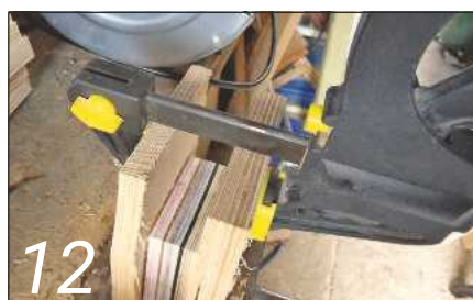
12 If layers come apart, simply apply some more adhesive, clamp, leave to dry, then re-turn
