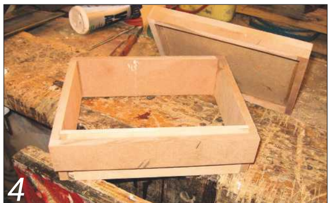
4 The sliding plank should be free to move almost the thickness of the side wall. If it can slide further than that thickness, the catch may jam when the box is opened
