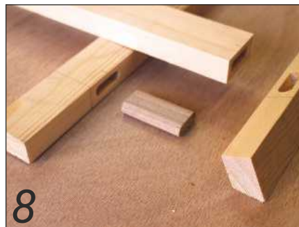
8 The door frame is simply – but accurately – Dominoed together for assembly on site
