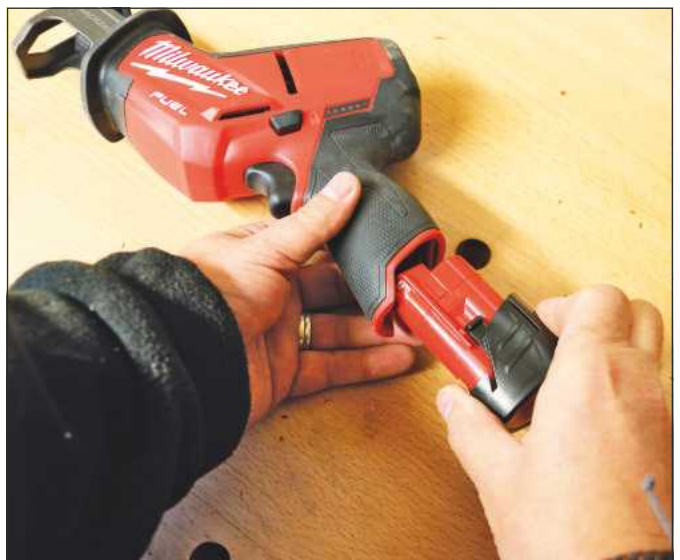
Batteries slide into the handle. 4Ah ones are available for longer run times
