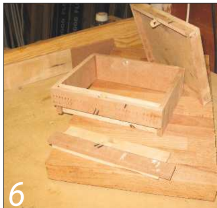
6 The three key pieces of the box – lid, carcass and catch – all ready for assembly, but notice that there is still no bottom
