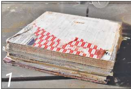
1 Cut your scrap paper into A4 sheets or large squares. Apply a thin layer of PVA to each layer
