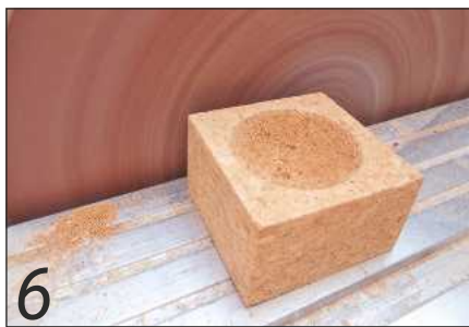
6 Sand the blocks on a disc sander to finish
