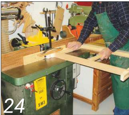
The sashes need a groove in their outer top edges to clear the sash cords and pulley wheels
