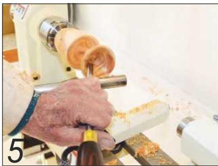
5 Carefully turn the top flute so it gently slopes down towards the centre hole
