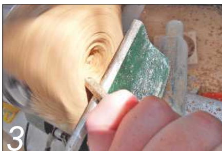
3 Mark the size of the hollow and turn the bowl, using a small bowl gouge
