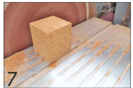
7 Hold the two blocks together when sanding to make sure they are the same size and square
