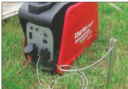
An earth spike is recommended for safety; this offcut of aluminium door track is just right for less-than-dry camping conditions
