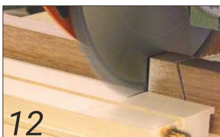
12 The trenches can be cut by various methods, a radial arm saw being the quickest
