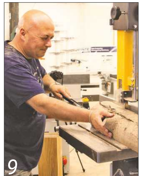
When you have two good faces, one for the table and one for the fence, you can start cutting boards
