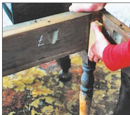
Rub joints are quick – it's cutting them to correct angles that takes time
