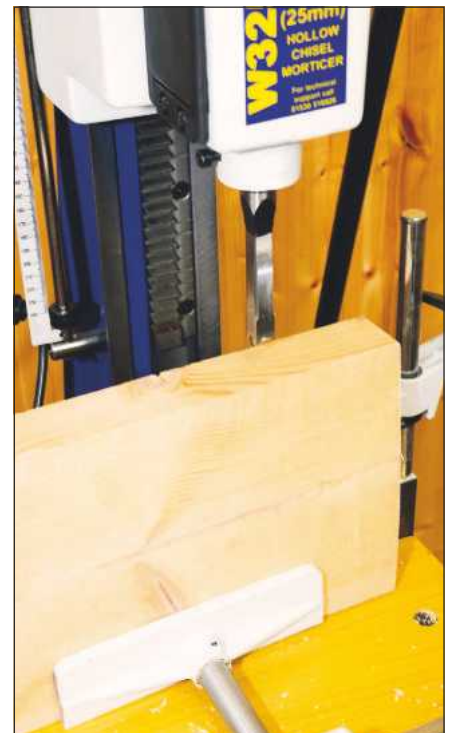
Timber up to 205mm deep will fit below a 13mm chisel
