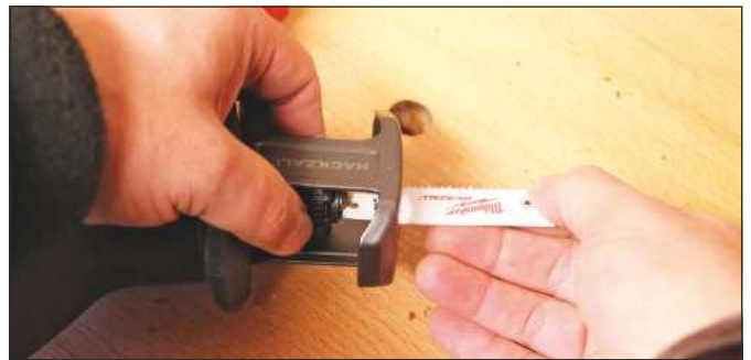
The Quik-Lok collar makes blade swaps very quick and easy
