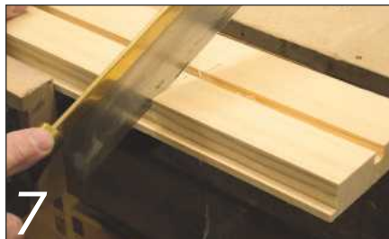
7 Next, you need to cut the pockets for the weights – the 'mysterious' part of the project!
