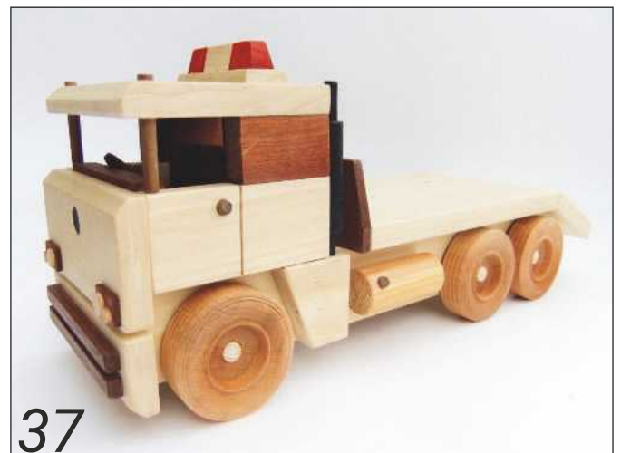
37 The final step was to seal the whole truck with cellulose sanding sealer followed by several coats of varnish before applying a final spray of gloss acrylic varnish. I was very pleased with the end result!
