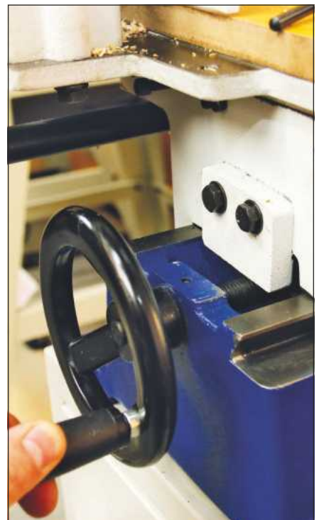
The front to back adjustment is altered with this large wheel
