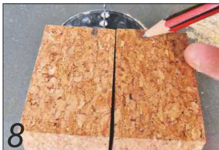
8 Mark two lines on the back of each block approximately 10mm from the middle on each side
