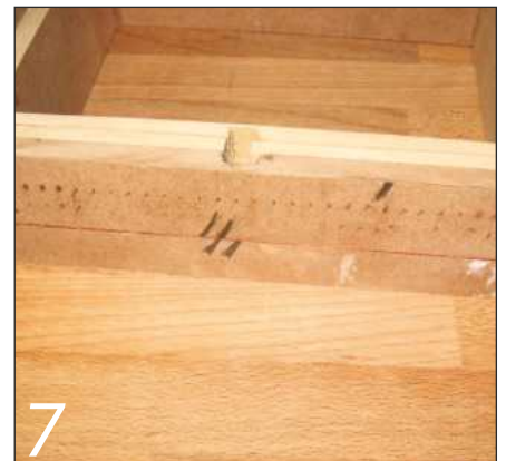
7 In the open position, the L-shaped slot lines up with grooves cut into the walls of the slot, and the eye on the lid can lift out freely. Notice the strip of veneer along the top edge of the cut-off section of the front wall; it compensates for the kerf
