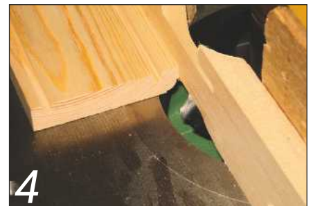
4 You'll need to cut an ovolo mould on the outer facings as shown
