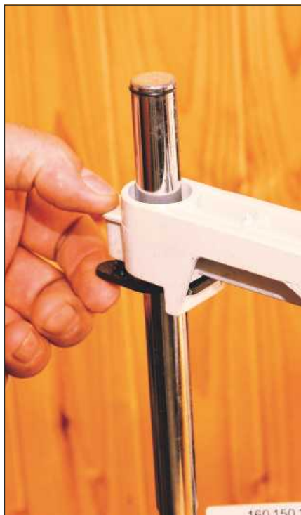
This quick-release clamp is very fast to adjust
