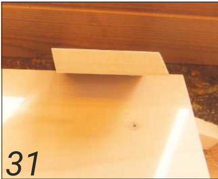
31 The beaver tail part of the bed as well as the main bed were cut at an angle to give a nice clean transition. I also angled the back to bring the tail lights to the correct angle
