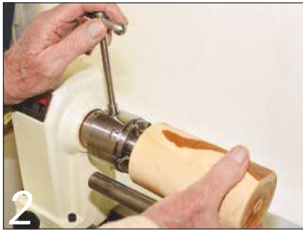
2 Remove the work from the lathe and screw on the chuck. Mount the blank in the chuck and tighten up the jaws
