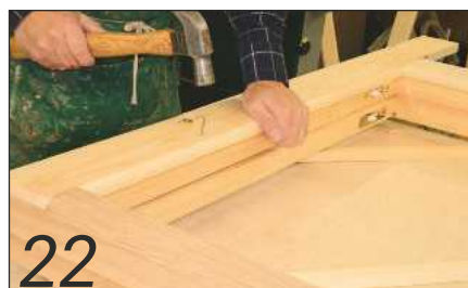
22 Finally, nail the inner and outer facings together and put to one side
