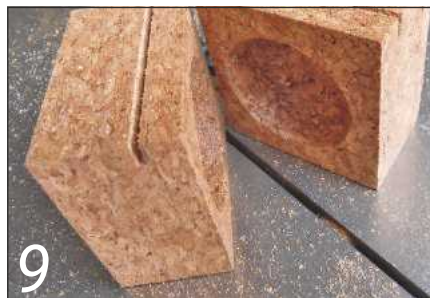
9 Using a fine bandsaw blade, cut two slits approximately 5mm deep
