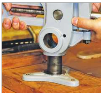
The easily secured vice slips onto the post and self locks once tightened against the work
