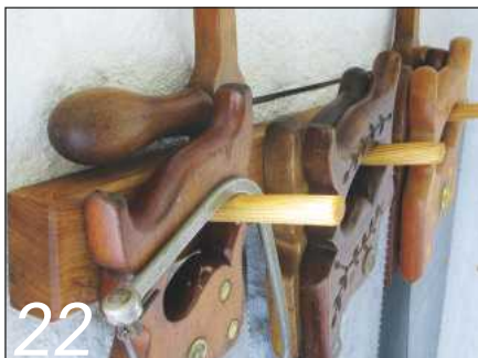
22 Cross-cut, rip, coping and bow saws hung on the rack
