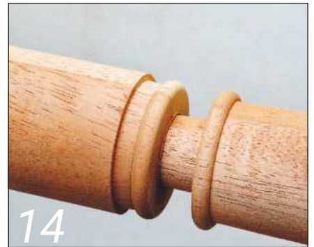
14 The beads side by side will hide the joint between them
