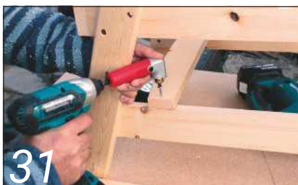
31 Once you are happy with the position, fix the lower back rail into place
