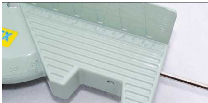
The mitre saw's table is made of aluminium alloy with four plastic and chrome uprights
