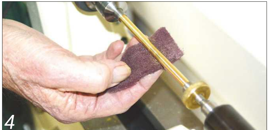
4 Clean the outside of the tubes with fine abrasive to remove any grease
