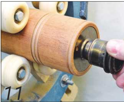
11 The steady rest supports the work
