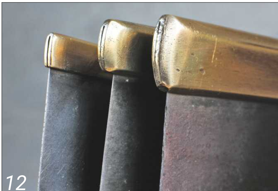
Folded brass backs of gent's, dovetail and tenon saws
