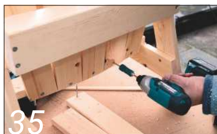
35 Set the intermediate slats central to the others and fix in place
