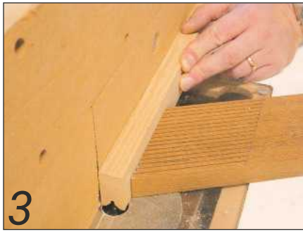
3 ... as was the rebate, here using a featherboard for accuracy
