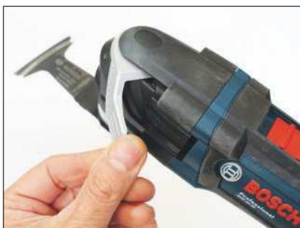
The old cutter is removed by simply pulling the SDS lever...
