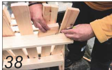
38 Using a gauge block, the back is scribed and cut with a jigsaw
