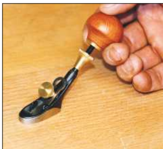
By unscrewing the top part of the handle the length can be extended
