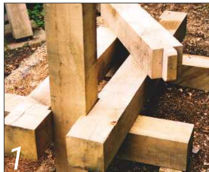
1 The press comprises two stabilisers, one sliding beam, two lower beams and two upright posts
