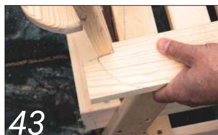
43 Once scribed, you should be left with a neat fit, as shown here
