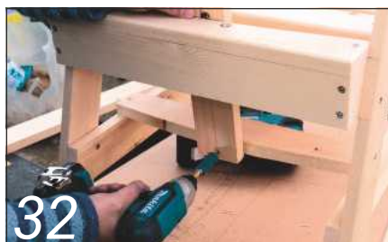
32 Fix the centre back slat to the lower rail with a 60 x 5mm stainless screw
