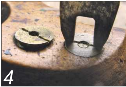
Old saw nuts require a special forked bit
