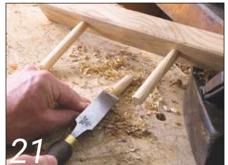
21 Tapering the ends of pegs to fit the holes
