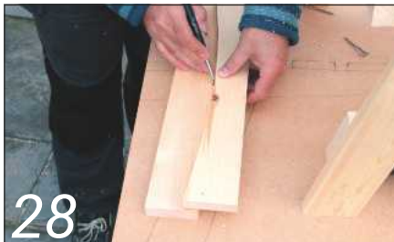
28 The slat is used to transfer the curve to the lower back rail
