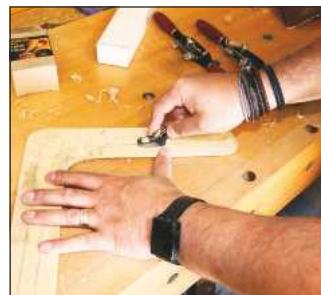
Here the convex plane is ideal for contouring the underside of a boomerang
