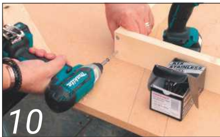
10 The seat frame is screwed together using stainless steel fixings for durability
