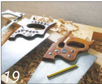
19 Laying out saws to mark peg positions on the rack
