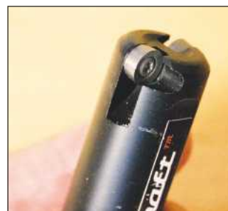
The cutters are made from solid tungsten carbide for durability
