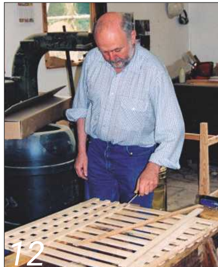
The cheese racks lock the package of apple pulp in place and provide drainage
