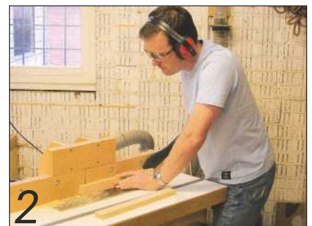
The central 'V' groove of the frame was cut on a router table...
