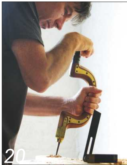
20 Boring holes for pegs using the sliding bevel as a guide
