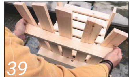
39 Check the fit of the stiffener against the slats
