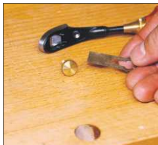
You have to remove the retaining knob to hone the iron
