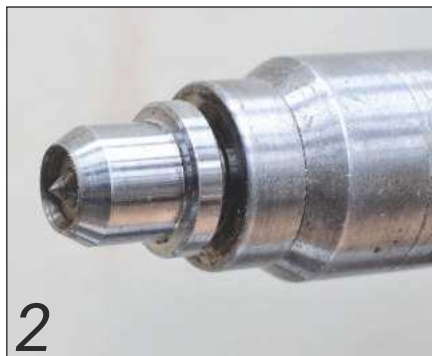
2 A ring centre cannot split the joint
