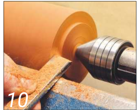
10 Form a dovetail spigot to hold in the chuck
