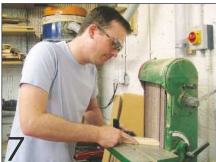
7 After rough sawing, I used a belt sander to ensure I met the cut line accurately
