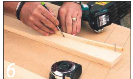
6 The lath is used to transfer the curvature of the seat to the frame component
