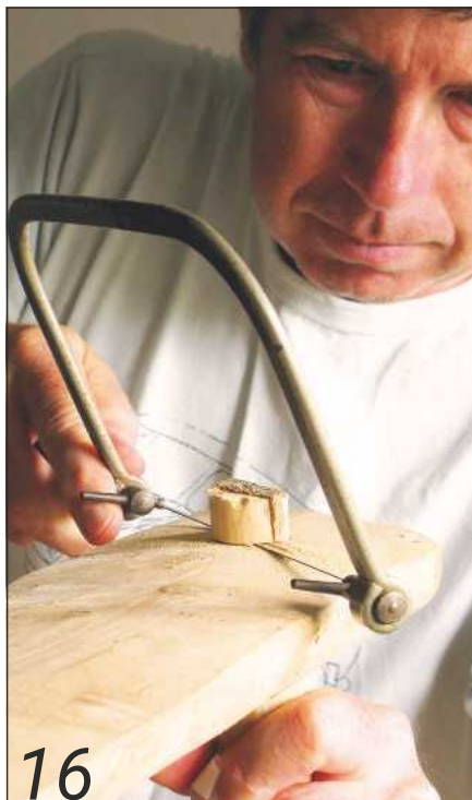
16 Trimming a wedged tenon flush with the coping saw
