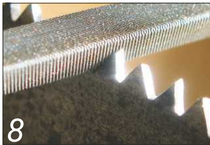
A tapered triangular file for saw sharpening
