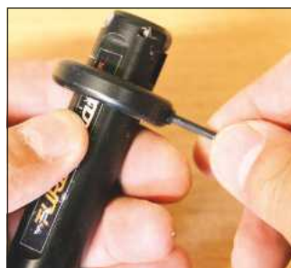
The collar can be used to restrict the plunge depth of the tool
