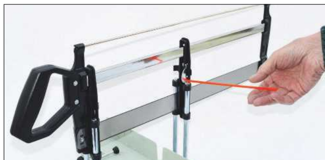
A simple clamp holds the wood in place and can be moved from right to left as required
