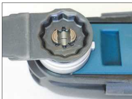
... and the sprung jaws keep it firmly in place
