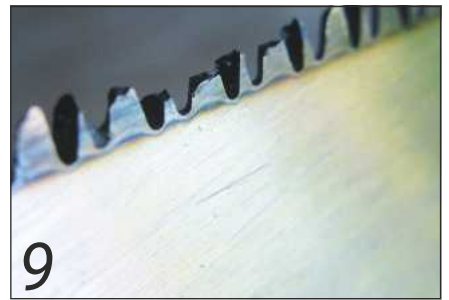
The damaged hardpoint teeth seen on a disposable saw
