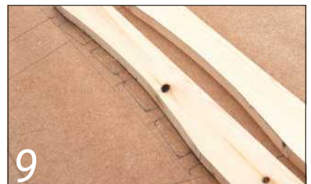
9 The pieces can be dropped onto the rod to check for accuracy or to transfer further marks
