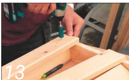
13 Screw the slats into place using 60 x 5mm stainless screws
