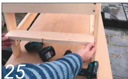
25 Next, cut the back leg rail to the inside width of the legs
