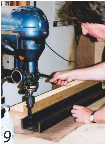
Drill two sets of holes into the steel channel beam for the bolts that will fix it to the posts
