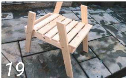
19 Check the chair sits flat and the legs are correctly in contact with the floor
