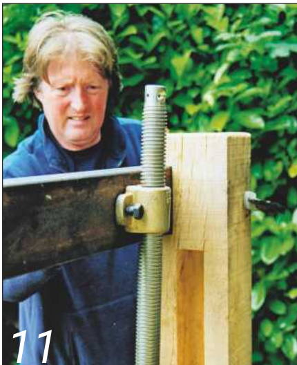
Using galvanised coach screws, fix the swivel feet of the jacks to the sliding beam
