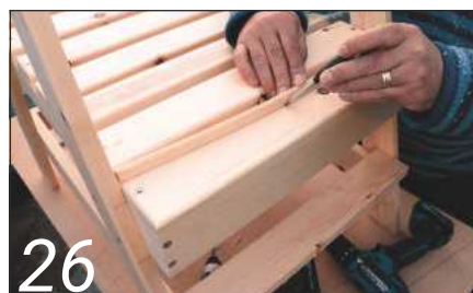
26 Use the lath to mark a concave curve on the back seat slat
