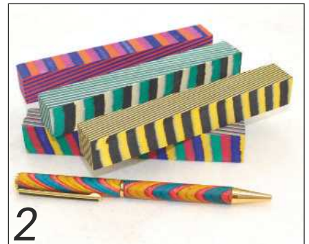
2 Laminated plywood pen blanks produce a very striking effect once turned
