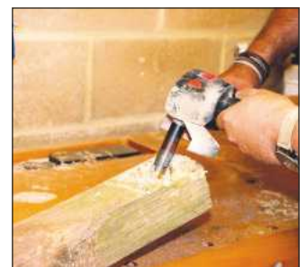
On softer, wet timber the TurboShaft struggled to cut
