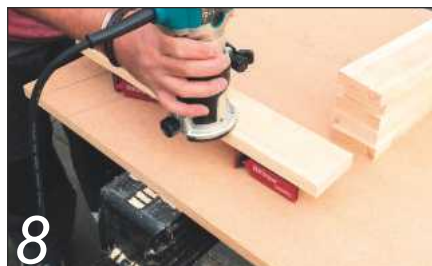
8 Using a roundover bit, the slats are routed to ease the top edges
