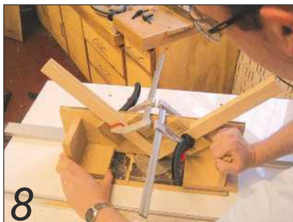
8 A dovetail jig was used on the router table to create the dovetail keys
