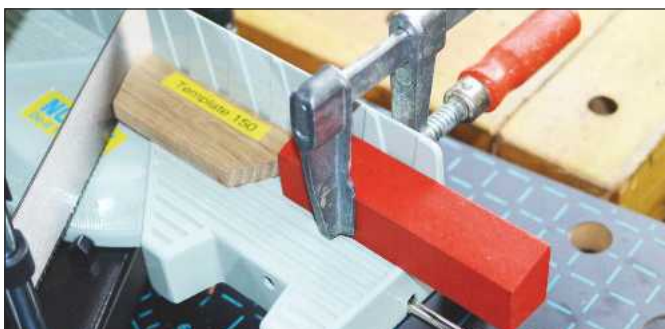
When cutting small pieces, I use a carefully prepared block of wood – again, clamped to the base to hold the block down
