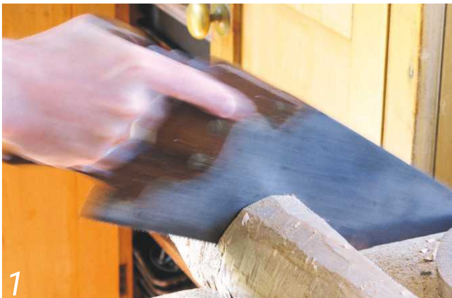
A relaxed grip keeps the saw running sweetly
