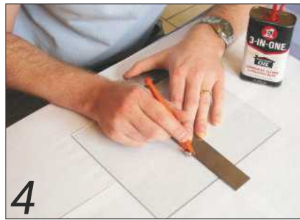
4 Cutting the glass – use a set square here and a drop of oil also helps the glass cutter
