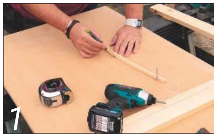
1 Mark the curvature of the seat onto the rod using a thin, flexible lath
