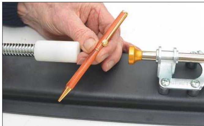
A wooden pen assembled using the pen press
