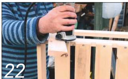
22 Before fitting the front rail, round over the edges of the legs
