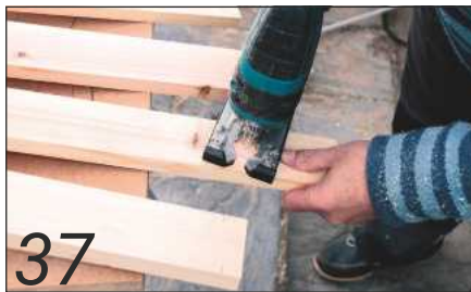
37 Cut the slats to length with a jigsaw and clean up as necessary
