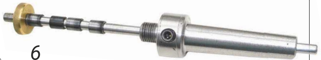
A pen mandrel is used to turn most pen barrels and is adjustable in length
