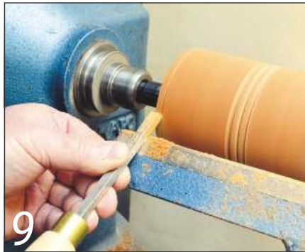
9 Using the bead-forming tool
