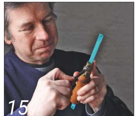
15 The pad saw's slotted handle accepts a standard hack saw blade
