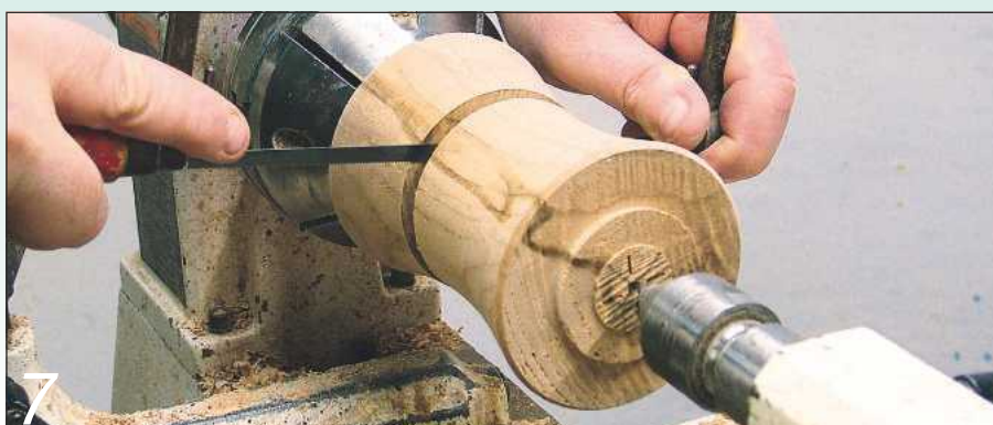
7 If you don't like the idea of parting through completely, then stop the lathe and cut the lid from the base with a saw. The piece that is left in the chuck will be the lid
