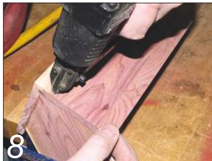
8 Nail along the chamfered edge of the second roof section
