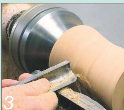
3 Mount the blank in your chuck and turn the cylinder to a flowing curve or cove
