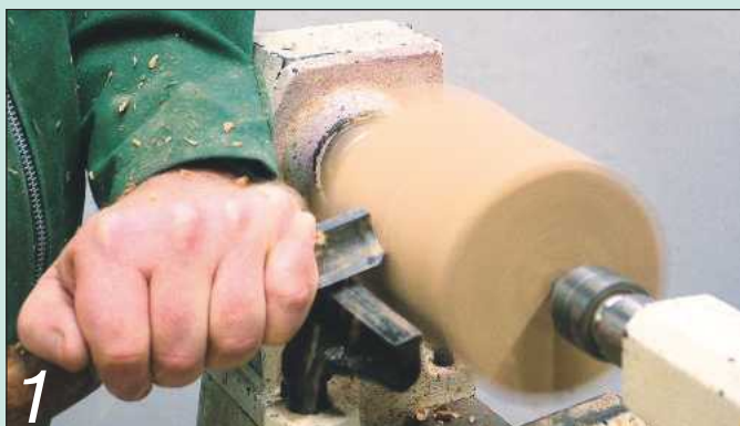
1 Start by mounting the blank between centres and turn to a cylinder using a spindle roughing gouge
