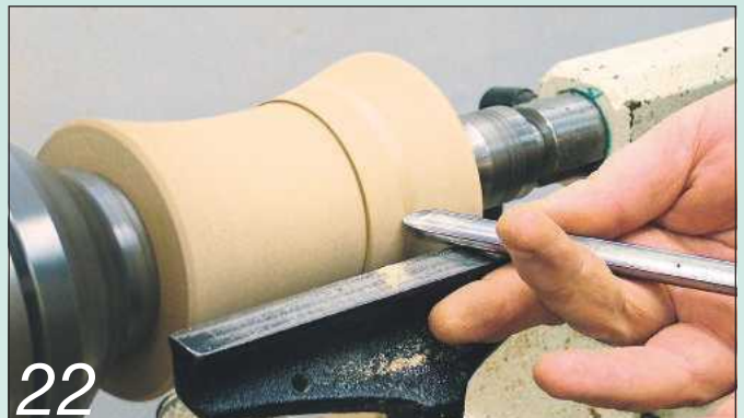
22 Fit the lid and re-shape the outside cove, blending the lid to the base
