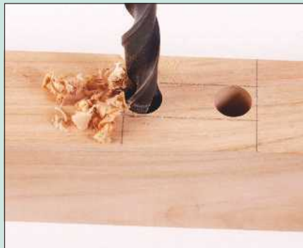
6 For faster waste removal on larger joints, it is worth boring some of it away with a drill. Select a bit size a little smaller than the width of the mortise and start by accurately drilling a hole at each end of the mortise, then remove as much of the waste in between with a series of overlapping holes. If you find it difficult to drill straight, stand a small try square on the workpiece to help guide you
