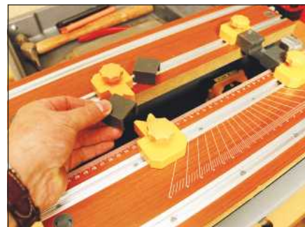
Slide-on shoes allow round work to be held
