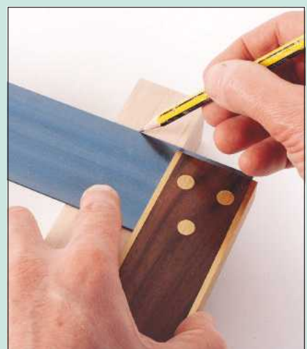
4 Mark out the tenon shoulder length on the rail using the try square. Carry the line on all round
