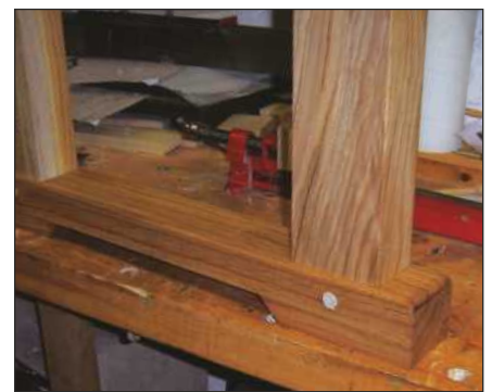
The lower cross-brace used draw-boring to ensure a tight joint
