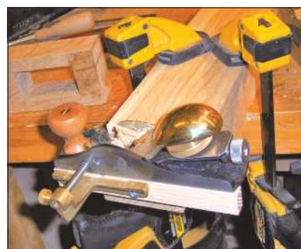
Clean up the shoulders and faces using a shoulder plane and rabbet plane
