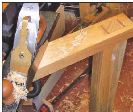
...that were driven in and trimmed back once dry
