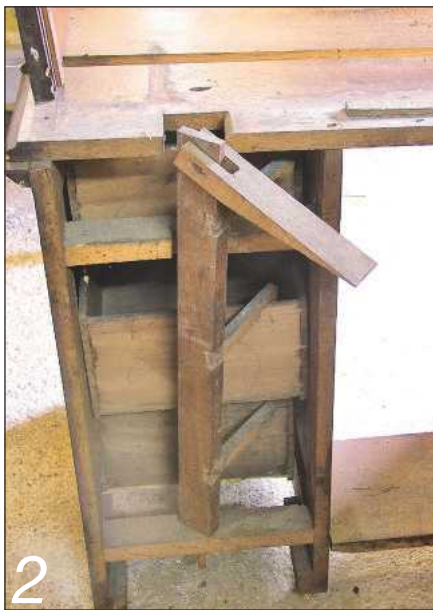
2 The simple but ingenious mechanism to lock the desk drawers
