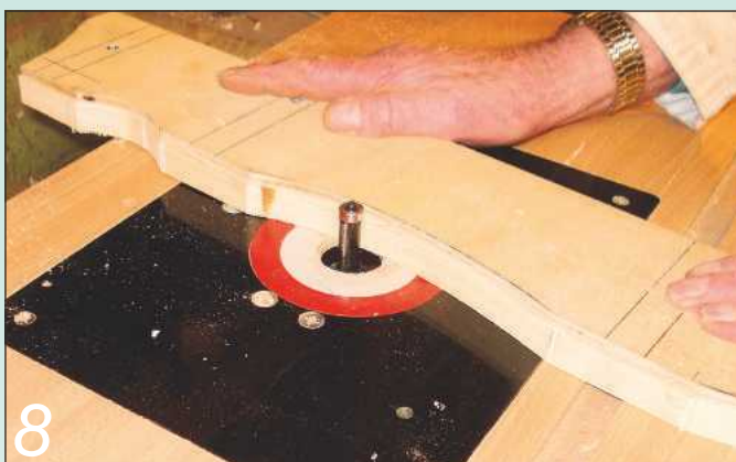
8 With the template still in place, the edge is trimmed on the router table
