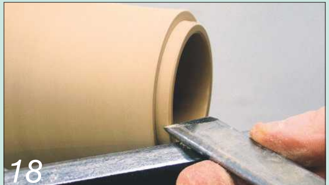
18 Use a skew chisel to cut a small chamfer on the tenon...
