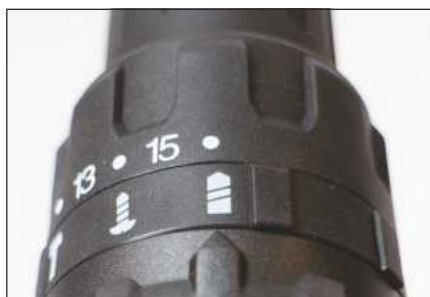
The two selector rings: one on 'drill', the other on 'max torque'
