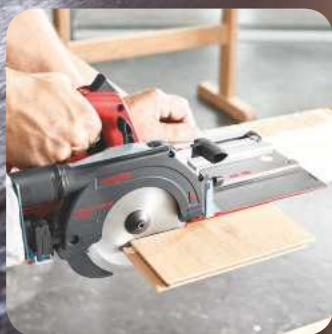
The smart stop and adjustable fence allow the saw to be used for angle cuts from -60° to +60°
