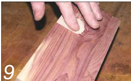
9 Apply a little masking tape to the joint, just to hold things aligned until the front panel is installed
