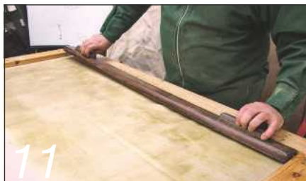
11 Rebuilding the tambour, starting with the lift rail
