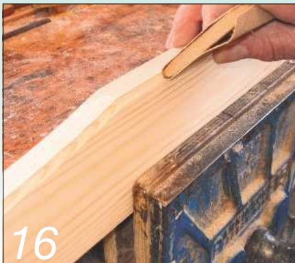
16 The small coves at the edges are smoothed using a shaped sanding block
