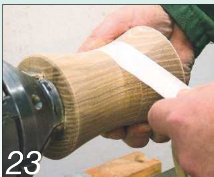
23 My lid was a good, tight fit but it is vital that the lid does not move during the next process. Use masking tape here to help keep it in place
