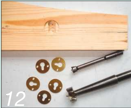
12 Holes for hanging plates completed and the bits used
