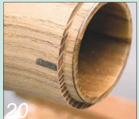
20 ... then the lid should leave a light burnish mark
