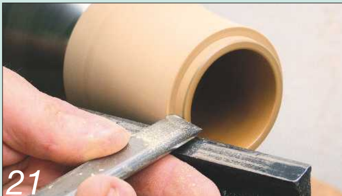
21 Reduce the size of the tenon to this burnish mark and, in theory, the lid should be a good fit. Aim for a tight fit at this stage – it can be eased later
