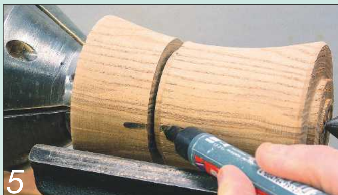
5 Before parting off, completely mark a witness line on both sides of the groove; this will help line up the grain
