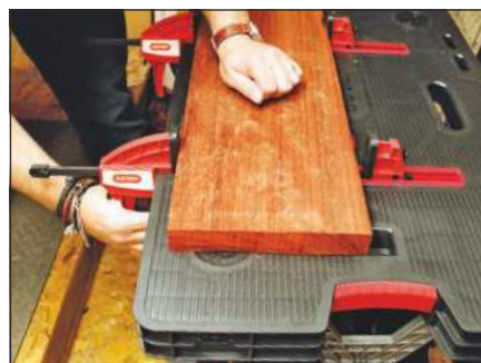
Two quick-release clamps are stored on board and are locked into slots in the bench top
