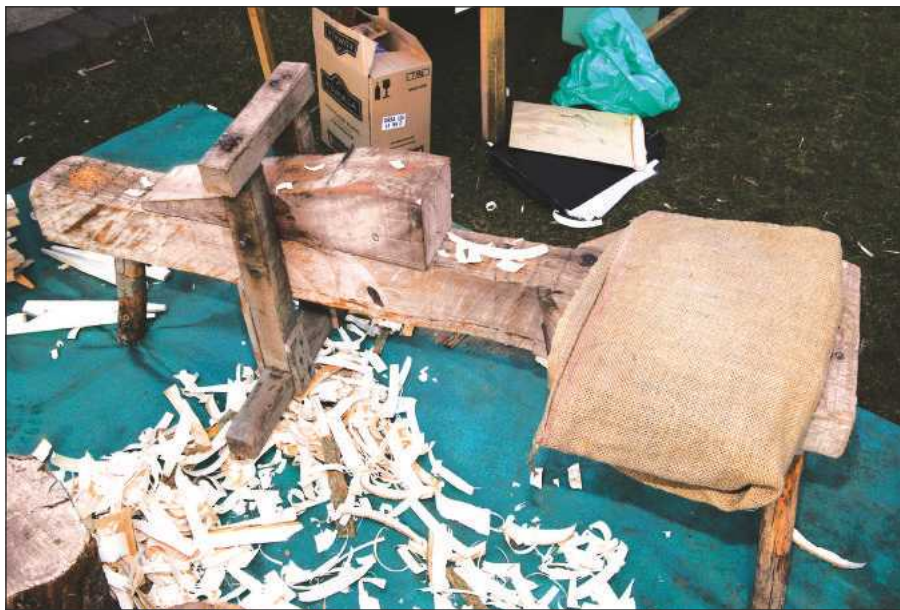
The shavehorse is a good aid when using the drawknife...
