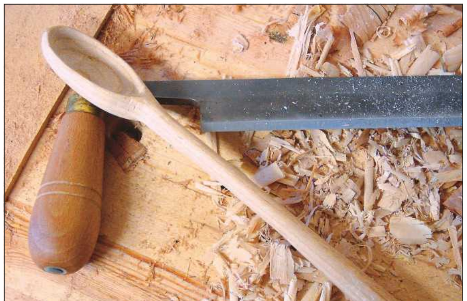
The drawknife is now my shaping tool of choice. It's what enabled me to create my elegant wooden spoons
