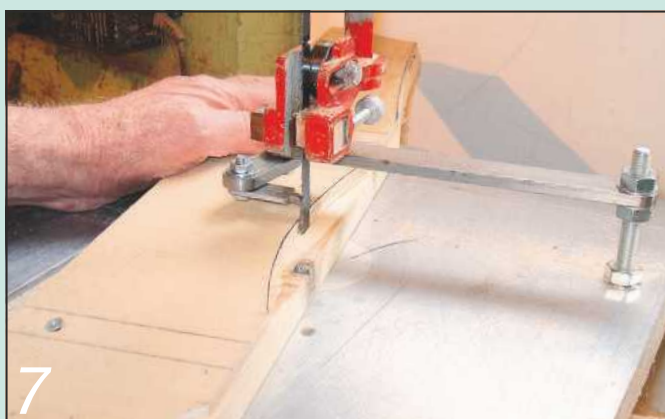
7 Bandsawing the end components with the template and the bandsawing jig
