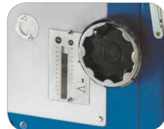
2 separate hand wheels for precise height & angle settings.
