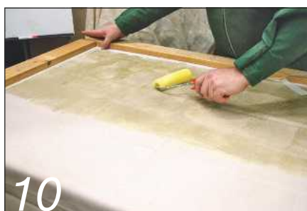
10 I applied two coats of contact adhesive to the canvas and the slats
