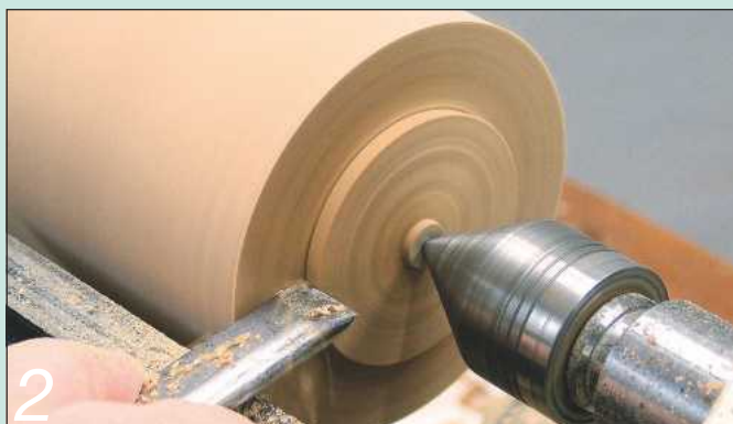
2 Square off and cut a spigot to fit your chuck on both ends of the blank
