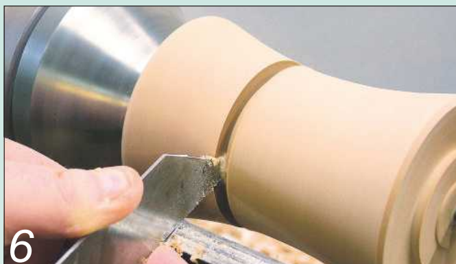
6 Use a narrow parting tool to part the blank into two. This will leave a tenon to the right of the cut; this will become the lip of the base
