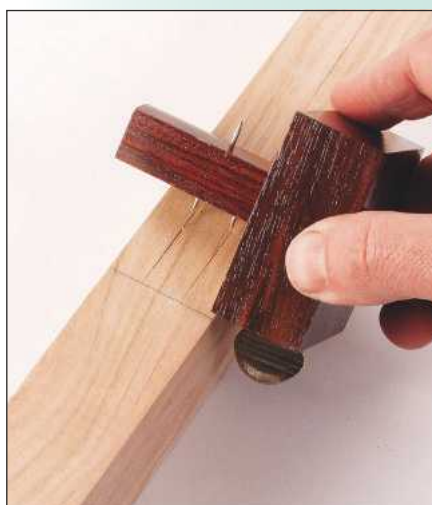
3 Choose a chisel whose width is close to one-third of the width of the stile, and use this to set your mortise marking gauge. Centralise the gauge and mark out the mortise. If cutting a through mortise, mark both sides. Put the gauge aside, but do not disturb the setting
