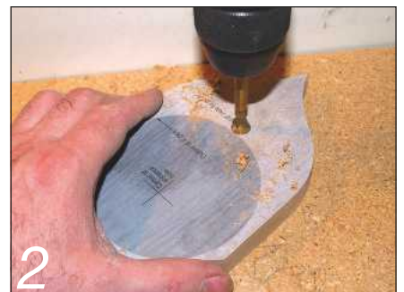
2 Chuck a 12mm bit in the drill press to create a perch hole in the front, and also one in the back
