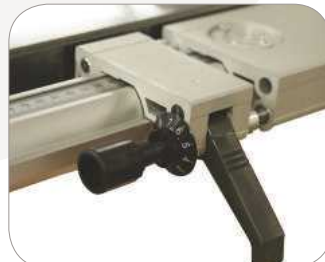
Micro fence setting scale to within 1/10th mm calibrations.
