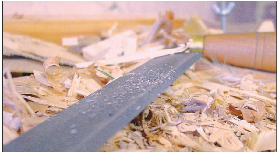
In appearance, the drawknife is essentially a chisel with two handles; it's perhaps better likened to a plane without a sole
