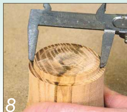
8 Measure the diameter of the tenon on the base using Vernier callipers...
