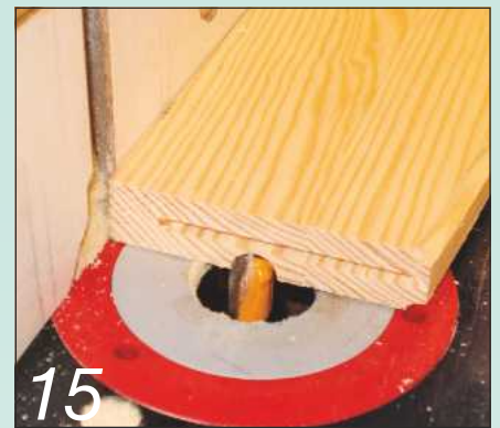
15 The cove cut to two of the shelves is also completed on the router table
