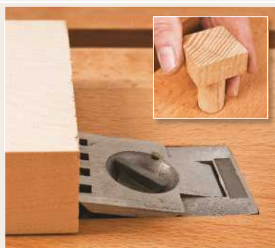
I also fitted a pair of recessed metal dogs at one end of the bench for extra versatility
