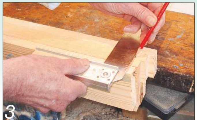
Marking out the length of all cross members while held in the vice
