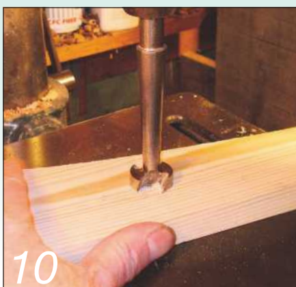
10 Boring the top rail for the hanging plate
