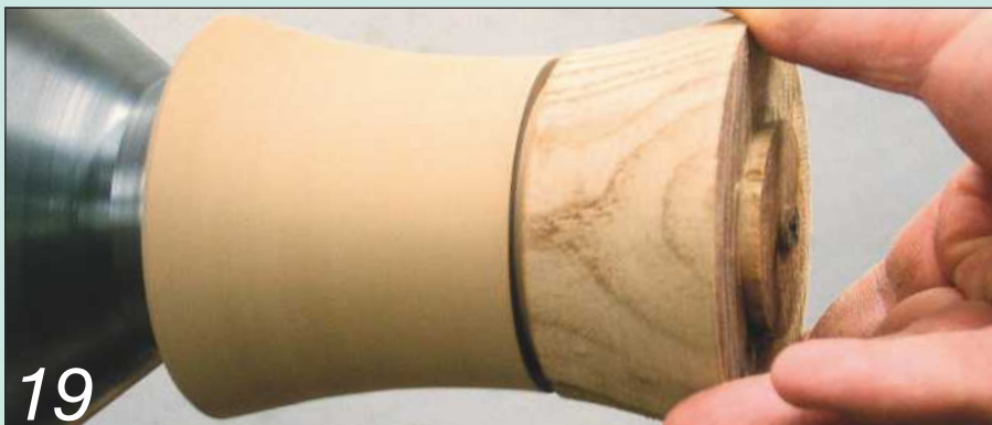
19 ... and offer up the lid. The lid should fit somewhere on the chamfer and if the lathe is running as you do this...
