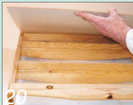
20 The back drops into the rebate before being secured with small pins
