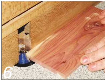
6 Cut the roof segments to length, then chamfer one edge of each segment to 45°
