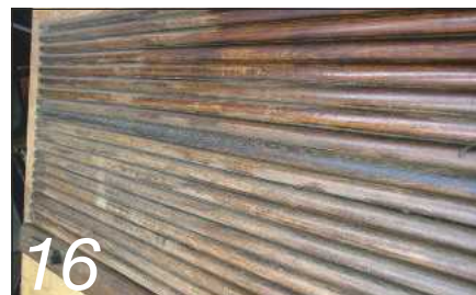
16 Here is the tambour back in one piece but looking patchy and worn
