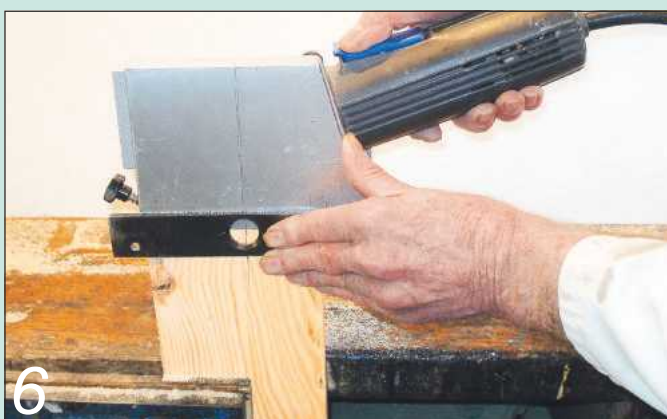
6 Forming kerfs for the biscuits in the ends of the cross members
