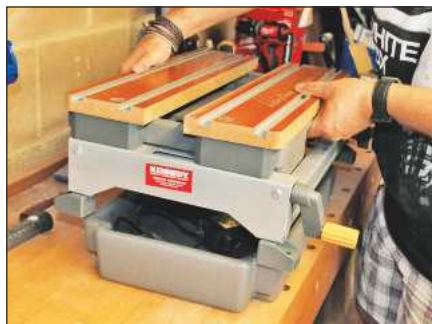
It also allows the work surface to be lifted away to access the lower storage
