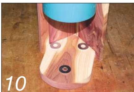
10 Lay the three washers inside and rest the plastic pipe on these
