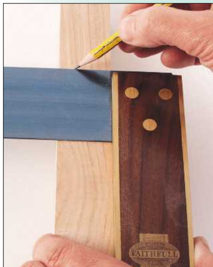
1 Use a try square to mark out the position of the mortise on the mortise member, or stile
