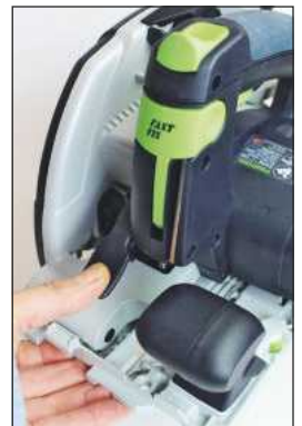
This lever controls the blade guard and will flip it back with ease
