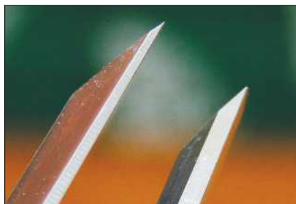
The 6mm chisel (right) has slightly thicker lands than the rest of the set
