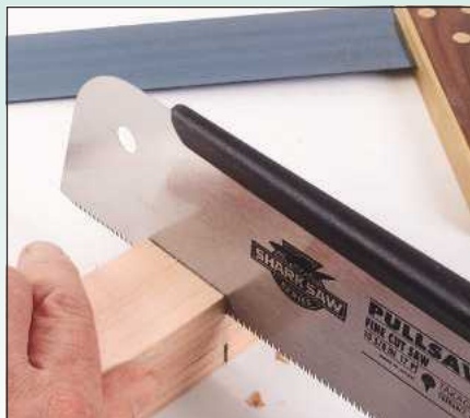
9 Now cut the tenon on the rail. Start by cutting the shoulders. Be careful to keep to the waste side of the marked line, and to stop before you cut into the tenon
