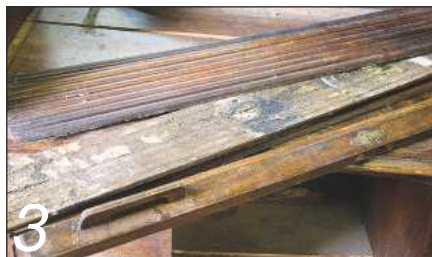
3 The broken tambour came in four pieces with brittle and torn backing canvas
