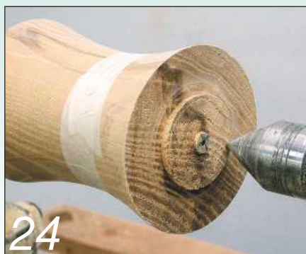
24 Mount the lid and base between centres, again with the lid at the tailstock end. Offset the centre of the lid by about 20mm
