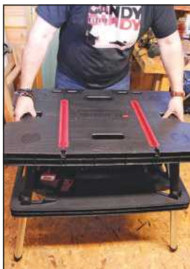
This hinged centre web clicks into place to lock the worktop rigidly
