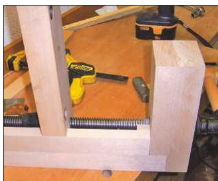
The construction of the tail vice laid bare
