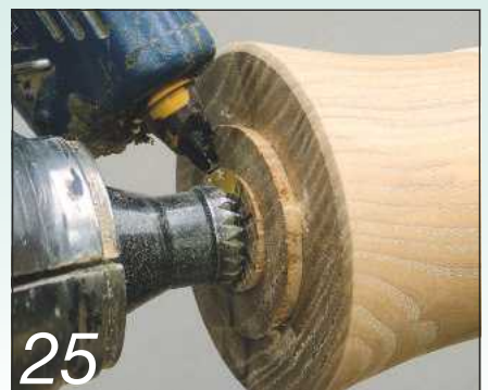
25 I used a Robert Sorby Steb centre in the headstock, but because only a few teeth are biting into the wood, use hot-melt glue to help secure it
