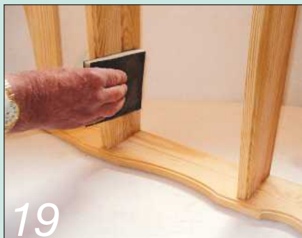
19 Flattening down between coats using an abrasive pad
