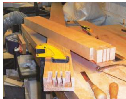
The front left-hand corner of the apron was reinforced using dovetail joints
