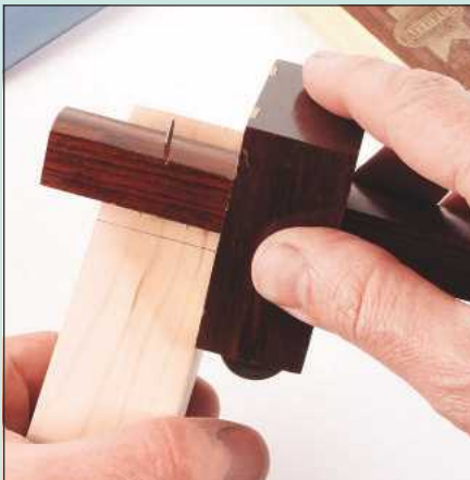
5 Using the mortise marking gauge as previously set, mark the tenon onto the rail. If the lines are very faint, run a sharp pencil along them to make them stand out more
