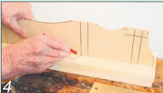
4 Transferring the shelf positions from the template to the ends
