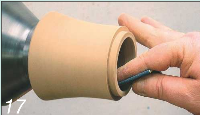
17 Sand the inside. When sanding the inside of a hollow, use only one finger like this and do not wrap the abrasive around the finger. Polish the inside
