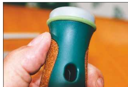
The plastic striking cap has a rubber shock absorption washer below it
