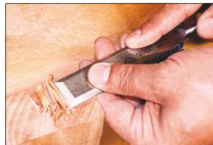
End-grain paring on a piece of beech is a cinch with these slender blades
