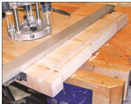
...and a tenon was formed on either end using a router and guide
