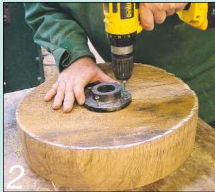
2 Decide which surface is to be the top and screw on the faceplate
