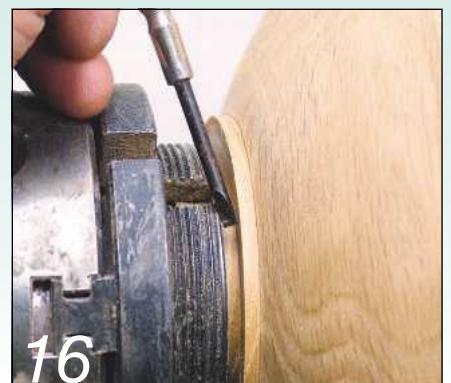
This gap allows the bowl to move, creating a weaker hold
