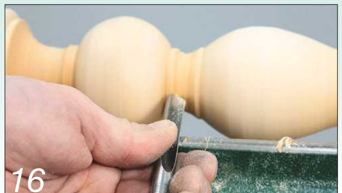
16 Cut the deepest coves last to maintain the spindle strength. Make the shoulders the same width, although not necessarily the same diameter
