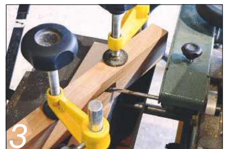
The slot mortiser on the Kity combi machine made easy work of the mortise
