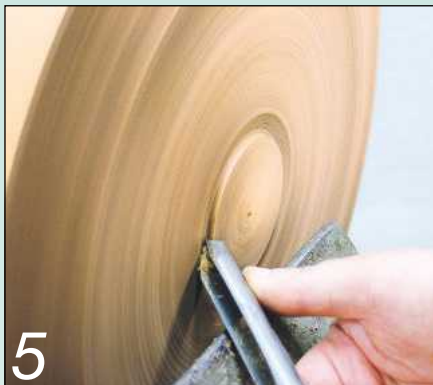
5 The tip of the gouge is used to start cutting the spigot
