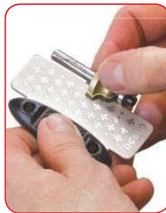
Specialist stone designed for router cutter sharpening.
