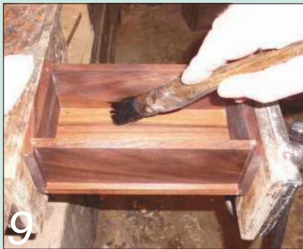
Box glued and cramped in the vice, removing excess glue with a small brush
