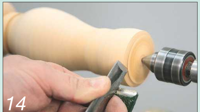
14 Clean up the top end using the skew chisel on its back edge to make a slicing cut down to the tailstock centre
