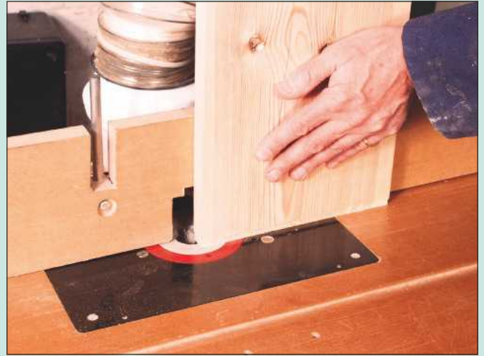
8 Position the fence so that the cutter will take a shallow cut and run the shelf board vertically past it. Machine both sides
