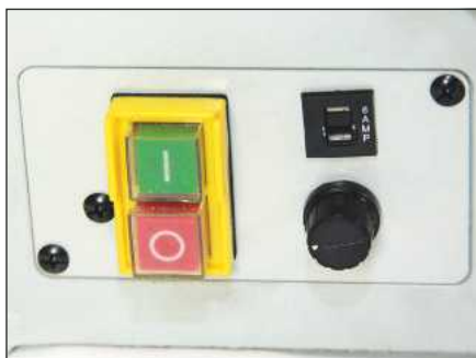
SS-12VS power switch and variable speed knob
