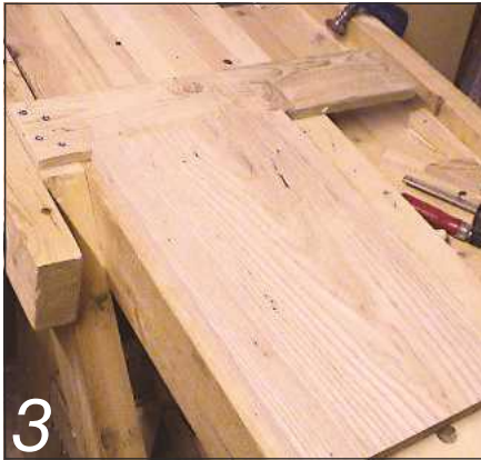
3 With a planing stop, you can rely on the downward force of the plane to hold the board in place
