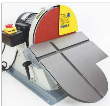
The DS12DLMB2 with its table tilted
