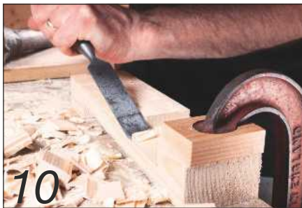
10 Chipping away waste with a chisel. The cross-cuts act as stops
