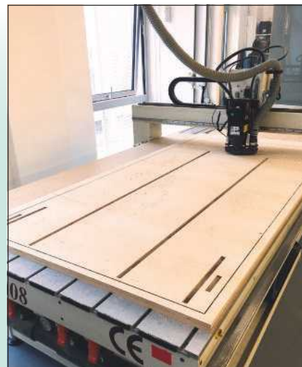
Cutting slots and grooving the underside of the table top
