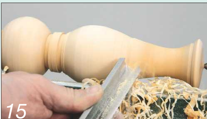
15 Form the bigger sections of detail using the spindle roughing gouge. Keep the bevel rubbing so that you're cutting off clean shavings
