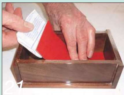
21 The inside of the bottom of the box is covered in baize
