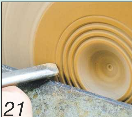
21 A series of grooves can help prevent the gouge from skating
