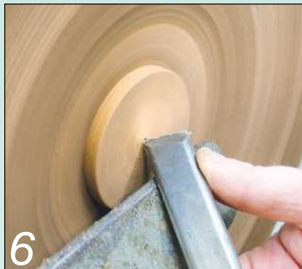
6 Use the point of the skew to cut a pop mark in the centre of the spigot
