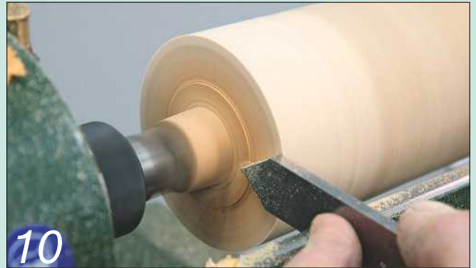
10 Slightly undercut the shoulder of the spindle to ensure that it sits down tight onto the base when the parts are assembled
