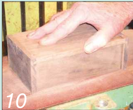
Rubbing box over abrasive sheet to gain smooth and flat upper edges
