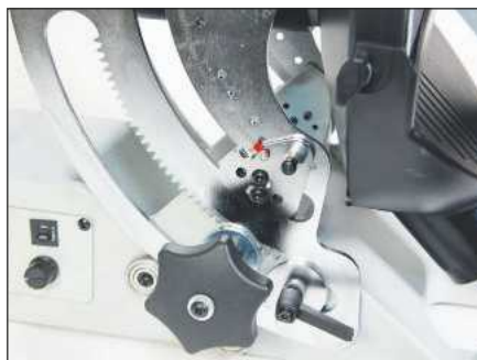
The SS-12VS's motor tilting mechanism
