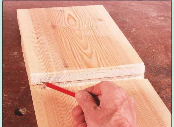
10 Lie the shelf board on the side panel and mark the end of the housing on it
