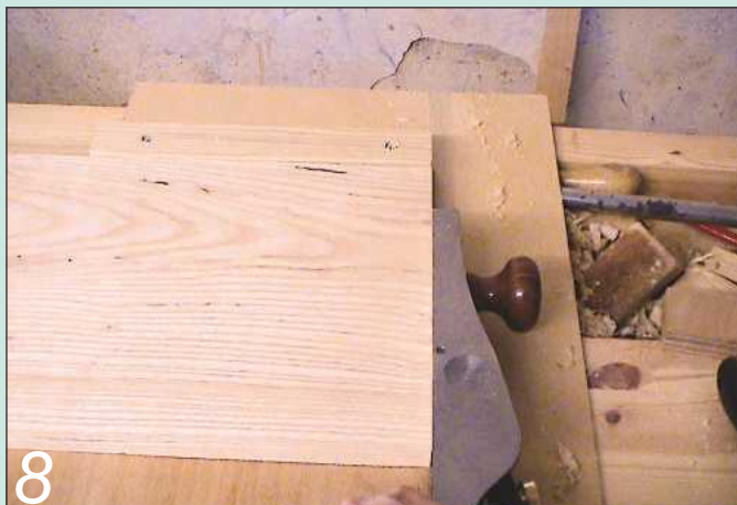
A shute, or shooting board, and a fiendishly sharp plane iron...
