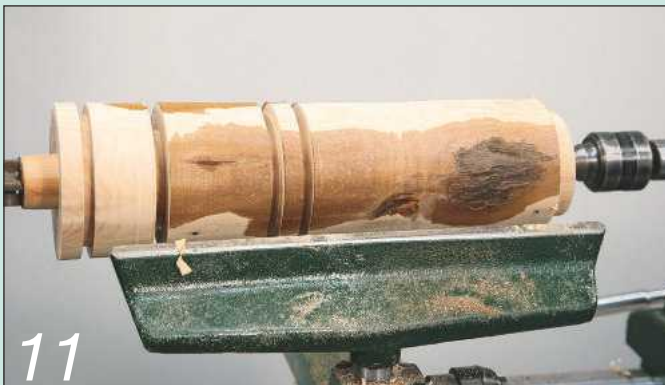
11 Use the parting tool to mark all the main changes of detail. This gives you an idea of the finished proportions of the overall piece
