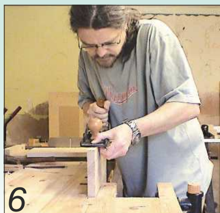
6 Successful edging: I hold the front of the plane body with my left hand, curling my fingers under the sole of the plane to act as a fence
