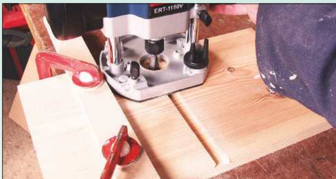
5 The housing does not need to be too deep and certainly not more than a third of the thickness of the side panel. Set the router to the required depth and place it on the edge of the workpiece. The joint must be cut with the cutter at full depth from start to finish. Plunge the cutter fully, start the router and move it smoothly into the work, keeping it hard against the batten. When you reach the end mark, stop the router and switch off. Do not release the plunge lock. Once the cutter has stopped spinning, pull the router back out of the cut
