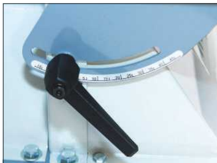
The DS12DLMB2's simple tilting mechanism
