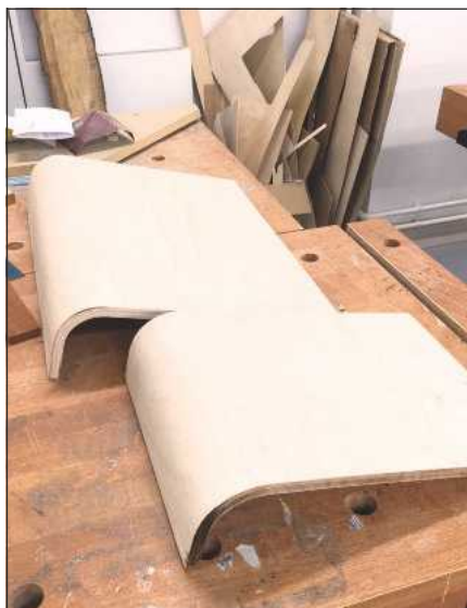
Developing the curved panels; the one in the foreground was rejected
