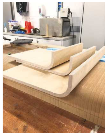
The final curved drawer fronts and the former they were pressed on
