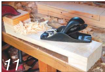
11 Levelling with an apron plane
