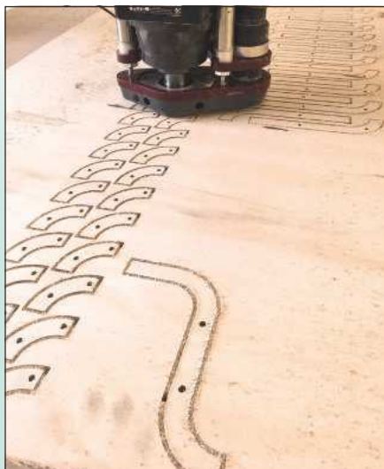
A sheet of birch ply is quickly converted into multiple table parts
