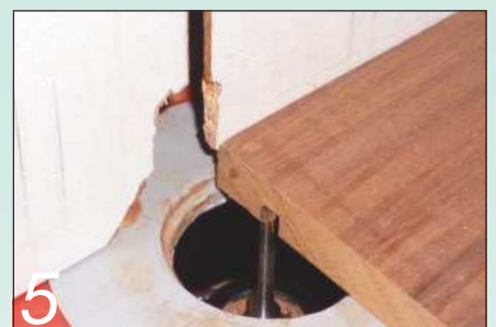
5 Using a piece of MDF to support the wood as it passes the cutter
