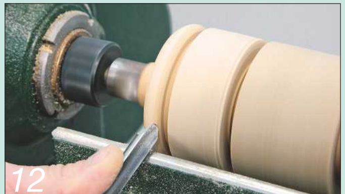
12 Use the 10mm spindle gouge to round over the bottom bead. Roll it fully onto its side to get into the tight corner by the shoulder
