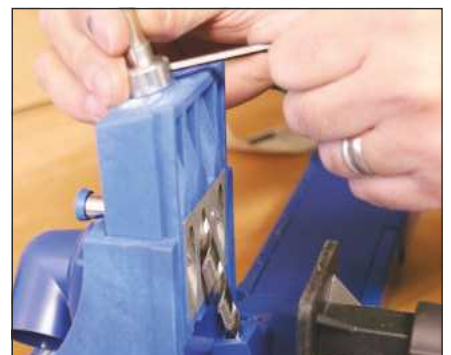
Once the guide block is at the right height, the drill can be set up with the stop collar
