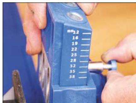
The spring-loaded indexing pin is used alongside the height scale on the side that relates to timber thickness
