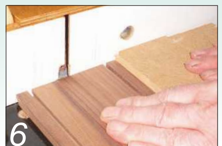
6 All joints are prepared on the router table
