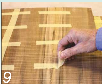
9 Out of the bag press, it's just a case of removing the tape as this particular veneer needs no cleaning up
