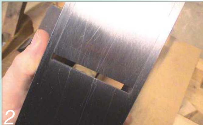
2 Grit or silica embedded in the timber will damage the sole of a plane
