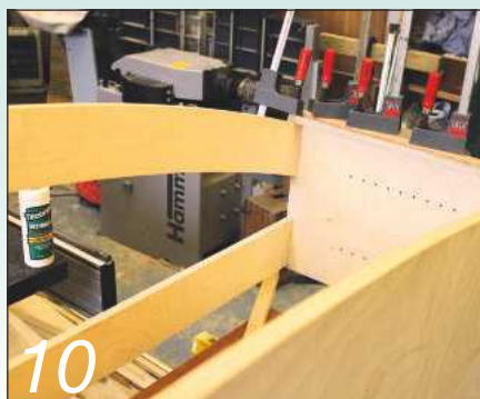
10 The carcass gets the side panels fitted. Note holes in the side for the adjustable shelf
