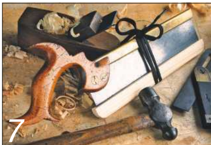
7 Edges are protected from blunting in the rough and tumble of the bench
