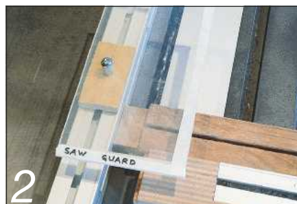
2 It's best not to run a workpiece against the rip fence while cross-cutting, as it can catch
