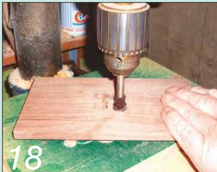
18 Most of the waste from the recess being removed on the drilling machine
