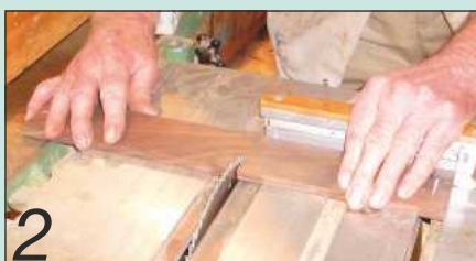
2 Cross-cutting to length – note that saw guard has been removed for clarity
