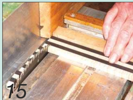
Sawing the lamination to give 10mm pieces
