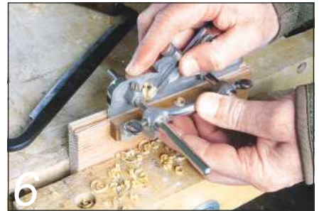
6 Ploughing a slot for a drawknife blade using the Record 043
