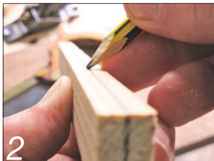
2 Mark the centreline freehand using your fingers as the fence
