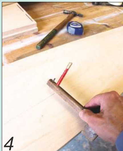
Using the front edge of the curved rail, the inner curve is marked out with a shop-made pencil gauge
