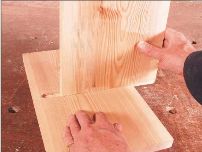
9 Check the fit, re-set the fence and take further shallow passes on each side of the shelf board until it is a sliding fit in the housing
