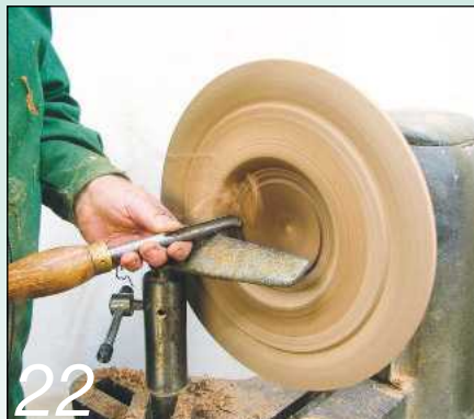
22 Continue hollowing, going a little wider and deeper each time
