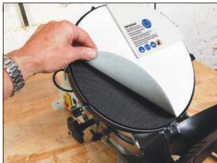
The SS-12VS uses a hook-and-loop disc
