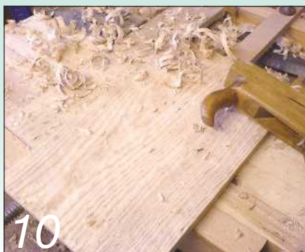
Use a scrub plane diagonally across the board to take down almost to the required thickness...
