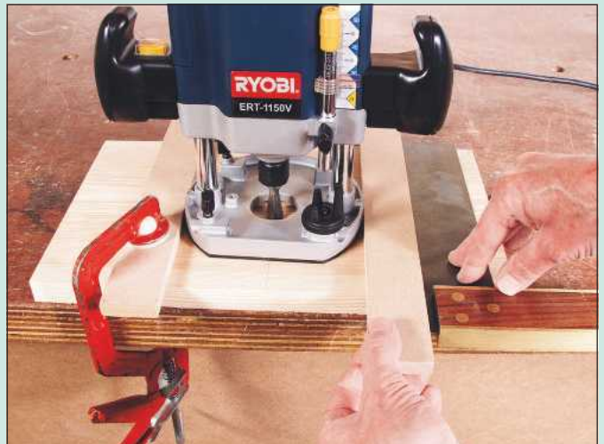
4 Using a try square, align a batten with the side of the router and clamp it in place. For added security, you can put another on the other side to sandwich the router, although this is not entirely necessary
