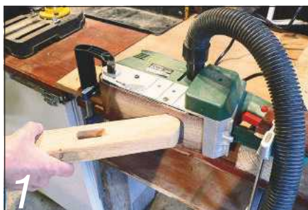
1 To round over the pole, clamp a sander to a bench and move the workpiece in an arc
