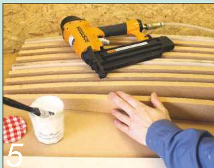
5 The curved former is built up of sawn and routed ribs with double ply to finish it off
