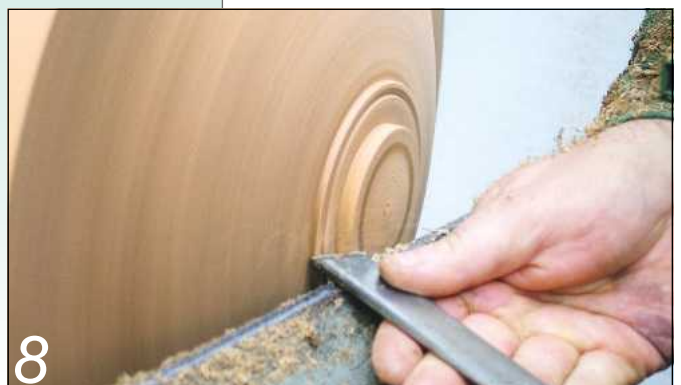
8 Cut a decorative bead on the foot with the skew chisel
