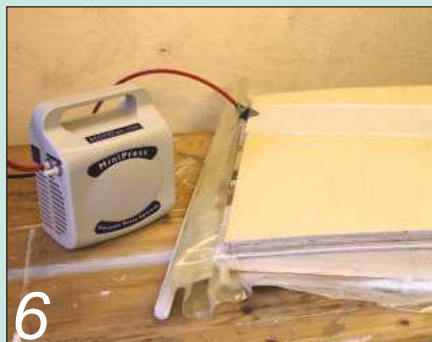
6 Laminating a curved door in the bag press: four layers of 4mm birch ply results in a nice door, and close to 18mm when veneered both sides
