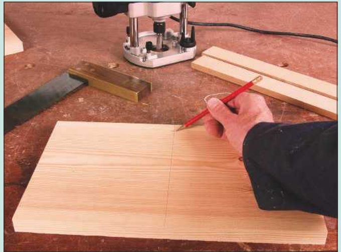
2 Unless you want the dovetail to show through on the front of the joint, you need to mark a point where the housing will stop. This should be 5-10mm from the edge
