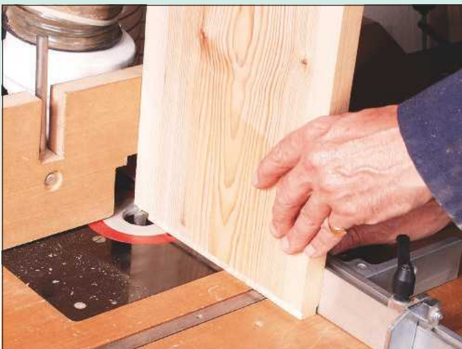
11 With the dovetail cutter set at the same height as before, move the fence back and take a series of cuts until you reach the marked line. Use the mitre fence to support the workpiece on the router table
