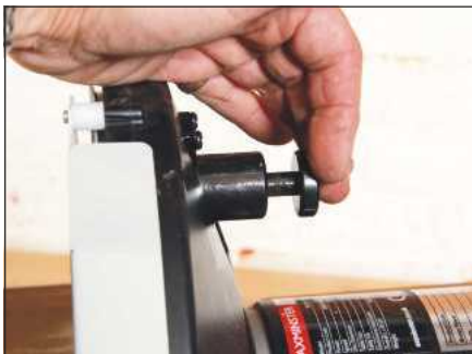
The SS-12VS's disc brake
