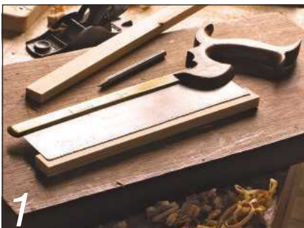
1 Use a slip of wood slightly longer than the blade for an edge guard
