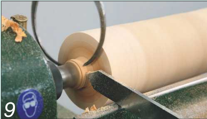
9 Use a pair of callipers and the parting tool to form a 25mm diameter pin about 20mm long on the bottom end of the spindle
