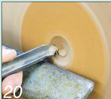
20 Swing the handle towards you and roll the tool up as it cuts down to the centre
