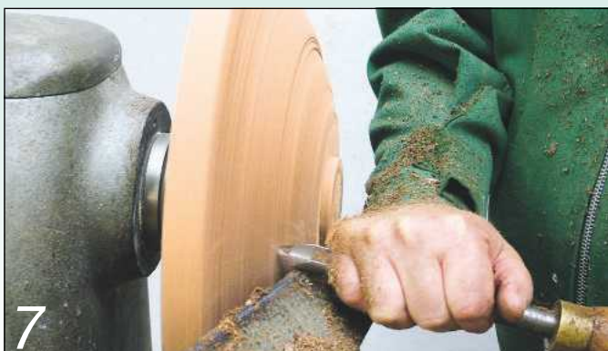
7 Shape the bottom of the bowl using both push and pull cuts
