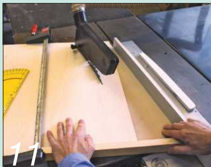
11 Cutting the triangle to achieve the sloping top. Repeat cuts are made with the template and board held in place with a sacrificial batten
