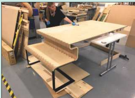
The first coat of Osmo oil goes on
