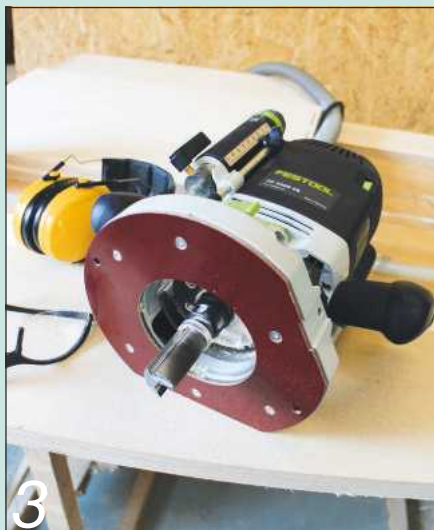
A template follower cutter on a big router will form a professional curve
