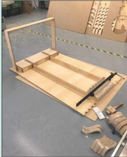
The table takes shape as the central section of 'S' blocks is cramped up
