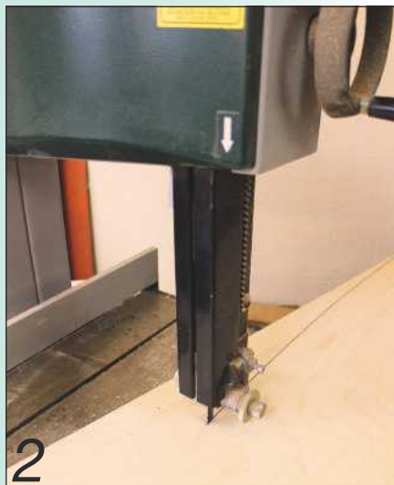
For a long and gradual curve, a steady hand is required on the bandsaw
