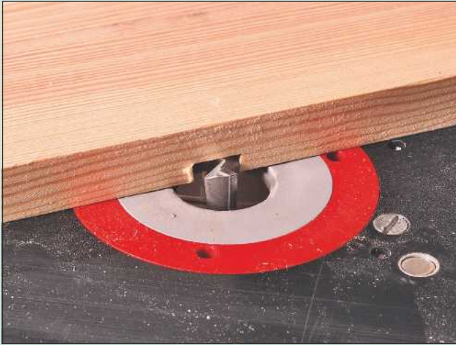
7 Fit the router cutter into your router table. To set the depth, lie the machined board on the router table and raise the cutter until it just touches the bottom of the housing
