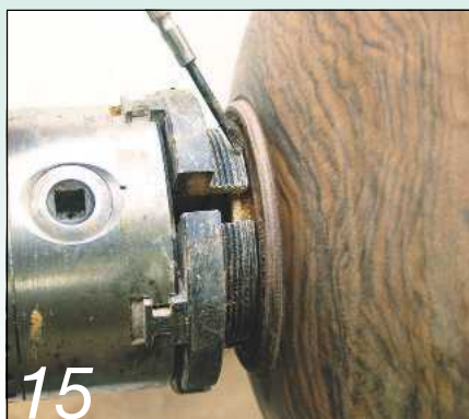
The bottom of the bowl should sit on top of the jaws
