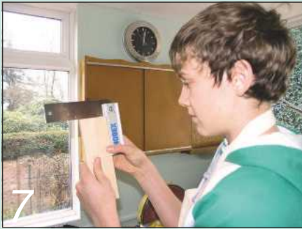
7 Use a try square to check that all the cut ends are a perfect right angle
