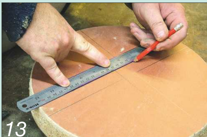
Mark lines parallel to the diameters that are half the width of the 3x2s
