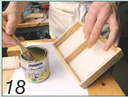
18 Fit the divider and varnish the tray inside and out
