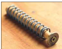
14 The sub's component parts; note small block to retain firing spring
