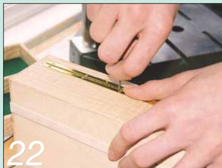
22 Screw the hinge in place, taking care to drive the screws in square
