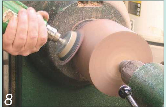
8 Power sand to a finish
