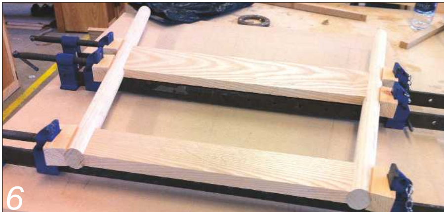
The end frames are clamped up; note that the clamp blocks are also profiled to improve grip and reduce glue-up stress!
