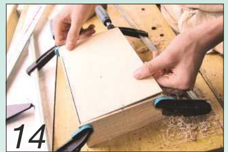
14 Glue the plywood top into place in the cramped-up box assembly
