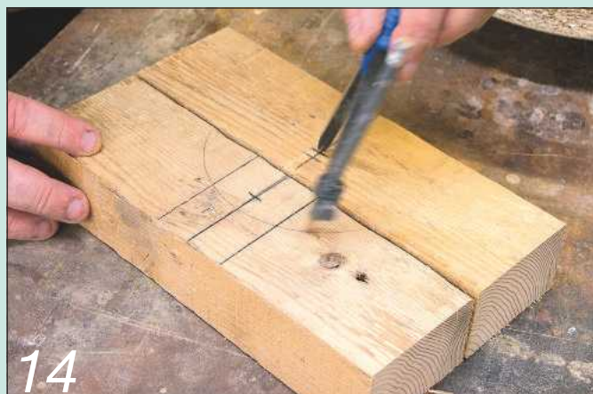
Mark out the 3x2s as shown
