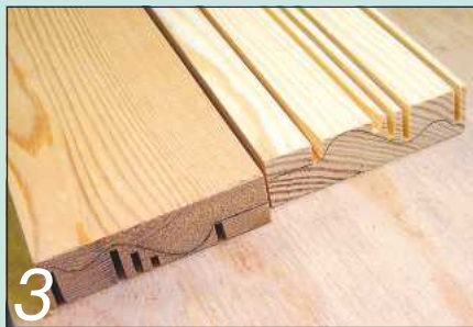
3 Initial table saw cuts mark the extent of the main curves
