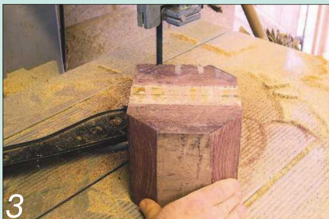
Removing the corners of the blank makes the initial turning easier
