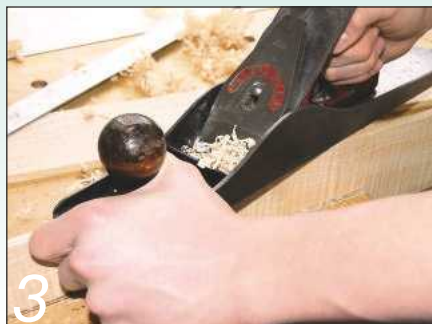
3 Plane one edge true before sawing the thickened boards to width
