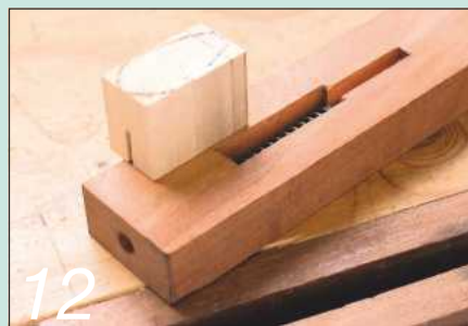
12 Conning tower roughed out and slotted for the brass trigger bar
