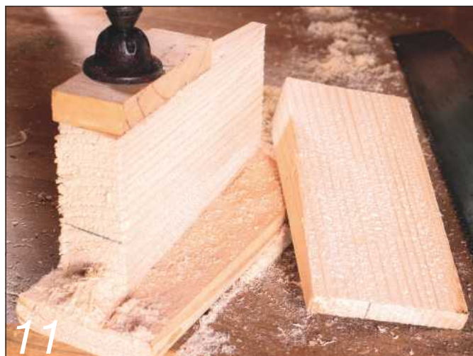
11 Making wedges is also useful practice with the hand saw
