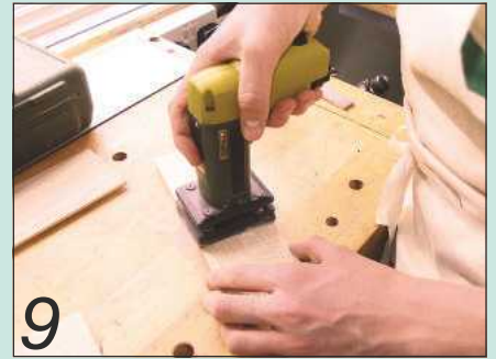
9 Another sanding session will remove any whiskers left by the router
