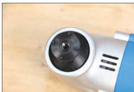
A mounting shaft makes it easy to attach accessories, using an Allen bolt and washer
