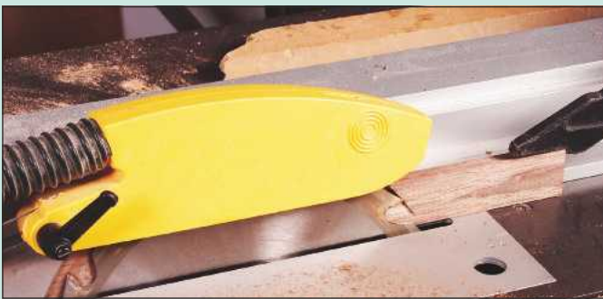
14 Set the rip fence a little wider than the base of the dovetail, and with all guards securely in place, rip down both sides of your timber to make the splines. Make up a long length, and trim it to size later
