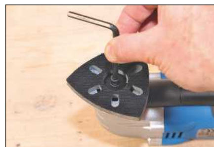
Fitting a sanding pad can be a bit of a fiddly process
