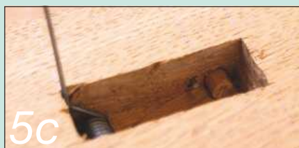
Detail of how the firing rod clears the spring leg of its retaining pin
