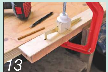
13 Working out the optimum trigger position by trial and error
