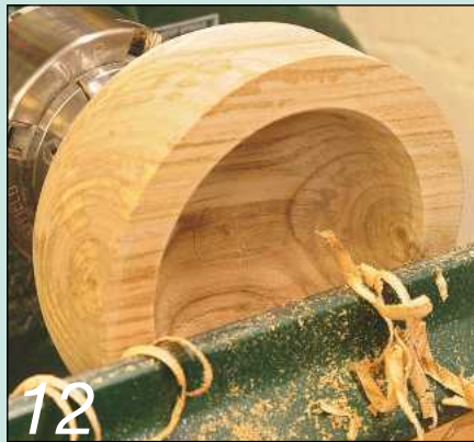
12 Rough turning the blank while it is still wet will speed up the drying time...
