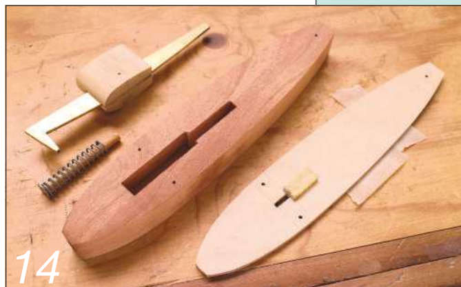
14 The sub's component parts; note small block to retain firing spring
