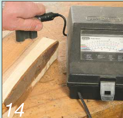
14 A moisture meter will let you know what is going on only at the point of testing
