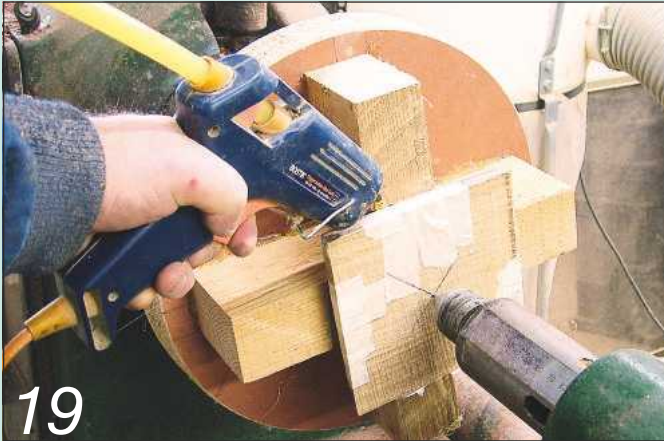
Hot melt glue one of your bowl blanks into the cradle
