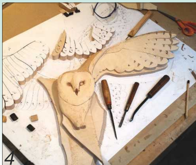
4 Carving the body of the owl is completed using a variety of tools and an Arbortech Mini Carver power tool
