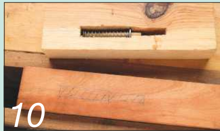
10 Torpedo firing mechanism softwood trial and hardwood marked out ready. Note wedged washer to reinforce spring-stop shoulders
