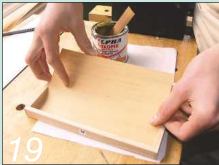
19 Glue in the veneer on the underside of the lid with a contact adhesive
