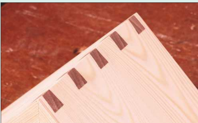
19 Finally, clean up the joint with a plane then fine abrasive paper
