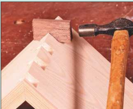
16 Cut the splines into short lengths, apply a little glue and gently drive them into place with a hammer
