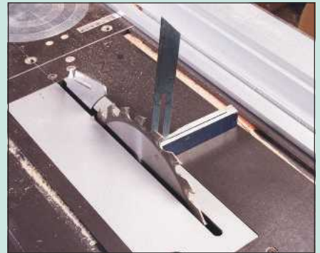
13 Transfer this angle setting to your table saw. Please note that the crown guard has been removed for clarity
