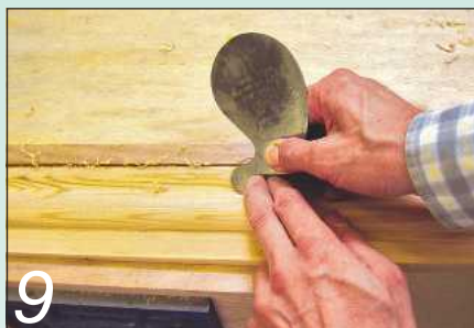
9 A curved cabinet scraper is ideal for this part of the task
