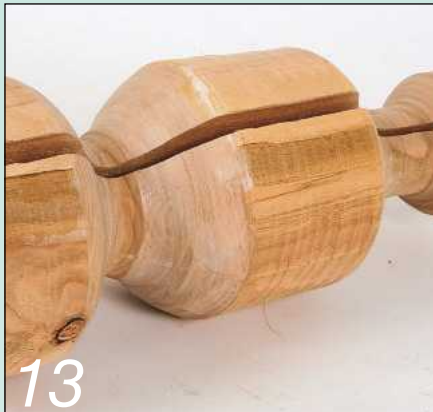
13 ... but you still need to seal the ends and even then expect a few failures
