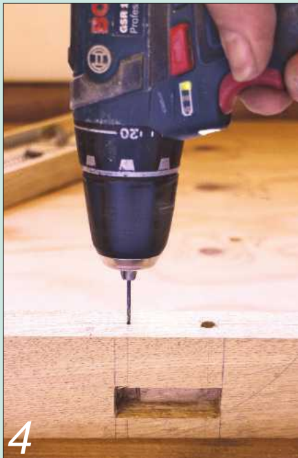
Drilling a guide hole for the one of the pins, which will keep the main spring in position
