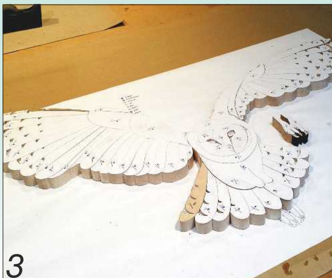
3 When all the pieces have been cut using the scrollsaw, they can be resassembled to create the shape of the owl, as shown here
