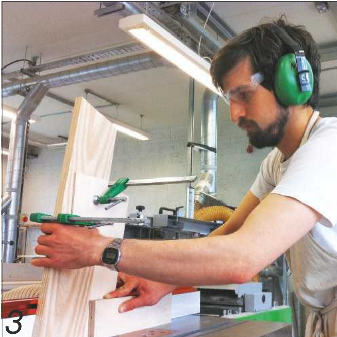
3 The ends of the rails are profiled on the router table to form the concave necessary to meet the legs
