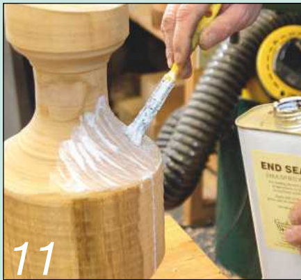
11 Coating the end-grain with cold liquid wax to slow down the drying process
