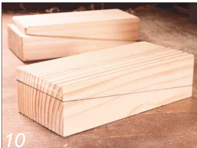
10 Spruce offcut marked with a 1 in 8 gradient for folding wedges
