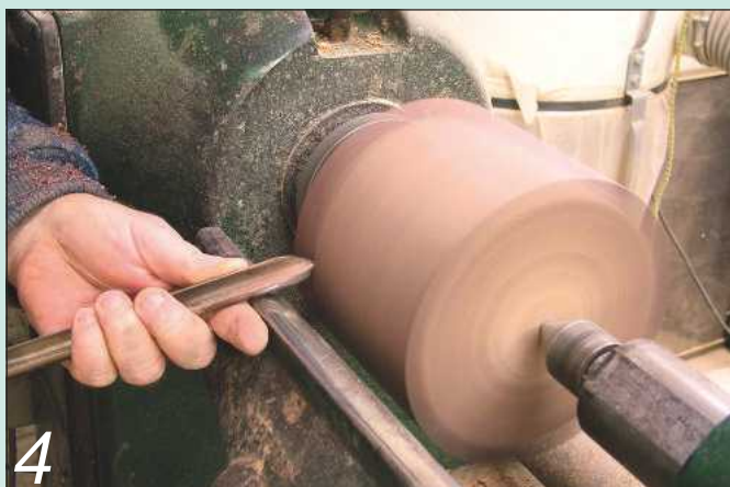
A bowl gouge gives a cleaner cut than a spindle roughing gouge in this instance
