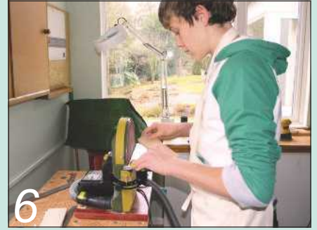
6 True up all the cut ends using a disc sander
