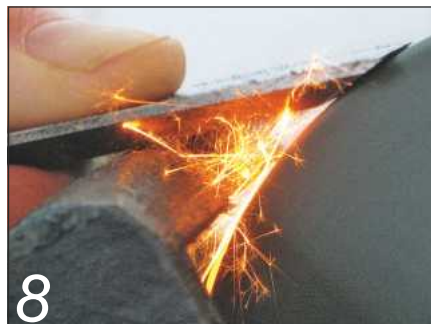
The swarf flies mainly downwards towards the operator's feet
