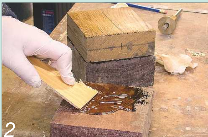
Glue the two bowl blanks to the sacrificial block
