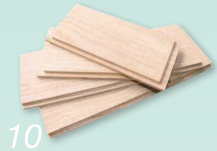
10 The four box side components with all the rebates prepared and checked
