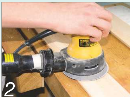
2 Sand the thickened wood with an orbital sander before cutting it to length
