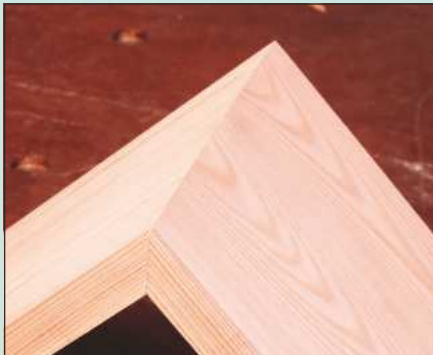
1 Clamp your mitre joint in the bench vice so that it faces upwards
