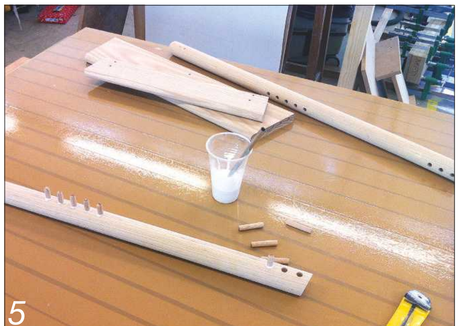
5 Multiple dowels provide a large gluing area for necessary strength
