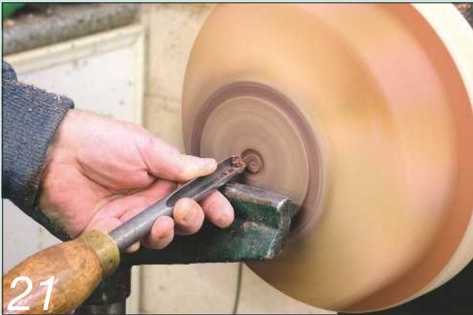
Hollow the bowl in the normal way
