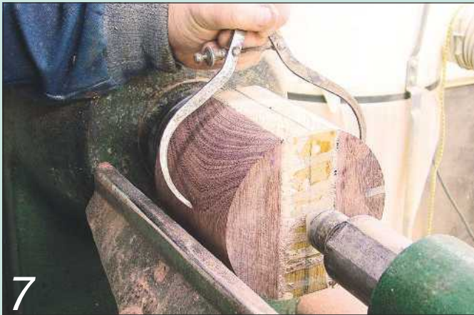
7 Make sure the blank is not tapered
