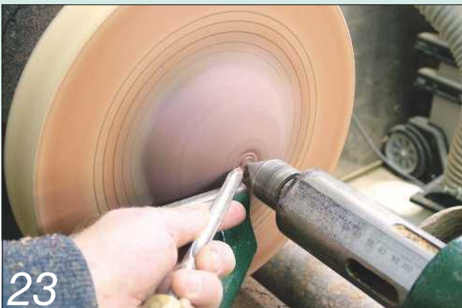
Reverse the bowl and cut a small flat for it to sit on
