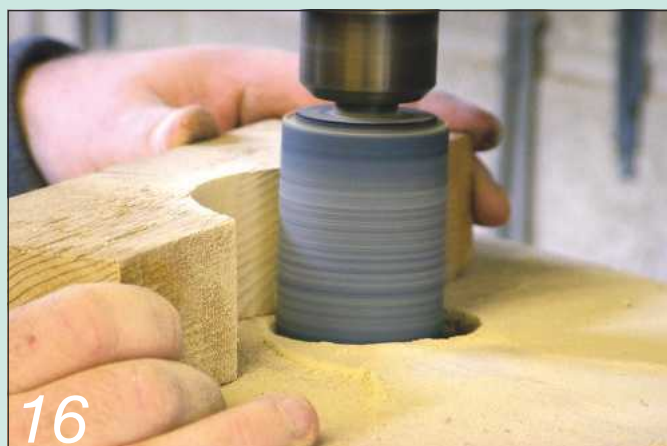
...and sand smooth using a drum sander
