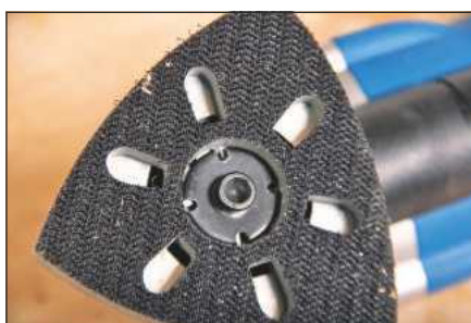
Pad fitted showing slotted washer
