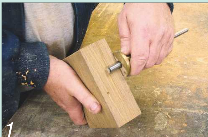
Mark a centreline around the sides of the sacrificial block
