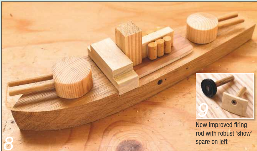
The superstructure is now in place; note hole for firing rod
