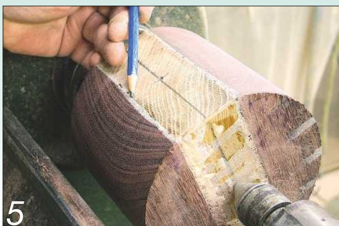
Stop when the curve reaches the waste wood
