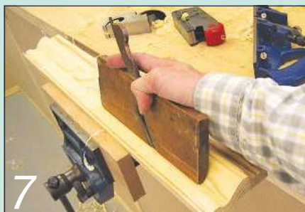
7 The replacement moulding soon begins to take its final shape
