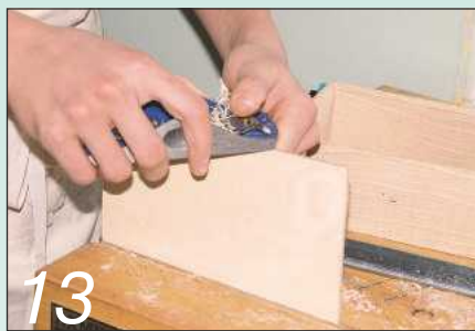
13 Plane the plywood for the top using a low-angle block plane
