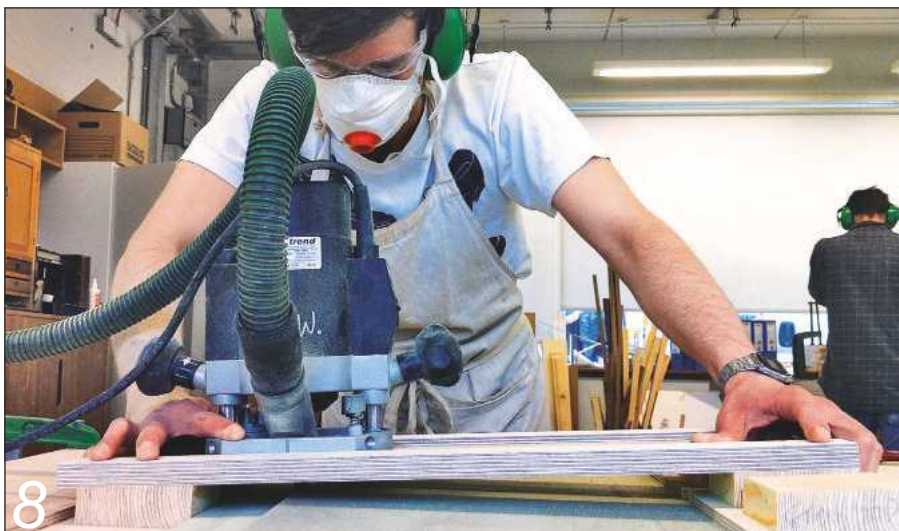
Here the chamfer routing jig is seen in use at the start of a bit of a routing marathon
