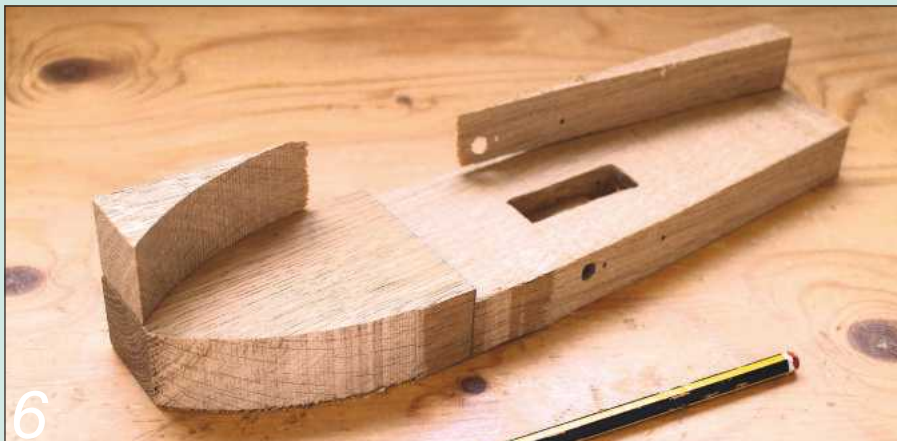
Shaping the destroyer's hull; note use of offcuts to mark out the starboard side
