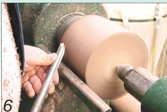
Light finishing cuts remove any torn grain and leave you with fine shavings
