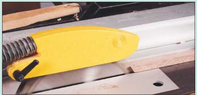
15 To adjust the fit, lay the timber on its side and with the blade still tilted, take shaving cuts off the bottom until the piece will just tap into the dovetail sockets with a light hammer
