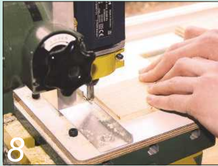
8 Rout the rebates on the box ends with the router mounted overhead. Guard removed for clarity
