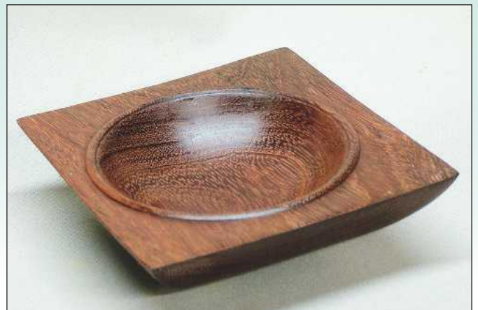
I used a skew chisel to cut a bead at the rim
