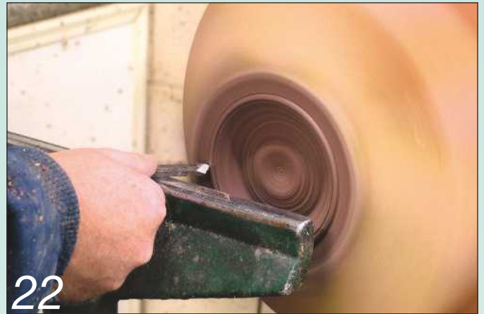
I used a skew chisel to cut a bead at the rim
