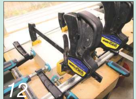
12 Cut the base to size, then glue and cramp up the box assembly
