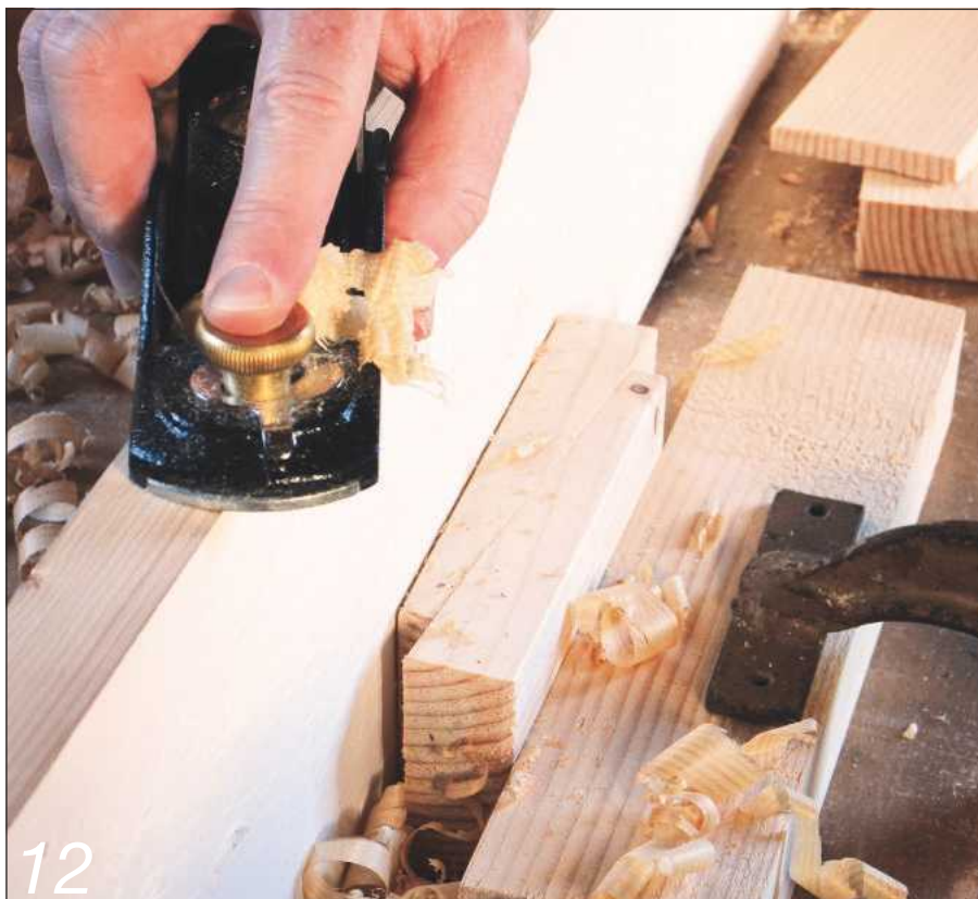
12 Folding wedges supporting a board on edge for planing. Who needs a vice?
