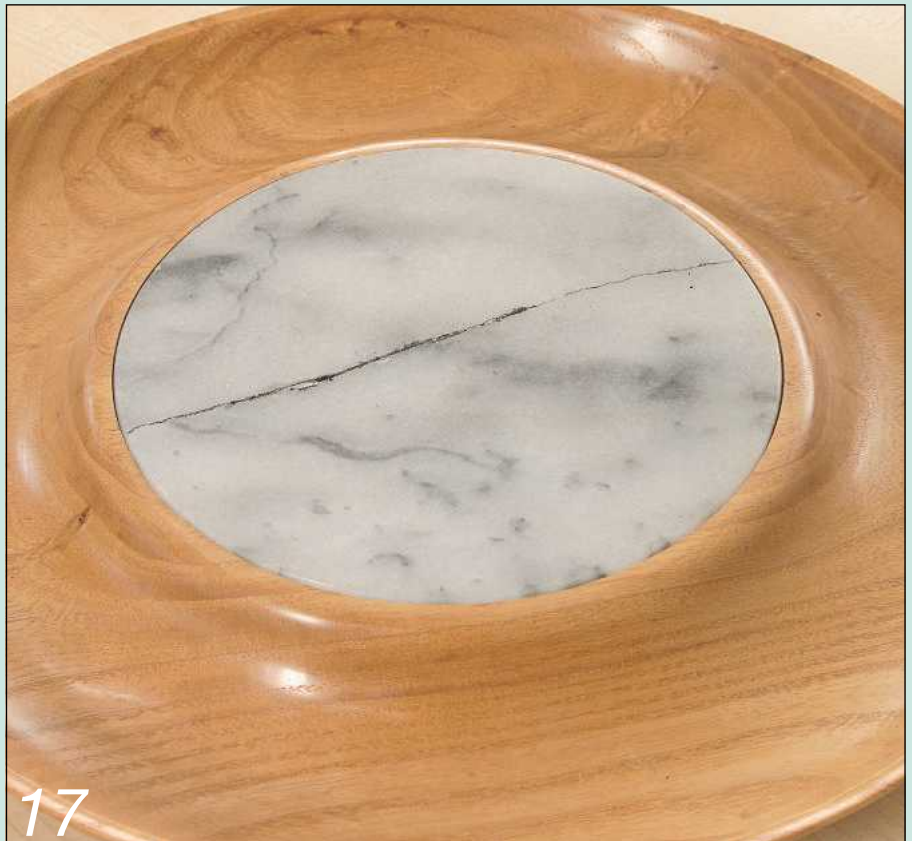
Bowls can warp with enough force to crack a marble insert
