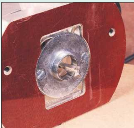
6 In order to set up your jig accurately, make a setting bar. This should fit snugly in the guidebush groove and have its centre clearly marked
