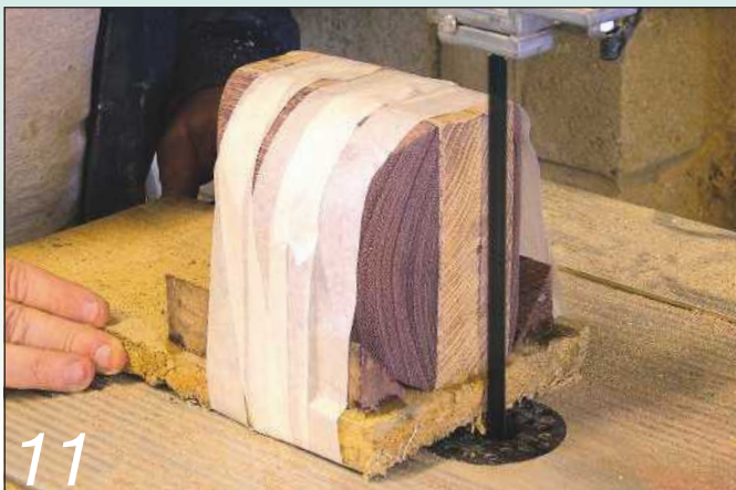
11 Keep your fingers away from the blade by mounting the work on a piece of scrap
