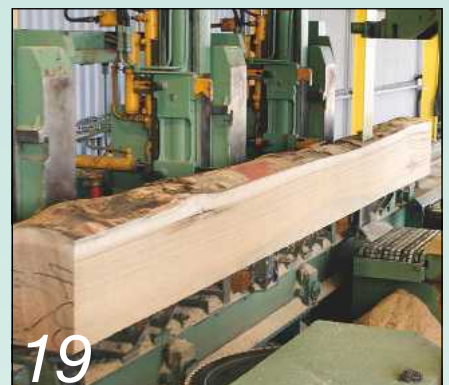
Bandsawing a log is much the same as it would be done at home but the blade is a bit wider
