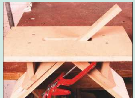
8 Clamp the jig in place
