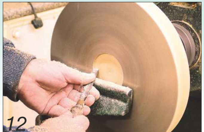
12 Turn a chucking recess on the plywood disc
