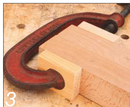
Clogs protecting the work while clamping
