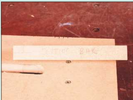
6 In order to set up your jig accurately, make a setting bar. This should fit snugly in the guidebush groove and have its centre clearly marked
