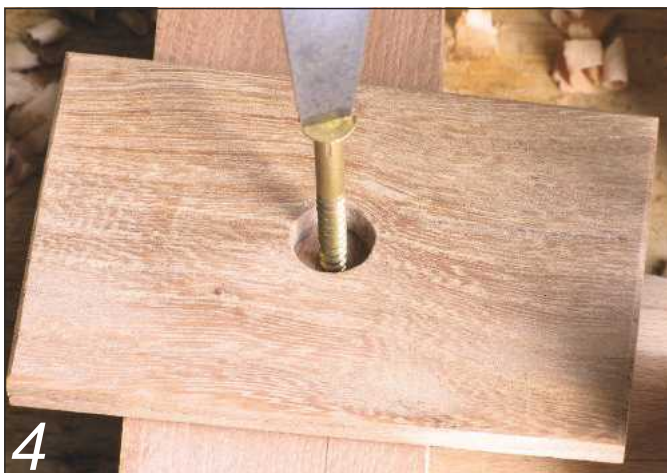
The screw guard protects the work if the blade slips from the slot
