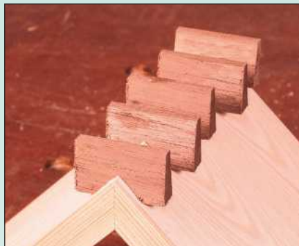
17 Here you can see the oversize splines in place
