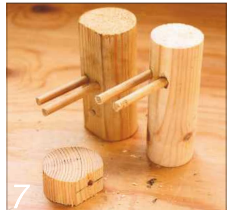
The gun turrets are best drilled over-length then trimmed down afterwards
