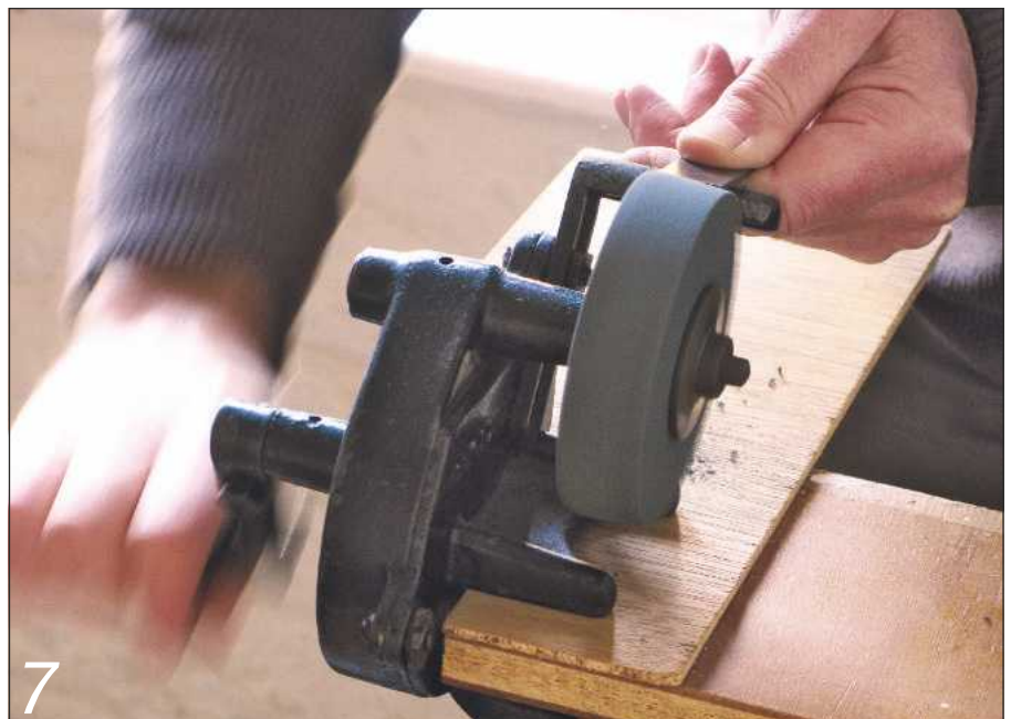
The plywood swarf catcher slots around the hand-powered grinder
