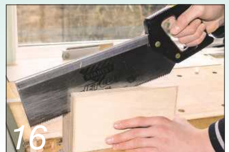
16 Use a fine-toothed saw to part the top from the bottom
