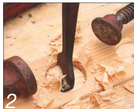
Clogs for a G-clamp, bored with a centre bit
