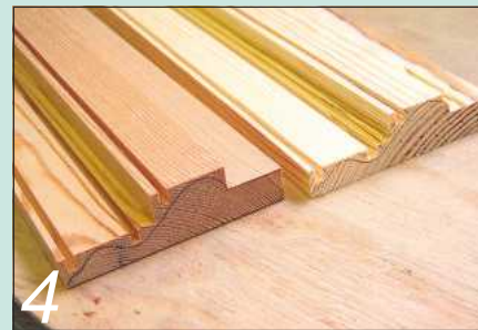
4 The bulk of the waste can then be removed on the saw bench
