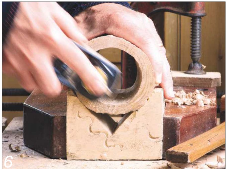
A pallet block with a 'V' channel holds round work when planing end-grain
