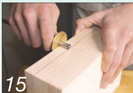
15 Use a marking gauge to indicate where the box is to be cut in two
