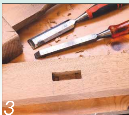
3 The mortise housing is chopped out for the torsion spring
