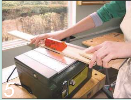
5 Cut the boards to width on the circular saw. Note the use of a push stick
