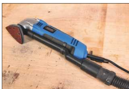
Ready for sanding with extraction fitted
