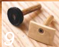
New improved firing rod with robust 'show' spare on left
