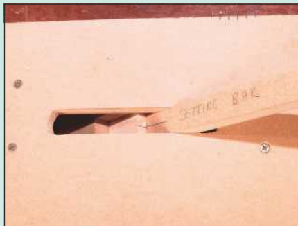
7 Insert the setting bar through the jig and line it up on the marked lines
