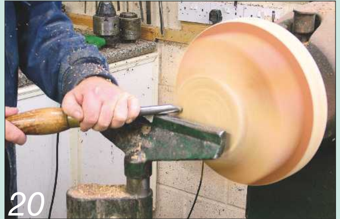
Use a pull cut to flatten the top of the bowl
