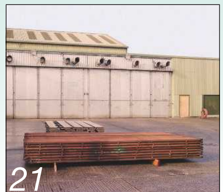
Drying kilns are like huge ovens with both humidity and temperature control
