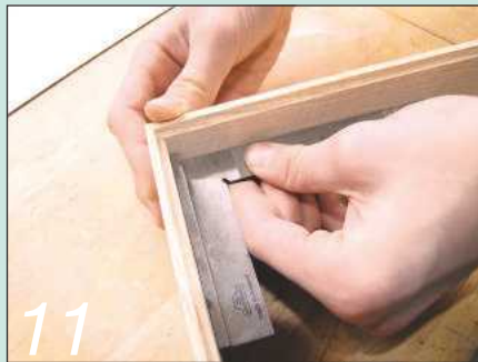
11 Assemble the box dry and check that all the corners fit squarely
