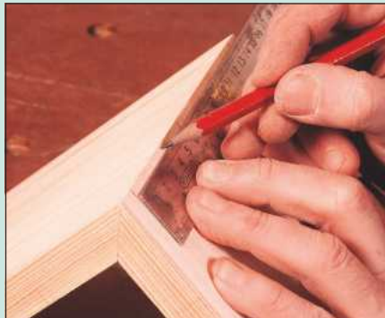
2 Mark out the dovetail spacings across the joint. Keep the outside splines away from the edge, so start by marking a line about 10mm in from each edge for the outside pair, then divide the space between these lines equally across the joint
