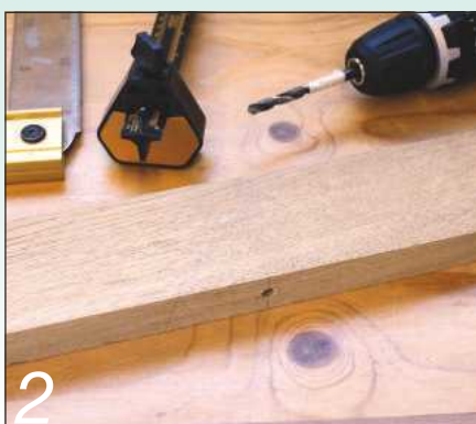
2 The boat blank, carefully marked and drilled for the firing rod
