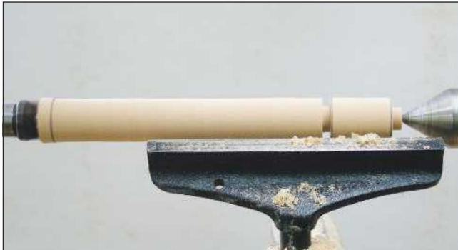
1 Cut a groove with the parting tool just to the left of your 30mm line
