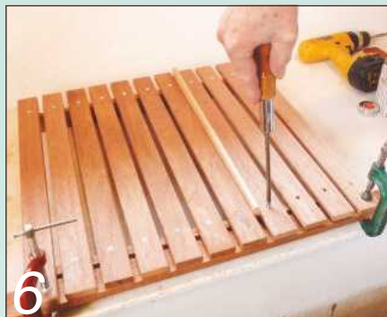
6 Screw the slats to the bearers. Note the spacer, and the cramped batten to aid alignment
