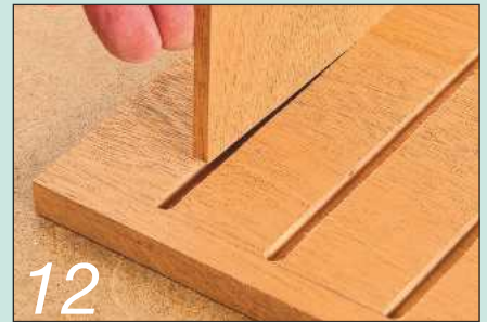
12 Thickness the shelf material down so each one is a smooth sliding fit in its grooves
