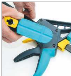
The jaws are fitted with soft pads that are grooved to hold round stock
