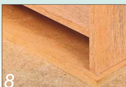
8 The intermediate shelf is fitted in place with two biscuits at each side
