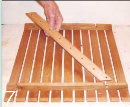
7 Screw the diagonal brace to the underside of the top after drilling the clearance holes
