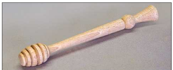
5 Part off the dipper and use abrasive paper to sand both ends smooth
