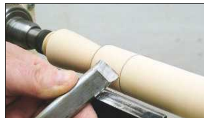
10 Use just the long point of the skew to cut the left-hand side...
