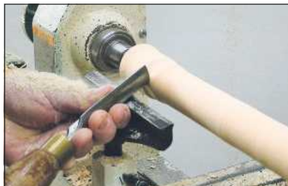
3 For the last 50mm, change direction so you always start with the tool on the wood
