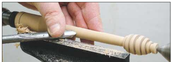
4 Damp down any vibration caused as the wood flexes away from the tool by supporting it with your fingers
