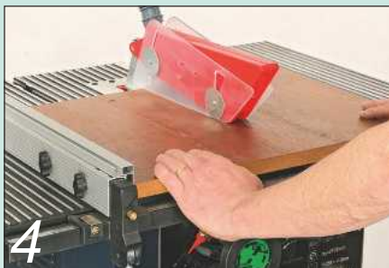
4 Rip the widened boards down to the required widths
