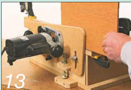
13 Round over the shelf edges using a tall temporary sub-fence as a support
