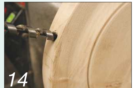
14 Drill an 8mm diameter hole in the edge of the platter to take the handle dowel
