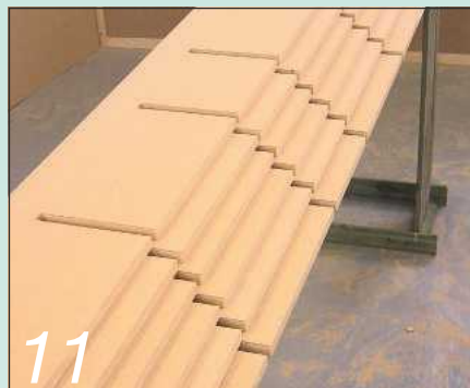
11 All the sides and centre uprights were at last fully prepared for assembly
