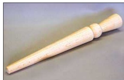
18 Clean up the ends with abrasive paper and your spurtle is ready to use
