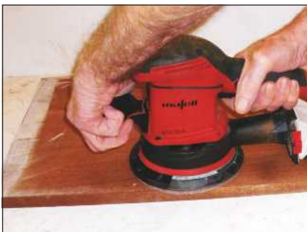
The coarser grades are ideal for heavier-duty sanding jobs
