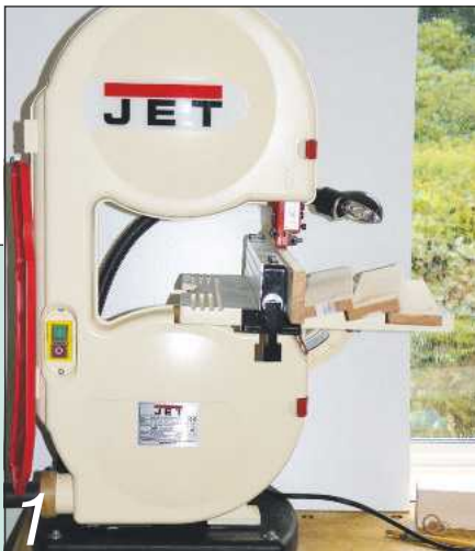
1 A small Jet bench-top bandsaw saves a good deal of floor space
