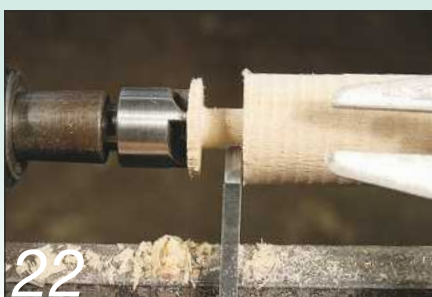
Use a parting tool to form the dowel on one end of the cheeseboard handle
