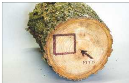
1 Mark out your blank to avoid including the pith in the centre of the log
