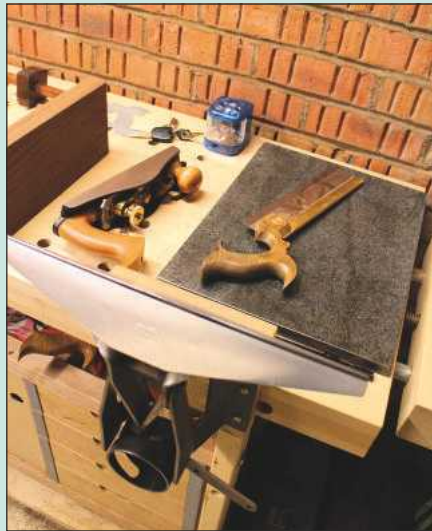
Shane uses these jaws for metalworking and a granite slab for final dressing
