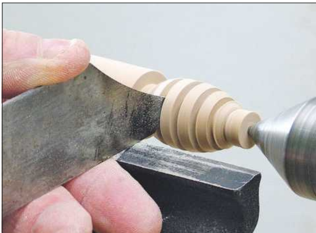
3 Then cut a series of parallel grooves in the egg shape using a narrow parting tool
