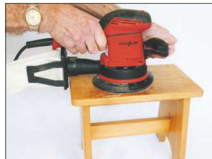
Fine abrasives are best used for final sanding of existing finishes
