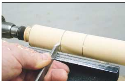
5 Use a parting tool to cut grooves to the left of the first two lines
