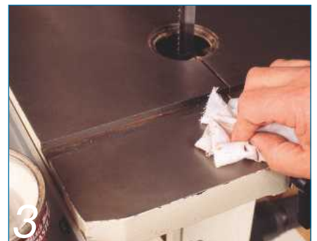
3 Keep the table clean, and protect it from rust by maintaining it regularly
