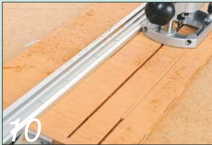
10 Lock the two halves together with a wood strip while making subsequent cuts
