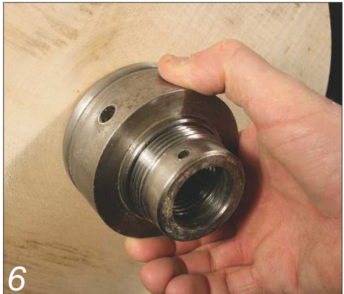
6 Test the fit of the expanding chuck in the recess
