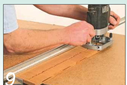
9 Cramp the two sides together side by side and machine the first slot for the shelves
