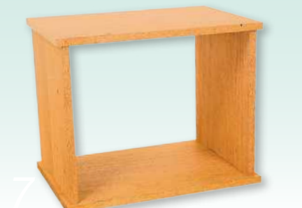
7 Assemble the main carcass dry to test the fit, and do any necessary trimming
