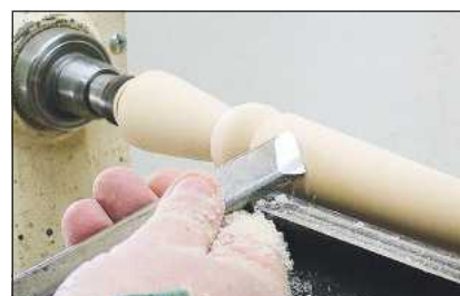
16 Start each successive cut a little further to the left, working towards the handle
