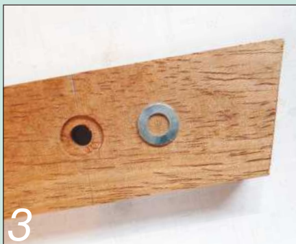
3 Bore a shallow hole for the washer at each rivet position, then drill the rivet hole
