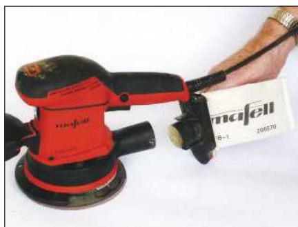
The sander can be used with a dust bag or a vacuum extraction hose
