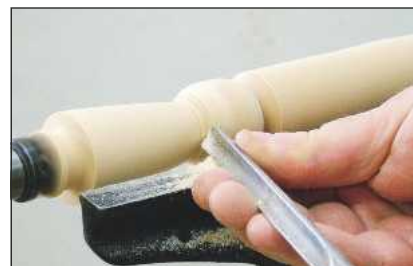
14 ...but you still need to swing the handle as the tool cuts the bead
