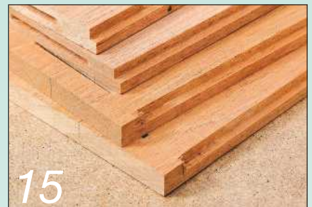
15 Note that the rebates in the carcass top and bottom are stopped
