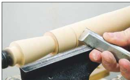
11 ...and then reverse the tool and your stance to cut the right-hand side
