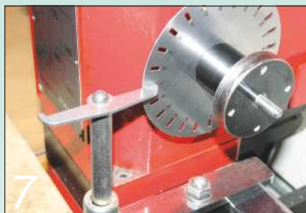
7 The indexing wasn't calibrated. One solution was to fit a Sorby indexing plate
