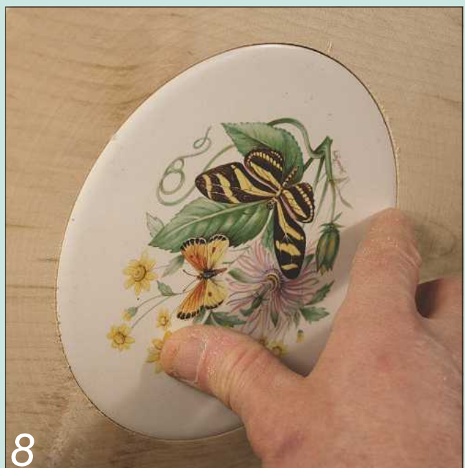
8 Check that the tile fits in the recess and sits slightly proud of the disc
