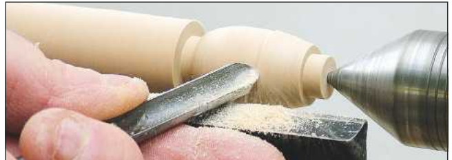
2 Turn an egg shape at the tailstock end, either with a skew or a spindle gouge, in the same way as turning the spurtle bead
