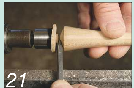
After sanding and polishing the handle, slice it with a skew chisel
