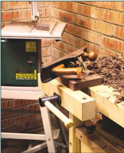
The Indian rosewood stock for the handles is all thickened by hand
