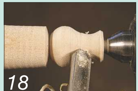
Then form the small pear shape at the neck of the handle
