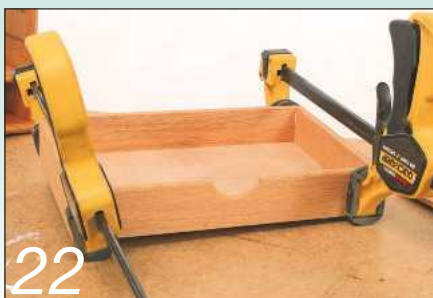
22 Shape the radiused finger pull using a small drum sander and assemble the drawer
