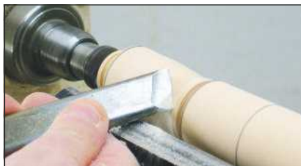
9 Slide the tool along the toolrest to complete the planing cut
