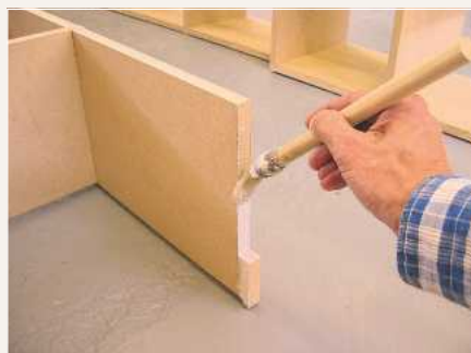
The top and bottom were then glued and screwed into place to complete each carcass
