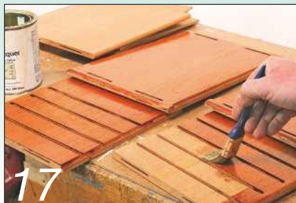
17 Apply brushing lacquer to all the internal surfaces before doing any assembly work
