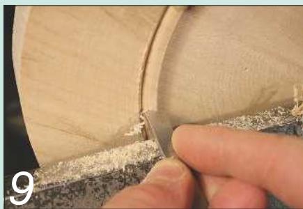
9 Form a rounded bead at the edge of the recess
