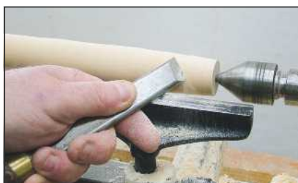
15 Start the taper near the tailstock end, traversing the toolrest from left to right
