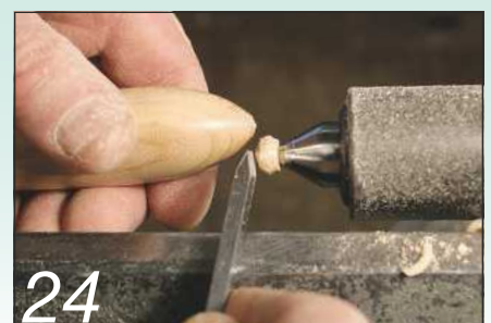
Part off the handle carefully with the point of the skew chisel and sand it smooth
