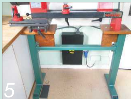
5 ...but its three-phase motor required a converter and special wiring
