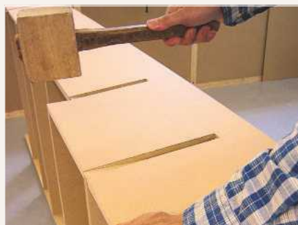
... and then to offer up and fit the other side to them. The mallet came in very handy here
