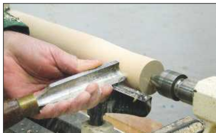
2 Use the spindle roughing gouge to turn the square blank to a cylinder
