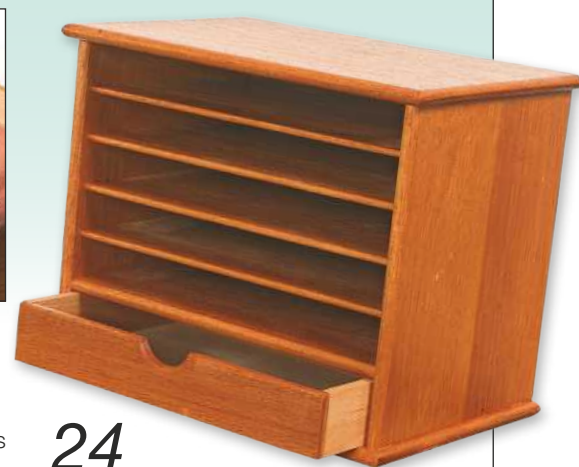
Finish the lacquering, but leave the drawer sides bare so they don't bind in the cabinet
