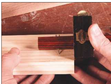
1 Take a marking (or ideally a cutting) gauge set to the thickness of the wood and mark a shoulder line on the inside of both pieces
