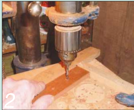
2 Boring holes accurately in the slats on the drill press was aided by a simple jig
