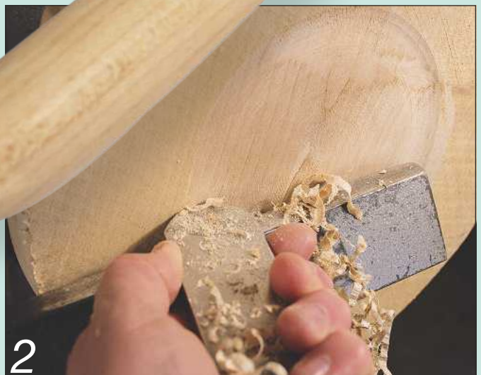
Flatten off the face with a round-nosed scraper
