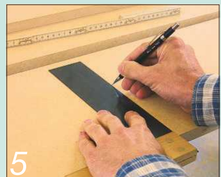
5 Accurate marking out for the shelf positions was particularly essential here
