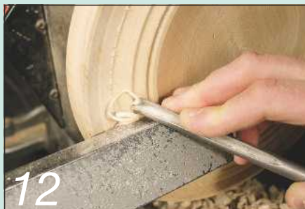
12 Use the same gouge to form a shallow hollow across the front of the moulding
