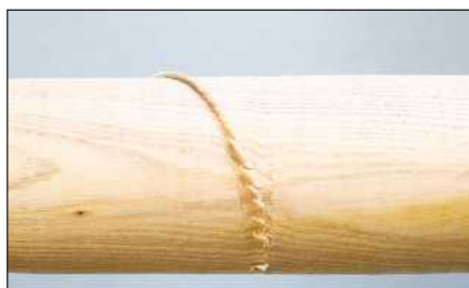
8 This is what can happen if you roll it too far. Avoid at all costs!
