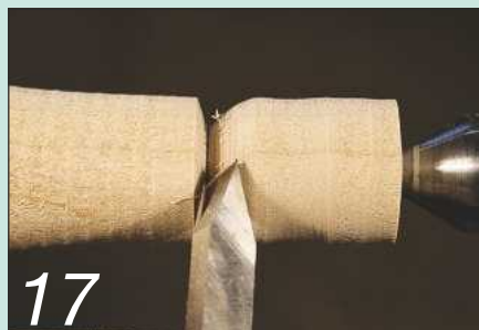
Shape the convex half of the handle's decorative neck first
