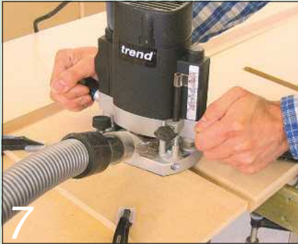
7 They were then accurately machined with my template and the router
