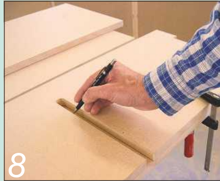
8 The completed first side was then used as a master for all the other parts
