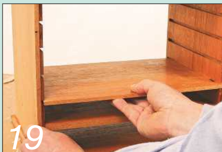
19 Then slide the four centre shelves into place in their grooves from the back of the unit
