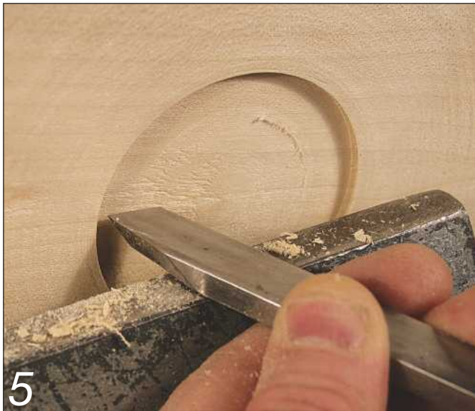
5 Use an angled scraper to form the dovetail in the recess
