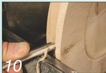
10 True up the rim by slicing in from the rear first
