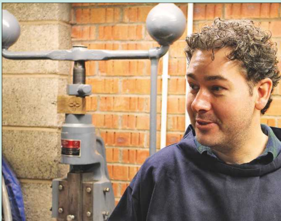
The classic fly press – a staple of engineering for years – sees a lot of manufacturing action
