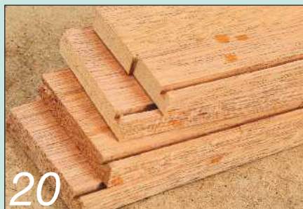
20 Prepare the four sides of the drawer box and cut the grooves for the drawer base
