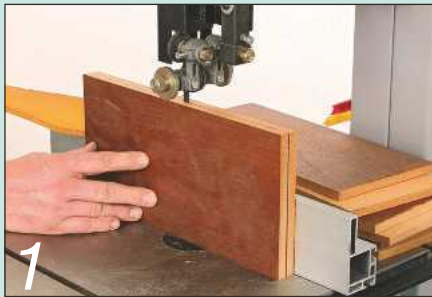
1 Cut the thinner sections down to size on the bandsaw
