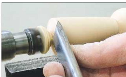
17 Use a skew or a parting tool to reduce the diameter at each end to a small stub
