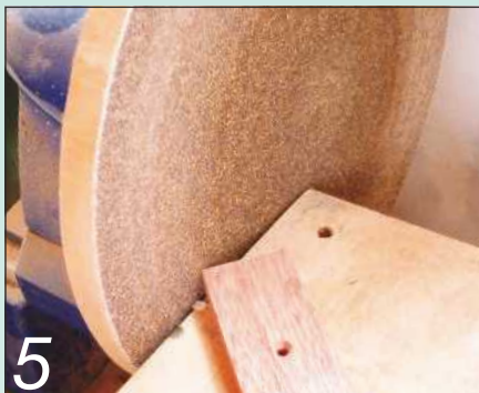
5 I formed tiny chamfers on the edges and ends of all the slats to avoid splinters
