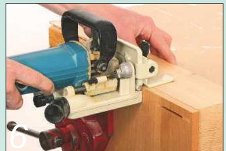
6 Use the fence again to provide the correct offset and keep the slots vertical
