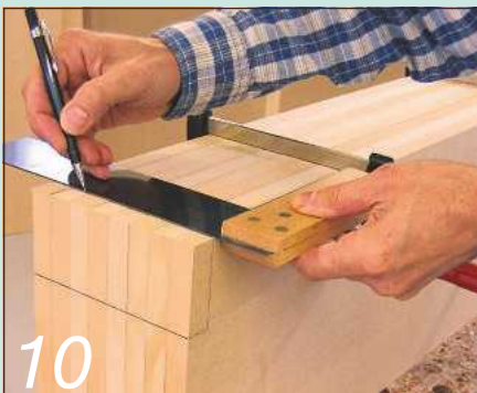
10 The cut-outs in the ends of the shelves were marked out en masse
