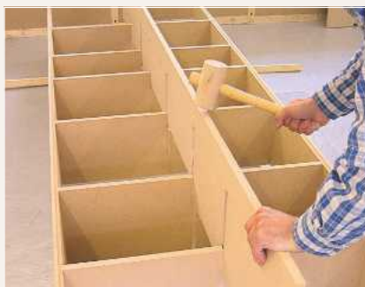
The next job was to remove the cramps and carefully ease the divider into position
