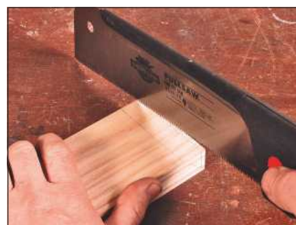
6 Carefully remove the square section of waste wood to create the lap using a fine-toothed tenon saw or a pullsaw
