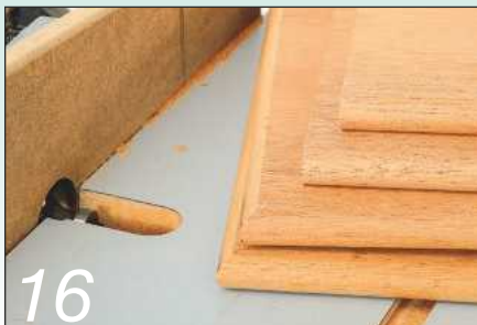
16 Round over the carcass edges on the router table; make the end-grain cuts first
