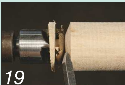
Turn the butt end of the handle to a cone shape using a skew chisel
