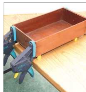
Each bar has two blocks that can be used as feet when cramping boxes
