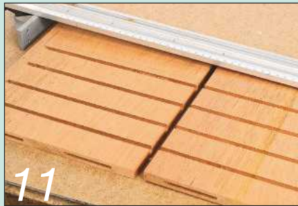
11 You could make a repeat jig, or just reset the position of the cramp guide as required
