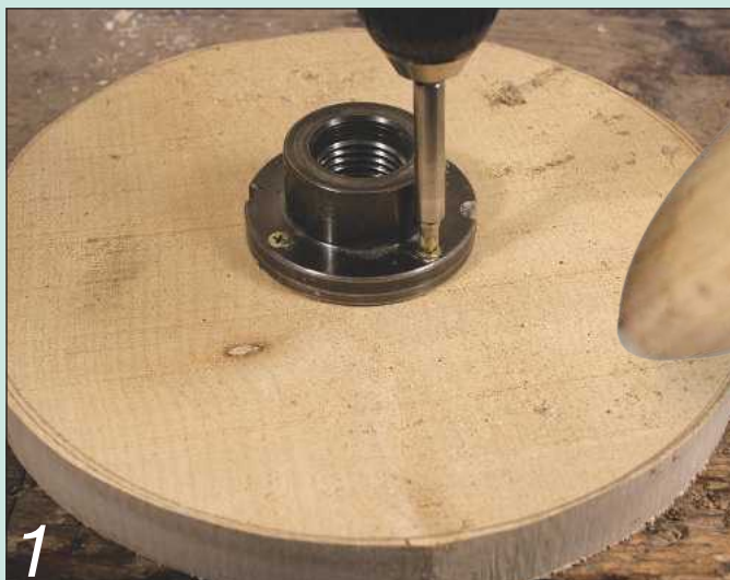
Screw a faceplate securely to the back of the disc
