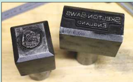
Shane has designed custom die-stamps for the brass back and handle screw
