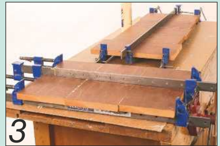
3 Cramp the widened sections together and set them aside to dry
