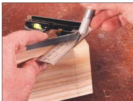
2 Using a marking knife or scalpel and a mitre or combination square, mark the mitres on both sides of both pieces
