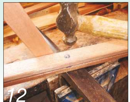
12 Assemble the pivot and dome the other end of the rivet. Note the metal support underneath
