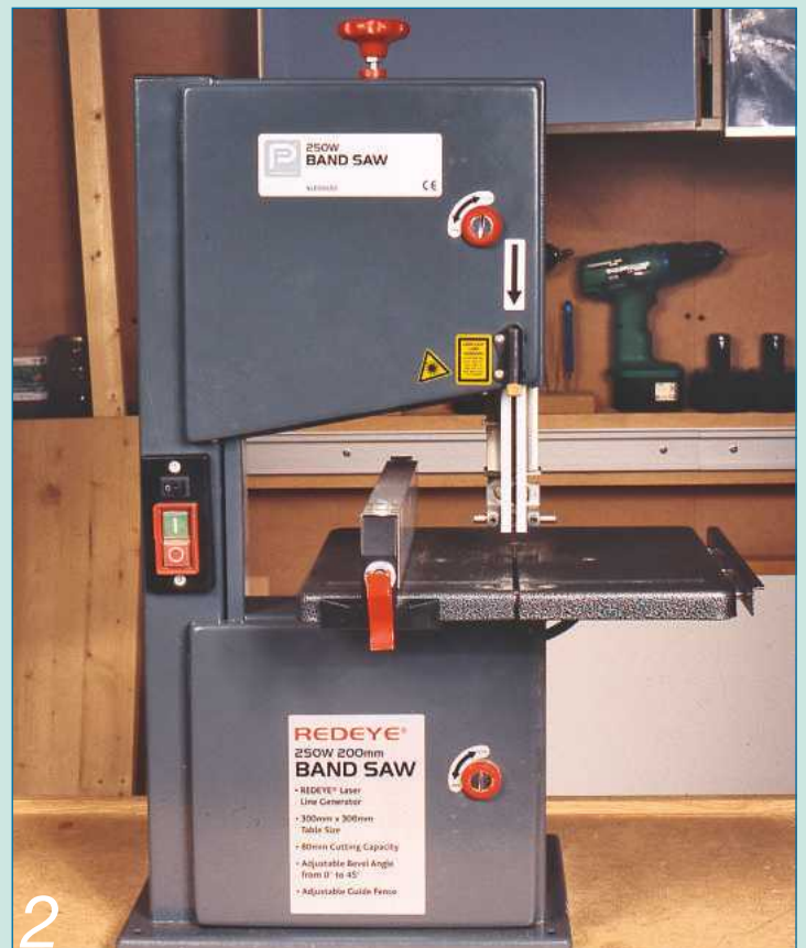
Small bench-top bandsaws may look like toys but they can be very productive if workshop space is limited
