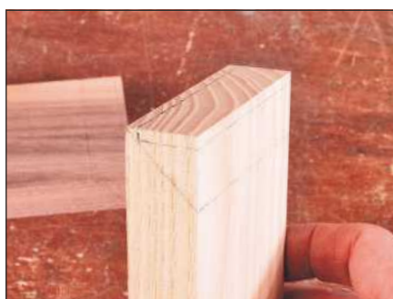
5 The marked-out component should look like this, showing the mitre and the lap
