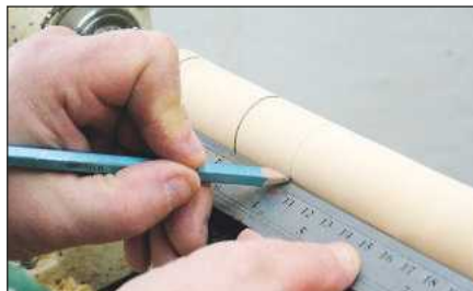
4 Mark out the various handle dimensions with the lathe running
