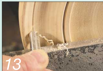
13 Complete the hollow by working from the opposite direction
