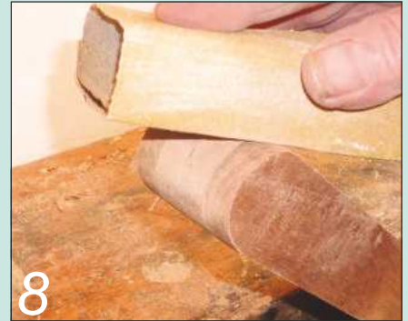
8 Round over the top ends of the legs on the disc sander, and finish the job by hand
