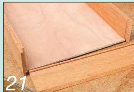
21 The corner joints are half laps, which are easy to cut on the router table
