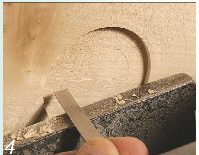
4 Cut a recess in the disc centre for your expanding chuck
