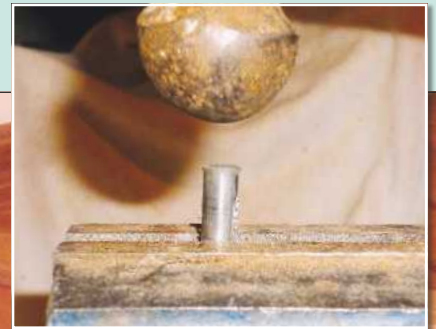
8 Round over the top ends of the legs on the disc sander, and finish the job by hand
