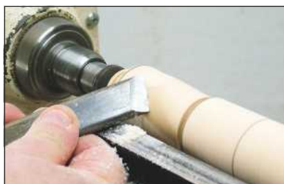
7 Roll the tool clockwise until the cutting edge just starts to bite
