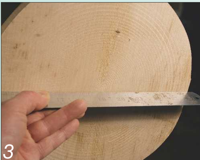
3 Test the flatness of the disc with a straightedge
