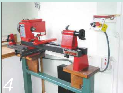
4 My Myford Mystro short-bed lathe had given me many years of faithful service...
