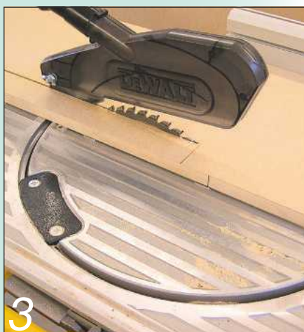
3 The sides were carefully profiled on the table saw. I've raised the guard to reveal the cut
