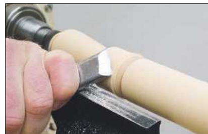
12 With the V cut giving some clearance, start to roll the bead with the skew
