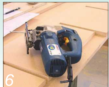
6 All the slots on one of the sides were rough-cut using a jigsaw...
