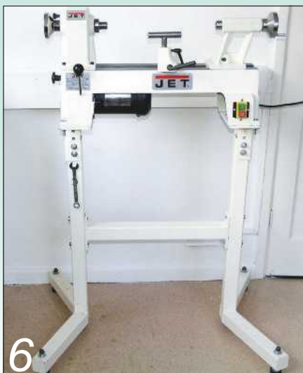
6 Its place was taken by a Jet JML1014, a quiet and compact ½hp model
