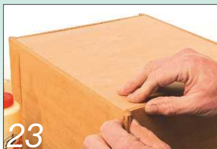
23 Glue the back panel into place in the rebates. There's no need to pin it
