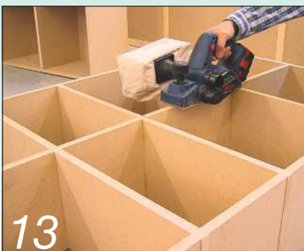
13 As the carcass went together, I used a power planer to level up the worst edges...
