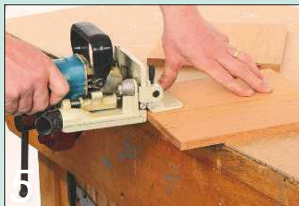
5 Align the biscuit slots using the fence on the jointer as a guide
