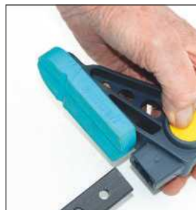
Pressing the yellow button allows the tail to be removed and reversed
