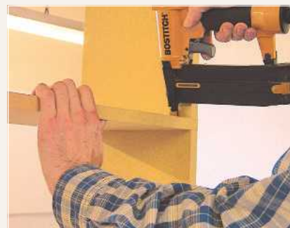
A few 18g brads fired from my nail gun strengthened any vulnerable joints
