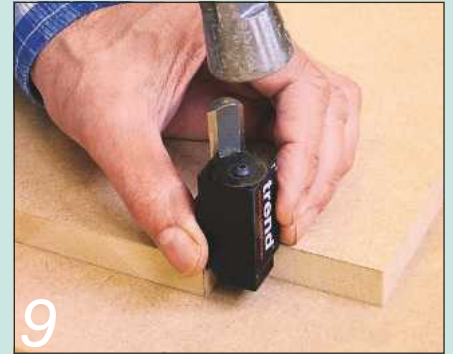
9 Trend's corner chisel cutter proved invaluable for squaring up the round corners
