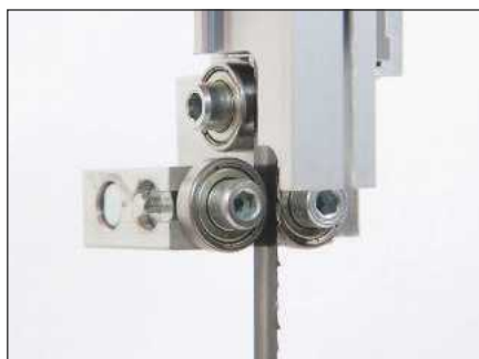
Upper and lower ball-bearing blade guides give excellent blade control
