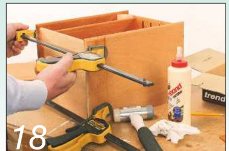
18 Assemble the main carcass and check that everything is square as you tighten the cramps
