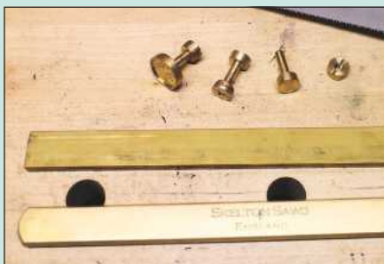
The back is shaped from solid brass strip, while the blade screws are custom-made
