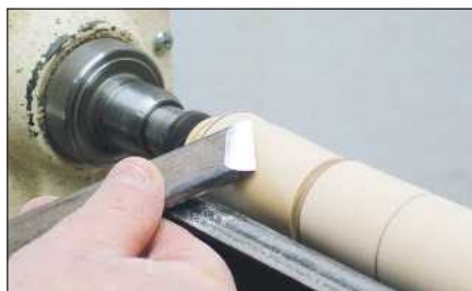
6 Start the planing cut with the bevel of the skew resting on the wood
