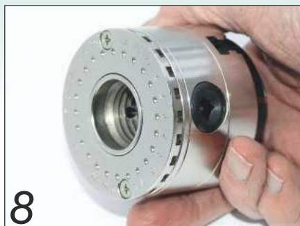
8 Another possibility was to use the CSC500K chuck from Axminster
