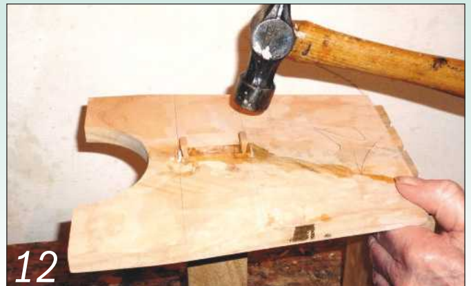
12 Assemble the rail and legs, then drive wedges into the tenons
