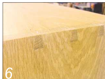
6 The finished through dovetail joints on the carcass corners look neat and tidy
