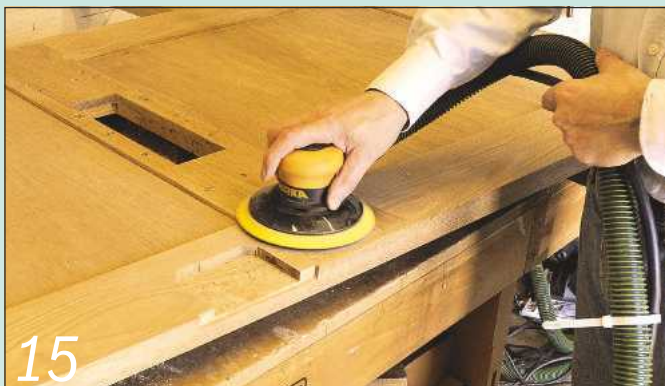
Cut the lock recesses and sand the inner faces of the two frames
