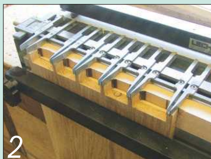
2 I used a Leigh Jig to form the through dovetail joints I used on the carcass corners
