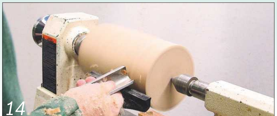
14 Turn the stem blank to a cylinder using a spindle roughing gouge
