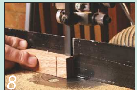
8 Set the fence position precisely on the bandsaw and cut the tenon cheeks
