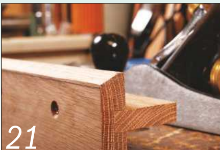
21 Plane the required angle across the bottom edge of the front panel
