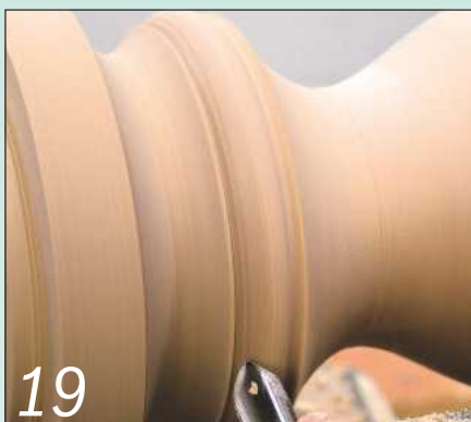
19 When you cut the beads in this way, sharp fillets are cut automatically
