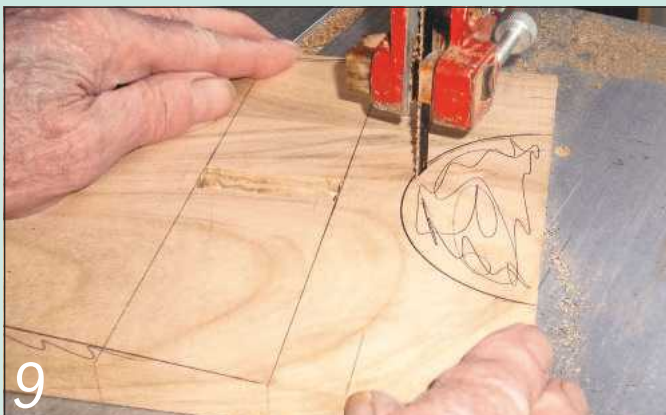
9 Use the bandsaw to make the semi-circular cutouts in the two legs
