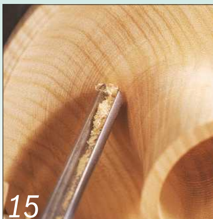
15 Use the finest of cuts with the flute of the gouge held upwards to create a smooth finish
