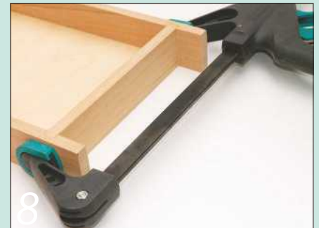
8 Glue and cramp up the truck sides and the base, and set the assembly aside to dry
