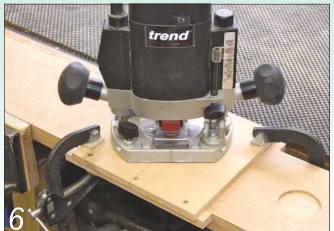
5 I made up a simple router template to cut the hook recesses accurately
