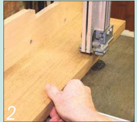
2 Rip the plank along its length on the bandsaw, leaving it slightly oversize
