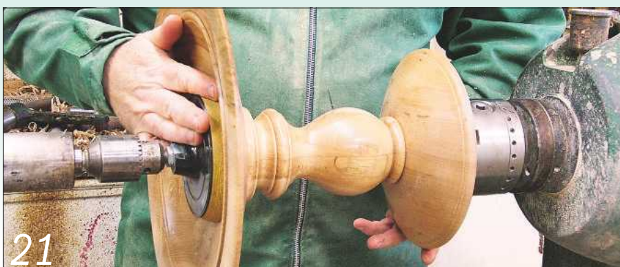
21 Use the lathe as a clamp when gluing up the three components to ensure accurate alignment
