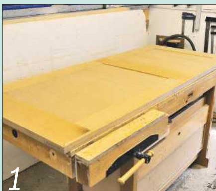
1 After cutting grooves for the plywood panels, I assembled the frame
