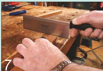
7 Cut the tenon shoulders down to the marked lines with a fine-toothed backsaw
