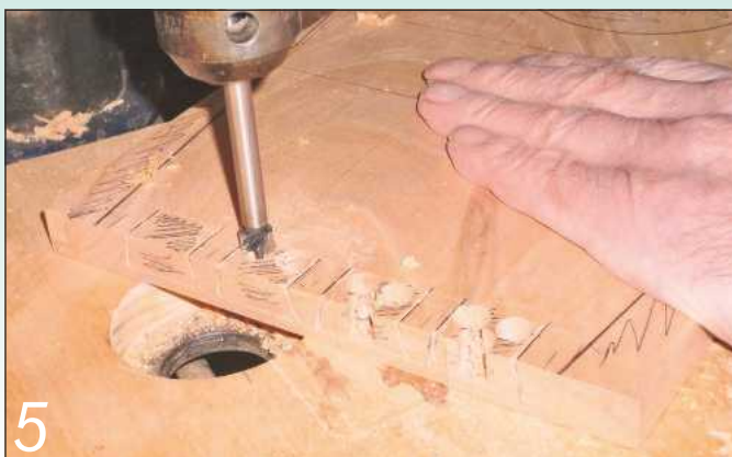
Use a Forstner bit to remove most of the waste from the dovetail sockets
