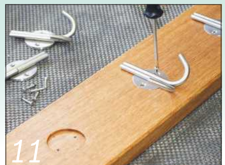
11 Position each hook accurately in its socket and drive in the fixing screws
