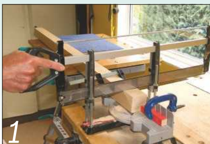
1 Use a hand mitre saw to cut the blocks. Note the red length stop cramped to the saw table
