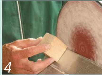
4 Lightly chamfer the edges of each block with the disc sander table set to an angle of 45°
