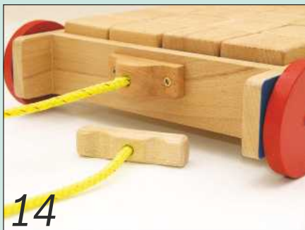
14 Finish off by fitting the cord to the pull toggle and bracket, then screw the bracket in place
