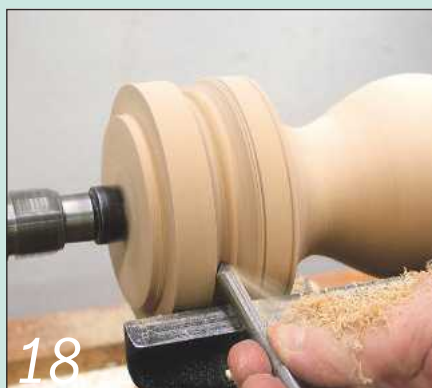
18 Cut the cove between the top two beads next using the spindle gouge
