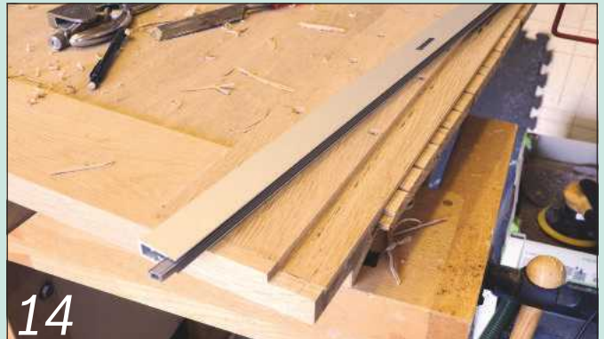
The threshold seal fits in rebates cut along the bottom edge of each frame
