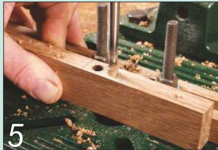
5 Define the length of the mortise by drilling a hole to the required depth at each end
