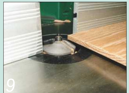
Field the door panels using a bearing-guided panel-raising cutter in the router table
