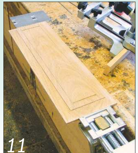
I held each door panel in a Zyliss clamp while routing the grooves for the inlay banding
