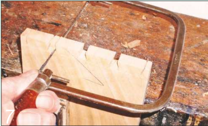
7 Use a coping saw to cut away most of the waste between the pins
