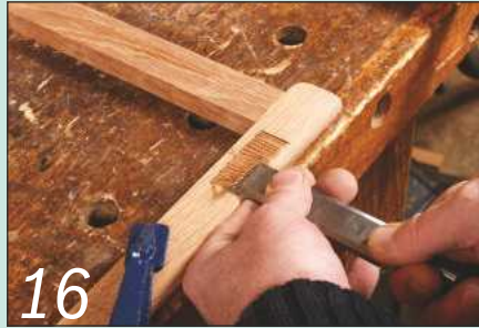
16 Mark the depth of the recess using a marking gauge, then trim away the waste wood
