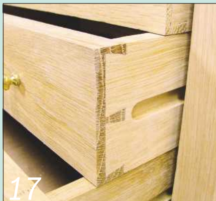
17 Screw the drawer slips to the carcass sides and test the fit of the four large drawers
