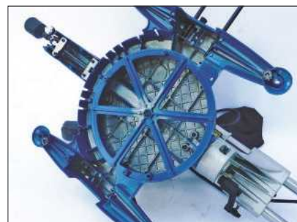
The underside of the turntable has several gates for setting common cutting angles
