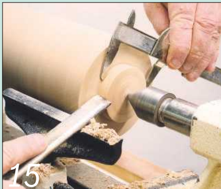
15 A peeling cut made using a skew chisel quickly cuts the tenons to size
