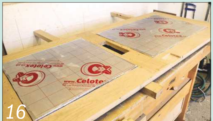
Tape the edges of the Celotex panels and fit them into their recesses
