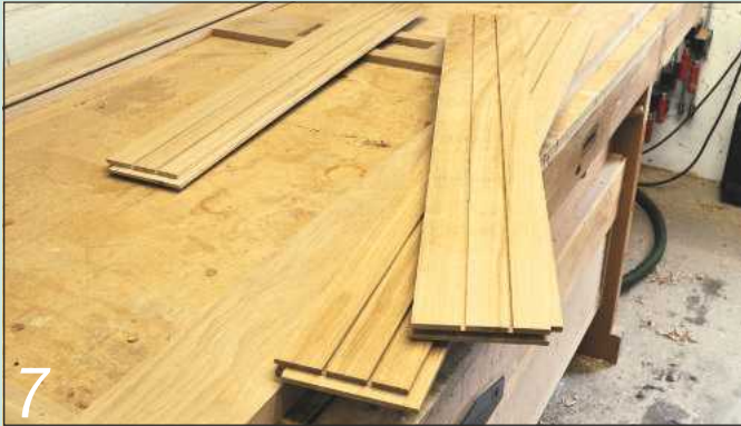
7 Then cut the middle boards in two and tongue and groove their ends
