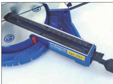
Movement of the turntable is controlled by moving and locking this arm
