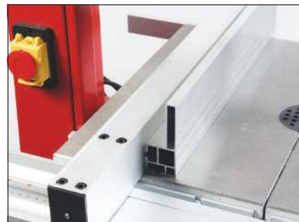
The two-part rip fence runs on an alloy rail at the front of the table
