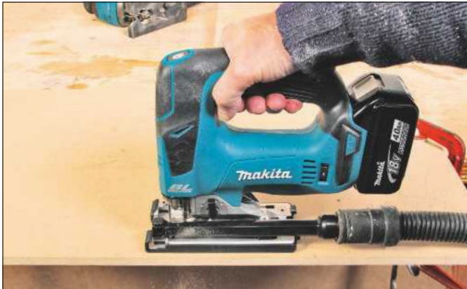
The conventional D-handled model is easy to control for regular cuts
