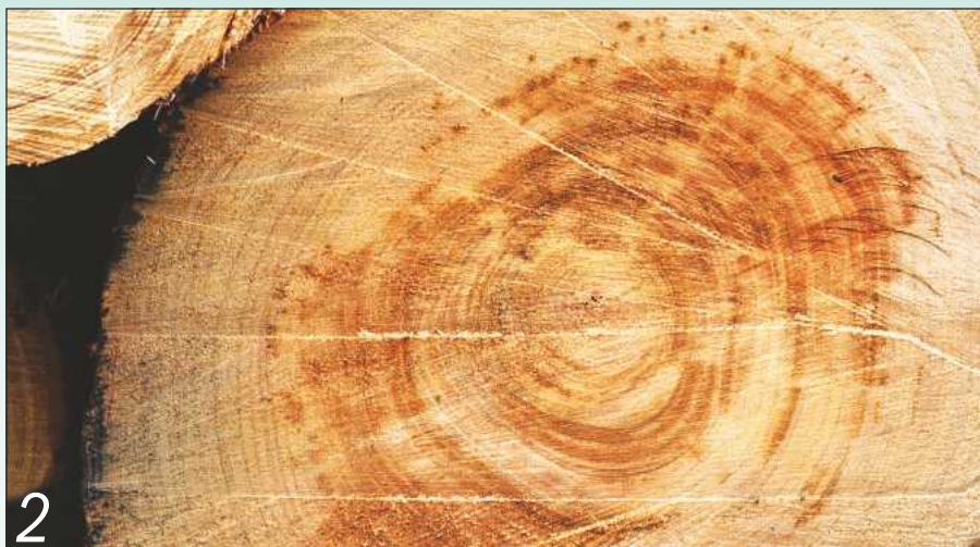
The earliest stage of rot infestation usually causes some form of staining
