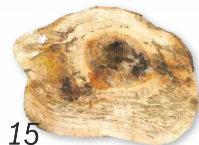
Secondarily decayed timber can be attractive but may be structurally unworkable
