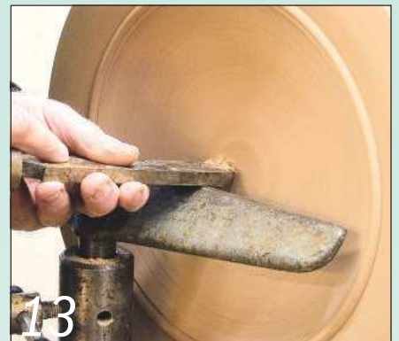
13 Use a bowl gouge or a round-nosed scraper to refine the inside surface of the bowl
