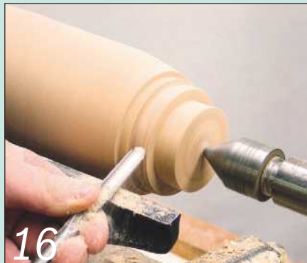
16 Work from the tailstock end towards the headstock. Cut the first bead...
