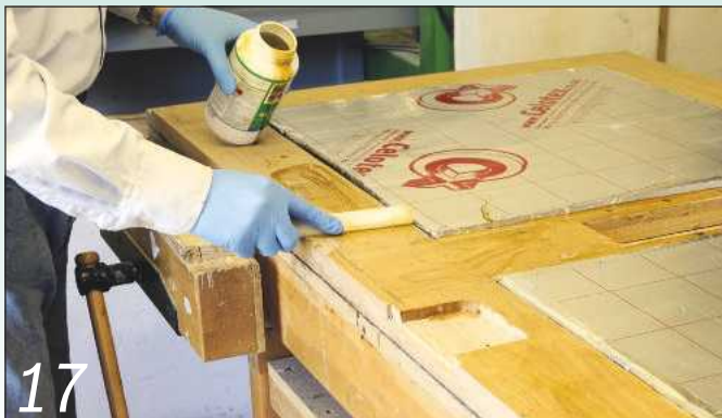
Apply a thin coat of polyurethane adhesive to both faces of the frames
