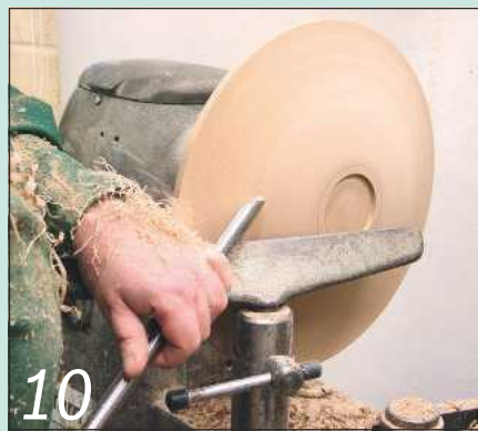
10 Here I'm using a pull cut to shape the underside of the bowl
