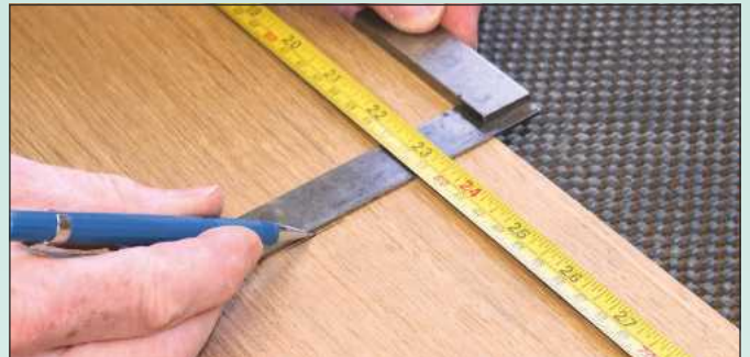
4 Mark out the hook positions at regular intervals along the back board
