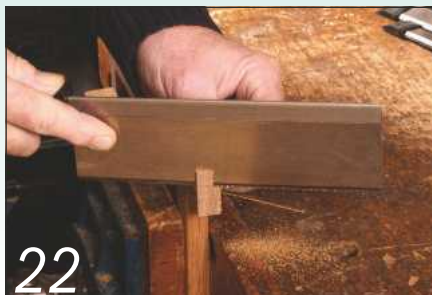
22 Use a fine-toothed backsaw to trim the frame legs to the same angle
