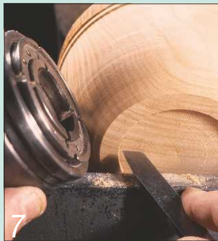
Then cut the dovetail in the side of the recess
