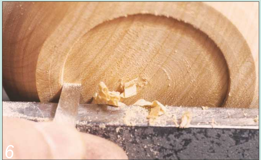
Form the recess for the chuck jaws in the base of the bowl using a small square-ended scraper
