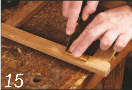
15 Mark up the hinge positions on the leg frame first using a marking knife
