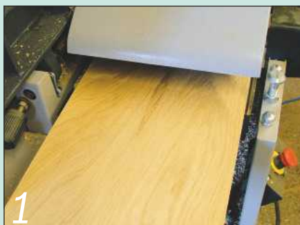
1 Thickening the raw boards soon revealed some very attractive figuring in the oak
