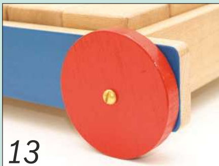
13 Attach the wheels to the truck with screws driven through the truck sides and into the ends
