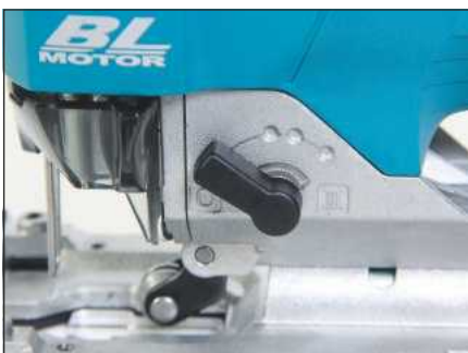
Both models feature a standard four-position orbital action selector switch
