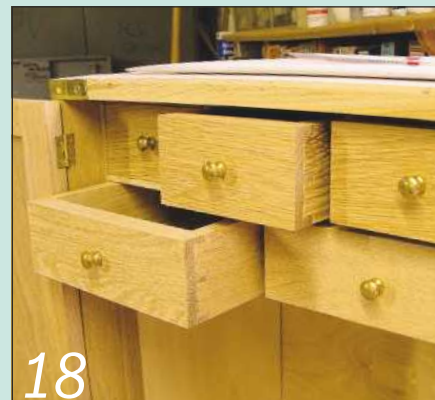
18 Check that the five smaller drawers fit neatly into their pigeonholes in the lining box
