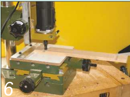
6 Cut the 12 x 6mm grooves for the ends. The cutter guard has been removed for clarity
