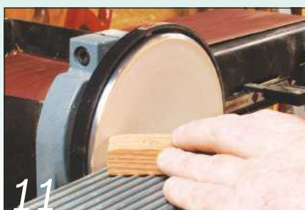
11 Use a 5p coin to mark a radius on the crosspiece corners and sand it to a smooth finish
