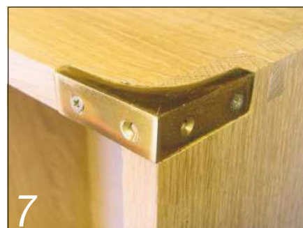
7 Recess the brass corners individually, and retain them temporarily with screws
