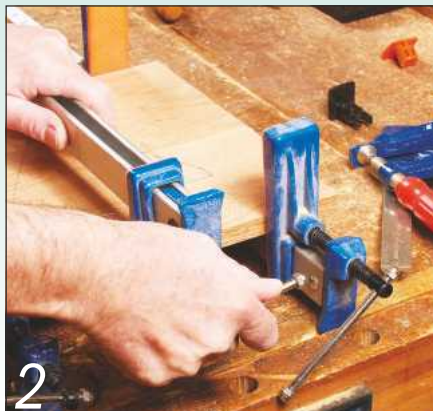
2 Glue the two components together and cramp them securely while the glue sets
