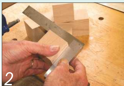
2 Check that all the blocks are perfectly square in each dimension
