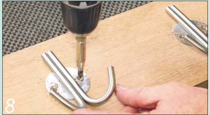
8 Use a hinge centring drill to locate the holes in the centre of the countersinks
