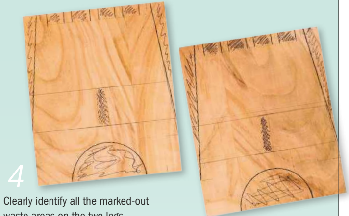
Use a cutting gauge to mark out the extent of the dovetails
