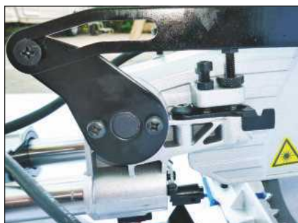
The head of the machine can be locked in the lowered position when required
