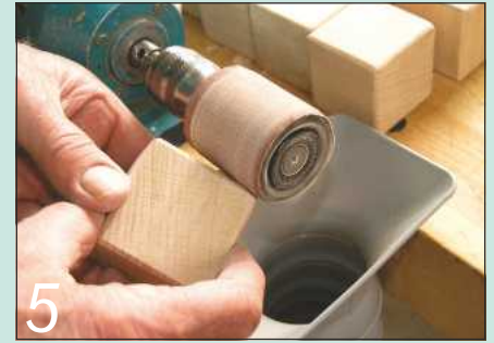
5 Round off the chamfers with a drum sander. Note the extractor pipe used to collect the dust
