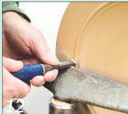
12 Cut a bead next to the rim with a skew chisel held on its side
