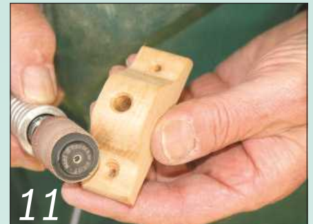
11 Cut the towing bracket to size and shape, drill the cord and screw holes and sand it smooth
