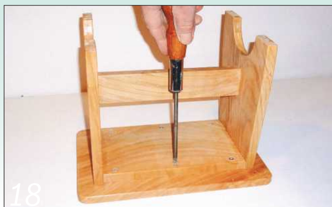
Attach the seat by driving screws up into it through the seat support
