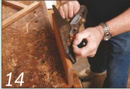
14 Plane a rounded profile on the top edge of the front panel and sand it smooth
