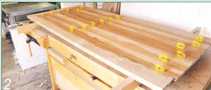
2 The inner boards were cut and dry-fitted with 2mm spacers in between
