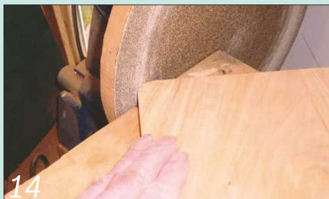
Round the corners of the top slightly and soften all the arrises
