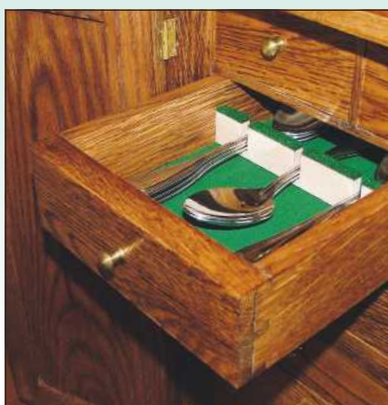
The chest is completed and ready for its spirit stain, Danish oil and wax finish
