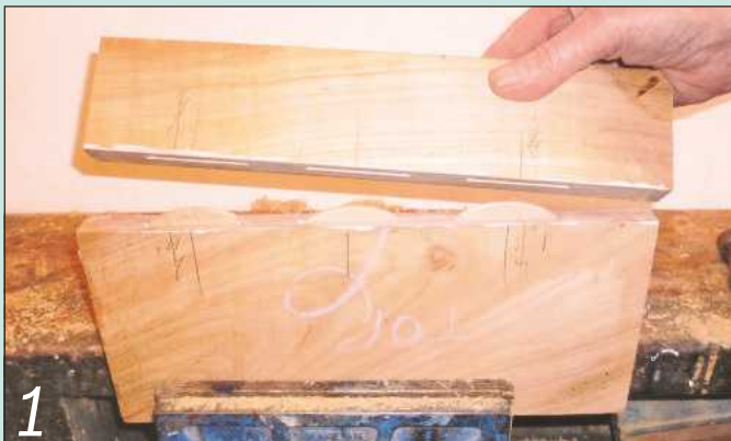
The joints between the sections were strengthened with biscuits
