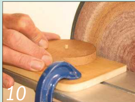
10 Sand the wheels to get them perfectly round. I used a simple jig cramped to the router table
