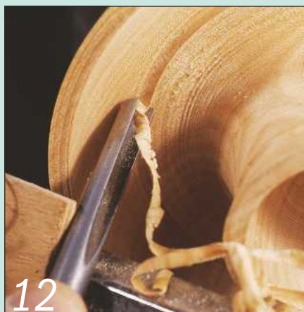
12 Work down one curve of the outer side bowl at a time...
