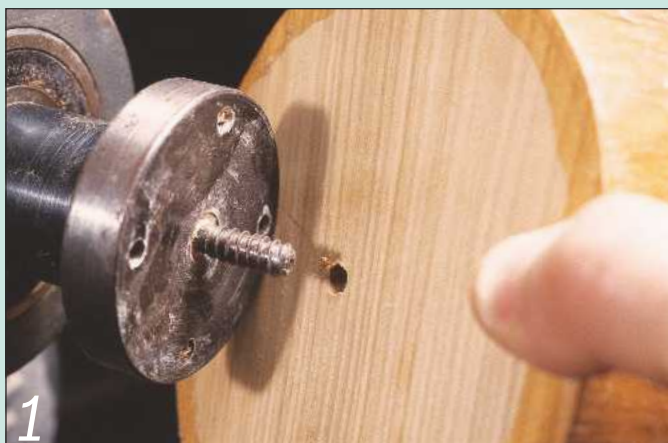
1 Fit the disc onto a screw chuck. You'll need to drill a pilot hole first
