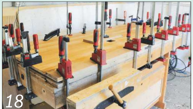
Assemble the two frames on a flat bench and cramp them tightly
