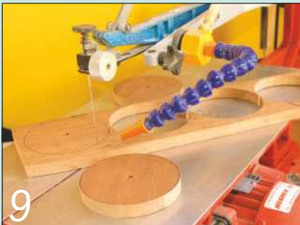
9 Mark out the wheel circles and drill a centre hole in each one. Cut them out with a scrollsaw
