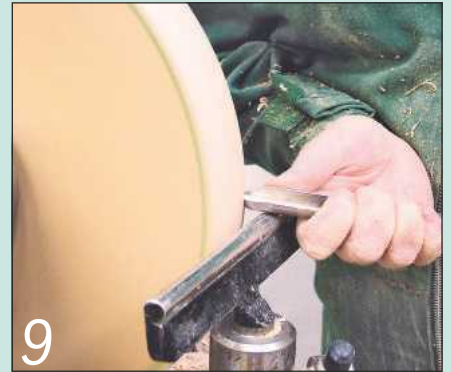
9 Use the tip of the bowl gouge to true up the edge of the bowl blank
