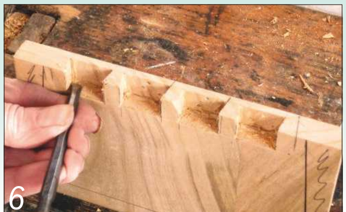
A small chisel with an angled edge is ideal for trimming out the corners
