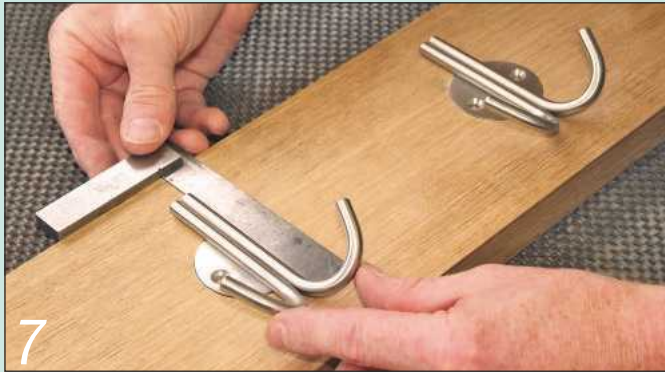
7 I used a small engineer's square to align the hooks on the back board
