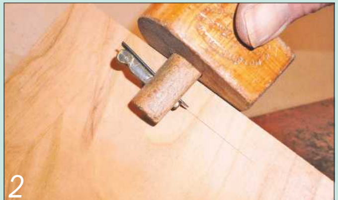
Use a cutting gauge to mark out the extent of the dovetails
