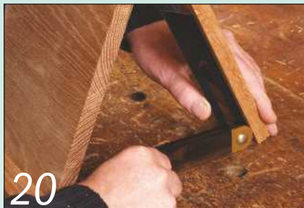
20 Use a sliding bevel to set the 60° angle at which the frame will stand on the worktop
