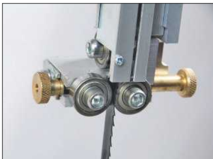
The upper blade guides are easy to adjust using knurled knobs and locking bolts
