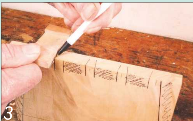
I used a home-made dovetail template to mark out the joints
