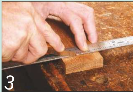
3 Scribe the shoulder positions across both legs at once to ensure accuracy
