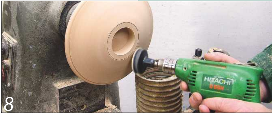
8 Power-sand, seal and polish the base. Have your dust extraction nearby
