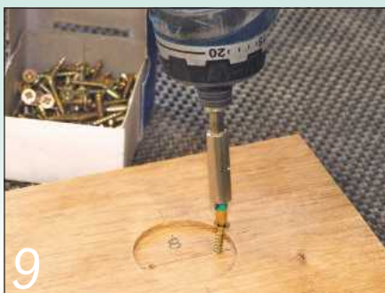
9 Pre-cut the threads in the pilot holes using an ordinary steel wood screw
