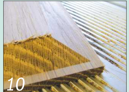
You may need to use abrasive paper to remove any tear-out occurring on the panel angles
