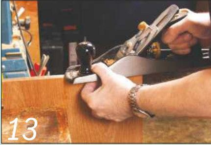
13 Trim the front panel to length and width and clean up the edges with a sharp plane
