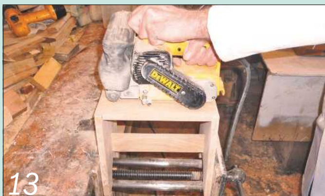
After assembly, level the lap dovetails off using a belt sander
