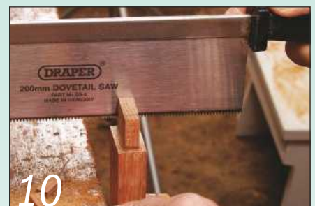
10 Then cut the tenons carefully to the required width with your backsaw
