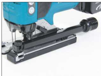
The saws are supplied with a rather neat – and efficient – clip-on dust extraction tube
