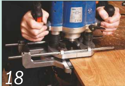
18 Rout a 12mm wide channel across the front panel to receive the shelf
