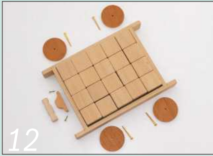
12 Varnish, stain, paint or decorate all the parts to taste before starting the final assembly
