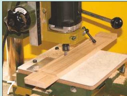
7 Cut the 6mm wide groove in the sides for the plywood base. Again the guard has been removed
