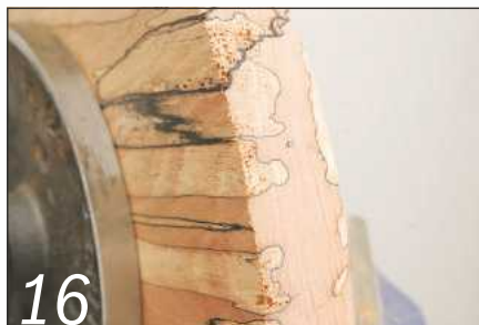
Spalted wood can be difficult to work, as the density can vary from area to area
