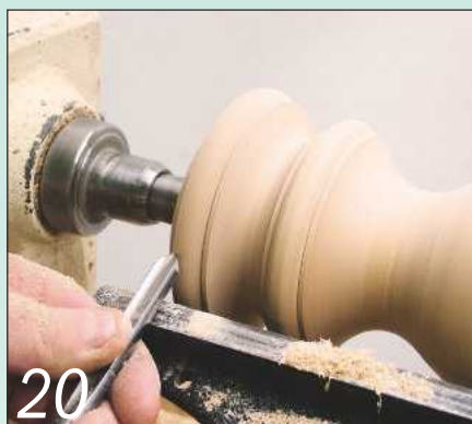
20 Finally, cut the bead at the top of the stem, once again leaving a fillet
