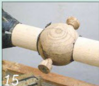
15 Mount the two chucks, rotate the sphere through 90° and secure it between them
