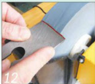
12 A grinding wheel helps to speed up forming the cambered edge on the cutting iron during my scrub plane conversion
