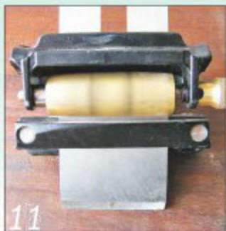
11 The cambered roller on the Veritas honing guide allows the edges to be feathered back to prevent dig-in
