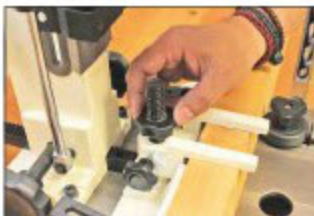
The heavy-duty hold-down fork is secured in place with a locking knob
