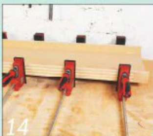
14 Assemble the pairs of components and cramp them securely while the glue sets
