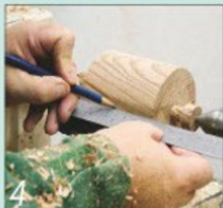
4 Measure the length of the cylinder and mark a line at its mid-point
