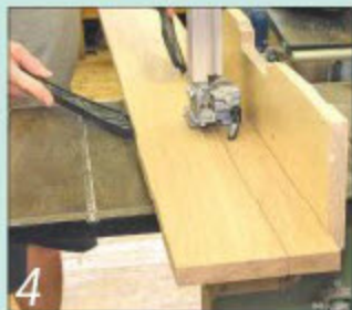
4 Cut your boards to match the slat length and rip them down to their finished width
