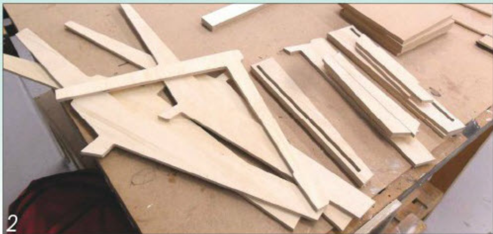
After cutting on the CNC machine, the components simply needed cleaning up and sanding in preparation for gluing
