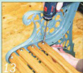
13 The bolts are very easy to tighten using a hex bit fitted in a power drill/driver
