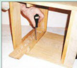
6 Use one of the drawer sides to locate the two drawer runners on the side panels
