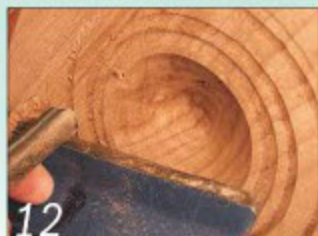
12 Hold the tool down on the tool rest to stop the cut spiraling out of control
