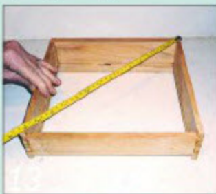
13 Glue up and assemble the four drawer components, and check for squareness
