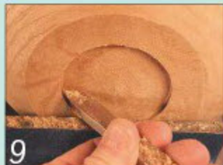
9 Create the dovetail in the corner of the recess with an angled scraper
