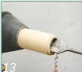
13 Drill out the end of the other cup chuck to fit over the revolving centre
