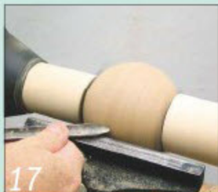
17 Remove any visible ghosting with light cuts using the spindle gouge
