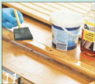
11 I used a foam brush to apply several liberal coats of boiled linseed oil to the slats
