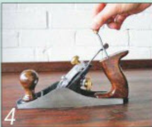
4 As I loosened the cap nut to remove the tote, the entire retaining bolt came free
