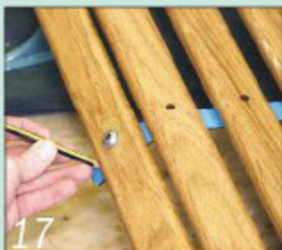
17 Mark the remaining hole positions on the spreader, and also where to trim the ends
