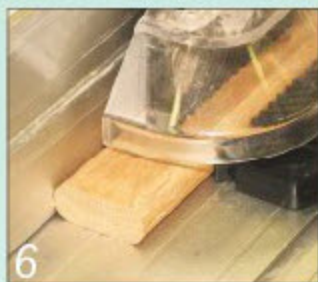
6 Soften all the slat edges using a roundover cutter in the router table
