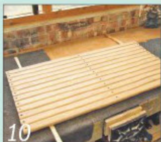
10 Mark the centre line of the slats and drill all the fixing holes slightly over-size
