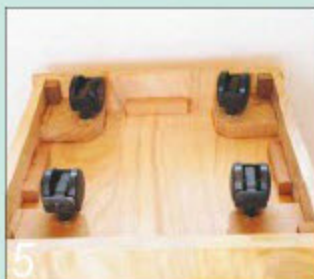
5 My recycled castors were fitted to the base using glued mounting blocks
