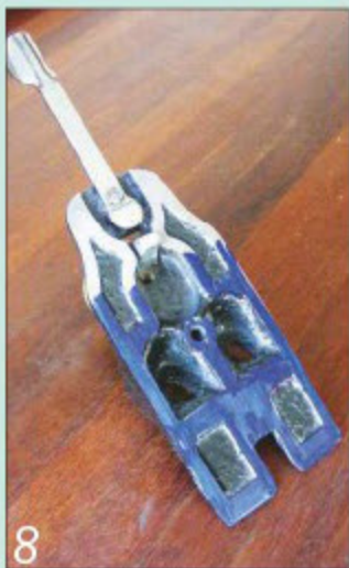
8 Ink the frog using a permanent felt-tipped pen so you can test it for flatness
