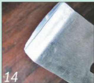
Fit the cap iron further back from the blade edge to allow a clear passage for shavings
