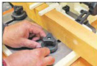
These rollers are pushed against the work to hold it securely to the fence
