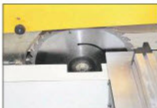
The carriage slides away to give good access for changing the blade
