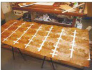
The gorgeous table-top was made by shooting and taping together a series of separate leaves, as shown
