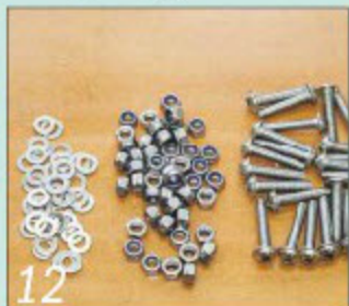
12 I chose M8 x 40mm stainless steel flange-head bolts with Nyloc nuts and washers as the fixings
