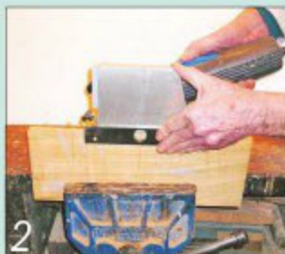
2 After preparing the panel parts, cut all the slots for the biscuits
