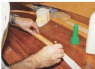
For edge strips, apply PVA or yellow glue to the back of the strips...
