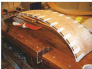
Use a wallpaper stripper and a piece of pipe to steam the ebony veneer lines, before gluing them into position
