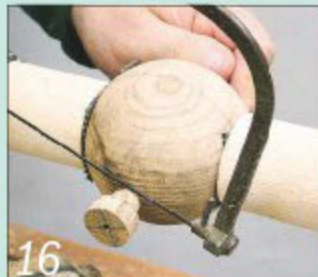
16 Cut off the two tenons with a fine-toothed saw and start the lathe
