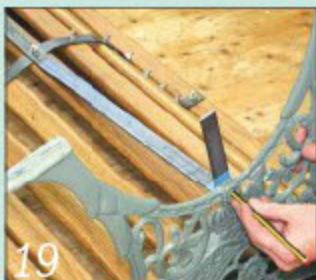
19 Mark the positions of the brace's fixing bolts, and also the finished length
