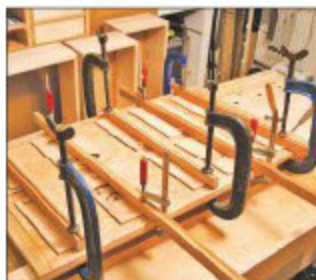
To keep veneer pressed while an adhesive is curing, use boards or cauls together with lots of clamps
