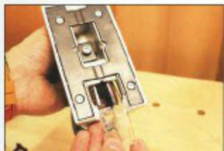
An clear plastic anti-splinter shoe is supplied for finer cutting
