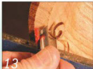
Start the cut with the tool post supporting the back of the gouge
