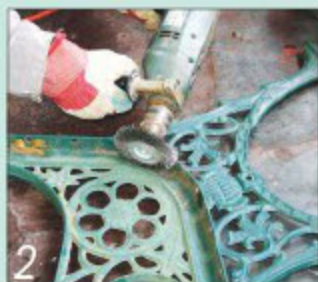
2 Remove the old bolts using bolt cutters, then wire-brush the castings to remove loose debris
