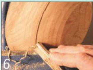
6 Use an open-handed grip so that the tool slides through your fingers
