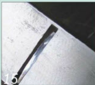
A wide throat allows large shavings to be cut: you can file this even wider if required
