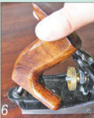
6 I then had to twist the tote slightly to get it past the frog assembly before replacing the nut
