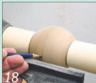
18 Mark another centre line and then rotate the sphere through 90° again
