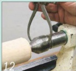
12 Use callipers to measure the diameter of your revolving centre
