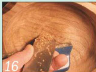
Use a scraper to flatten off the bottom of the inside of the bowl
