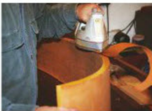
...and iron the veneer in place, ensuring the edges are well and truly attached
