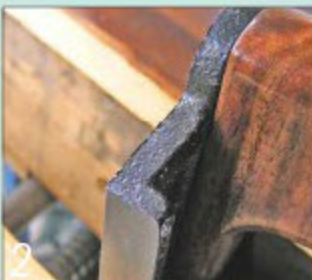
2 Rough edges around the outside of the casting must be removed to prevent damage to work surfaces...
