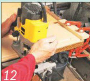
12 Use an offcut to work out the spacing for the flutes and cut them one by one
