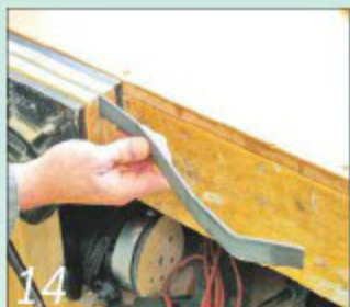
14 Shape the centre spreader in stages by hand while holding it in a bench vice
