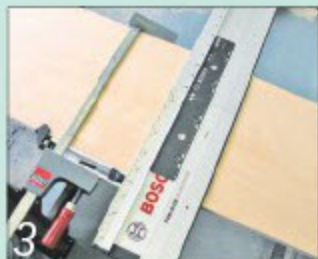
Setting up for square cuts with the angle guide
