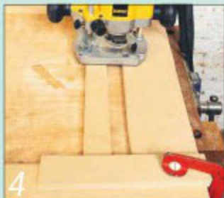
4 Fit stop blocks when cutting stopped chamfers. Support the router base on an mdf offcut
