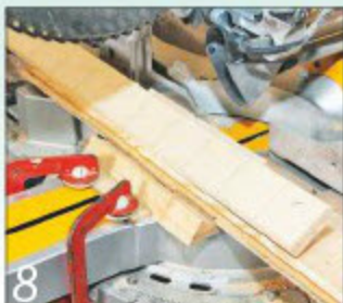
8 The first step was to mark out the workpiece into equal sections...
