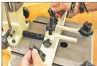
A rack-and-pinion knob sets the back fence position. Once set, it's held with twin cam levers
