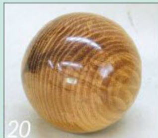
20 Finally apply a wax-over-oil finish and the sphere is completed
