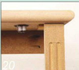
20 The front panel is held in place using a pair of roller catches fixed to the underside of the top
