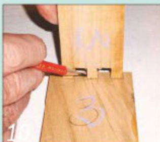
1 Mark out the sockets directly from the pins with a hard pencil
