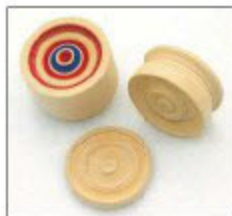
The decoration produced by the tool is small and delicate, almost like embossing
