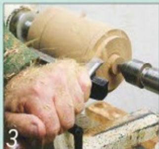
3 Turn away the waste wood at each side of the marks with a peeling cut
