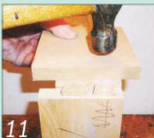
11 Test the fit of the dovetails, and ease any that appear to be tight
