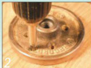
2 Screw the faceplate to the blank with four No 8 Spax or similar screws
