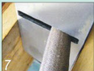
7 Keep the file perpendicular to the sole when removing excess paint from the throat
