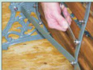
20 Drill the holes, trim the bar to length and fix it in place to check its fit
