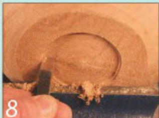
8 Cut the recess for the chuck with the 1/4in beading and parting tool
