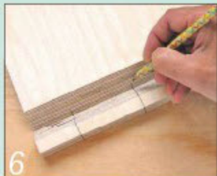
A plywood offcut makes a mini rod for marking the biscuit positions
