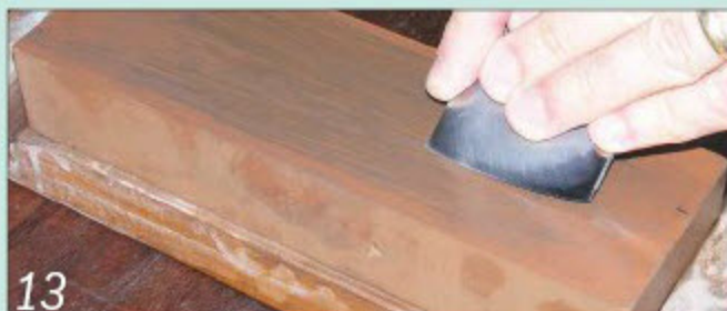
Sharpen from right to left with the trailing edge up to prevent dig-in
