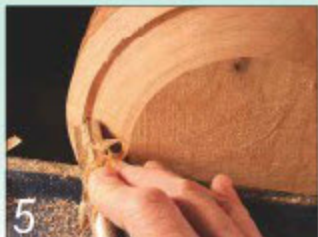
5 Maintain this depth of cut until the gouge has completed its pass
