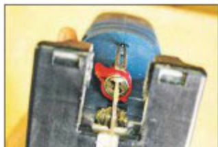
When correctly fitted, the collar wraps around the blade shank
