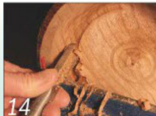
All that is required is a little pressure to propel the cut forward
