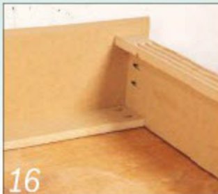
16 ...and attached the side panels and the rear rail to the top panel
