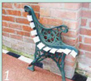
1 Stick Post-it notes on the ends to mock up the slat positions and decide on the slat width
