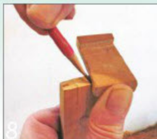
8 I then used my home-made dovetail gauge to mark the slope of the pins
