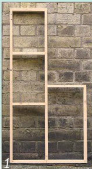
It's always a good idea to make a full-sized rod to better gauge the proportions
