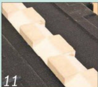
11 The finished moulding was an excellent copy of the original version
