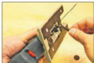
There's a hex key adjustment for tilting the base by up to 45°
