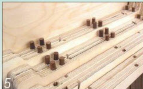
5 Fixing the seat back and base to the plywood frame was achieved by gluing in walnut dowels at specific locations
