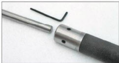
The blade is secured by two grub screws, which marked its shank
