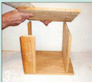
3 Assemble the sides, the shelf and the rails to form the carcass
