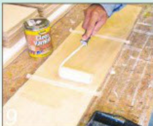
Varnish the inside faces before gluing up. Note the masking tape over the biscuit slots
