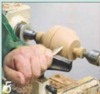
5 Start the shaping by cutting chamfers on both sides of the centre line
