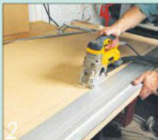
2 Use a jigsaw and a guide rail or batten to make the cut-out in the front panel
