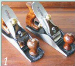
1 The Faithful and Draper planes are born of the same mould: all parts are identical and interchangeable
