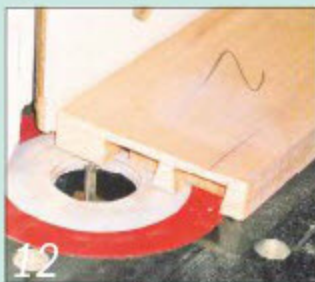
12 Form grooves for the plywood drawer base on the router table
