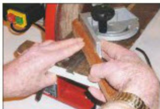
...and the other face to trim the second component of the joint
