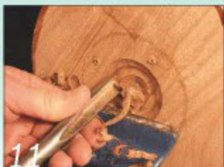
11 Start hollowing out the bowl with a freshly sharpened bowl gouge
