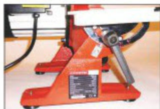
The table tilts up to 45° and is secured with a couple of locking levers
