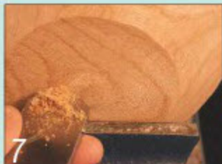
7 Flatten off the base of the bowl using a scraper supported by the tool rest
