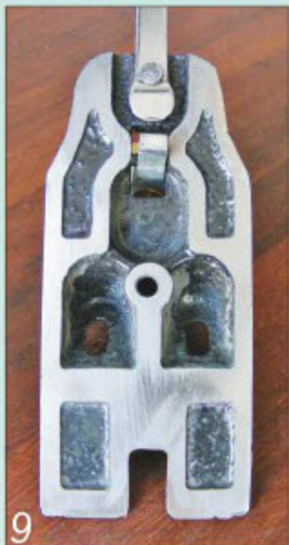
9 Rub the surface of the frog below the adjustment lever on wet and dry paper until the colour has gone
