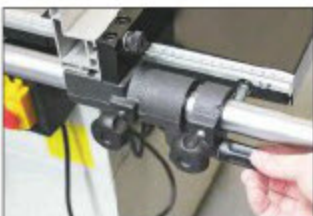
There's a micro adjuster on the fence to allow you to fine-tune the cut
