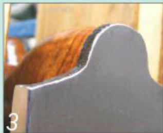
3 ...but a little work with a fine file is all you need to smooth the soft iron
