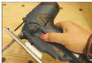
The slider is positioned more favourably for a right-handed operator
