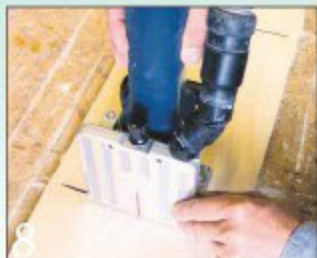
A steady hand and a non-slip biscuiter face produce accurate slots
