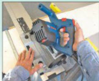
The plunge saw is tilted to 45° for cutting the board-end mitres
