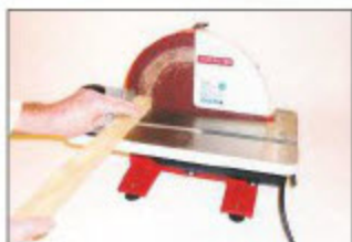
The fence is set at 90° for basic trimming of end grain
