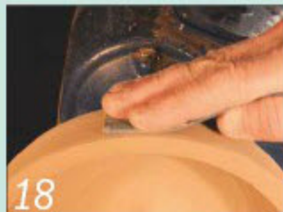
Always keep your hands in line with the rotation of the work when sanding
