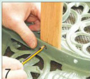
7 Hold each slat in place against the bench end and mark the position of its fixing bolt
