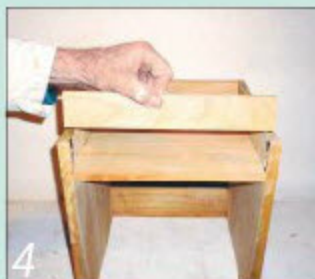
4 The two plinths are glued into shallow grooves routed in the side panels
