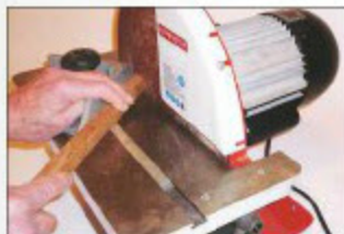
Use one face of the mitre fence to trim one component of a mitre joint...
