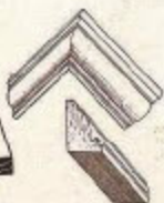
FIG. 13.—2 IN. SQUARE MOULD MITRED (2 SEPARATE).
