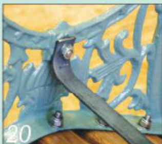
20 Drill the holes, trim the bar to length and fix it in place to check its fit
