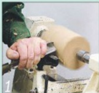
1 Rough your stock down to a cylinder using a spindle roughing gouge
