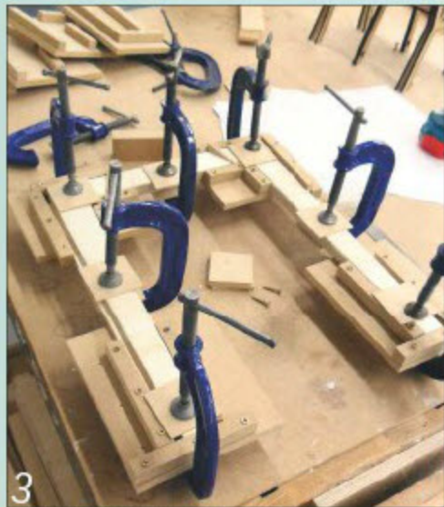
3 I created this makeshift jig for gluing the front panels of the larger chair together
