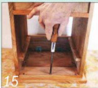
15 Screw on the top panel. Note the expansion brackets attaching the top at the back
