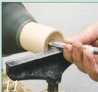
11 Hollow out the end of the headstock cup chuck with a spindle gouge
