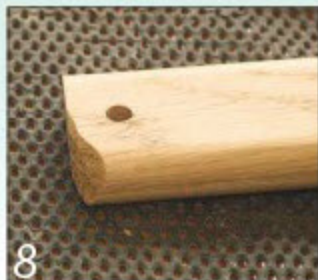
8 You may need to sand the corners of the two outer slats to fit within the bench ends
