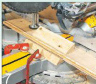
7 I chose to use a sliding mitre saw combined with a simple angled jig
