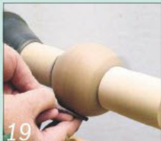
19 Sand the sphere, starting with 180 grit and finishing at 400 grit
