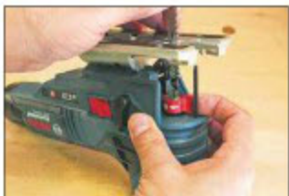
Pulling this lever allows the blade to be slipped in or ejected
