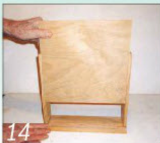
14 Slide the plywood base panel into place, and glue and pin its rear edge
