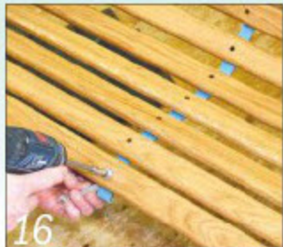
16 Drill the two holes and temporarily fit the spreader in place to the outer slats
