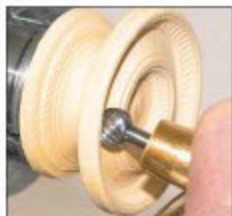
You push the tool into the wood to form the texture rather than moving it across the surface
