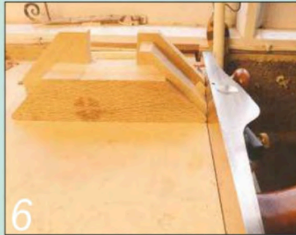
6 Plane the mitres true using the bird-house jig and shooting board; note scrap slip
