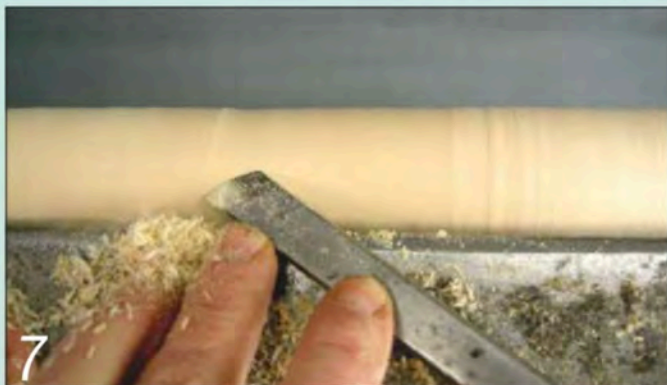
7 Use the gouge on its side to get a smooth finish, then switch to the skew chisel
