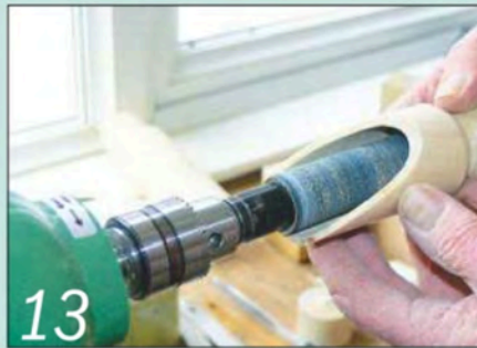
13 Switch to a smaller drum to sand the scoop's interior to a smooth finish
