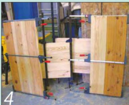
In rebuilding the carcasses, the older timbers would be presented to the front of each unit
