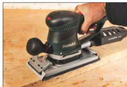
A front handle is fitted, but the sander can also be used single-handed
