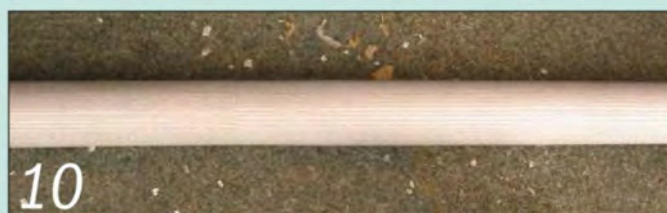
10 The join is reinforced with an ash spigot inside, and is virtually invisible
