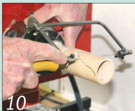
10 Fit a good-quality fretsaw blade into a jeweller's saw and start cutting
