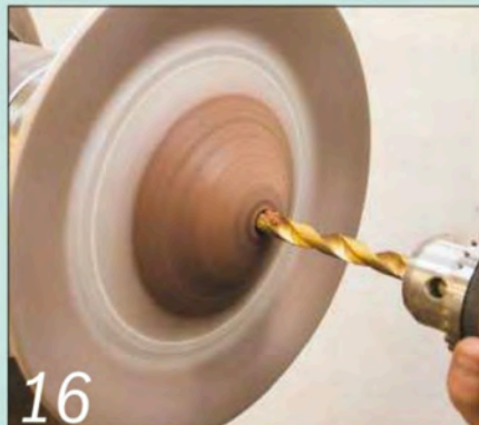
16 Drill a 10mm hole through the centre of the lid using a Jacobs chuck to take the finial
