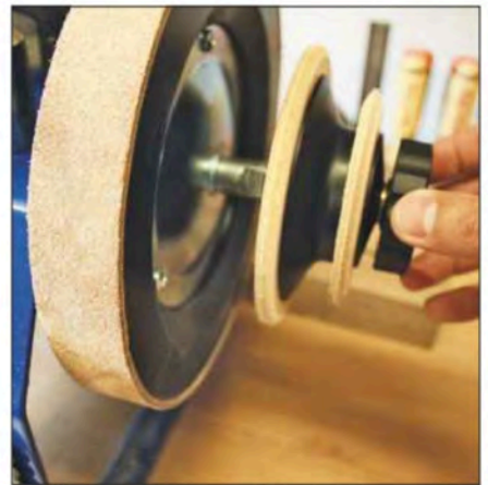
6 Shaped wheels are also available on some models for profiled blades
