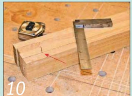
10 Work out the finished leg length and scribe a line (arrowed) at 12° at the top of one leg
