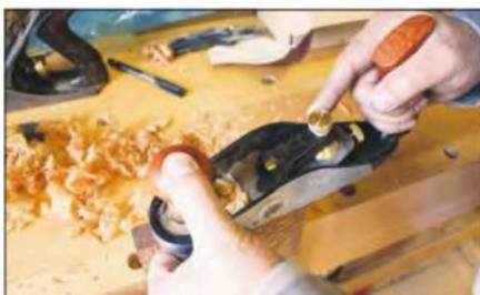
End-grain planing on some lacewood gave a smooth ride with no chatter
