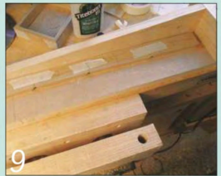
9 Lay out the pieces on a flat surface and tape them together end to end in numerical order
