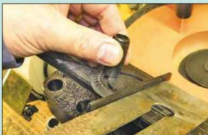
2 They also have a basic mitre fence to set the blades to specific skews
