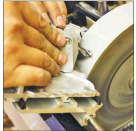
3 Top-end models have jigs available for specialist jobs such as tackling drill bits
