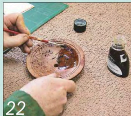
22 Paint the area to be gilded with size and allow it to become tacky
