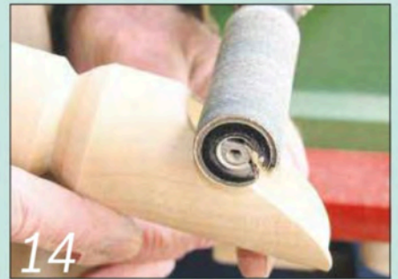
14 Use the same sanding drum to give the sawn edge a final smoothing
