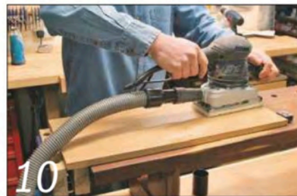
10 Ribbed extraction hoses can snag on the edge of the bench top, pulling the tool off-line
