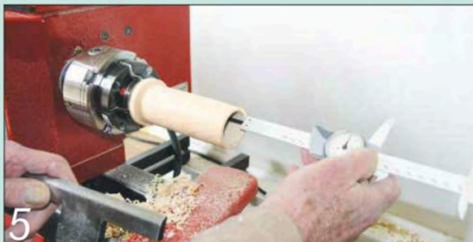
5 Measure the depth of the hole using a depth gauge or tape measure
