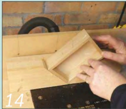
14 Rout the corner key slots using the key-slotting jig on the router table
