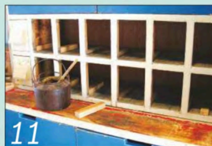
11 I brought in my classic glue pot to stick the replacement box drawer guides into place
