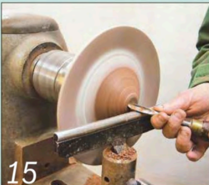
15 Refine the shape of the top of the lid by taking light cuts with a small spindle gouge
