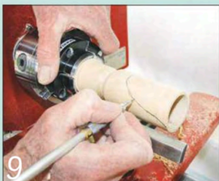
9 Draw a pencil line on the scoop to show where the wood is to be cut away
