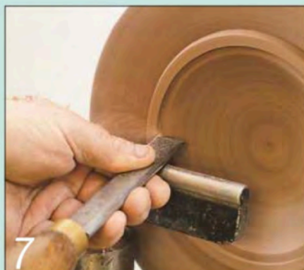
7 Cut a step at the junction of the rim and bowl for the lid to fit in
