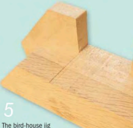
5 The bird-house jig makes simple work of planing mitres true
