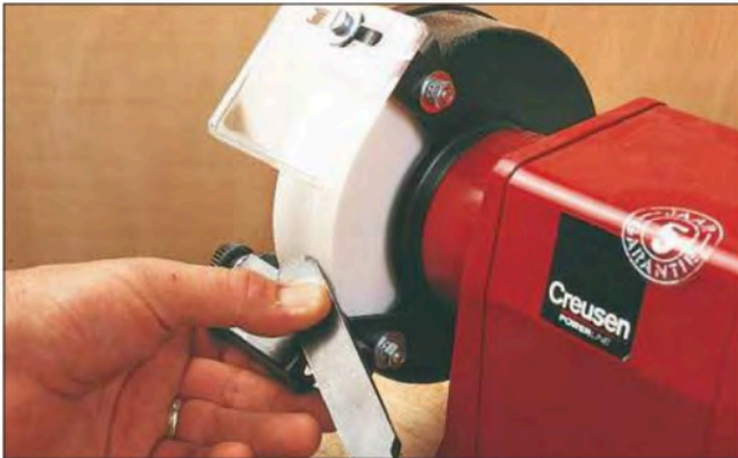
4 A competent user can shape turning tools by working freehand...
