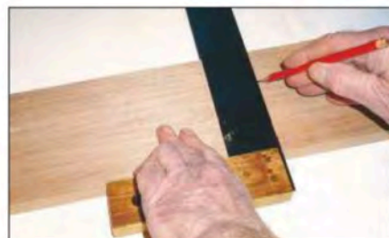
The try square's steel blade is at a true 90° to the brass-faced stock
