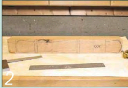
2 Mark the outline of the central column on a square oak blank...
