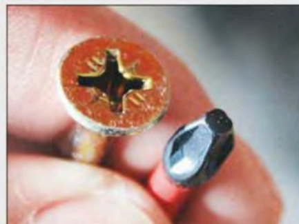
A special bit is provided with each box, matched to the screw head
