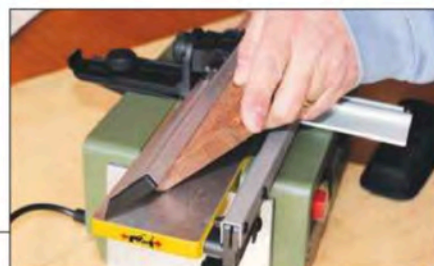
The fence will also tilt inwards, stopping the work sliding down the fence
