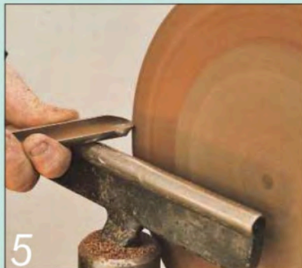
5 Use the tip of the bowl gouge to define the first 40mm of the rim
