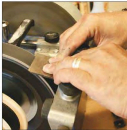
5 Polishing on a leather wheel can give the ultimate edge on your tools
