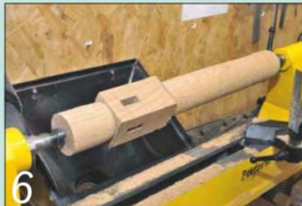
6 Cut the sharp corners of the square centre section with a skew chisel
