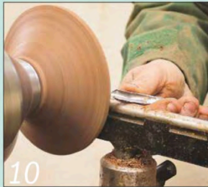
10 Take light cuts on the edge of the lid to create a small chamfer
