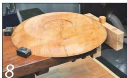
These dogs and a modified tail vice allow me to hold curved work securely
