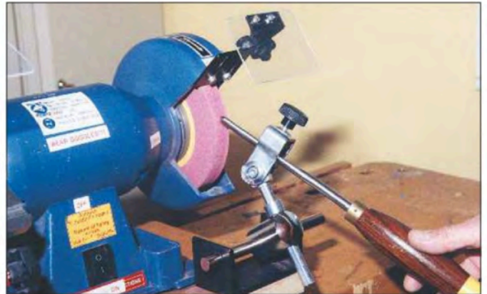
5 ...but jigs are better for getting repeat accuracy on shaped profiles
