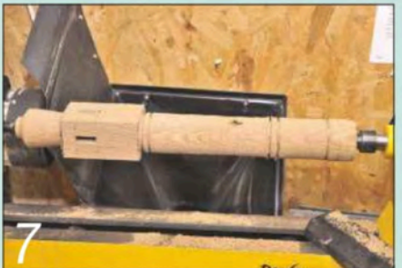
7 Cut down to the lowest points in the design with a parting tool to act as a datum
