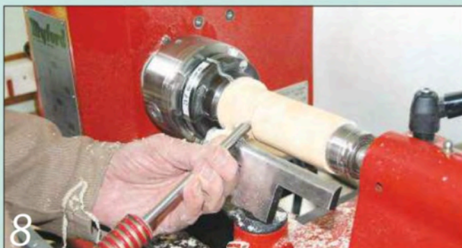
8 Cut a V-shaped groove on the line to begin the shaping of the scoop
