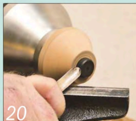
20 Make a small button with a 10mm spigot to fit in the hole on the inside of the lid
