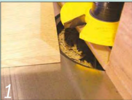
I fielded the edges of the top and bottom panels using the spindle moulder
