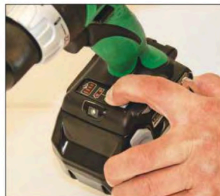
The battery check and light on-off buttons are located on the base
