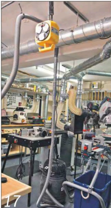
I've tie-wrapped its flex and hose together to keep them out of harm's way
