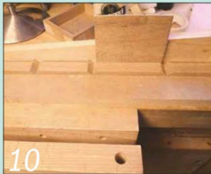
10 Flip the strip over onto its back and insert the base panel into one of its grooves
