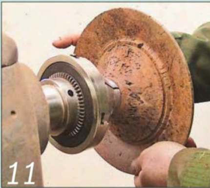
11 Offer up the base to the lid to check the fit, and adjust it as necessary
