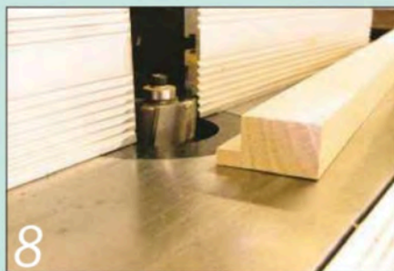
8 I cut rebates in the door rails and stiles on the router table before assembly
