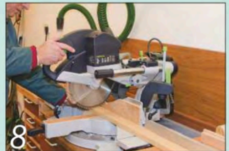
8 I always use a bench stop on my saw when I'm making repeat cuts
