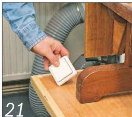
I can now turn the cleaner on from anywhere in the workshop using the remote control
