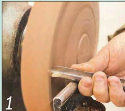
1 Mount the base using a faceplate and shape the outside with a bowl gouge
