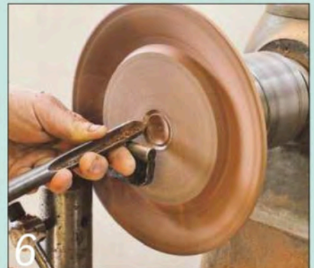
6 Then hollow out the central section, gradually working out towards the rim
