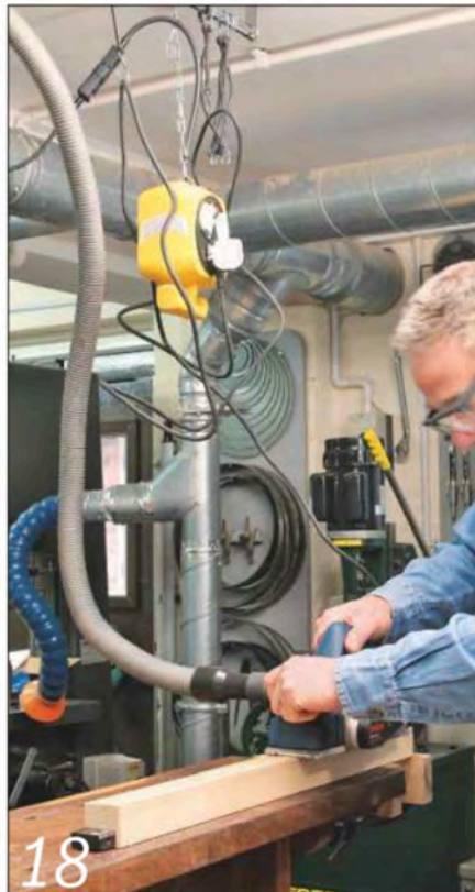
The rail and bungee strap system allows me to keep flexes off the bench
