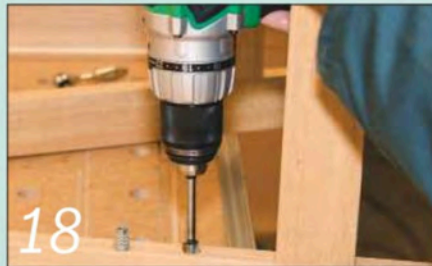
Use a 16mm Forstner bit to drill a shallow recess so the insert will fit flush
