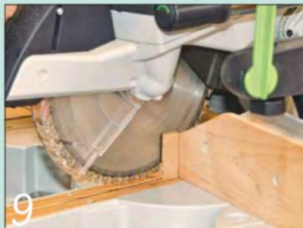
9 Use the saw again to trim one end of each leg to an angle of 12°
