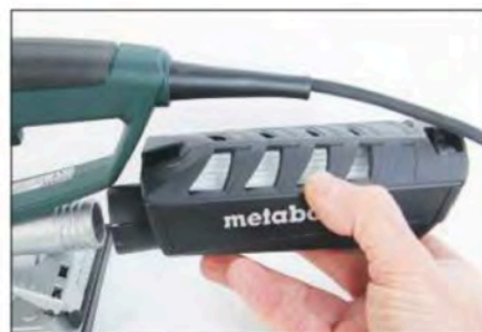
The filtered dust bag is a simple push fit on the extraction port
