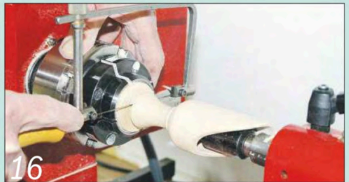
16 Turn off the lathe, cut through the handle stub and sand it smooth
