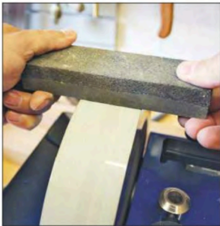
4 You can alter the stone to give a faster or finer cut with a grading stone
