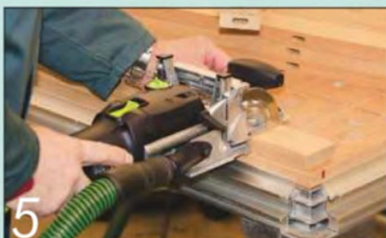
5 The Festool Domino is a power tool that has revolutionised my joint making
