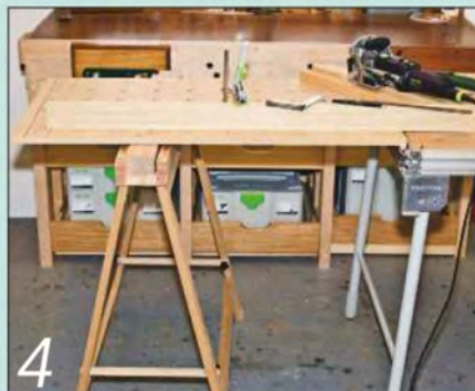
4 Rotate the insert through 90° and it's perfect for supporting the MFT3 extension
