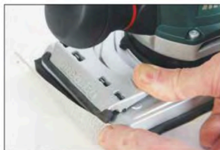
Strongly sprung metal clamps secure the abrasive sheet to the pad
