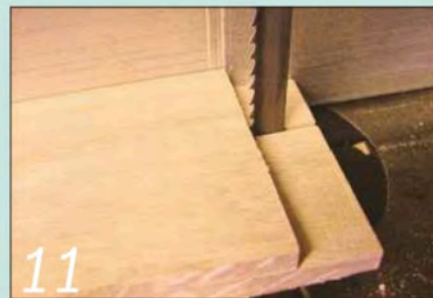
11 I then cut the tenon haunch on the bandsaw; once again, you can use a tenon saw instead
