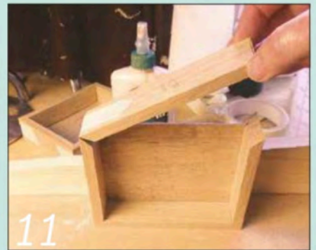
11 Roll up the box to form a rectangle round the base panel and tape the final corner closed
