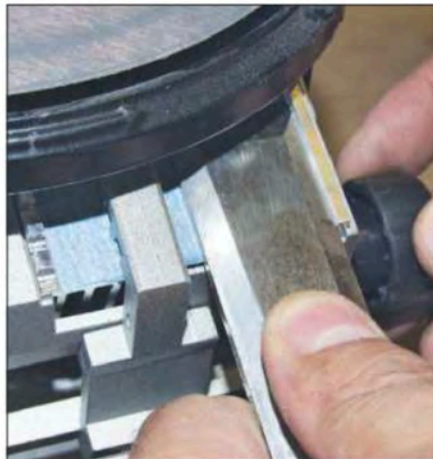
1 The Worksharp system has an adjustable angle setter for sharpening basic tools
