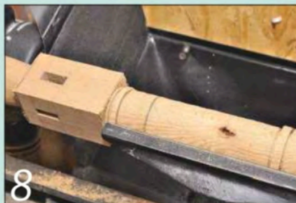
8 The thick pencil line shows the point where the column is at its widest
