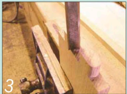
I cut the tenons on my WoodRat and chiselled their ends to match the shape of the mortises
