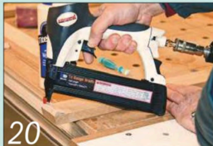
Glue and pin a softwood reinforcing pad to the outer edge of each foot
