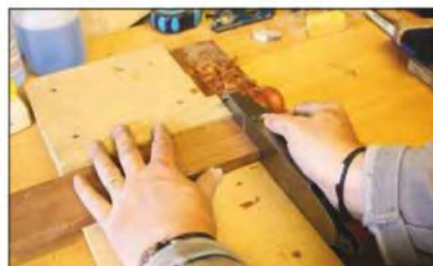
The plane is particularly easy to control when used on the shooting board
