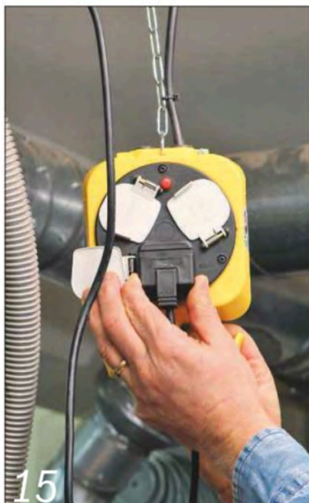
15 It allows up to six power tools to be connected to the one outlet point (but beware of overloading)
