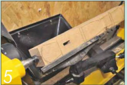
5 Centre the blank carefully and set the lathe to run at its lowest speed
