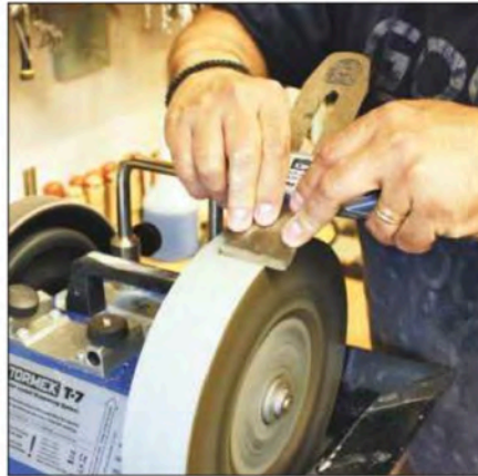
2 All vertical wetstones come with a jig for straight-edged blades
