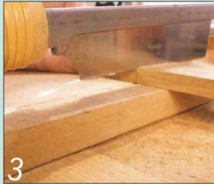
3 Separate the four box sides by cutting squarely across the strip
