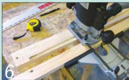
6 Routing a slope on one of the sides for the draining board
