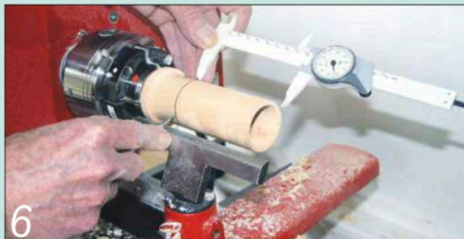
6 Mark a line on the outside of the blank to indicate the extent of the hole
