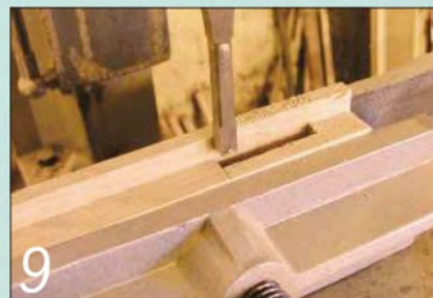
9 The mortises in the door stiles were cut flush with the face of the rebate
