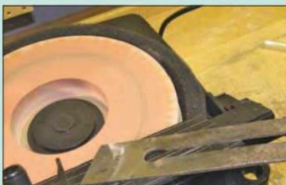
1 Horizontal grinders have a magnetic tool rest that tilts to suit the grind angle
