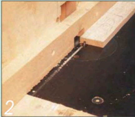
2 Cut grooves in the box sides on the router table to take the base panel
