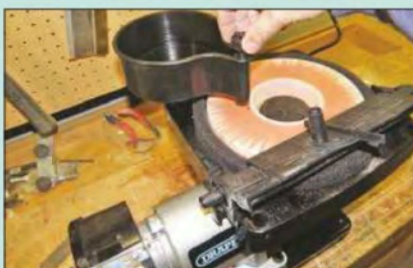
3 A reservoir with adjustable flow keeps the stone wet during grinding
