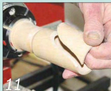
11 The fine No 7 blade leaves an exceptionally smooth and accurate cut
