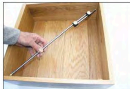
Use the pointed tips for diagonal measurements. You can add extension rods as required
