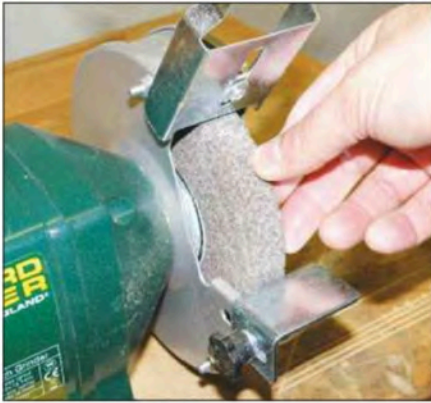
1 Budget grinders often come fitted with a basic grey carborundum wheel
