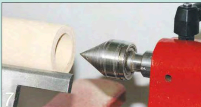
7 Remove the drill chuck and fit a large-diameter revolving centre
