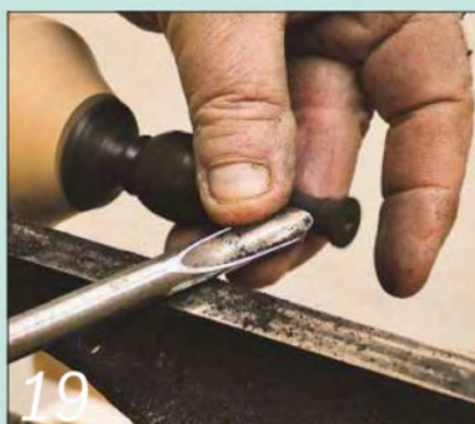
19 Remove the tailstock and support the piece by hand while you make the final cuts
