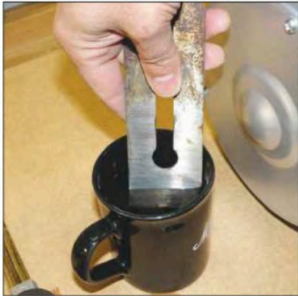
1 Dry-grinding steel needs constant quenching to prevent edge bluing
