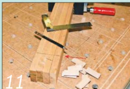
11 Measure down from the scribed line to mark the centre line on all four legs
