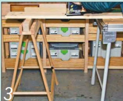
3 The trestle is 900mm high with the sacrificial insert fitted this way round
