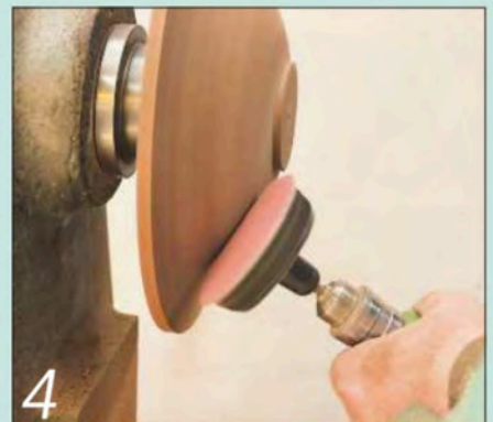
4 Power sanding is a quick process, but it does create a lot of dust. Finish sanding by hand
