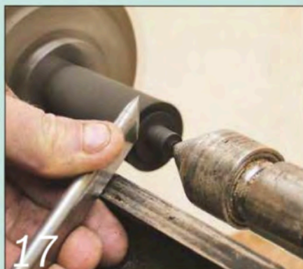
17 Cut a 10mm spigot on the finial and undercut the shoulder with a slicing skew chisel cut
