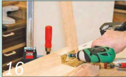
Support each leg frame with cramps while you hinge it to the top section
