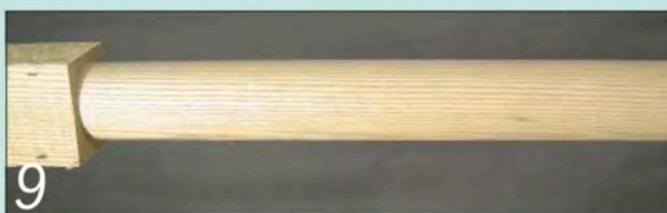
9 Really sharp tools guarantee a clean finish on both slicing and planing cuts
