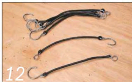
12 To attach the hoses to the rail, I bought some bungee straps with hooks
