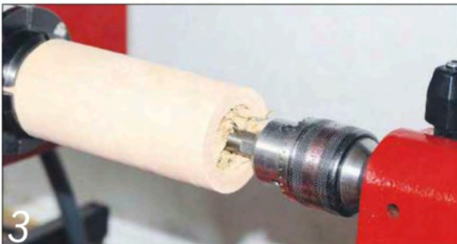
3 Advance the tailstock and bore a hole in the cylinder to a depth of 75mm
