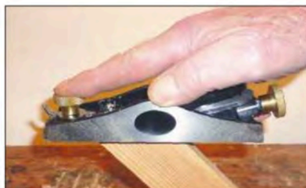
The block plane is ideal for one-handed use on end-grain surfaces
