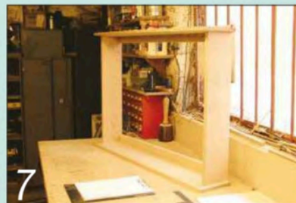
7 The two rear cleats were biscuit-jointed to the top and bottom panels
