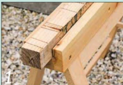
1 The sacrificial insert in the U-shaped top extends the life of these trestles
