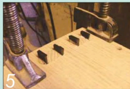
5 I bandsawed slots in the tenons and tapped a small glued ebony wedge into each one
