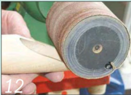
12 Sand the sawn edge of the scoop smooth using a large drum sander
