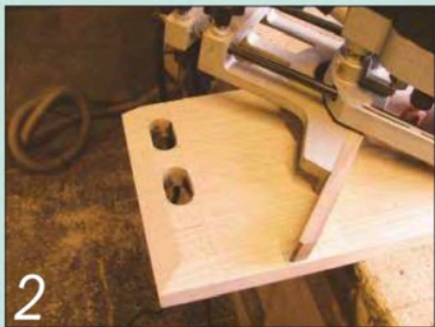
The rounded mortises in the top and bottom panels were cut using the router
