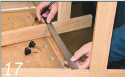
Lay the assembled trestle on its side so you can measure up the leg braces
