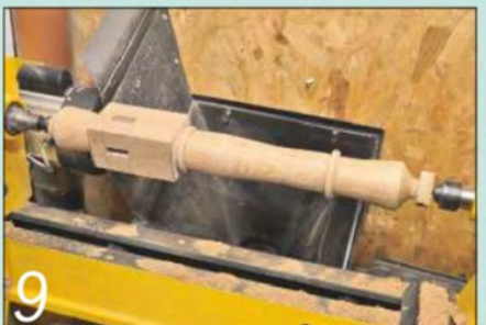
9 Finish shaping the central column by forming the two half-round beads
