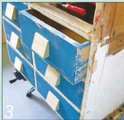
I fitted new drawer bearers where necessary, but kept other interventions to a minimum
