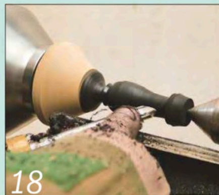
18 Fit the spigot in a hole in a scrap block. Then shape the finial with a spindle gouge
