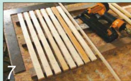
7 Remaking the slatted shelves, note spacer and pin gun for speed and convenience
