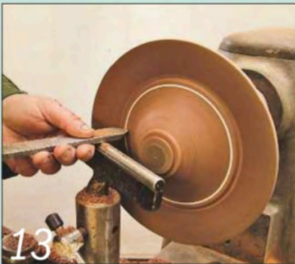
13 Re-chuck the base, fit the lid and blend in the curve with a scraper
