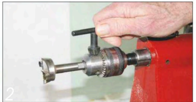
2 Fit a Forstner bit in a drill chuck in the tailstock and tighten the chuck
