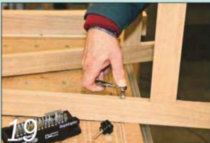
Fit the screw inserts in their holes using either an Allen key or a hex driver
