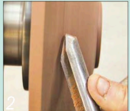
2 A shear cut with the bottom wing of the gouge should leave the surface with few blemishes
