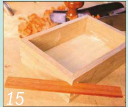
15 The thin key strip should be a sliding fit in the corner slots
