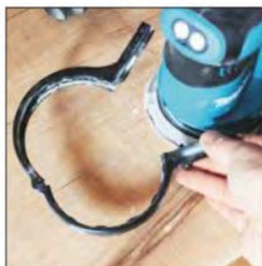
The dust collar fits round the base, and can be rotated easily
