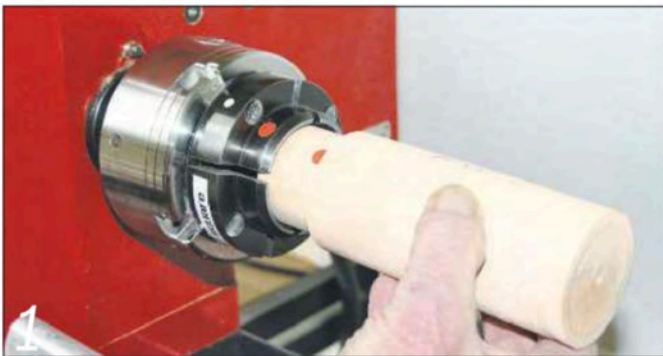
1 Turn the blank to a cylinder and form a spigot to suit your chuck jaws
