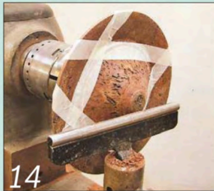
14 Masking tape will prevent the lid from flying off across the workshop!
