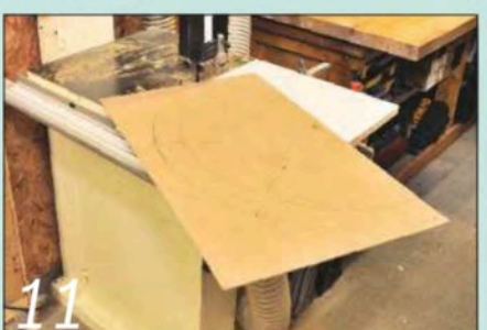
Mark the quadrant on a piece of mdf and use a circle cutting jig on the bandsaw
