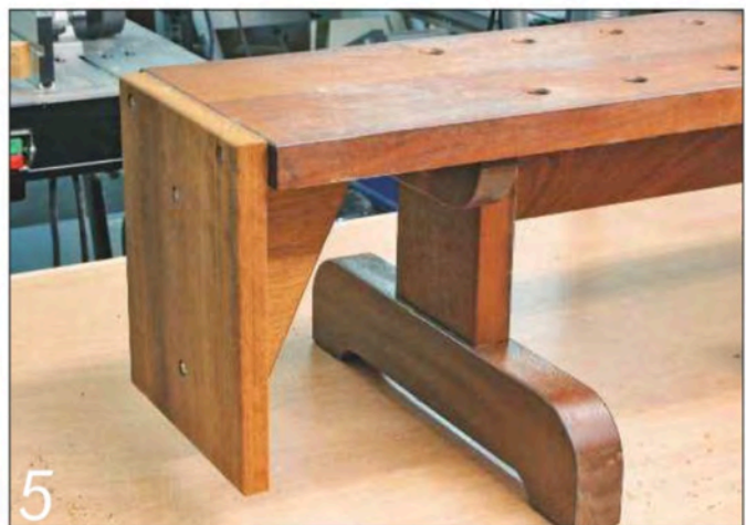
I screwed a vertical cramping board to the end of the new routing bench...
