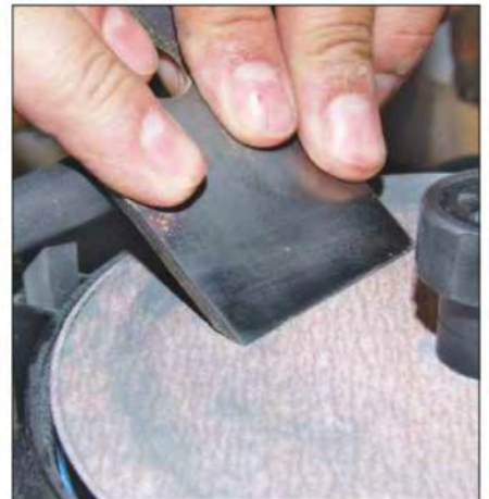
2 Wider blades such as plane irons can be worked on the top of the platen
