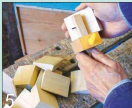
I followed the design of the original drawer handles in close-grained tulipwood
