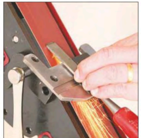
4 The advantage of a dry abrasive belt is that the resulting bevel is flat
