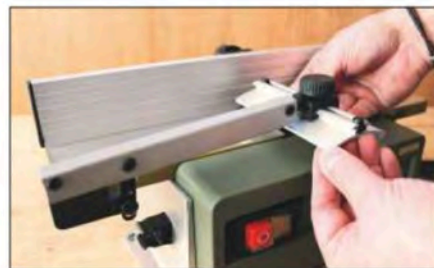
The bridge guard has a sprung arm to keep it tight to the beds
