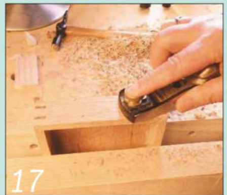
17 Clean up the corners and the keys with a sharp block plane
