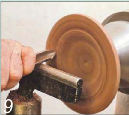
9 Then reverse-mount it on the chucking spigot and hollow out the inside
