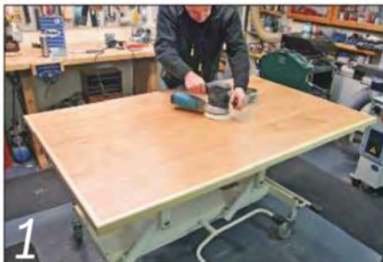
1 The adjustable-height assembly bench I converted from an old hospital bed has been a superb addition to my workshop facilities
