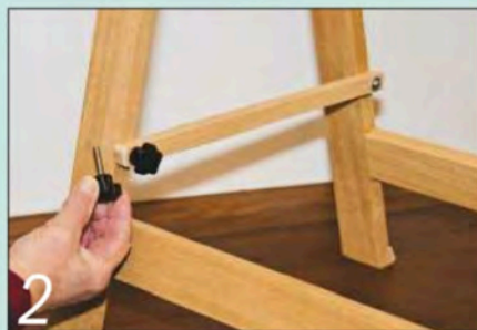
2 Horizontal braces between the leg frames are essential for stability
