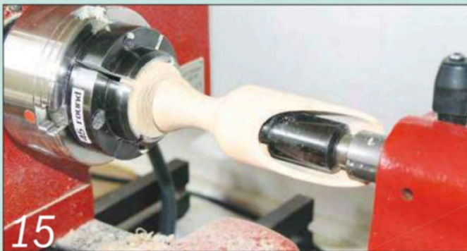
15 Shape the handle and the base of the scoop to match the pattern
