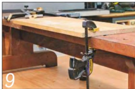
9 The wide overhang of the top makes it easy to clamp flat work anywhere on the bench
