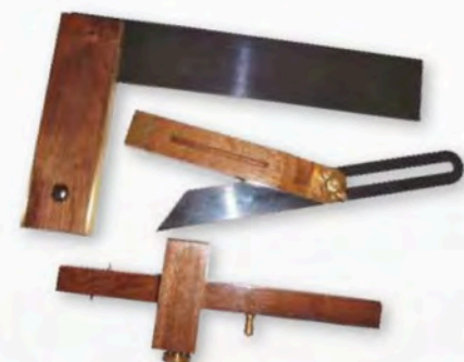
The measuring and marking tools are unbranded but quite serviceable
