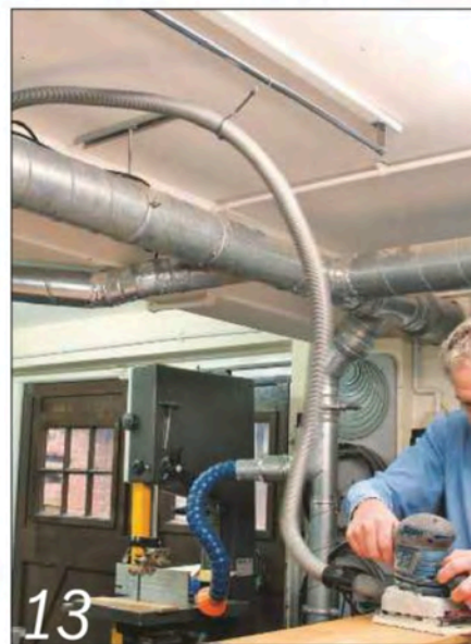
13 This overhead arrangement worked perfectly, allowing the hose to move as I did
