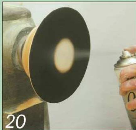
20 With the lathe revolving very slowly, spray the rim of the bowl with ebonising lacquer and allow it to dry. Then remove the faceplate from the lathe and undo all but one of the fixing screws
