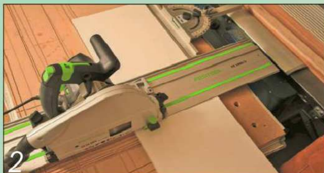
2 My Festool TS75 plunge saw is the ideal tool for cutting mfc to length...
