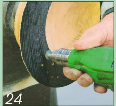
24 I use a sharp countersink bit in a power drill to add the stars to the rim. The different sizes are made by drilling to different depths. Cover the whole rim randomly with the stars...
