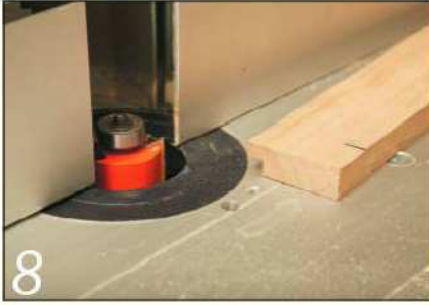
8 Rout a rebate in the meeting stiles of paired doors to keep dust out
