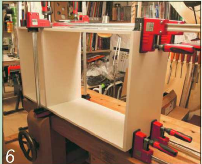
6 Apply glue to the remaining joints, assemble the carcass and clamp it up
