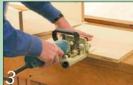
Biscuit joints are the ideal way of assembling the open box frame
