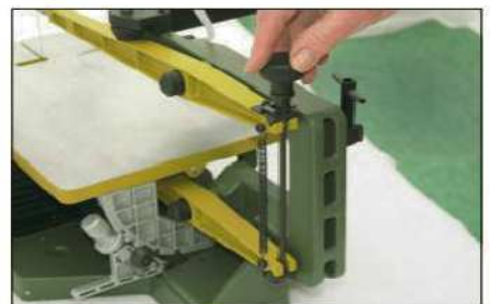
This knob at the back of the top arm sets the blade tension
