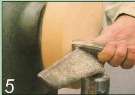
5 You can use the same bevel-supported push cut to start shaping the bottom of the bowl
