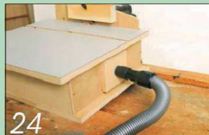
24 The extraction set-up worked well, with the table kept free of shavings
