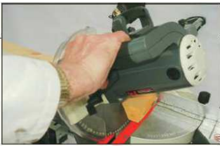
Bevel cuts can be made only with the body tilted left
