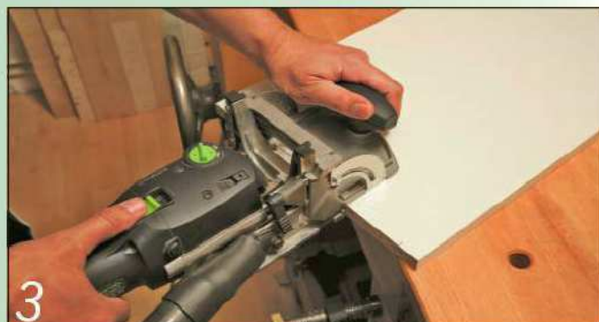
3 ...while my Festool Domino makes light work of creating loose tenon joints
