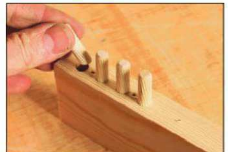
9 Drill the dowel holes, remove the jig and glue the dowels into one component
