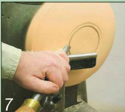
7 Cut away the waste near the foot with a pull cut. Then finish shaping the bottom of the bowl with a combination of both push and pull cuts
