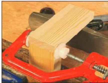
4 Use a clamp if necessary to hold the two components you want to join in position
