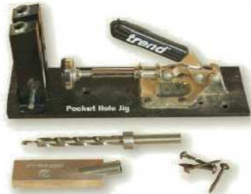
1 The jig can be a complex affair with clamps and fences (top) or a simple guide block (bottom)
