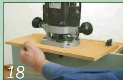
18 Drill a second hole for the locking bolt and mark the line of the curved slot (see text)
