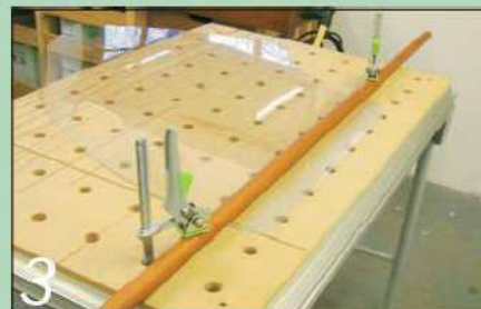
3 I found it helped to trap one edge of the cyclone body under a broomstick...
