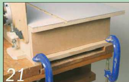
21 It's a good idea to clamp the router table to the workbench for extra stability
