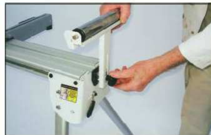
The two support rollers are readily adjustable for height
