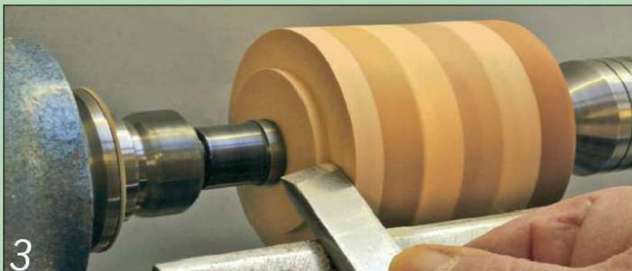
Form a dovetail spigot at one end of the blank with the toe of the skew
