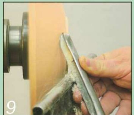
9 Take fine finishing cuts with the bowl gouge, keeping the handle down low and the cutting edge at about 45° to the surface of the wood
