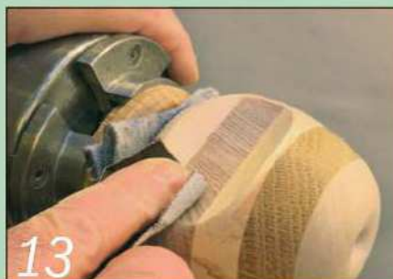
13 Stop the lathe and sand the bite, softening its edges slightly
