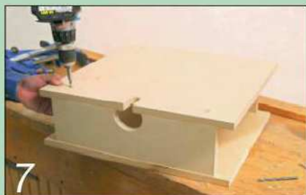
Centre the work table on the sub-top and screw it into place
