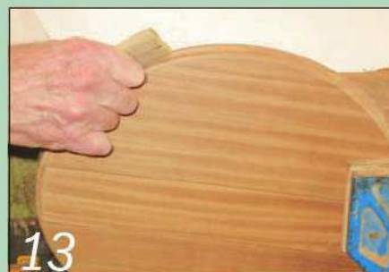
13 Smooth the finished edge with fine abrasive paper wrapped round a curved former
