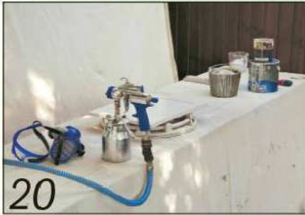
20 I used a spray system out in the garden to paint the face frames and doors
