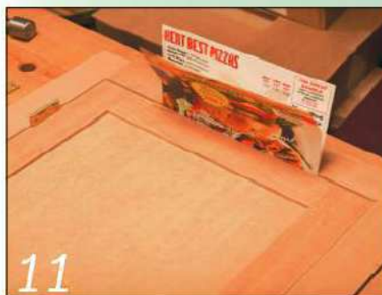
11 As a general rule I allow 1mm of clearance all round cabinet doors. A card spacer does the trick
