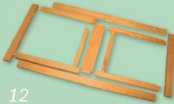
12 This shows all the components of the H-frame and the two sliding leaf frames
