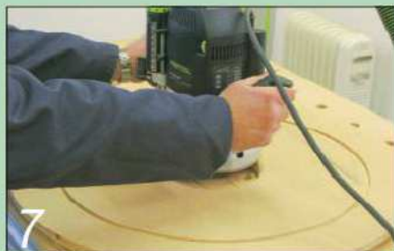
7 I cut out and grooved a circle of 19mm thick mdf to form the drop box lid...
