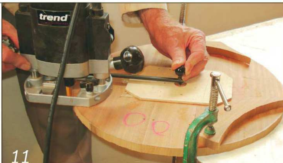
11 Trim the edges of the circle precisely to size using a router fitted with trammel bar
