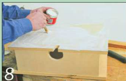
Brush contact adhesive onto the surface of the work table and the laminate
