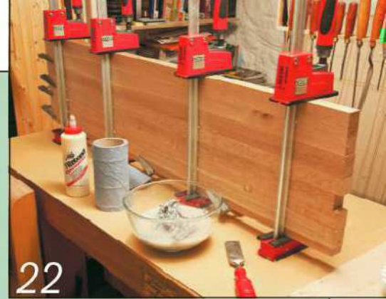
22 I laminated a number of oak offcuts together to make the TV shelf
