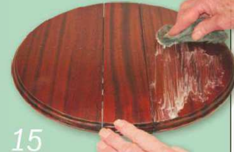
15 After applying the lacquer, treat the final coat with steel wool and wax
