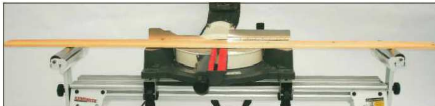
The extension beams slide out to provide a work support span of almost 3m
