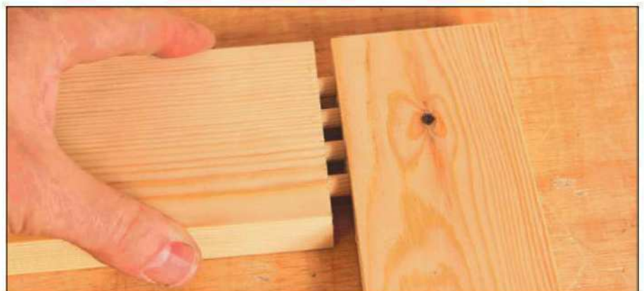
10 Apply glue to the exposed dowels and assemble the joint. Cramp it if necessary to get a tight fit
