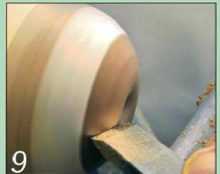
9 ...and then use the same tool to round over the edges of the recess
