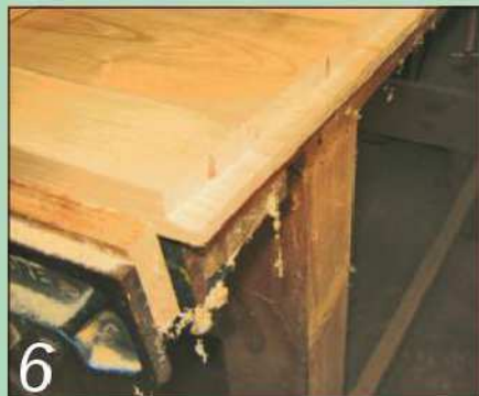
6 Make up the chestnut panels to size and cut rebates all round them
