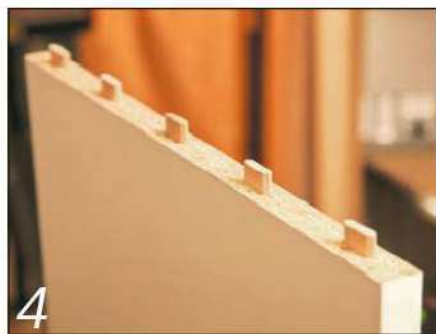
4 I used five evenly-spaced loose tenons in the end of this 300mm wide board
