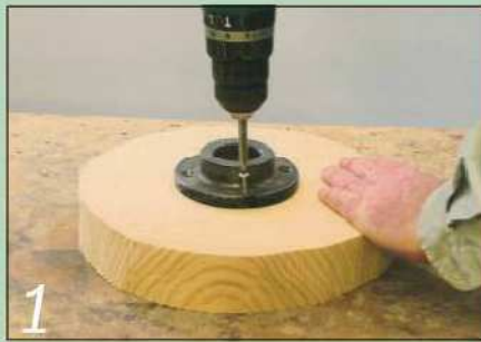
1 Decide which face of your blank is to be the top of your bowl, find its centre and screw your faceplate securely to it
