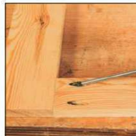
4 Align the two components and drive a screw in through each pocket hole
