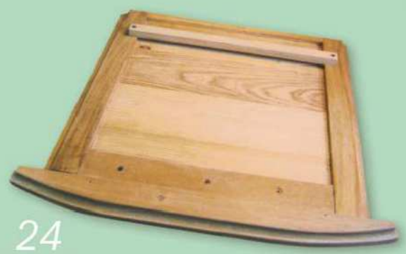
21 Then cramp the sliding leaves in the closed position and rout a profile all round the top
