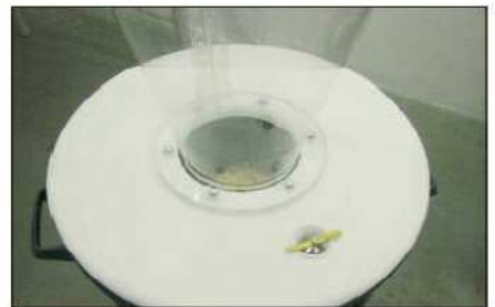
The completed lid is fitted with an improvised pressure relief valve
