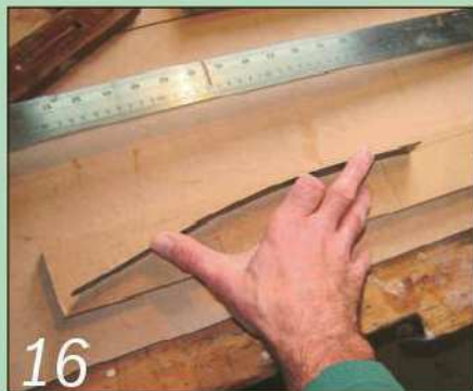
16 I made an mdf template to help me shape the two outer end rails
