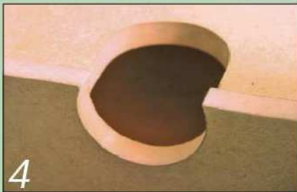
4 Form a clearance hole for the cutter in one side and the sub-top
