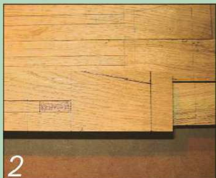
2 Use the same gauge setting to offset the markings on the face side of the legs
