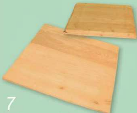
7 When the glue has dried, remove all the panels from their cramps
