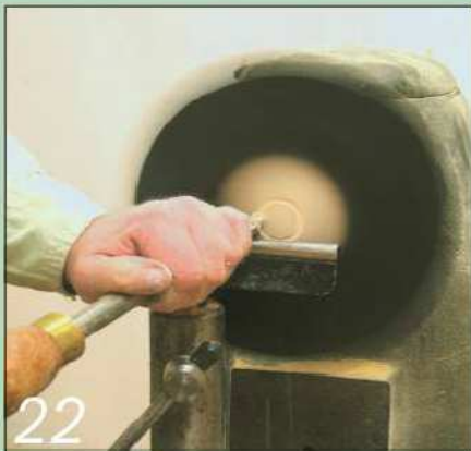
22 Remount the bowl on the lathe and reduce the speed. The whole piece is now considerably out of balance and must be turned much more slowly. Start the hollowing cuts near the centre...
