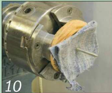
10 Pad the screw chuck's backing plate with a clean rag to avoid bruising the wood
