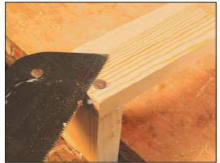
7 When the glue has set, trim the projecting dowels with a saw...
