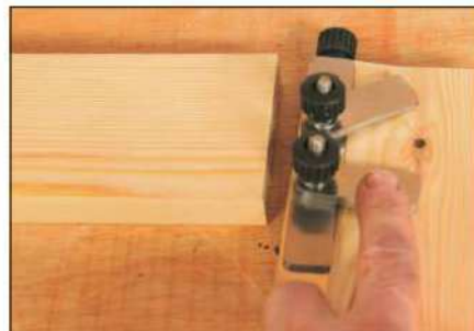
8 Place the components together again, with the jig still in position. Flip the end stop and the spacer tabs over onto the other component and screw the jig to it
