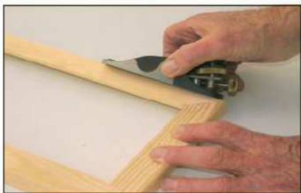
10 Chamfer the outside edges of the frame with a small apron plane
