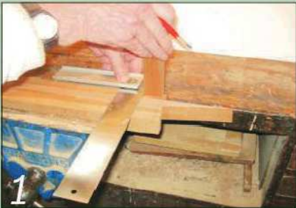
1 Mark out all similar components together to ensure their accuracy
