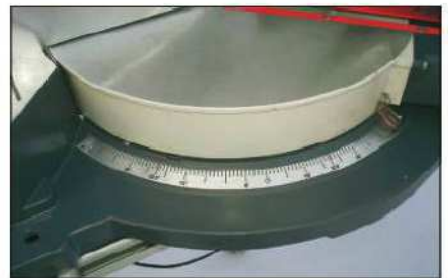
The base is embossed with a clear protractor scale
