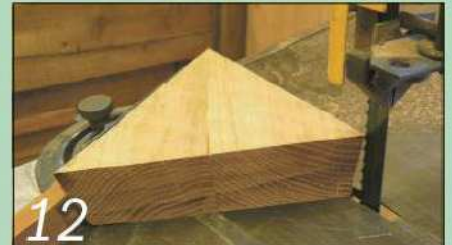
12 The second cut is made using the first cut as the register
