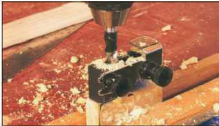
4 Clamp the jig and component in a bench vice and drill out the holes. Repeat the process for the other component
