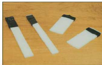
I wrapped self-amalgamating tape round one end of each strip to form a handle
