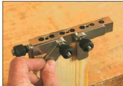
5 Clamp the workpiece vertically in the vice and use the spacer tabs to adjust the jig so it's in the centre of the workpiece
