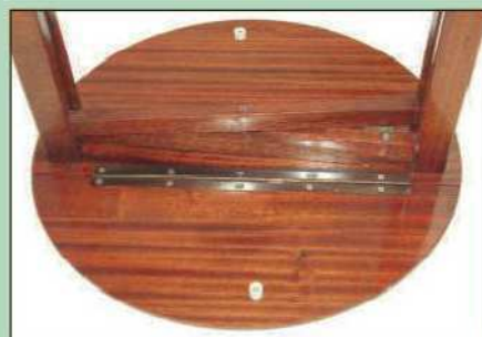
14 Drive in the four screws that attach the leg assembly to the top
