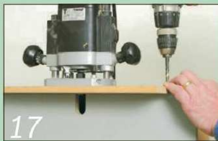
17 Position the router plate on the end of the table and drill the pivot point
