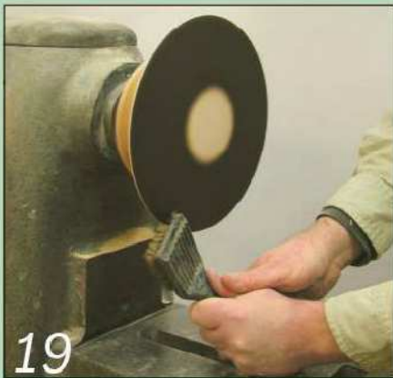
19 Use a soft brass wire brush to remove any loose carbon residue from the scorched area. The brush will also pick out the softer, spring growth, enhancing the grain of the wood
