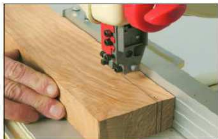
Replacing the supplied blade worked miracles; the original one made the cut alongside
