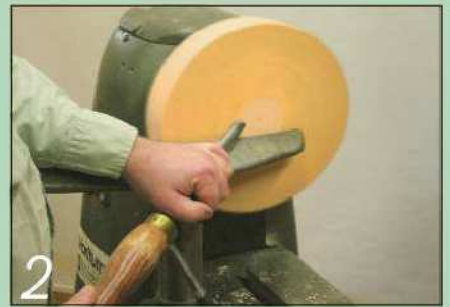
2 Mount the blank on the lathe and true up the base, using a pull cut with a fingernail profile bowl gouge
