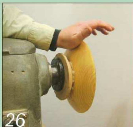
26 A couple of gentle taps from behind are normally enough to break the hot glue joint and release the bowl. If it's stubborn, remove the piece from the faceplate and microwave it for 30 seconds on low heat. This should soften the glue enough for you to remove the bowl from the mdf
