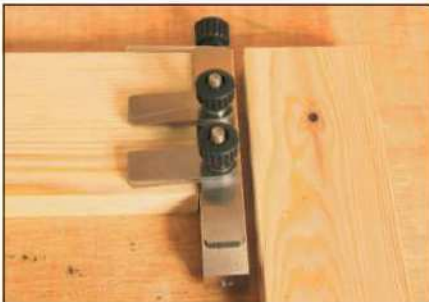
4 Place the jig between the two components and turn the end stop to locate the jig flush with the edge of the tenon component
