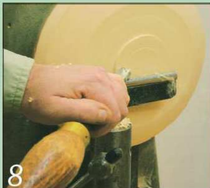
8 Give the underside of the foot a slightly concave profile so the finished piece will stand flat on the table or shelf surface
