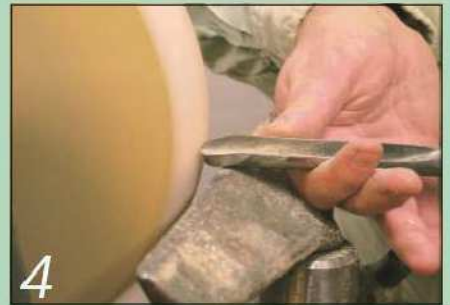
4 True up the edge of the blank with the same gouge, this time using a push cut
