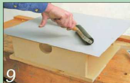
Stick the laminate in place and roll it to remove any air bubbles
