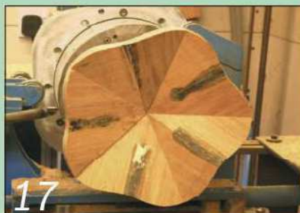
17 Remount the piece and remove the sacrificial wedges so you can turn the interior to shape
