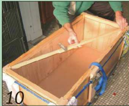
10 Assemble the carcass, cramp it up, check that it's square and set it aside to dry
