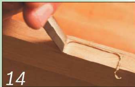
Square up the rounded corners of the hinge recesses with a sharp chisel
