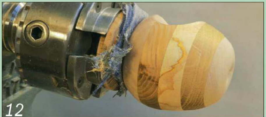
12 Sand the whole surface smooth and blend the edges of the layers together
