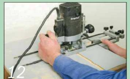
12 Cut the slot for the mitre guide with a single pass of the router
