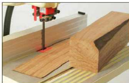
The new blade produced a wafer-thin veneer with ease from 75mm thick material
