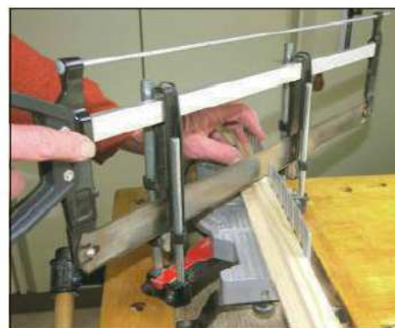
6 I cut the corner mitres on my Proman saw, which has a very fine blade
