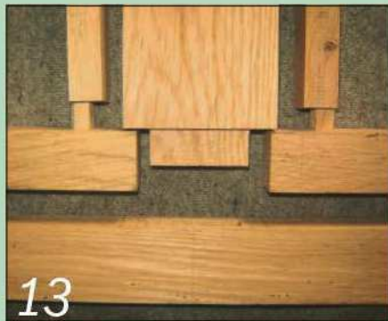
13 Here you can see how the various parts fit together around the centre rail
