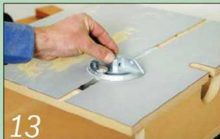
13 This will help to ensure that the mitre guide fits snugly in the slot
