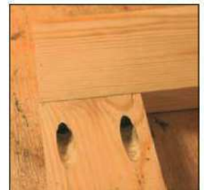
5 The pocket holes can be filled with specially shaped hardwood dowels
