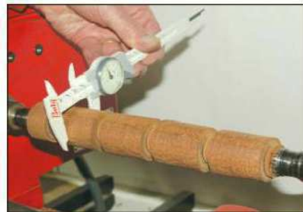
1 Mount the blank between centres and turn it to a diameter of 40mm
