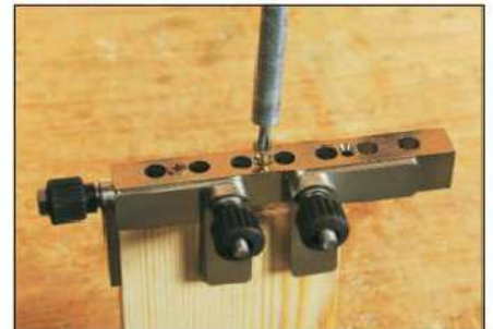
6 The jig can be screwed or clamped to the workpiece. If it's screwed, the screw holes will be hidden within the assembled joint
