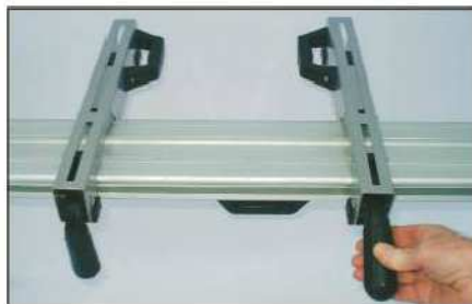
The cross supports lock to the rails with good-sized cam-action levers
