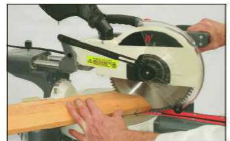
Cutting mitres to left or right is quite straightforward
