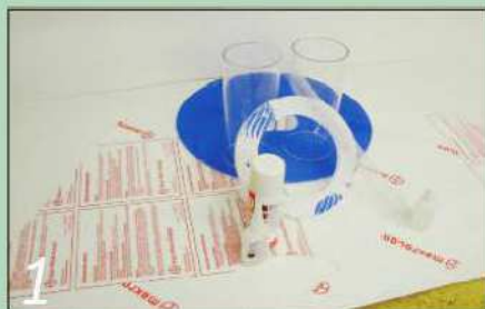
1 The kit includes the cyclone body, the foot, the lid and two tubes of special adhesive
