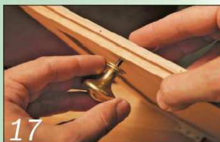
Drill clearance holes for the door handles and fit them in place
