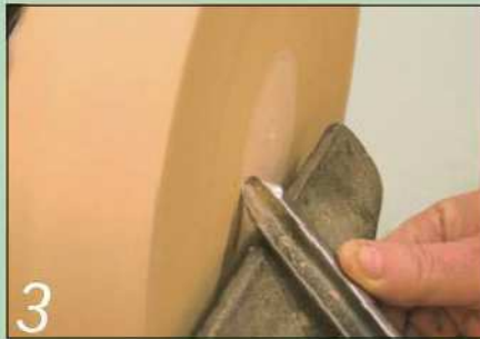
3 This is a close-up shot of the pull cut, showing exactly where the shaving should come off the flute of the gouge
