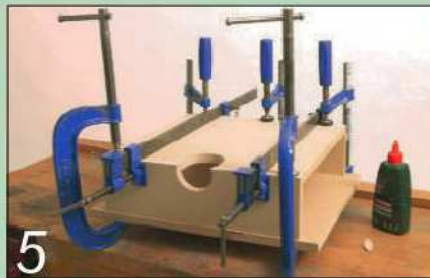
5 Glue and clamp up the box frame and check that it's square
