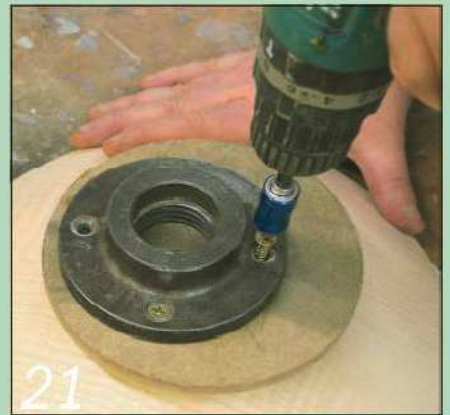
21 Loosen the last screw and rotate the faceplate through about 15° (the same as moving it by one hour on a clock face). Tighten the loose screw and drive in the others
