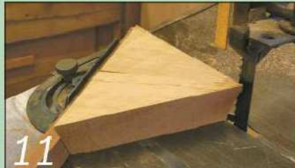
11 The base of the glued-up triangle acts as the register for the first cut
