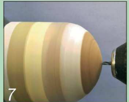
7 Drill a 3mm diameter hole deep enough to take the screw chuck
