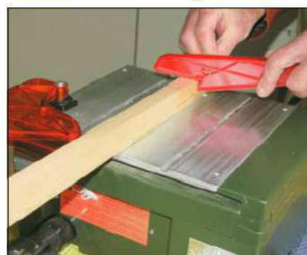
4 I cut the rebate in the frame timber on my Proxxon table saw
