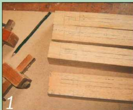
1 Mark the positions of the mortises and grooves on the face edge of the four legs
