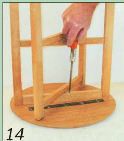
14 Drive in the four screws that attach the leg assembly to the top
