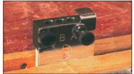
3 Take one of the parts and locate the jig on it with the centre line set on the alignment marker of the jig
