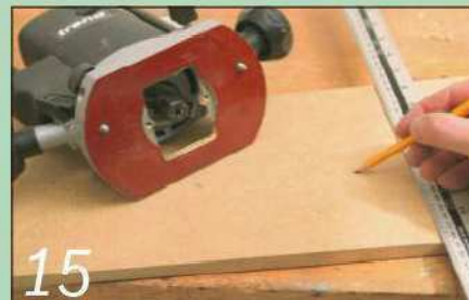
15 Mark the positions of the router fixing screws on the router plate
