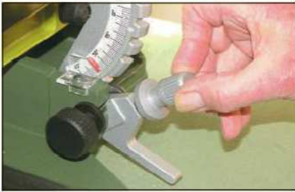
The knob that secures the table angle needs a locking mechanism to stop it from moving while the saw is in use
