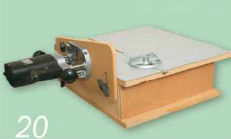
20 Finally reattach the router to the plate and you're ready to start work
