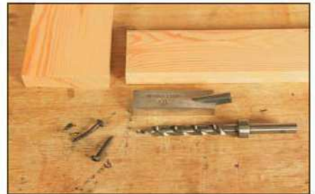
2 Prepare the two components, ready to be butt-jointed together
