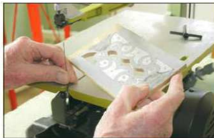
Reconnecting the blade for internal cutting was very difficult
