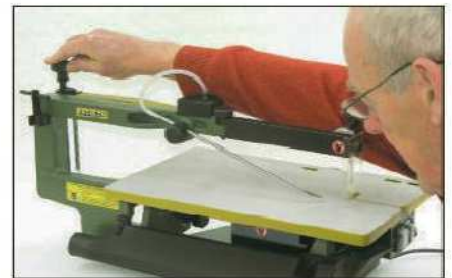
The quick-release blade tension lever is a long reach away
