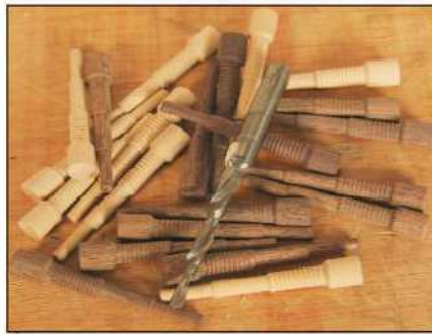
2 Three sizes of drill and dowel are available, in a choice of four woods
