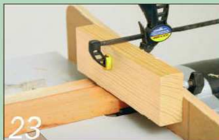
23 I created a temporary guard by clamping a block of wood to the router plate
