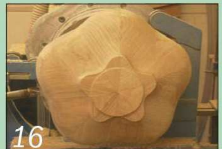
16 Then make further cuts to start refining the shape of the exterior
