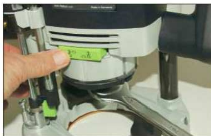
The clever ratchet system on the spindle lock makes cutter changes quick and simple
