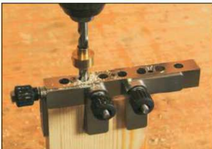
7 Set the depth stop on the drill bit and bore out the dowel holes in the end of the workpiece
