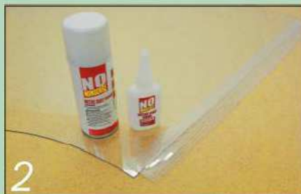
2 The joining strip supplied with the kit is first attached to one side of the cyclone body
