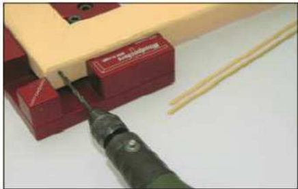
9 Reinforce the mitre joints by inserting a short length of glued bamboo dowel
