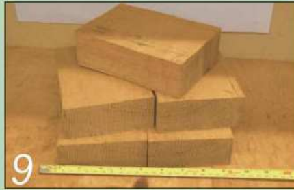
9 The starting point was a pile of five Japanese oak offcuts measuring 150 x 110 x 50mm...
