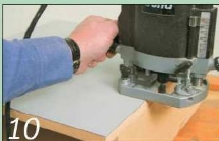
10 Use a bearing-guided cutter to trim the laminate all round...
