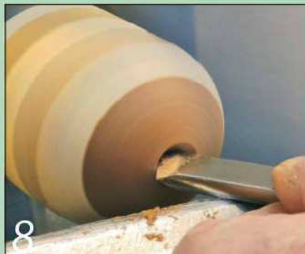
8 Form the recess where the stalk will go using the toe of the skew chisel...
