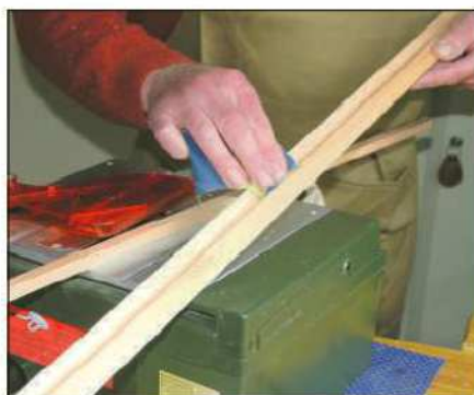
5 Its dado head accessory and TCT saw blade gave a very fine finish to the frame sections
