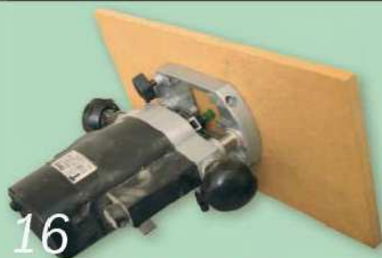
16 Attach the router, fit a straight cutter and plunge a hole in the plate
