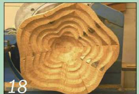
18 The internal shape is established slowly, working level by level. See page 69 for the finished bowl
