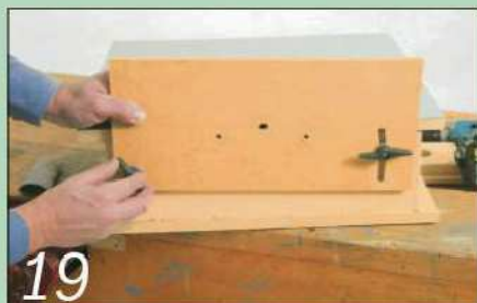
19 Cut the curved slot with the router, then reattach the router plate
