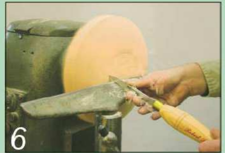
6 Start to form a foot for the bowl using a parting tool. It's just under one third of the bowl's diameter and about 3mm deep
