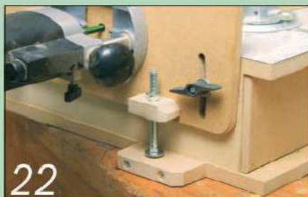
22 My first modification was to attach a simple fine-height adjuster to the router plate
