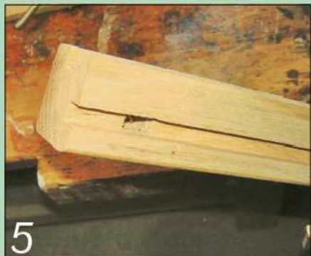
5 Form the grooves on the inner faces of the legs, running them through the top mortises
