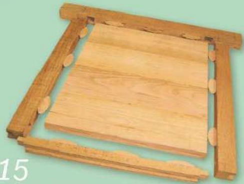
14 I made up the panels for the two sliding leaves using biscuit joints for strength
