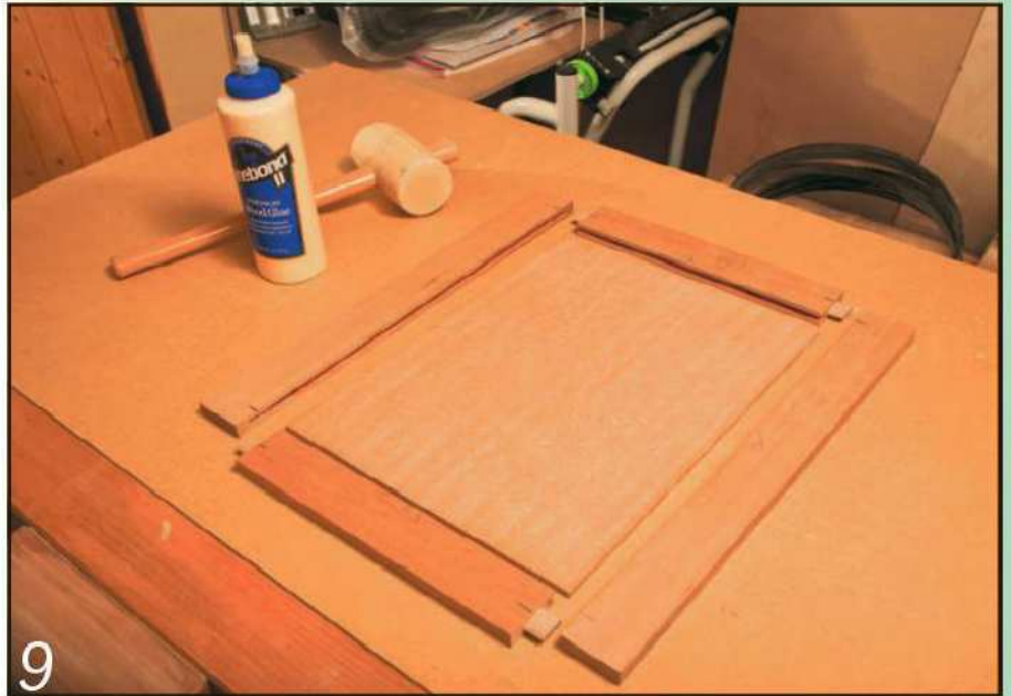
9 Cut the grooves in the door frame for the mdf panel and test its fit
