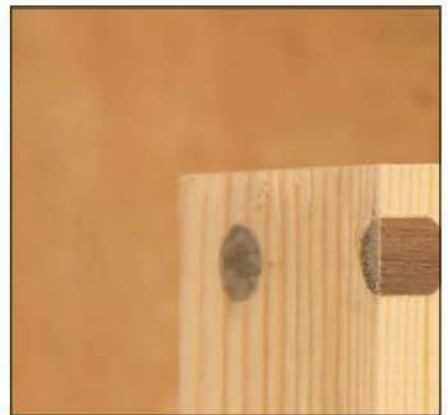
9 A cross-section through the finished joint reveals the dowel's excellent fit
