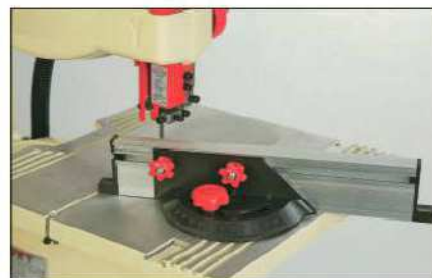
The fence is fine, but the mitre guide is only any use for setting approximate angles
