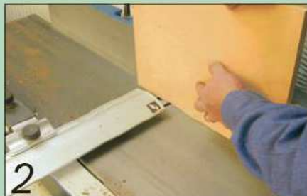
Use just one end of the cutter block when planing up the components
