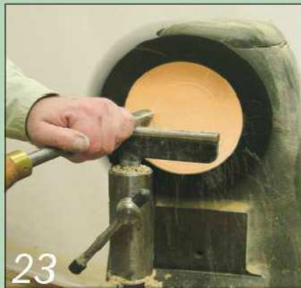
23 ...and work out towards the rim. When you're happy with the profile of the bowl and the width of the rim, power-sand it to a finish. Take great care not to damage the lacquered rim
