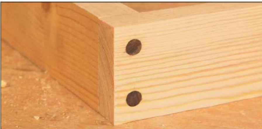
8 ...and finish them perfectly flush with the surface using a sharp block plane
