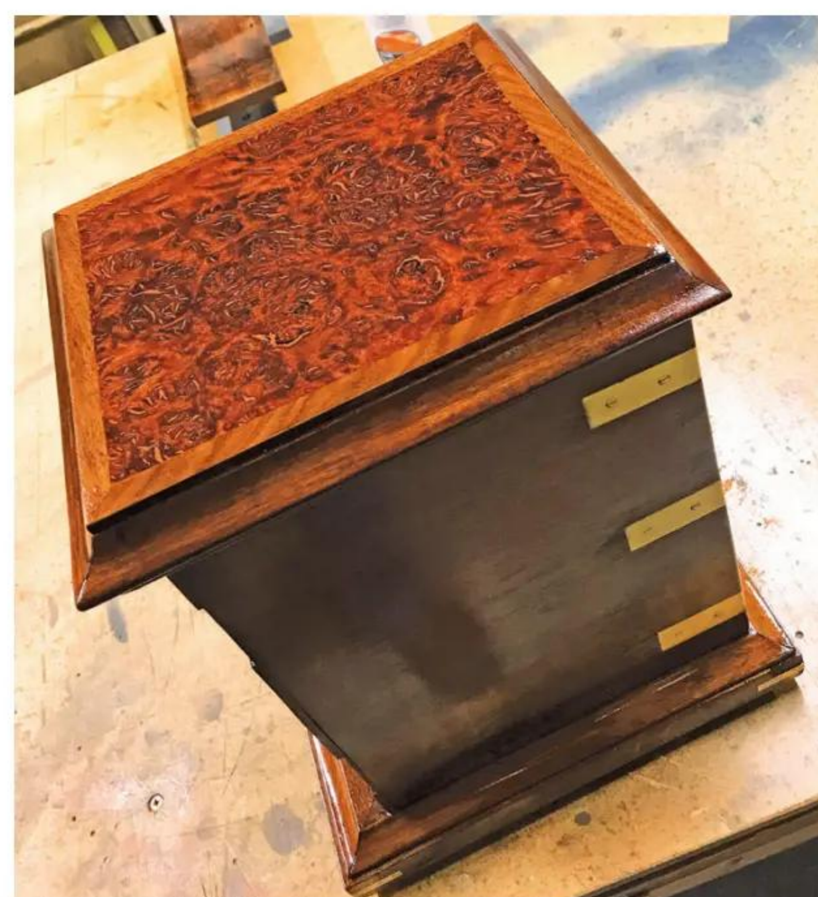
20 This was followed up by lacquer, then, eventually, cut back and waxed
