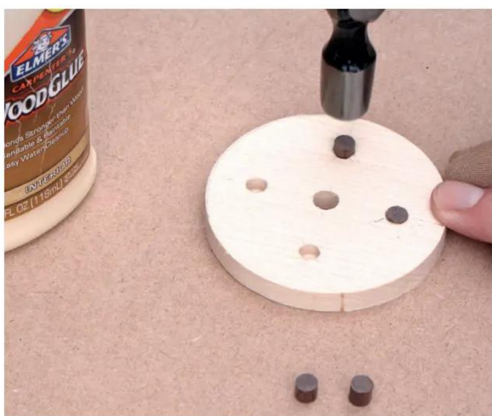
19 Carefully mark 3, 6, 9 and 12 positions on the dial. Drill to half depth, then glue dots in place
