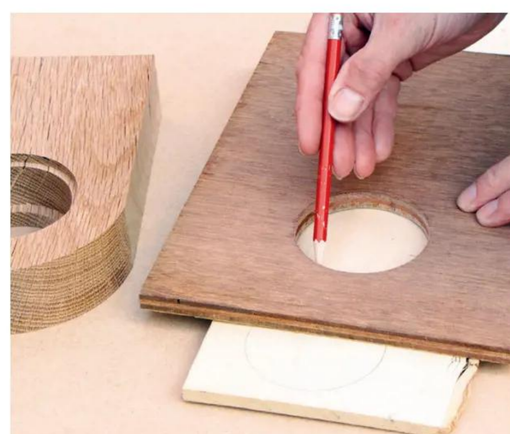
15 Make another template with a cut-out to match the dial diameter, which in this case is 75mm; draw on to the contrasting wood
