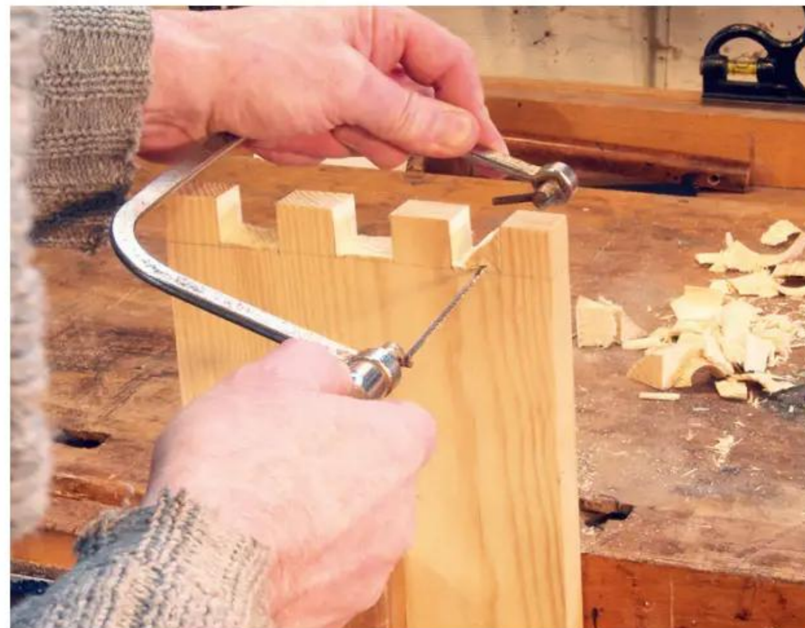
10 Cutting out waste with a coping saw, but you could also use a piercing or fretsaw
