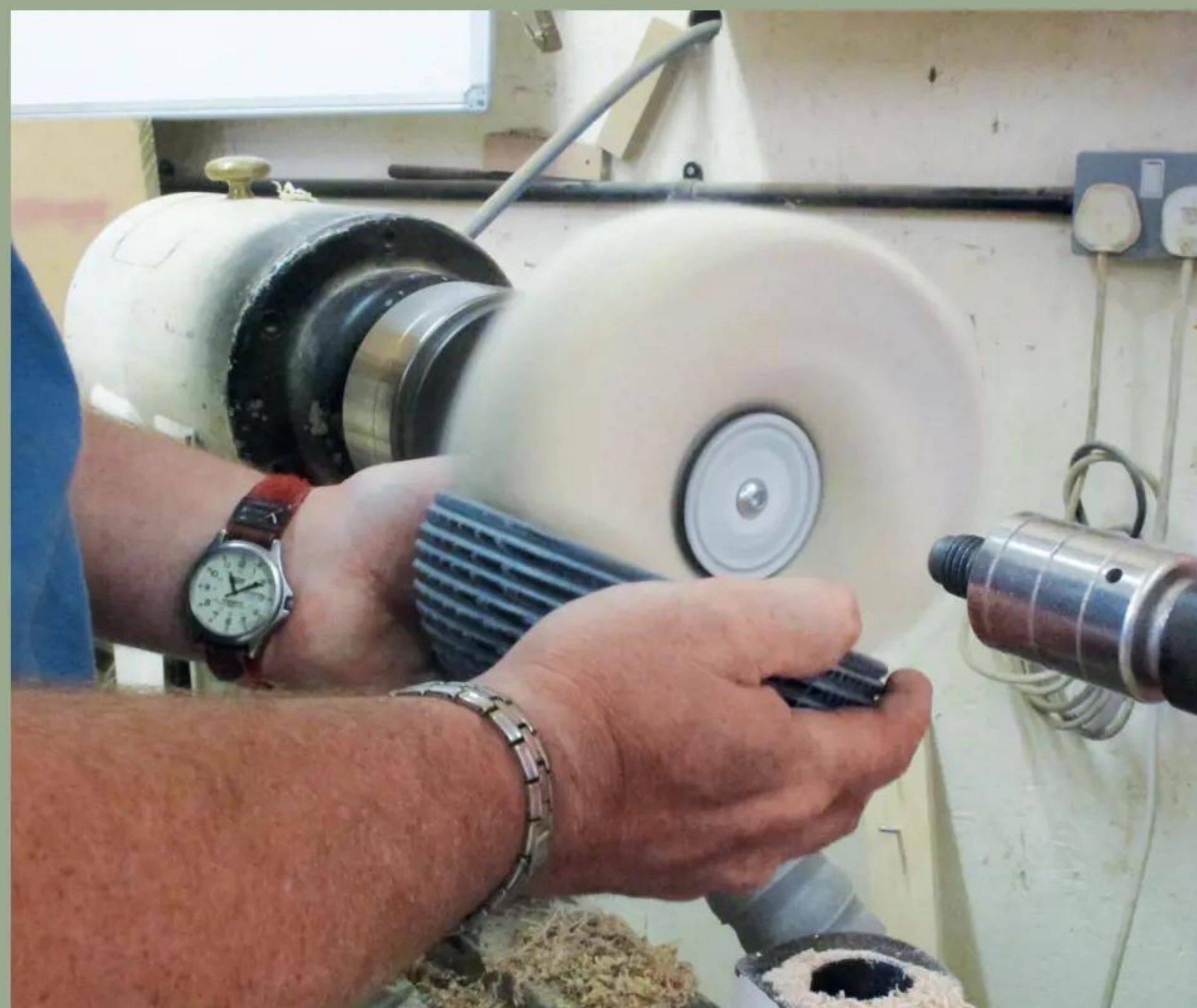
14 ... so slow down the lathe and hold on tight
