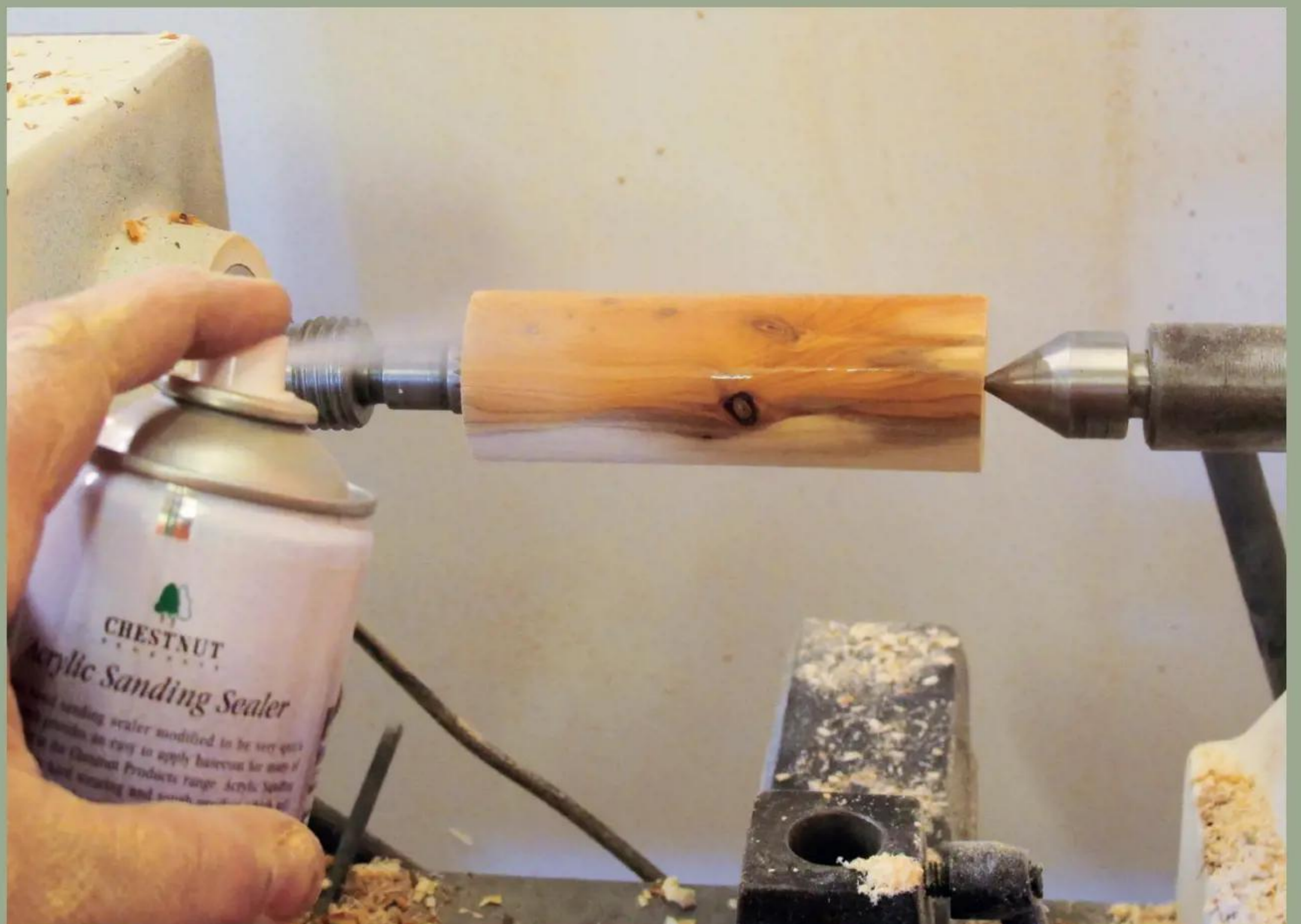
1 I apply the sanding sealer via an aerosol can prior to reaching for the finish
