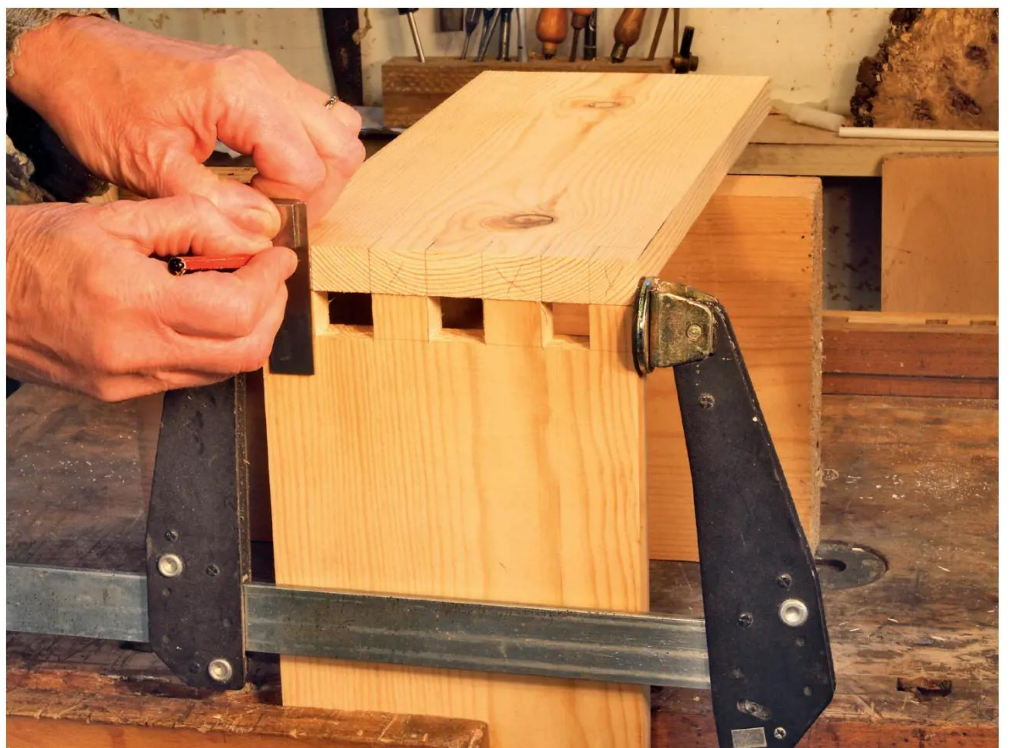
12 Method of transferring marks for the fingers as a practice for dovetails
