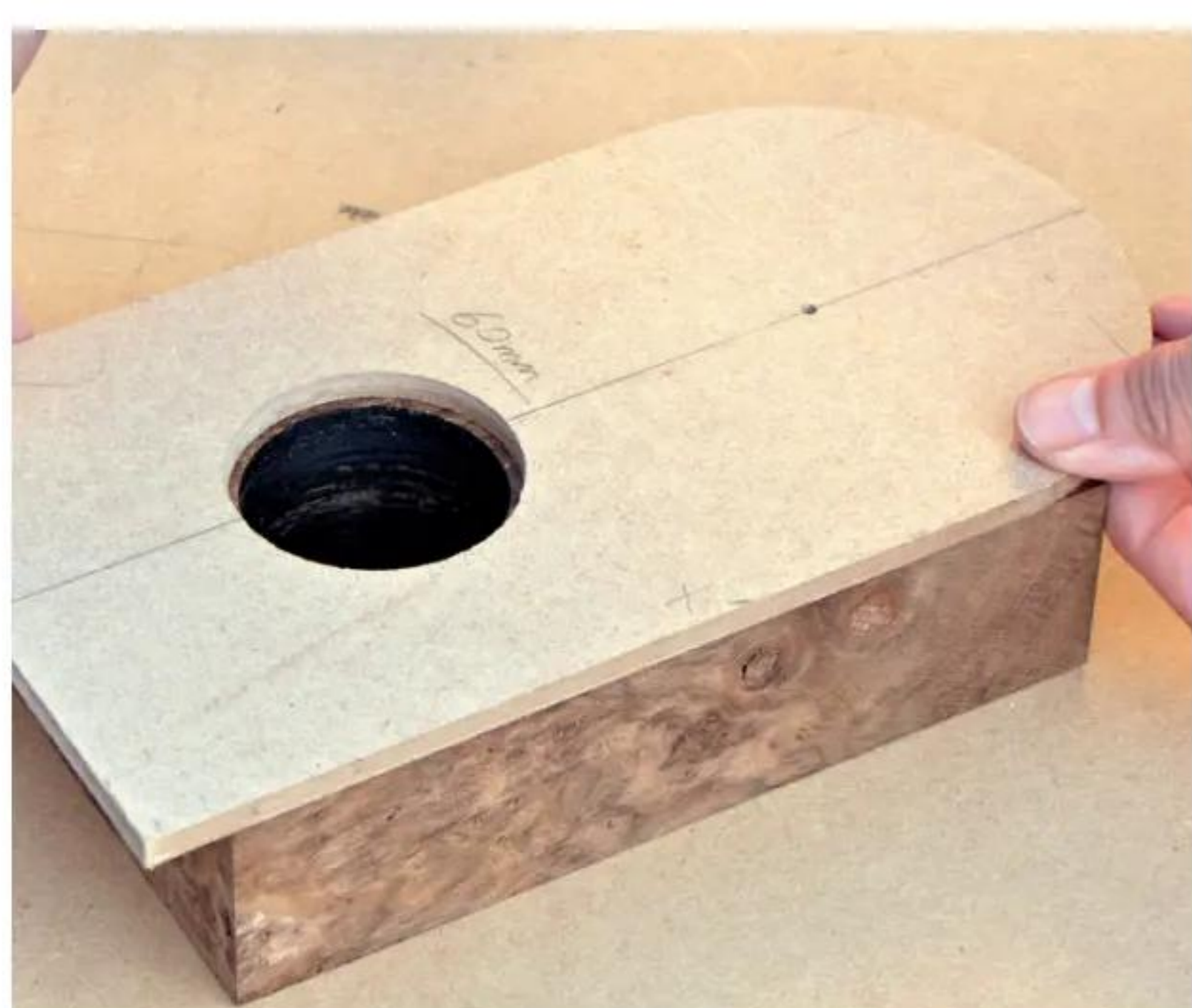
10 Rout a hole in the template with a Dremel tool to suit the clock dial – this is 60mm diameter on both clock designs
