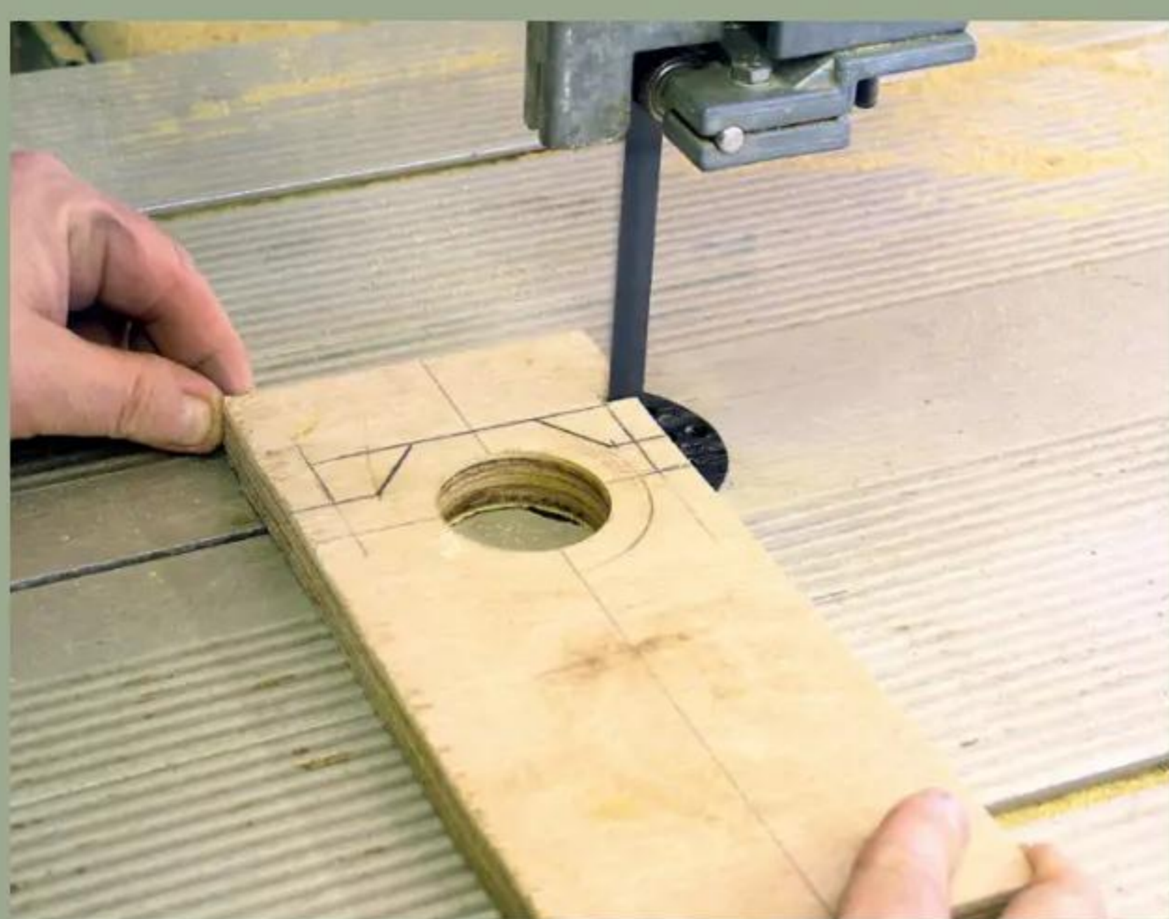
7 Draw the top bracket's shape on the front upright and cut it out
