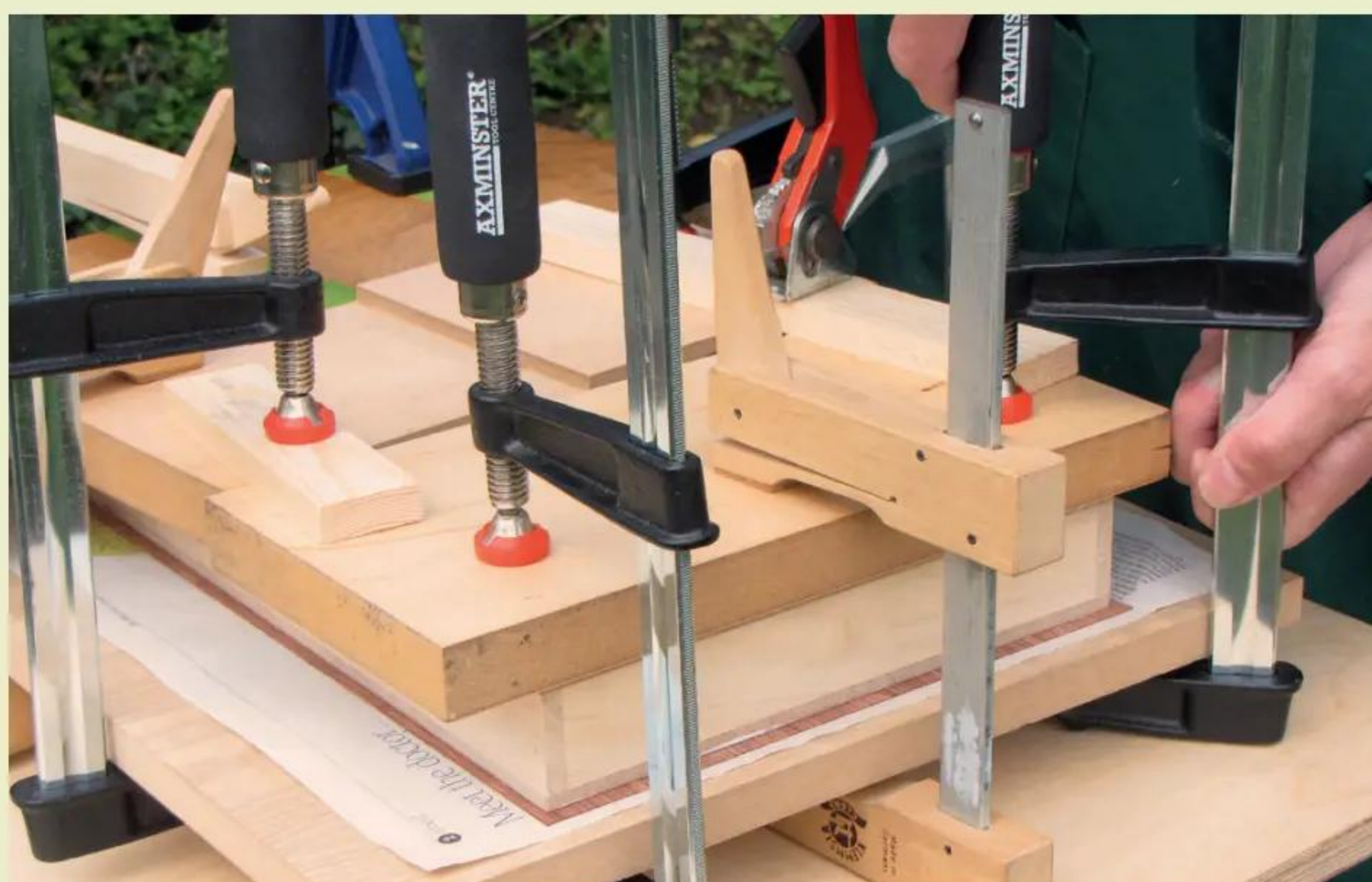
9 With newspaper under the veneer, cramp box to a flat board and leave to dry
