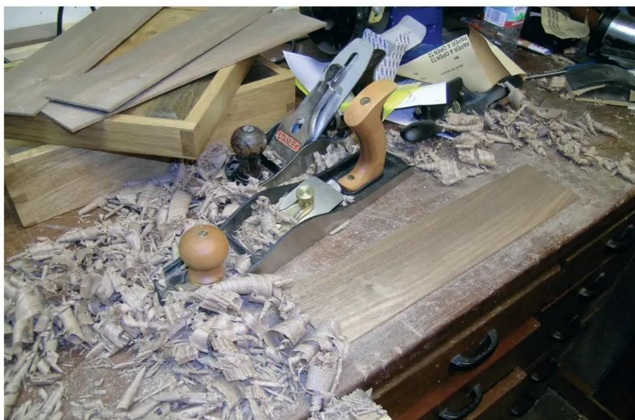
The Lie-Nielsen was the only plane that worked this timber without tear-out
