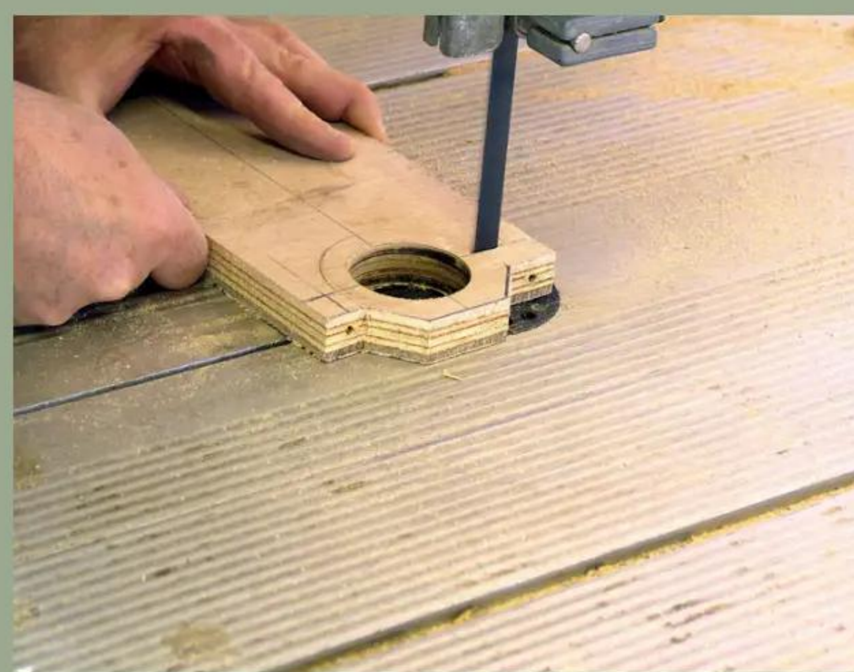
9 Cut across the hole diameter in order to separate bracket from upright
