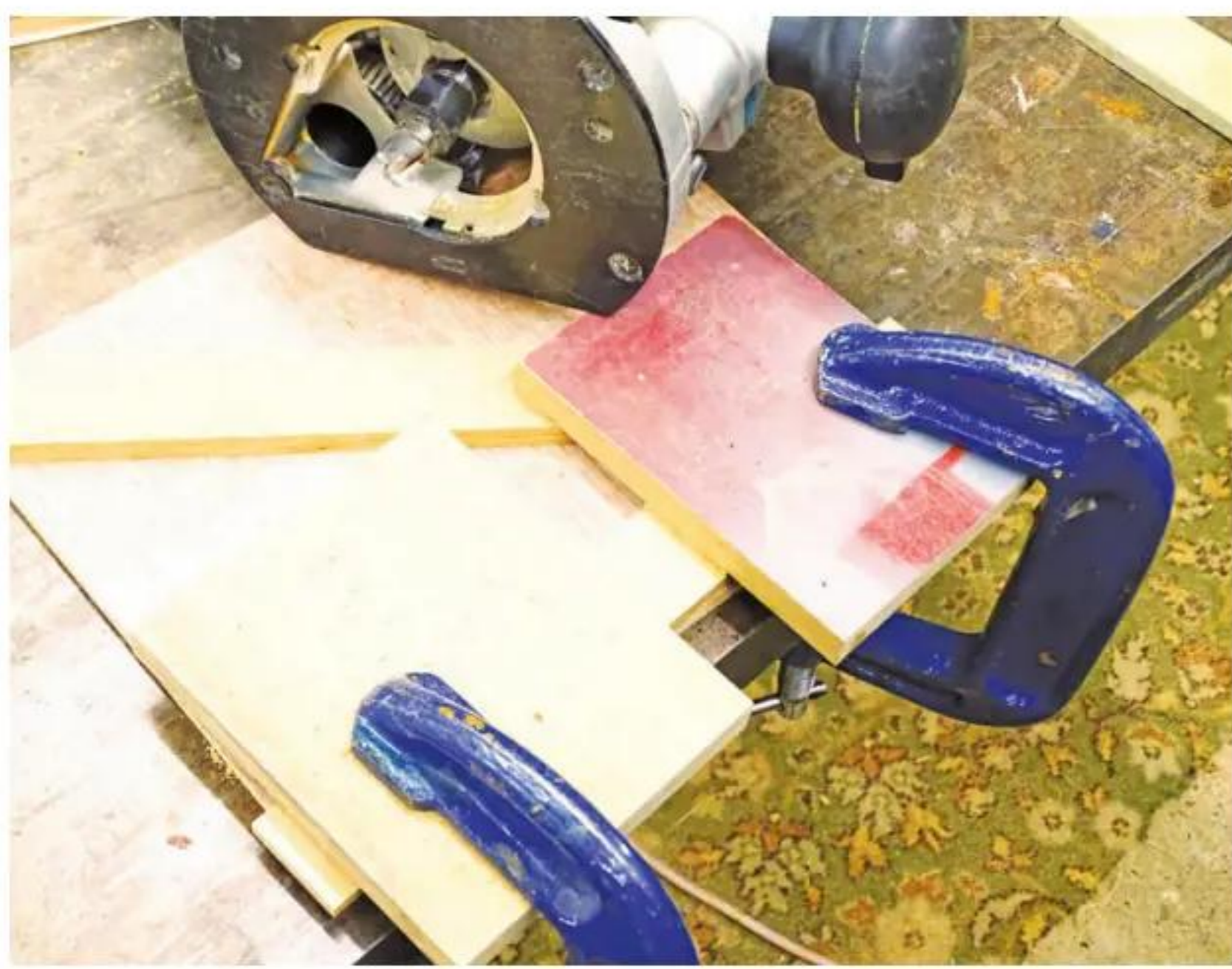
10 Carefully set the depth of cut
