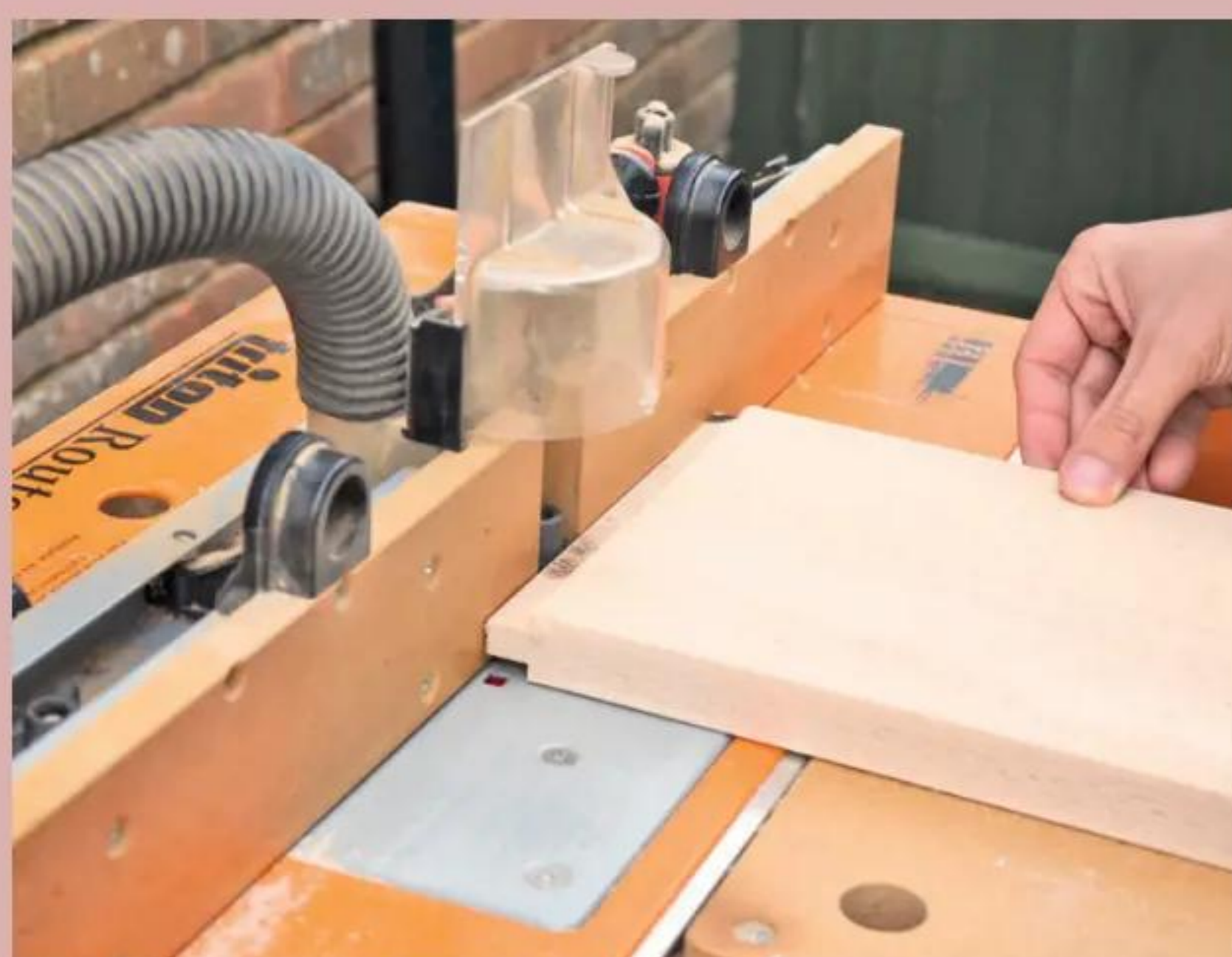
5 The tenon on one end of the board is almost complete; remember to keep the board pressed tightly to the fence and flat on the router table
