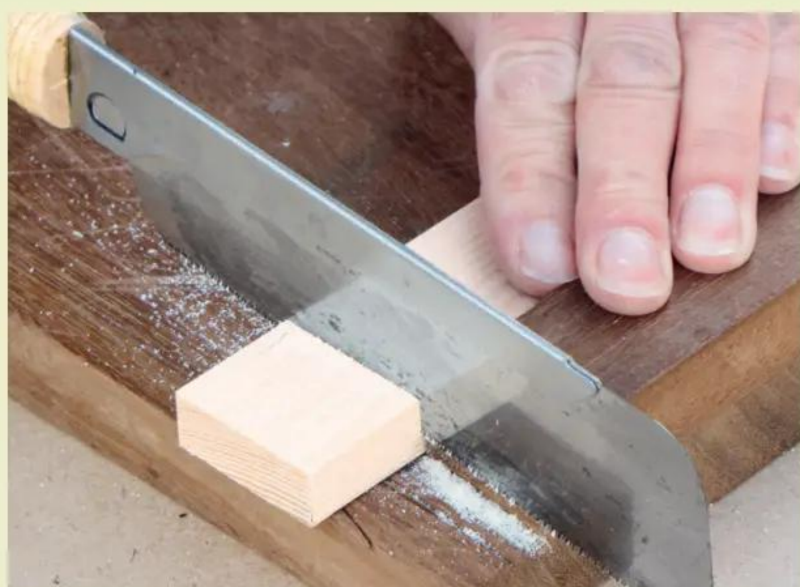
3 Measure accurately and saw cross-pieces so they're a perfect fit between longer rails
