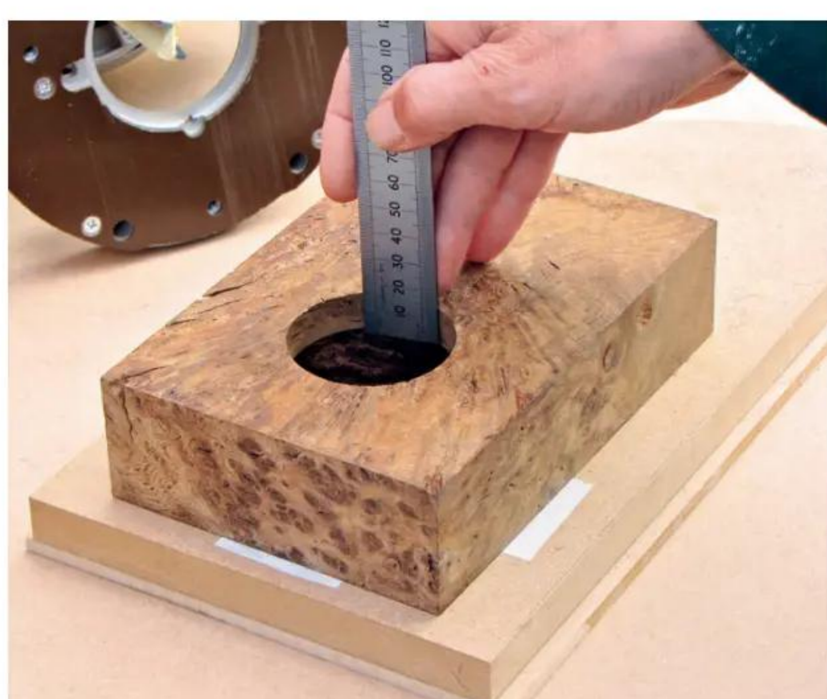
13 Check the front hole's depth is sufficient for the clock spindle and hands; quartz movements are available in three sizes
