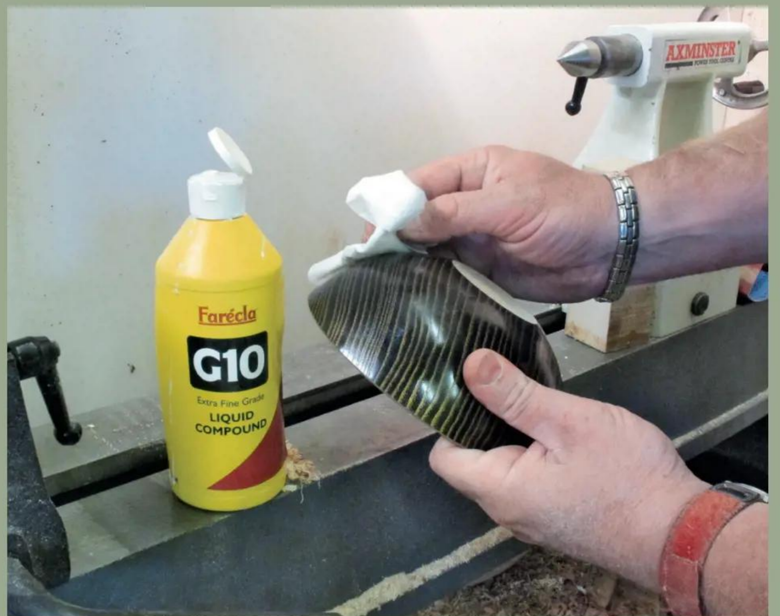
9 It's best to cut back with paste to ensure optimum results
