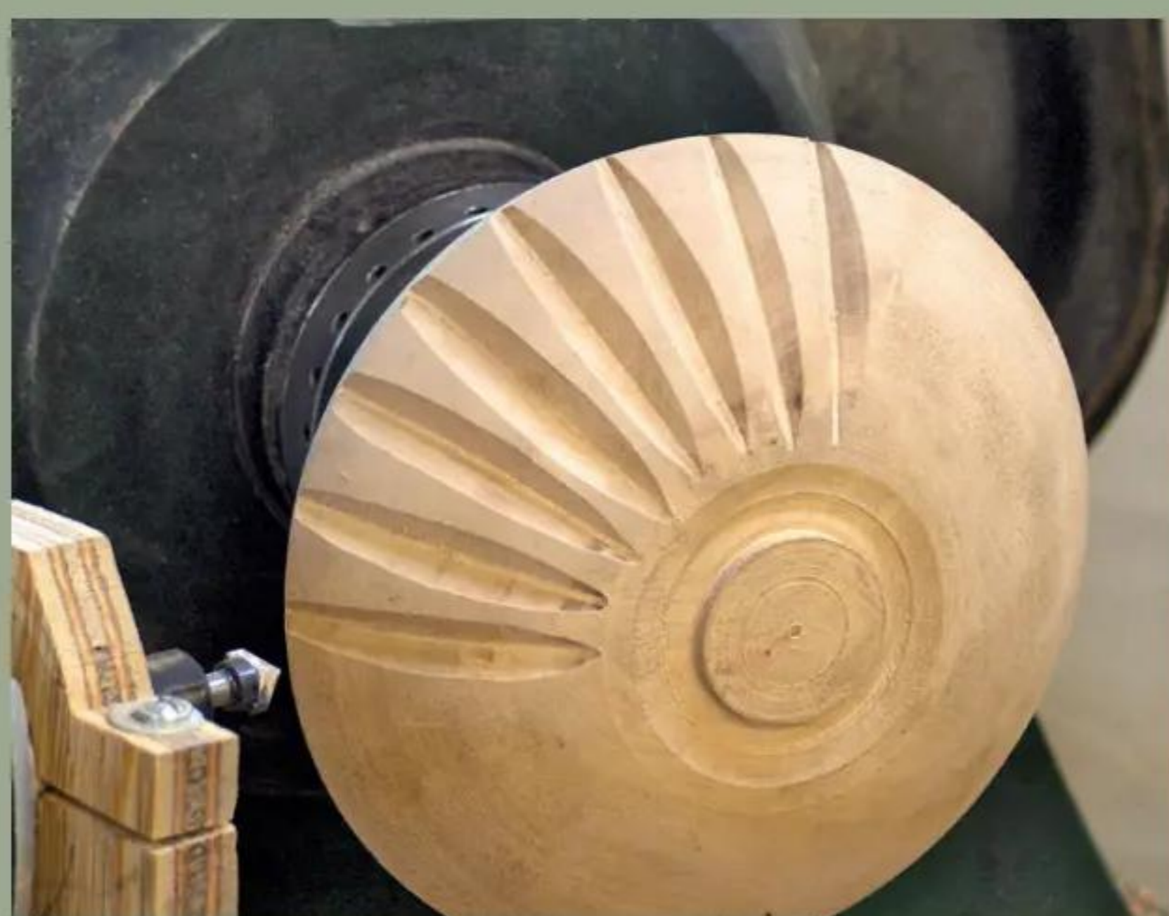
14 If using a different-shaped template, you can create tapered grooves
