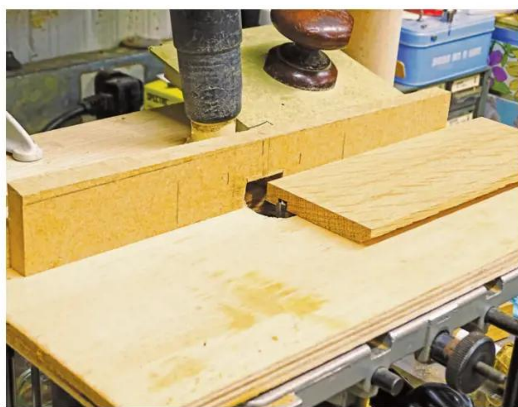
2 Next, cut a rebate along the lower edge to suit the plywood
