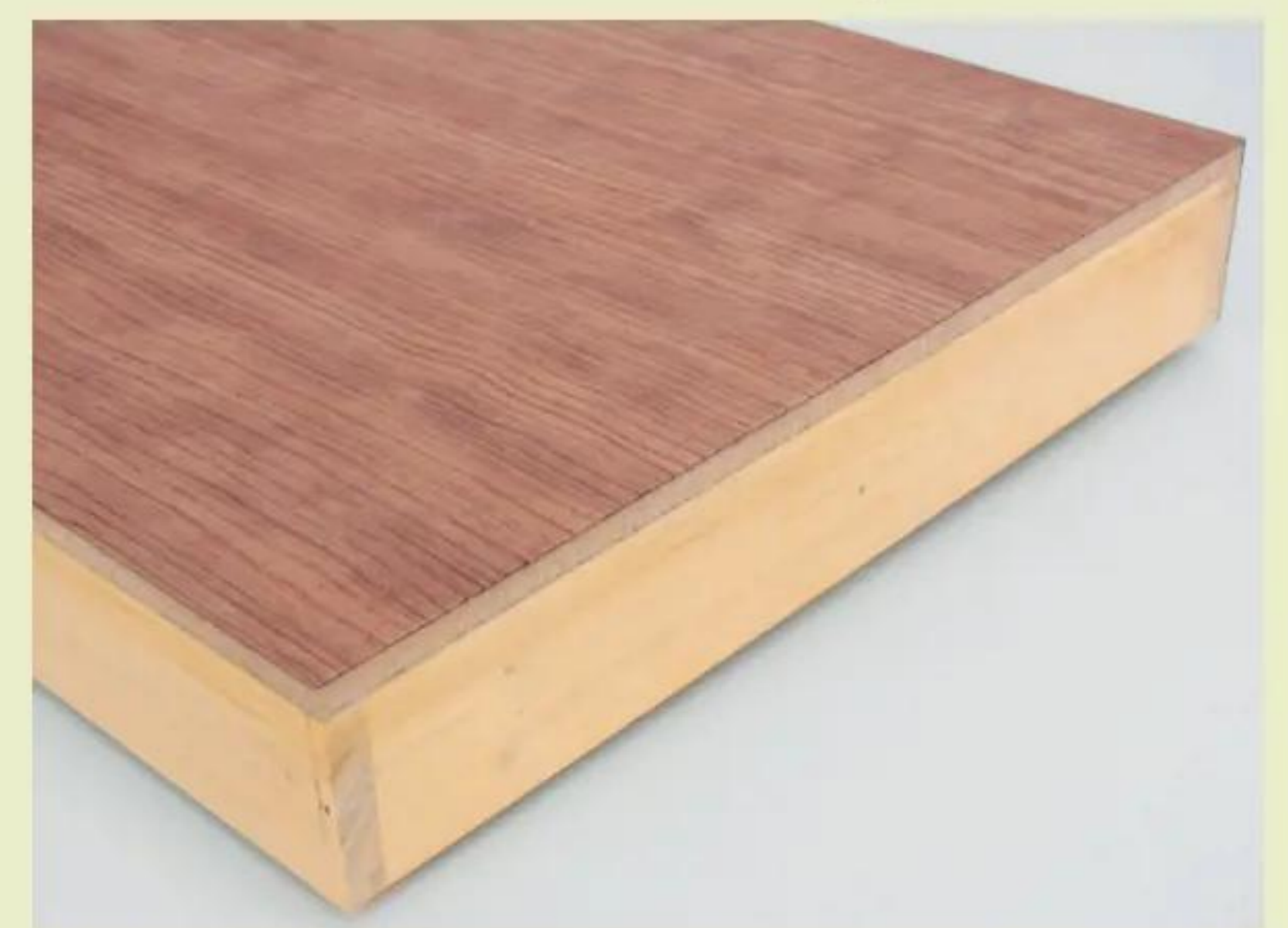
Despite the lightweight construction, torsion boxes are remarkably strong and durable
