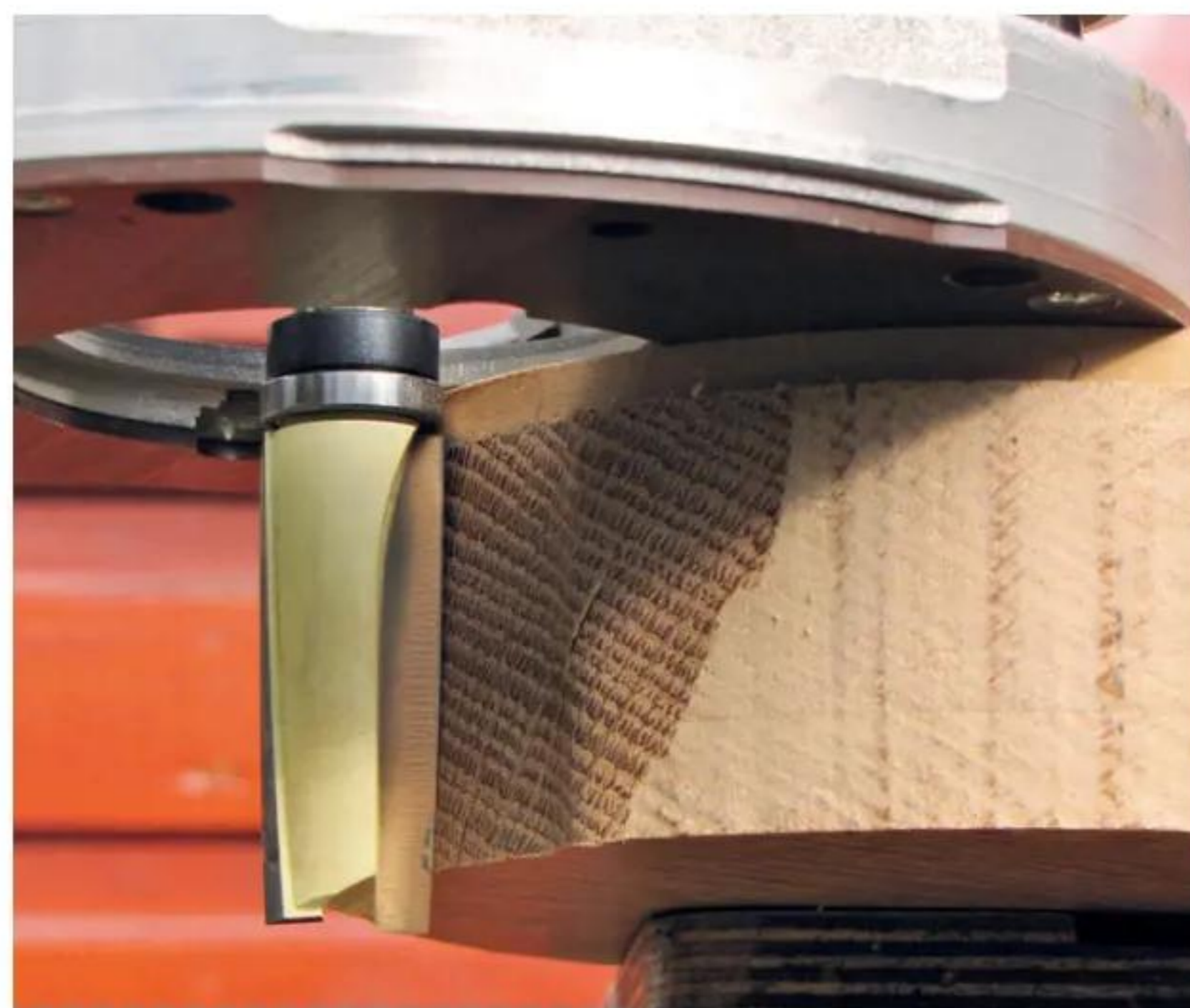
8 Secure timber to the bench, then using a router, carefully follow the template using a bearing-guided flush-trim cutter
