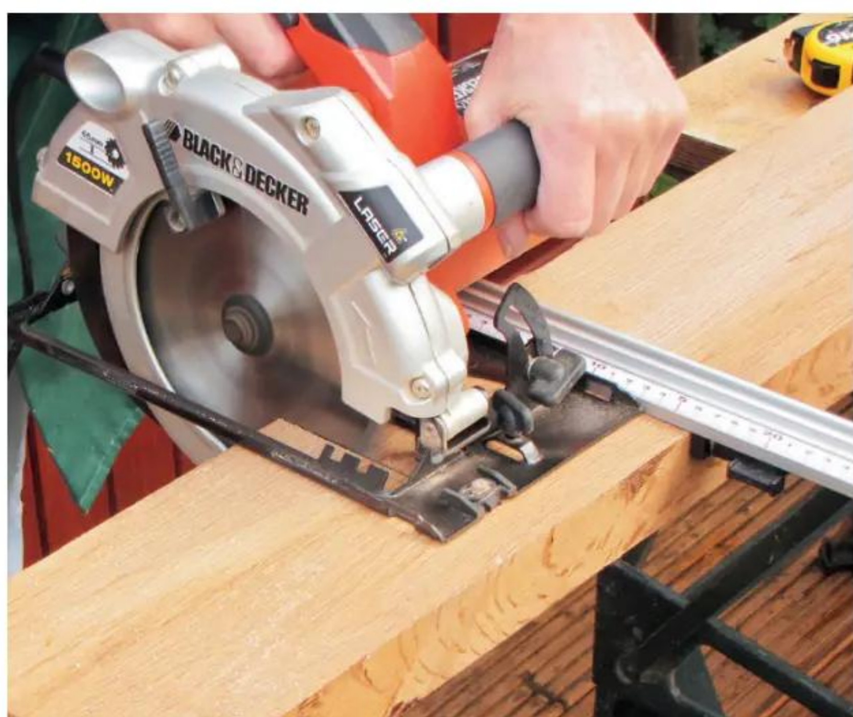
1 Thickness timber to around 50mm, then saw to length; overall clock blank size isn't too important
