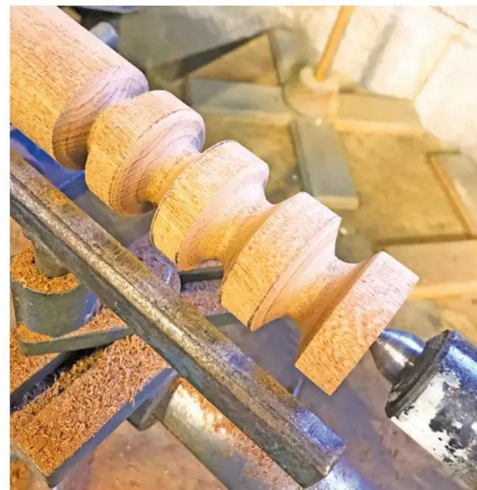
17 The four bun feet were turned from one length of sapele
