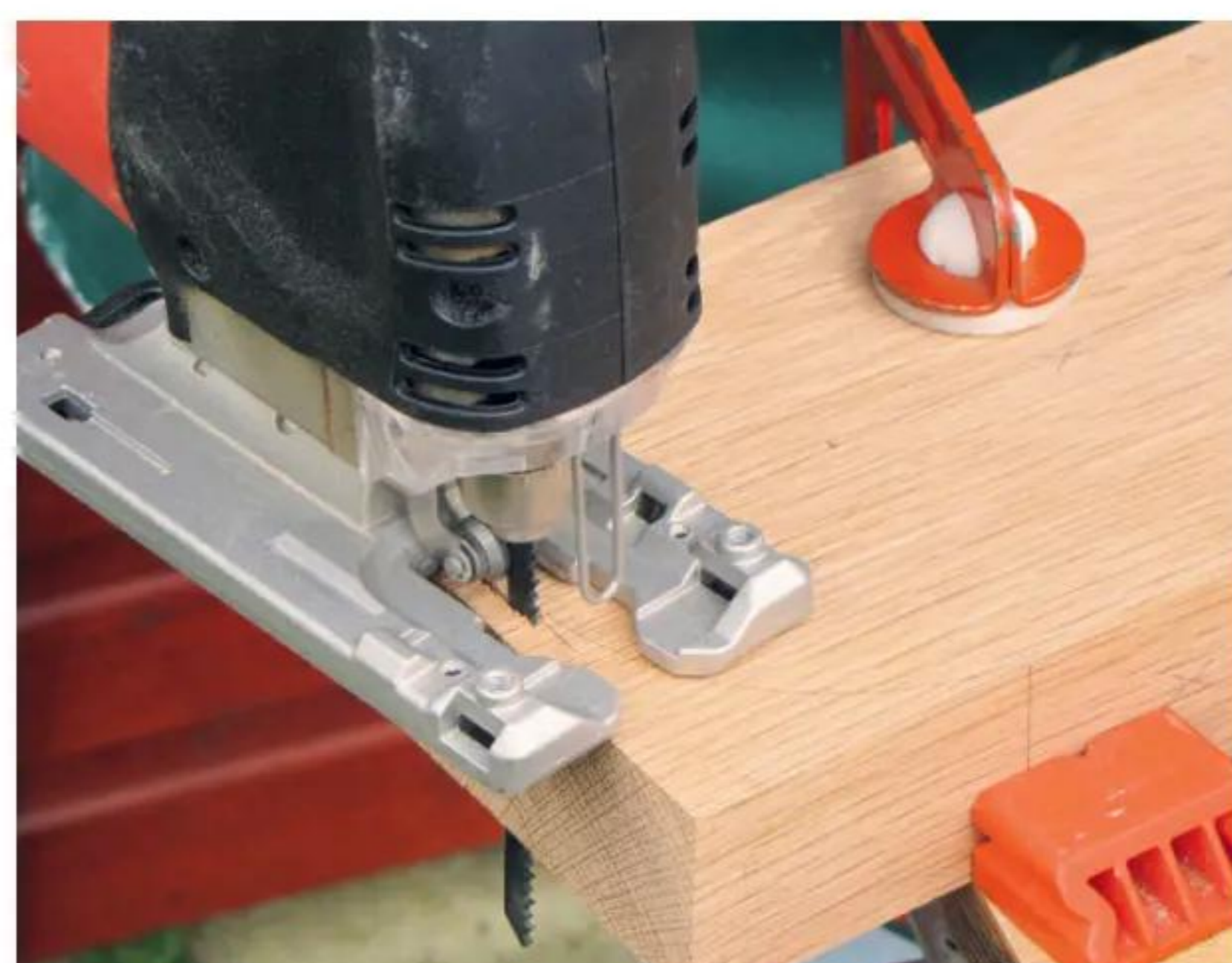
5 Draw around the template and onto the blank; cut with a jigsaw or bandsaw, keeping to within 3mm of the pencil line
