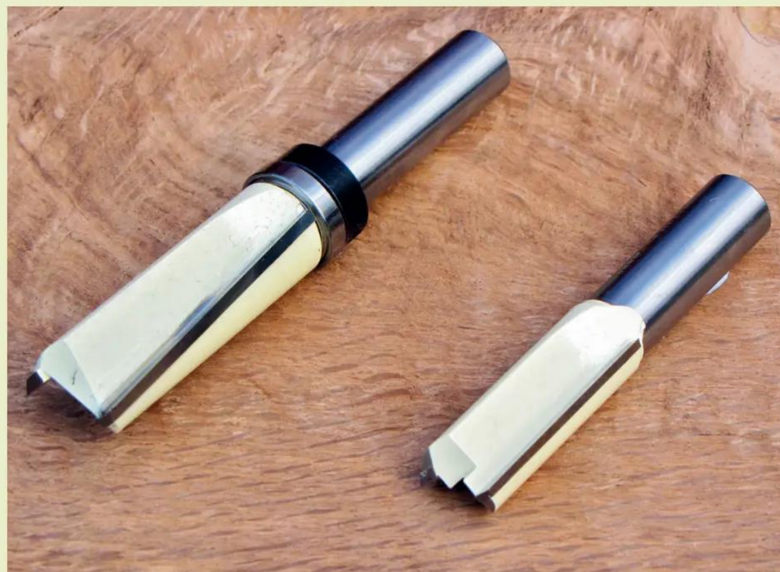
I removed waste with an Axcalibur 16mm twin-flute bit
