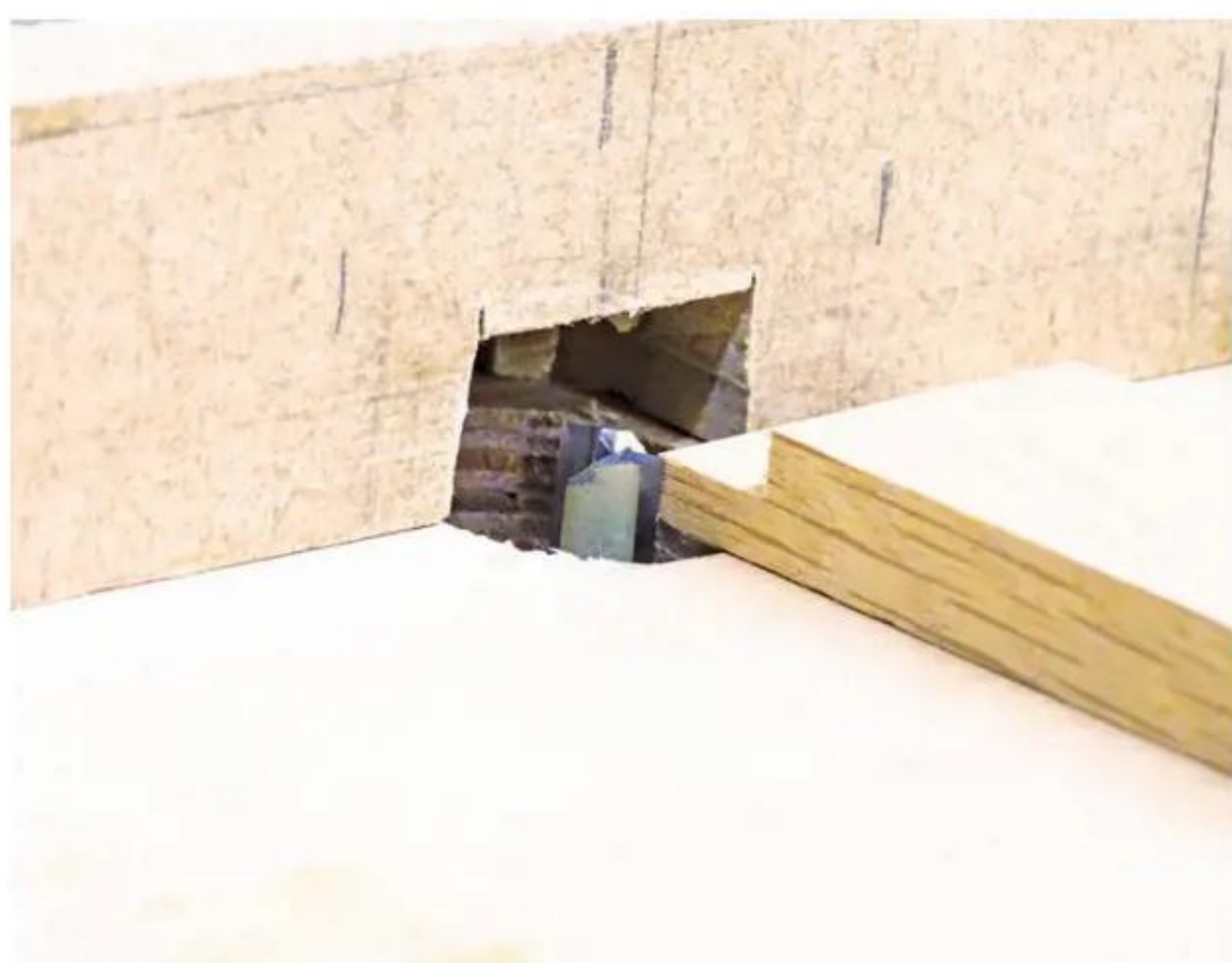
7 Using the rail as a guide to set depth of cut
