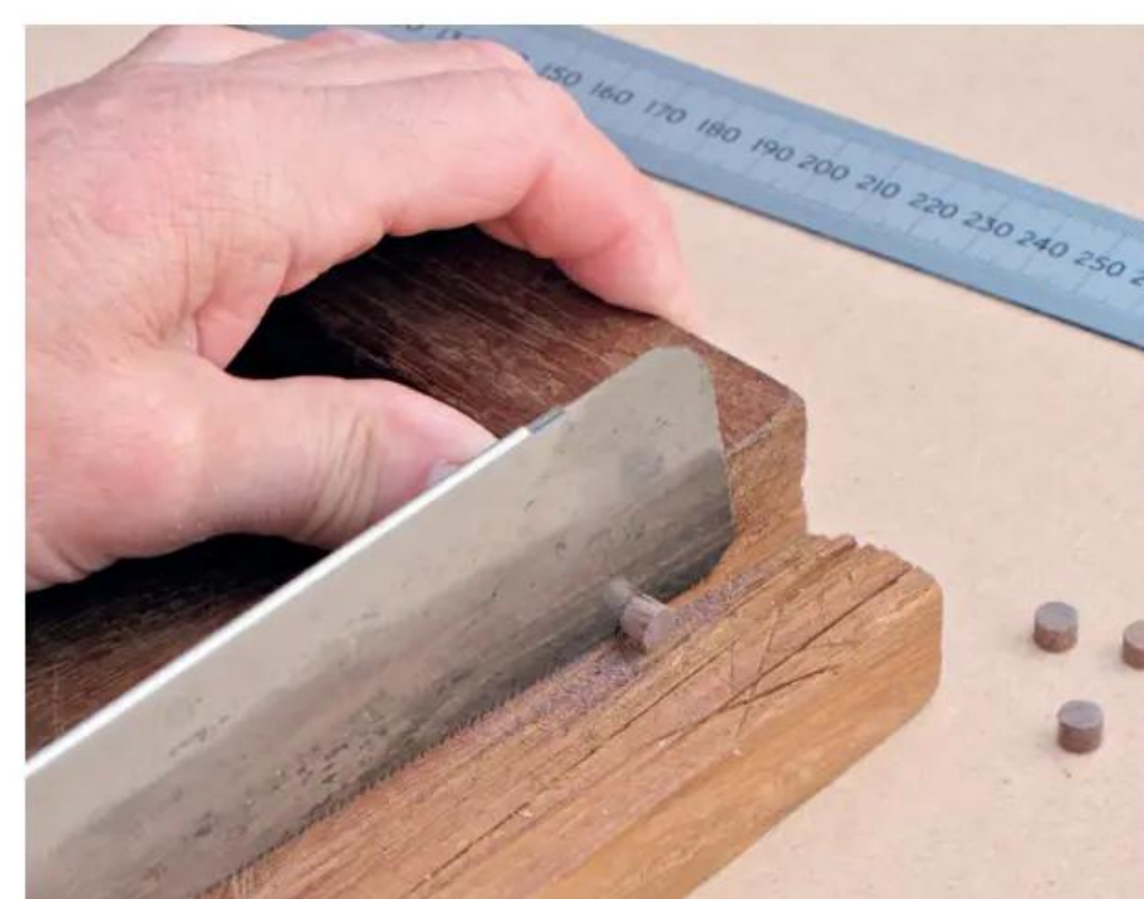
18 Saw dots to around 6mm with a fine-tooth saw; sand ends lightly to remove any whiskers
