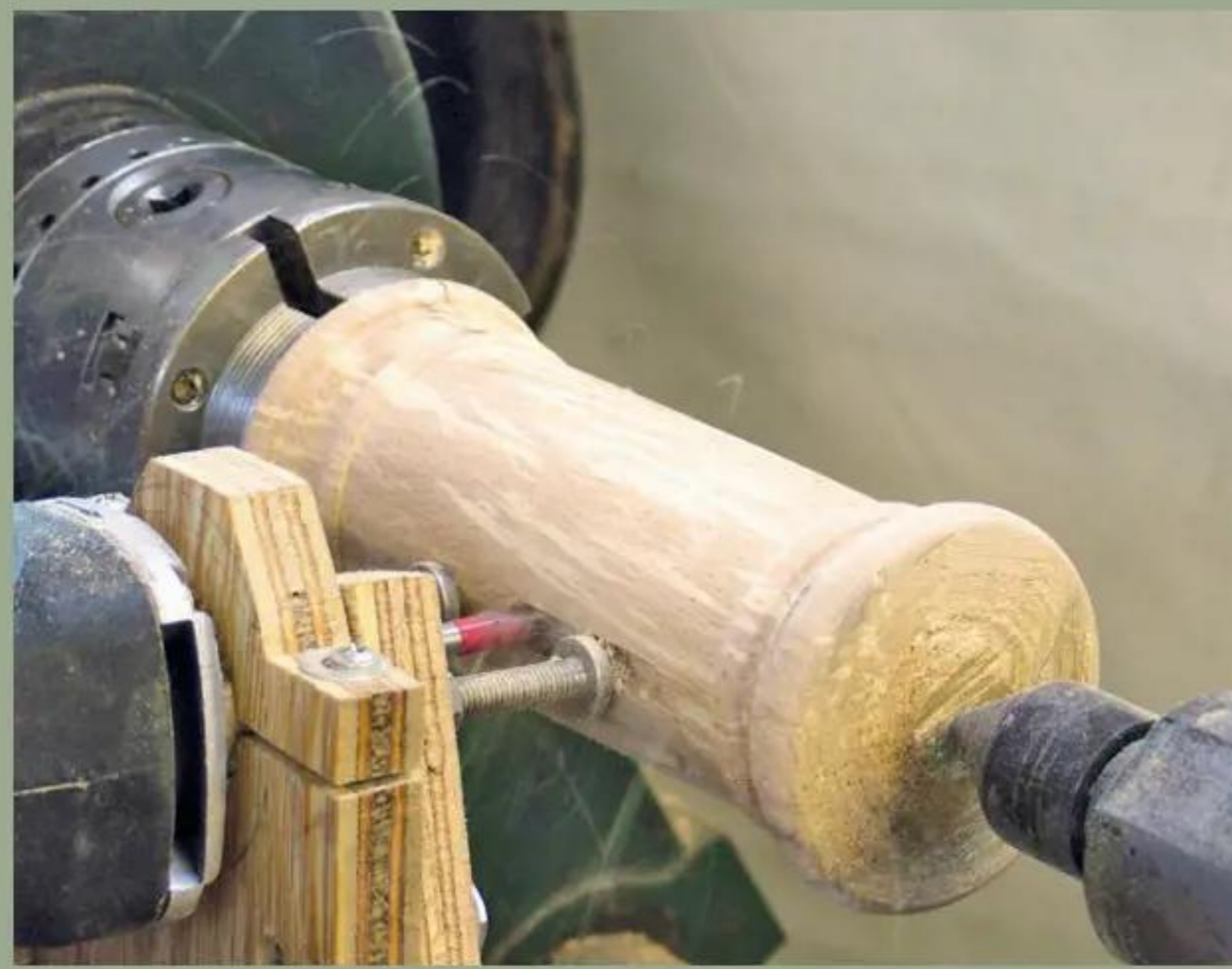
17 The completed cradle runs along the workpiece's centre...
