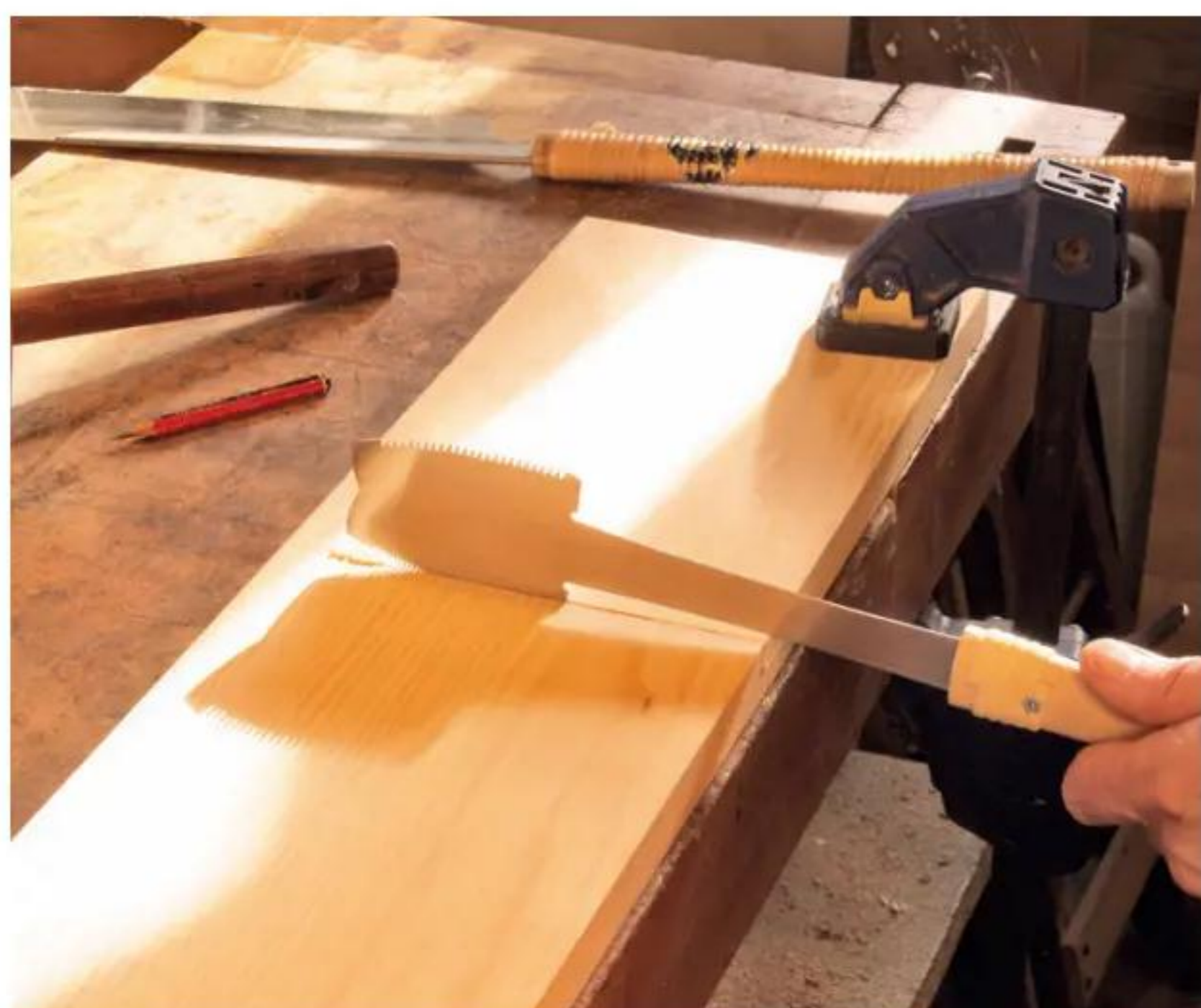
6 Cutting a stopped housing with an azebiki
