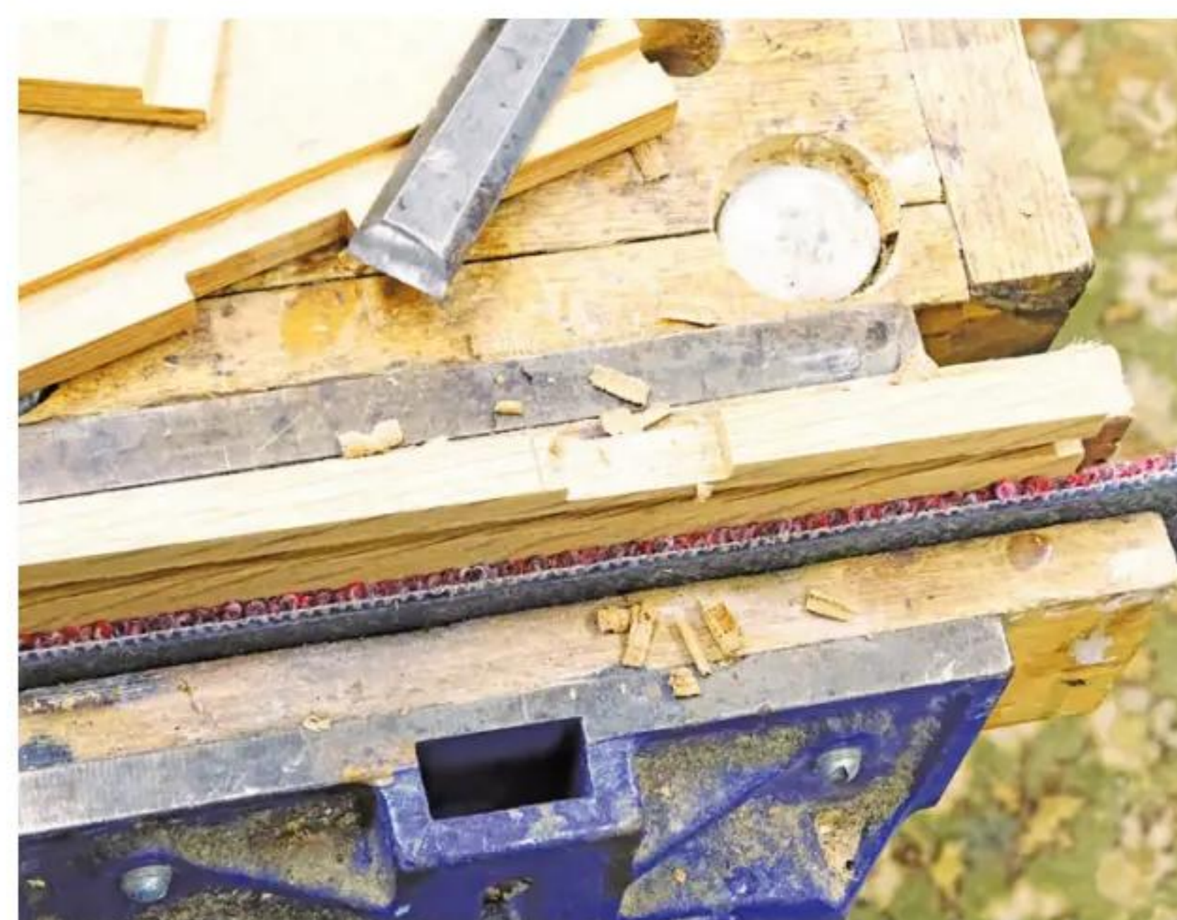
9 Square the end of the cut with a sharp chisel
