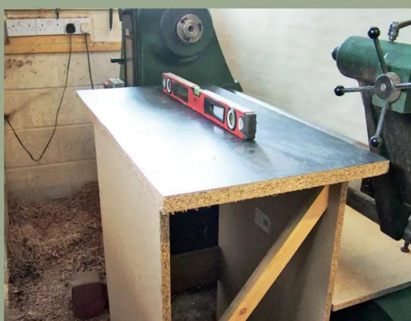
4 A floor-standing platform such as this is a better bet for non-standard lathes
