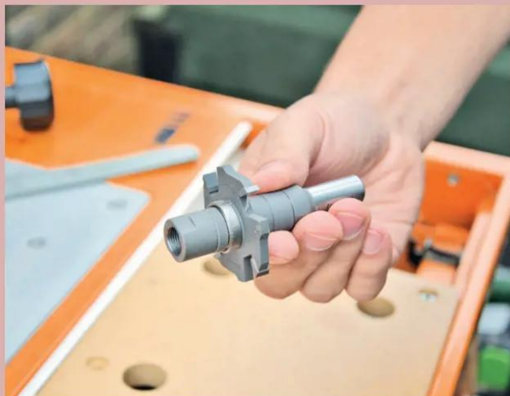
2 A slot cutter is perfect for making breadboard ends; this robust version from Trend features a good long shank, which is ideal for router table use
