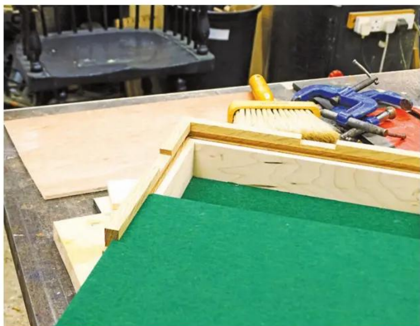
21 Slide the plywood base into place
