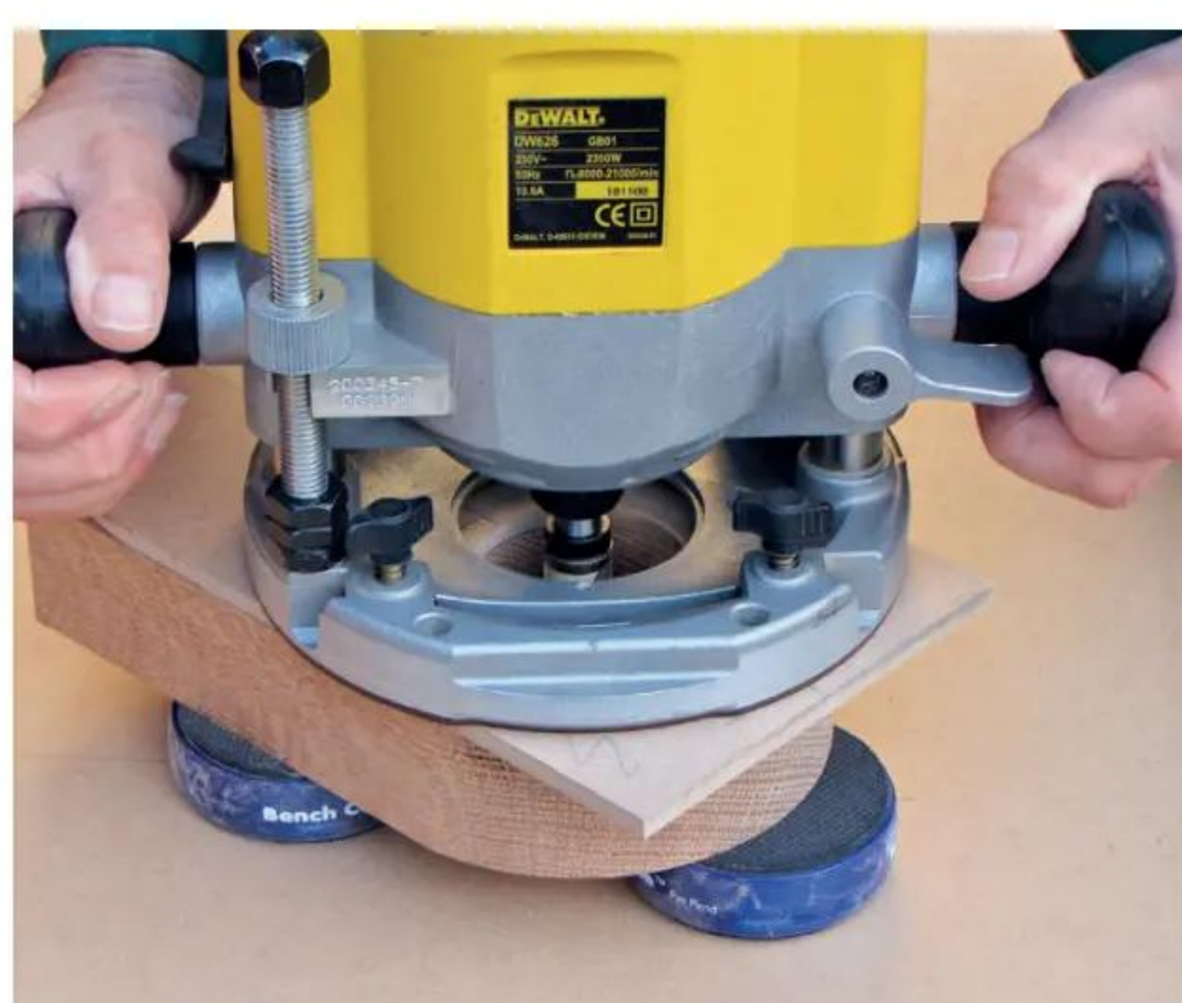
11 Carefully position the template on the blank's front; rout around the inside at full depth using a flush-trim cutter
