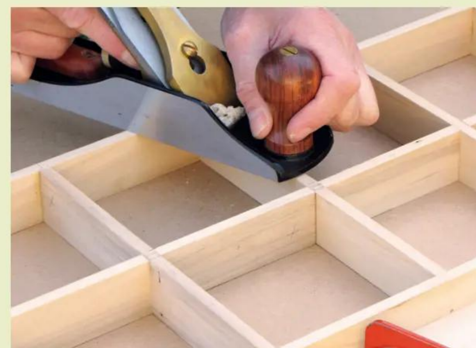
5 When the glue has dried, carefully plane the framework edges flush if required
