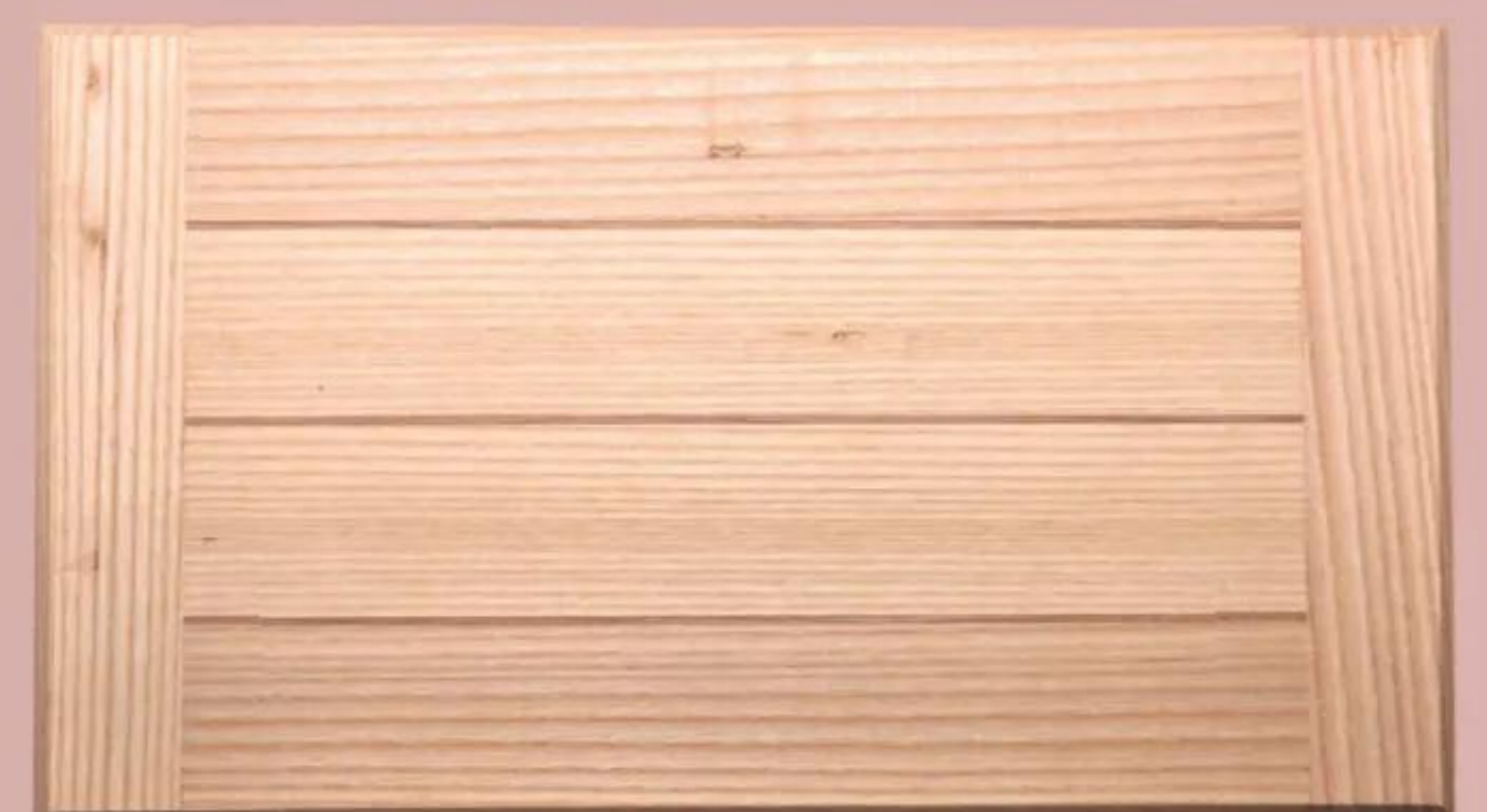
1 Breadboard ends are a traditional construction that reinforce the ends and make the end-grain less likely to be penetrated by water
