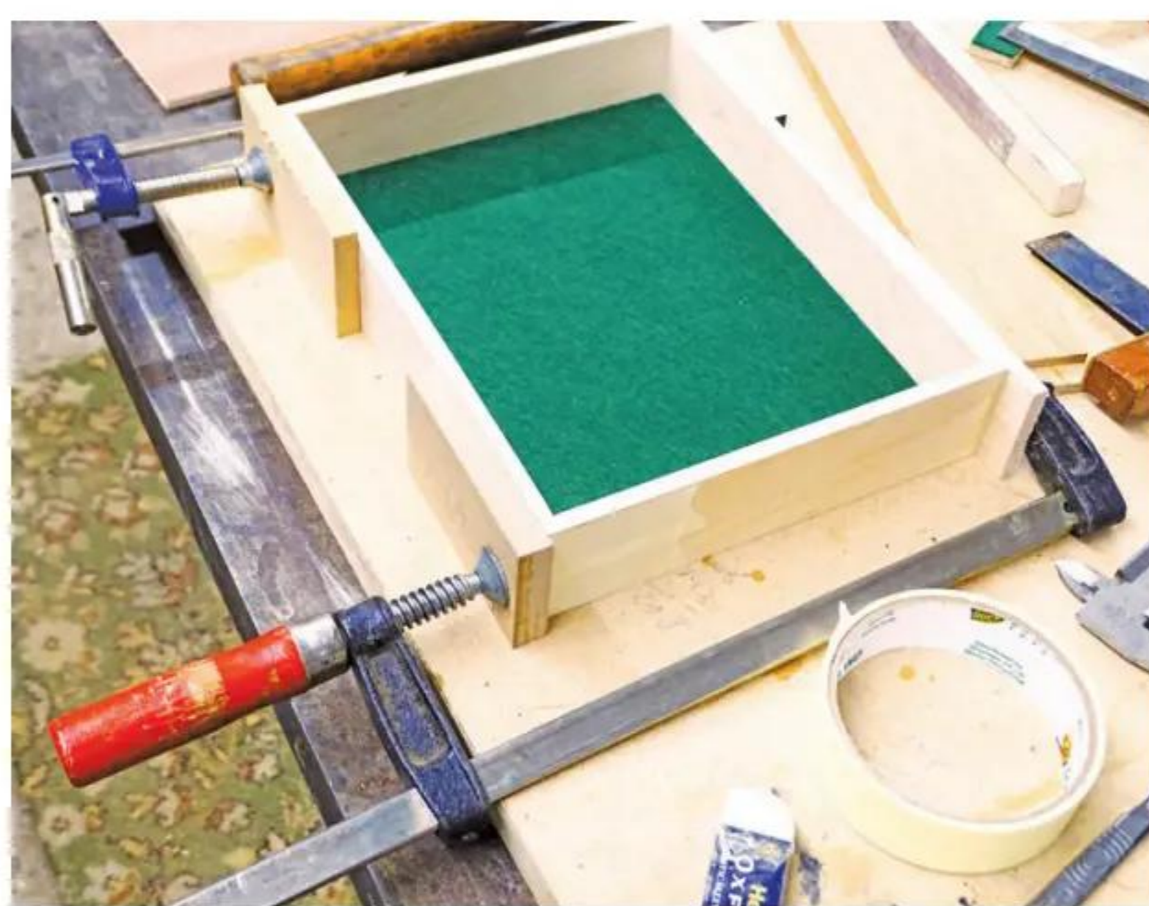
19 Note the use of softeners to protect the drawer
