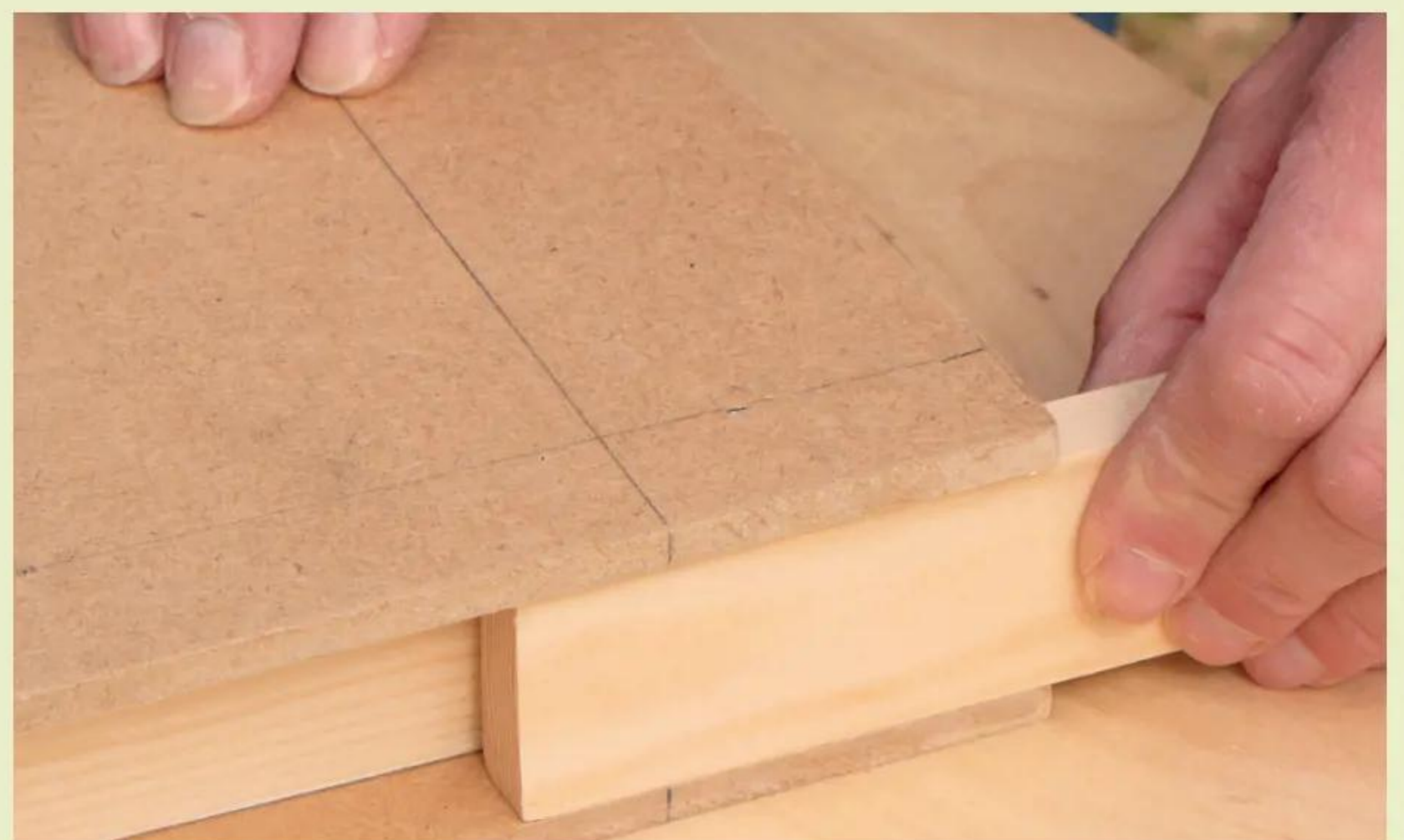
12 Ensure the support battens will slide inside the box's ends
