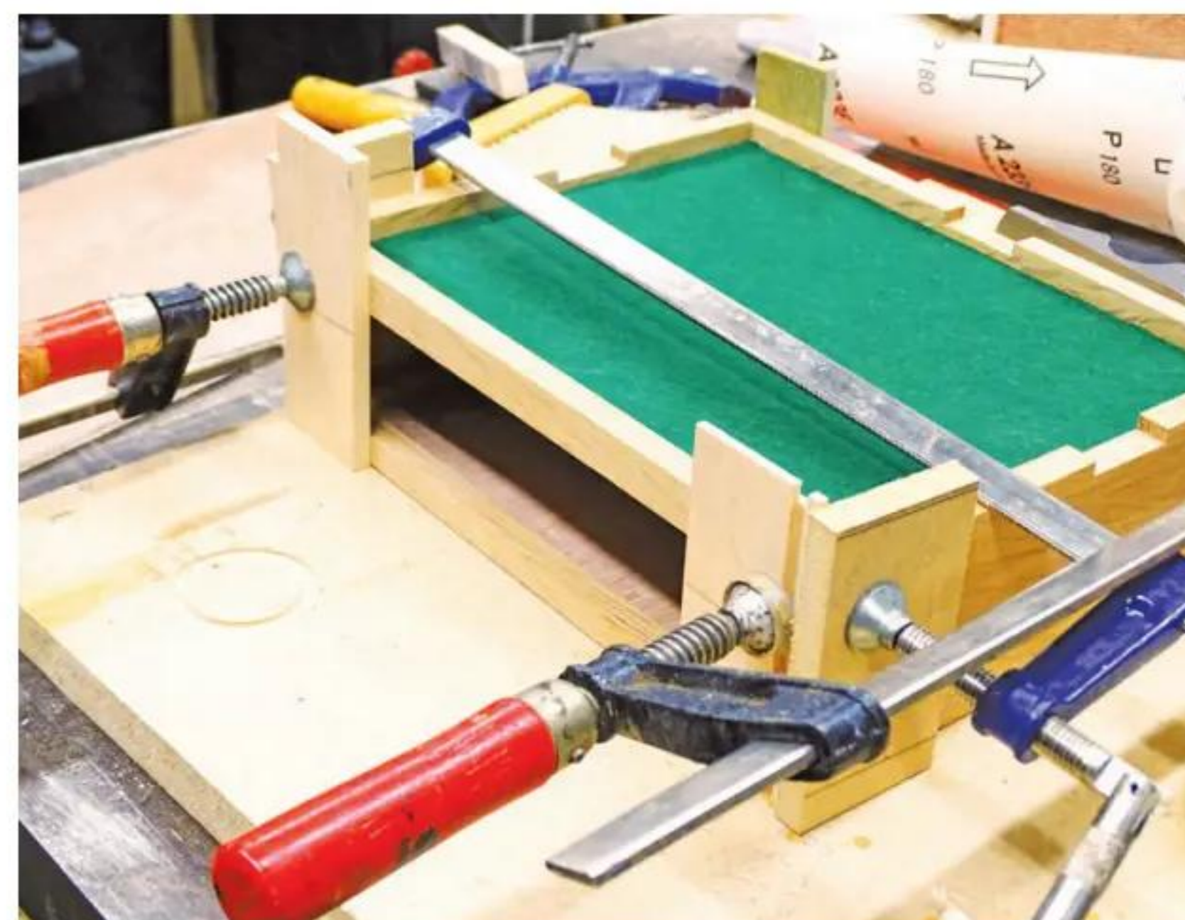
22 Clamp the upper rail into position
