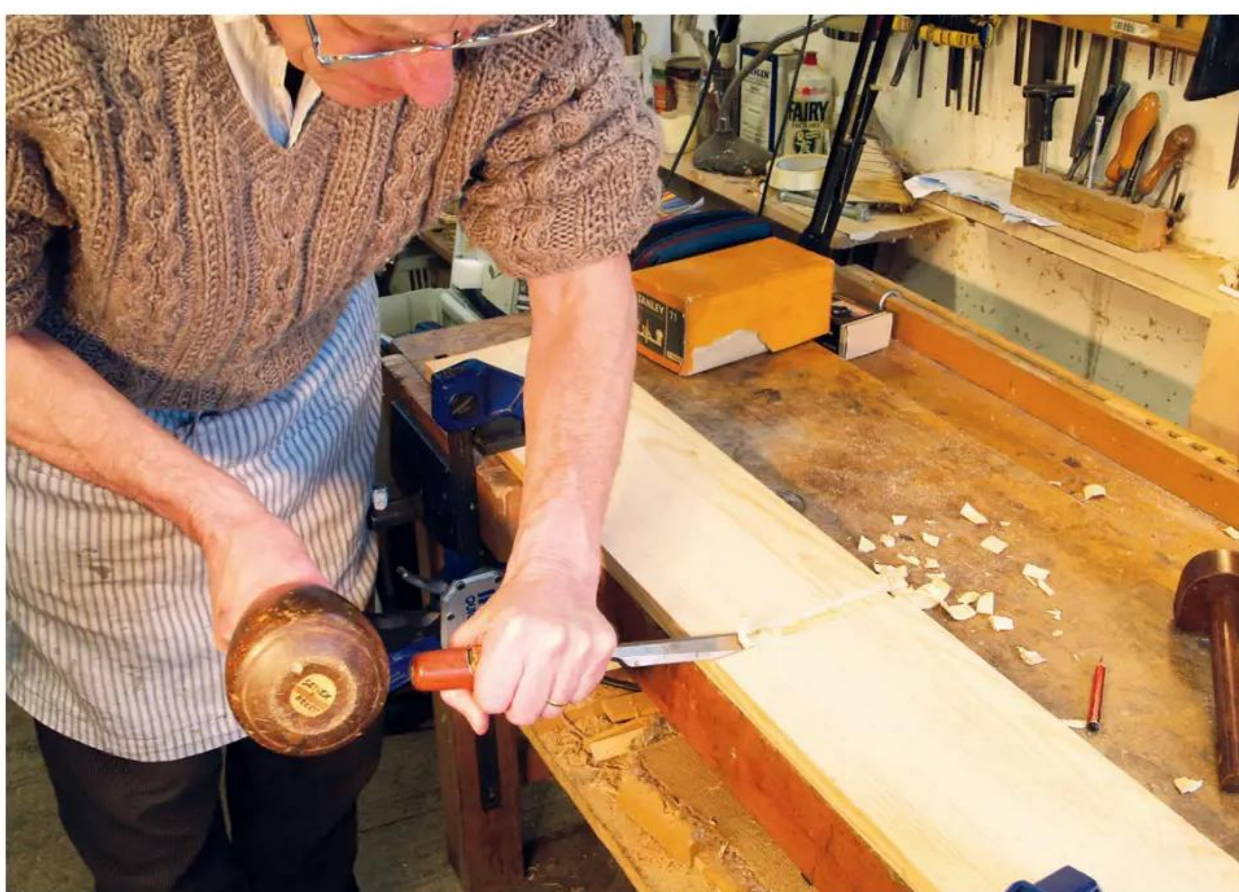
4 Coming back in from the other side to avoid breakout
