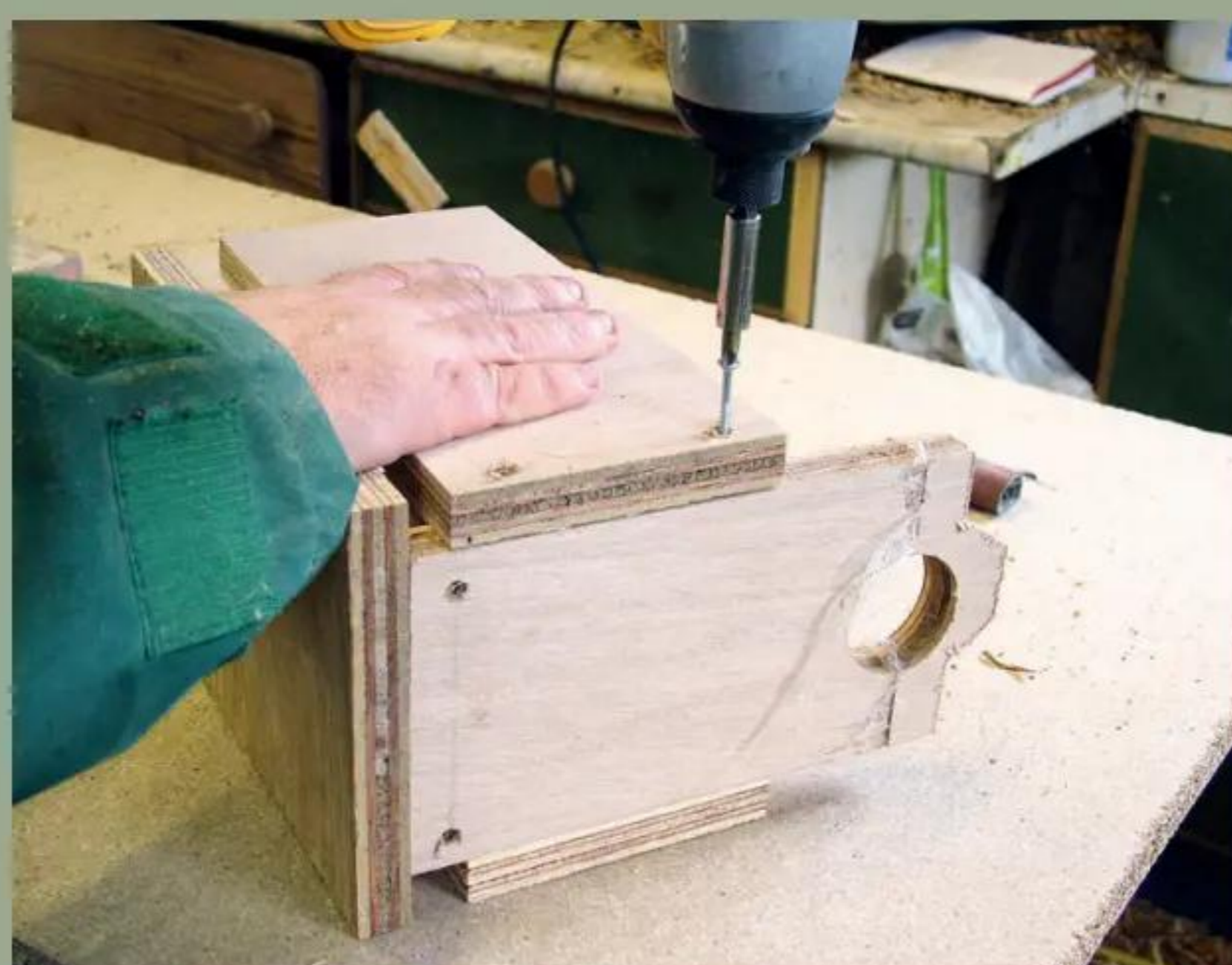
11 Make up the remaining cradle from 18mm plywood, glued and screwed together
