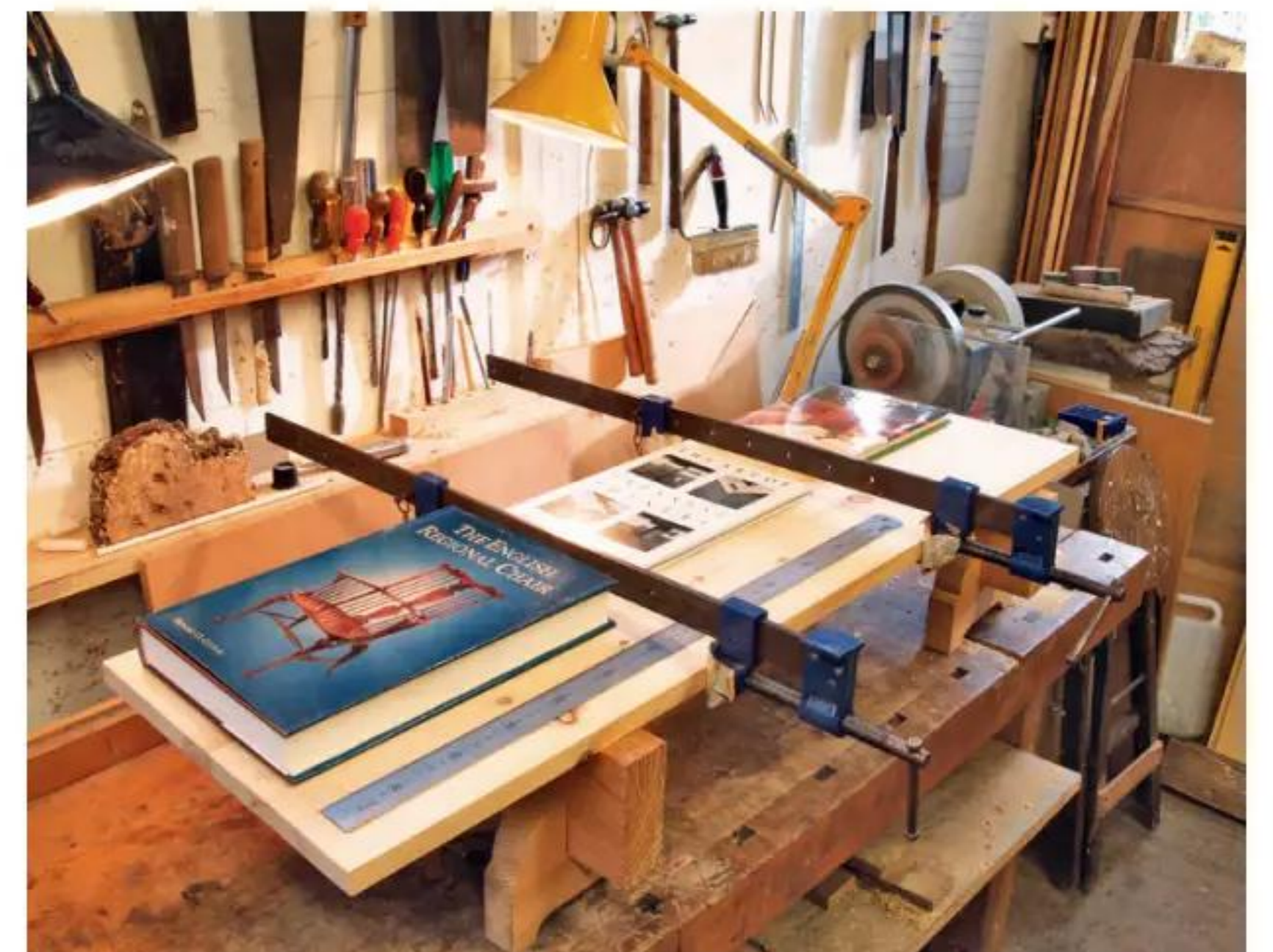
1 Laying out the shelf spacing
