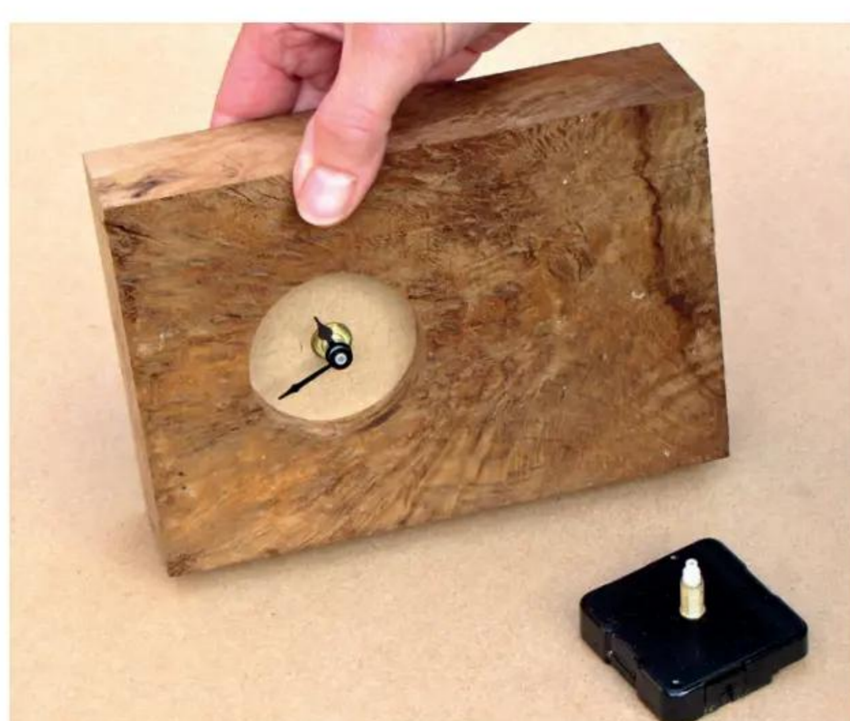
14 Cut a test dial from 6mm MDF and drill an 8mm hole for the spindle; fit the retaining nut and hands to check clearance
