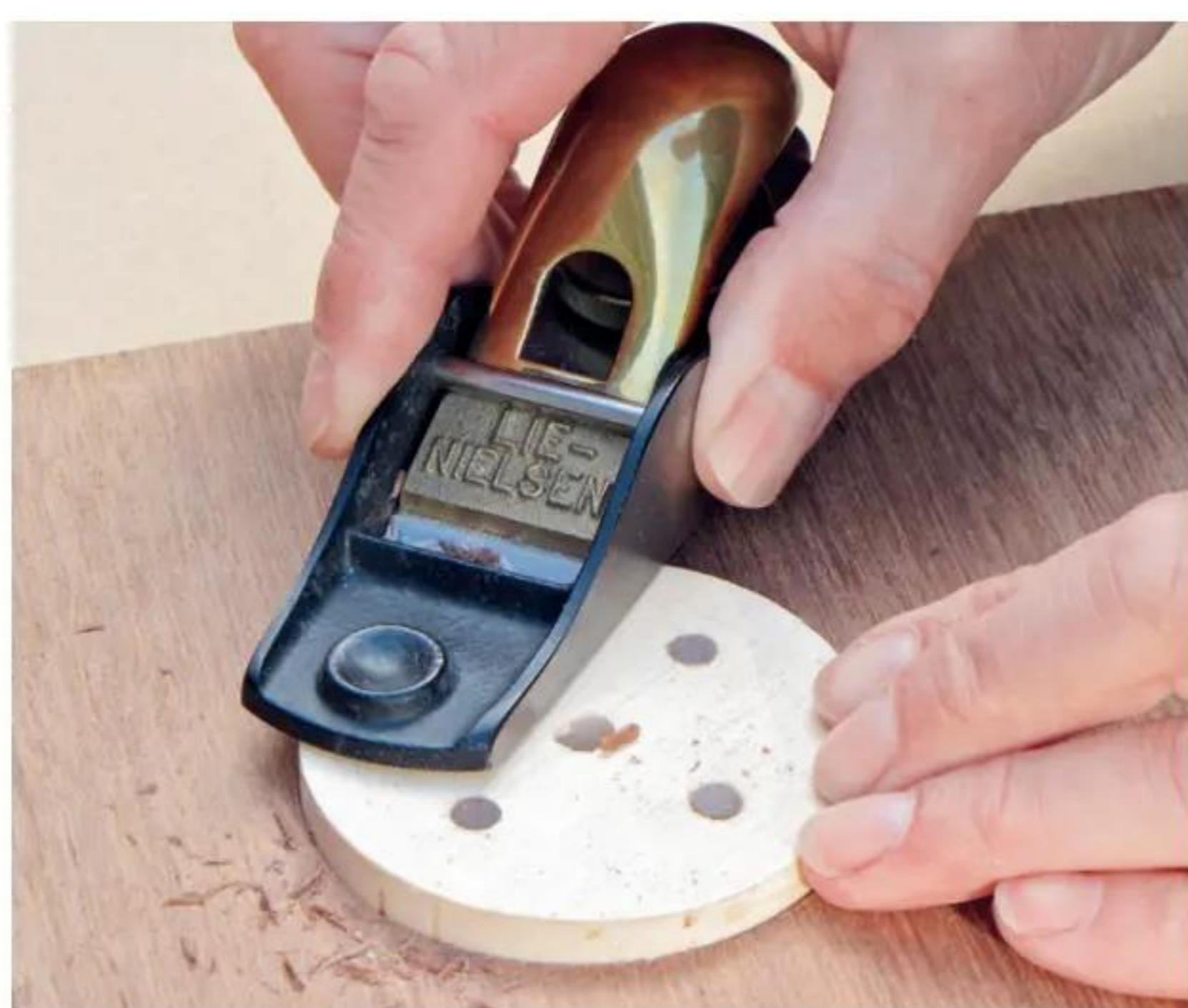
20 Once dry, trim away excess with a block plane; sand the dial to 320 grit and seal with lacquer or oil
