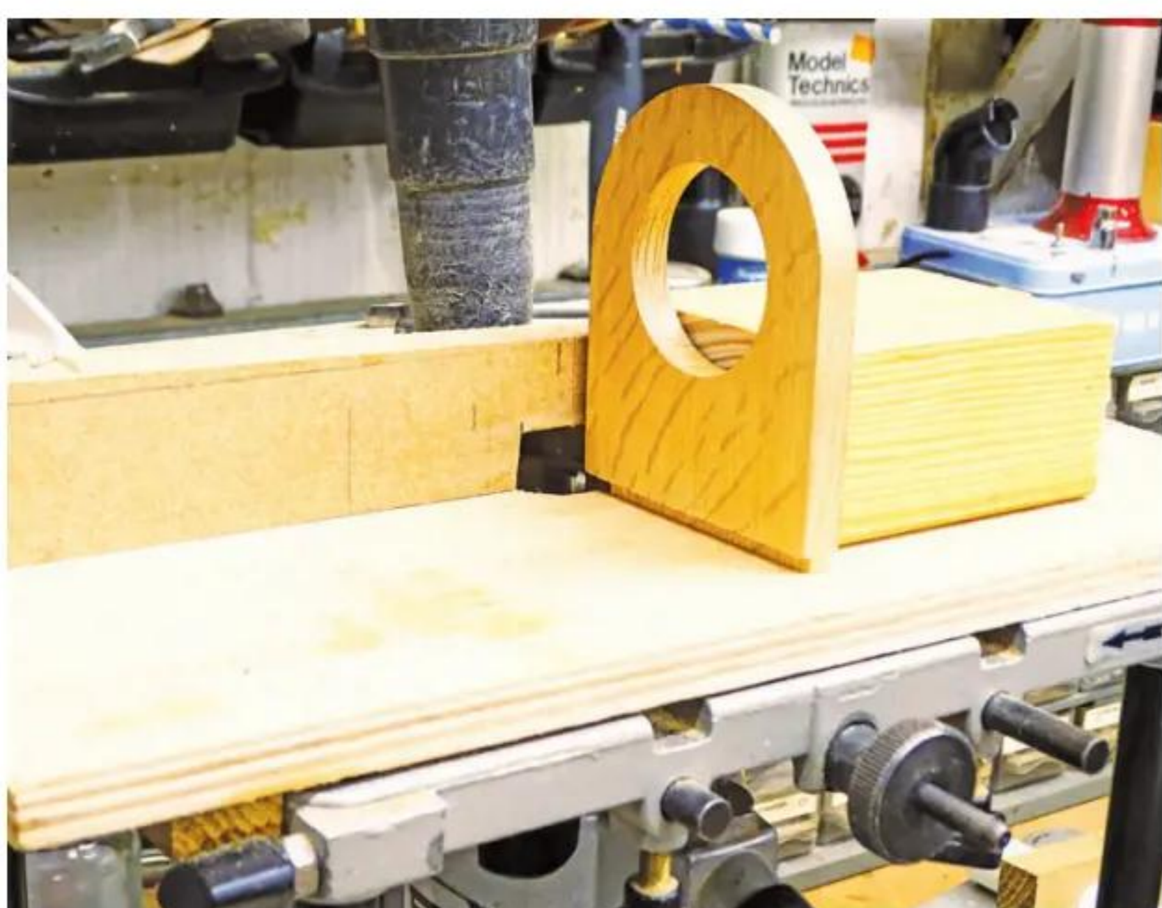
15 A support block makes this part easy
