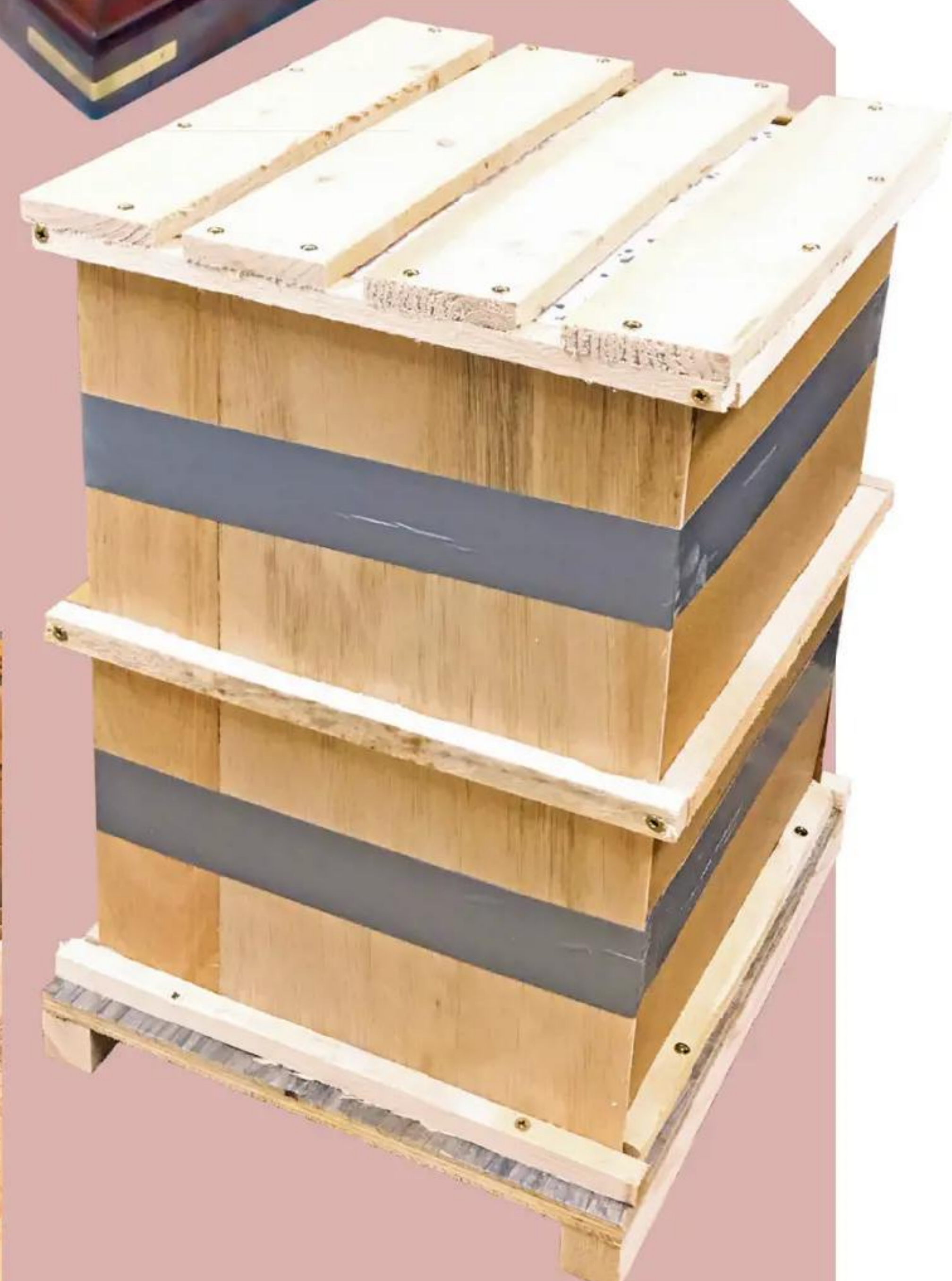
3 The polystyrene was covered in ply and outer battens, then it was ready to send
