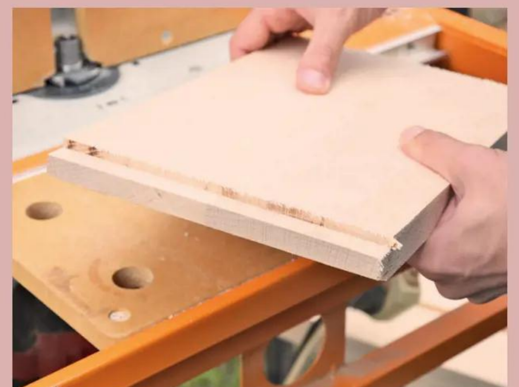
7 The ends as they come off the router table; remove the splch with abrasive before you start fitting or gluing up
