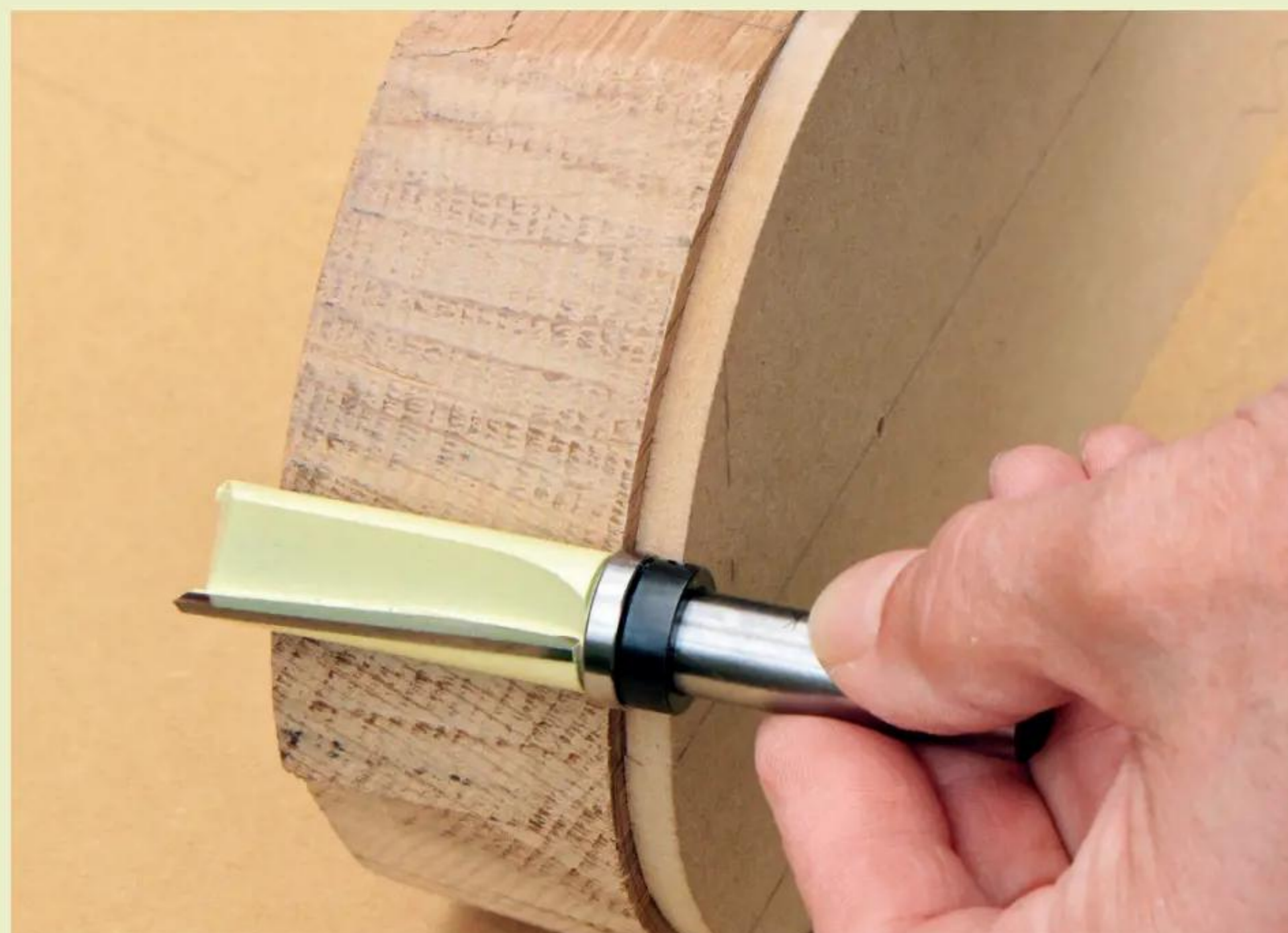
This project calls for a flush-trim bit with top roller bearing
