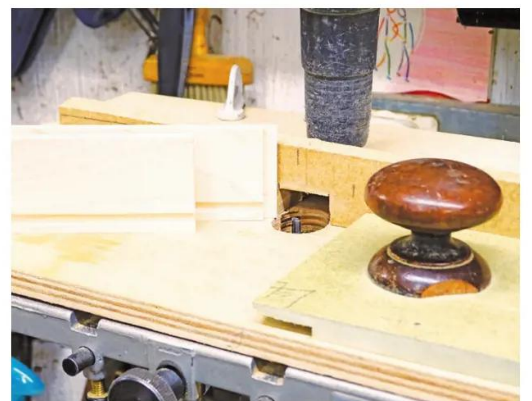
17 Rebates for the box's drawer sides are cut on a router table
