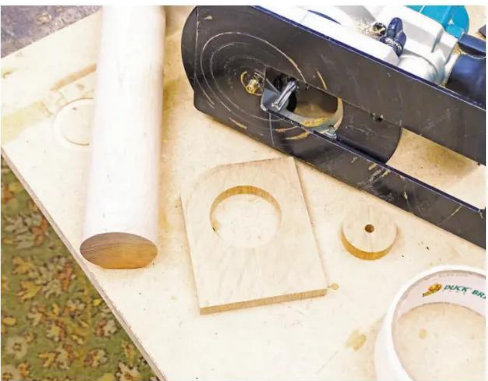
13 A circle cutting jig is really useful
