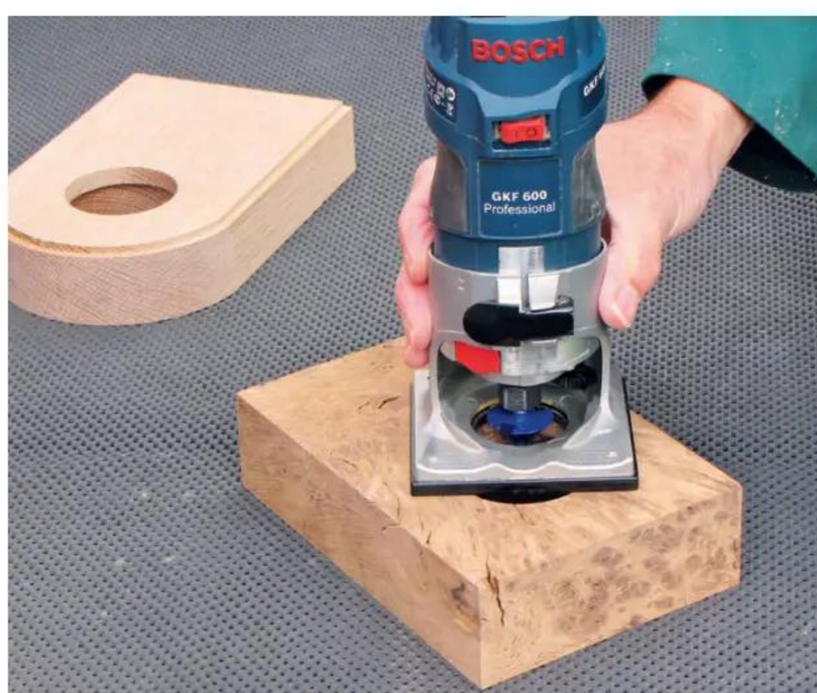
23 Sand the clock blank, finishing with 320 grit abrasive; add a fine chamfer to the straight edges and dial recess
