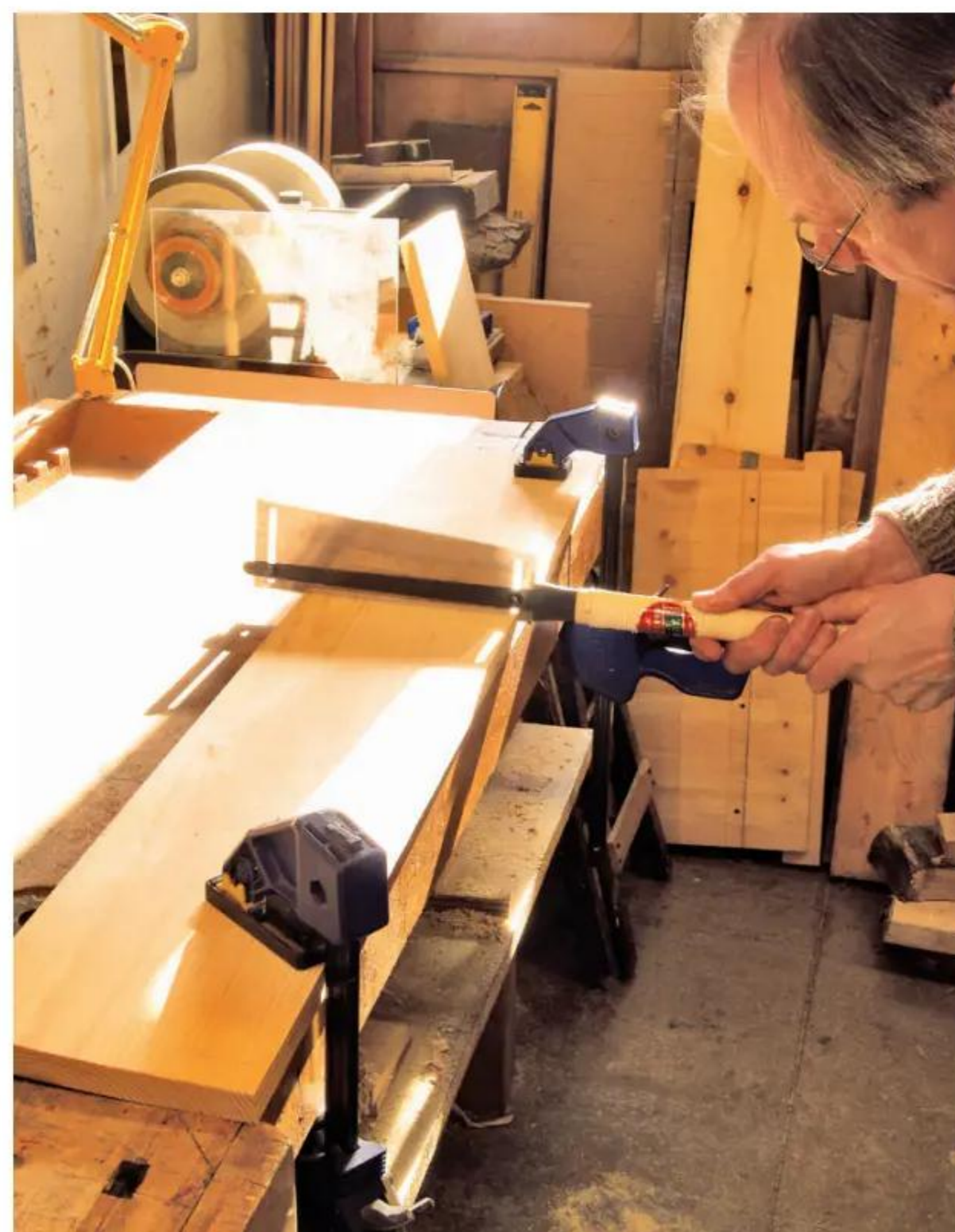
2 Cutting shelf housings to depth
