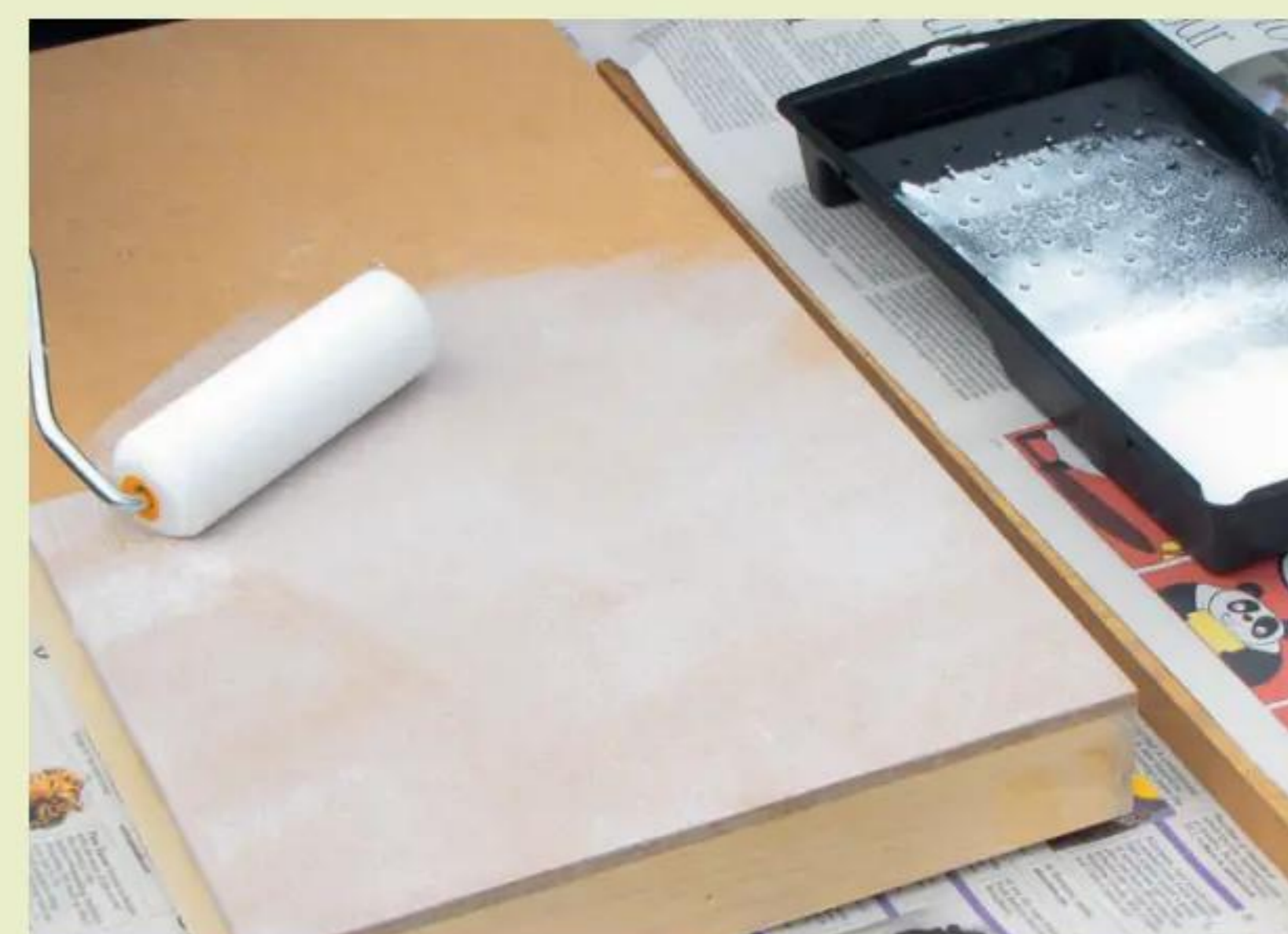
8 Trim MDF edges flush when dry. Cut veneer slightly over-size and apply glue to the top
