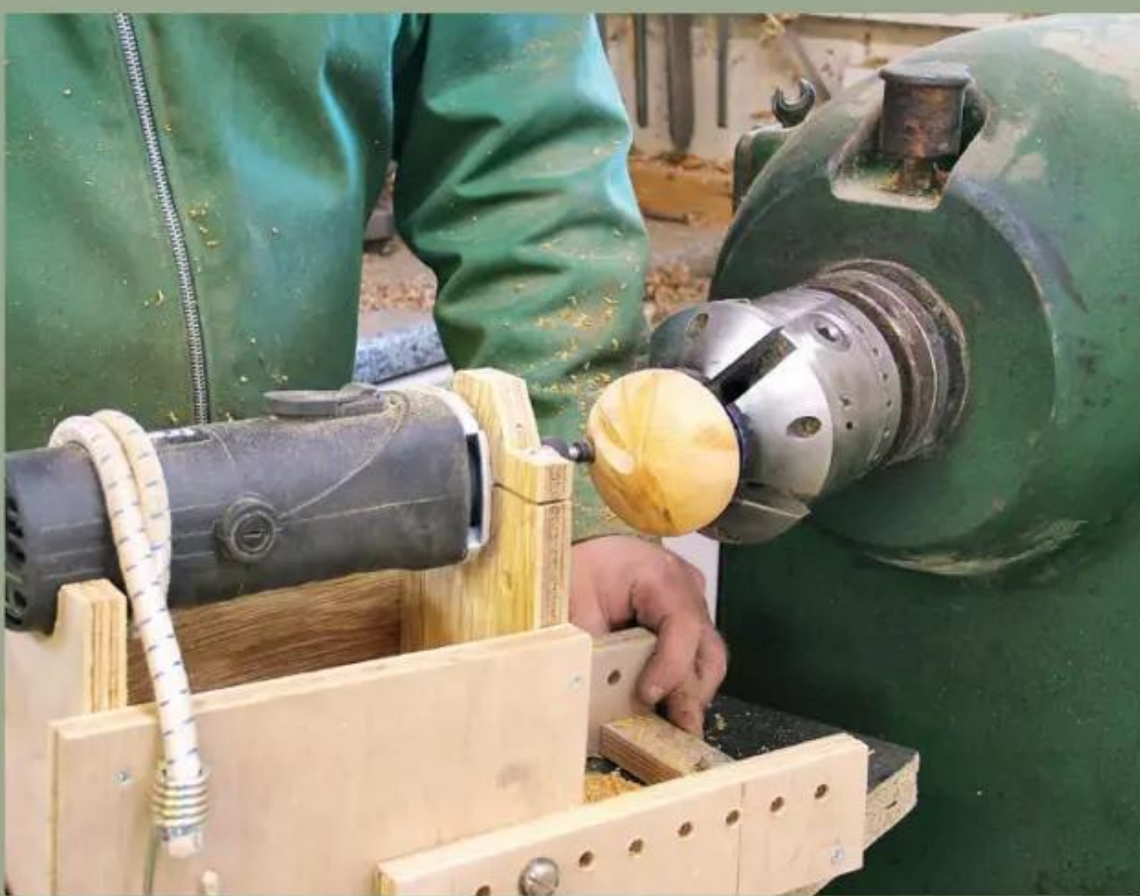
22 As the cradle rotates, the router cuts elegant grooves in the work
