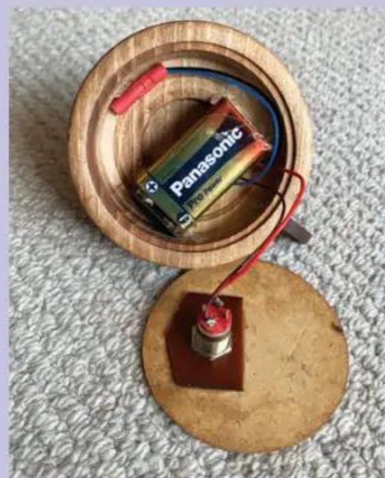
2 The battery was hot-glued into place, offset from centre to create space for the switch
