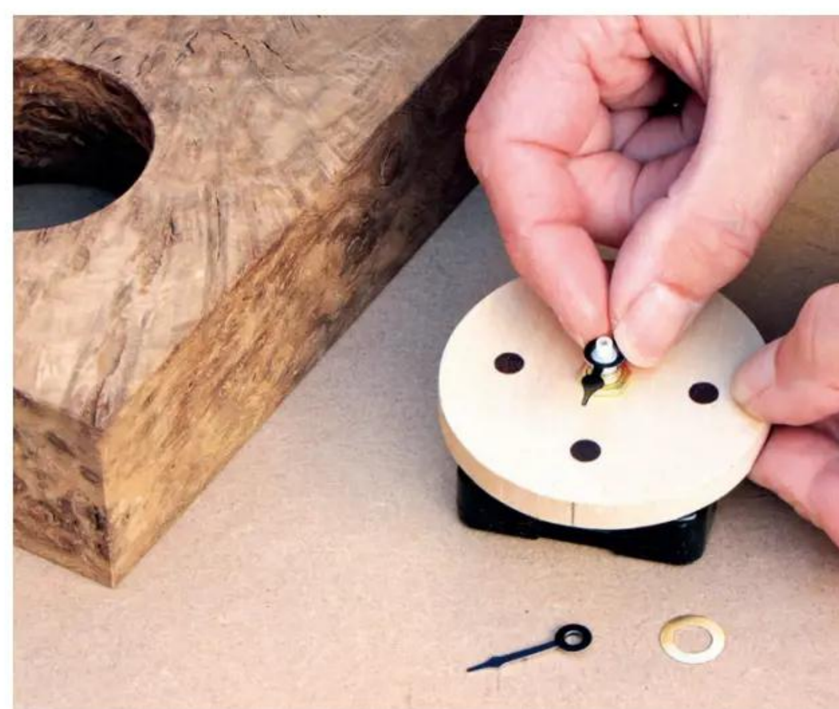
21 Mount the quartz movement on the dial's reverse and carefully fit metal hour and minute hands – these are 24mm long
