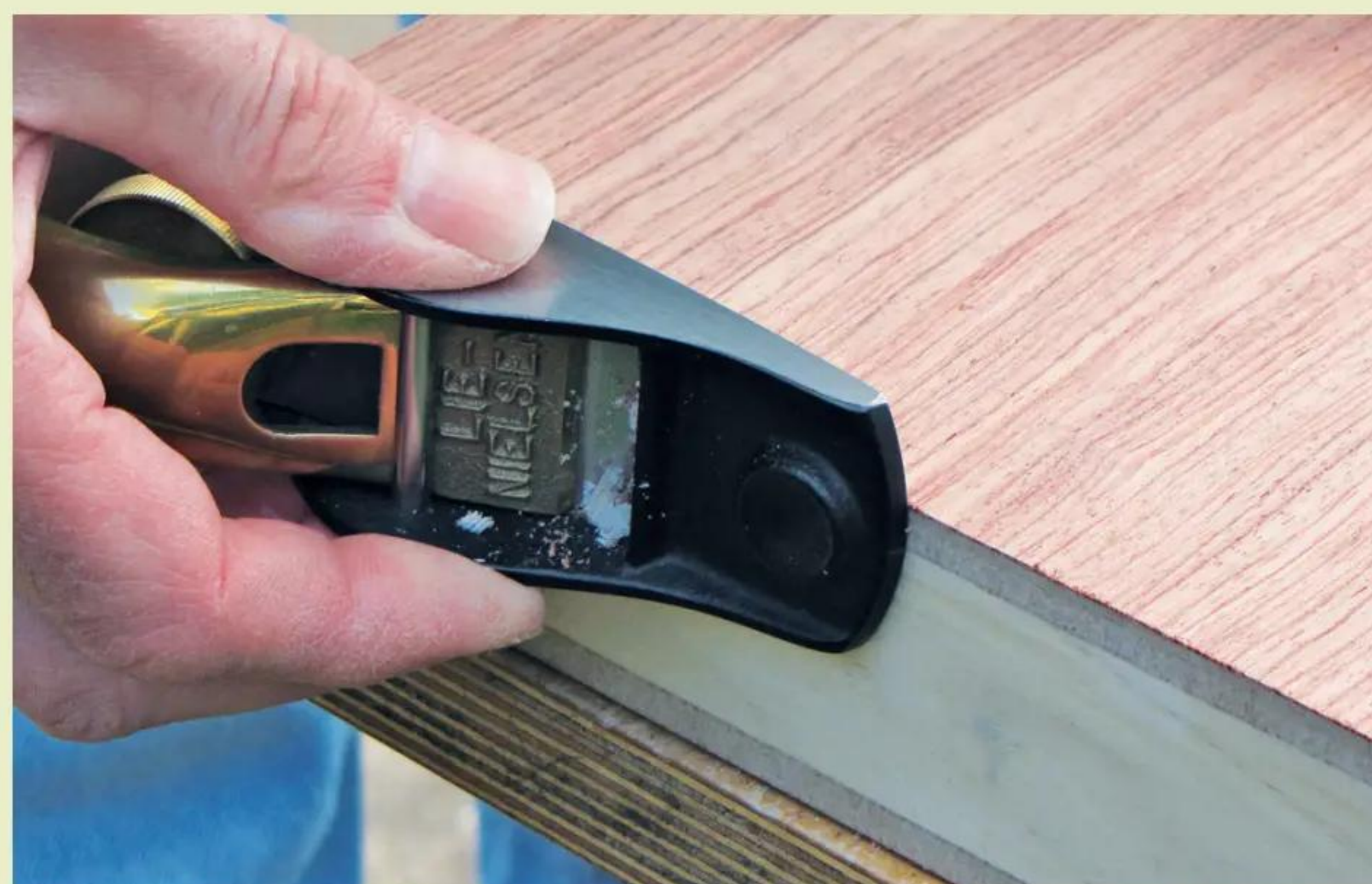
10 Trim the veneer edges flush with a router or use a finely-set block plane
