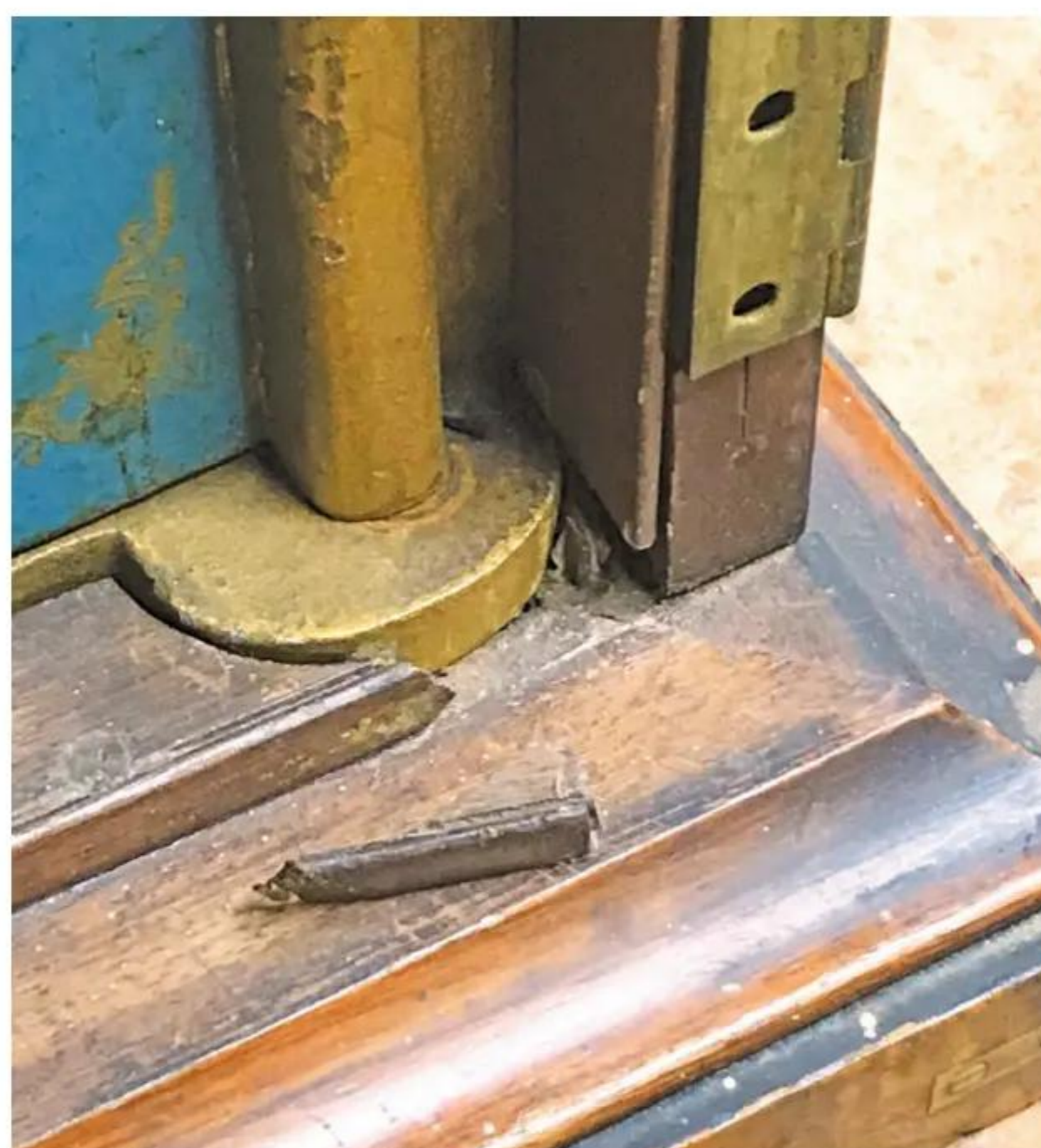
10 This tiny piece was broken away at the cabinet's bottom and some of the facing veneers were loose
