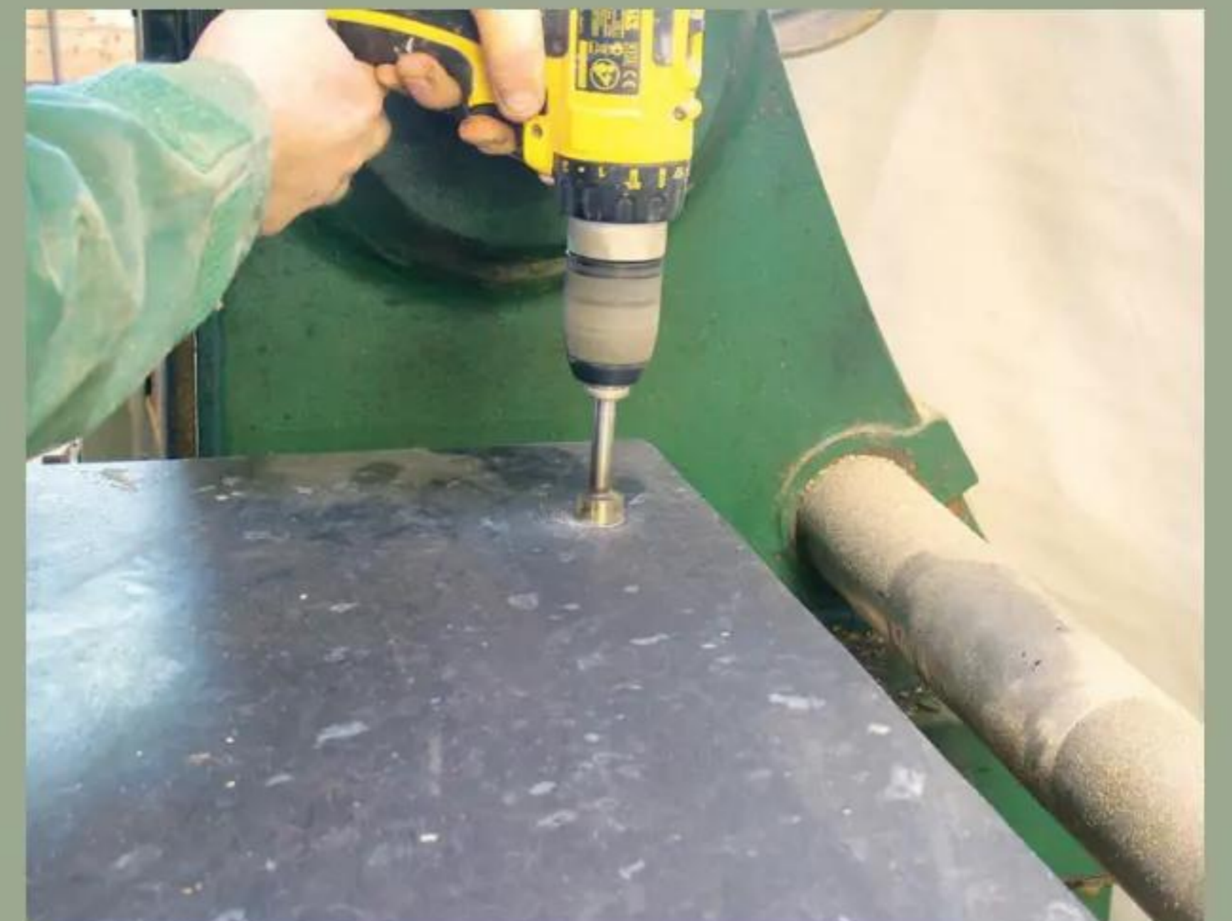
21 Drill a hole for a T-nut in the baseplate to secure the pivot point
