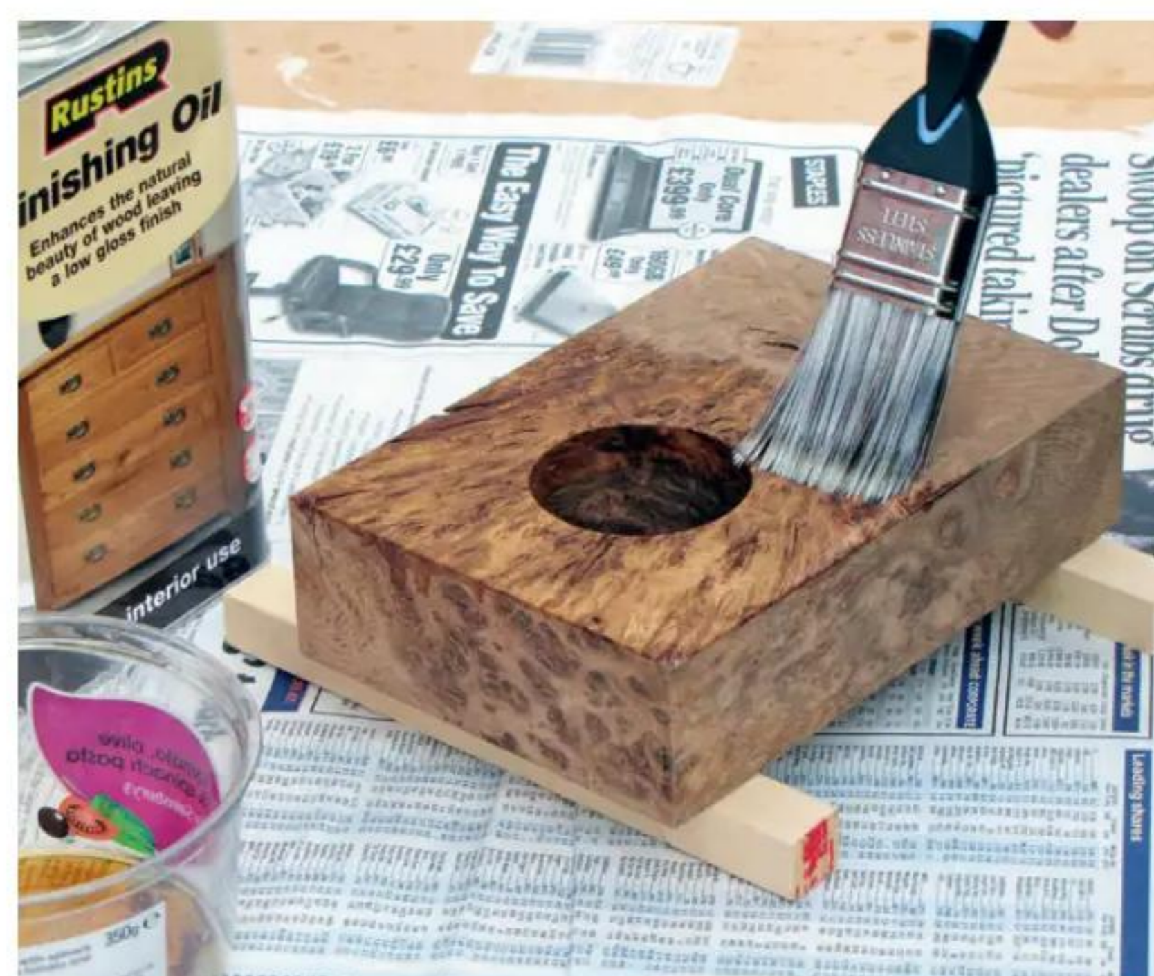
24 Brush on two coats of finishing oil, followed by clear wax, then insert the dial before securing in place with a dab of glue ✂
