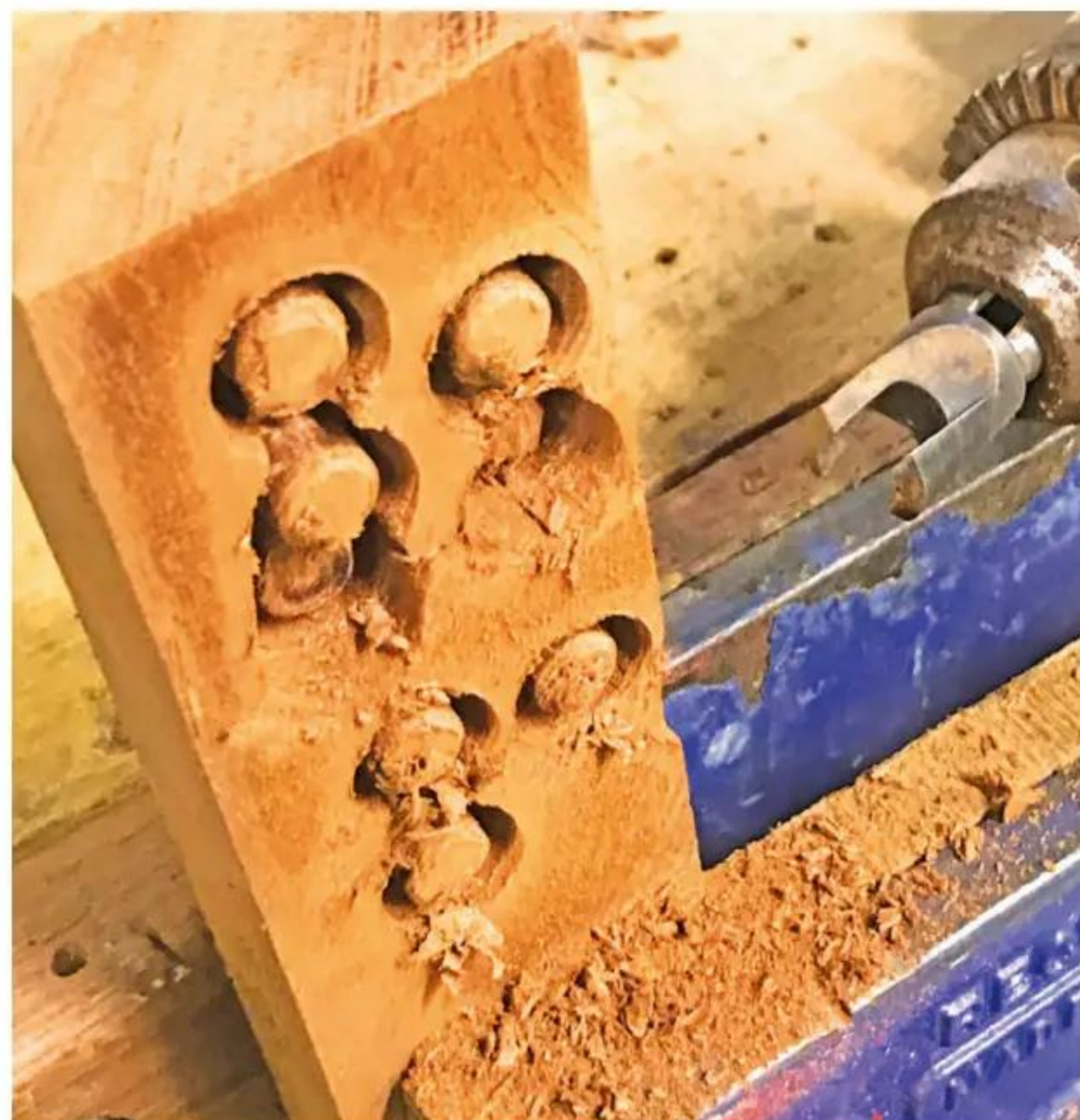
7 Small plugs were cut out of a piece of gash stock
