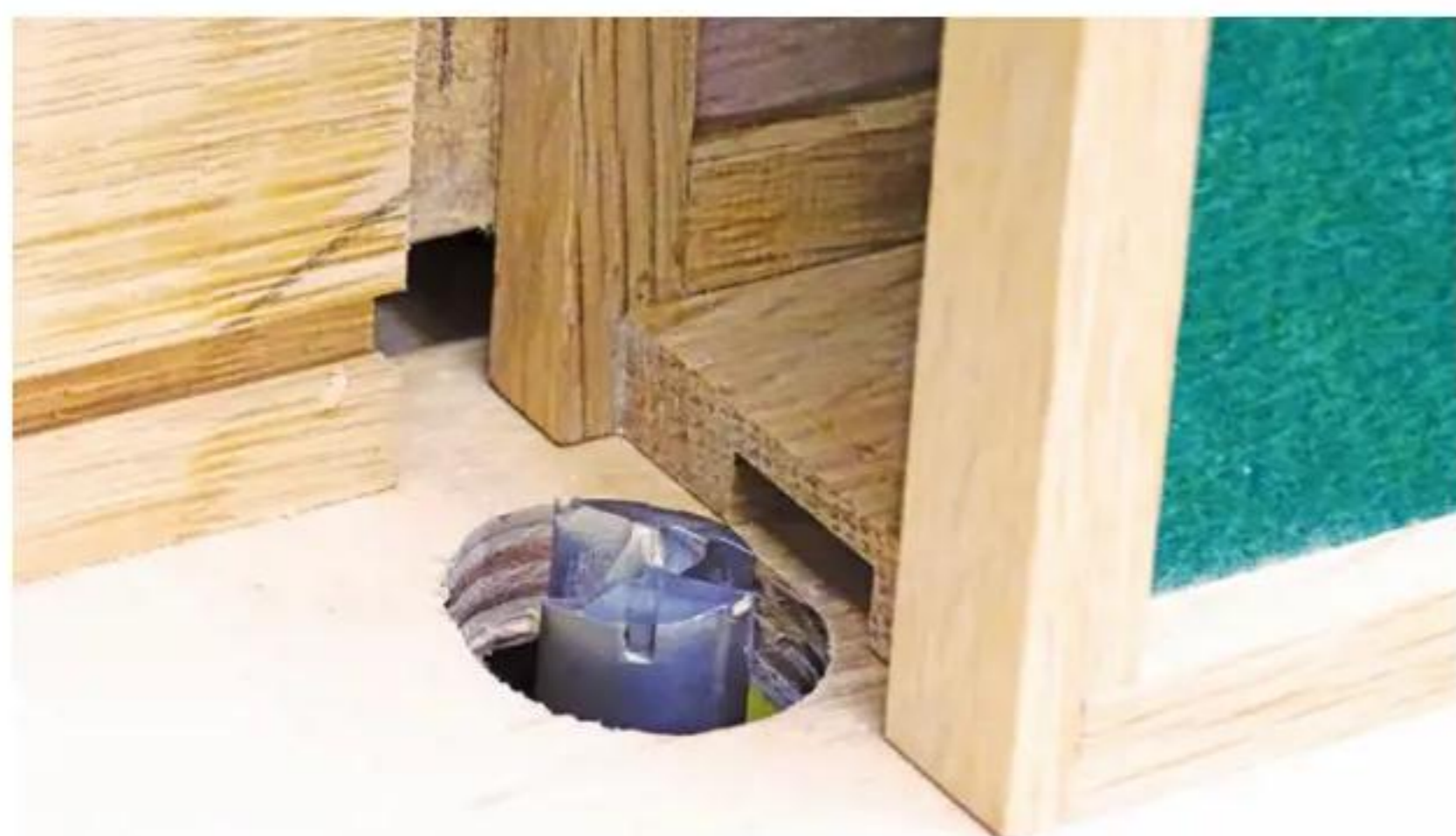
23 Cutting a finger slot on the router table
