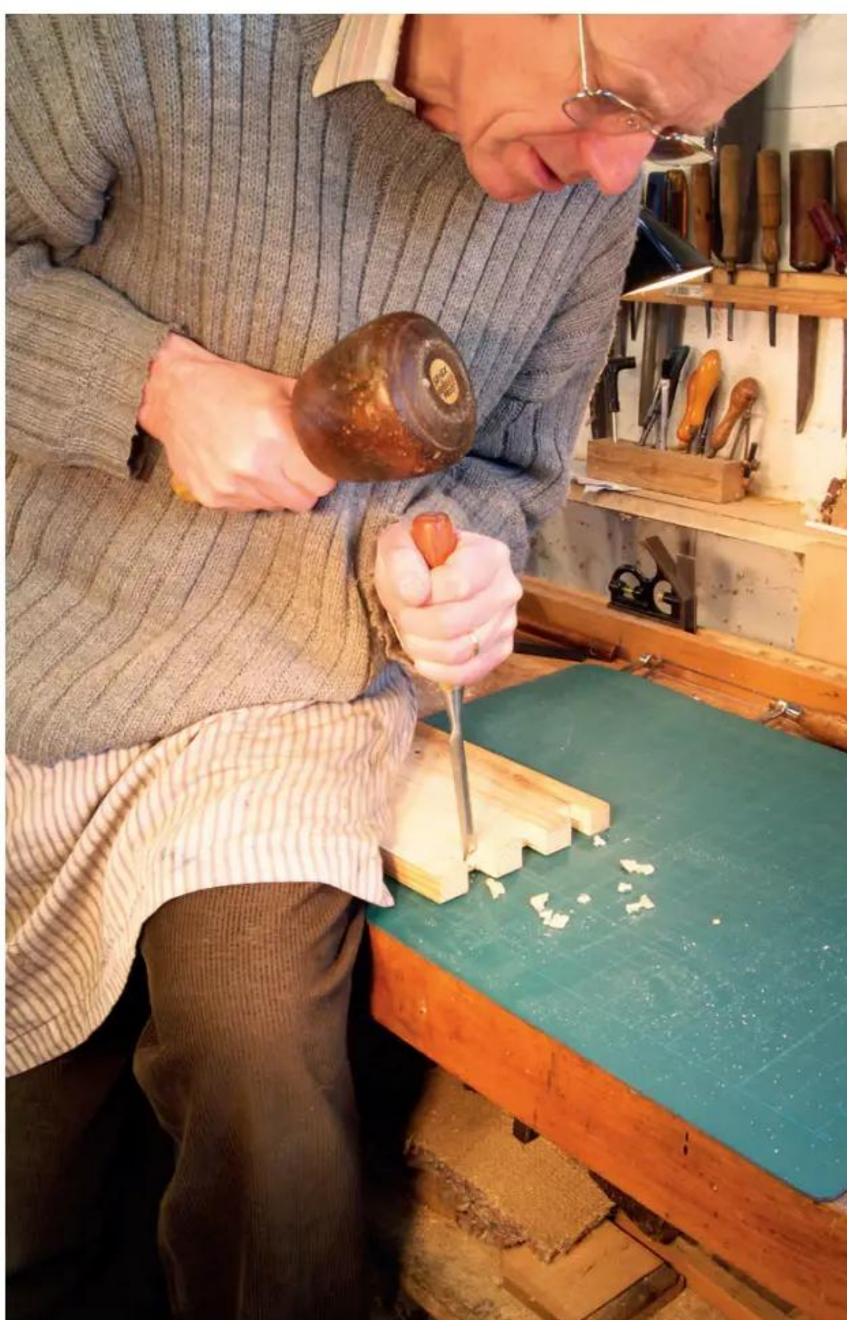
11 Cleaning up to the line: a very slight undercut will help
