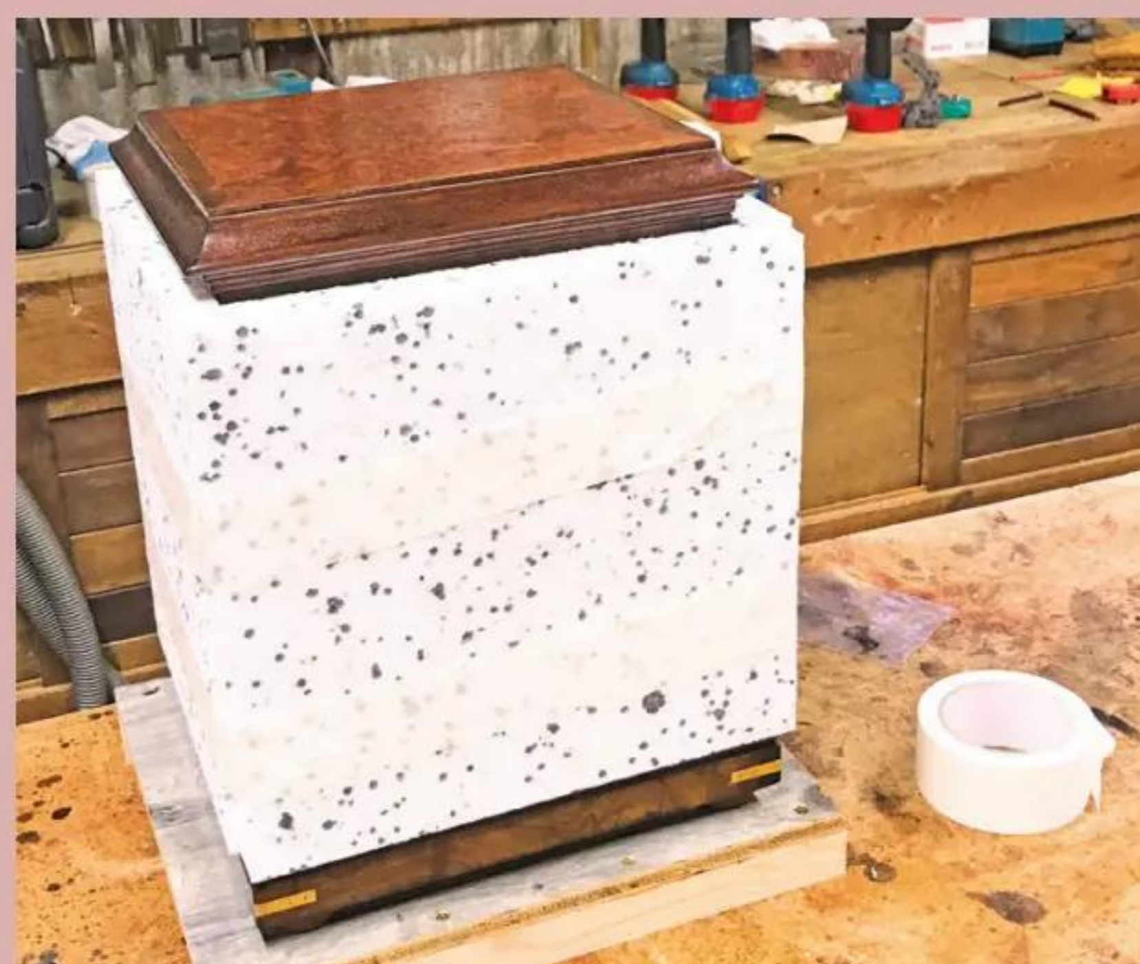
2 I made a dedicated, small pallet and placed polystyrene panels all round
