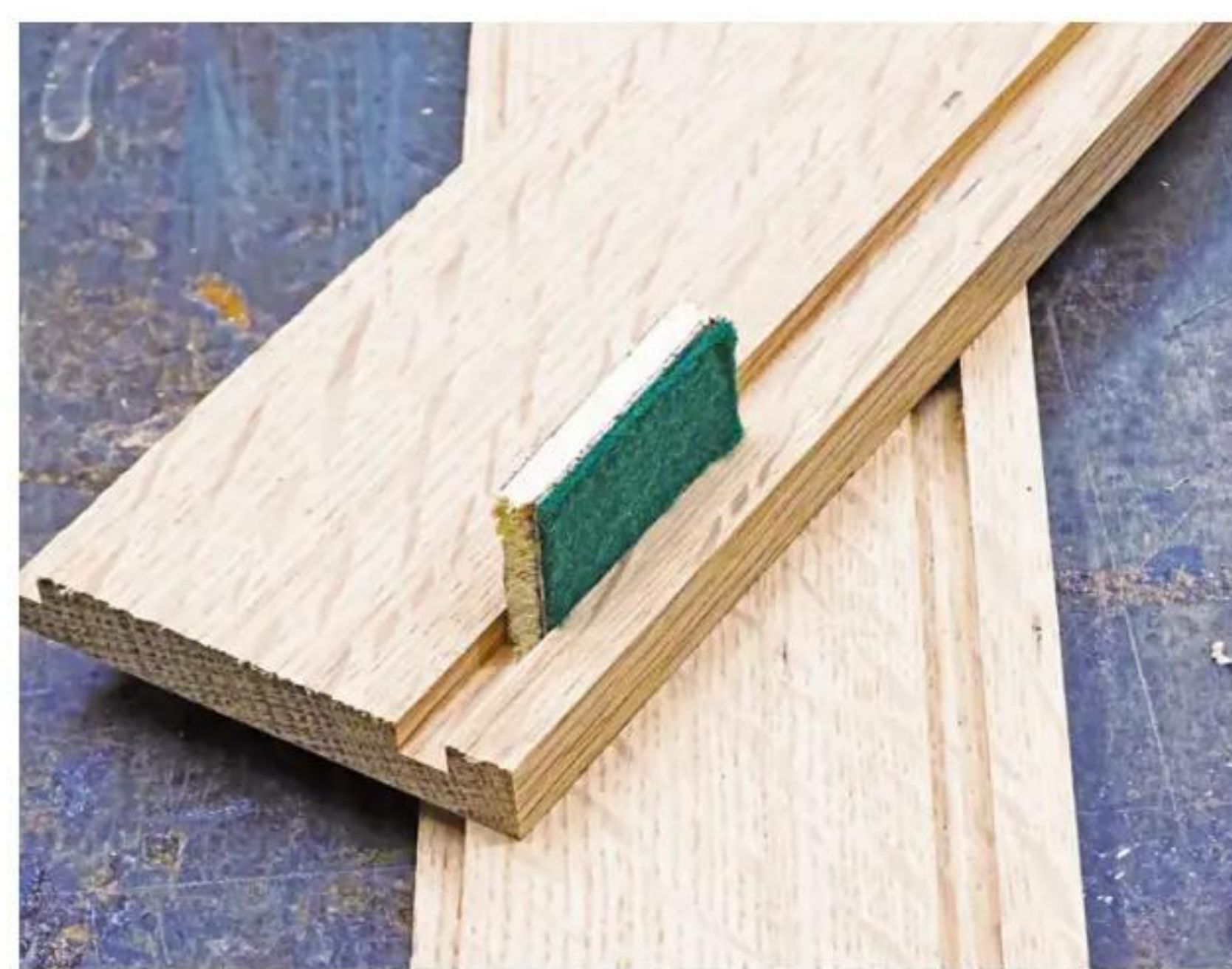
3 Make a small test piece from a plywood scrap to check the groove's thickness
