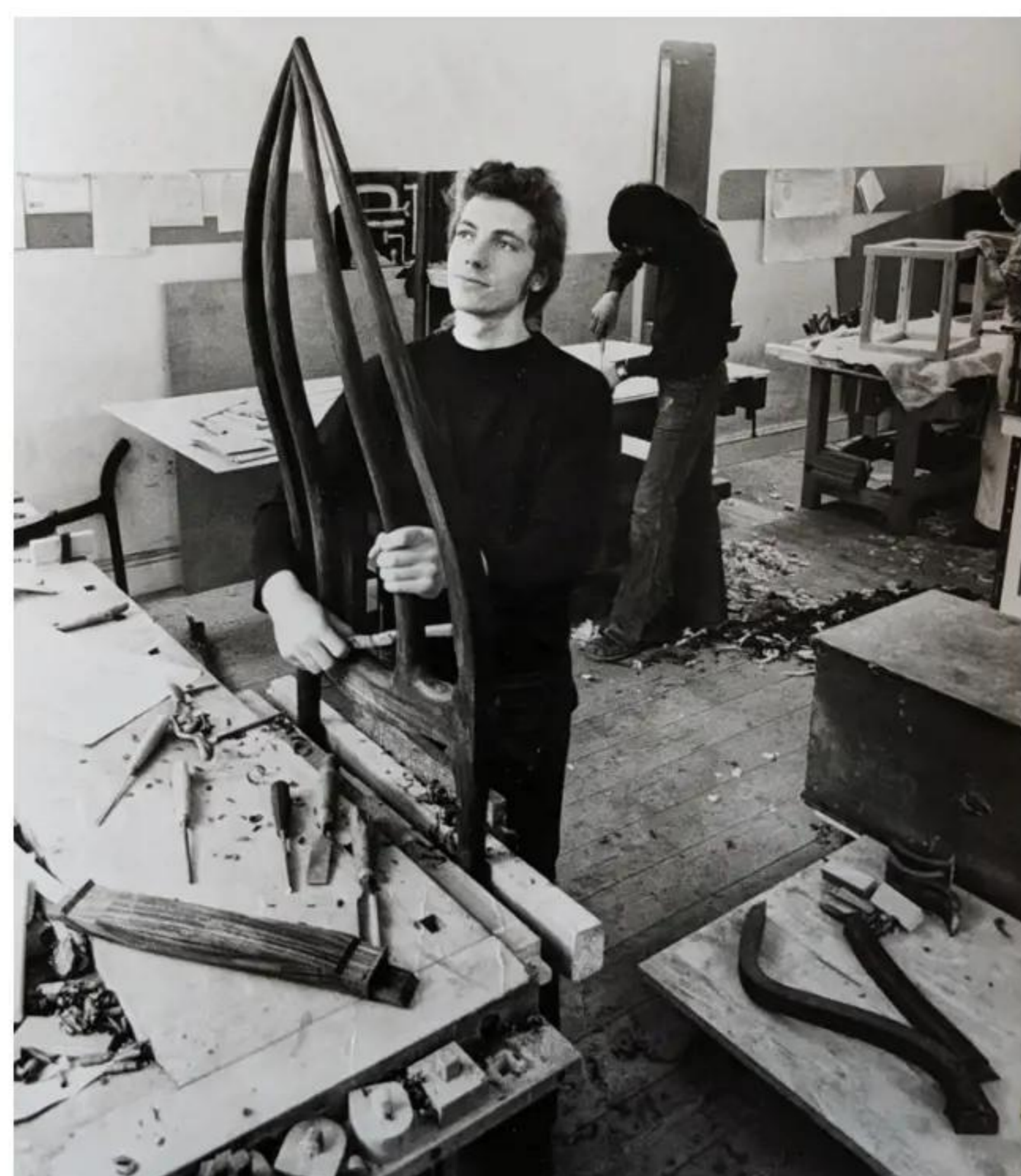
Andrew Whateley in the workshop practising his highly developed kerf lamination techniques
