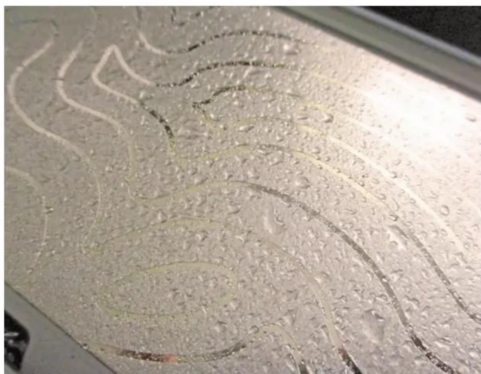
Grind stone sprinkled with honing fluid
