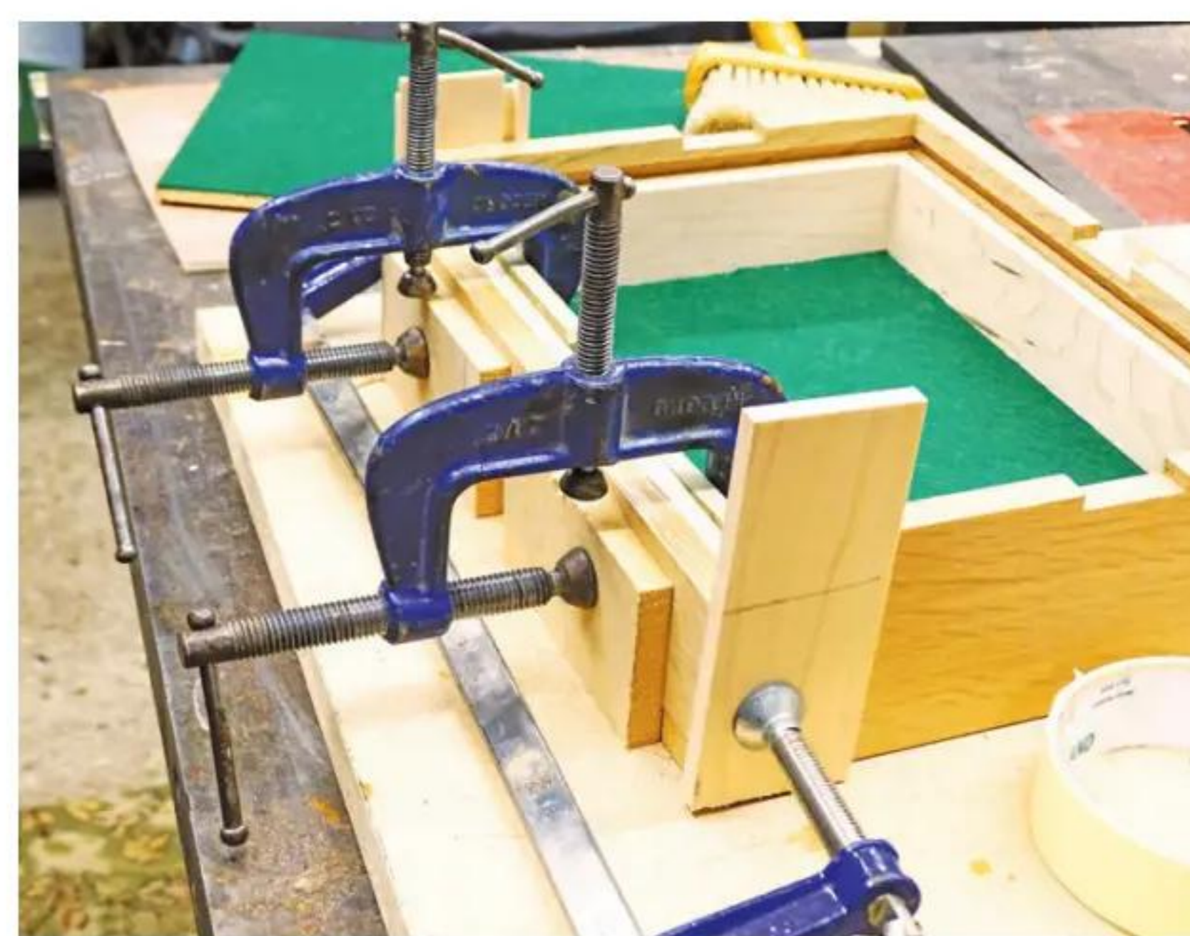
20 The drawer front is glued to the drawer in situ
