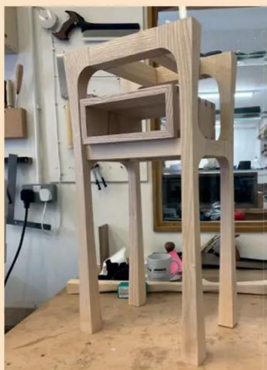
Work in progress, prior to beginning shaping
