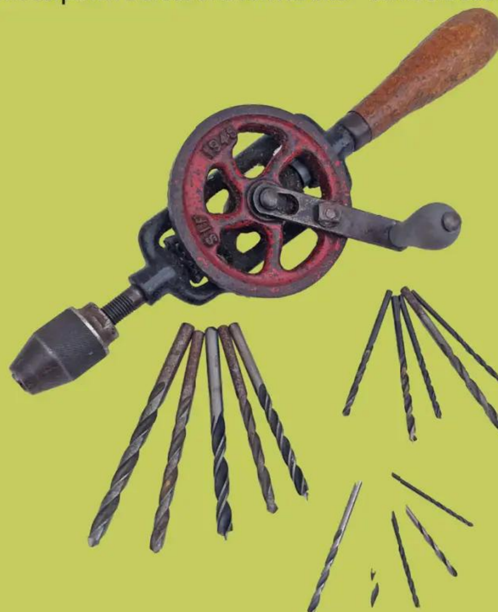
The wheelbrace, with bits – no charging, no cable, and a drop of oil every few years
