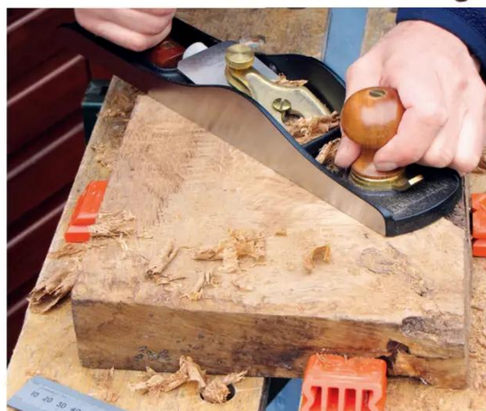
2 Wild grain is more difficult to tame, though a low-angle jack plane will help; alternatively, use a belt sander
