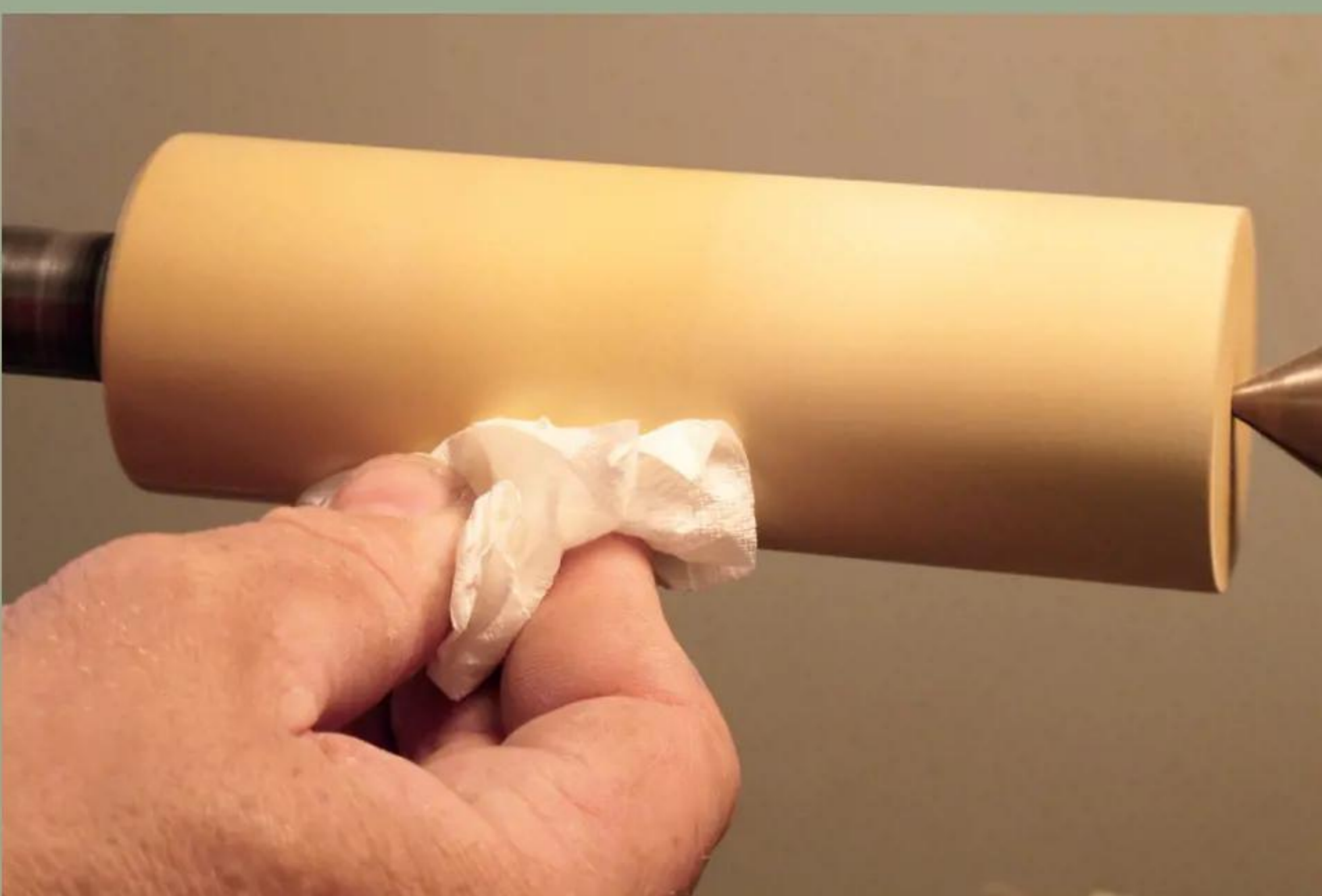
5 Friction polish needs, well, a good rub!
