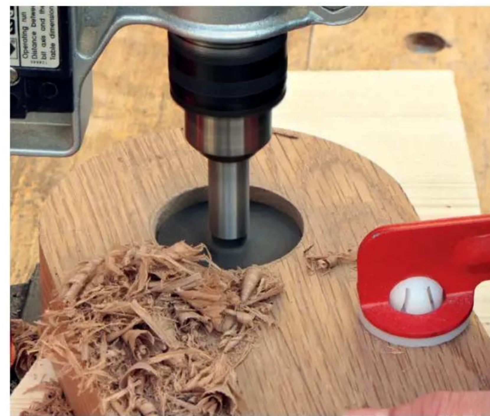
9 Mark the clock movement's centre, then bore all the way through the blank with a large-diameter – 54mm – Forstner bit
