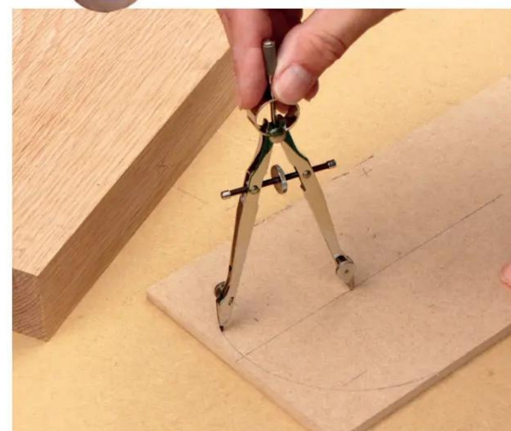
3 For a curved-top clock, it's easiest to make a template from 6mm MDF; draw a 70mm radius with a pair of compasses
