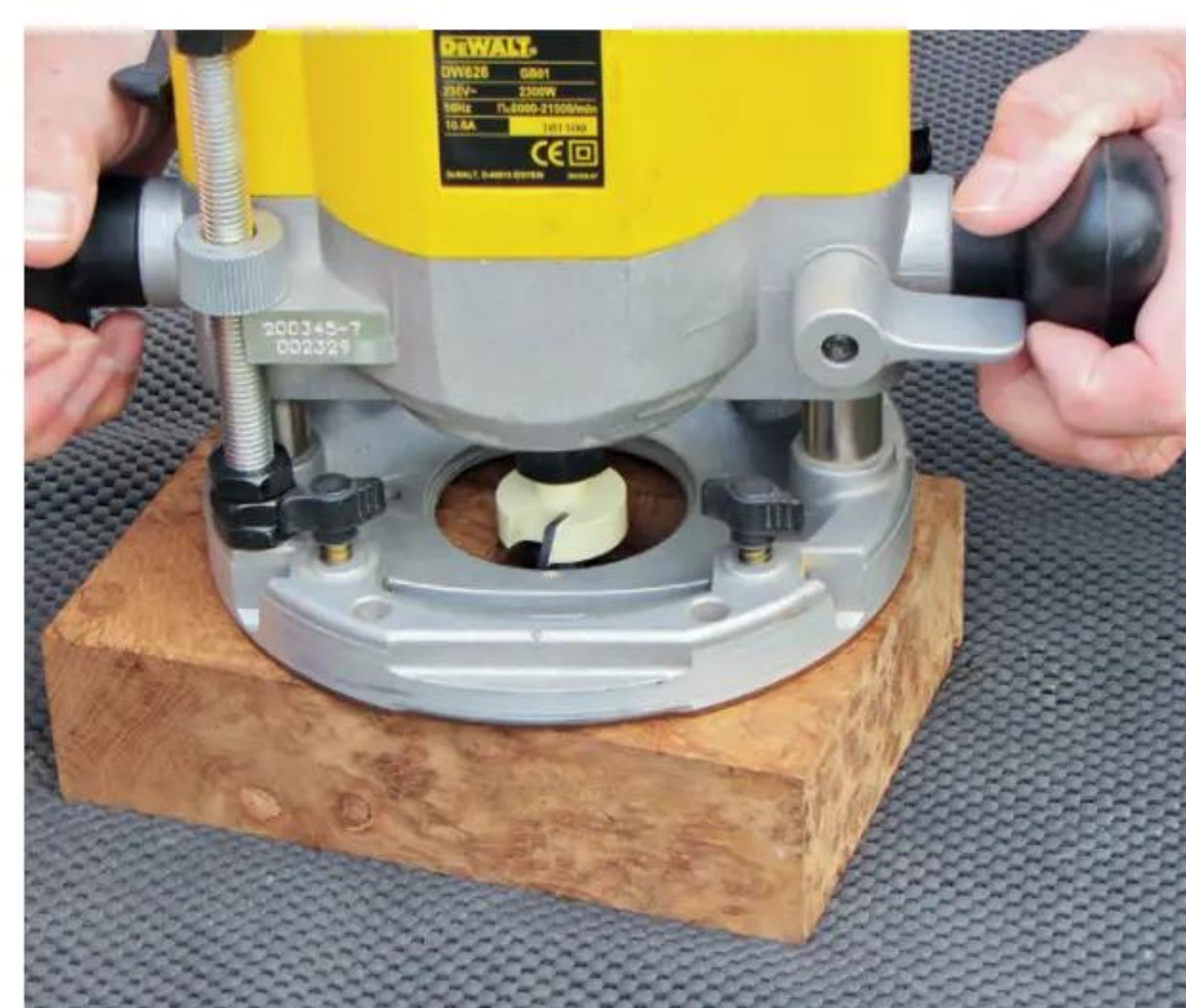
12 Now use a template with a 75mm-diameter hole to rout from the back; finish with a rebate cutter for the rear plate
