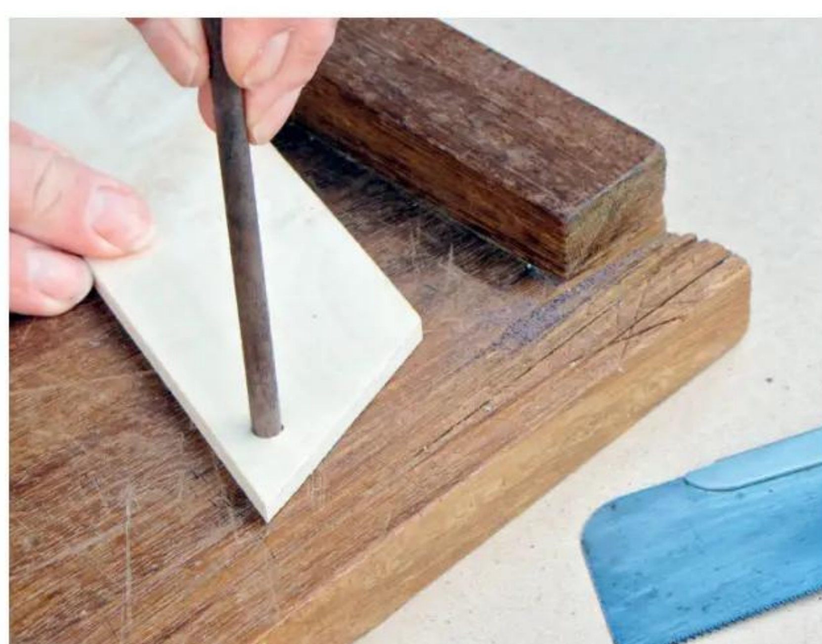
17 Hour marker dots on the dial are made from 6mm walnut dowelling; drill a 6.5mm hole to check the dowel fits snugly
