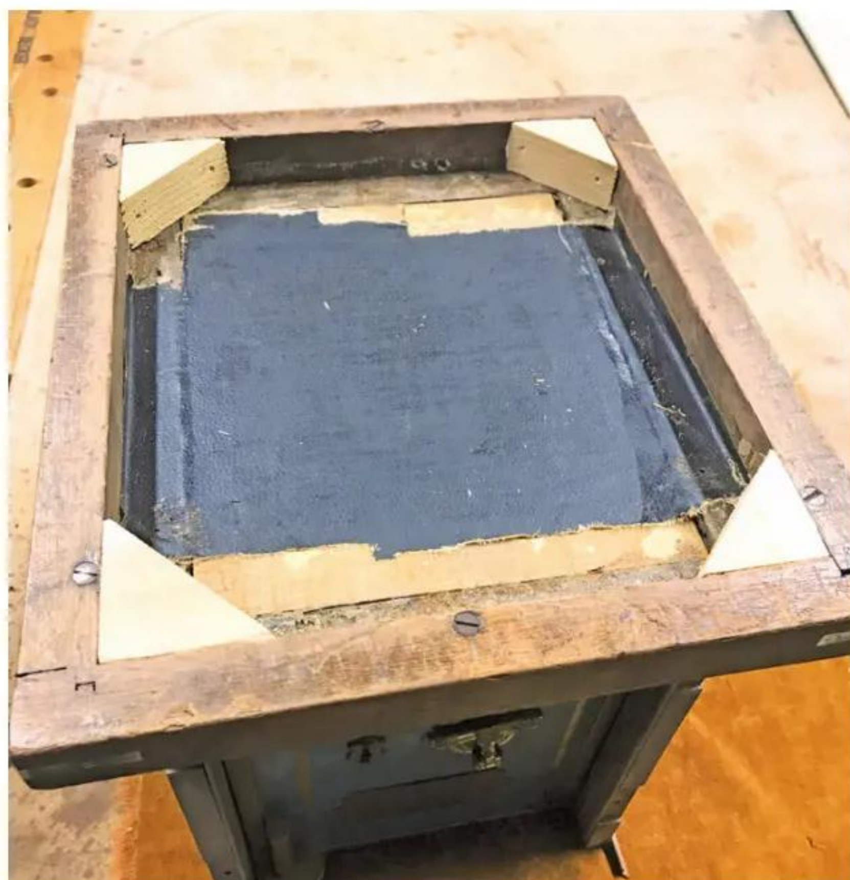
16 On the bottom diagonal, brackets were fitted for the new bun feet
