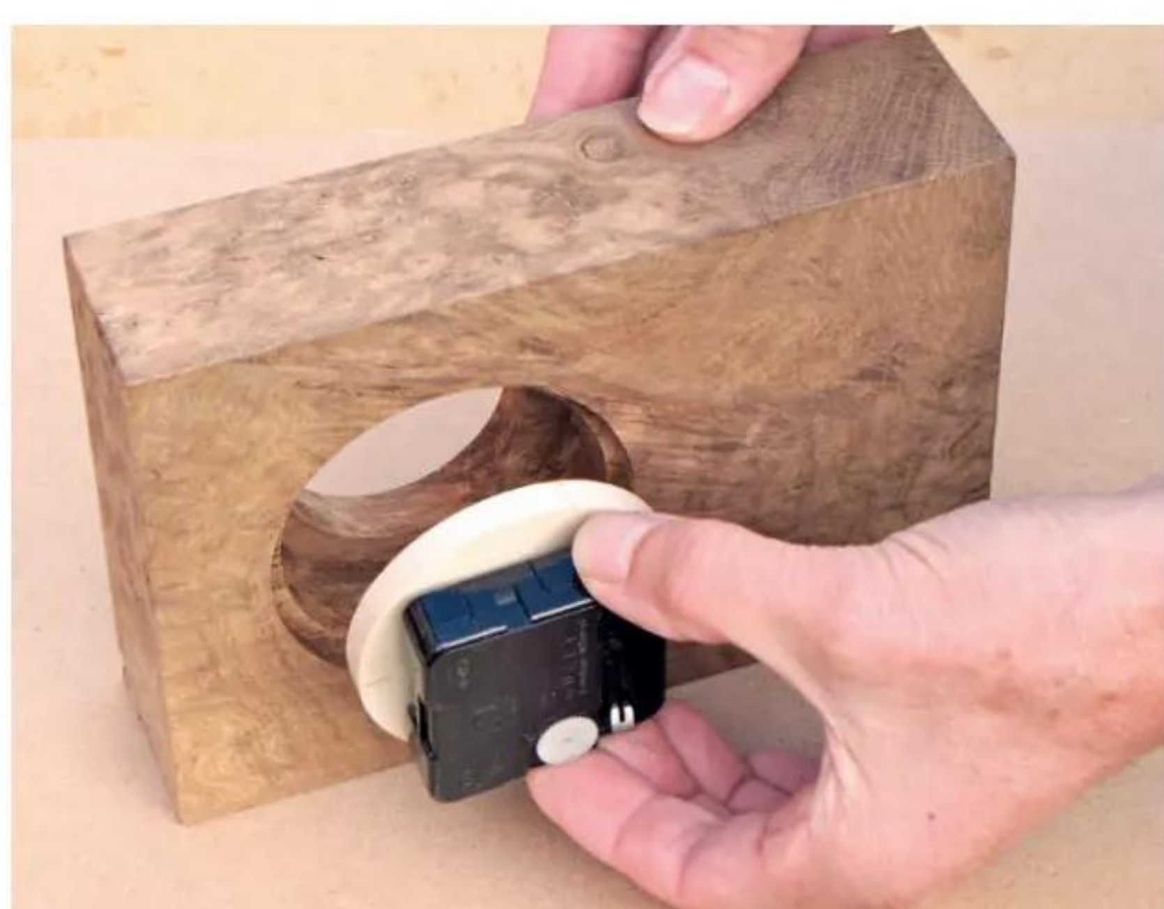
16 Cut a 8mm sycamore dial with a Dremel tool or flush-trim bit and template; check the movement fits in the recess
