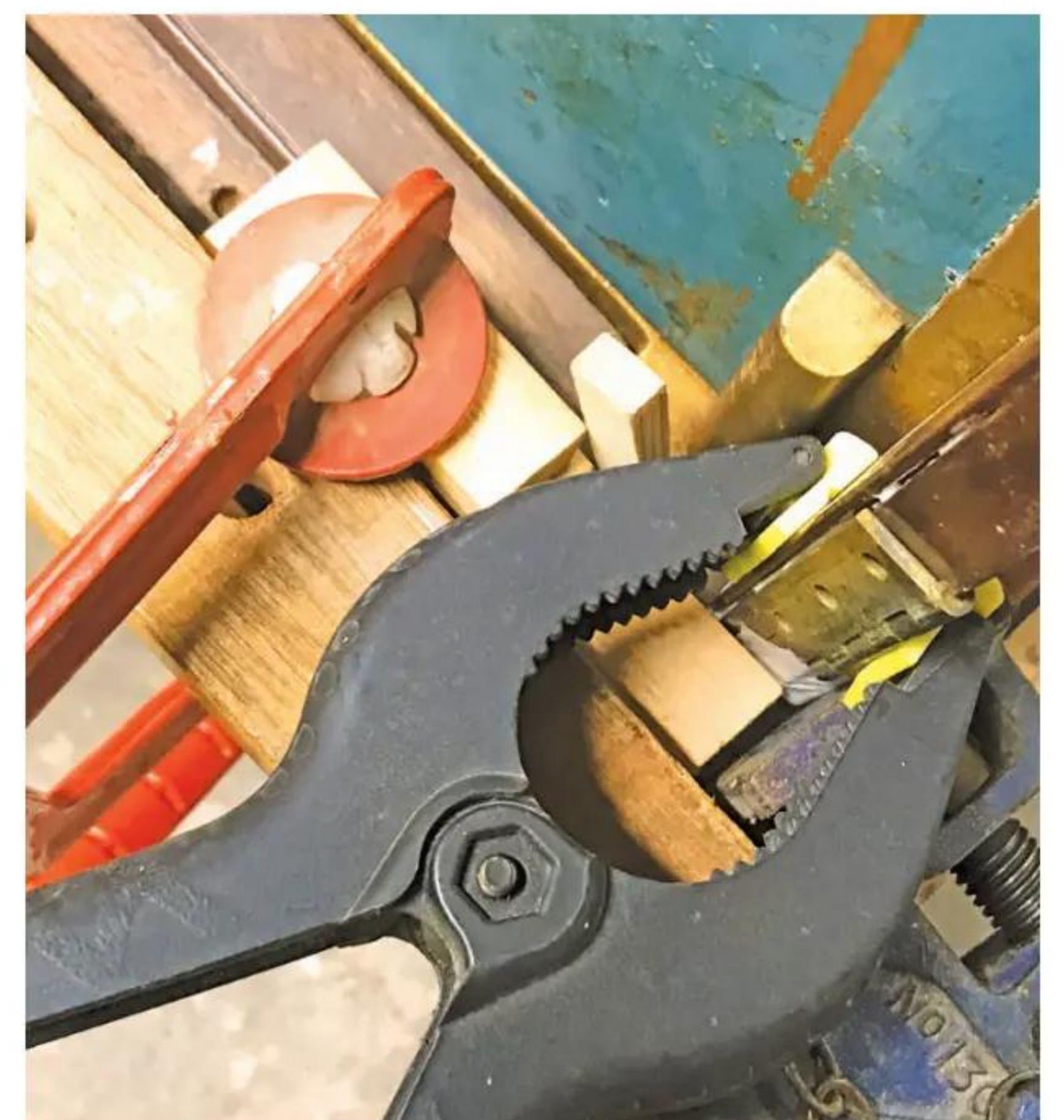
11 A complicated array of cramps fixed the loose bits back in place
