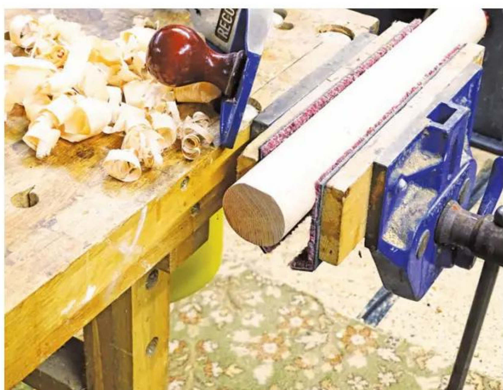
24 Plane a flat on the dowel's surface
