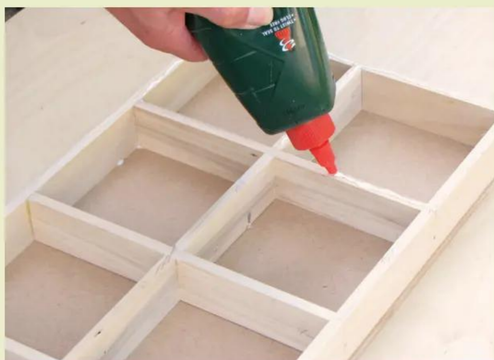
6 With top and bottom panels cut over-size, apply glue to the framework's upper surface
