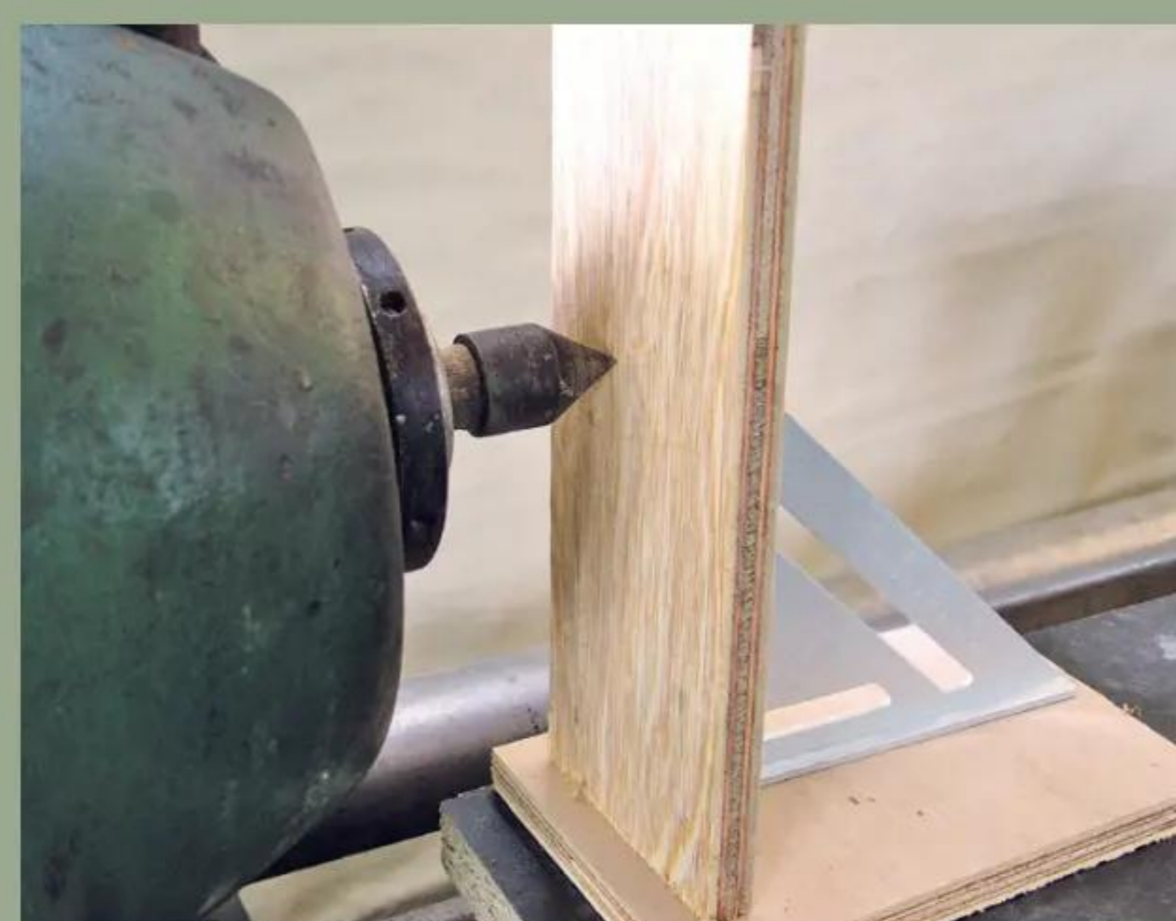
5 Use a revolving centre in the headstock to mark the cradle upright
