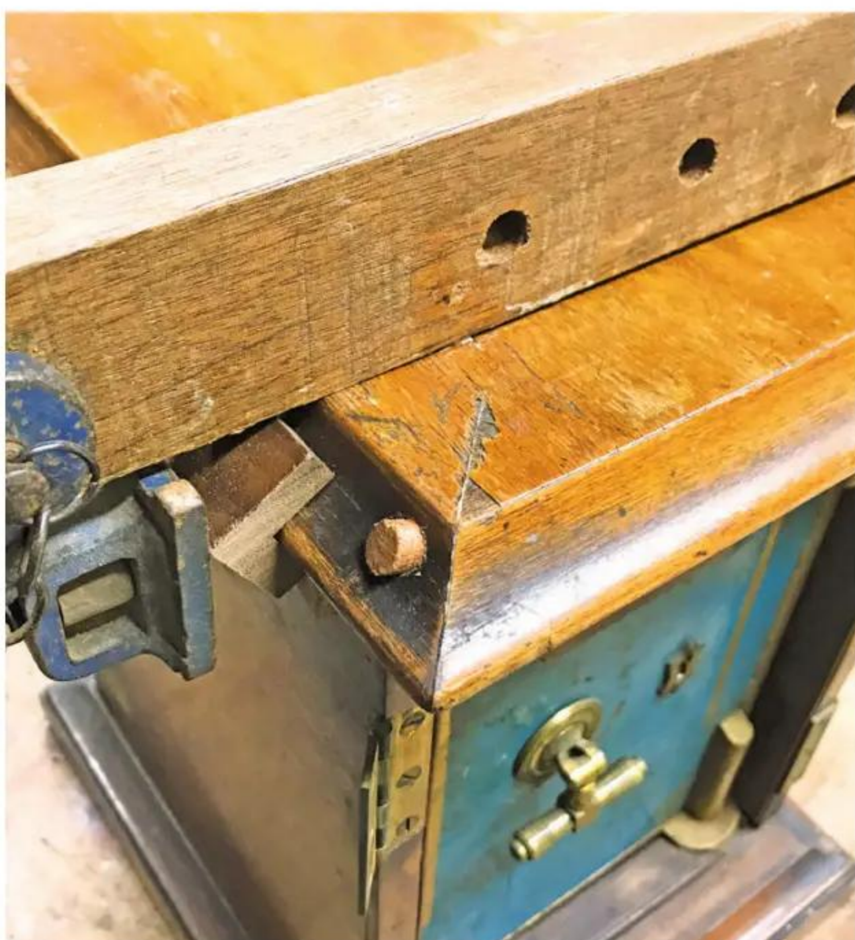
9 Clamps, an angled screw and a plug sorted out the joint
