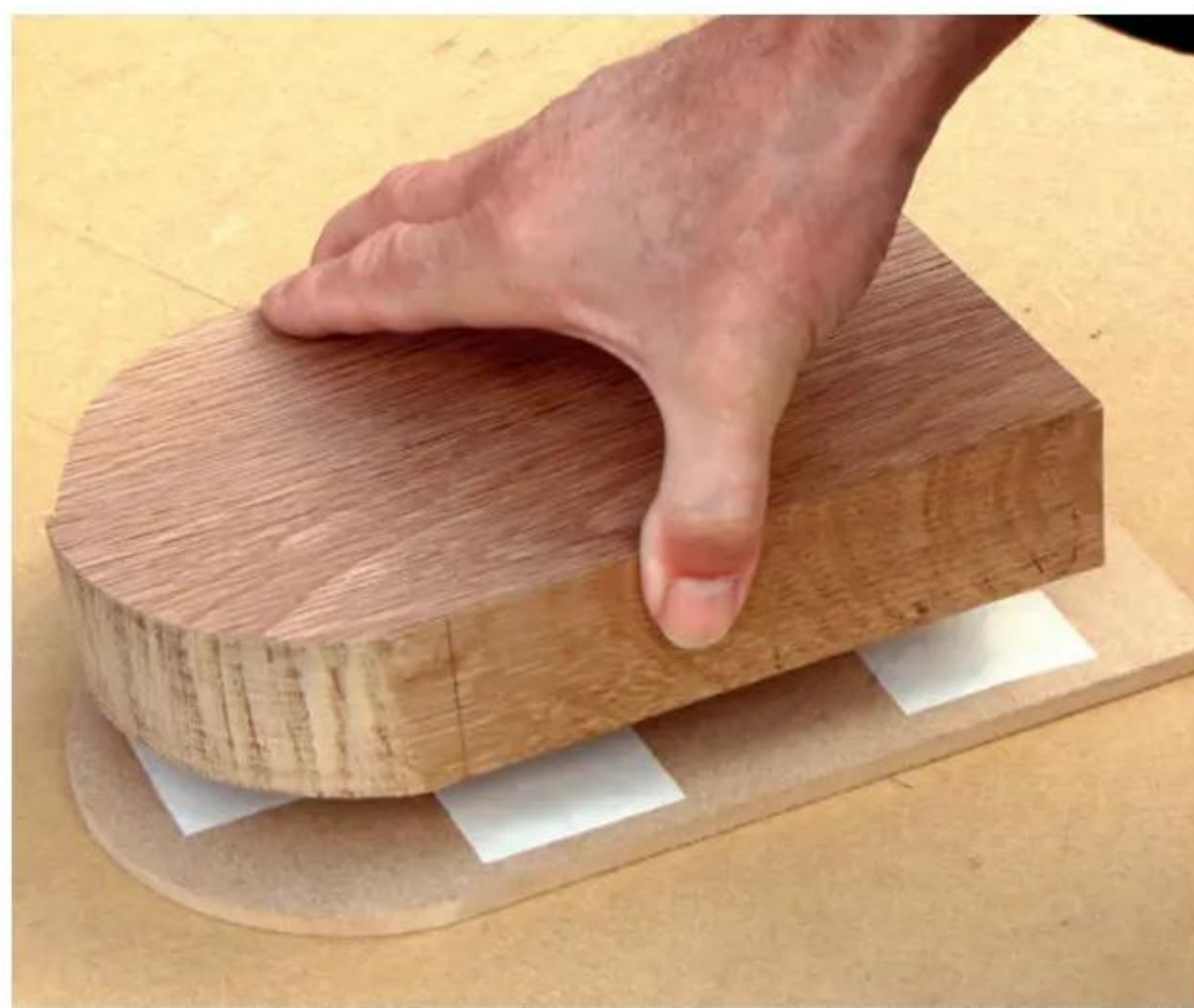
7 Carefully position the blank onto the template and press down firmly; you could fix with panel pins if preferred
