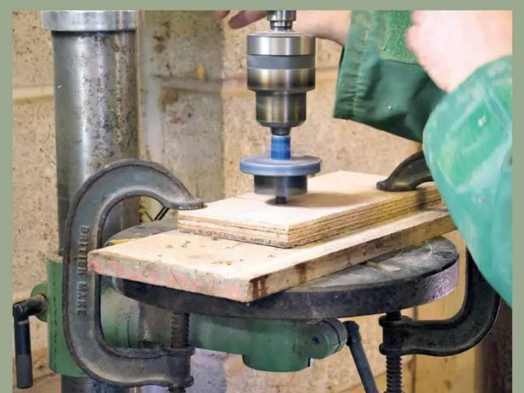
6 A hole saw is the best tool for cutting a hole for the router collar
