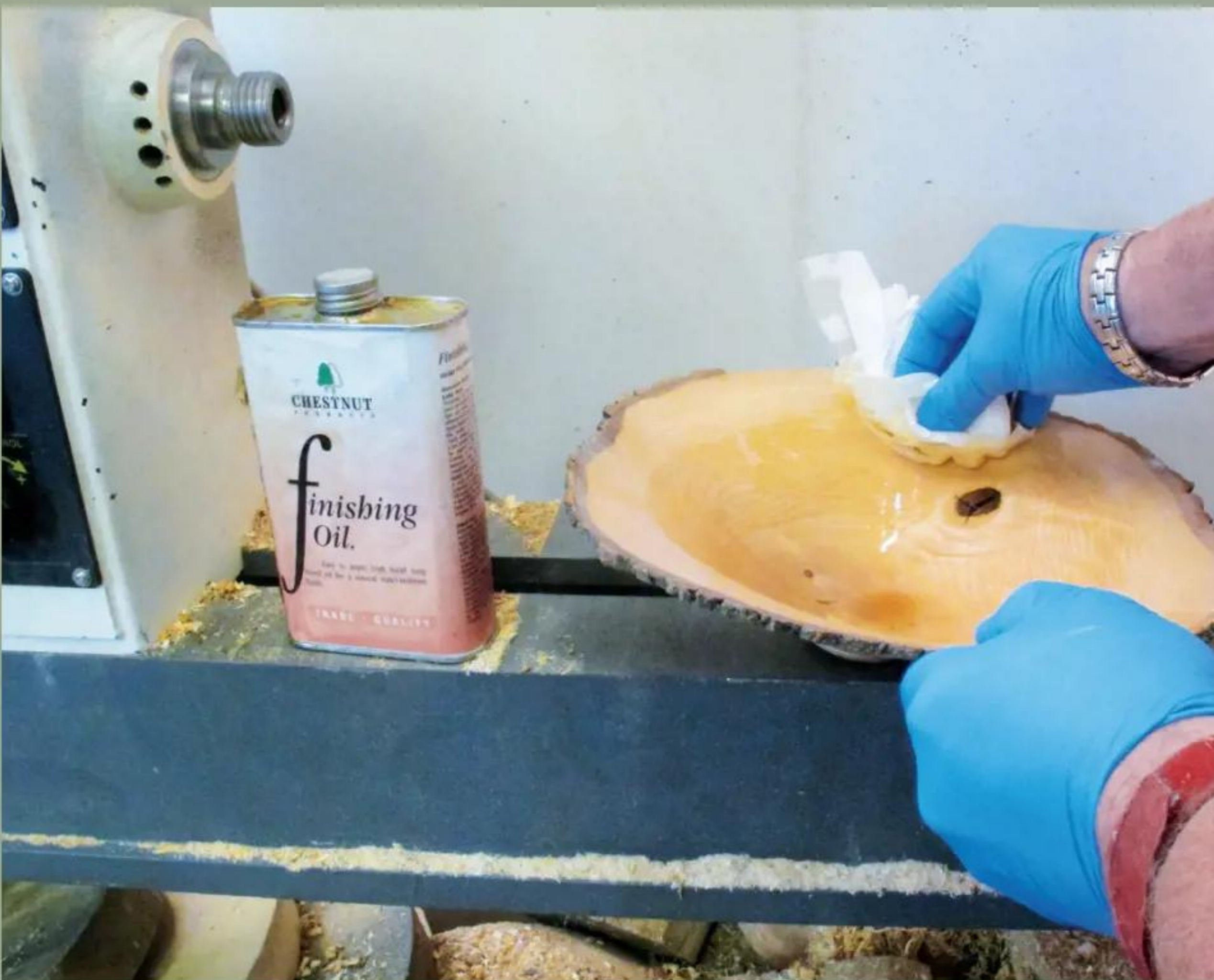
4 Slap on the oil – the more the merrier!
