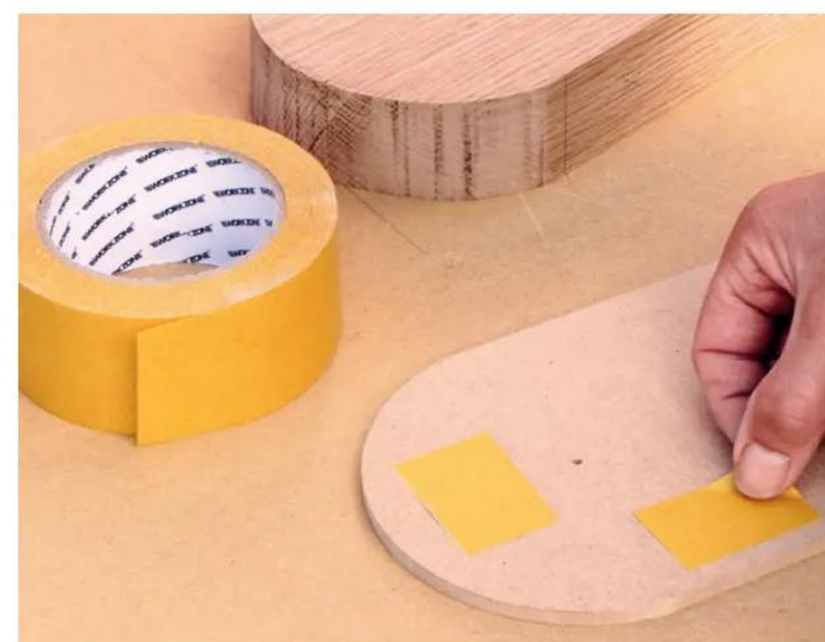
6 The template needs to be accurately made for routing; stick this to the clock blank with double-sided tape
