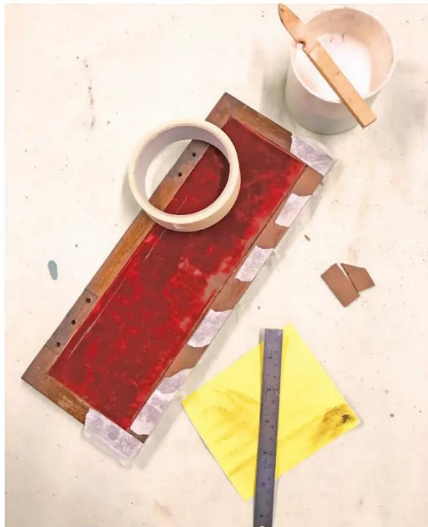
5 PVA and marking tape are used to fix the strips in place
