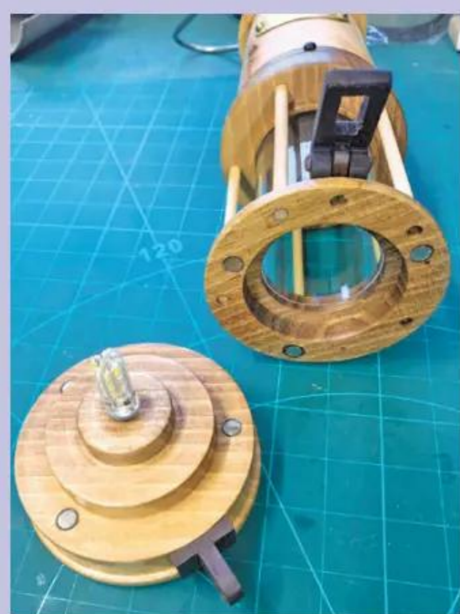
3 The original's lamp housing bottom section is secured with a screw thread – John relied on a fairly snug fit and magnets
