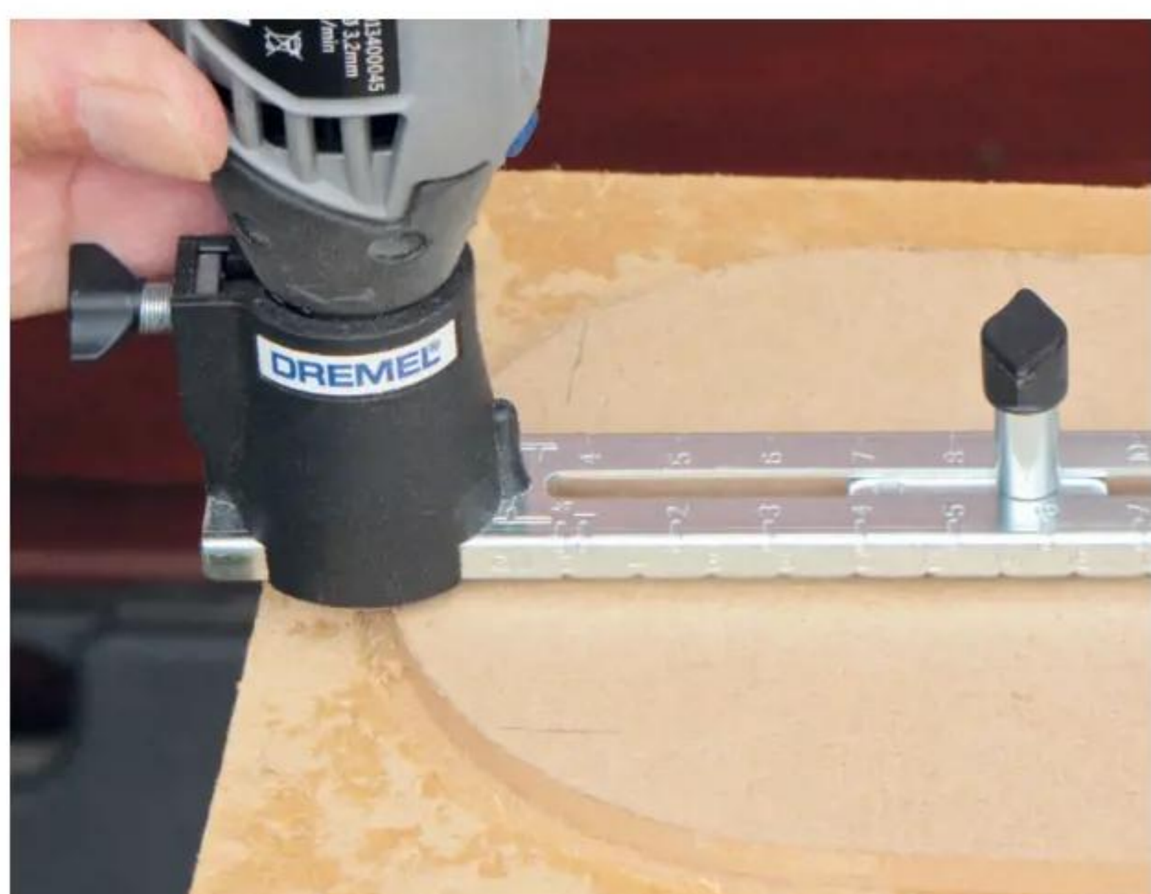
4 Cut out the template curve with a Dremel tool or router and trammel arm; alternatively, use a jigsaw and clean up
