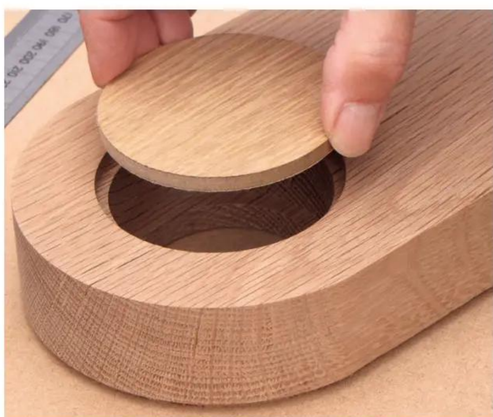
22 Cut the rear cover plate from veneered MDF or hardwood; this is fitted in place with two countersunk brass screws
