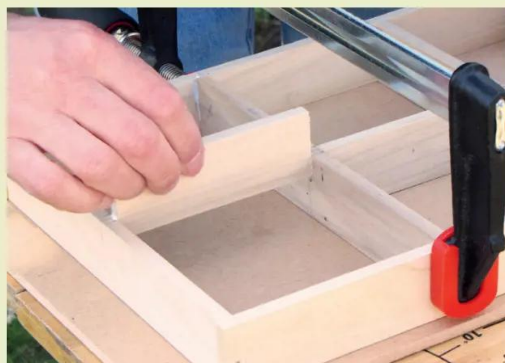
4 Glue ends and slide into place. Nail diagonally down from the adjacent rail where necessary
