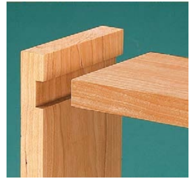
▲ A dado joint can be used to hold a shelf in a bookcase or to join the parts of a cabinet or case.
