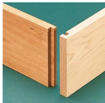
◀ The drawer front and back interlock with the sides using this tongue and dado joint.
