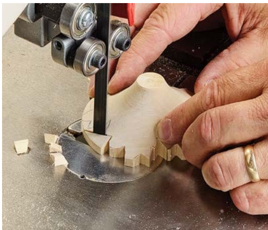
Form Branches. Trace portions of the paper patterns onto the sections. Cut along the lines at the band saw to shape the branches.
