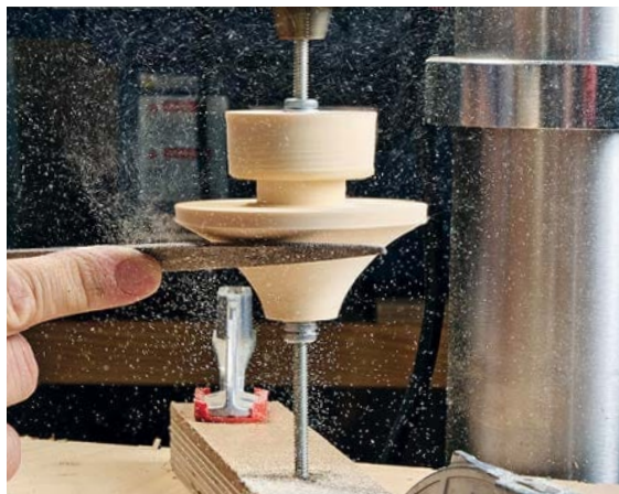
Turn With a Rasp. Capture tree sections on threaded rod with washers and nuts. Shape the profiles with rasps and files.
