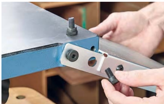
▲ Aluminum extension wings can be flipped out to support longer workpieces. With the wings out, the jointer offers 56" of table length.
