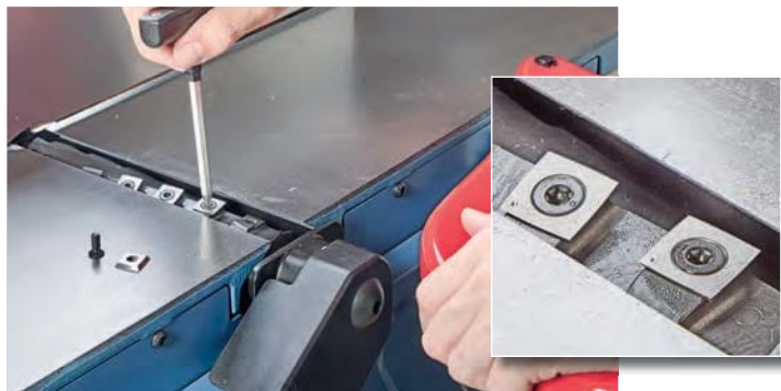
▲ The helical cutterhead of this jointer contains four-edged blades, which can be rotated as they dull. The dots in the corner indicate which sides have been used.
