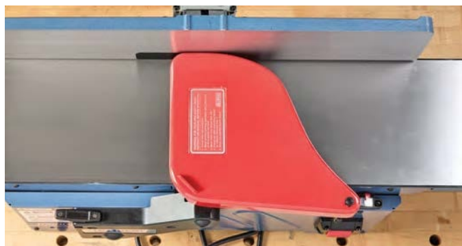
▲ The benchtop jointer offers up to 8" of width, which allows me to face-joint most pieces I work with. The 2HP motor can limit your depth of cut on workpieces that approach the max width.
