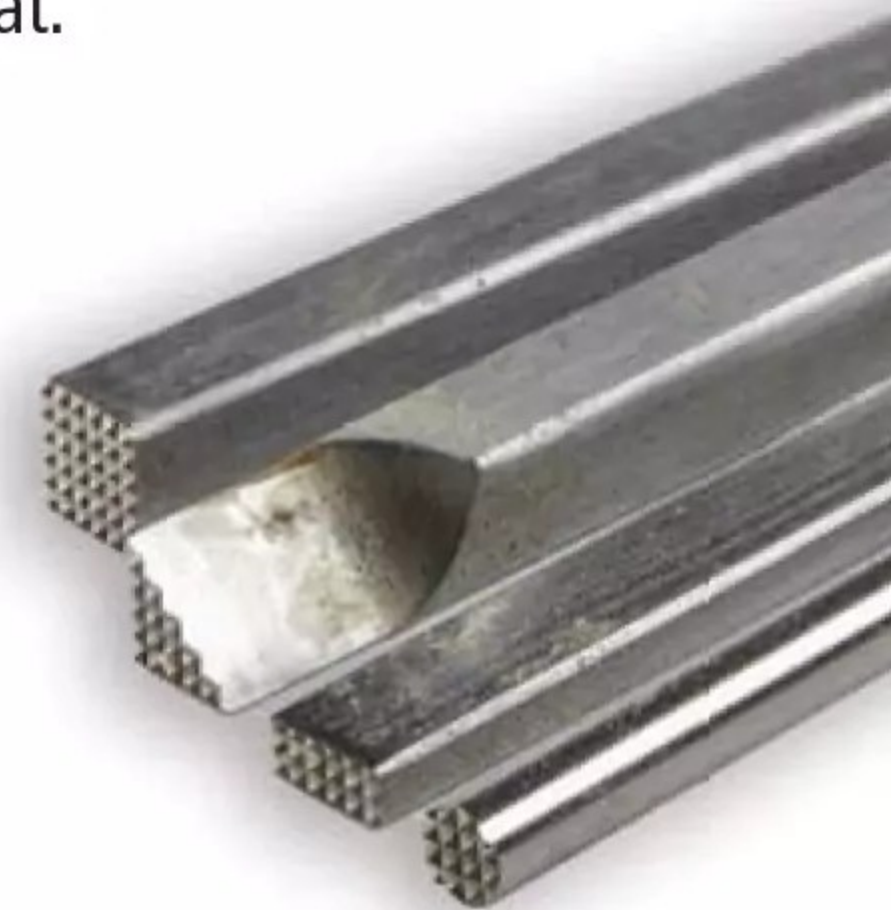
▲ Stamping tools come in a variety of shapes to get in between those tight spaces.
