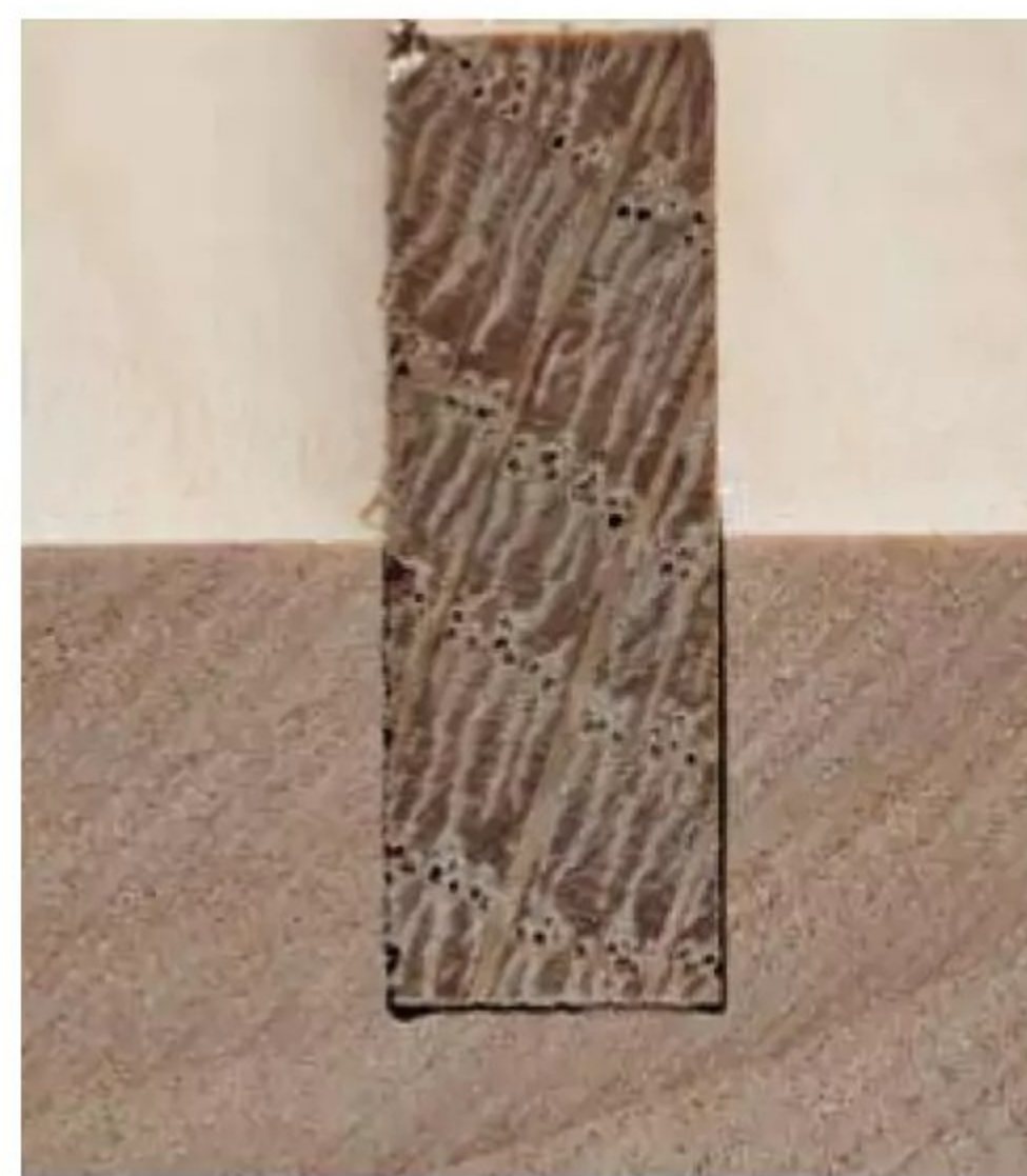
▲ A standard dado blade has bevel-top teeth on its outer blade, which aid in cutting but leave "vampire fangs" in their groove or dado (left photo). By contrast, a flat-top grooving blade can be used to create square-cornered channels (right photo).
