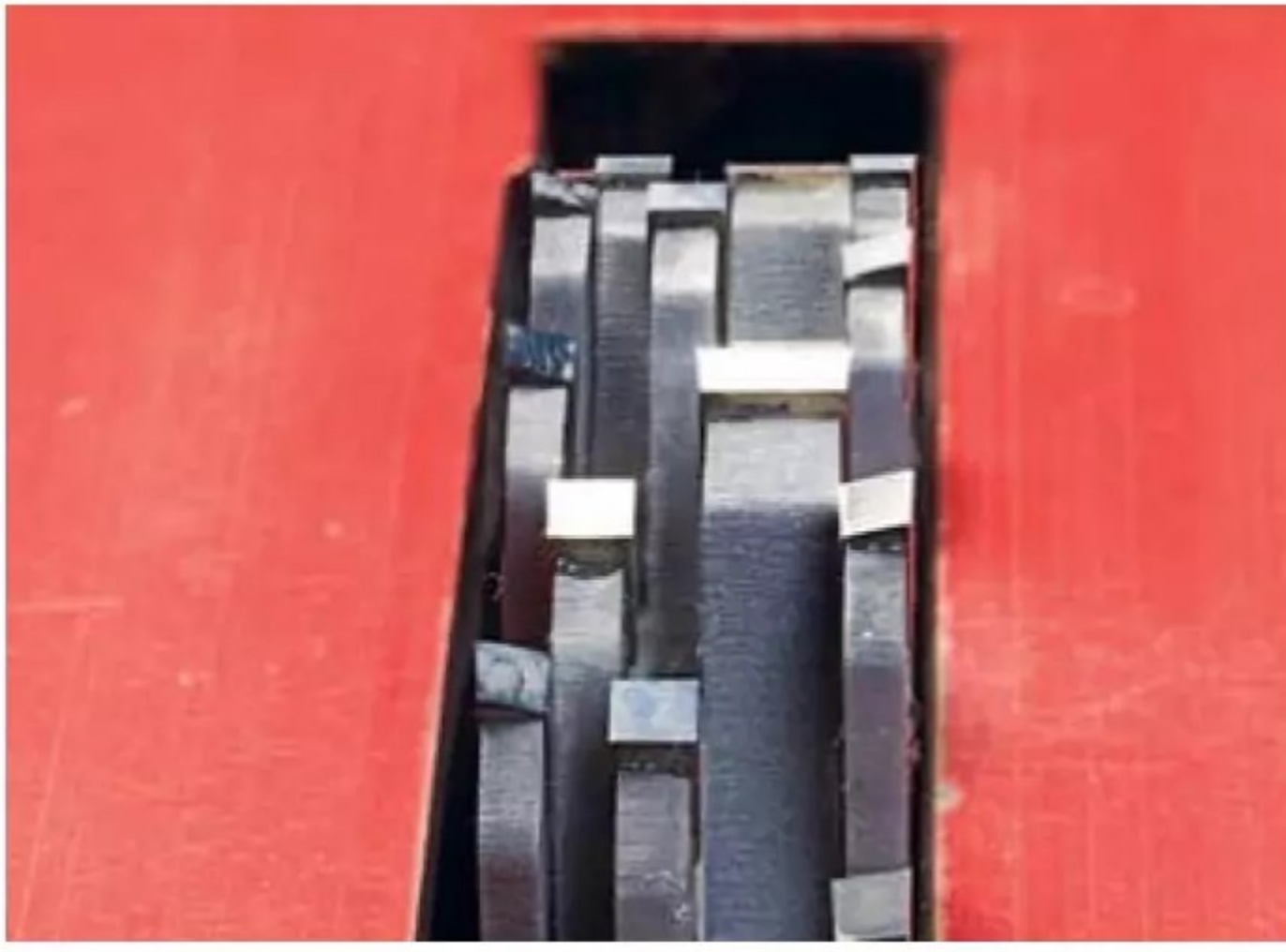
▲ The Ultra-Shear dado set has three sizes of chipper: 1/16", 1/8", and 1/4". This saves on the number of chippers you need to install.
