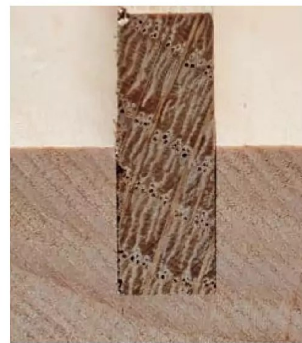
▲ A standard dado blade has bevel-top teeth on its outer blade, which aid in cutting but leave "vampire fangs" in their groove or dado (left photo). By contrast, a flat-top grooving blade can be used to create square-cornered channels (right photo).
