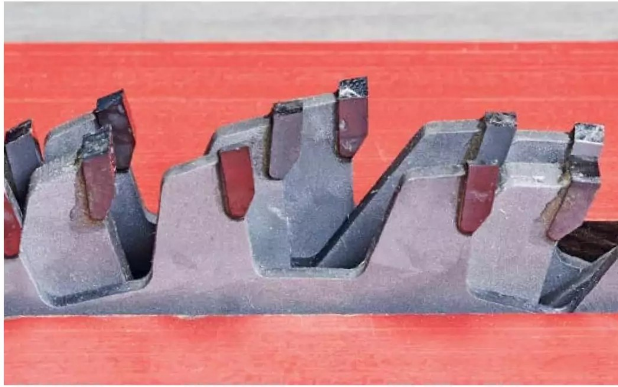
◀ The negative hook angle of the outer blades' teeth helps cleanly shear the sides of a joint, while the positive hook angle and high tooth count of the inner chippers creates a flat bottom.
