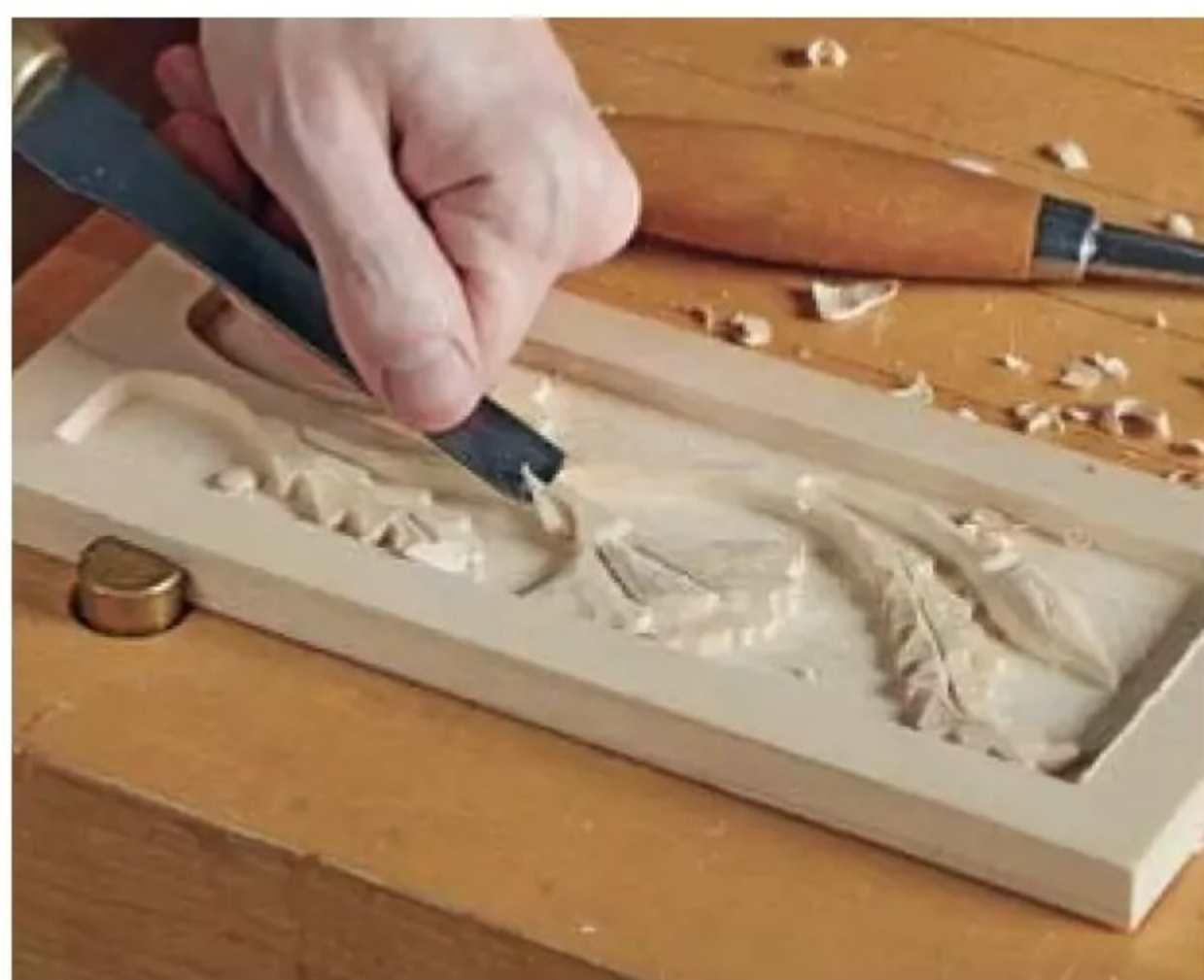
▲ The stem and frame shaping is cut using a combination of the #3 x 1/2" gouge and knife.
