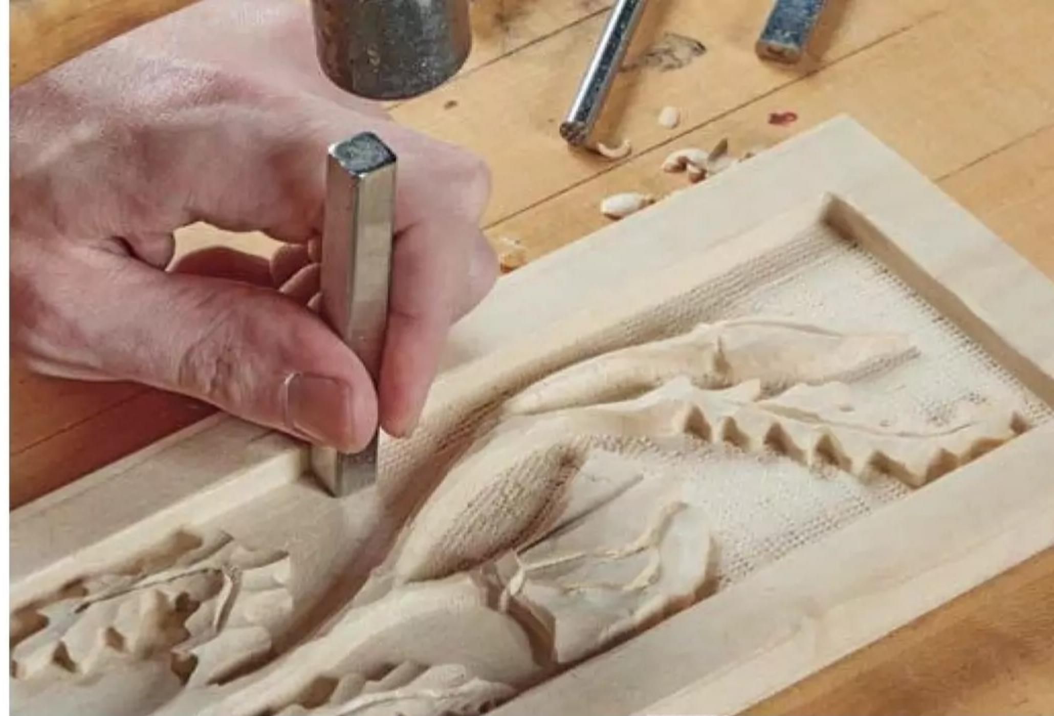
▲ Working from one end to the other, I struck the stamp, then repositioned it being careful to not overlap the previous impression. Rinse and repeat.
