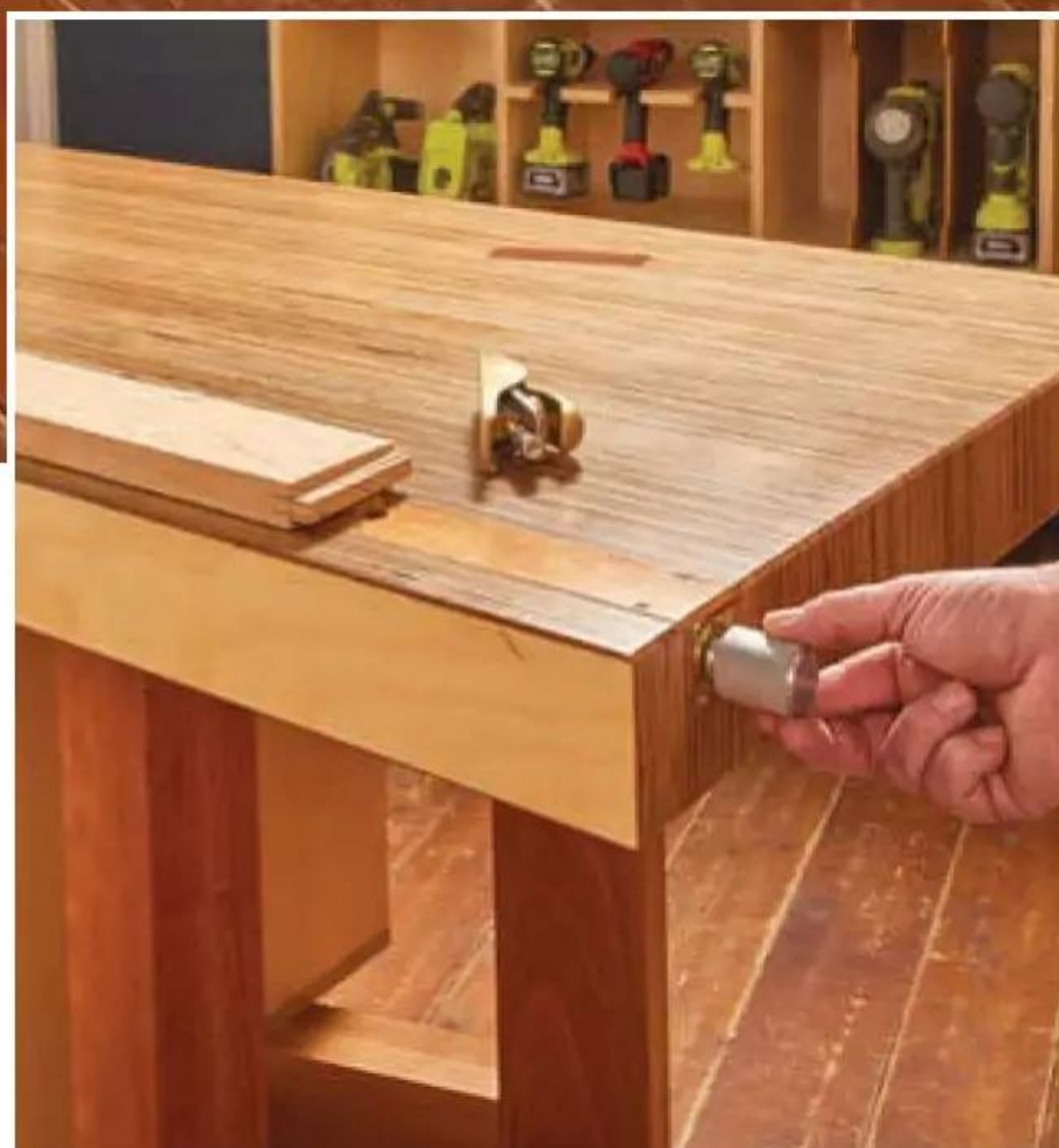
▲ Tail Vise. The knurled knob of this tail vise makes it easy to tighten and loosen pieces held in the dogholes.
