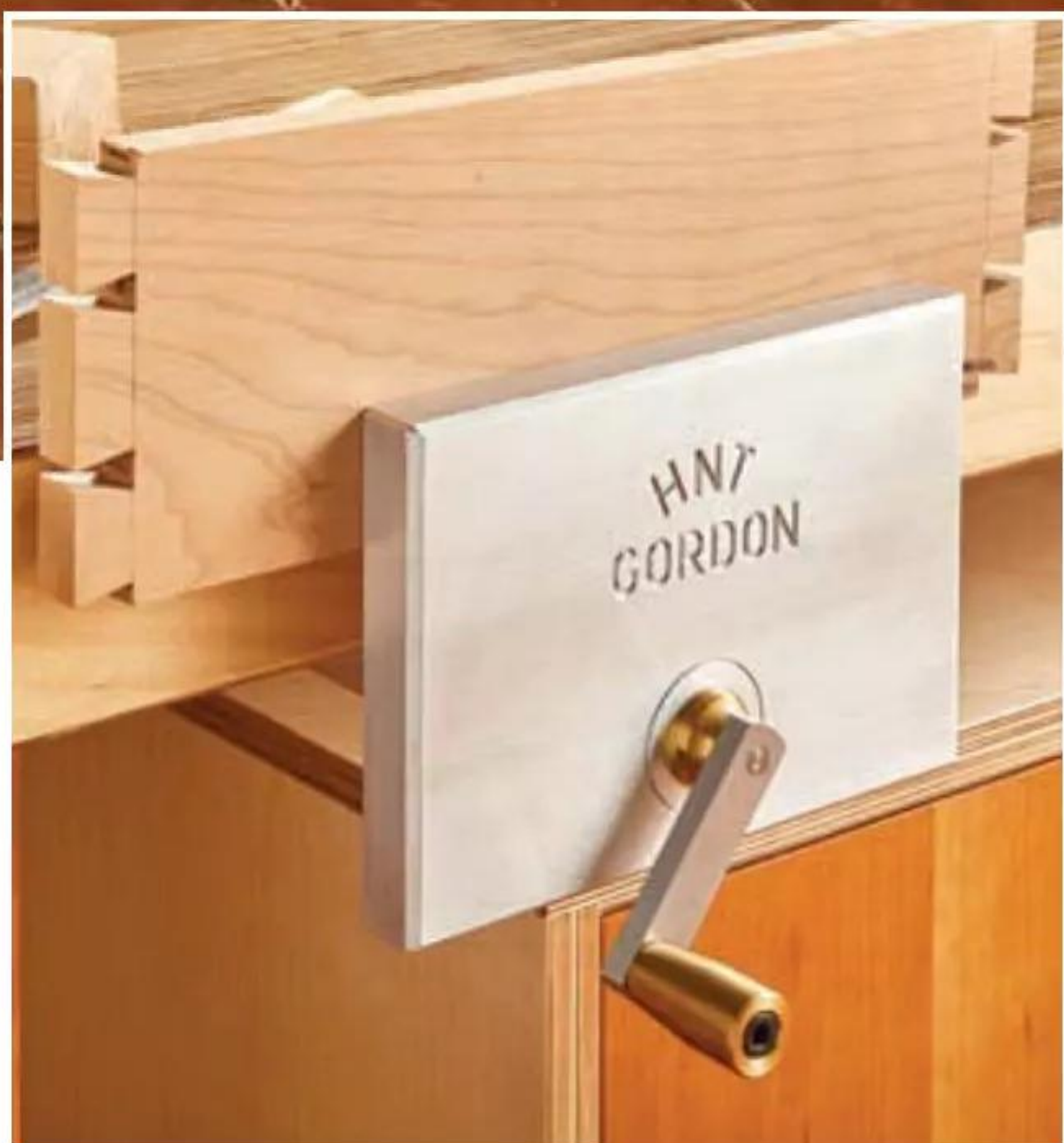
▲ Face Vise. A face vise made from machined aluminium provides a strong grip without marring the piece.
