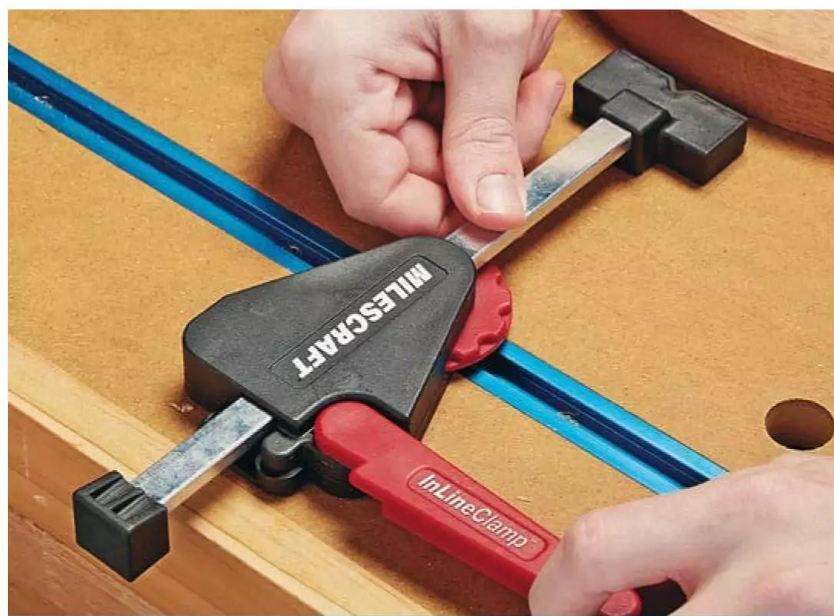
▲ These InLine Clamps are a versatile option. The screw secures them in the T-track while the cam lever locks the workpiece in place.
