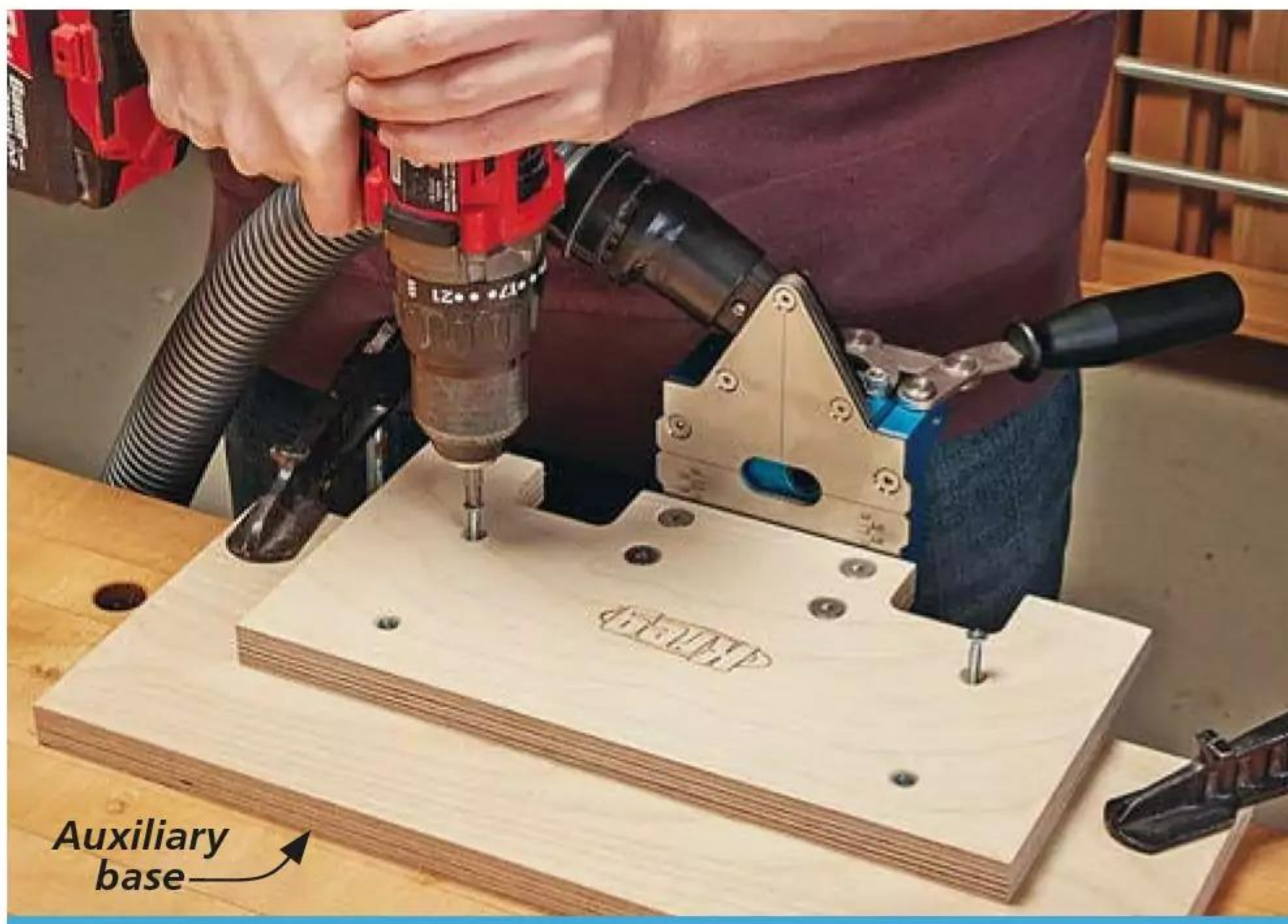
▲ Attaching an auxiliary base to main base allows for more options when clamping the jig onto your workbench.
