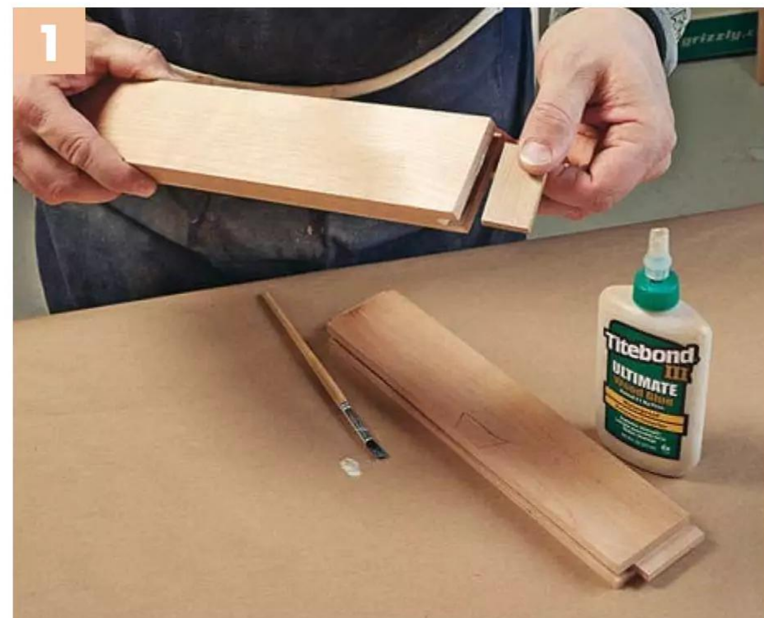
▲ Apply glue to the slot on the end of the rails and insert the spline. Allow the glue to set up before proceeding.
