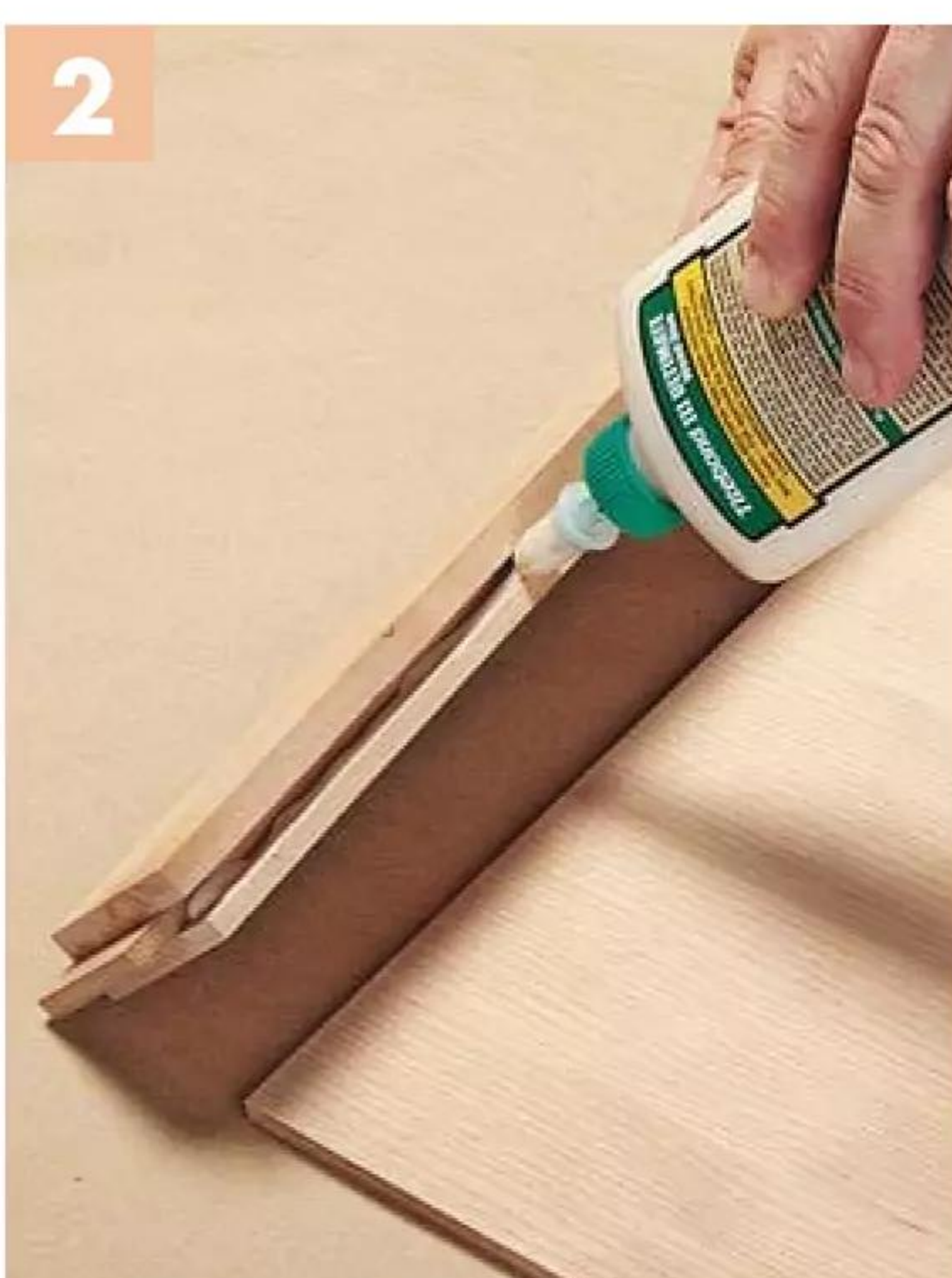
▲ Run a bead of glue into the grooves in the two rails then fit them over the ends of the panel.
