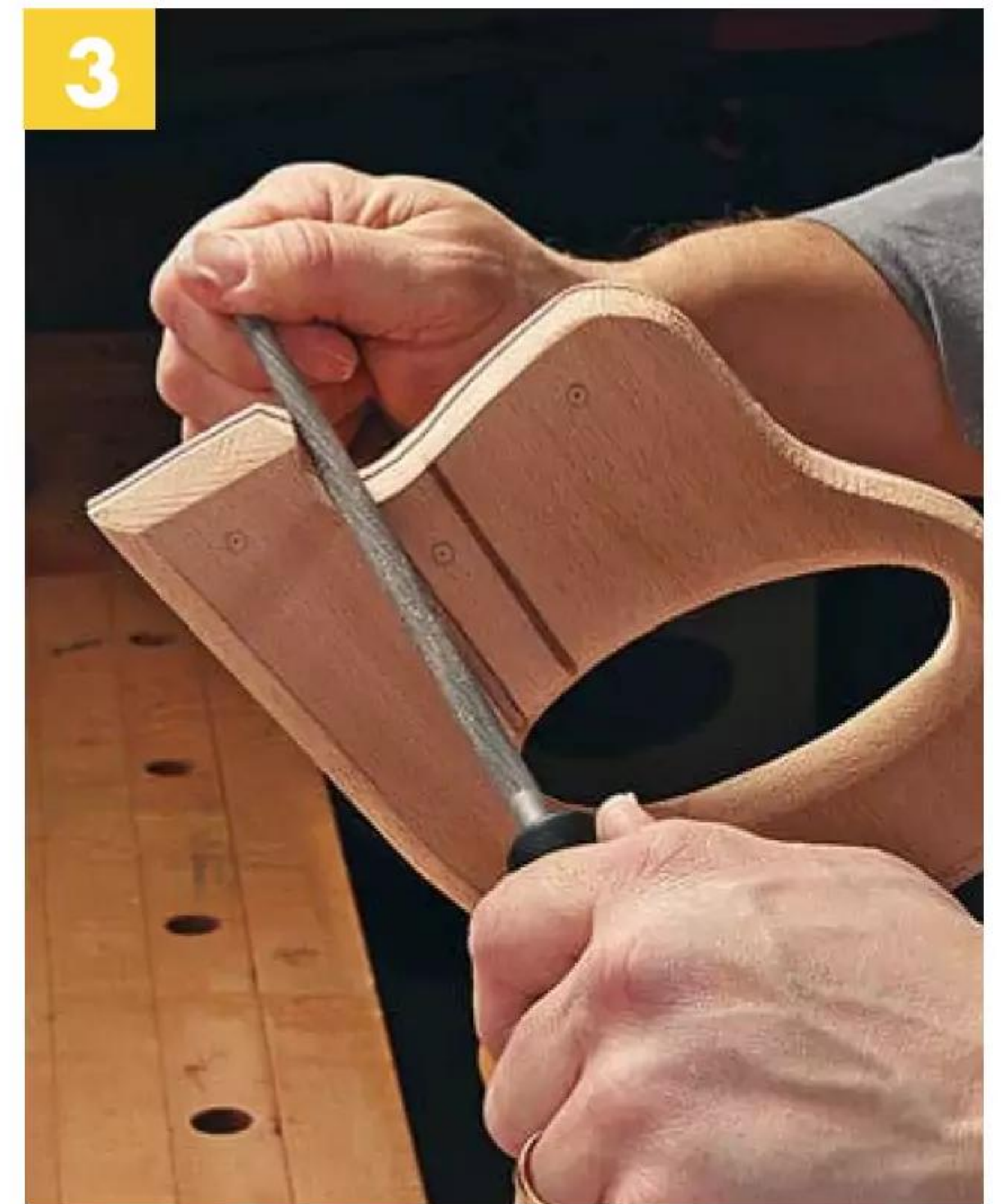
▲ A round file tucks into tighter curves than the half-round file.
