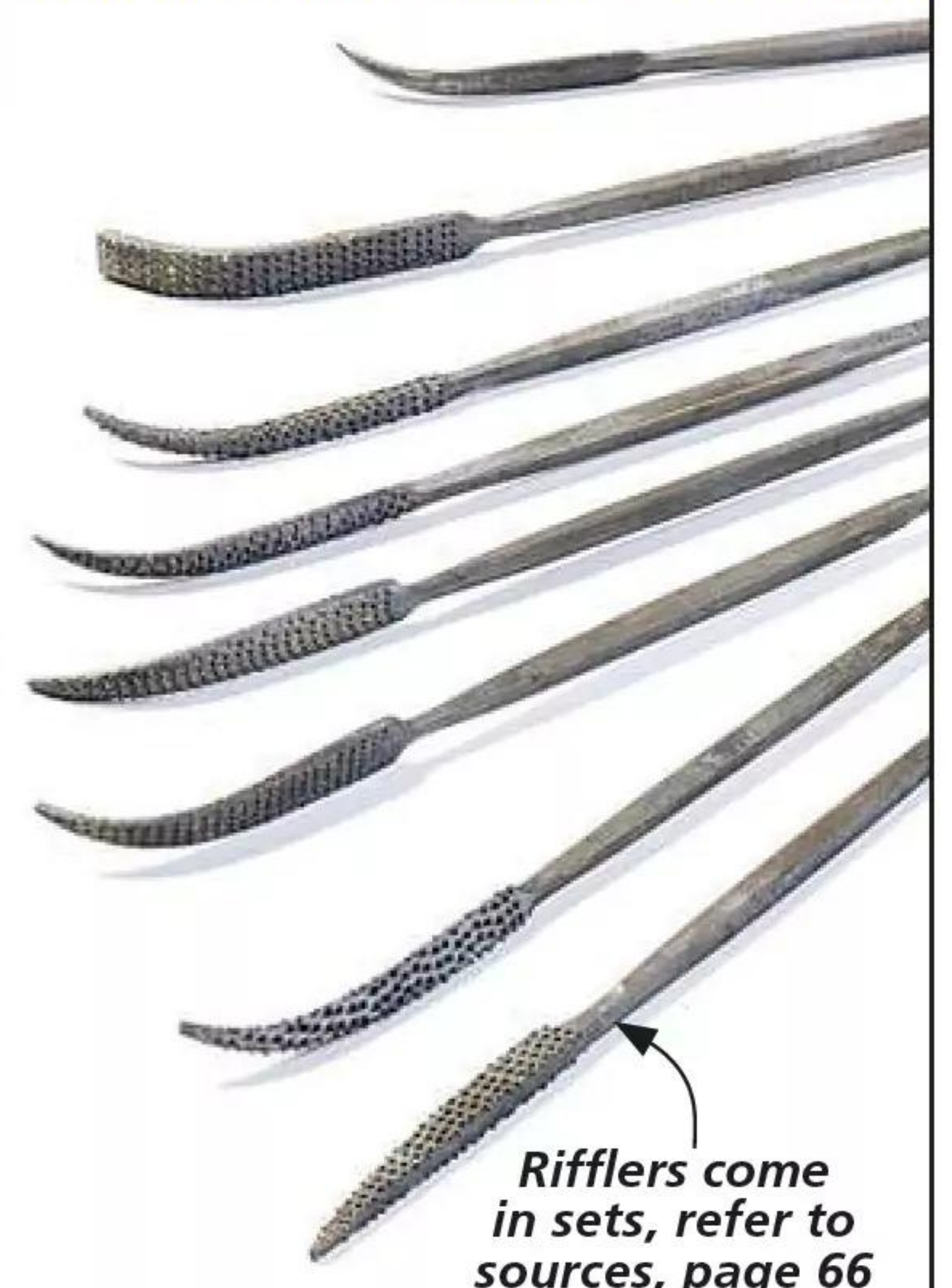
Blending. Rifflers work best in tight spaces to shape surfaces and ease transitions from adjoining sections.
