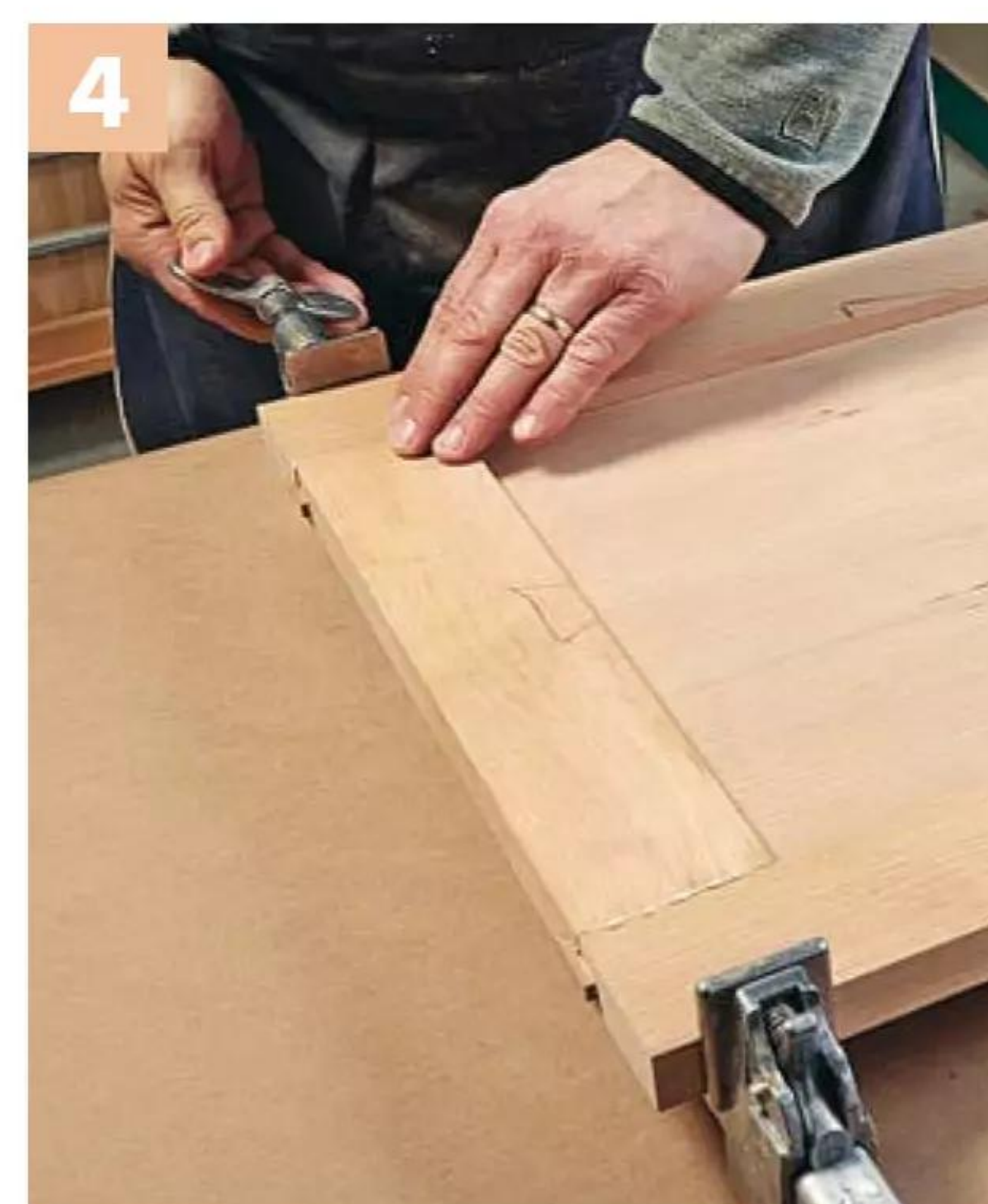
▲ Draw the clamps tight to close up the joints. Trim the exposed splines flush after the glue dries.
