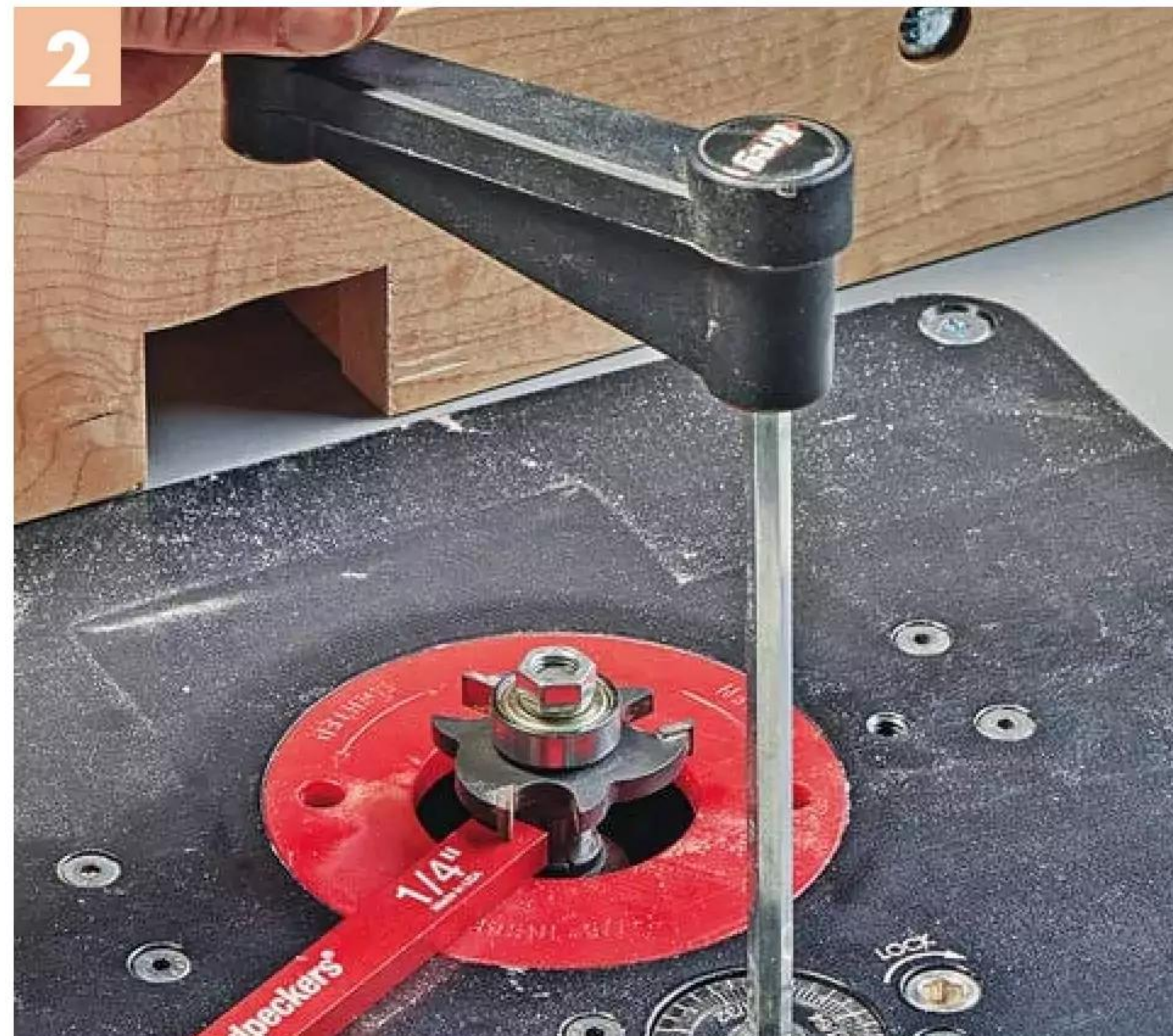
▲ Setup blocks offer a physical reference point for setting router bits to the correct height.
