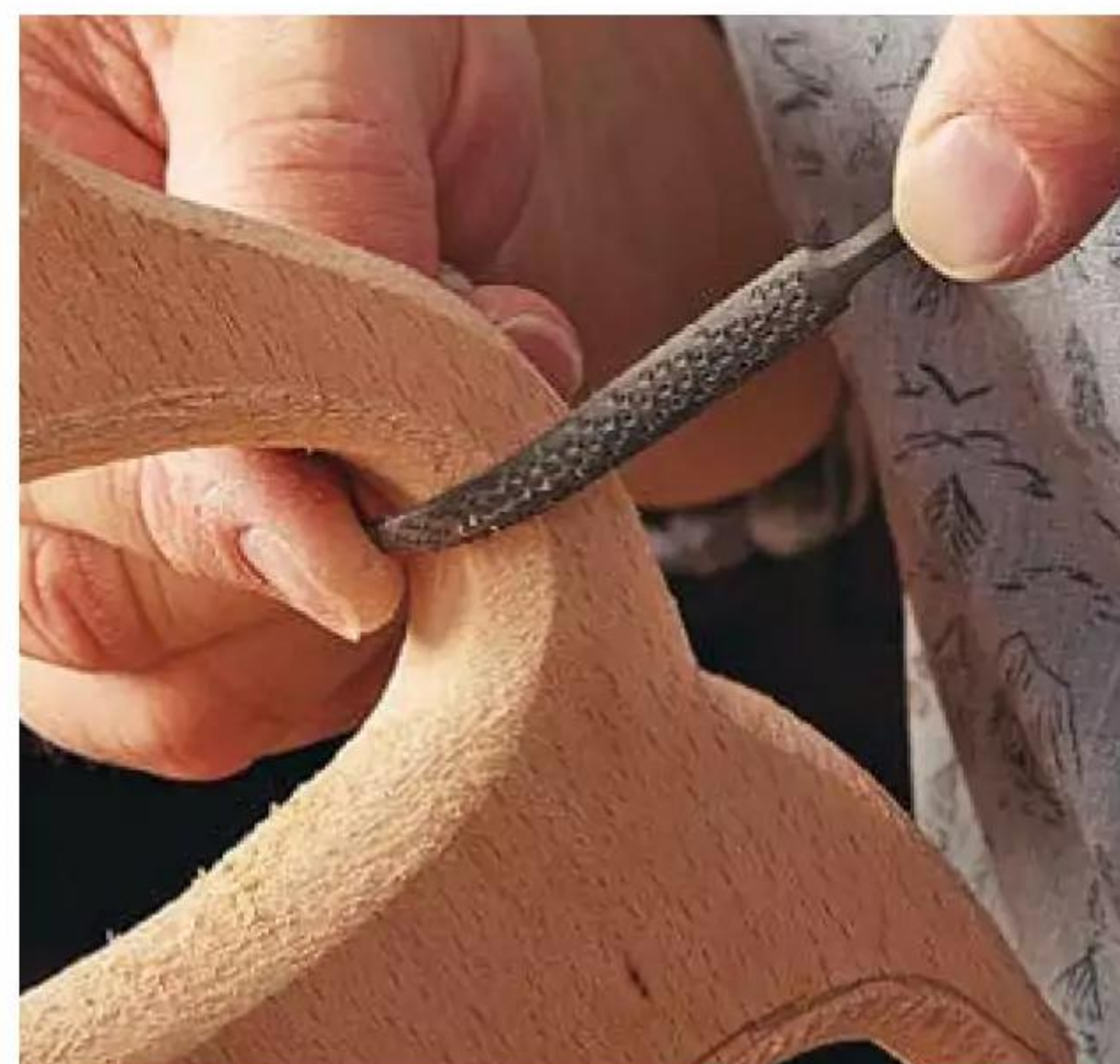
Blending. Rifflers work best in tight spaces to shape surfaces and ease transitions from adjoining sections.
