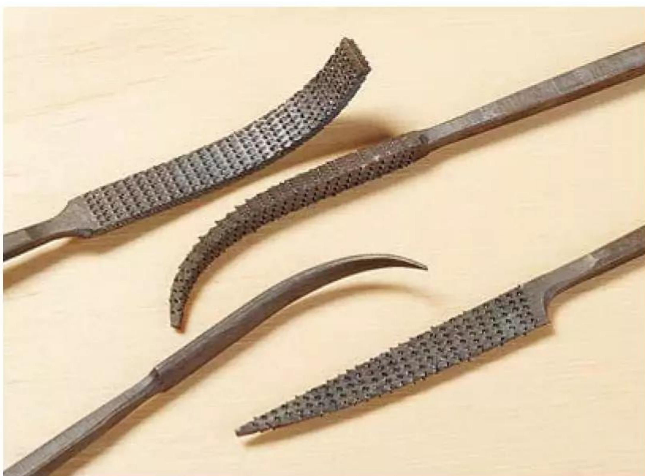
One of Each. The blades on rifflers feature rasp or file teeth on curved surfaces with flat, round, triangular, or square cross sections.
