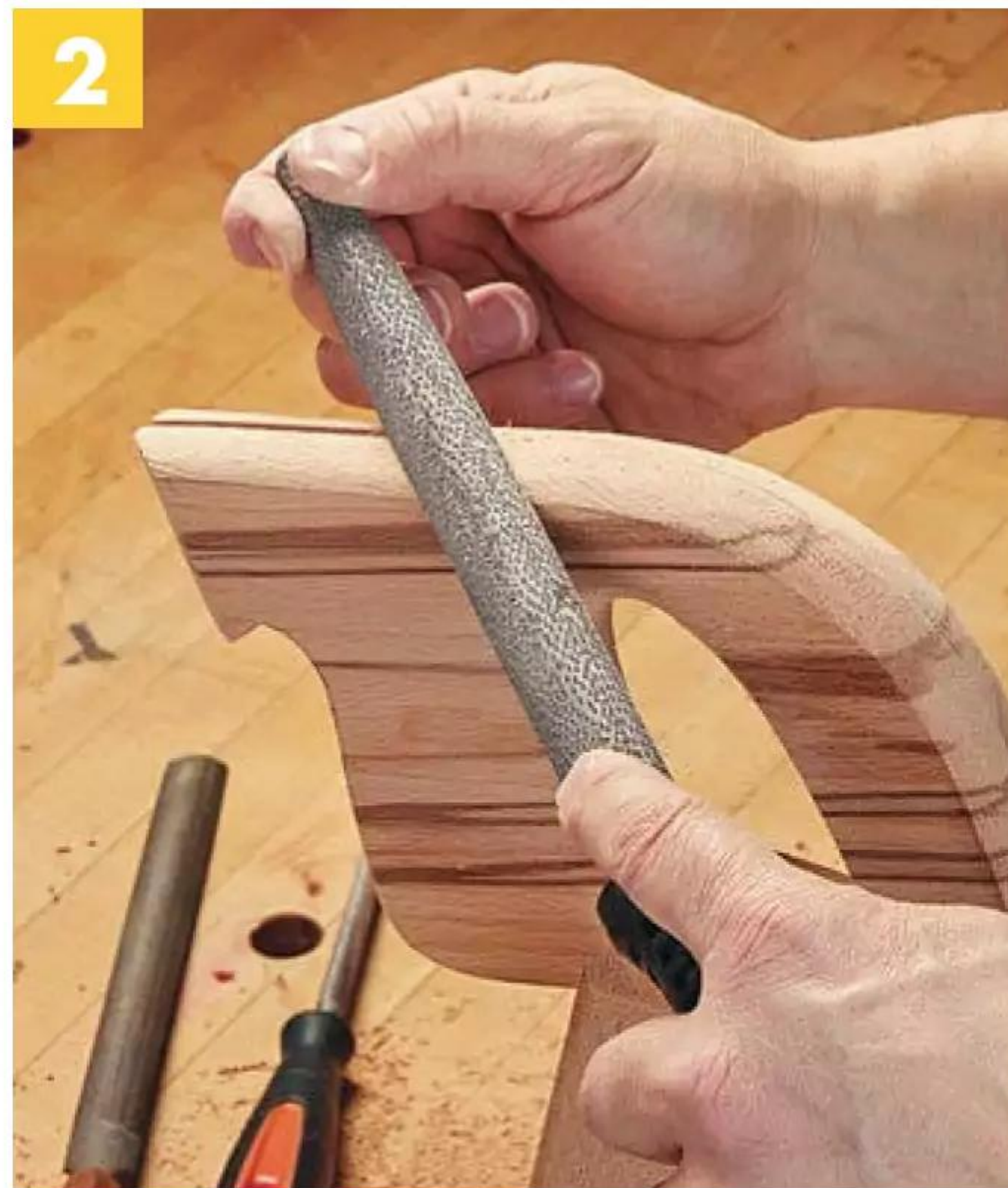
▲ A finer rasp (then a file) are used to refine details and remove tooth marks.
