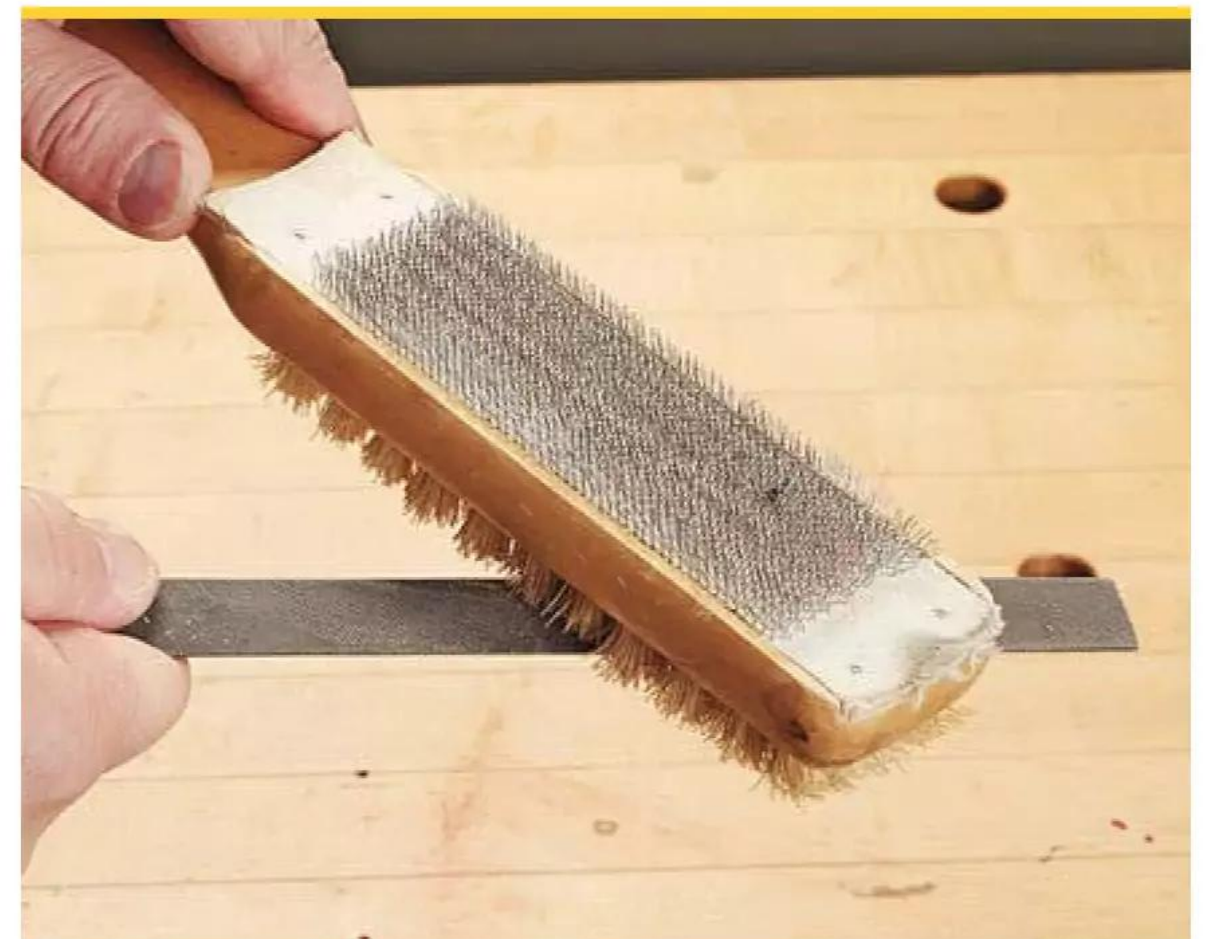
▲ A file card has fiber bristles on one side and wire bristles on the other to keep files and rasps clean.
