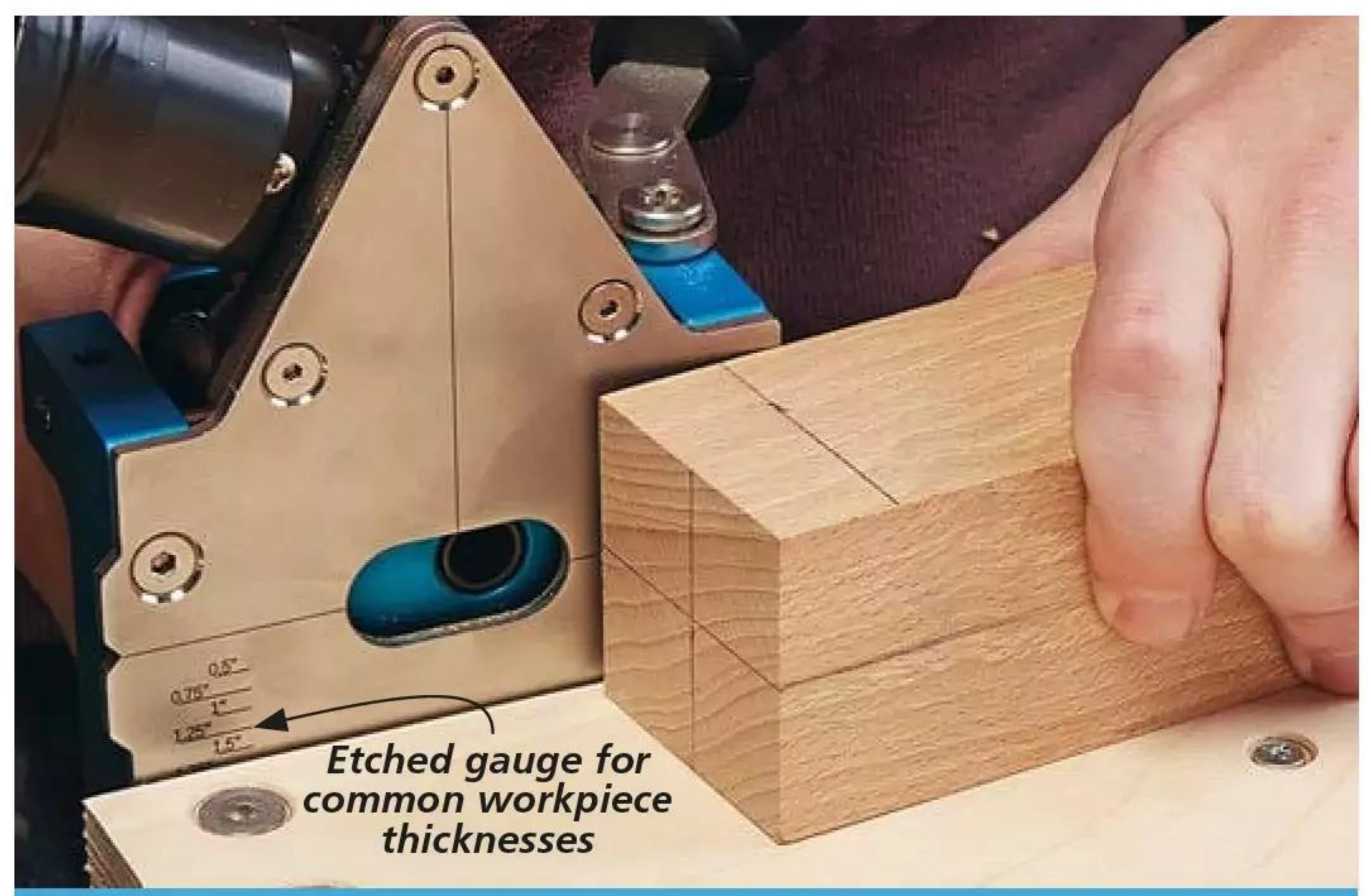
▲ To locate the mortise, align the jig's centerline with marked lines on one of your workpieces. Or you can use the built-in gauge.
