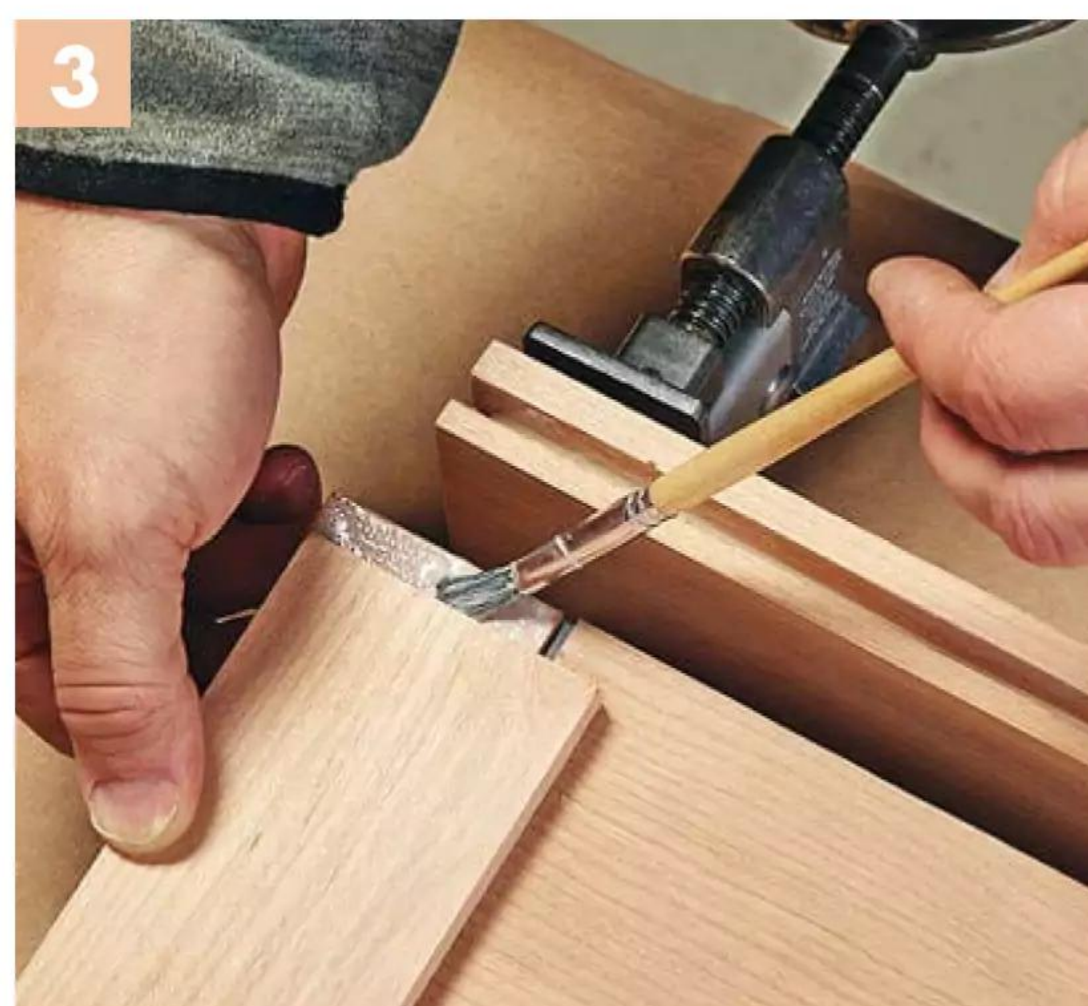
▲ The final step in the process is to bring in the stiles. After brushing glue onto the exposed splines, add more glue to the groove in the stiles.
