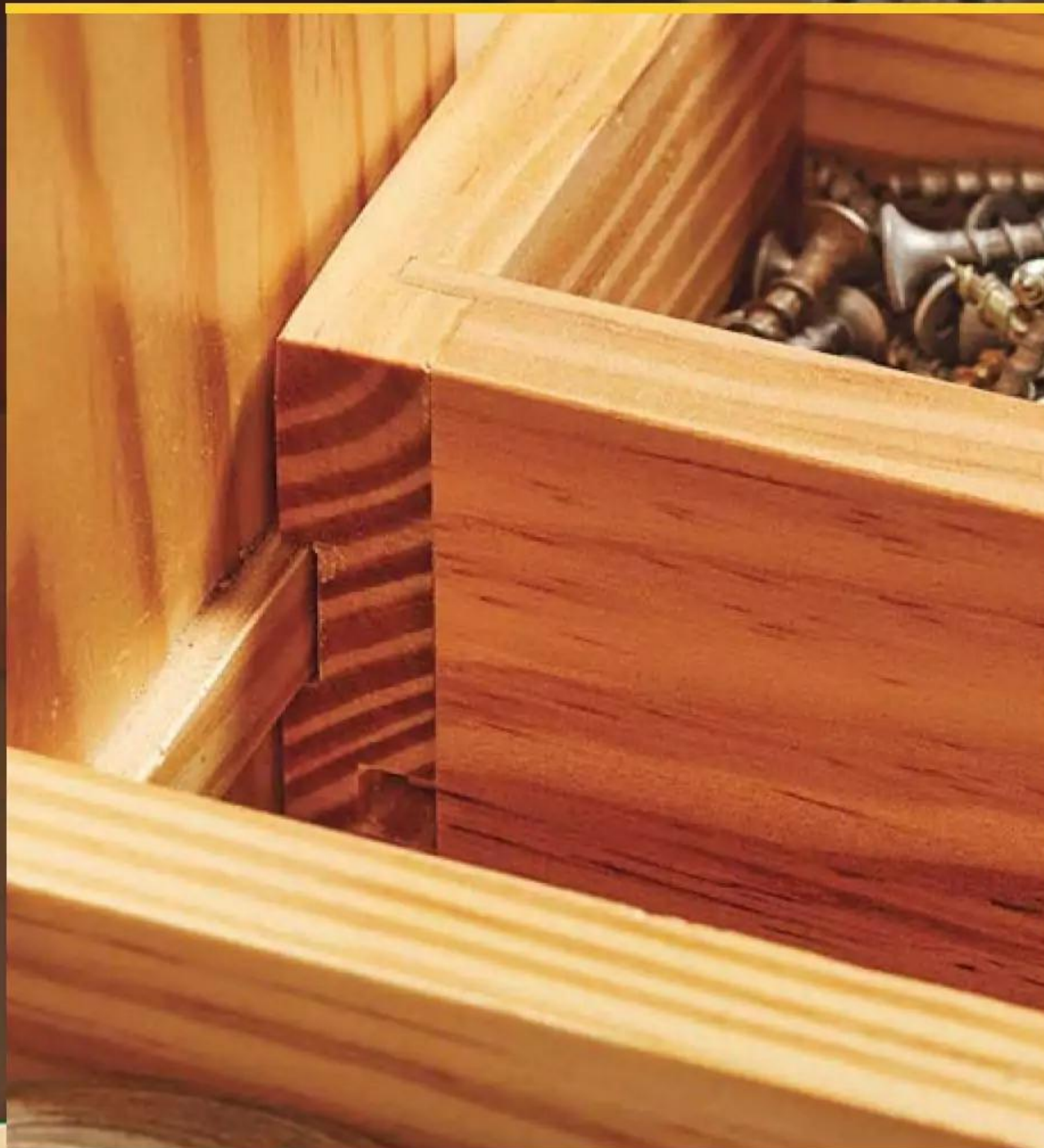
▲ Wood runners support a drawer with tongue and dado joinery, making for simple yet effective storage for smaller pieces of hardware like screws and washers.
