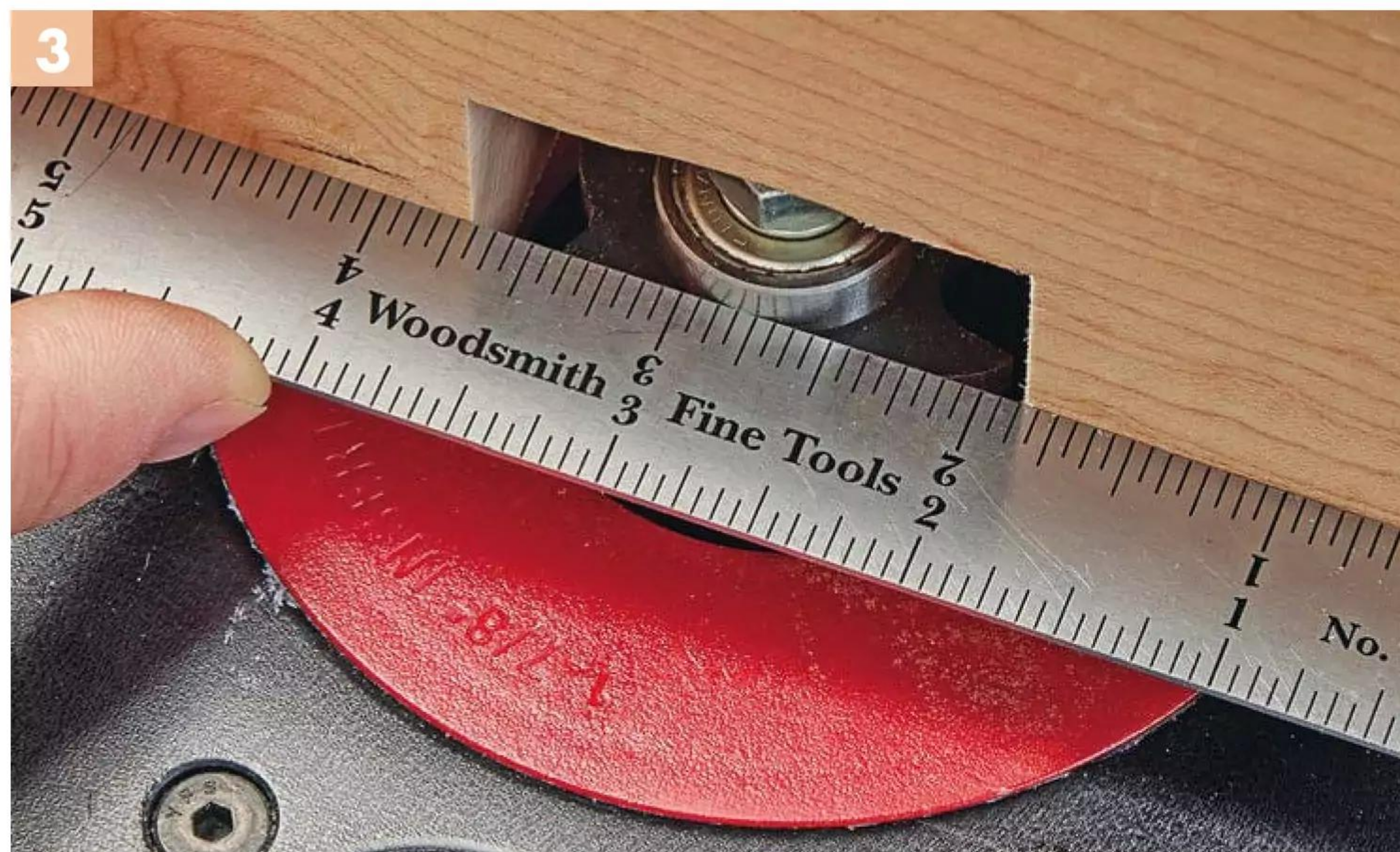
▲ Using the router table fence along with the bearing on the bit provides a smooth entry and exit of the workpiece as it is cut. A steel rule helps you see when the two are aligned.
