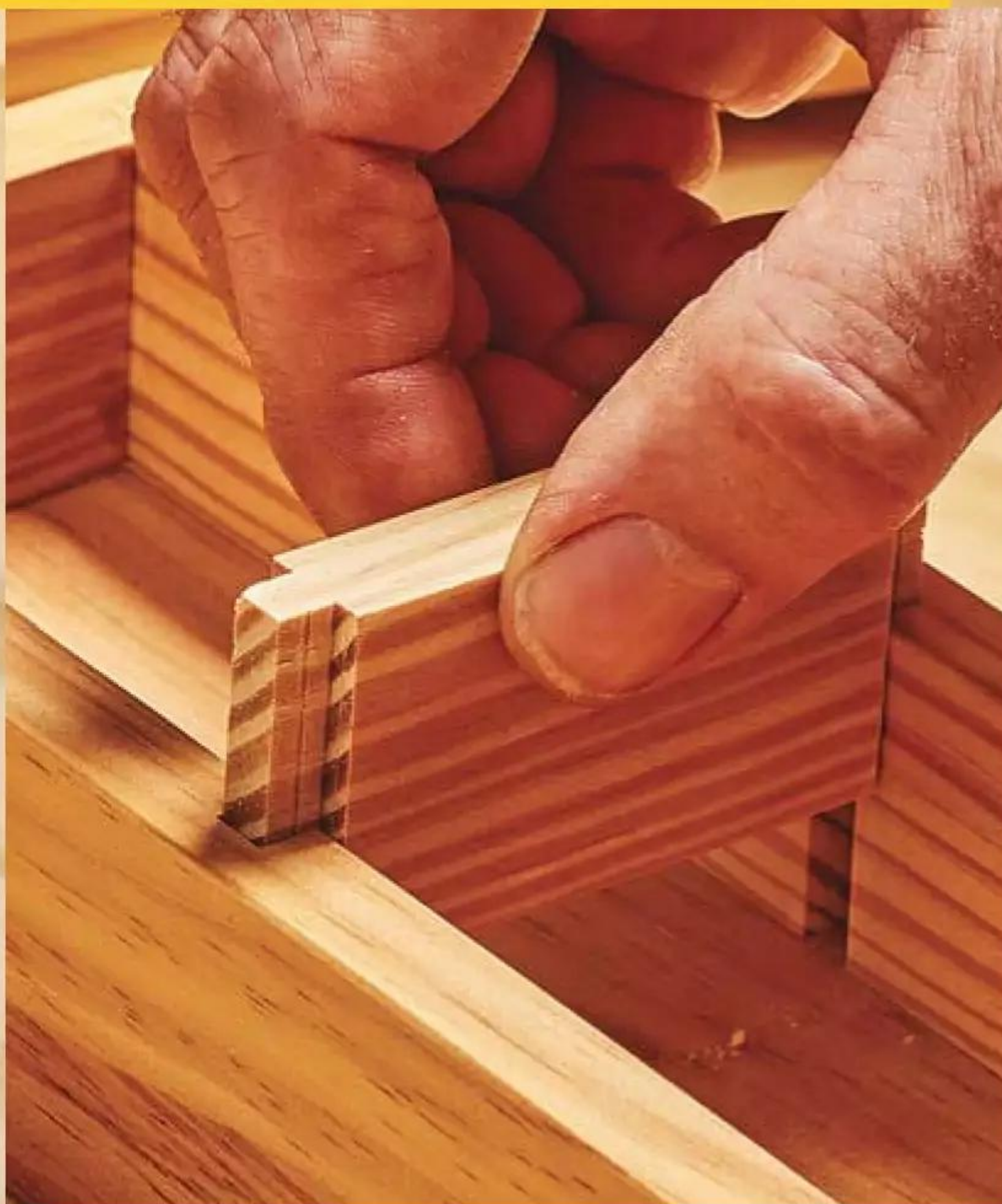
▲ Dividers slot into dados without glue, allowing you to adjust the size of the tote's cubbies for large or small tools as needed.
