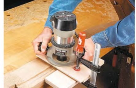
Groove Jig. This simple jig from Woodsmithspecials.com makes routing the groove on the underside of the bent arm easy.
