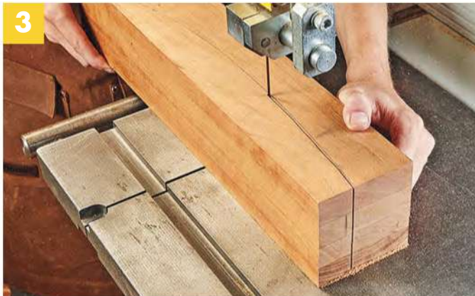
▲ Tape your cutoff back on for support when making the second cut. A few pieces of double-sided tape secure the workpiece and cutoffs.
