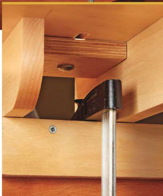
▲ A system of braces and cleats elevates the top and allows it to be secured with clamps.
