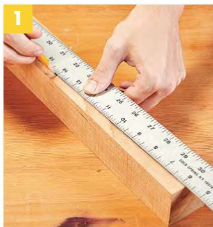
▲ Lay out the start and end points of the taper, then connect them. Transfer these lines across the end for visibility.
