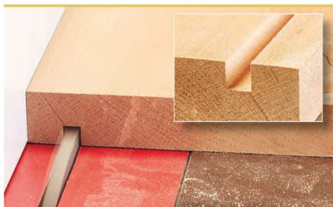
▲ With flat-topped teeth, the grooving blade plows a crisp channel along the length of hardwood and plywood.
