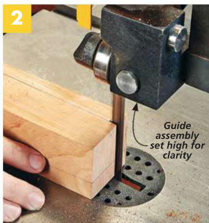
▲ Set the guide assembly 1/4" above the workpiece. Begin the cut from the narrow end of the taper for the best results.
