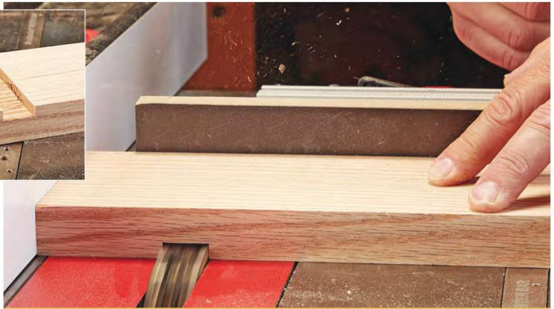
▲ A zero-clearance insert and an auxiliary miter fence keep tearout at bay while cutting dados in hardwood.
