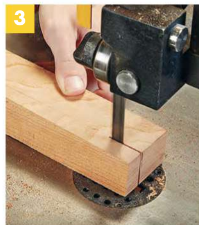
▲ Finish the taper with the second cut. Smooth, steady cuts will get you the best results here.
