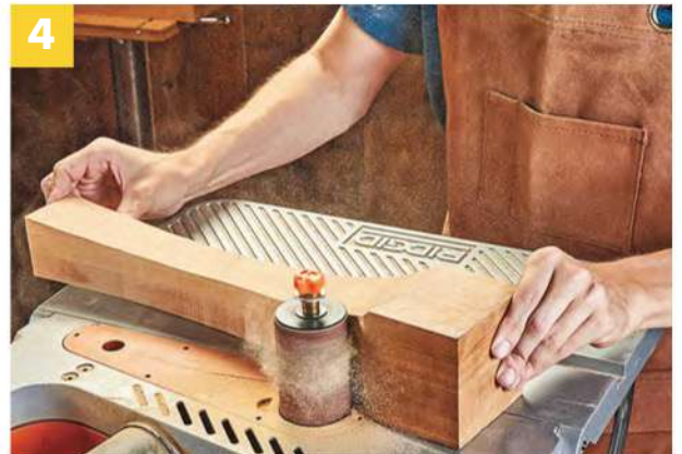
▲ Finish out the shape of the curves at the spindle sander. Long, even motions will make for smooth, elegant curves.
