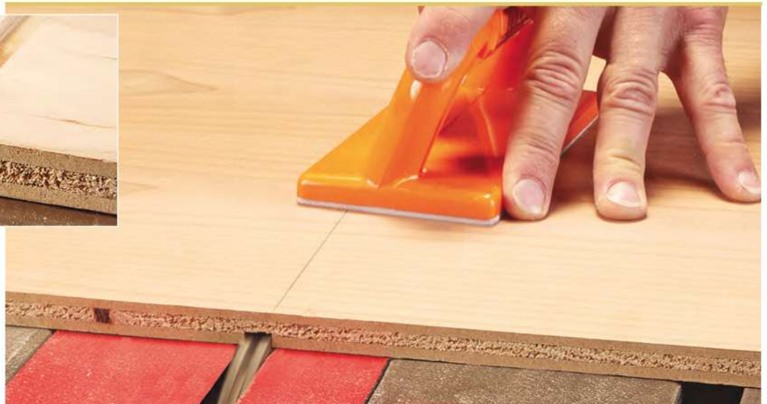
▲ Push pads distribute pressure for an even depth of cut across wide plywood panels.
