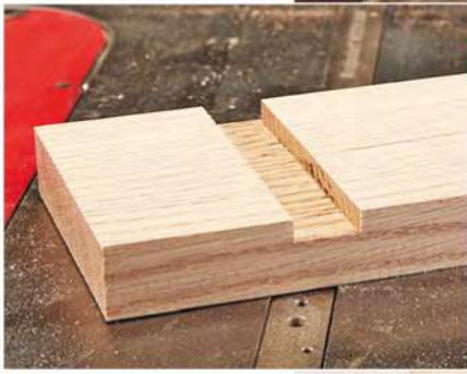
▲ A zero-clearance insert and an auxiliary miter fence keep tearout at bay while cutting dados in hardwood.
