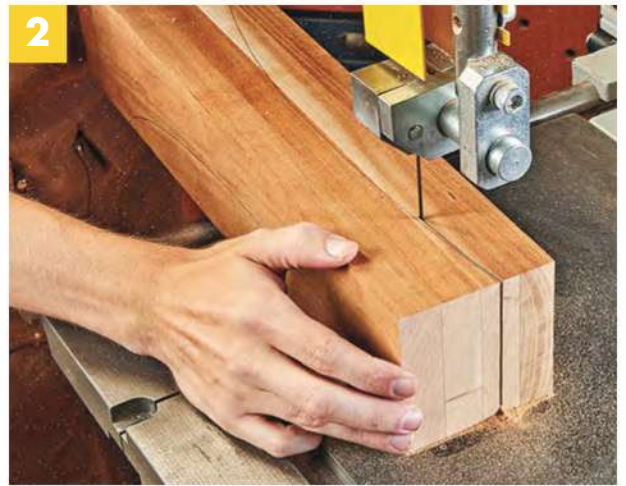
▲ Make the first cut in one, even go. Getting close to your layout lines is ideal, but be sure to stay on the waste side.
