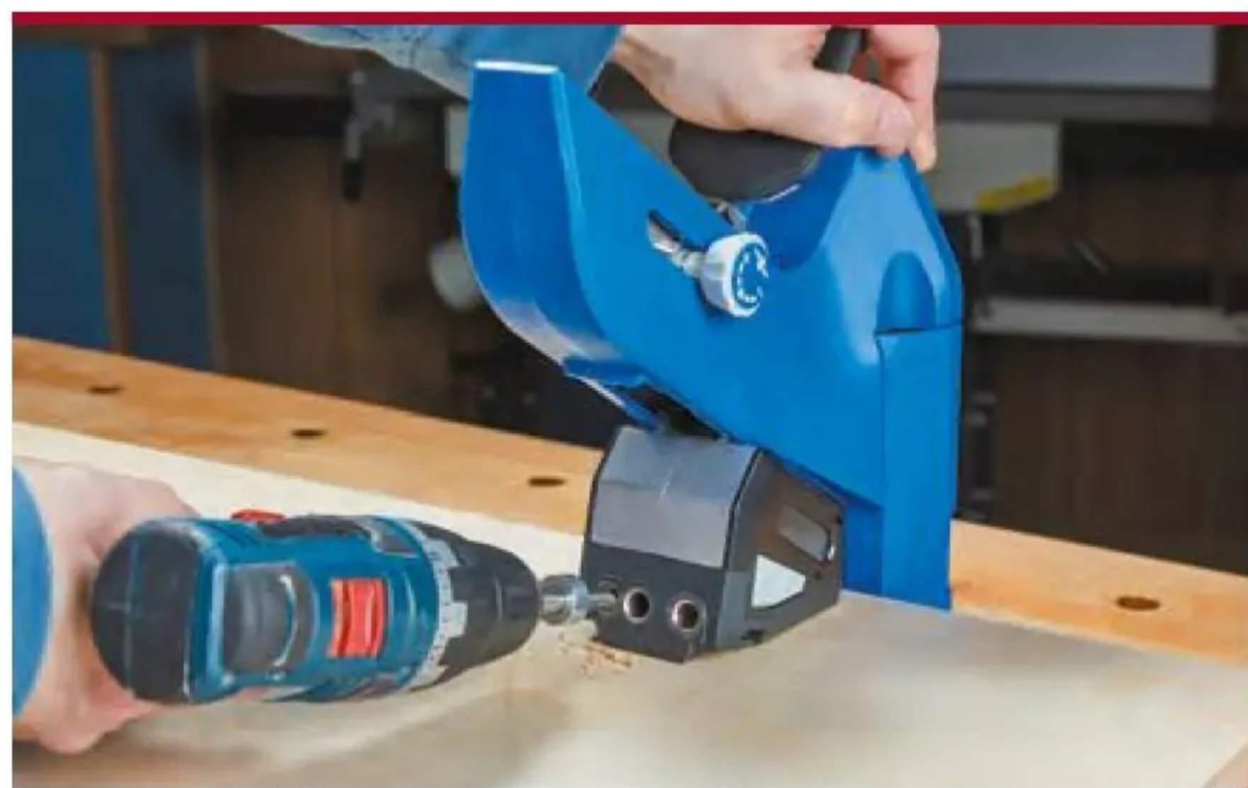
▲ The Kreg 720 pocket hole jig clamps to plywood panels while lying flat. This means you don't have to balance large pieces on edge while drilling holes.
