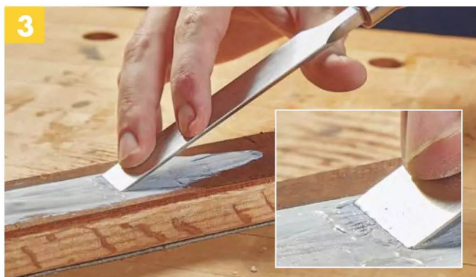
3 Pull the chisel back across the strop to hone the edge. As you repeat the action, it'll get easier to find the bevel angle quickly. If you hone consistently, ten to fifteen passes should be sufficient.
