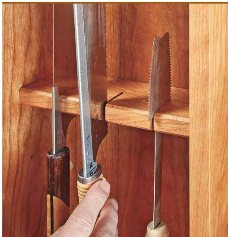
▲ Kerfs cut in the central shelf provide clearance for saw blades, holding them upright and keeping the teeth safe.
