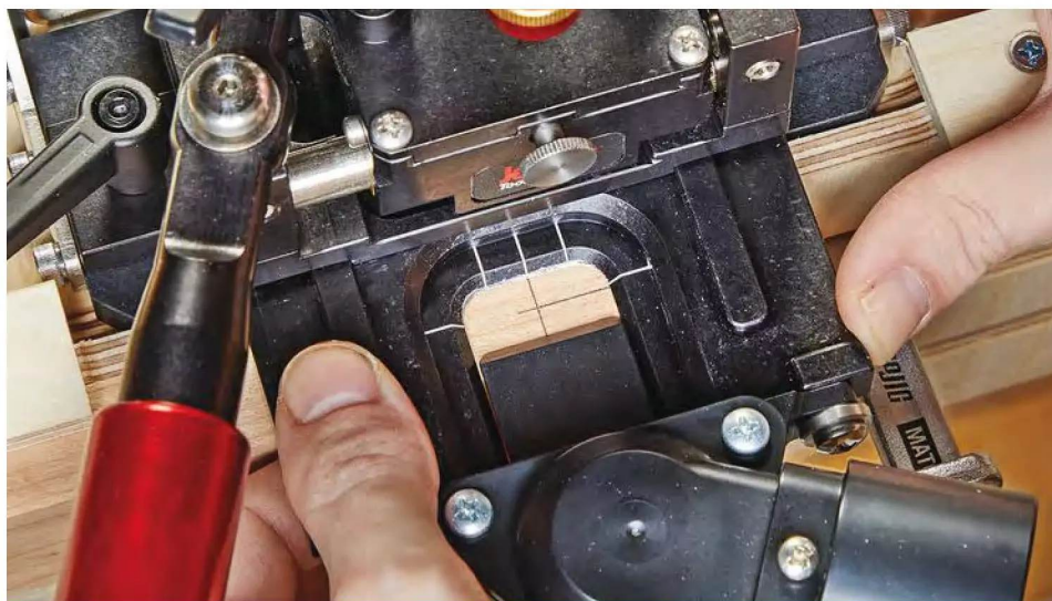
▲ The base of the mill has a locating guide that slides and locks to accommodate pieces of various thicknesses. It shows the centerpoint and ends of the mortise. Once it's been set, the carriage slides in overtop.
