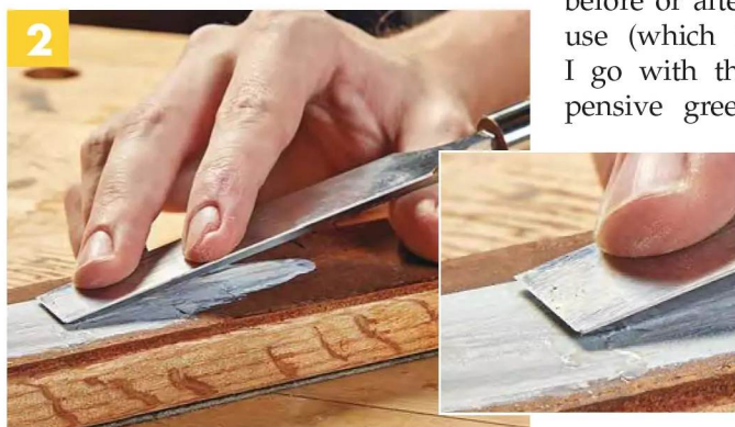
2 Begin by laying the chisel down with the edge raised, resting on the crest of the bevel. Lightly press the tip of the chisel down until you feel the bevel making full contact with the strop.
