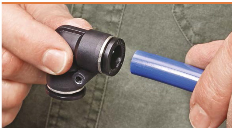
▲ To install the tubing simply push the squared-up end into the fitting until it's firmly seated. Teeth inside the coupling holds the tubing in place.
