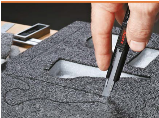
▲ A utility knife with a narrow blade works best to cut through the foam and follow the tool's profile. Stay to the inside of the line for a snug fit.
