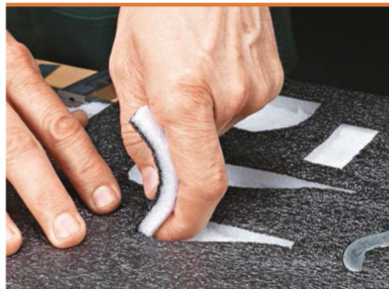
▲ Dig your finger down to the desired depth, then work to peel back the foam. Flip back and pull away additional layers until the tool sets flush to the surface.
