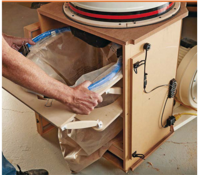
▲ Changing out dust bags couldn't be simpler. Remove the hatch door and slide out the catch container by grabbing the upper layer and sliding it out off the rails and down. Replace the bag and slide the container back in place.
