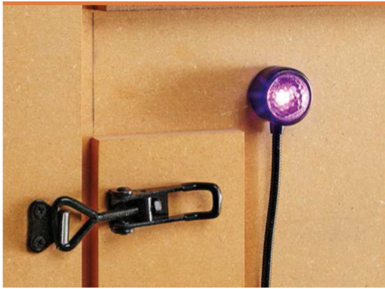
▲ The latch provides an air-tight grip for the hatch door of the collector. The light of the DC Guard Dog comes on to let you know it's time to empty the bag.
