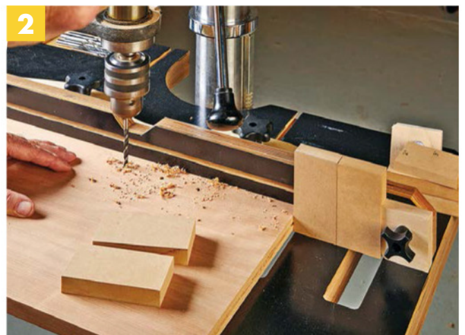
▲ Drill a hole, remove a spacer, and slide the workpiece down. That's all it takes to drill as many holes as you need. You can repeat this process on any number of parts.
