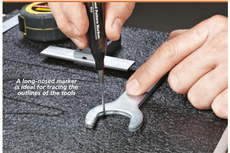
▲ Once you have the tools placed to your liking on the foam, trace their profile on the surface of the Kaizen Foam with the marker you see here.
