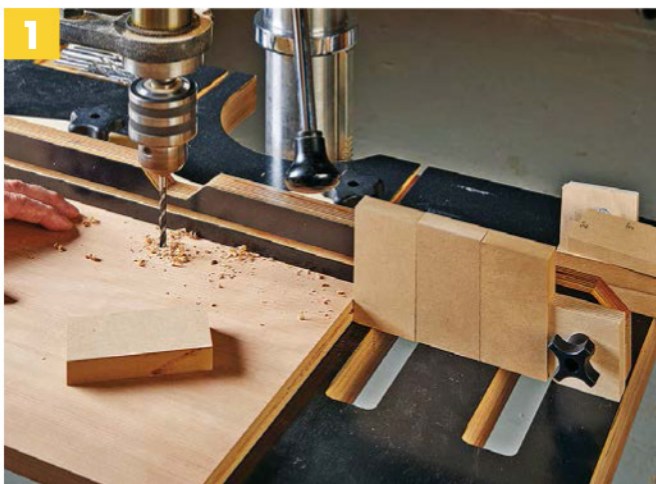
▲ When you need to drill shelf pin holes in case parts, consistent spacing is critical. Set up a stop block on the fence then add multiple spacers that match the hole spacing you require.
