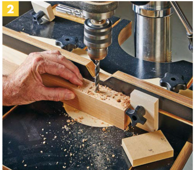
▲ Hold the workpiece against the spacer to drill out one end of the mortise (left photo). Remove the spacer and shift the piece against the stop block to drill out the other end.
