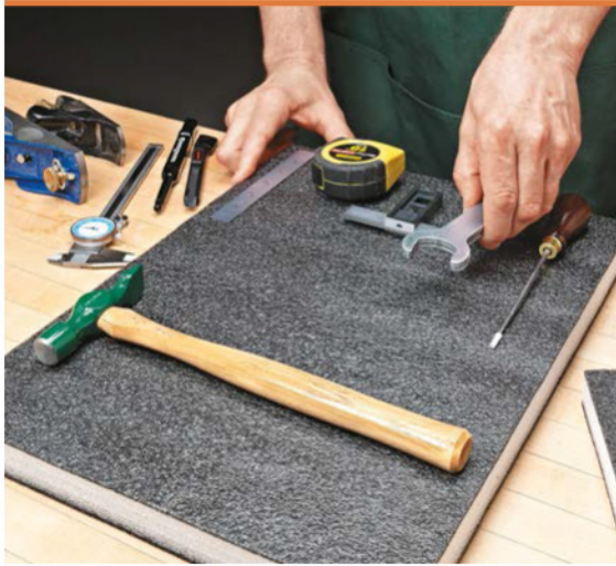
▲ After cutting the foam to its final size, lay out your tools for the easiest access and organization.
