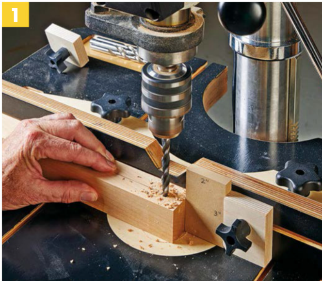
▲ Drilling out the waste in a mortise is a common drill press task. Using a stop block and a spacer block adds consistency to the process for a low investment in time and effort.
