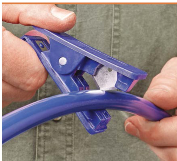
▲ There's a cutter included in either kit. The tool makes it easy to cut the tubing square for an air-tight fit.
