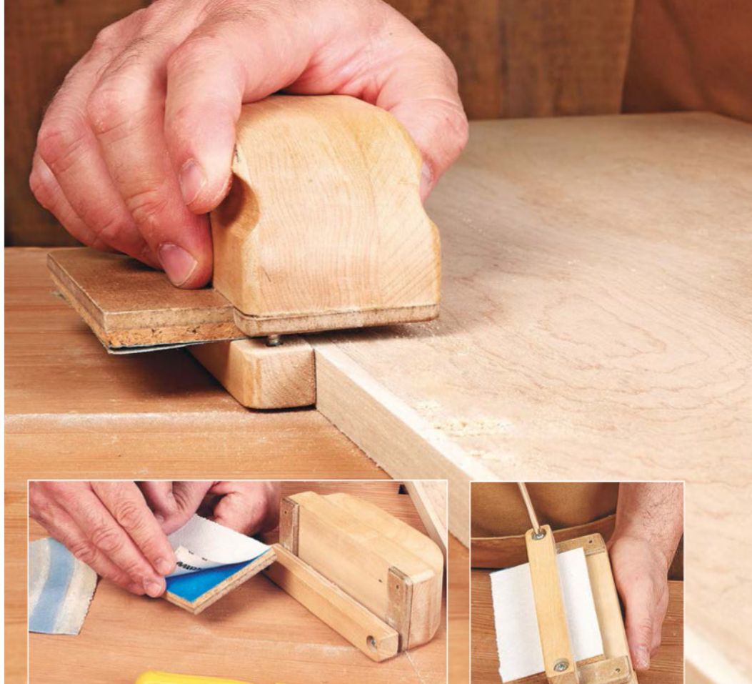
▲ A layer of painter's tape protects the cork layer from wear as adhesive-back sandpaper is applied and removed.
