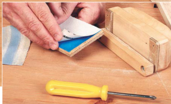
▲ A layer of painter's tape protects the cork layer from wear as adhesive-back sandpaper is applied and removed.
