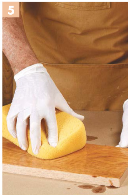
No Puddles. You want the surface to be damp, not wet, for the next step. Use a sponge to dab up the excess.
