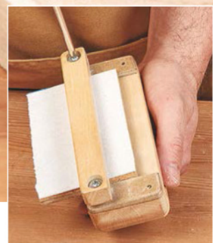
▲ The exposed sandpaper can be easily adjusted by sliding the pad.
