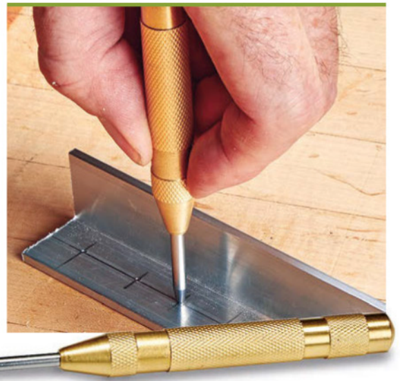
▲ A spring-loaded center punch has a self-striking mechanism, making it quick and easy to use. The force it delivers is limited, making it best on softer metals.
