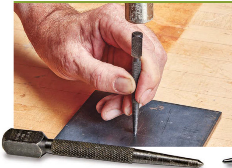
▲ A basic center punch needs to be hammered, but the force of the blow works better on harder metals and is often the most accurate method.
