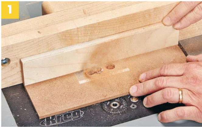
▲ Dot to Dot. Set up a matching straight bit in the router table to complete the slot. The jig's fence registers off the router table fence for consistent alignment.
