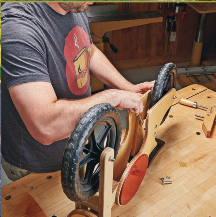
▲ Lock nuts, washers, and carriage bolts secure the adjustable hardwood seat in one of three positions.
