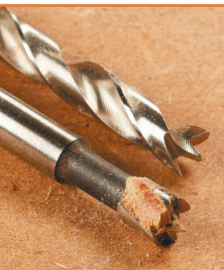
▲ Small Forstner bits clog easily. Brad point bits are a better solution for mortises less than \frac{3}{8} " wide.
