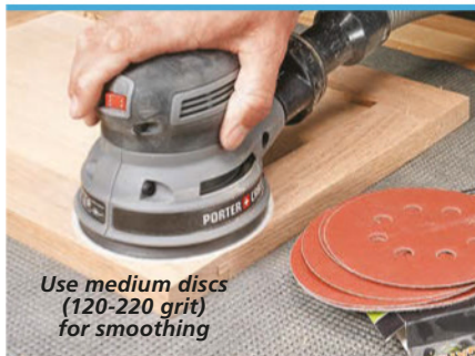
Fine discs (320 grit and up) are perfect for finishing
