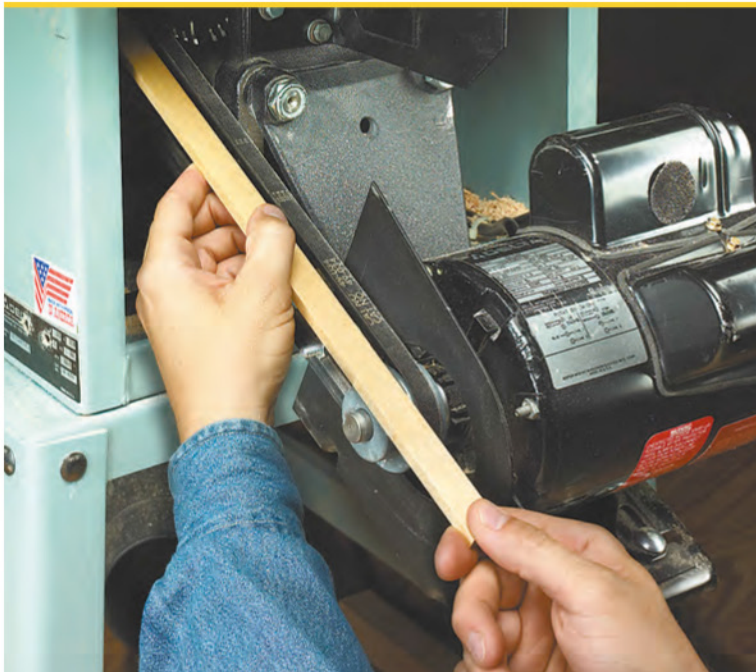
▲ Rest a straightedge against the outside faces of the two pulleys. Ideally, the straightedge will rest flush against both faces. If it doesn't, shift either the pulleys or the motor to bring them into alignment.
