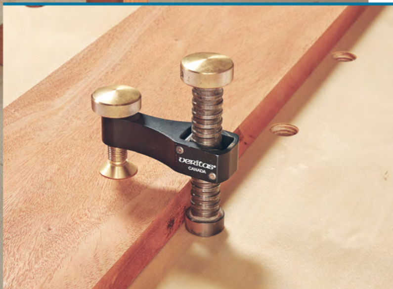
▲ Dog holes in the worksurface let you use hold-downs and other accessories to work on pieces of all sizes, wherever you need them.
