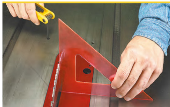
▲ Most table saws have set screws that can be adjusted with Allen wrenches to set the stops. Adjust the screw until the blade is positioned at the correct angle.
