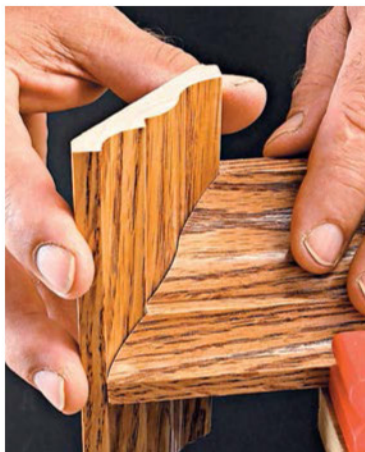
▲ To check the fit, hold the coped end against a scrap piece of molding. A file will fix small gaps.
