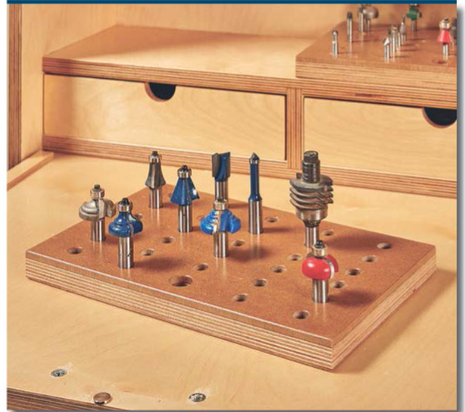
▲ Simple bit trays allow you to customize your bit storage. For example, this one sorts bits by the shank size.
