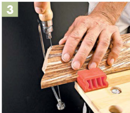
3 ▲ Starting from the back of the molding, make a second relief cut up to the transition line where the ogee profile begins.
