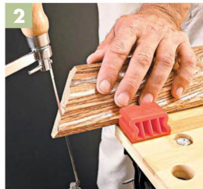
2 ▲ With the coping saw held at a steep angle, make a backcut along the cove profile, stopping at the relief cut.
