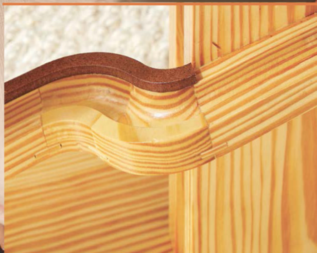
▲ Splines join the individual pieces of track that make up the start and end ramps for a sturdy connection.
