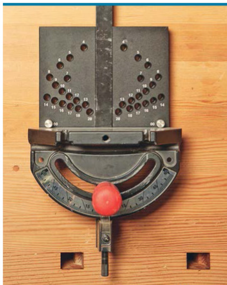
▲ Like the Standard plate, the Segments plate starts with a pair of '00' holes that each holds one pin as a point of reference.
