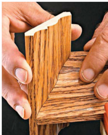
▲ When you have arrived at a tight-fitting joint, the line between the two boards will all but disappear.
