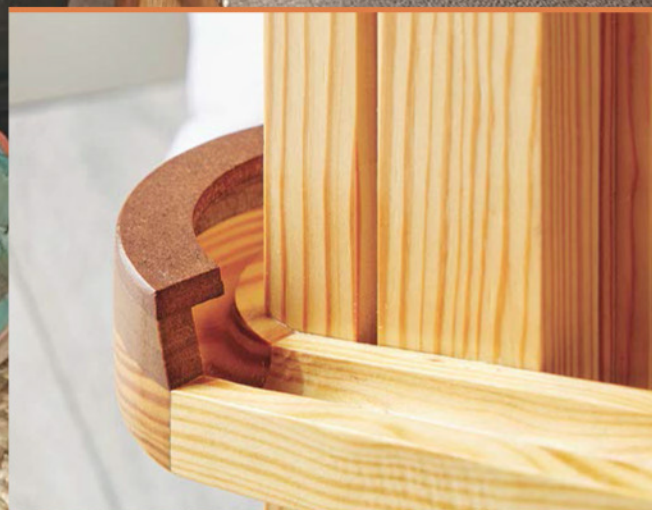
▲ The marbles build speed rapidly as they follow the track, but a series of hardboard bumpers keeps them in line.
