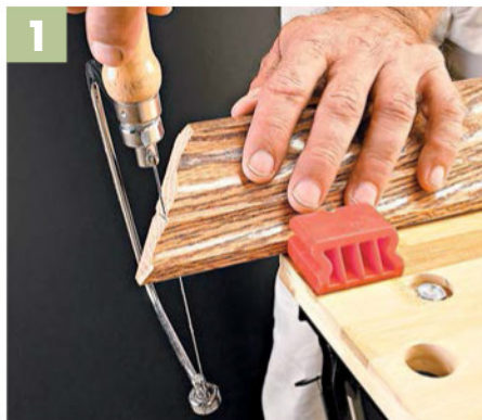
1 ▲ The first step is to make a relief cut from the back of the molding to the transition line between the two decorative profiles.
