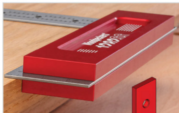
We've packed many of the great features of our aluminum squares into our new stainless-steel models and then gave them some unique features, too. Notice the lip formed by the central core being slightly wider than the beam cheeks. Your square won't roll over. That's a feature you'll see in Woodpeckers squares from 6" to 26".
