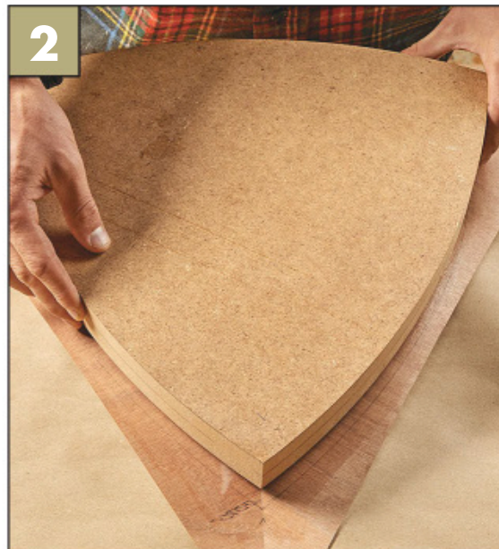
Press It Down. Align the tabletop's corners with the veneer seams and press it in place to bond the parts.
