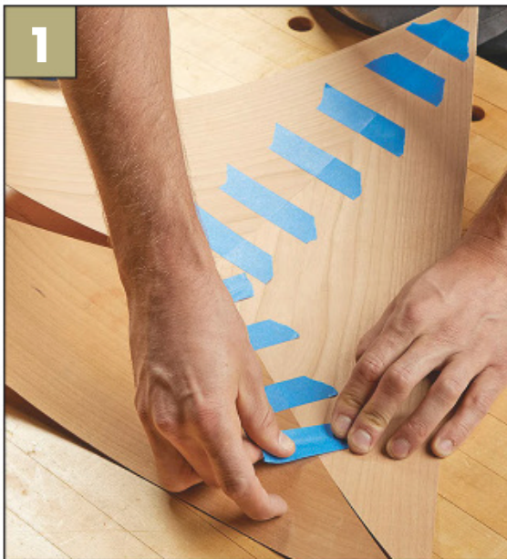
Tape Assembly. Pull masking tape across the joints to hold the veneer sections together.
