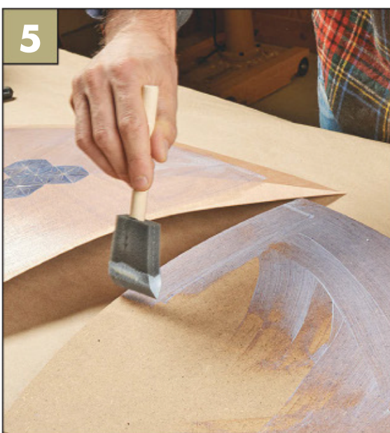
Contact Adhesive. Brush a thin coat of adhesive to each of the mating surfaces. Then let it dry.
