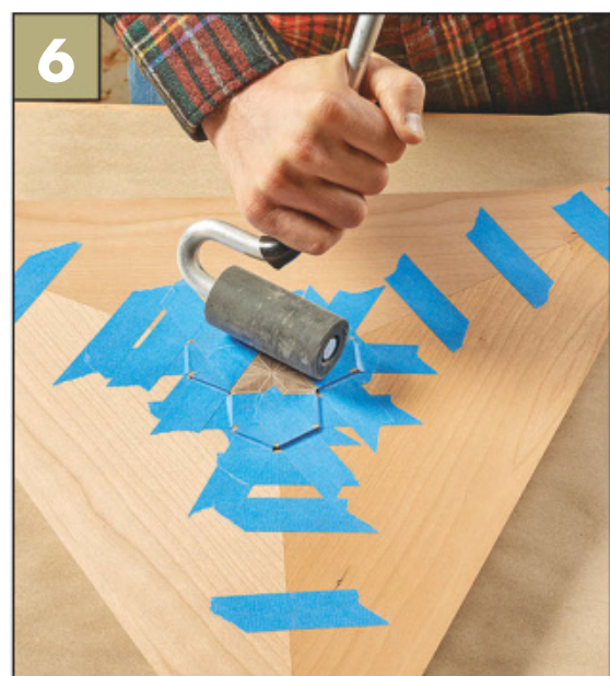
Roll & Trim. A J-roller ensures the solid bond and smooth surface. Trim the excess veneer with a knife.
