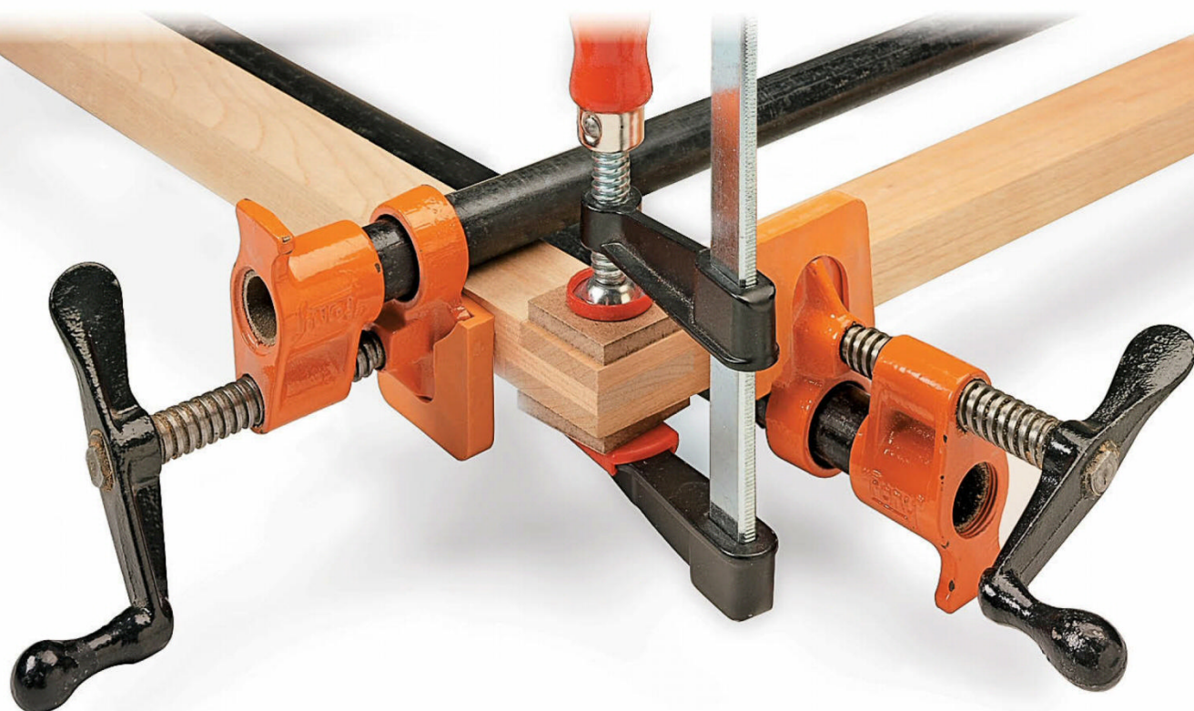
◀ Assembling a bridle joint often requires an array of clamps to keep the parts aligned.
