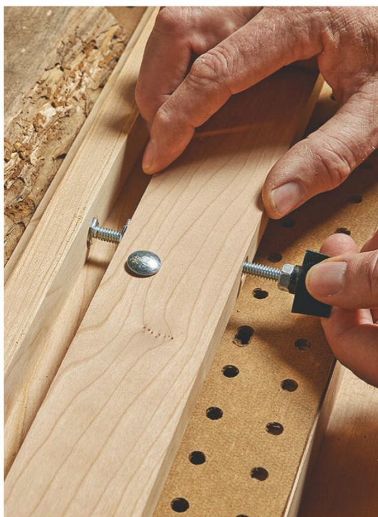
Secure the Workpiece. Tighten the hex nuts until the adjustable plate firmly grips the workpiece.
