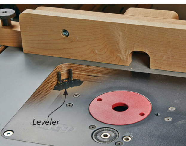
Kreg insert, lift, and levelers work together to keep the insert flush with the table
