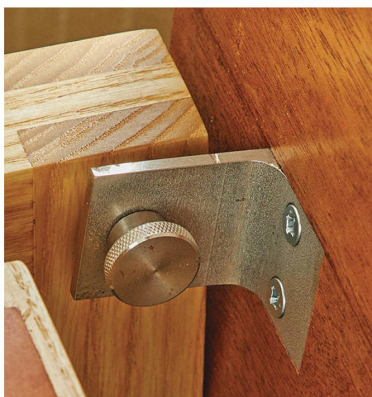
▲ The seat rotates on a custom-made L-shaped mechanism that consists of a bracket, a thumbscrew, and a threaded insert installed in the leg.
