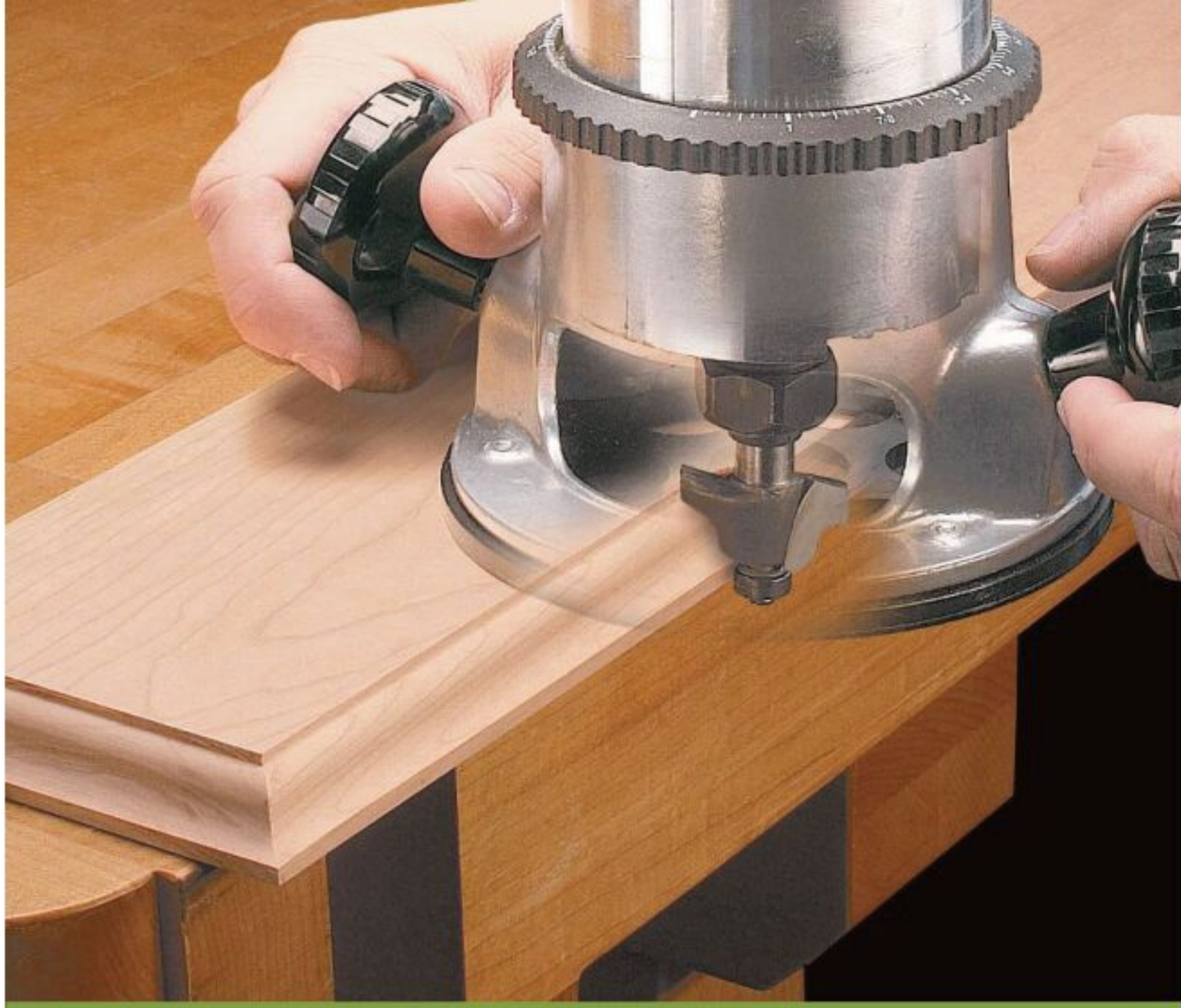
▲ On large routed profiles, you can use freehand passes to work your way to the final cut without needing to adjust the bit depth.
