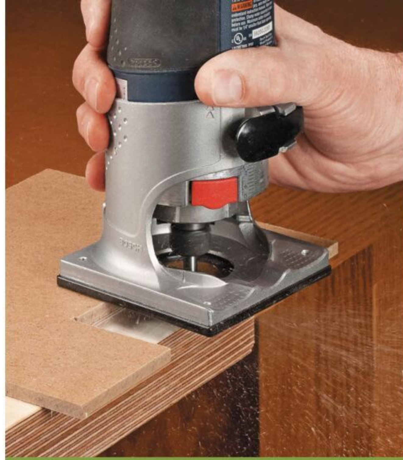
▲ Trace the hinge template with a pattern bit then sweep across the waste material to clear away a mortise.
