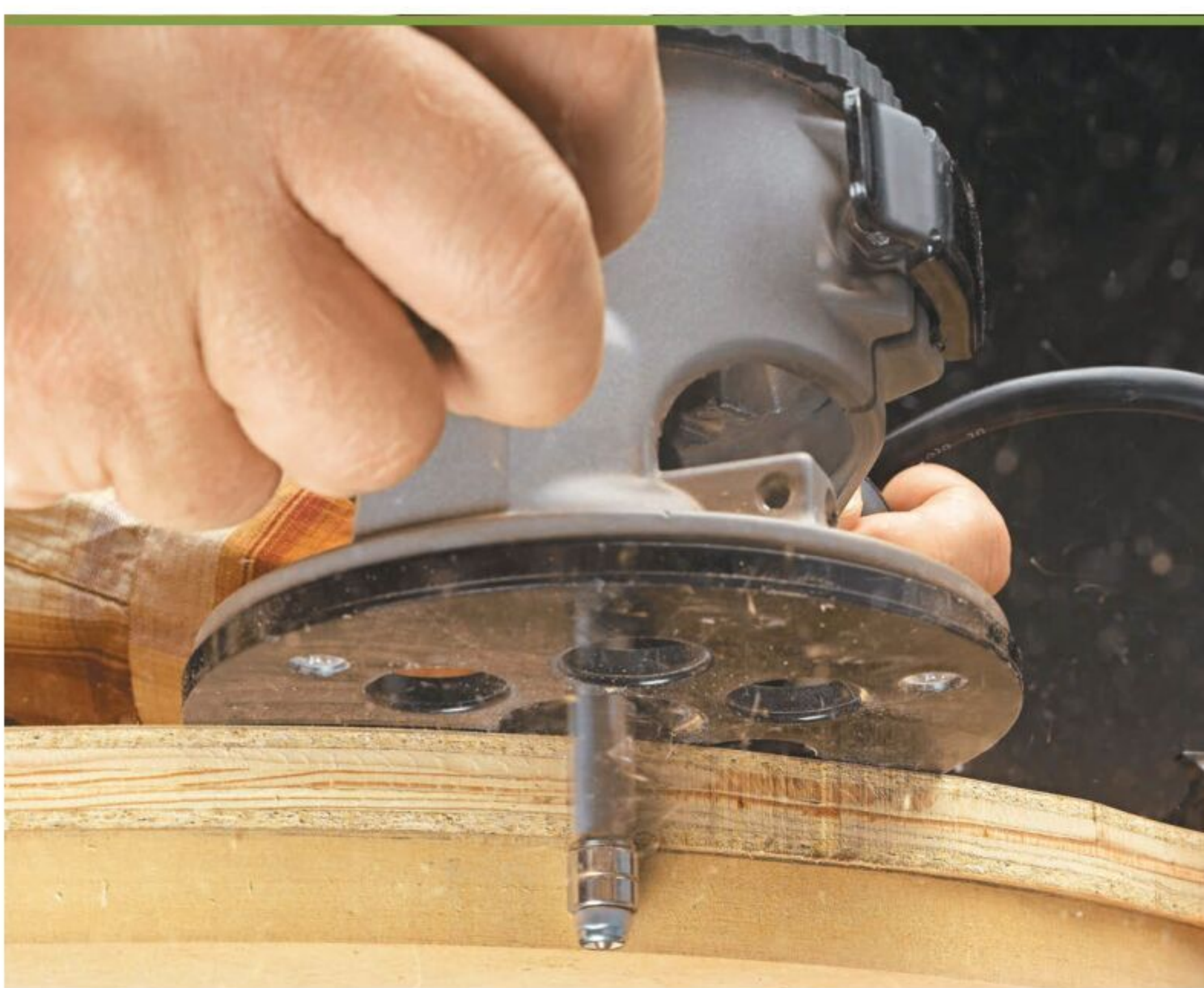
▲ Taking freehand skim cuts along the overhanging edge (right side of image) clears away much of the waste. The final pass only needs to remove a small amount and ends up being much cleaner.
