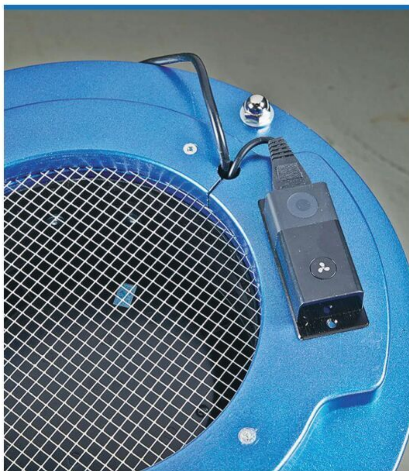
▲ The six-speed controller is mounted to the top for easy access. Hardware cloth caps the air cleaner to keep debris out.
