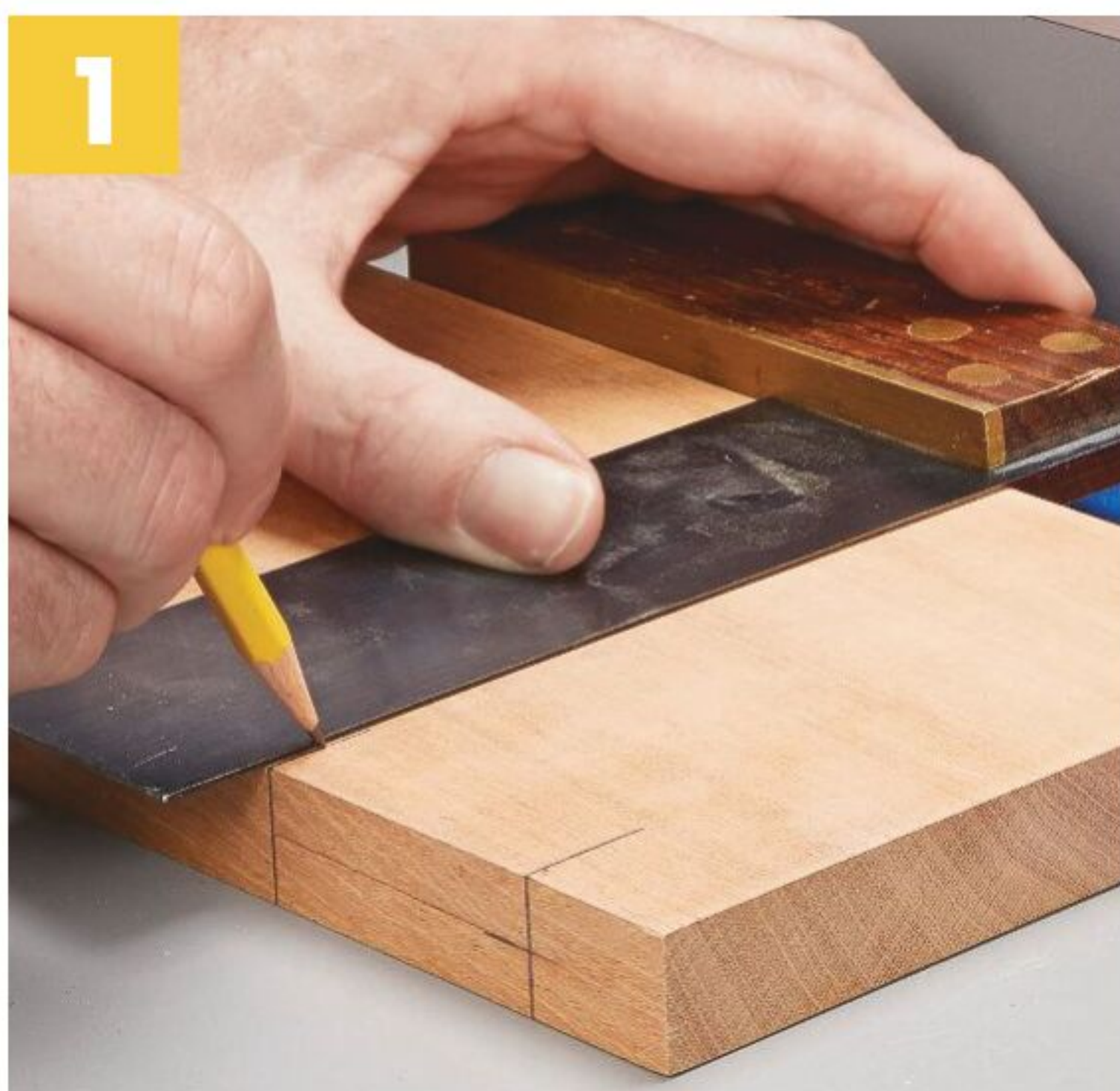
▲ Transfer the ends of the grooves onto the face of the workpiece to see what you're doing.
