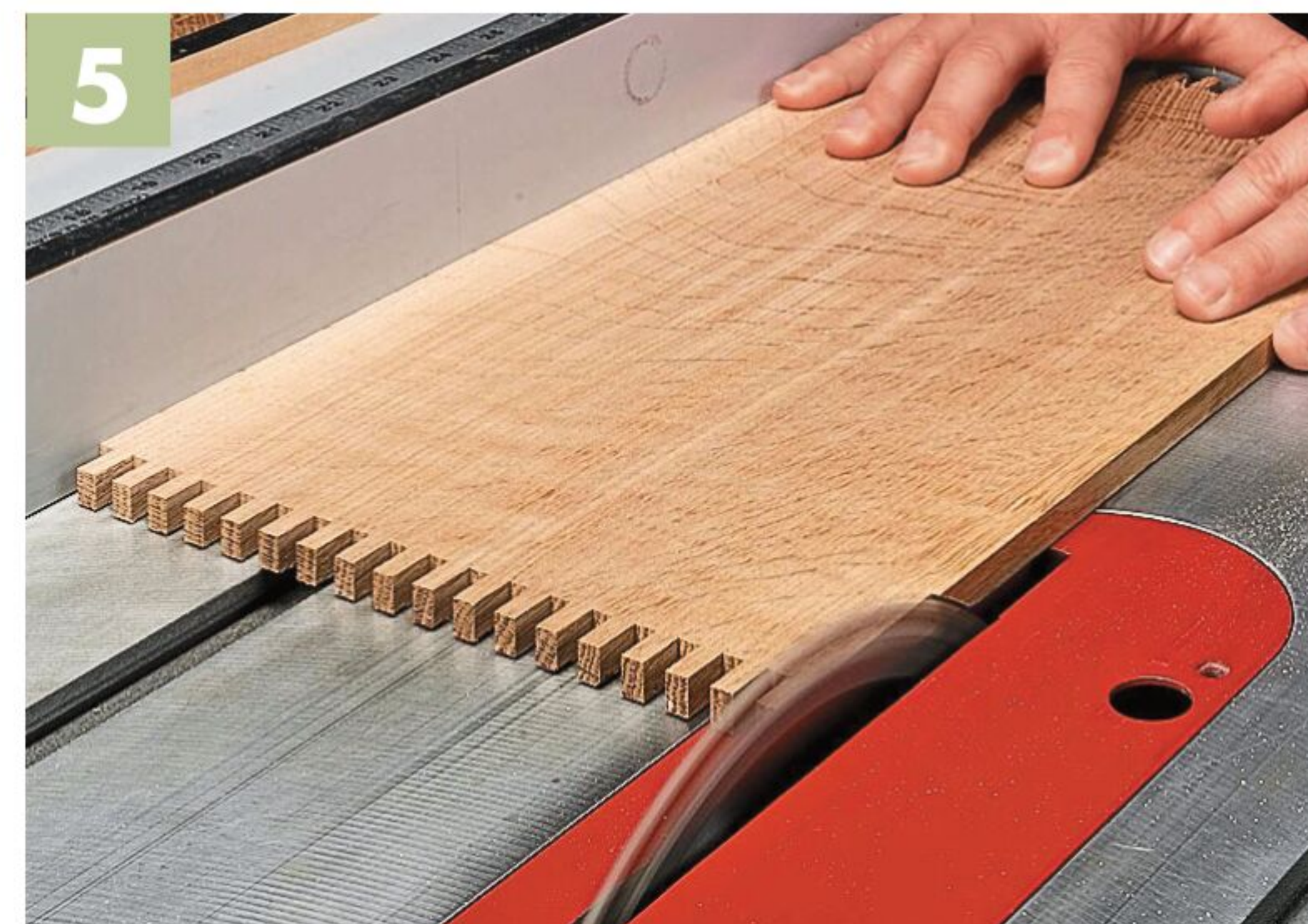
▲ Trim to Fit. If needed, trim the workpieces so that each one ends with a full pin or notch for a more finished look.
