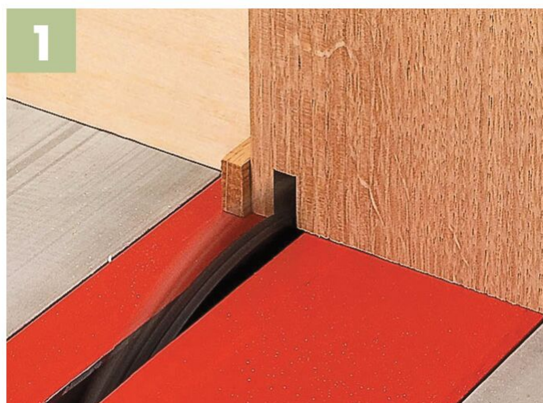
▲ First Cut. Maintain a firm grip to keep the workpiece squarely in position against the fence and tight against the key.
