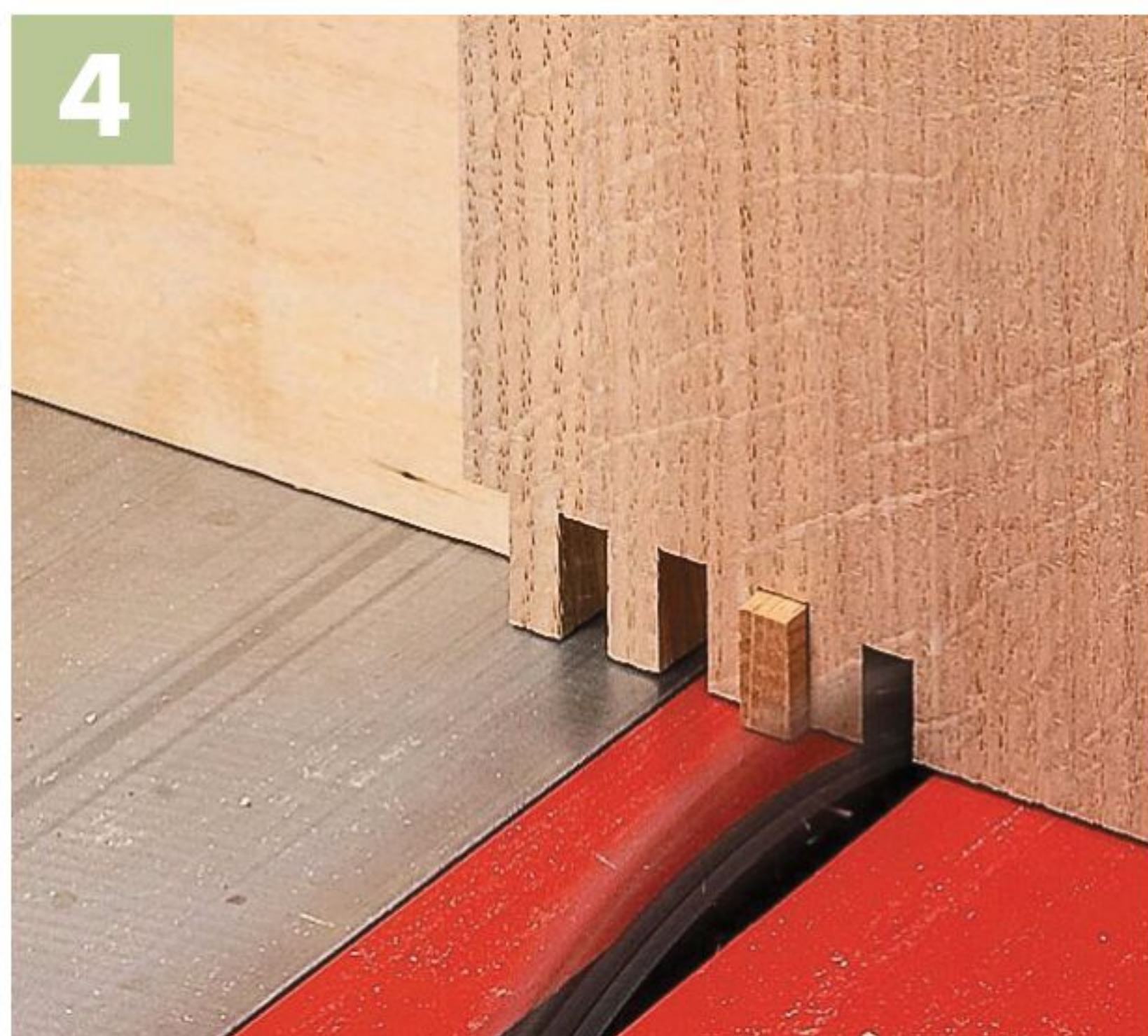
▲ Finishing the Pair. Cut the second piece in the same manner as the first, using steady speed and force.
