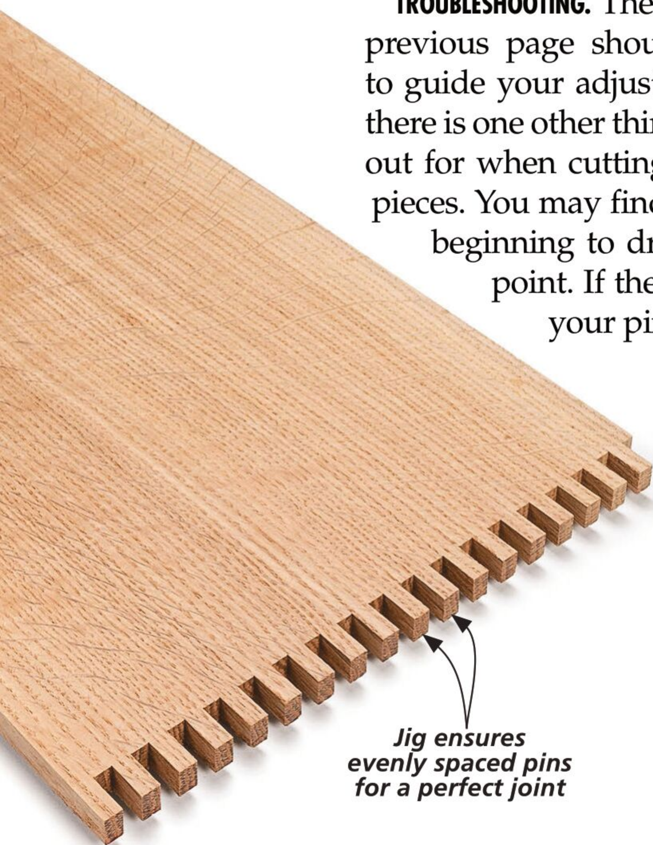
▲ First Cut. Maintain a firm grip to keep the workpiece squarely in position against the fence and tight against the key.
