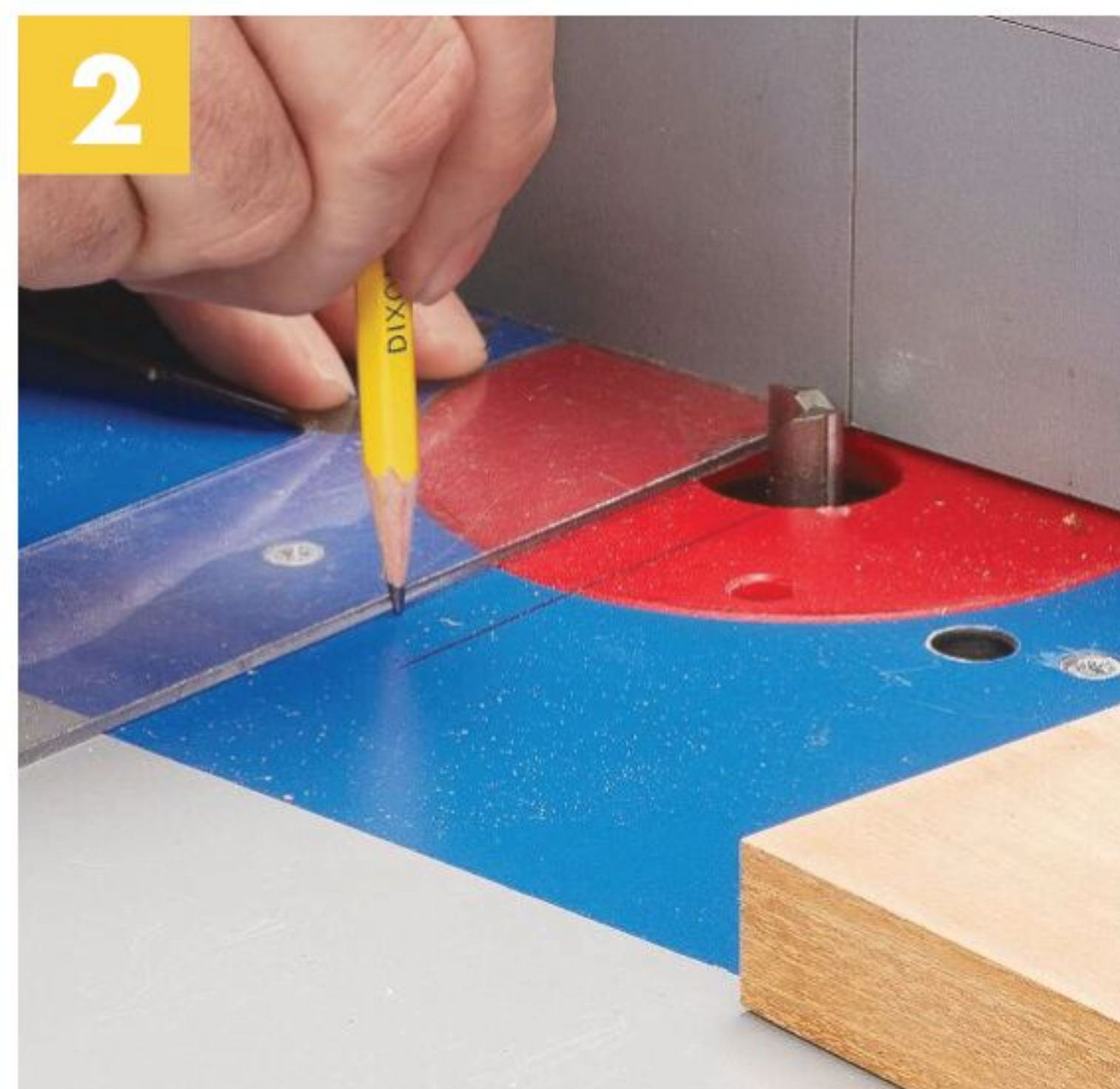
▲ Use a drafting triangle to mark the edges of the router bit on the tabletop (or fence).
