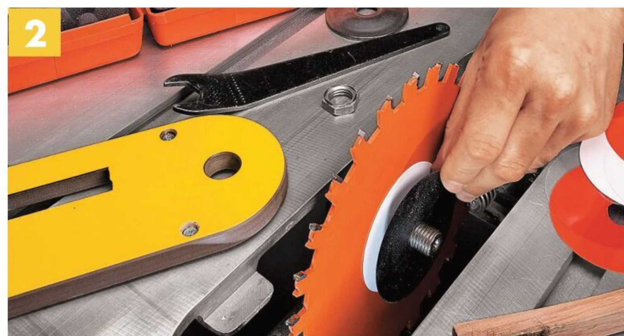
▲ To avoid creating gaps in the dado (and the resulting cut), avoid placing more than two shims in one location. Keep the shims snug against the blade.
