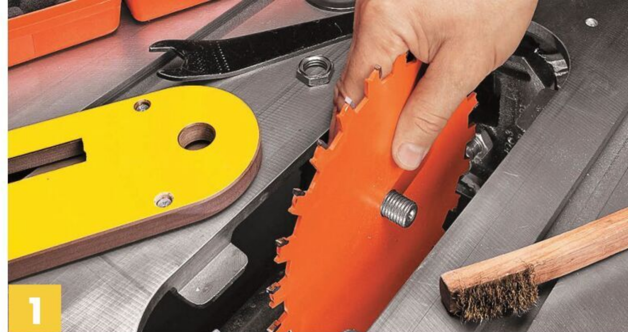
▲ For easy access, raise the arbor to its highest point. Clear away any debris from the threads and then set the first scoring blade in place.
