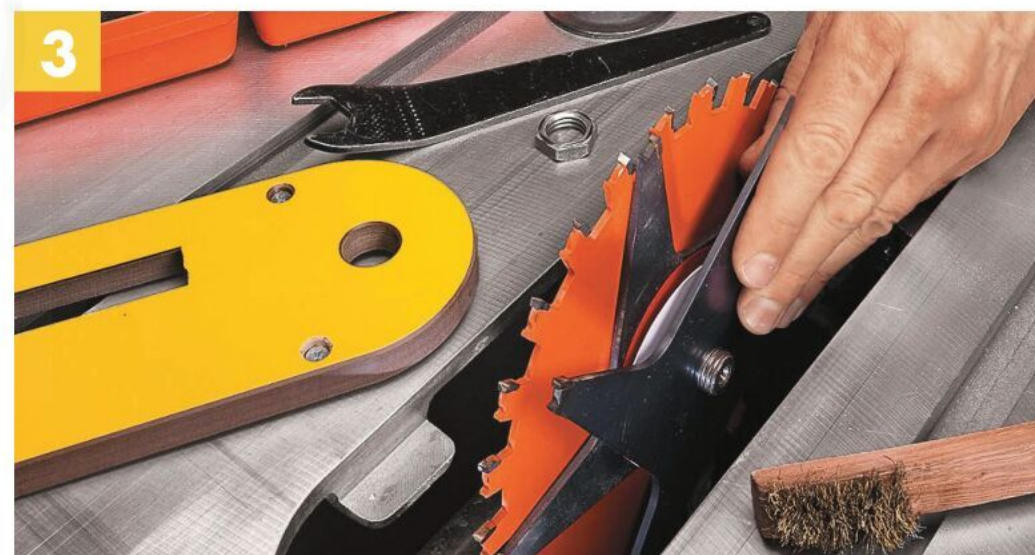
▲ Stagger the chippers so the carbide teeth won't contact adjacent blades and chippers. The design of the chippers keeps the blade balanced regardless of the arrangement.
