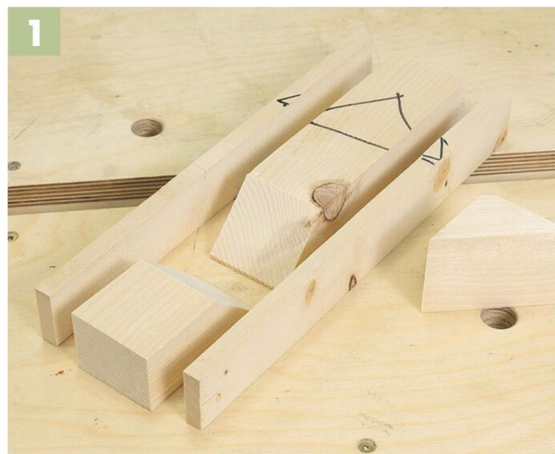
▲ The Krenovian plane is built by sandwiching together multiple parts. It's adaptable and easy to build, making this style a good choice when building your own plane.
