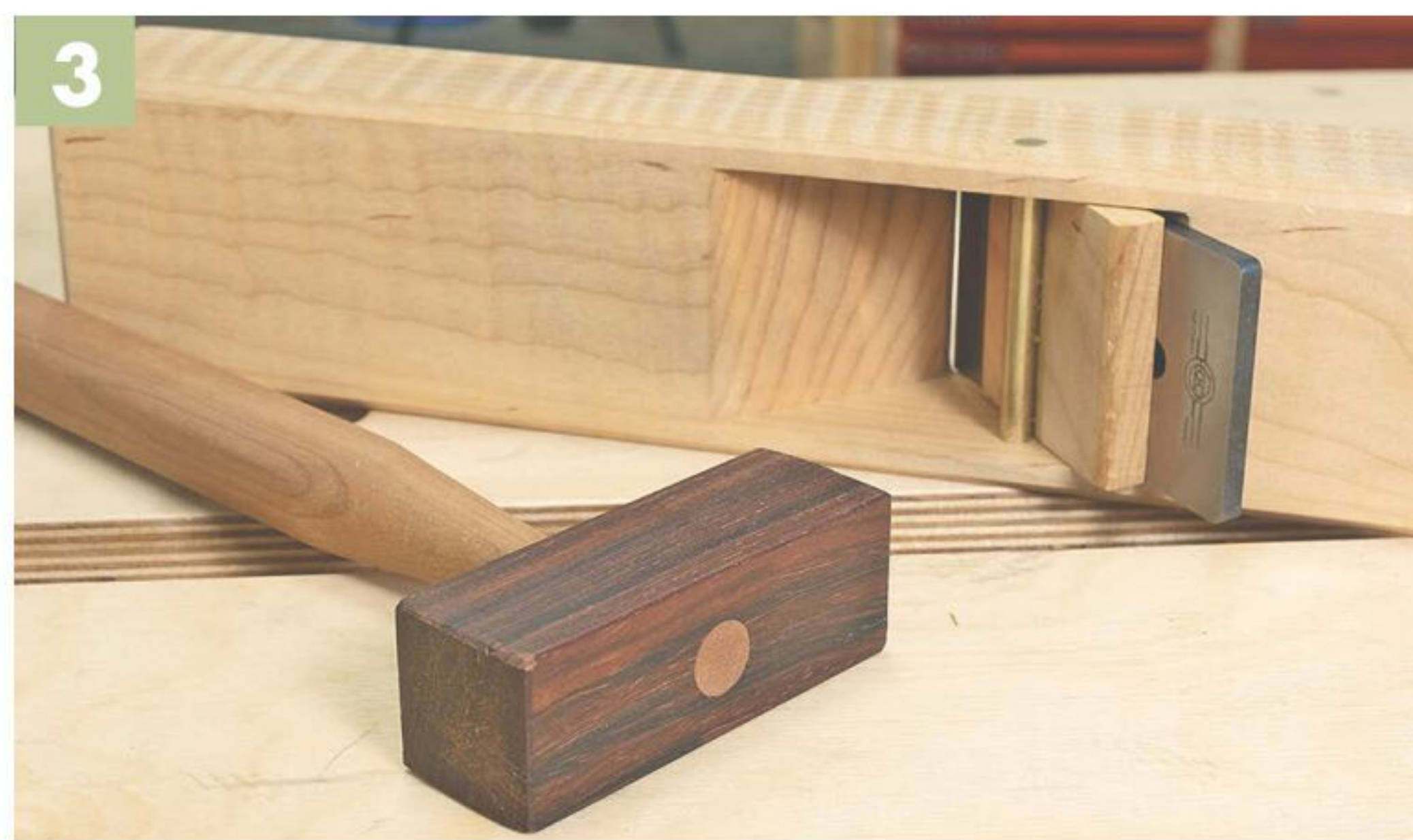
▲ A light wood mallet offers a great amount of dexterity and control in its swing. When adjusting, make a pass across a scrap piece of stock after each tap to fine-tune your plane.
