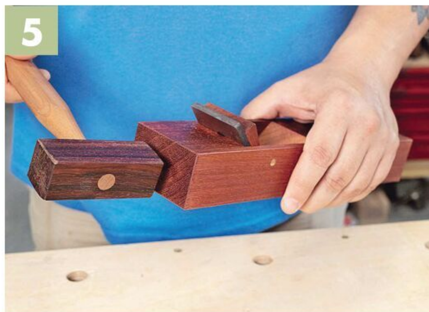
▲ Tapping the rear of the plane will cause the blade to retract. To remove the blade entirely, tap repeatedly until the wedge releases it.
