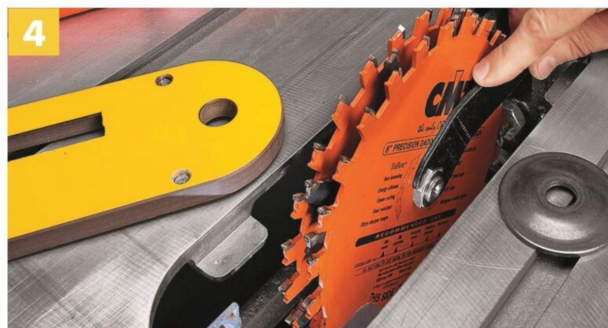
▲ Install the other scoring blade and double-check the setup for proper installation. The nut should fully thread onto the arbor. Then install an insert sized for the dado set.
