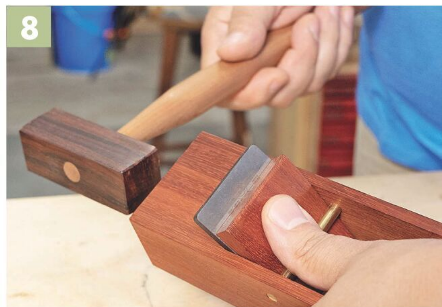
▲ When removing the blade, be careful not to let it slide out of the bottom onto a workpiece or the floor. Use your thumb to keep the wedge and blade in place.
