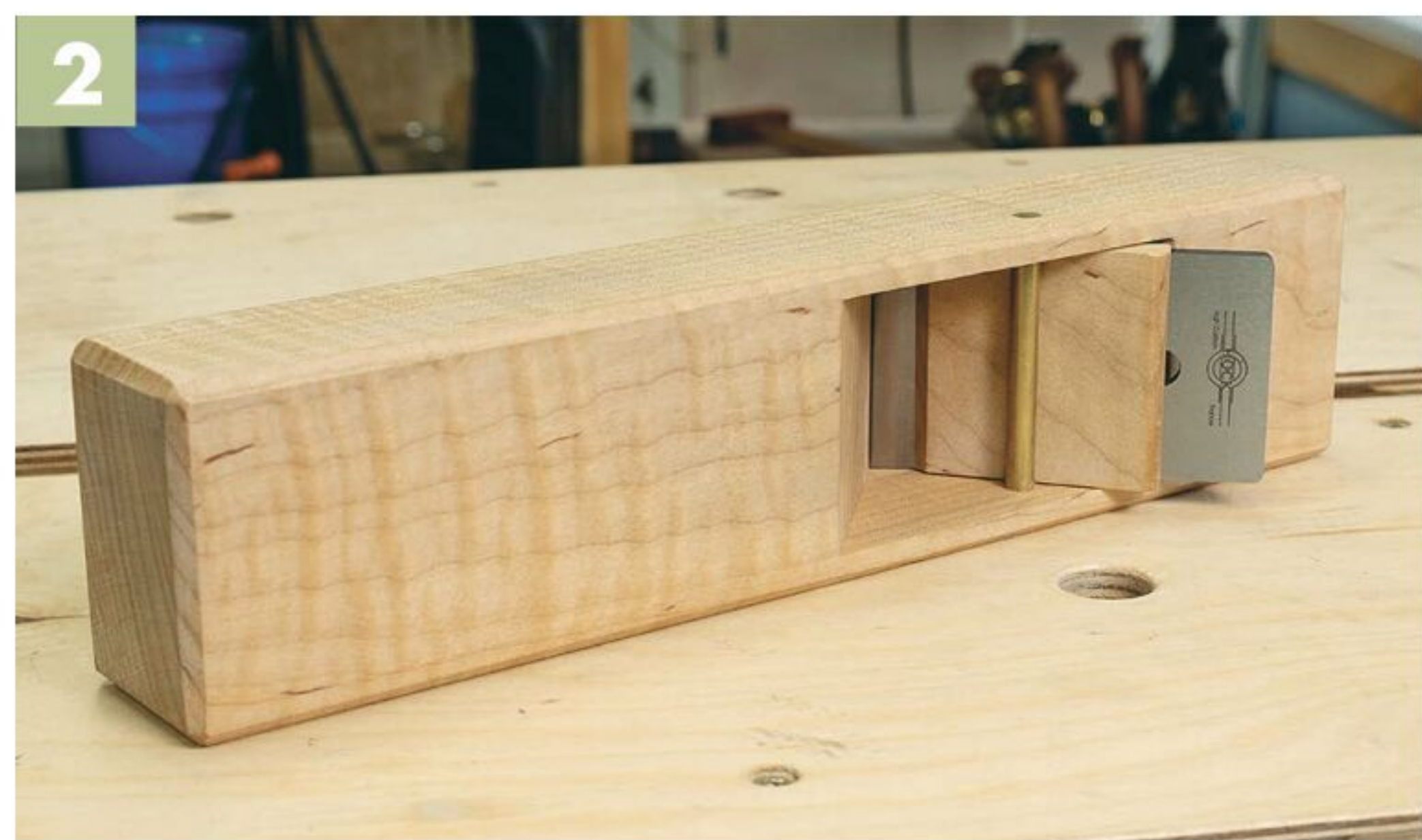
▲ Between the price of the blade and the wood, this pull-style plane set me back less than a third of what a commercial alternative would have, plus I could make it to suit my own preference.
