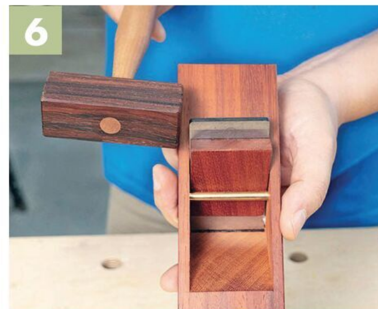
▲ Once the blade has reached the correct depth, tap gently on the sides of the blade to center the blade.
