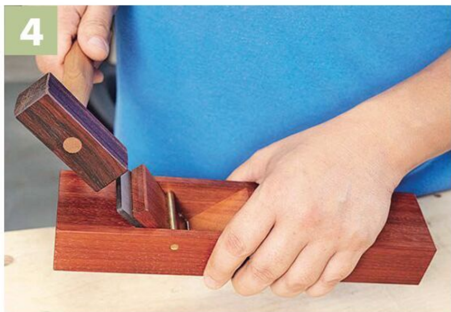
▲ In order to advance the blade, tap the back of it gently with the mallet. This sinks the blade down for a deeper cut.
