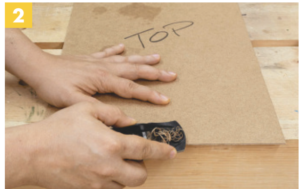
▲ A few swipes with a block plane eases the edges (and corners) of the two cauls. This slight rounding eliminates sharp edges that can damage the vacuum bag.
