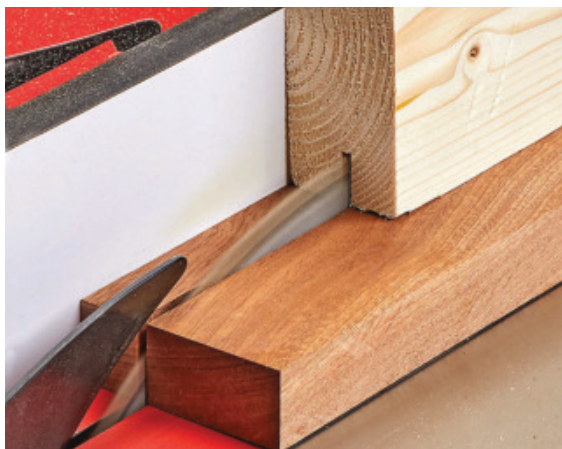
▲ Shop-made push blocks can pass across a table saw blade safely. This allows you to push both the workpiece and the offcut clear of the blade.
