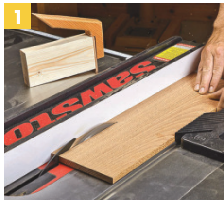
Beginning. Use your right hand to guide the workpiece into the saw blade. Your left keeps the board against the fence.
