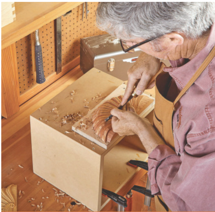
▲ While a stout bench is foundational, it may not be the best place for long-term working. For smaller pieces, a riser box made from MDF allows you to stand more upright and maintain fine tool control.
