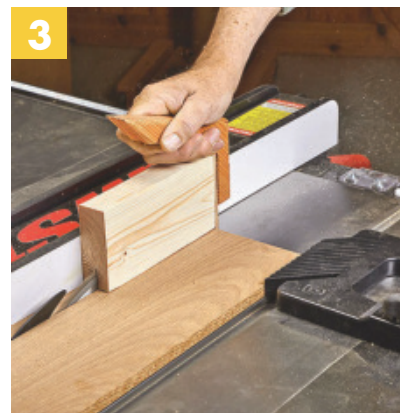
Completion. Follow through the cut with your right hand guiding the workpiece with the push block.
