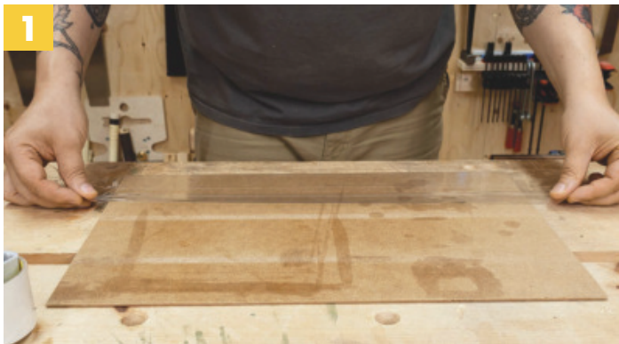
▲ Tempered hardboard makes an ideal smooth upper caul. Apply a layer of clear packing tape to one face. This prevents any glue that bleeds through the veneer from sticking.
