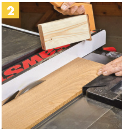
Middle. Your left hand keeps the workpiece moving while you reach for a push block (or push stick).
