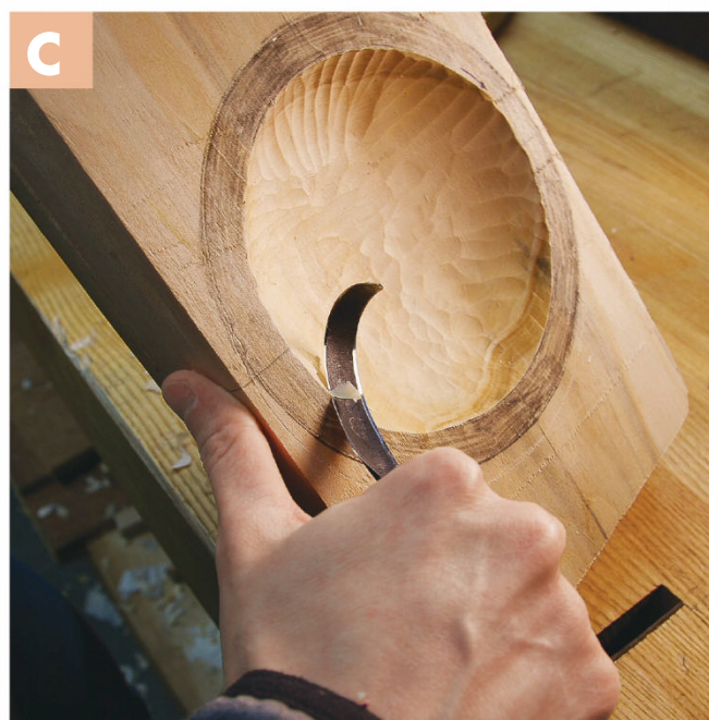
▲ For fine, trim cuts, extend your hand with your thumb protected. Choke up on the handle for maximum control.
