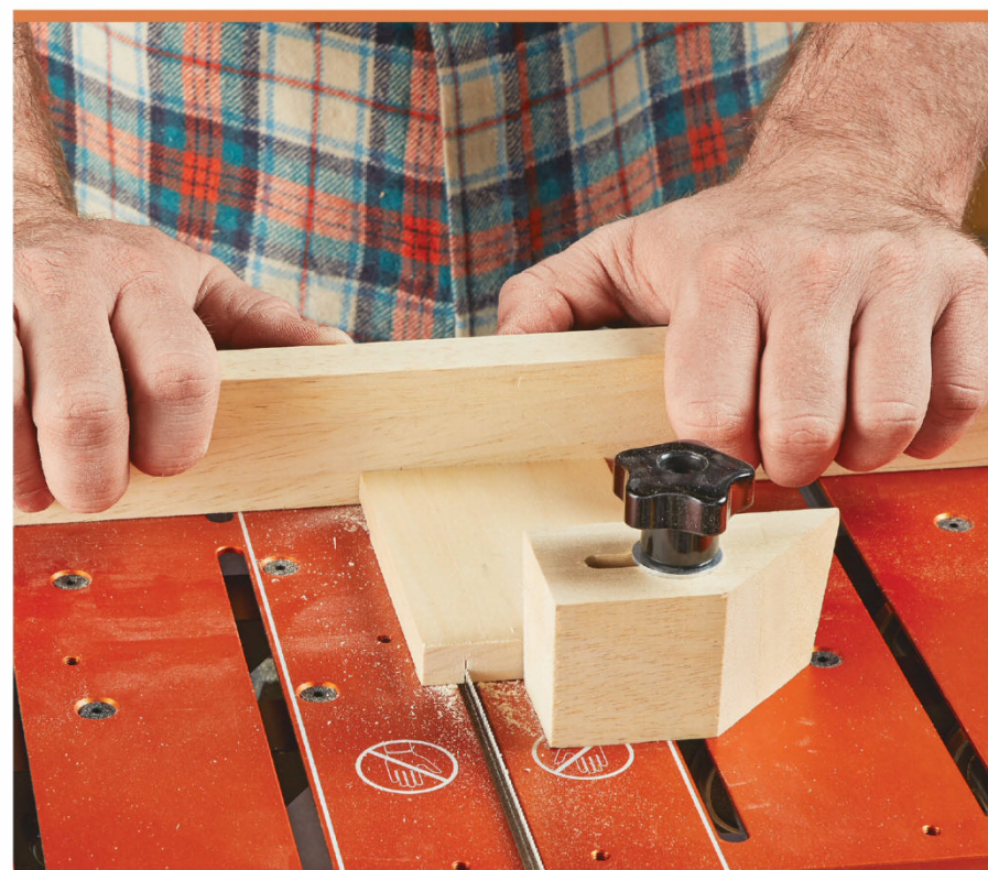
▲ Rip cuts are made in nearly the same fashion as the cross cuts. The workpiece is positioned lengthwise and clamped in place. I found a lower pitch worked better during rip cuts.
