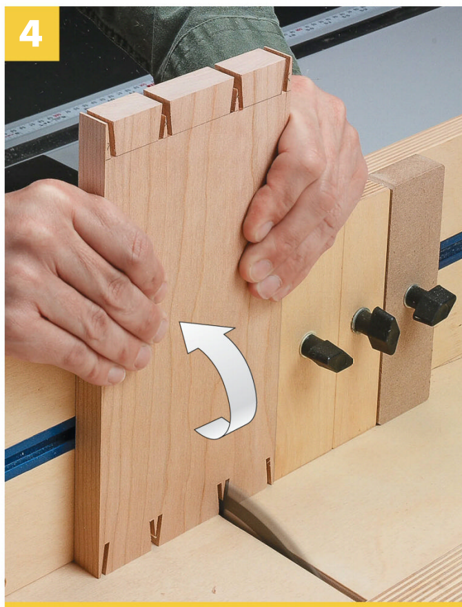
▲ One more step at the table saw. To complete the tails on the other end of the workpiece, flip and rotate everything one more time.
