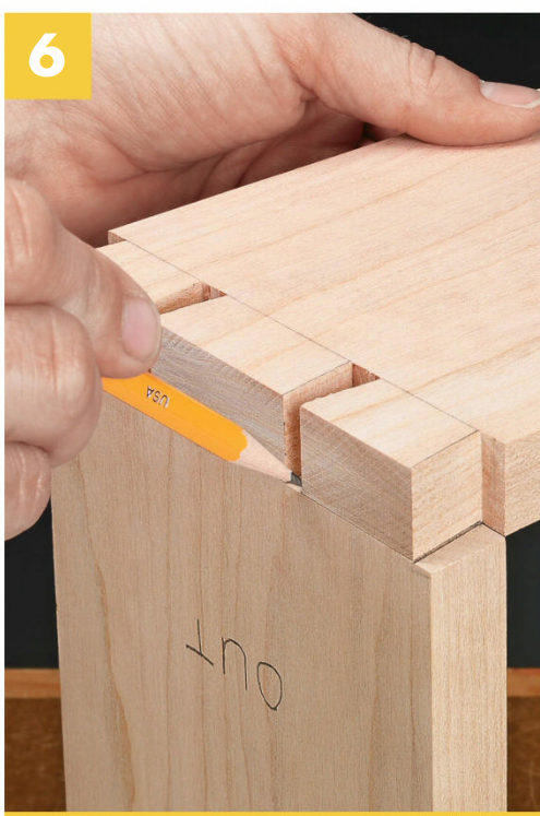
▲ Use the completed tail workpiece with the original layout to locate the pins on the mating workpiece.
