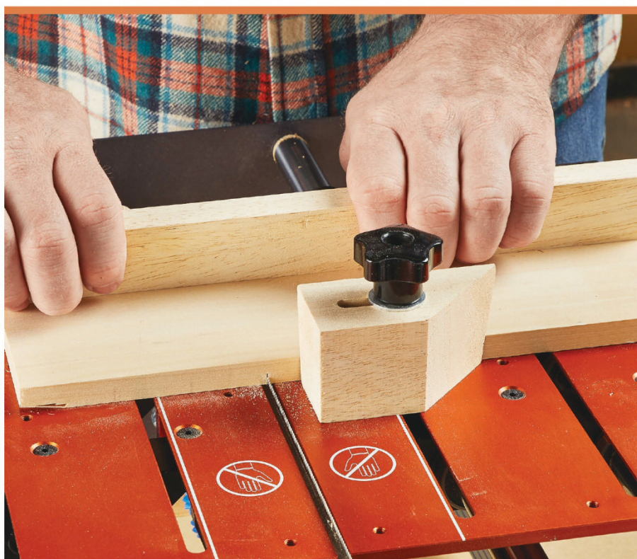
▲ Cross cuts can be made by pinching the workpiece between the rear fence and the moveable stop blocks. The tapered inside faces of the fence and block hold the workpiece securely.
