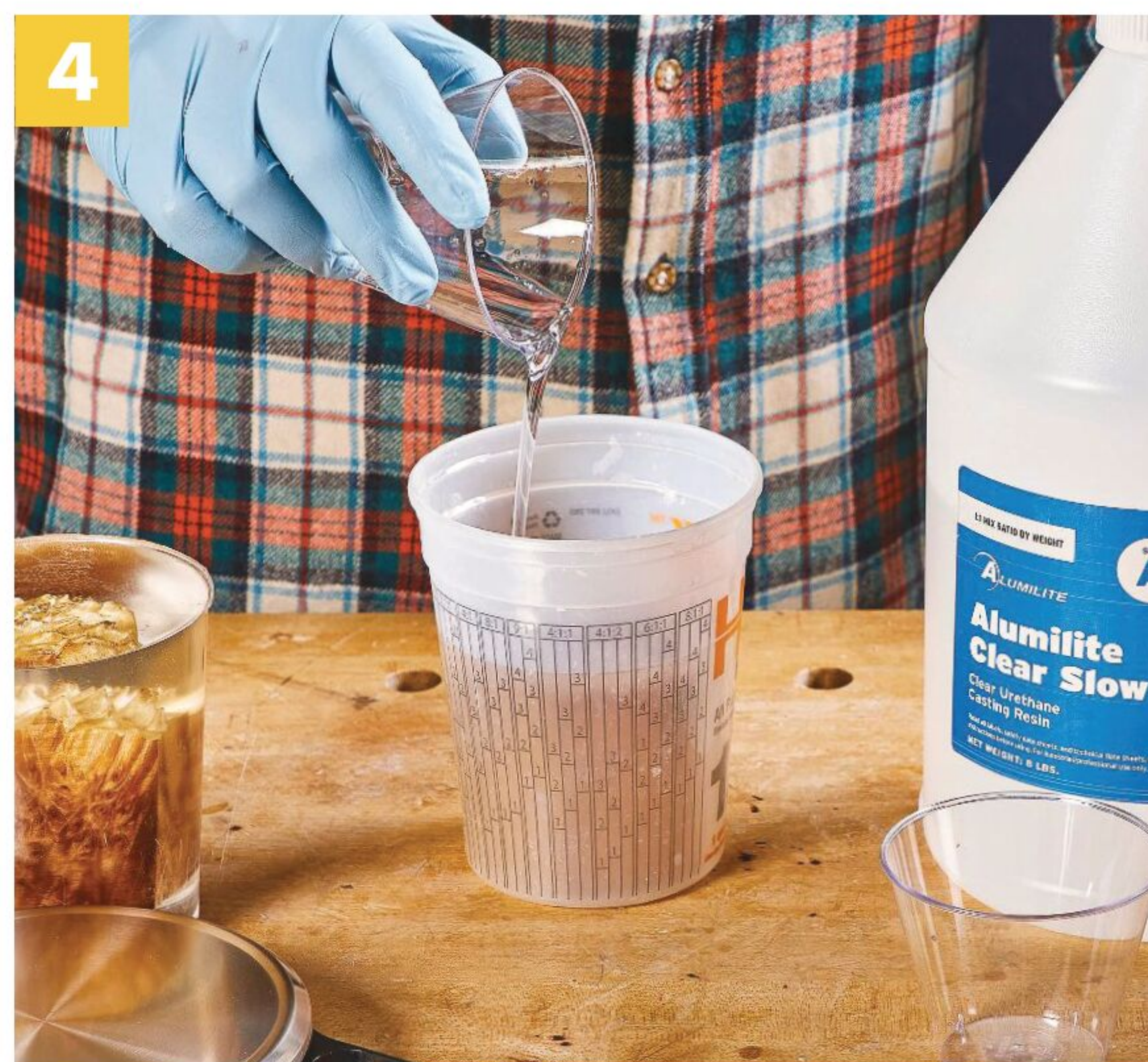
Pour the Resin. Measure the resin by weight. Standard Alumilite can be used with smaller blanks, but larger blanks require slow curing resin to reduce heat buildup.
