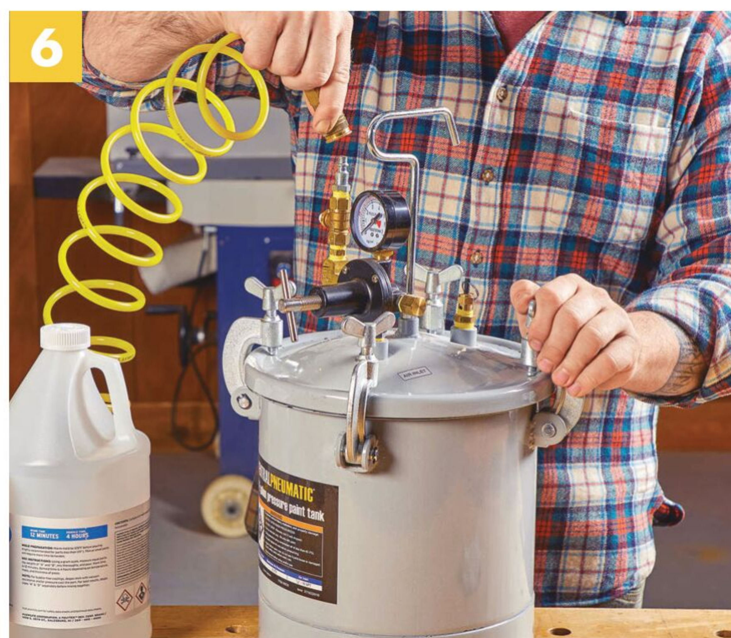
Cure the Blank. Apply pressure until the blank is cured. Curing can take from 1 hour to 6 hours, depending on the resin used and the size of the blank being cast.
