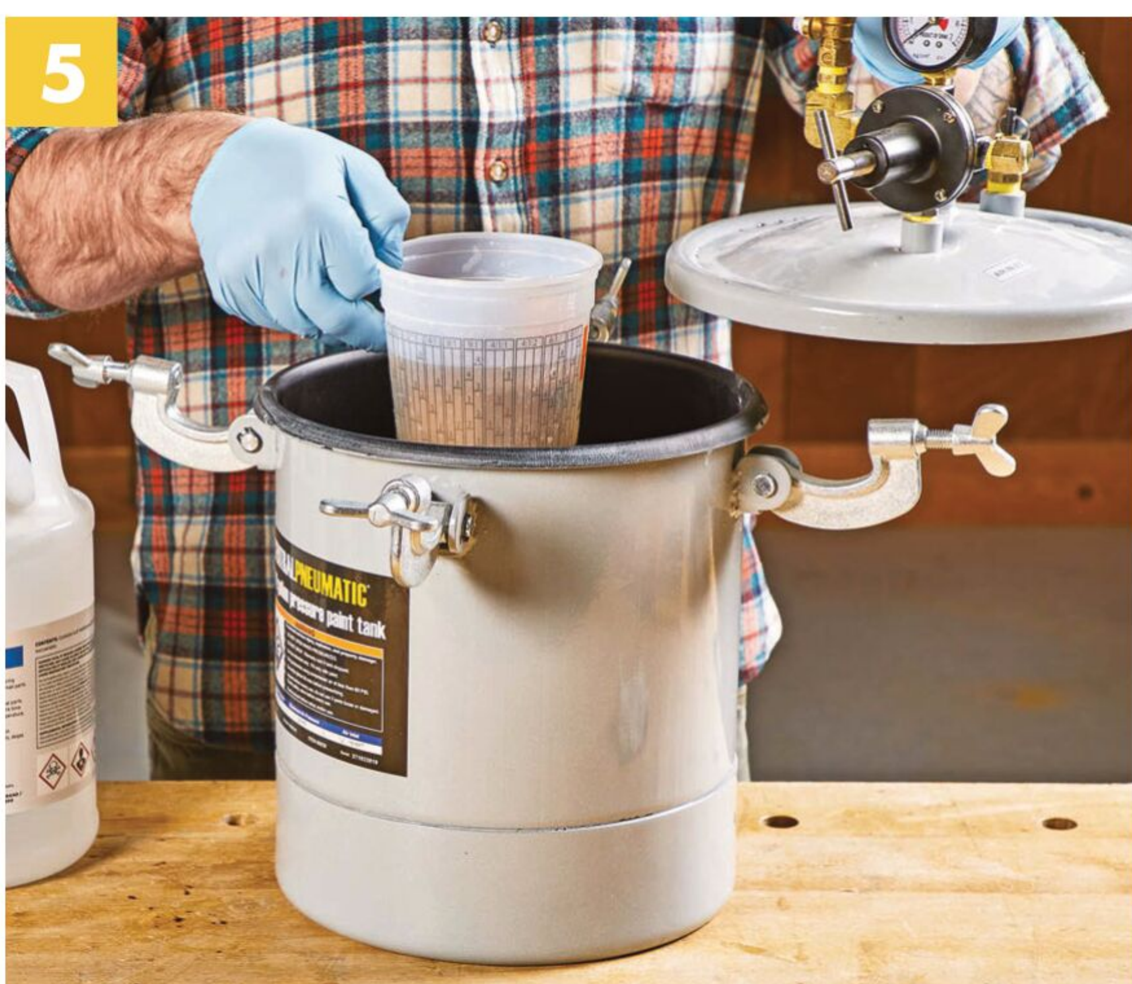
Add Pressure. A pressure pot compresses any bubbles in the resin to a microscopic level, so the final product will be crystal clear and bubble free.
