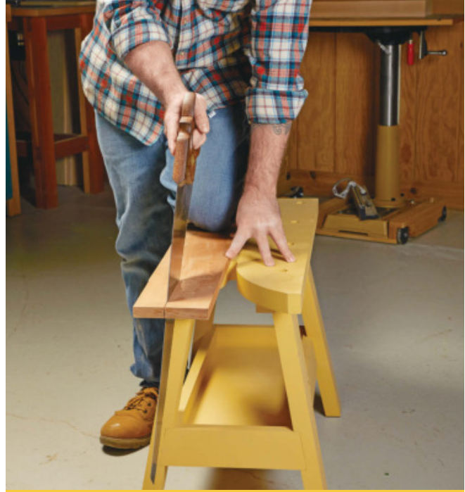
▲ Poor sawing form, shown here, is not only uncomfortable to saw with, but also will lead to an inaccurate cut and sawing that will leave you exhausted.
