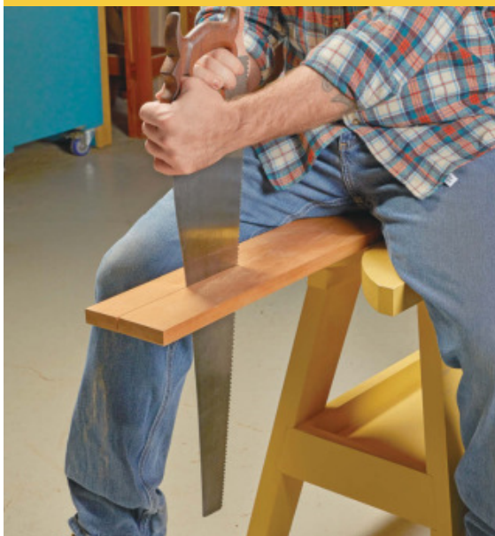
▲ An alternative to kneeling on a saw bench is using your weight and sitting on the workpiece. I find this is easier on the back and makes long rip cuts much easier.
