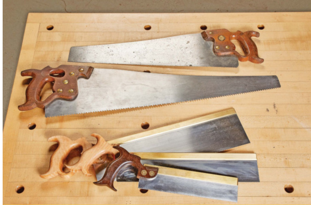
▲ Saws come in all shapes and sizes, varying in form and the intended use. From top to bottom: a panel saw, hand saw (with thumb-hole handle), tenon saw, carcass saw, and a dovetail saw.
