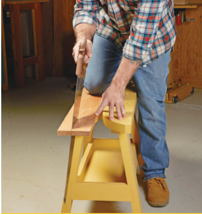
▲ Ripping at a saw bench utilizes the sawing knee to hold the work down. Keep your body in position so that the saw plate is lined up with your hand, elbow and shoulder to ensure an accurate cut.
