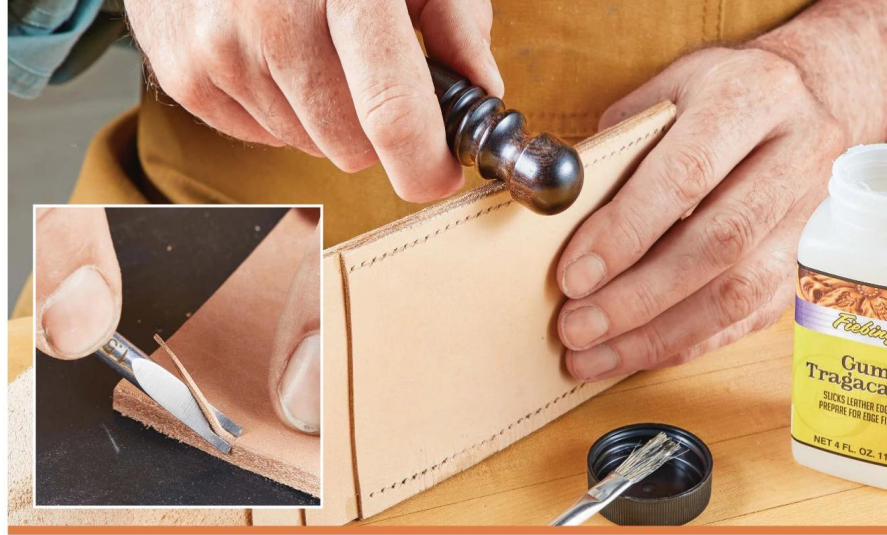
▲ After easing the corners with an edger (inset), rub some gum tragacanth along the edge and then run a slicker back and forth to burnish the edge.
