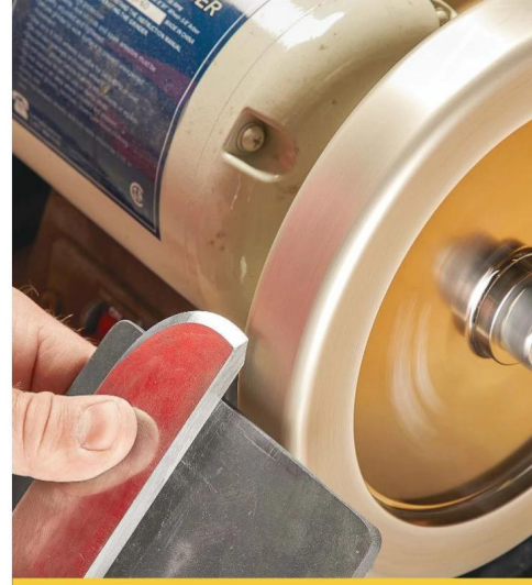
▲ Negative rake scrapers are sharpened long bevel (bottom) first, then the shorter second bevel for a 70° edge.
