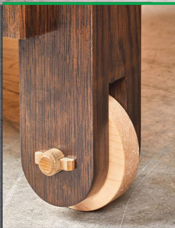
▲ Shop-made wheels and axles — yes please. The plastic bushing is the only part at this end of the project that you'll need to purchase.
