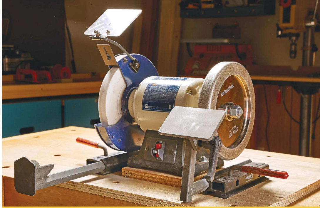
▲ A basic turning sharpening setup is shown here. The Oneway Wolverine system includes a V-cradle and a platform. Both of which slide into receivers mounted below the wheel to adjust for different tools and bevel angles.
