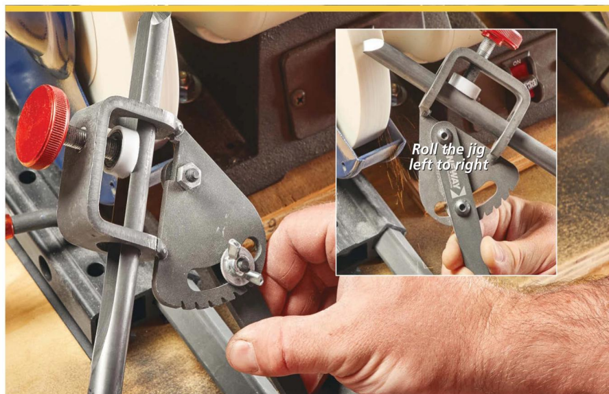
▲ Sharpening a bowl gouge starts with one wing. Then, in a smooth, fluid motion roll the tool from left to right sharpening the entire edge. You'll know the edge is sharp when the sparks travel down the flute as you sharpen.
