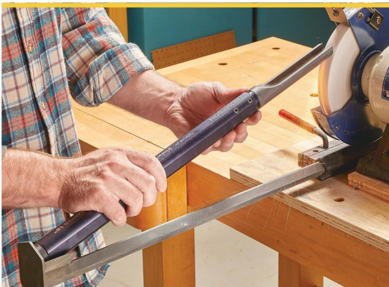
▲ Adjust the V-cradle out until the angle of the tool bevel matches the profile of the wheel. Then, lock it in place and turn the grinder on. Rest the butt of the tool in the cradle and rotate the cutting edge on the wheel to sharpen it.
