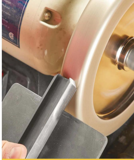
▲ An SRG can also be sharpened with the adjustable tool rest and is the safest way to sharpen an SRG with a CBN wheel.
