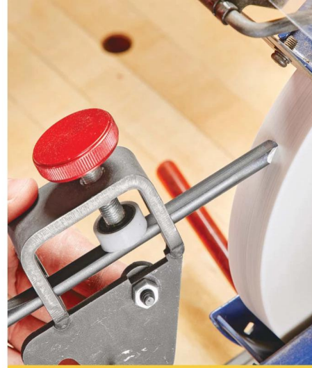
▲ The spindle gouge can easily be sharpened using the Vari-Grind jig. The tool is rocked back and forth to sharpen the entire bevel.
