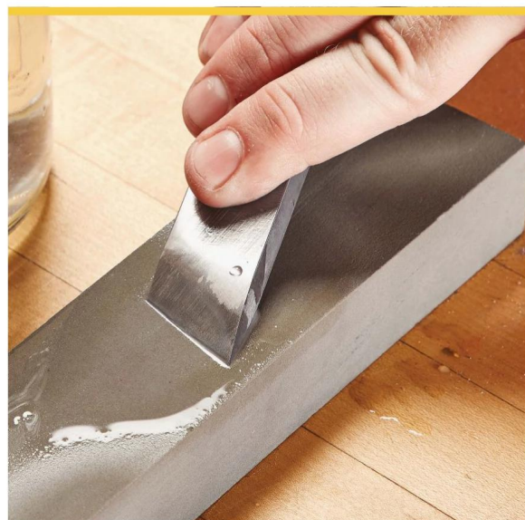
▲ For final sharpening after shaping the skew, I go to an oilstone. Then, it's just a simple matter of putting an edge on like you would a normal bench chisel.
