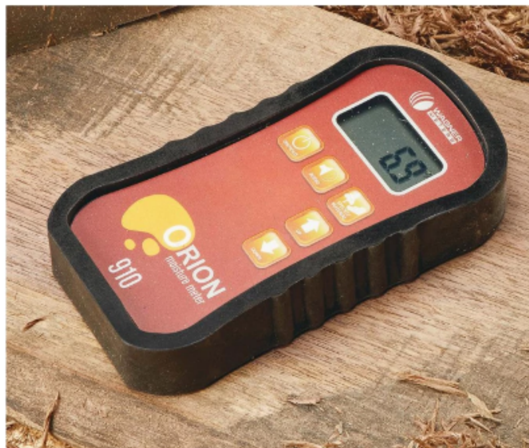
▲ After calibrating, the Orion 910 reads the moisture on this walnut at nearly 7%. That's 2.5 percentage points higher than the lower cost Dr. Meter version shown above.
