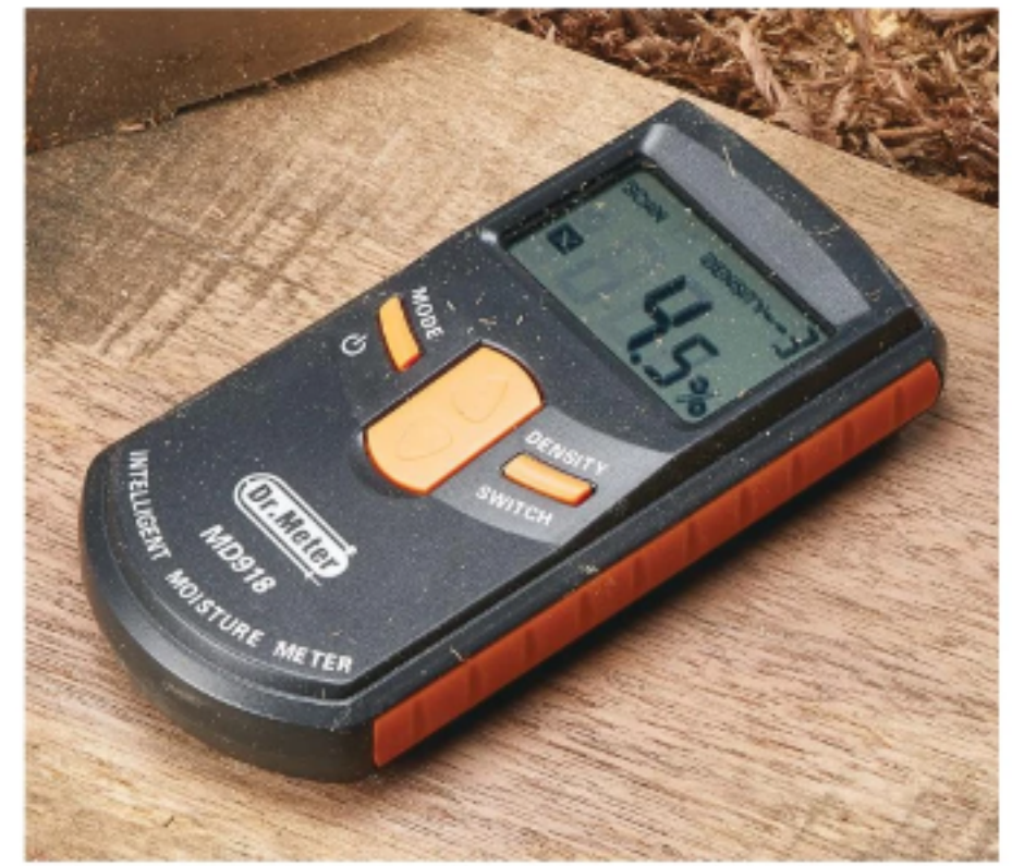
▲ Scanning meters need a clean, flat surface in order to take a reading. Simply plane down a section of rough sawn stock to clean fresh wood.
