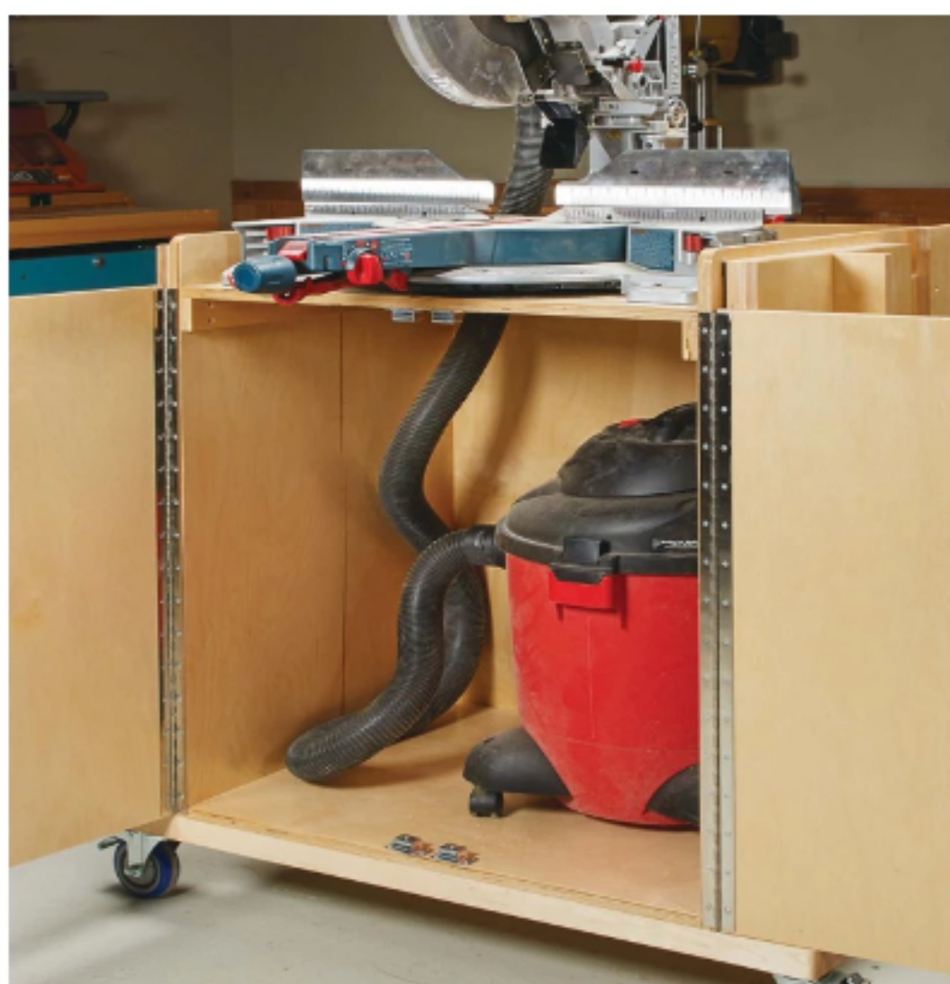
▲ The compartment below the saw is large enough to house a shop vacuum. The hose for the vacuum passes through the hole in the shelf to connect to the saw.
