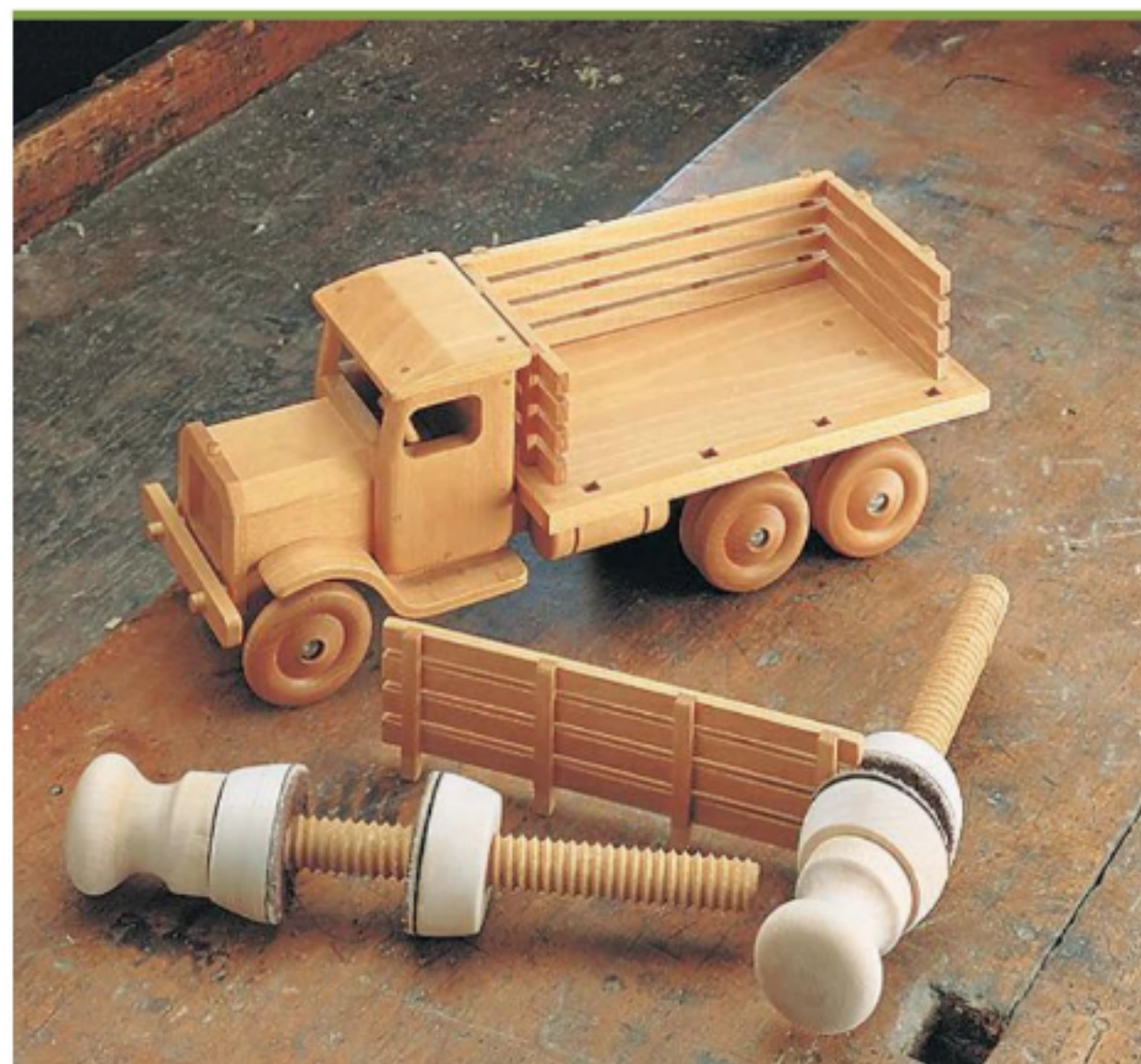
▲ Small-Piece Clamps. Cutting small wood threads are ideal for small, delicate work such as these micro clamps. Just thread a short dowel and then tap threads in the lower nut.
