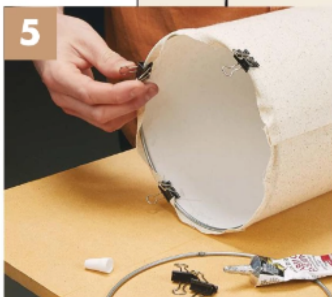
Ring to Styrene. Glue the rings to the ends of the shades. Binder clips hold the rings in place.
