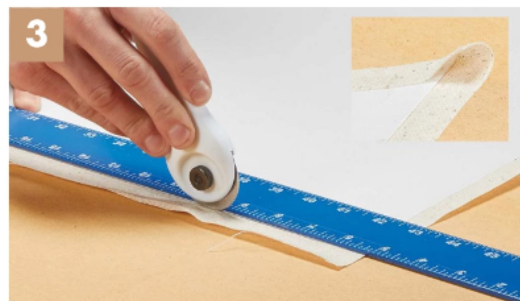
3 Final Trim. Three edges of the fabric are trimmed longer than the backing. The long edge is folded and glued to the styrene (inset).
