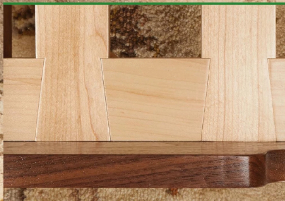
▲ The hardwood slats that support the mattress of the pet bed are dovetailed into the rails for a rigid connection.
