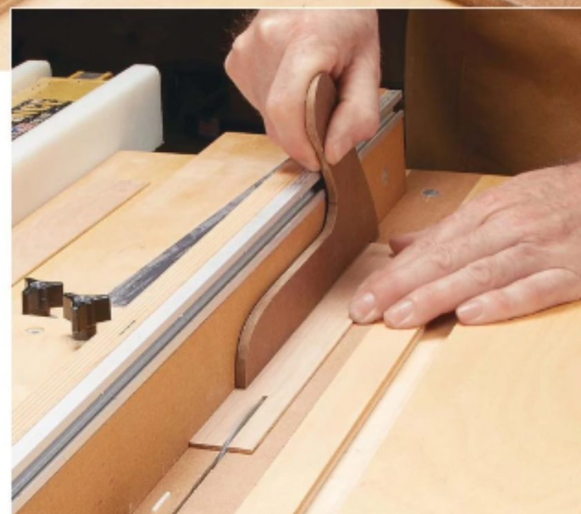
▲ Best. A cutting system like this ( ShopNotes Issue 105) scales your table saw down to a smaller size. It features accessories for all your table saw cutting tasks, like a sled for precision crosscutting and a micro-adjust fence for ripping (right).
