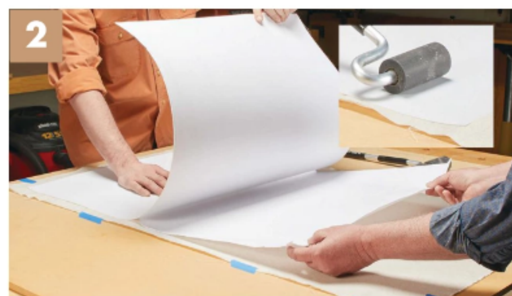
2 Attach the Styrene. With the help of a friend, peel the backing off the styrene. A J-roller (inset) does a good job of adhering the backing to the fabric.
