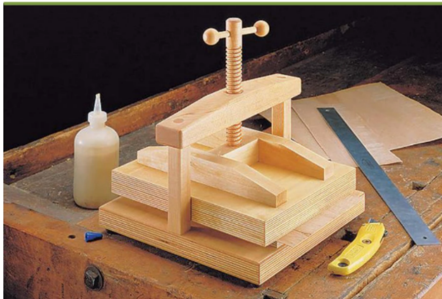
▲ Veneer Press. Tightening a single wood screw applies all the clamping pressure that's needed for this small veneer press. With different sets of threadboxes and taps, you can make the wood screw in various sizes.
