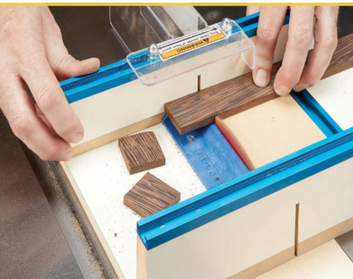
▲ Better. A commercially available small parts sled has handy features like a replaceable zero-clearance insert as well as T-track for accessories.
