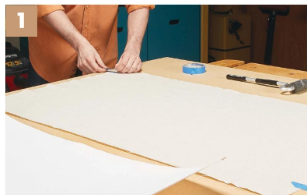
1 Rough Sizing. To start, iron the fabric and tape it in place. This is the time to ensure that any pattern in the fabric weave is aligned with the backing.
