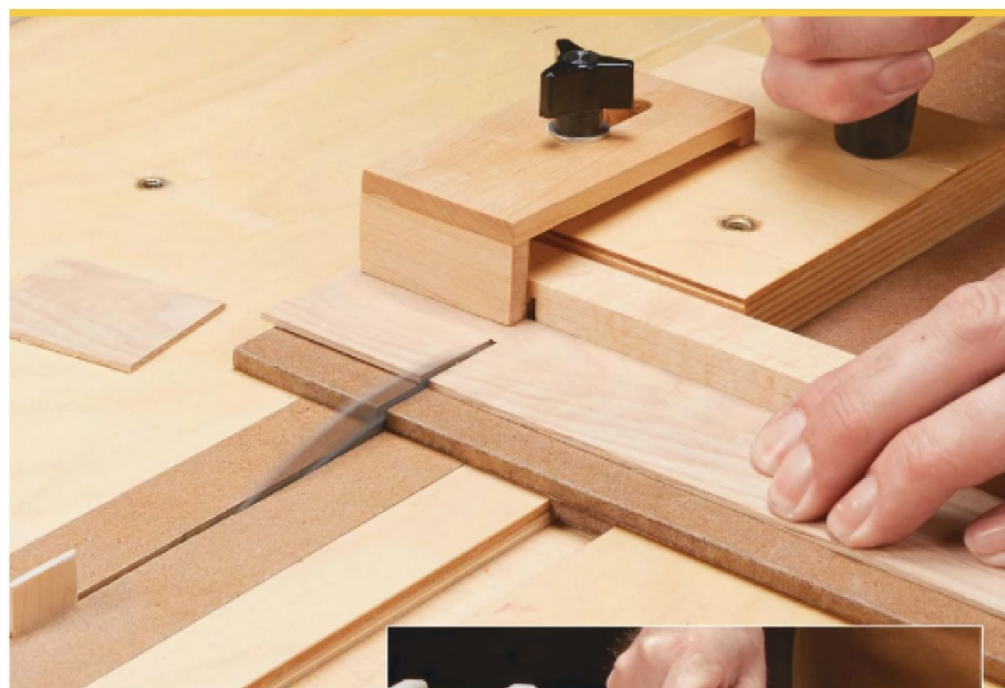
▲ Best. A cutting system like this ( ShopNotes Issue 105) scales your table saw down to a smaller size. It features accessories for all your table saw cutting tasks, like a sled for precision crosscutting and a micro-adjust fence for ripping (right).
