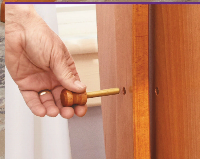
▲ Custom-made brass pins slip through the legs and into the ends to keep the cradle from rocking. The caps are turned on the drill press.
