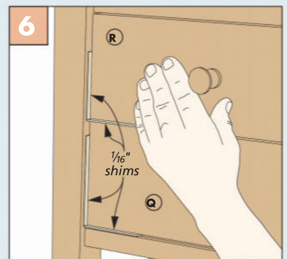
Fit the False Front. Use shims to ensure even spacing between the doors and in the opening.
