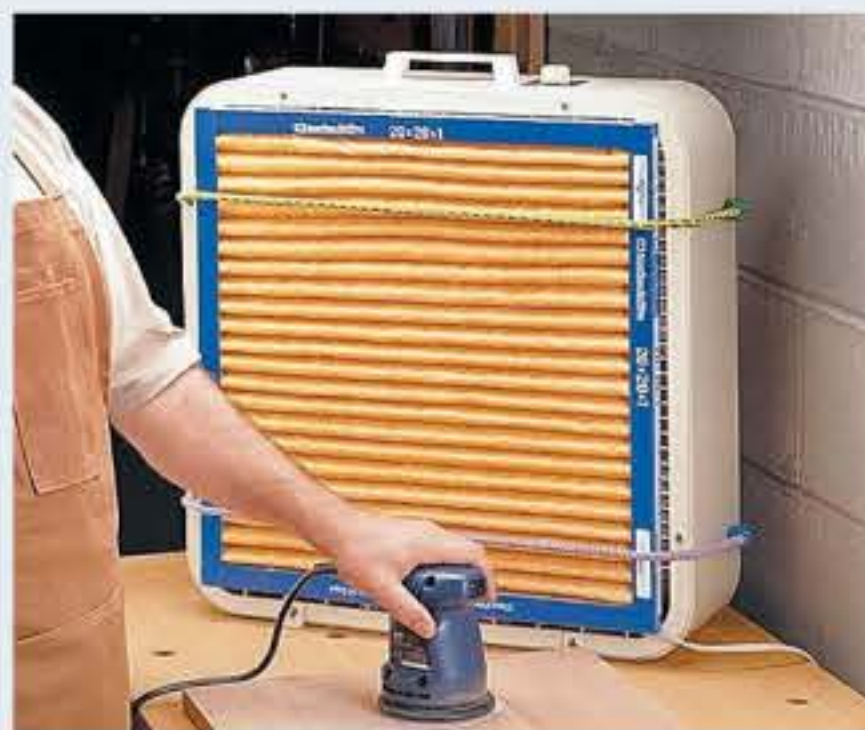
▲ This simple air filter can be made relatively inexpensively, yet works great for removing the dust from a small area.
