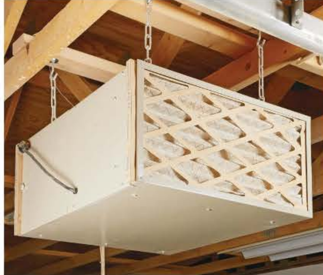
▲ Ceiling-mounted air filtration units (left photo) continuously circulate large volumes of air through the shop. Most come with a remote and timer for easy operation. You'll be surprised at just how much dust a filtration system captures in its filter (right photo).
