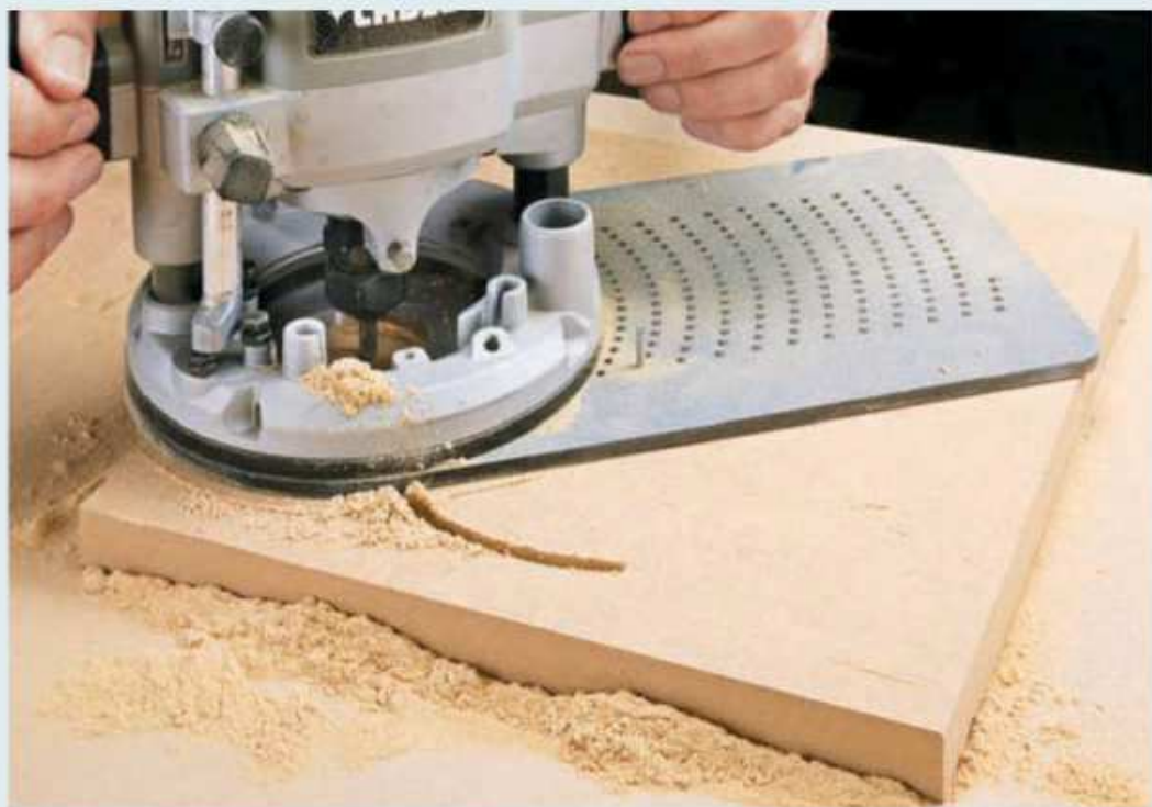
▲ Pre-made trammels (like this one from Jasper Tools ) are readily available. They fit various routers and accurately cut multiple circle diameters or arc radius.
