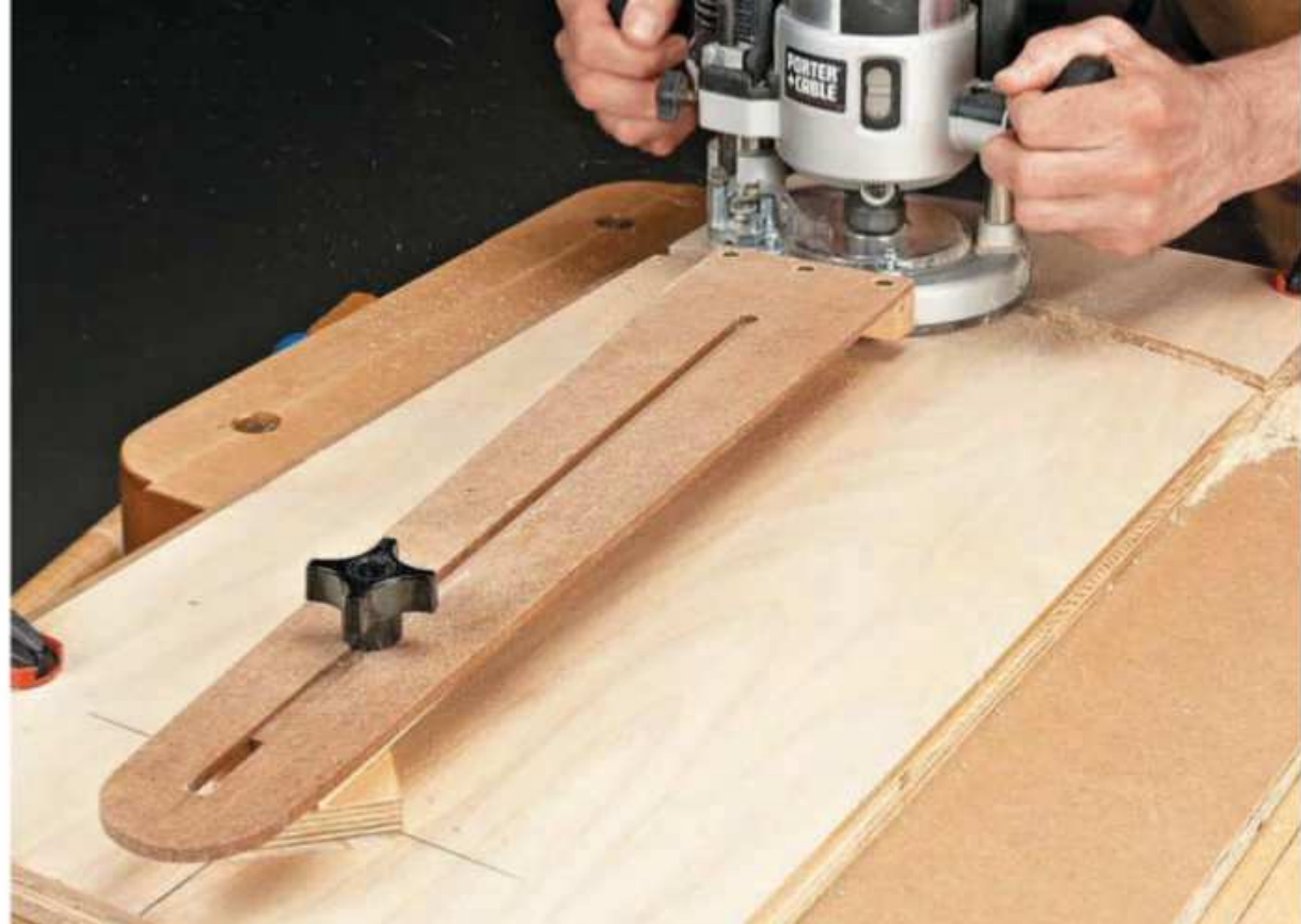
▲ Specially designed shop-made trammels may include features like adjustable pivot blocks (that are taped to the work surface) and router mounting hardware.
