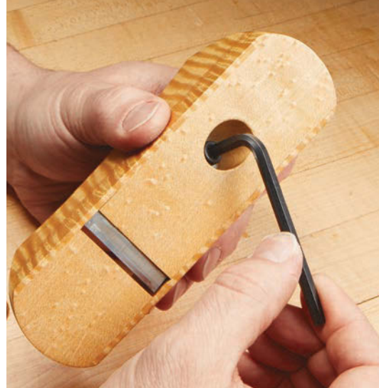
▲ The blade is held in place by tightening the socket head cap screw with an Allen wrench.
