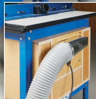
▲ The rear of the router table storage cabinet is equipped with a duct to attach to a dust collection system.
