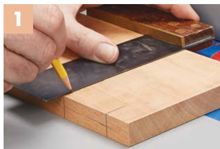
▲ Depending on where the groove is located, it may be necessary to transfer layout lines around a corner.
